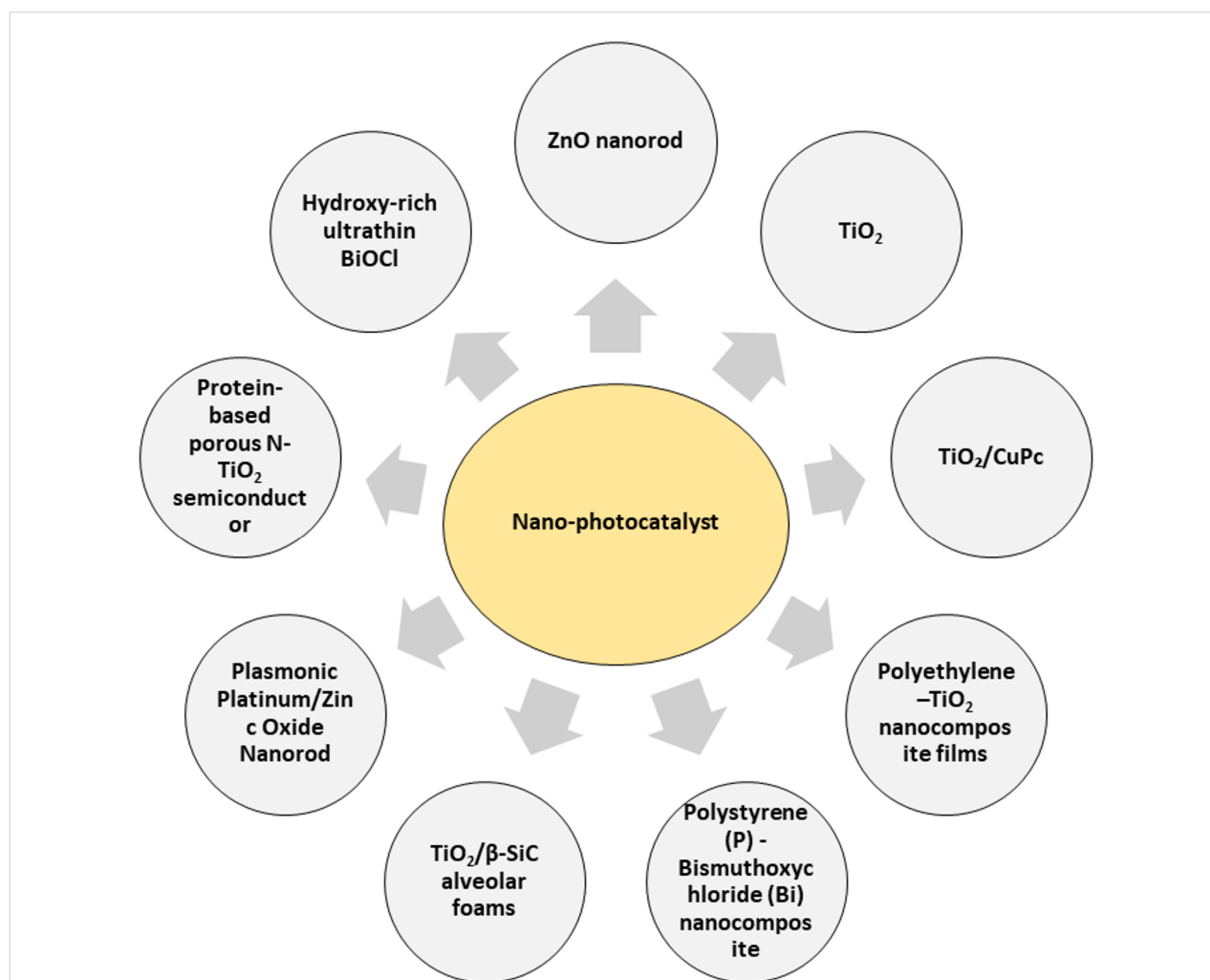
Figure 8: Different types of nano-photocatalysts used for the treatment of MPs.
