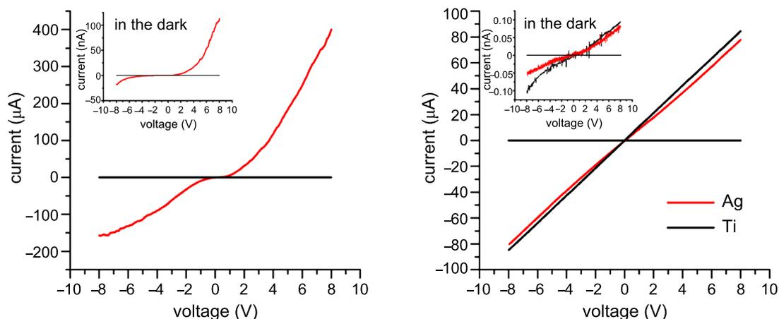
**Figure 3:**  $I$ – $V$  curves of ZnO nanowire films under UV illumination and in the dark. (a) The device in PDMS with Ag–PDMS paste electrodes; (b) two devices in air, with vacuum-deposited metal electrodes (Ti or Ag).
