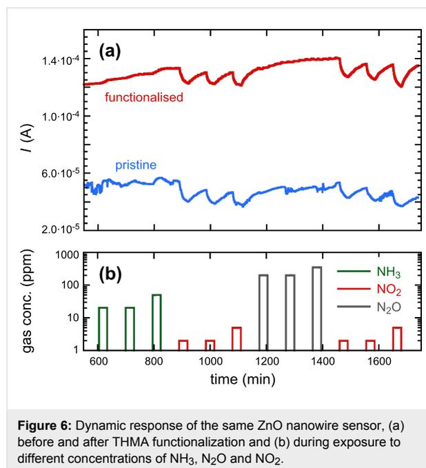
vidual sensor above the measurement range of our instrument (which corresponds to a minimum conductance value of  $G_{\max} = 10$  mS). We conclude from this that chemisorption of the thiol significantly increased the density of electrons present in the ZnO NW conduction band. We note that ZnO NW sensors modified by DT-functionalised or THMA-functionalised ZnO NPs showed a small increase in baseline conductivity, as can be seen in Table 1.
