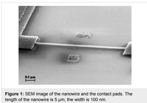
**Figure 1:** SEM image of the nanowire and the contact pads. The length of the nanowire is 5  $\mu\text{m}$ , the width is 100 nm.
