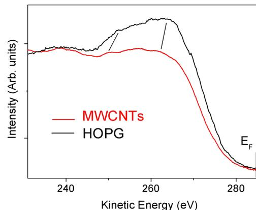
**Figure 4:** Core-valence-valence (CVV) Auger spectra of MWCNTs (red curve) and HOPG (black curve). An electron gun with a primary beam energy of 1500 eV was used as the exciting source. In the case of the MWCNT sample, the Auger peak is shifted towards lower kinetic energy with respect to HOPG. The Fermi level is at 284.4 eV.
