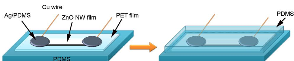
**Figure 6:** Illustration for the device fabrication process.
