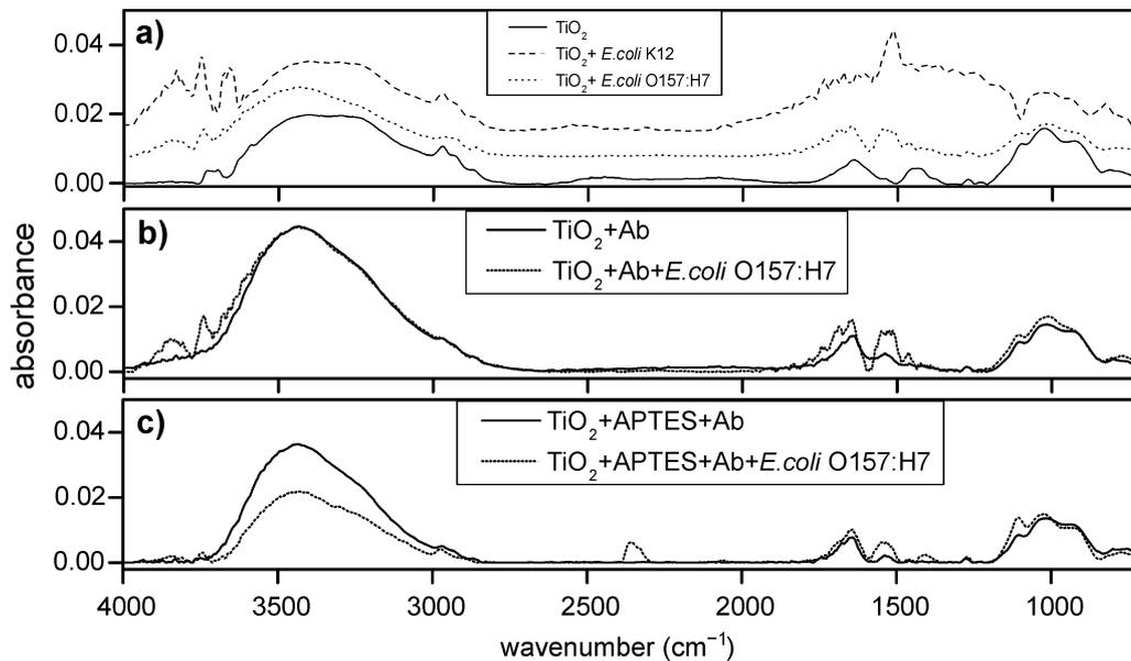
**Figure 5:** (a) FTIR spectrum of mesoporous titania films before (solid line) and after the immobilization of pathogens *E. coli* O157:H7 (dotted line) and *E. coli* K12 (dashed line). (b) FTIR spectrum of mesoporous titania films functionalized with anti-*E. coli* O157:H7-antibody (solid line) and after the immobilization of the pathogen (dotted line). (c) FTIR spectrum of titania films with APTES and antibody (solid line) and after the immobilization of *E. coli* (dotted line).
