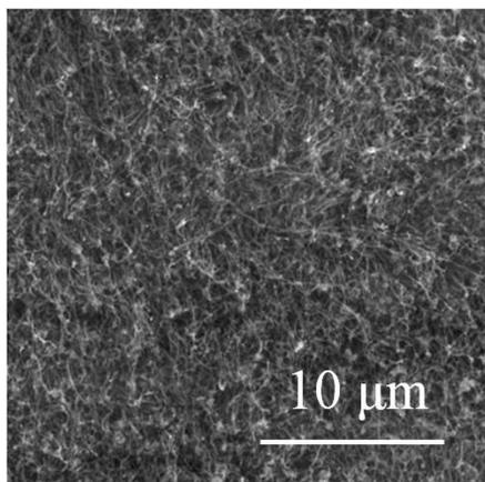
**Figure 2:** SEM image of the MWCNTs after growth on a stainless-steel substrate. The MWCNTs are randomly oriented, and no traces of other carbonaceous materials were detected in the large scanned area.
