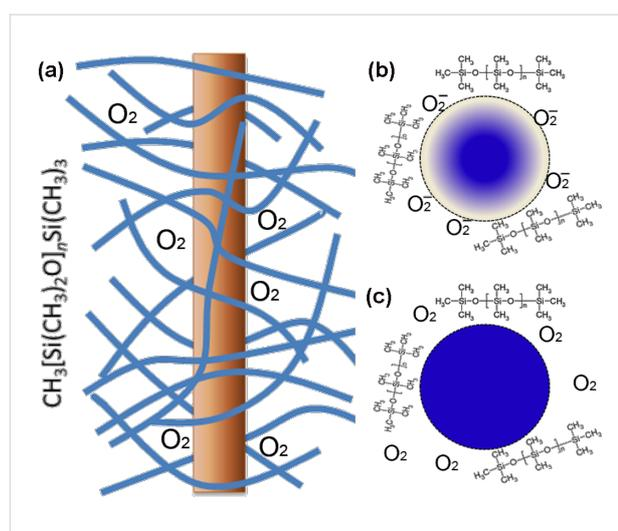
**Figure 5:** (a) Illustration of a ZnO nanowire in cross-linked PDMS. The blue lines represent PDMS molecule chains; (b) Illustration of a nanowire in PDMS without UV illumination, with oxygen adsorbed on parts of the surface. The colour gradient across the cross-section indicates a depletion layer near the surface; (c) Under UV illumination the oxygen molecules desorb from ZnO and diffuse into the molecule network.
