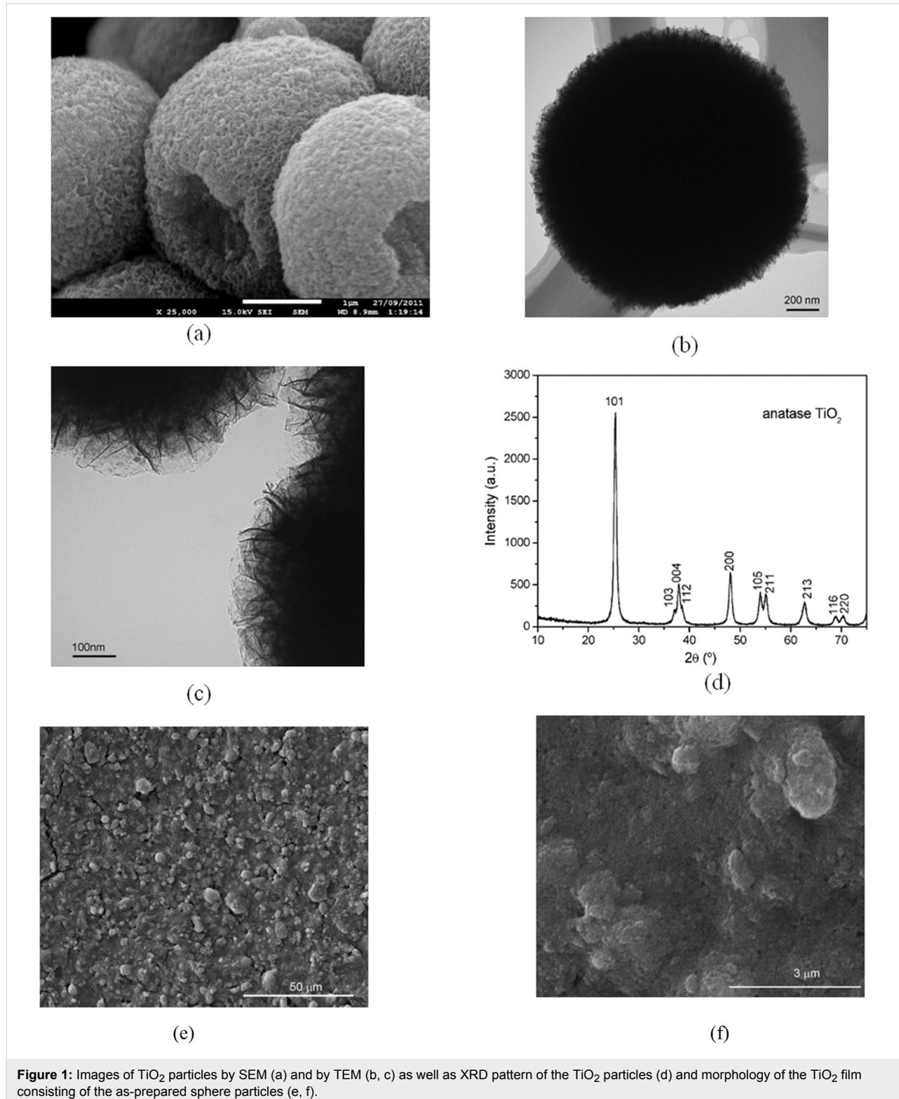
**Figure 1:** Images of TiO<sub>2</sub> particles by SEM (a) and by TEM (b, c) as well as XRD pattern of the TiO<sub>2</sub> particles (d) and morphology of the TiO<sub>2</sub> film consisting of the as-prepared sphere particles (e, f).
