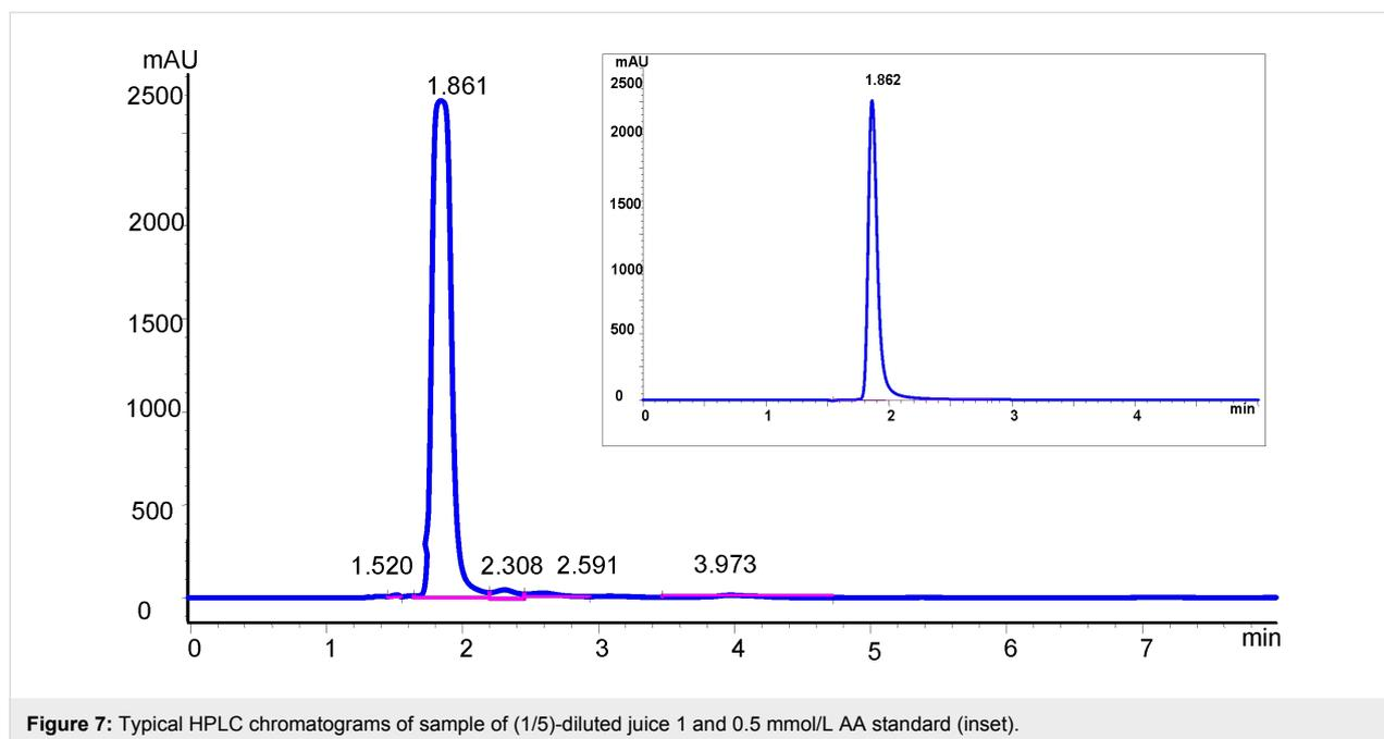
**Figure 7:** Typical HPLC chromatograms of sample of (1/5)-diluted juice 1 and 0.5 mmol/L AA standard (inset).
