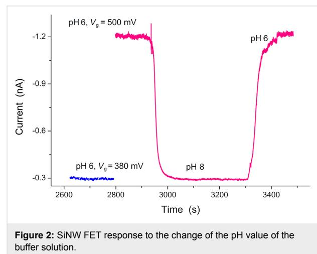
**Figure 2:** SiNW FET response to the change of the pH value of the buffer solution.
