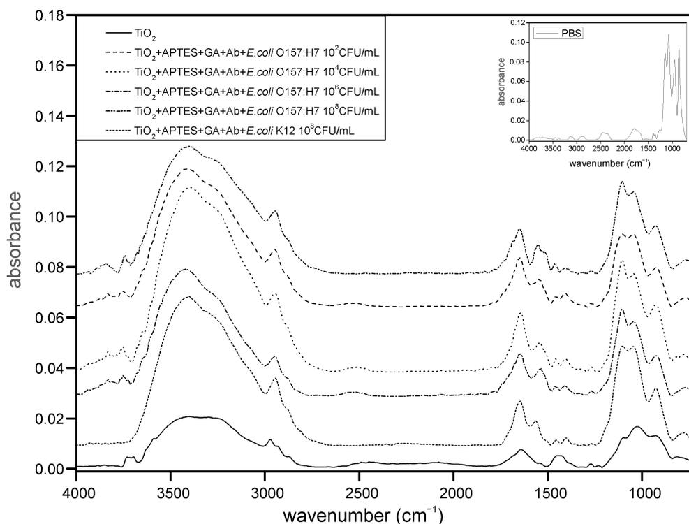
**Figure 8:** FTIR spectra of titania films alone (solid line) and functionalized with APTES–GA–anti-*E. coli* O157:H7–Ab after exposure to different concentrations of *E. coli* O157:H7 ( $10^8$ – $10^2$  CFU/mL) and *E. coli* K12 ( $10^9$  CFU/mL) in order from the top to the bottom. The negative control of PBS is reported in the inset.
