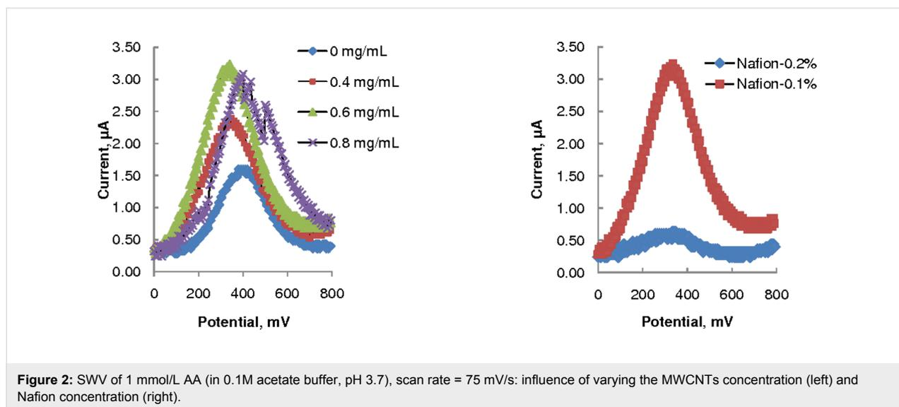
**Figure 2:** SWV of 1 mmol/L AA (in 0.1M acetate buffer, pH 3.7), scan rate = 75 mV/s: influence of varying the MWCNTs concentration (left) and Nafion concentration (right).
