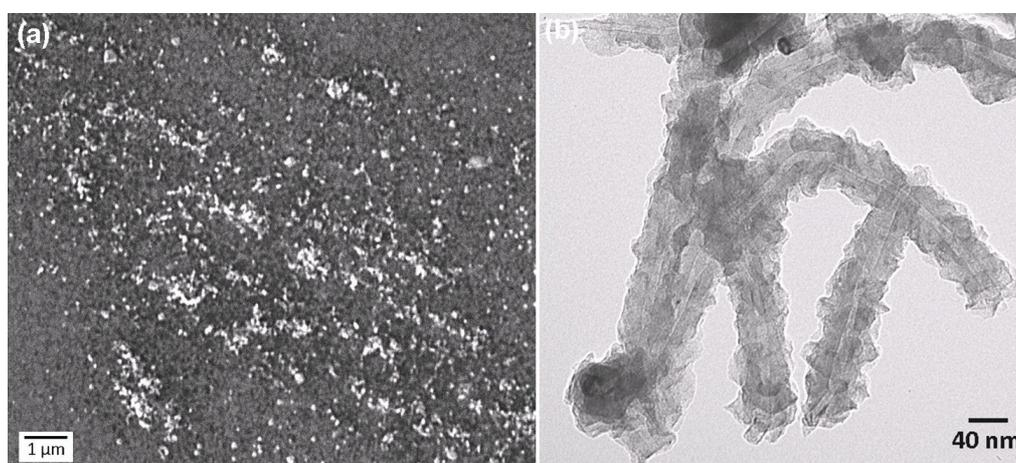
**Figure 3:** (a) SEM image showing the surface of Sample C, on which a low density mat of MWCNTs is grown after CVD at 500 °C for 30 min. (b) TEM image of CNTs from Sample B (grown in CVD for 30 min at 525 °C).
