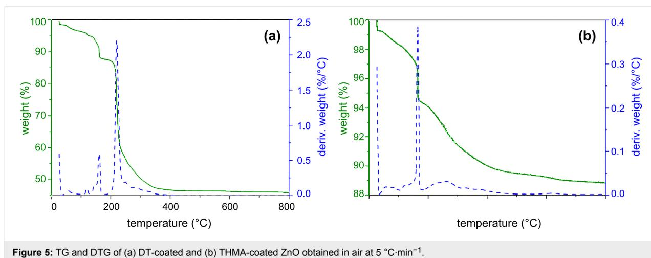
rather than single-crystal form and therefore a range of different ZnO crystal surfaces were exposed rather than a single surface, but more importantly, the fact that the XPS study was performed in ultrahigh vacuum rather than in dry air. Taking the TG results into account, a sensor operating temperature of 190 °C was chosen for all gas-response tests.
