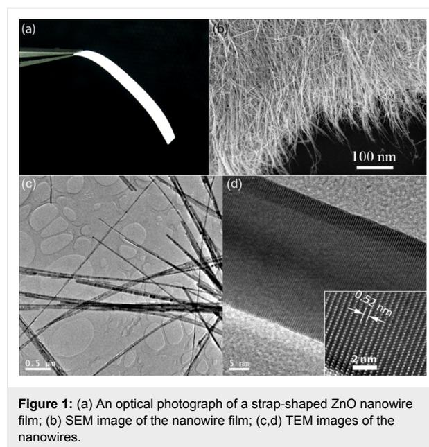
**Figure 1:** (a) An optical photograph of a strap-shaped ZnO nanowire film; (b) SEM image of the nanowire film; (c,d) TEM images of the nanowires.
