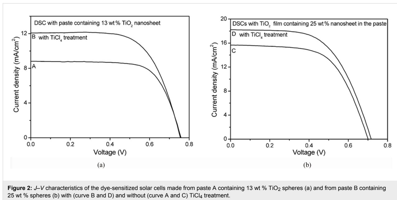
**Figure 2:** *J*–*V* characteristics of the dye-sensitized solar cells made from paste A containing 13 wt % TiO<sub>2</sub> spheres (a) and from paste B containing 25 wt % spheres (b) with (curve B and D) and without (curve A and C) TiCl<sub>4</sub> treatment.
