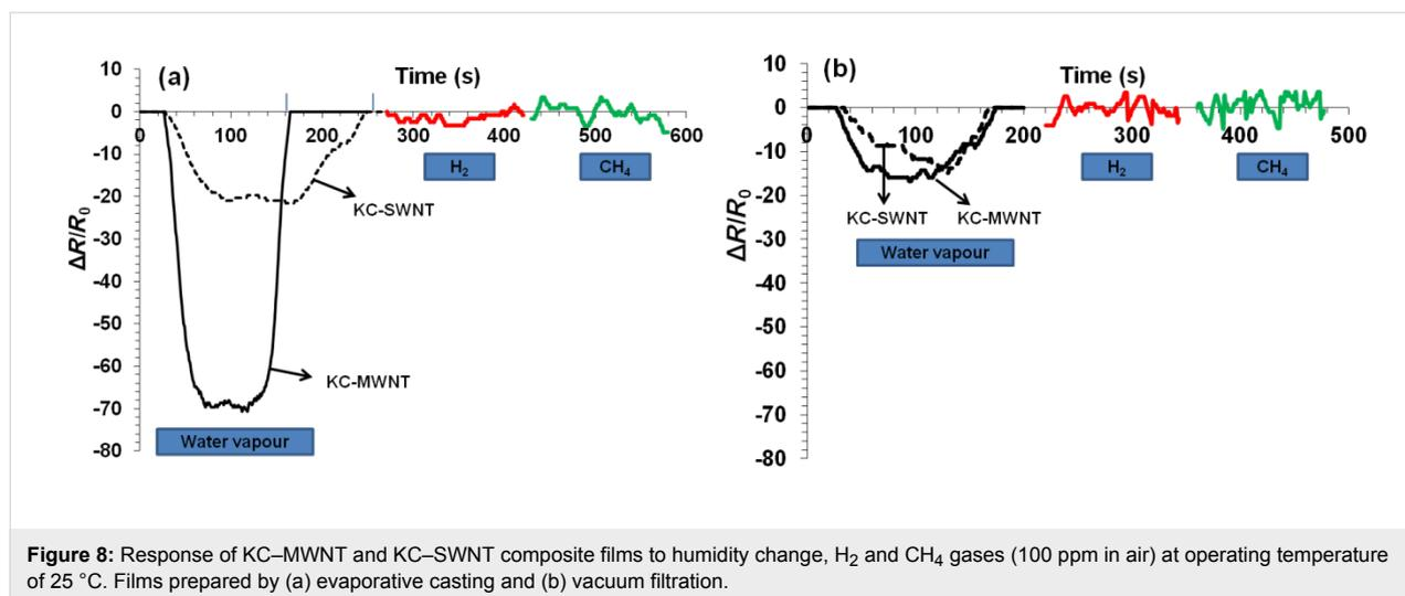
**Figure 8:** Response of KC–MWNT and KC–SWNT composite films to humidity change,  $H_2$  and  $CH_4$  gases (100 ppm in air) at operating temperature of 25 °C. Films prepared by (a) evaporative casting and (b) vacuum filtration.
