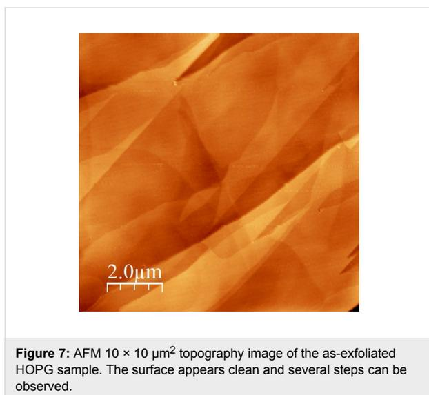
**Figure 7:** AFM  $10 \times 10 \mu\text{m}^2$  topography image of the as-exfoliated HOPG sample. The surface appears clean and several steps can be observed.
