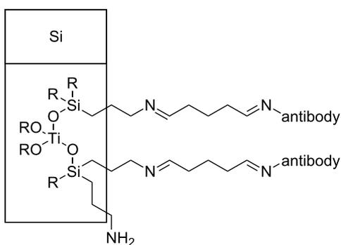
**Figure 4:** Structure of the chemical linking,  $\text{TiO}_2$ –APTES–GA–antibody.
