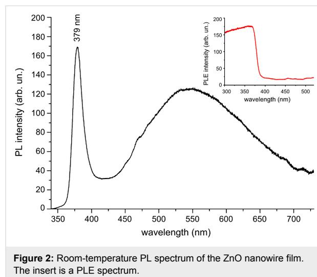
**Figure 2:** Room-temperature PL spectrum of the ZnO nanowire film. The insert is a PLE spectrum.
