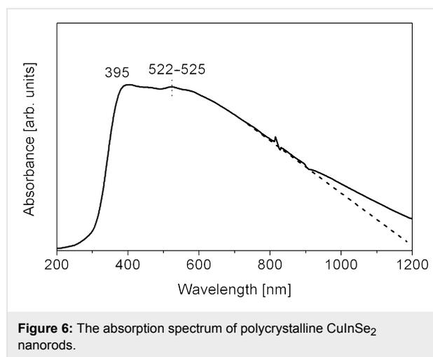
**Figure 6:** The absorption spectrum of polycrystalline CuInSe<sub>2</sub> nanorods.
