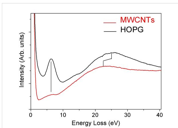
**Figure 5:** Energy-loss spectra of MWCNTs (red curve) and HOPG (black curve). In the case of MWCNTs, the  $\sigma+\pi$ -plasmon is shifted towards lower energy with respect to that of HOPG, located at about 26 eV, as indicated by the tick marker. The  $\pi$ -plasmon turns out to be sharp in HOPG (centred at 6.5 eV), whereas it is broader in MWCNTs.
