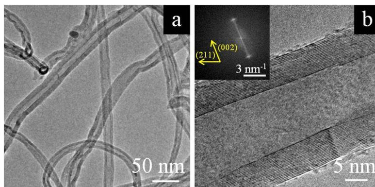
**Figure 3:** (a) Low-resolution TEM image assessing the multiwalled nature of the carbon nanotubes synthesized on SS. (b) High-resolution TEM picture of a single MWCNT with 19 walls. The inset displays the Fast Fourier Transform of the TEM image reported in (b). The two spots, at a semi-distance of 0.35 nm, represent the parallel walls.
