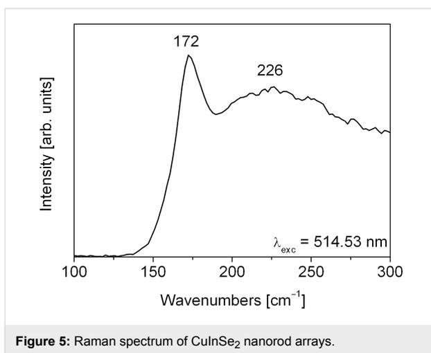
**Figure 5:** Raman spectrum of CuInSe<sub>2</sub> nanorod arrays.
