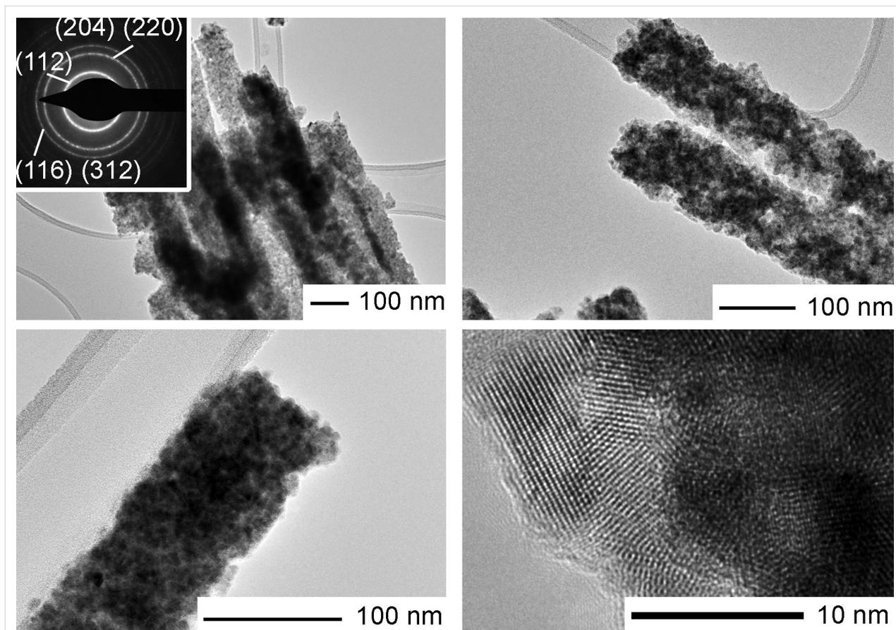
**Figure 4:** TEM images and SAED micrograph of polycrystalline CuInSe<sub>2</sub> nanorods.
