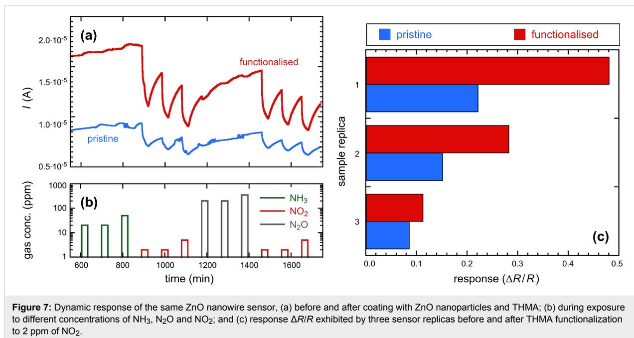
**Figure 7:** Dynamic response of the same ZnO nanowire sensor, (a) before and after coating with ZnO nanoparticles and THMA; (b) during exposure to different concentrations of NH<sub>3</sub>, N<sub>2</sub>O and NO<sub>2</sub>; and (c) response  $\Delta R/R$  exhibited by three sensor replicas before and after THMA functionalization to 2 ppm of NO<sub>2</sub>.
