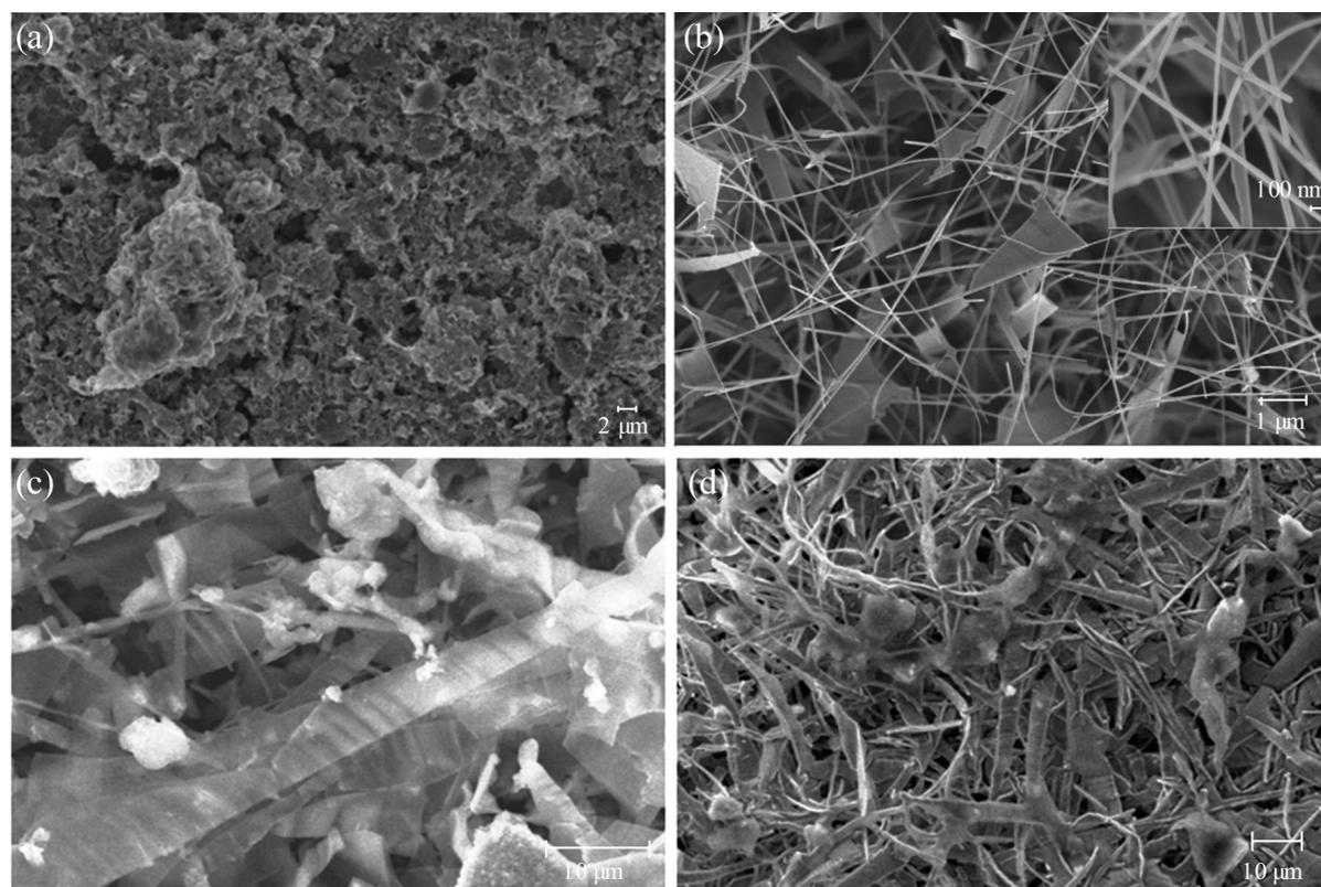
**Figure 1:** Scanning electron microscopy images of (a) the drop-cast ZnO nanoparticle sensor surface; (b) the pure ZnO nanowire sensor surface (inset: higher magnification FESEM image of ZnO NWs); (c) DT-ZnO NP + ZnO nanowire sensor surface; and (d) THMA-ZnO NP + ZnO nanowire sensor surface (note the change in scale).
