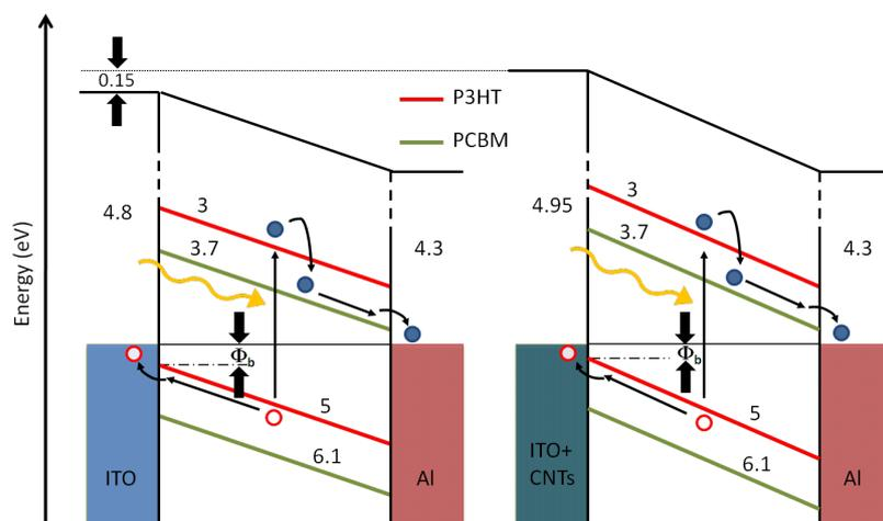
**Figure 4:** WF levels for cells with ITO (left) and ITO–CNT (right) electrode. (All reported values are in eV and negative).
