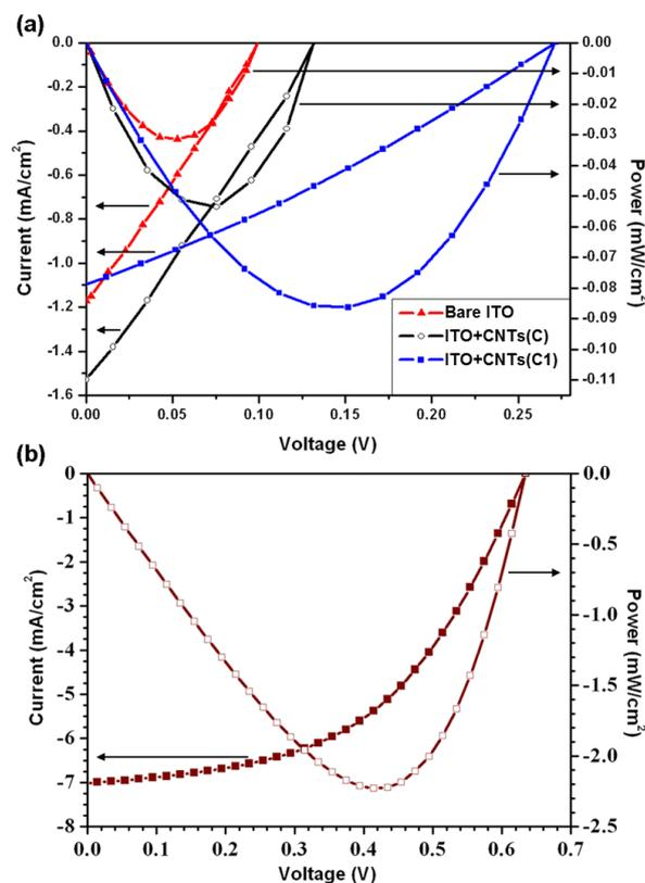
**Figure 5:** Current–voltage characteristic and output power of P3HT:PCBM solar cells: (a) Cell C and cell C1, compared to a reference cell made with bare ITO-coated glass; (b) classic ITO/PEDOT:PSS/P3HT:PCBM/Al cell manufactured in our labs.
