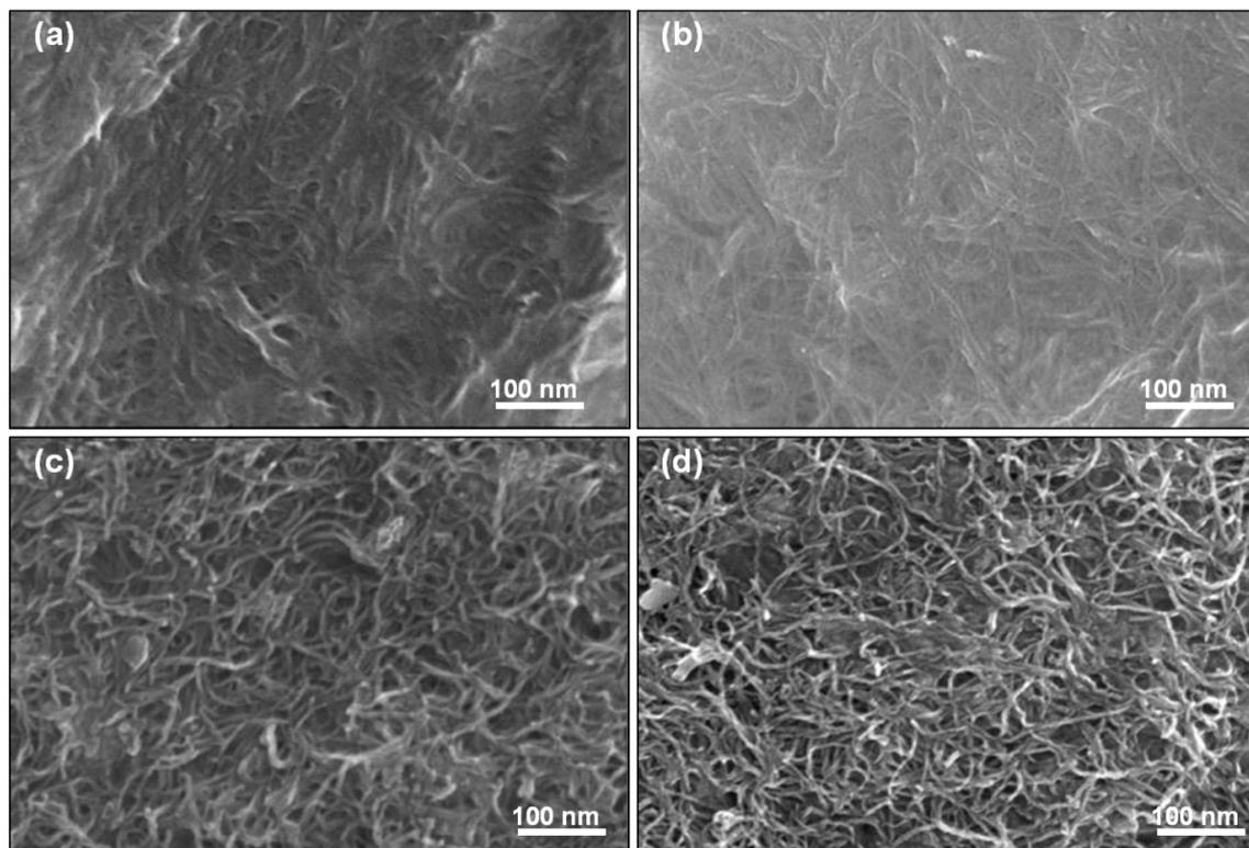
**Figure 6:** SEM image of (a) KC–CNT and (b) KC–CNT–G composite films prepared by the evaporative-casting method. (c) KC–CNT and (d) KC–CNT–G composite films prepared by the vacuum-filtration method. Contact angle values for (a–d) are  $64^\circ$ ,  $56^\circ$ ,  $77^\circ$  and  $72^\circ$ , respectively.
