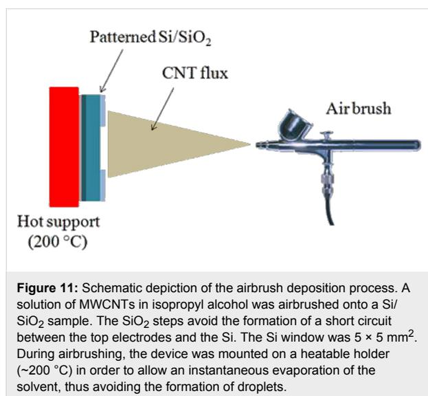
**Figure 11:** Schematic depiction of the airbrush deposition process. A solution of MWCNTs in isopropyl alcohol was airbrushed onto a Si/SiO<sub>2</sub> sample. The SiO<sub>2</sub> steps avoid the formation of a short circuit between the top electrodes and the Si. The Si window was 5 × 5 mm<sup>2</sup>. During airbrushing, the device was mounted on a heatable holder (~200 °C) in order to allow an instantaneous evaporation of the solvent, thus avoiding the formation of droplets.
