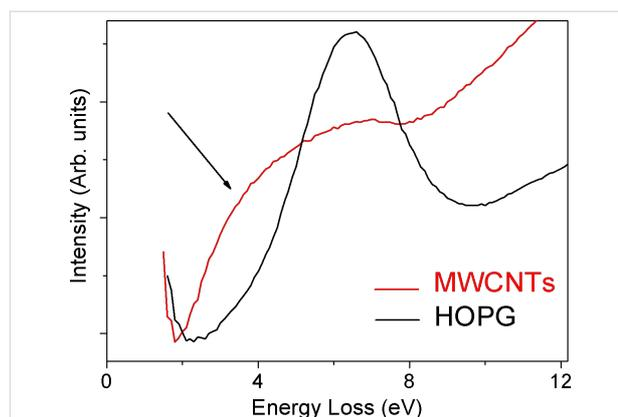
**Figure 6:** Comparison of the  $\pi$ -plasmon peak (0–12 eV) for MWCNTs (red curve) and HOPG (black curve). It is worth noting that in the case of MWCNTs we find electronic structures also at 2.0–4.5 eV, while in HOPG they are completely absent. These features contribute to the  $\pi$ -plasmon, giving rise to a very broad peak. Transitions between Van Hove singularities are thought to be responsible for these additional features.
