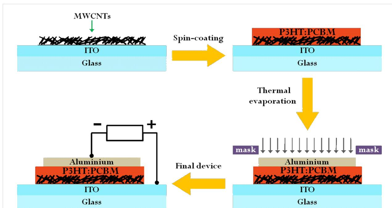
**Figure 7:** Schematics of the preparation of a P3HT:PCBM solar cell with CNT-enhanced ITO.
