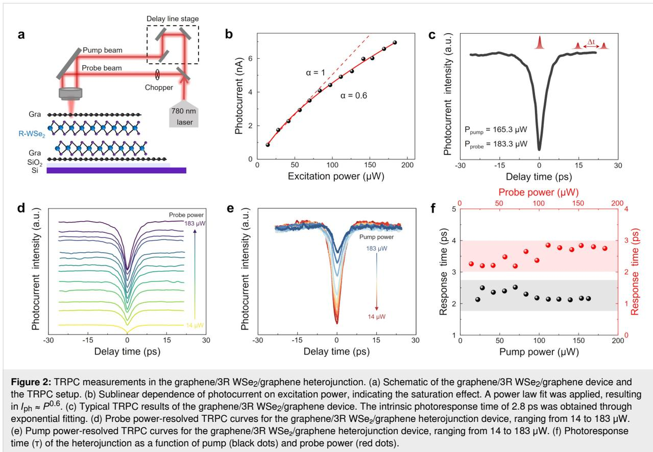
183  $\mu$ W (Figure 2d,e). Each TRPC curve has been individually fitted with an exponential function to obtain the intrinsic photoresponse time ( $\tau$ ), as summarized in Figure 2f. The response time ( $\tau$ ) of the device can be determined by fitting the time-resolved photocurrent signals with the following equation [40,41,43]:
