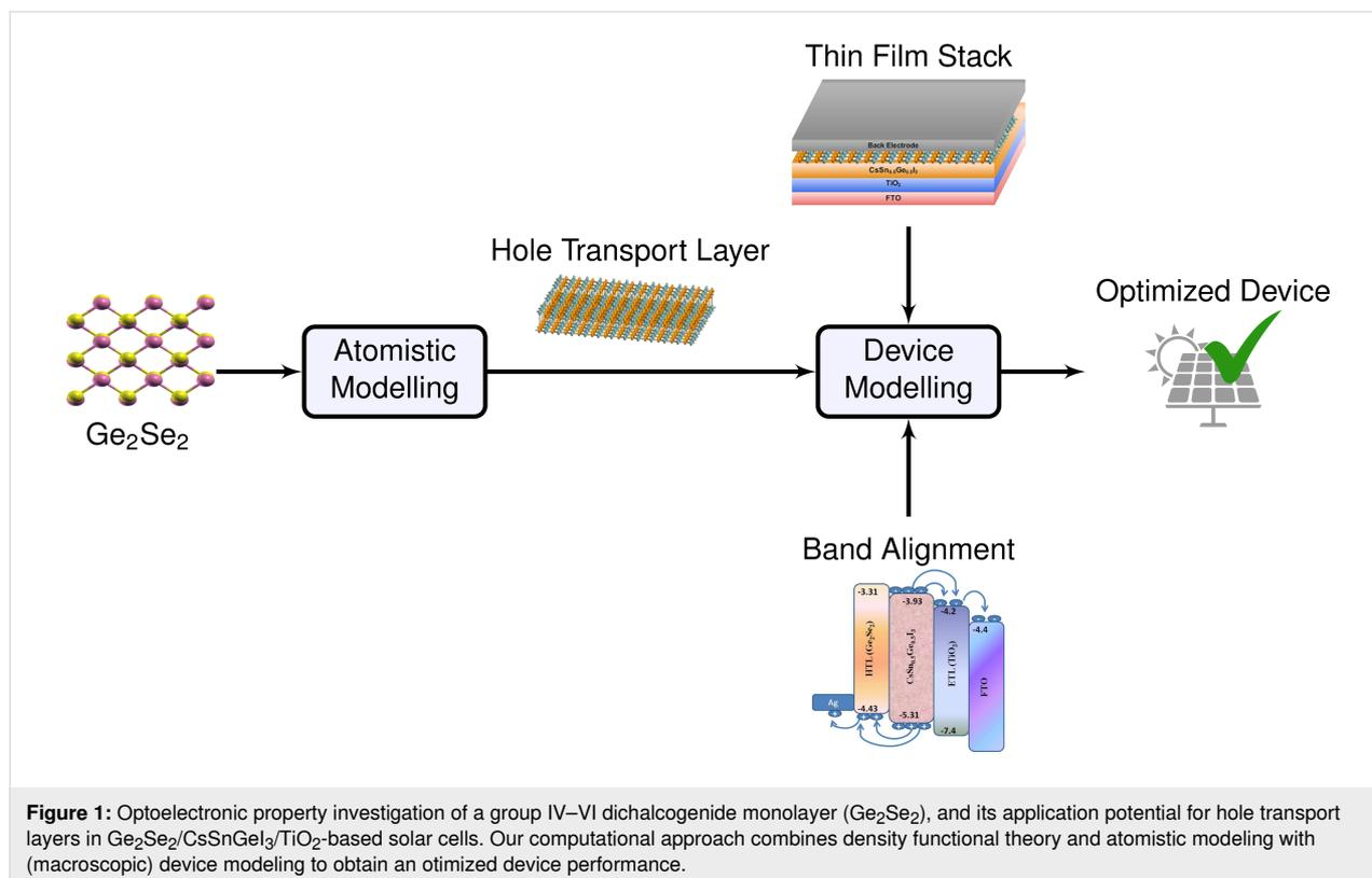
**Figure 1:** Optoelectronic property investigation of a group IV–VI dichalcogenide monolayer ( $\text{Ge}_2\text{Se}_2$ ), and its application potential for hole transport layers in  $\text{Ge}_2\text{Se}_2/\text{CsSnGeI}_3/\text{TiO}_2$ -based solar cells. Our computational approach combines density functional theory and atomistic modeling with (macroscopic) device modeling to obtain an optimized device performance.
