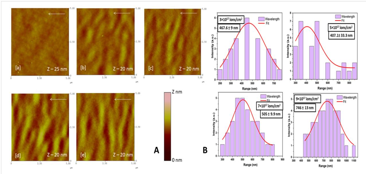
**Figure 1:** A. AFM images of pristine and 100 keV Ar<sup>+</sup> ion-irradiated Si samples. (a) Pristine and irradiated samples with (b)  $3 \times 10^{17}$ , (c)  $5 \times 10^{17}$ , (d)  $7 \times 10^{17}$ , and (e)  $9 \times 10^{17}$  ions/cm<sup>2</sup> (all images are in  $5 \mu\text{m} \times 5 \mu\text{m}$  scan size) with corresponding wavelength distribution shown in B.
