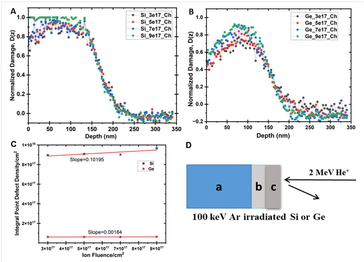
**Figure 5:** Damage fractions calculated for (A) Si and (B) Ge after irradiation (using the DICADA code). (C) Density of point defects with an increase in ion fluence. (D) Schematic representation of the analysis of amorphous (c) and amorphous/crystalline (b) zones with RBS-c.
