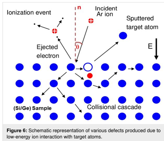
**Figure 6:** Schematic representation of various defects produced due to low-energy ion interaction with target atoms.
