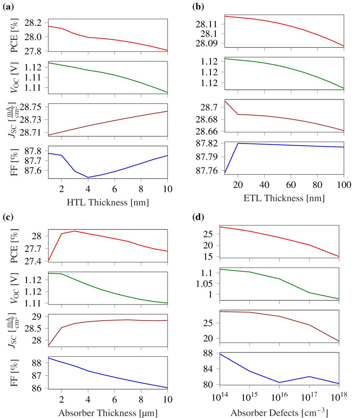
**Figure 7:** PSC performance parameters as functions of (a) HTL thickness, (b) ETL thickness, (c) absorber thickness, and (d) absorber defects. The device exhibits optimal performance at layer thicknesses of ETL, absorber, and HTL of 20 nm, 2  $\mu\text{m}$ , and 1 nm, respectively.
