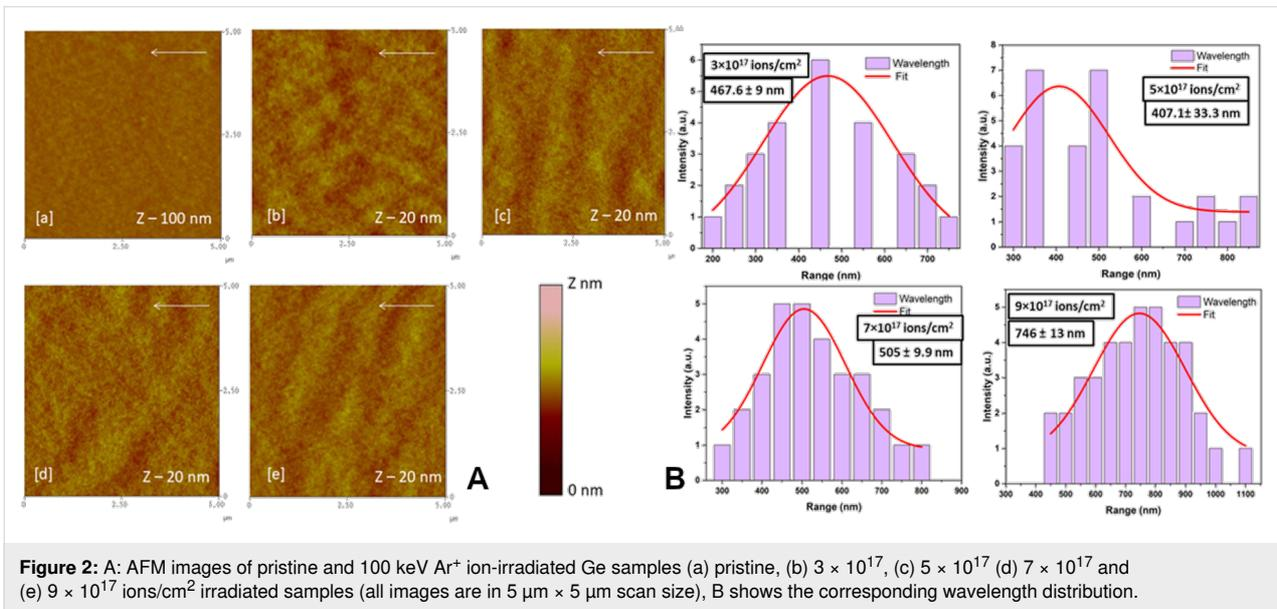
**Figure 2:** A. AFM images of pristine and 100 keV Ar<sup>+</sup> ion-irradiated Ge samples (a) pristine, (b)  $3 \times 10^{17}$ , (c)  $5 \times 10^{17}$  (d)  $7 \times 10^{17}$  and (e)  $9 \times 10^{17}$  ions/cm<sup>2</sup> irradiated samples (all images are in  $5 \mu\text{m} \times 5 \mu\text{m}$  scan size), B shows the corresponding wavelength distribution.
