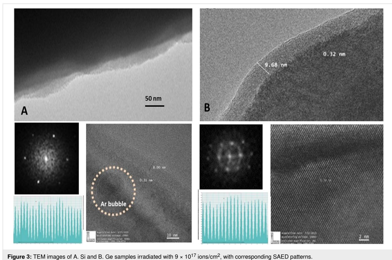
**Figure 3:** TEM images of A. Si and B. Ge samples irradiated with  $9 \times 10^{17}$  ions/cm<sup>2</sup>, with corresponding SAED patterns.
