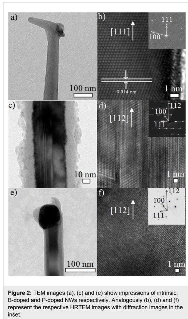
**Figure 2:** TEM images (a), (c) and (e) show impressions of intrinsic, B-doped and P-doped NWs respectively. Analogously (b), (d) and (f) represent the respective HRTEM images with diffraction images in the inset.
