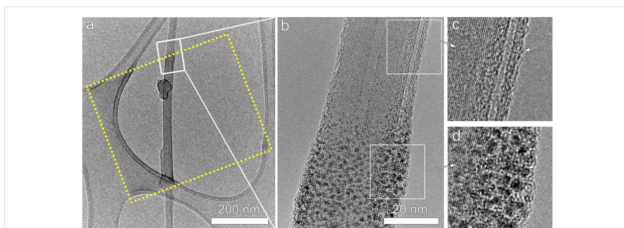
**Figure 3:** (a) TEM image of Pt nanoclusters deposited by FEBID on a CNT shows that site specific deposition has been achieved. The area indicated by the dotted lines is the predefined area during the deposition process. (b) Shows an enlargement of the rectangular dotted area in (a). The CNT structure has been preserved well during the deposition, as shown by HRTEM images (c–d).
