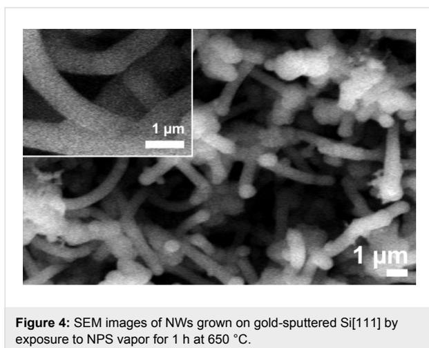
**Figure 4:** SEM images of NWs grown on gold-sputtered Si[111] by exposure to NPS vapor for 1 h at 650 °C.
