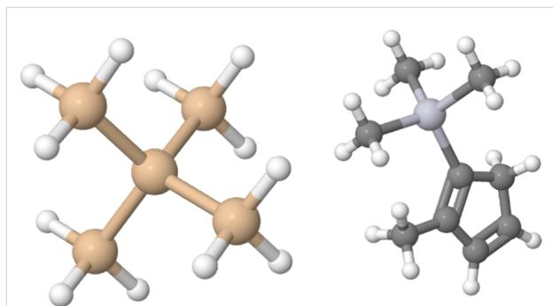
**Figure 5:** Molecular models of Si<sub>5</sub>H<sub>12</sub> (left) and Me<sub>3</sub>Pt(IV)CpMe (right). Rendered using Jmol.
