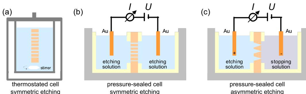
**Figure 4:** Schematic of etching equipment. Symmetric etching conditions leading to cylindrical channels in (a) thermostated cell and (b) pressure-sealed cell. (c) Asymmetric conditions leading to conical channels in pressure-sealed cell. Electric current measurements allow monitoring of the etching process.
