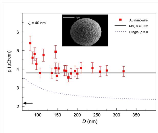
**Figure 16:** Specific electrical resistivity versus wire diameter for single polycrystalline gold nanowires (ammonium gold(I) sulfite electrolyte,  $T = 50\text{ }^{\circ}\text{C}$ ,  $U = -0.8\text{ V}$ ) together with the cap morphology. The symbols represent the data. The continuous and dashed lines are a fit of the resistivity predicted by the Mayadas and Shatzkes and the Dingle models, respectively. Adapted with permission from [135] – Copyright 2008 Elsevier B.V.
