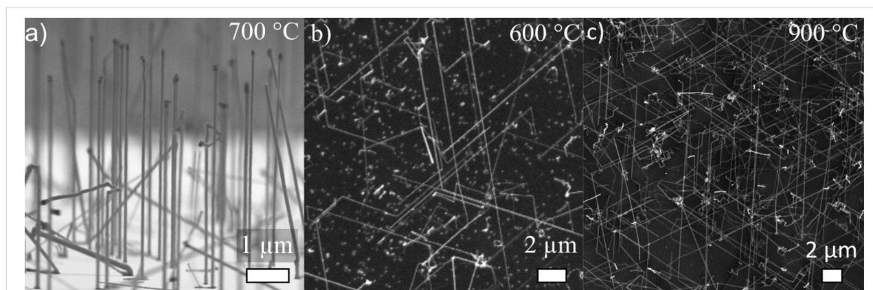
**Figure 1:** (a) tilted-view SEM image of Au-catalysed NWs grown at 700 °C with OCTS, (b) top-view SEM image of boron-doped Si-NWs grown at 600 °C, (c) SEM image of phosphorus-doped NWs grown at 900 °C.
