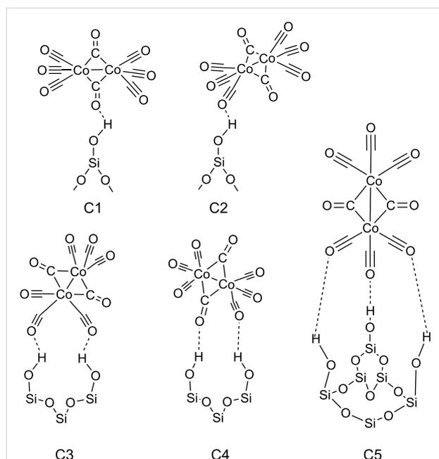
**Figure 6:** Schematic representation of the starting configurations with possible  $\text{Co}_2(\text{CO})_8$  orientations, considered in this study, on FOH- $\text{SiO}_2$  surfaces. In POH- $\text{SiO}_2$  surfaces some of the OH groups are partially removed in order to simulate the pretreated surfaces.
