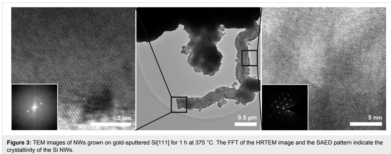
**Figure 3:** TEM images of NWs grown on gold-sputtered Si[111] for 1 h at 375 °C. The FFT of the HRTEM image and the SAED pattern indicate the crystallinity of the Si NWs.
