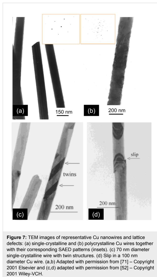
**Figure 7:** TEM images of representative Cu nanowires and lattice defects: (a) single-crystalline and (b) polycrystalline Cu wires together with their corresponding SAED patterns (insets). (c) 70 nm diameter single-crystalline wire with twin structures. (d) Slip in a 100 nm diameter Cu wire. (a,b) Adapted with permission from [71] – Copyright 2001 Elsevier and (c,d) adapted with permission from [52] – Copyright 2001 Wiley-VCH.
