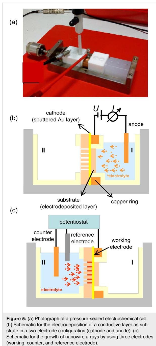
**Figure 5:** (a) Photograph of a pressure-sealed electrochemical cell. (b) Schematic for the electrodeposition of a conductive layer as substrate in a two-electrode configuration (cathode and anode). (c) Schematic for the growth of nanowire arrays by using three electrodes (working, counter, and reference electrode).
