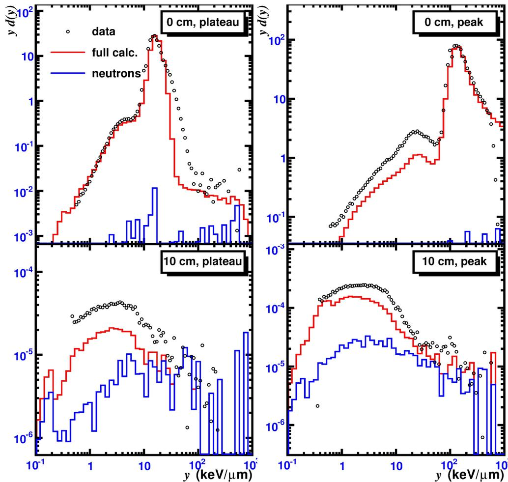
**Figure 5:** Microdosimetric spectra in a water phantom irradiated by 300 A MeV  $^{12}\text{C}$  nuclei. Upper (red) histograms are the total spectra calculated with MCHIT, the lower (blue) histograms show the neutron contributions. Data points from [6].
