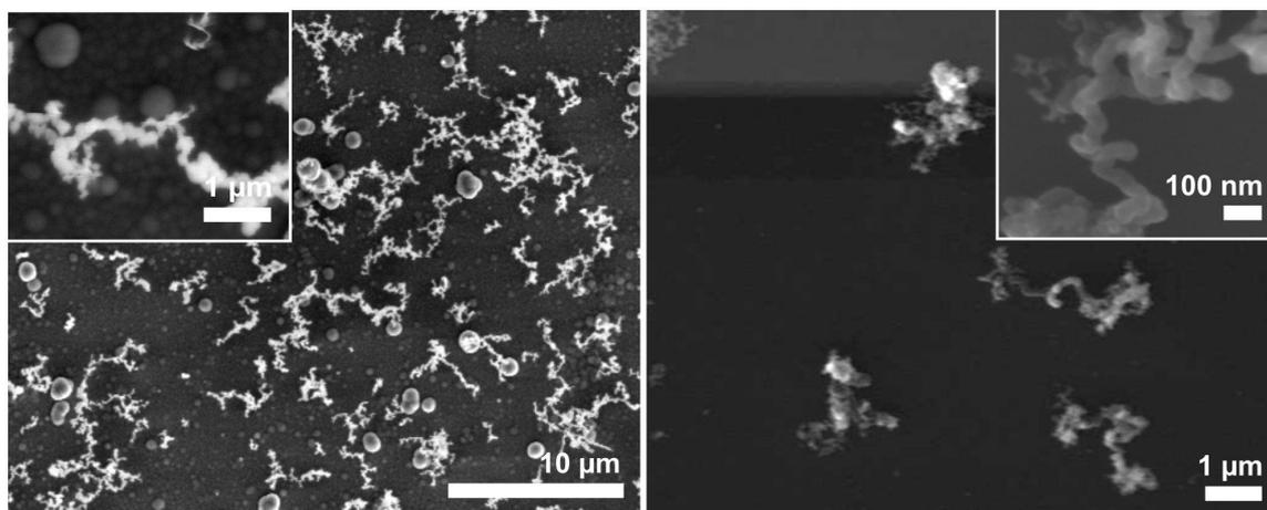
**Figure 9:** SEM image of NWs grown from nanoparticles at 650 °C without prior treatment (left) and at 375 °C after H<sub>2</sub>-plasma treatment for 40 min (right). Observe that at the lower temperature no round Si particles could be found on the sample.
