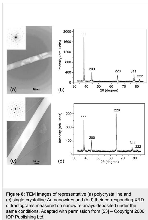
**Figure 8:** TEM images of representative (a) polycrystalline and (c) single-crystalline Au nanowires and (b,d) their corresponding XRD diffractograms measured on nanowire arrays deposited under the same conditions. Adapted with permission from [53] – Copyright 2006 IOP Publishing Ltd.
