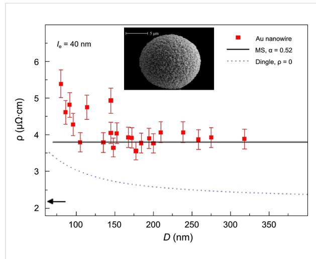
**Figure 16:** Specific electrical resistivity versus wire diameter for single polycrystalline gold nanowires (ammonium gold(I) sulfite electrolyte,  $T = 50\text{ }^\circ\text{C}$ ,  $U = -0.8\text{ V}$ ) together with the cap morphology. The symbols represent the data. The continuous and dashed lines are a fit of the resistivity predicted by the Mayadas and Shatzkes and the Dingle models, respectively. Adapted with permission from [135] – Copyright 2008 Elsevier B.V.
