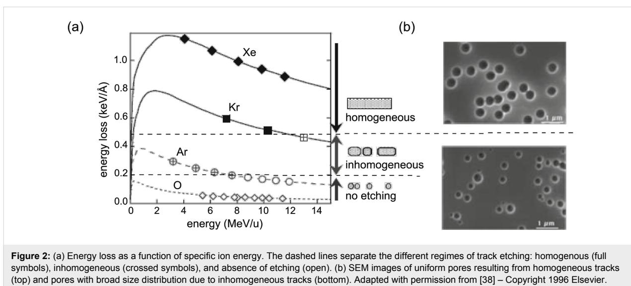
**Figure 2:** (a) Energy loss as a function of specific ion energy. The dashed lines separate the different regimes of track etching: homogenous (full symbols), inhomogeneous (crossed symbols), and absence of etching (open). (b) SEM images of uniform pores resulting from homogeneous tracks (top) and pores with broad size distribution due to inhomogeneous tracks (bottom). Adapted with permission from [38] – Copyright 1996 Elsevier.
