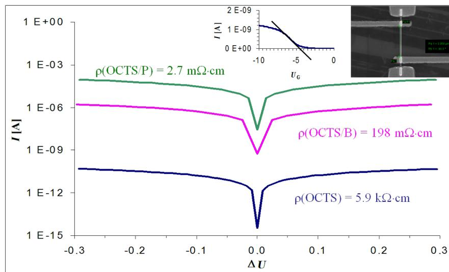
**Figure 3:** Semilogarithmic  $I/V$  plot of intrinsic, p- and n-type NWs. The calculated specific resistivity values are shown next to the respective curves. The transfer characteristic of the intrinsic NW integrated into a back-gated Schottky-barrier NW-FET and a SEM image of a four-point setup is shown in the inset.
