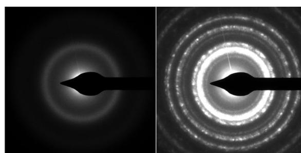
**Figure 9:** TEM electron diffraction pattern of samples on carbon membrane before (left) and after (right) postgrowth electron irradiation. The phase transformation from an amorphous to a crystalline state of the Co–Pt grains is apparent. See text for details. Images reproduced from Porra et al. [33].
