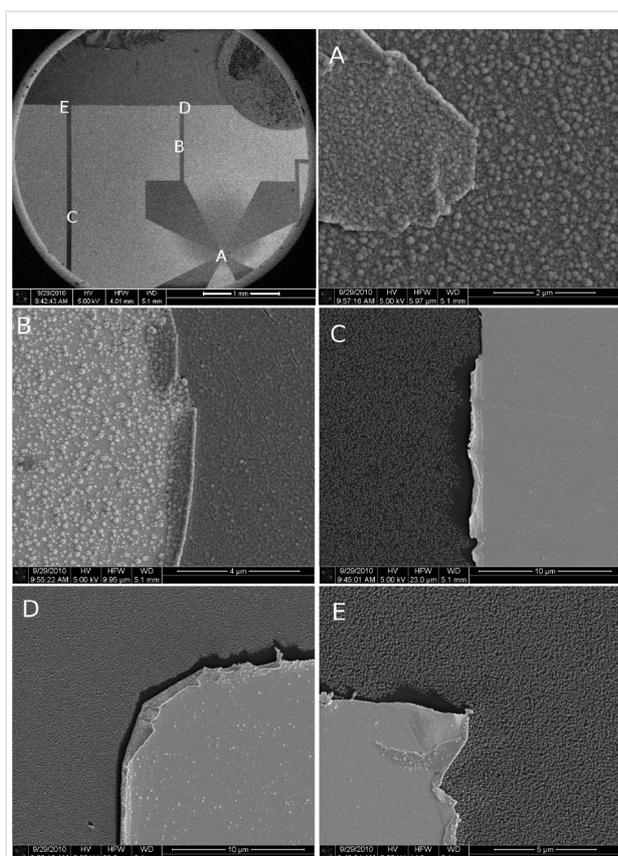
**Figure 2:** SEM images of Co deposited on the plasma-pretreated silicon oxide and gold. The picture on the top left is an overview of a SiO<sub>2</sub> surface prepatterned with Cr/Au contact structures. The labeling A–E indicates regions of different precursor flux, which was centered at A. The gas injection capillary is visible on the upper right. Gold surfaces appear as bright regions, SiO<sub>2</sub> surfaces as dark regions. Selected area SEM images are represented in images A–E.
