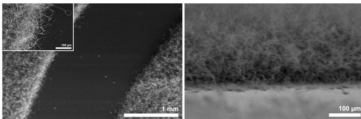
**Figure 14:** SEM image of the border region of a Si NW pattern obtained from UV-patterned “liquid bright gold” films after annealing at 650 °C, followed by treatment with NPS at 650 °C. Left: Top view, right: Side view.
