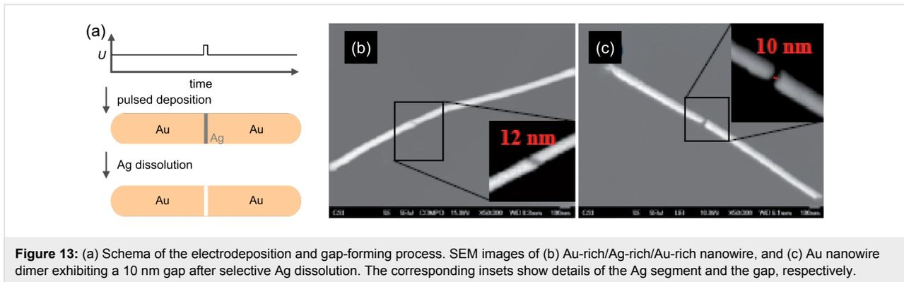
**Figure 13:** (a) Schema of the electrodeposition and gap-forming process. SEM images of (b) Au-rich/Ag-rich/Au-rich nanowire, and (c) Au nanowire dimer exhibiting a 10 nm gap after selective Ag dissolution. The corresponding insets show details of the Ag segment and the gap, respectively.
