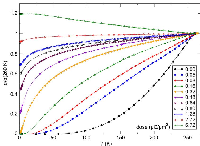
**Figure 13:** Temperature-dependent conductivity of Pt–C FEBID structures that have been exposed to different post-growth electron irradiation doses as indicated. See text for details. Adapted from [52].
