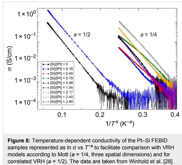
**Figure 8:** Temperature-dependent conductivity of the Pt-Si FEBID samples represented as  $\ln \sigma$  vs  $T^{-a}$  to facilitate comparison with VRH models according to Mott ( $a = 1/4$ , three spatial dimensions) and for correlated VRH ( $a = 1/2$ ). The data are taken from Winhold et al. [28].
