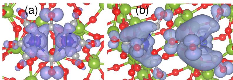
**Figure 8:** Band decomposed charge density for the valence band maximum for  $\text{Co}_2(\text{CO})_8$  on the (a) FOH-SiO<sub>2</sub> and (b) POH-SiO<sub>2</sub> surfaces.
