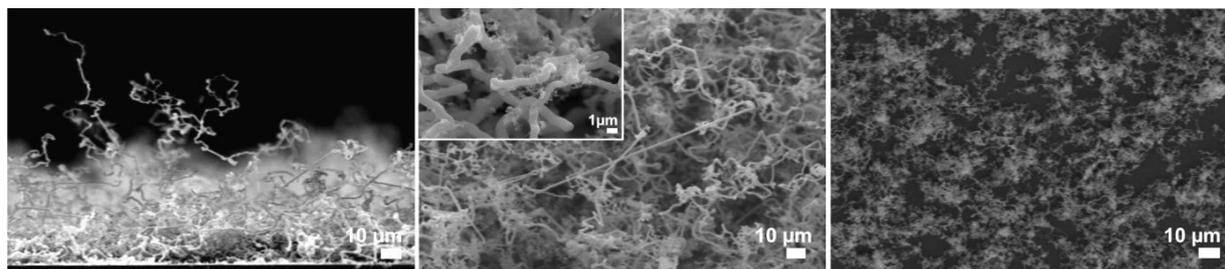
**Figure 1:** SEM images of NWs grown on gold-sputtered Si[111] exposed to NPS vapor at 375 °C for 1 h (left: side view; center: top view) and 30 min (right: top view). In the insert of the center view, the smaller, branching structures on the NWs become visible.
