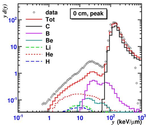
**Figure 6:** Contribution of various fragments to the microdosimetry spectra measured on the beam axis in the Bragg peak region in a water phantom irradiated by 300 A MeV  $^{12}\text{C}$  nuclei. Histograms represent MCHIT calculations. Data points from [6].
