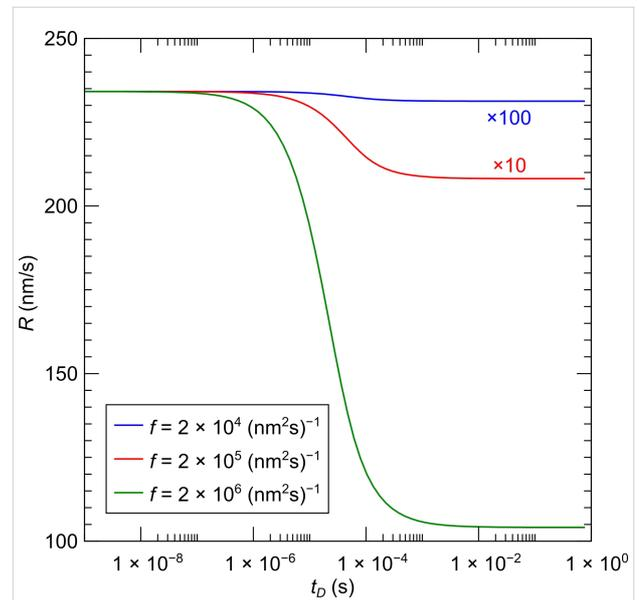
**Figure 2:** Single-species growth rate calculated for the precursor  $\text{Me}_3\text{Pt(IV)CpMe}$  assuming three different electron-flux values as indicated. The flux values correspond to beam currents of approximately 0.1, 1 and 10 nA with a beam diameter of 20 nm. The model parameters  $\sigma = 2.2 \times 10^{-2} \text{ nm}^2$  [23] and  $\tau = 29 \text{ } \mu\text{s}$  [24] were used. The effective precursor flux was set to  $sJ = 1.5 \times 10^3 \text{ (nm}^2\text{s)}^{-1}$ .
