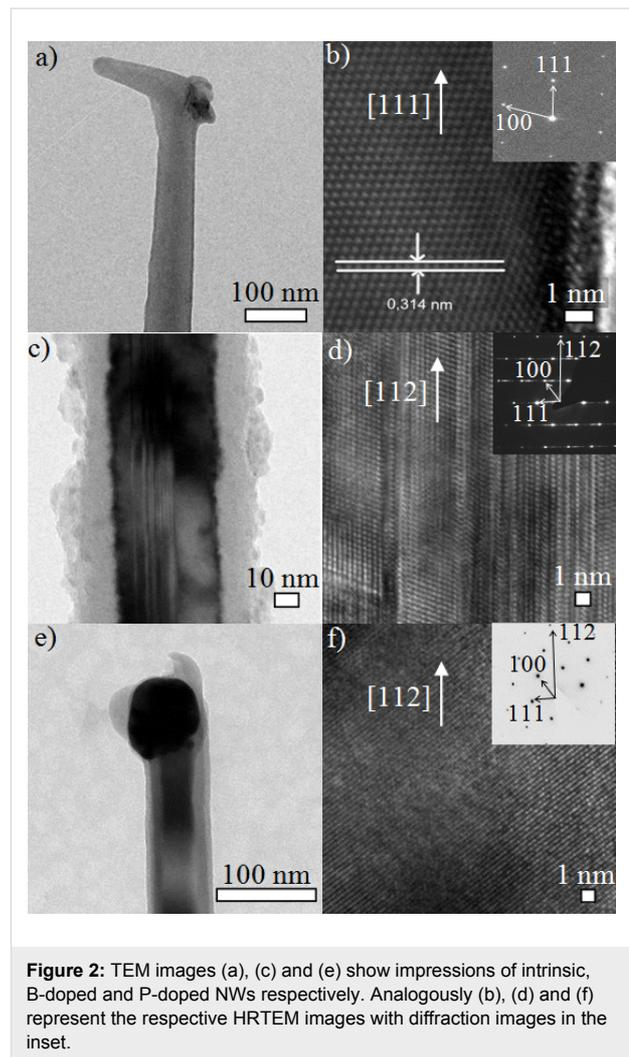
**Figure 2:** TEM images (a), (c) and (e) show impressions of intrinsic, B-doped and P-doped NWs respectively. Analogously (b), (d) and (f) represent the respective HRTEM images with diffraction images in the inset.
