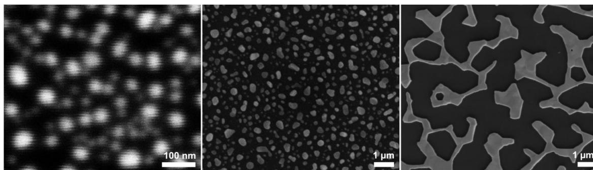
**Figure 5:** SEM image of gold nanoparticles formed on the native oxide surface of Si[111] after annealing of Au films deposited by sputtering for different lengths of time (left: 30 s; center: 1 min; right: 2 min). The annealing was performed at 650 °C for 1 h.
