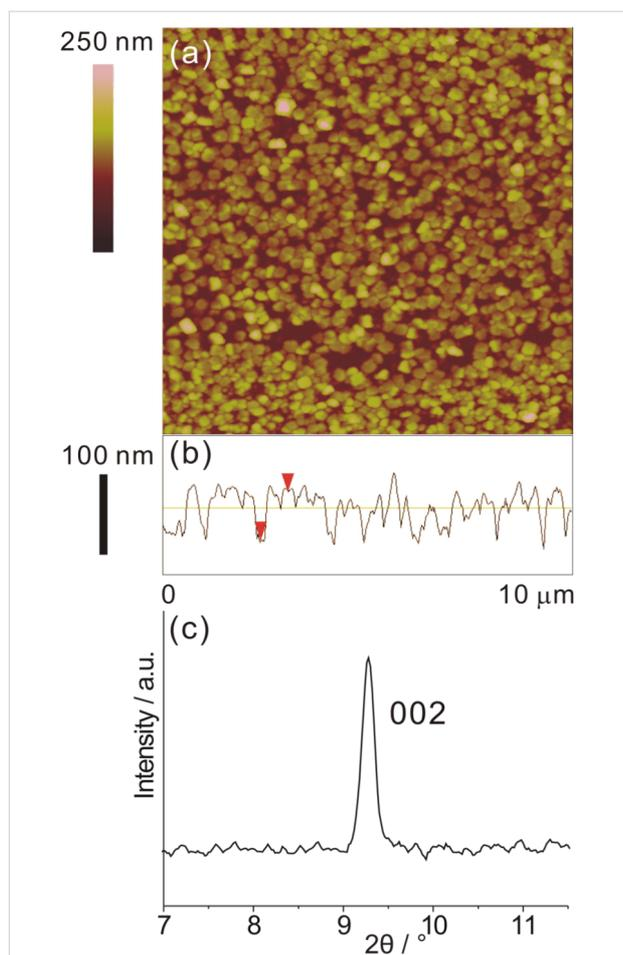
**Figure 5:**  $[\text{Zn}_2(\text{adc})_2(\text{dabco})]$  grown on a PPP1 surface at 60 °C after 45 cycles. (a) AFM image; (b) cross-sectional profile; (c) SXRD pattern of the range in which the (110) and the (002) reflections are expected.
