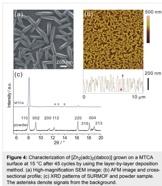
**Figure 4:** Characterization of  $[\text{Zn}_2(\text{adc})_2(\text{dabco})]$  grown on a MTCA surface at 15 °C after 45 cycles by using the layer-by-layer deposition method. (a) High-magnification SEM image; (b) AFM image and cross-sectional profile; (c) XRD patterns of SURMOF and powder sample. The asterisks denote signals from the background.
