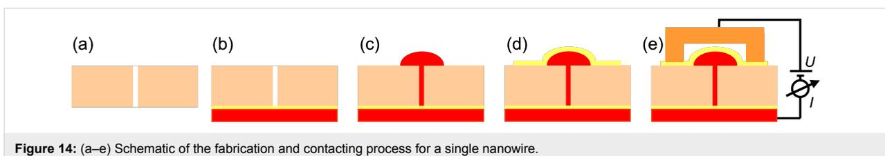
**Figure 14:** (a–e) Schematic of the fabrication and contacting process for a single nanowire.
