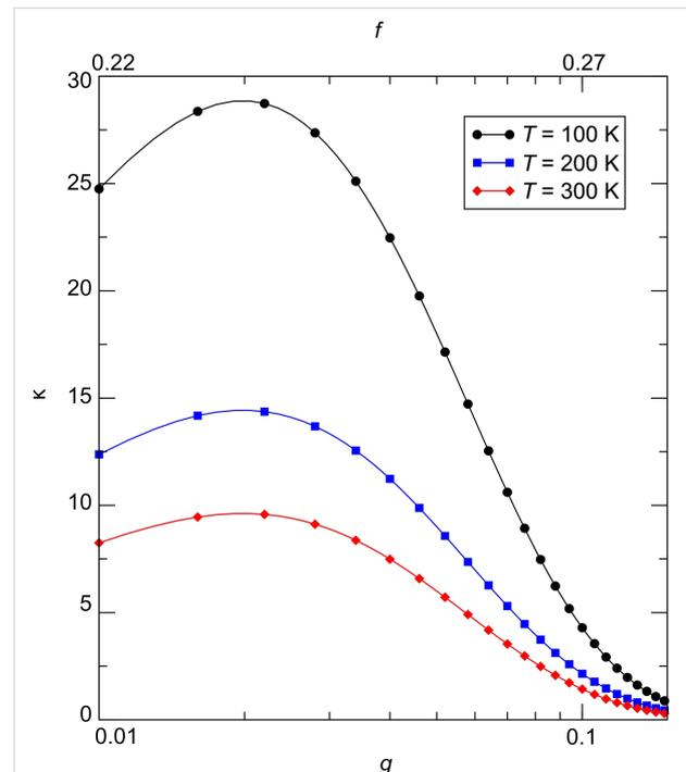
**Figure 15:** Calculated gauge factor  $\kappa$  as a function of intergrain coupling strength (bottom axis) and metal volume fraction (upper axis) at selected temperatures for the Arrhenius regime at intermediate coupling. Fcc-like packing of Au nanoparticles of 5.5 nm diameter in a dielectric matrix was assumed. The model parameters  $g_0^f = 3.29$ ,  $\varepsilon_i = 1.02$ ,  $\varepsilon_m = -16400$  and  $\bar{E} = E_C$  were used. For details see [59].
