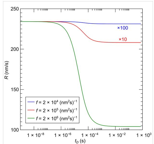
**Figure 2:** Single-species growth rate calculated for the precursor  $\text{Me}_3\text{Pt(IV)CpMe}$  assuming three different electron-flux values as indicated. The flux values correspond to beam currents of approximately 0.1, 1 and 10 nA with a beam diameter of 20 nm. The model parameters  $\sigma = 2.2 \times 10^{-2} \text{ nm}^2$  [23] and  $\tau = 29 \mu\text{s}$  [24] were used. The effective precursor flux was set to  $sJ = 1.5 \times 10^3 (\text{nm}^2\text{s})^{-1}$ .
