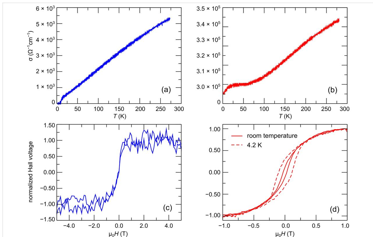
**Figure 10:** Temperature-dependent conductivity and Hall effect as a function of the applied magnetic field for samples B (a,c) and B' (b,d). The Hall data shown in (c) were taken at 228 K. Adapted from [33].
