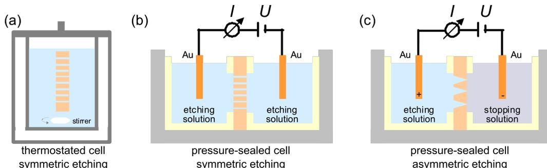
**Figure 4:** Schematic of etching equipment. Symmetric etching conditions leading to cylindrical channels in (a) thermostated cell and (b) pressure-sealed cell. (c) Asymmetric conditions leading to conical channels in pressure-sealed cell. Electric current measurements allow monitoring of the etching process.
