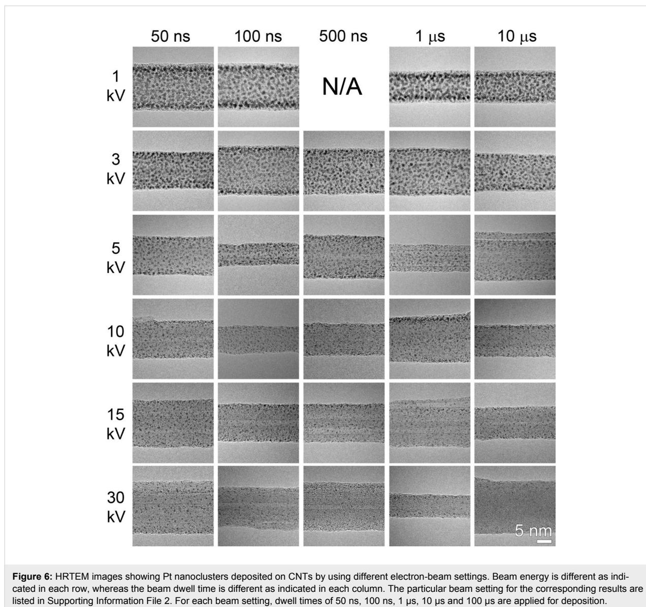
**Figure 6:** HRTEM images showing Pt nanoclusters deposited on CNTs by using different electron-beam settings. Beam energy is different as indicated in each row, whereas the beam dwell time is different as indicated in each column. The particular beam setting for the corresponding results are listed in Supporting Information File 2. For each beam setting, dwell times of 50 ns, 100 ns, 1 μs, 10 μs and 100 μs are applied for deposition.
