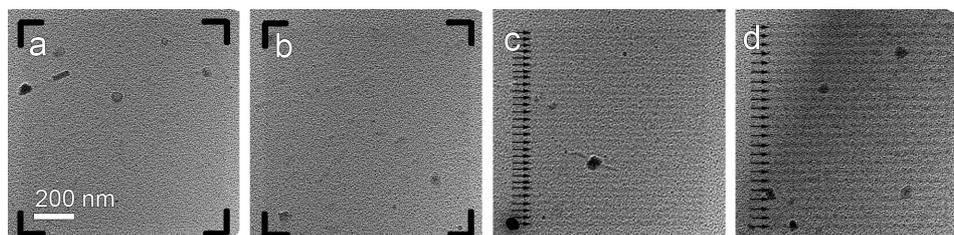
**Figure 4:** FEBID Pt on amorphous carbon at different defoci of the electron beam. (a) in focus, (b) at 4  $\mu\text{m}$  defocus, (c) at 8  $\mu\text{m}$  defocus and (d) at 10  $\mu\text{m}$  defocus of the 30 kV 0.2 nA electron beam. Stripes with high densities are indicated by arrows and illustrations.
