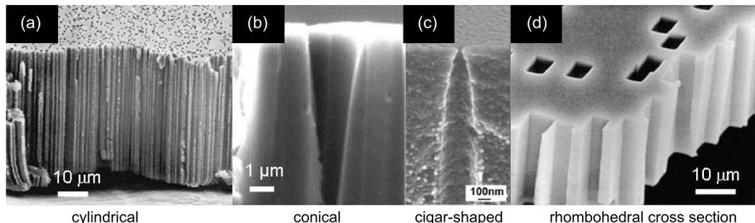
**Figure 3:** SEM images displaying the cross sections of the following membranes: (a) cylindrical channels in PI; (b) conical channels in PI; (c) cigar-shaped channels in PET, (d) cylindrical channels with rhombohedral cross section in mica. (a,b) Adapted with permission from [26] – Copyright 1996 Elsevier; (c) adapted with permission from [42] – Copyright 2007 IOP Publishing Ltd; (d) adapted with permission from [43] – Copyright 2012 American Physical Society.
