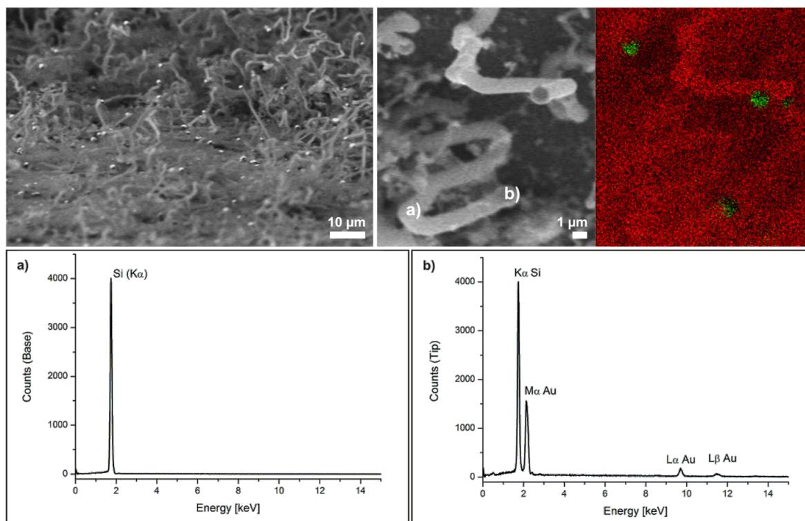
**Figure 2:** Analysis of NWs grown on gold-sputtered Si[111] for 1 h at 375 °C. Top left: Backscattered-electron image. The bright spots at the tips indicate the presence of a high-z material (gold). Top right: Composite EDX mapping image, green = gold, red = silicon. Bottom: EDX spectra obtained (a) at the base, (b) at the tip of the NWs.
