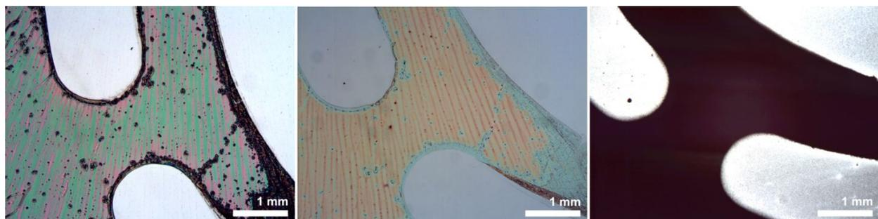
**Figure 12:** Optical microscopy images of the different steps of the irradiation-induced pattern formation. Left: The “liquid bright gold” film after UV irradiation and washing with dichloromethane. Center: The same area after annealing at 650 °C. Right: The pattern is reproduced after 1 h of treatment with NPS at 650 °C. The bright areas are due to the high reflectivity of the uncovered Si substrate.
