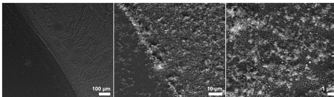
**Figure 13:** SEM images (different magnifications) of Si NWs obtained from UV-patterned spin-coated “liquid bright gold” films after annealing at 650 °C, followed by treatment with NPS at 375 °C for 1 h.
