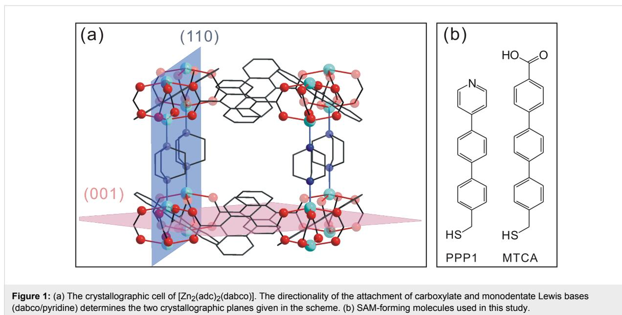
**Figure 1:** (a) The crystallographic cell of  $[\text{Zn}_2(\text{adC})_2(\text{dabco})]$ . The directionality of the attachment of carboxylate and monodentate Lewis bases (dabco/pyridine) determines the two crystallographic planes given in the scheme. (b) SAM-forming molecules used in this study.
