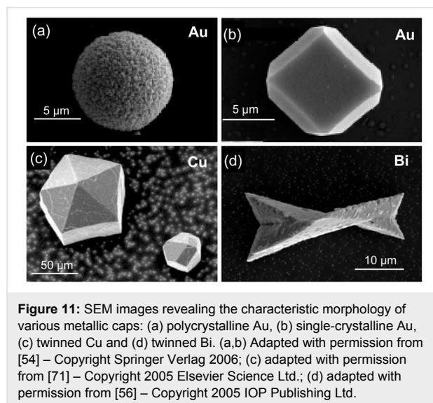
**Figure 11:** SEM images revealing the characteristic morphology of various metallic caps: (a) polycrystalline Au, (b) single-crystalline Au, (c) twinned Cu and (d) twinned Bi. (a,b) Adapted with permission from [54] – Copyright Springer Verlag 2006; (c) adapted with permission from [71] – Copyright 2005 Elsevier Science Ltd.; (d) adapted with permission from [56] – Copyright 2005 IOP Publishing Ltd.
