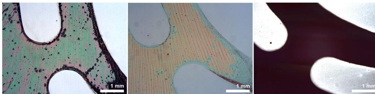
**Figure 12:** Optical microscopy images of the different steps of the irradiation-induced pattern formation. Left: The “liquid bright gold” film after UV irradiation and washing with dichloromethane. Center: The same area after annealing at 650 °C. Right: The pattern is reproduced after 1 h of treatment with NPS at 650 °C. The bright areas are due to the high reflectivity of the uncovered Si substrate.
