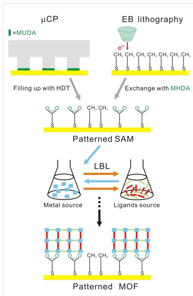
**Figure 6:** SAMs can be either patterned by  $\mu\text{CP}$  (top row, left) or by EB lithography (top row, right) before the layer-by-layer deposition of  $[\text{Zn}_2(\text{adc})_2(\text{dabco})]$  (bottom).
