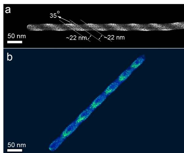
**Figure 5:** (a) HAADF-STEM image of a CNT with stripe-pattern of Pt nanoclusters from FEBID. (b) A snapshot from the 3D reconstruction of the nanostructure.
