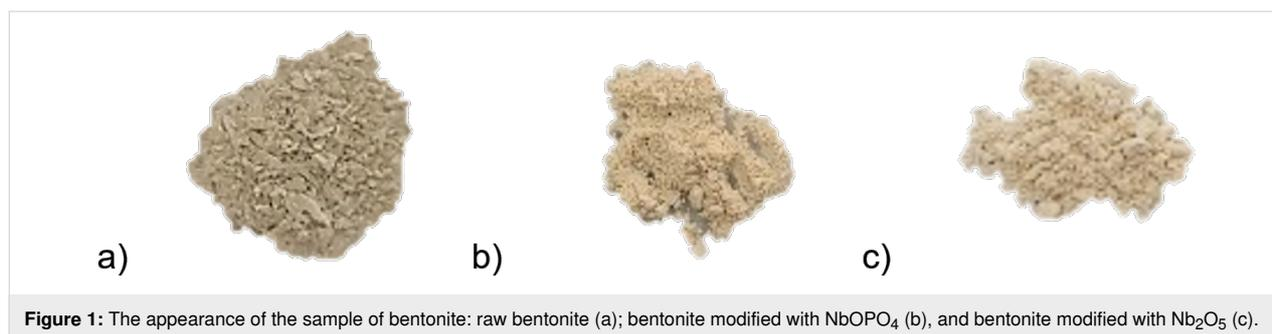
**Figure 1:** The appearance of the sample of bentonite: raw bentonite (a); bentonite modified with NbOPO<sub>4</sub> (b), and bentonite modified with Nb<sub>2</sub>O<sub>5</sub> (c).
