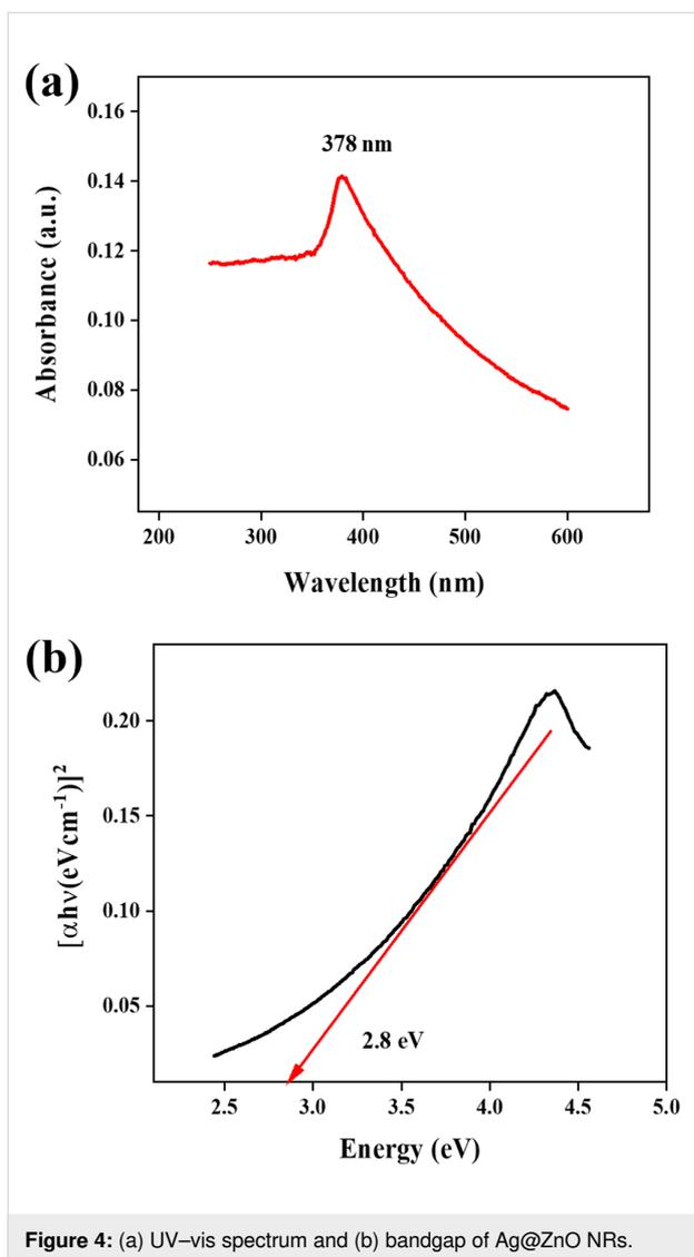
**Figure 4:** (a) UV-vis spectrum and (b) bandgap of Ag@ZnO NRs.
