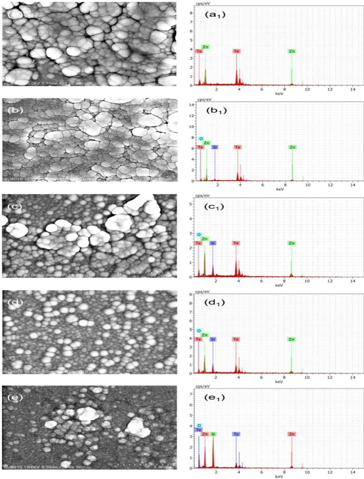
**Figure 4:** FESEM micrographs (a–e) and EDS spectra (a<sub>1</sub>–e<sub>1</sub>) of ZnTe films deposited at (a, a<sub>1</sub>) R.T., (b, b<sub>1</sub>) 300 °C, (c, c<sub>1</sub>) 400 °C, (d, d<sub>1</sub>) 500 °C, and (e, e<sub>1</sub>) 600 °C. (The scale bars are 2 μm).
