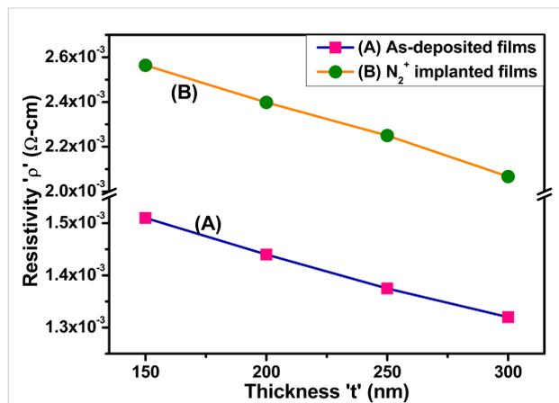
**Figure 11:** Resistivity of (A) as-deposited and (B)  $\text{N}_2^+$ -implanted Mo thin films as a function of the thickness.
