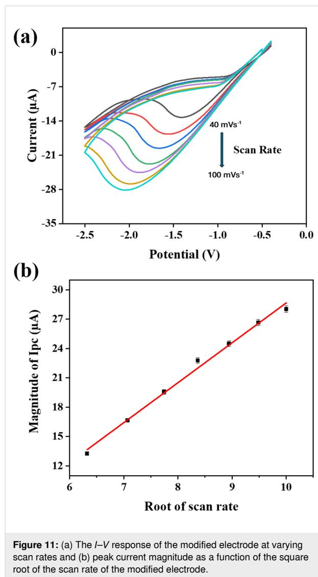
**Figure 11:** (a) The  $I$ - $V$  response of the modified electrode at varying scan rates and (b) peak current magnitude as a function of the square root of the scan rate of the modified electrode.
