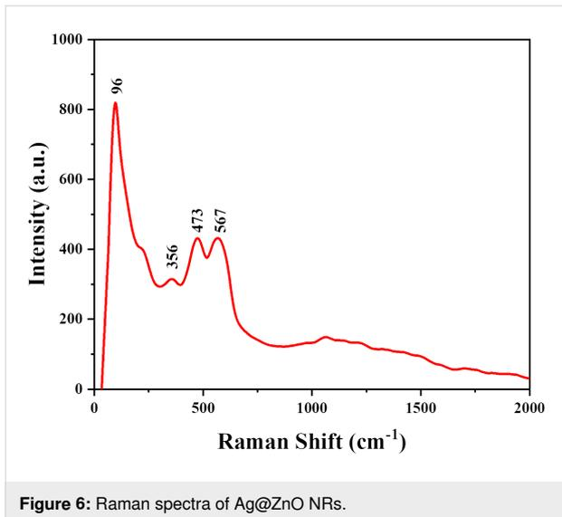
Figure 6: Raman spectra of Ag@ZnO NRs.
