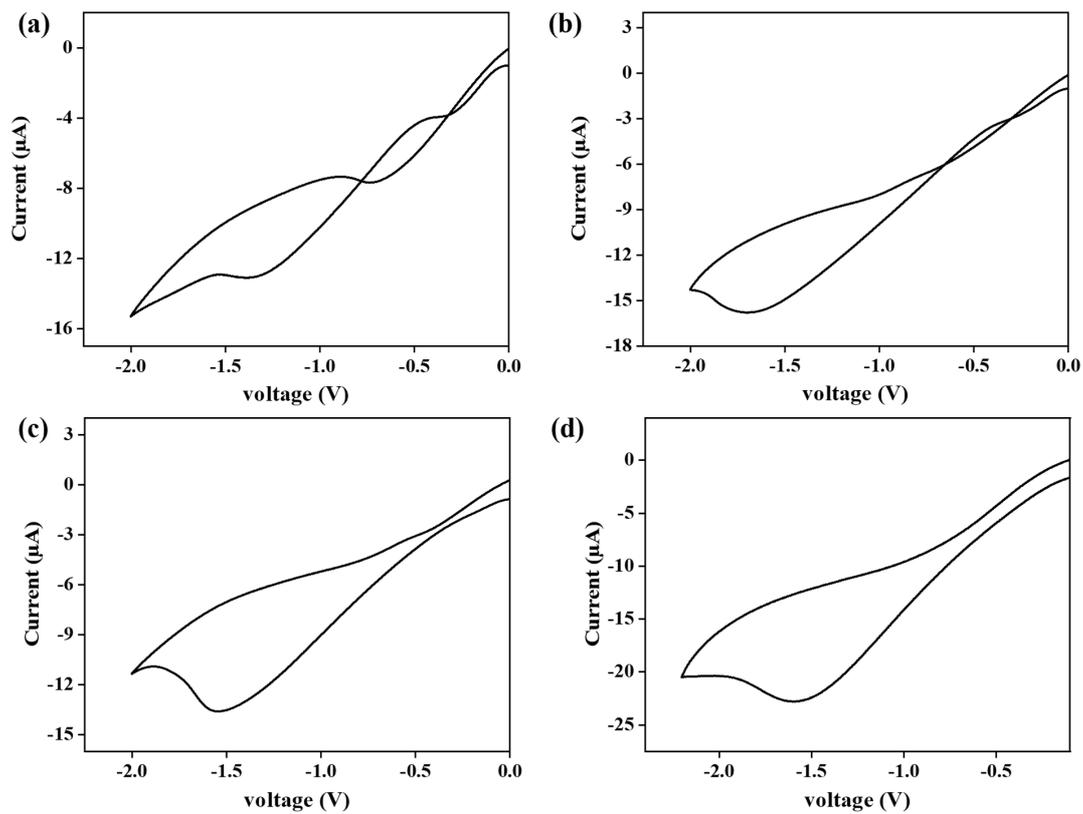
**Figure 13:** *I*–*V* response of the modified electrode at a varying concentration of lead in (a) canal water, (b) groundwater, (c) water obtained after reverse osmosis (RO) and (d), supply drinking water.
