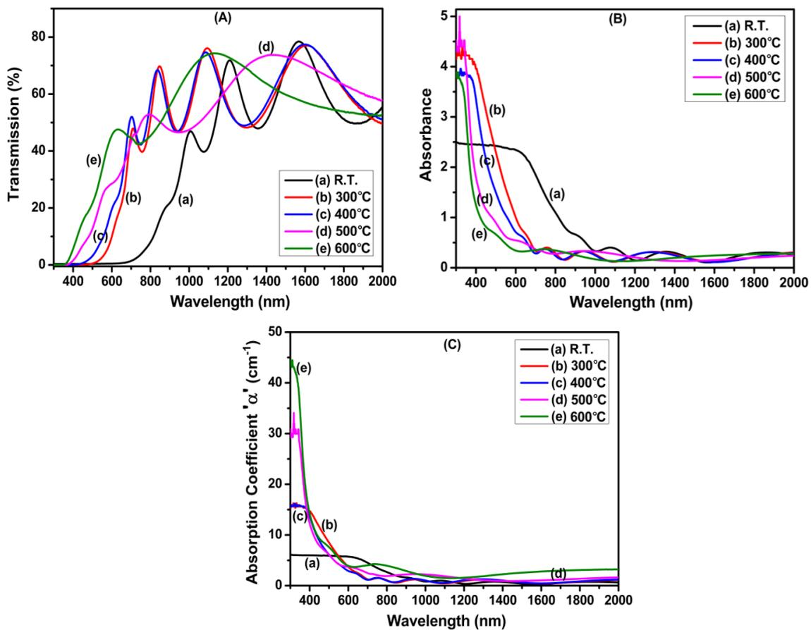
**Figure 5:** Variation in (A) transmittance, (B) absorbance, and (C) absorption coefficient with wavelength of ZnTe films produced at (a) R.T. and substrate temperatures of (b) 300 °C, (c) 400 °C, (d) 500 °C, and (e) 600 °C.
