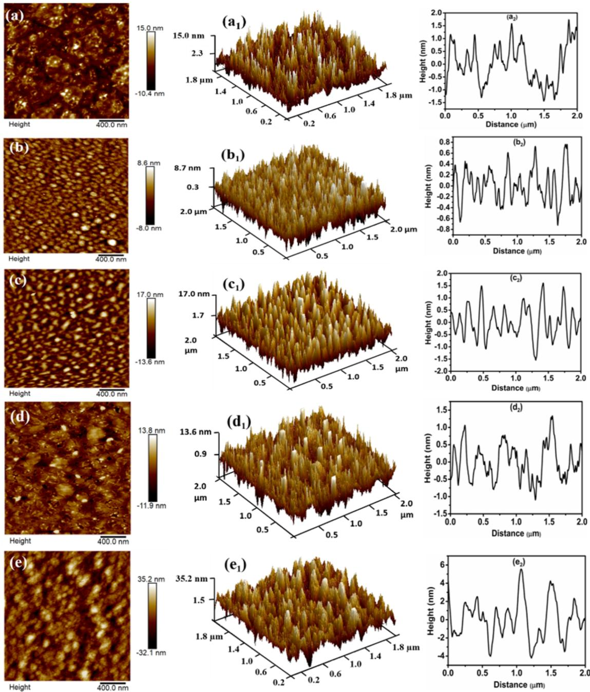
**Figure 2:** 2D (a–e) and 3D (a<sub>1</sub>–e<sub>1</sub>) AFM images and Height profile (a<sub>2</sub>–e<sub>2</sub>) analysis of ZnTe films deposited at (a, a<sub>1</sub>, a<sub>2</sub>) R.T. and substrate temperatures of (b, b<sub>1</sub>, b<sub>2</sub>) 300 °C, (c, c<sub>1</sub>, c<sub>2</sub>) 400 °C, (d, d<sub>1</sub>, d<sub>2</sub>) 500 °C, and (e, e<sub>1</sub>, e<sub>2</sub>) 600 °C.
