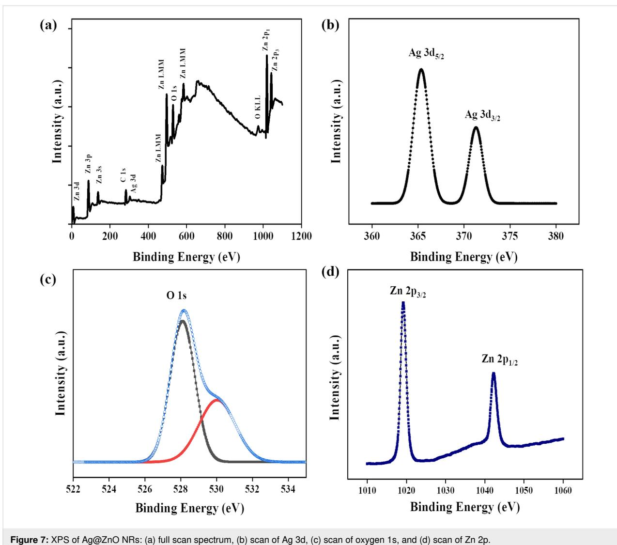
Figure 7: XPS of Ag@ZnO NRs: (a) full scan spectrum, (b) scan of Ag 3d, (c) scan of oxygen 1s, and (d) scan of Zn 2p.
