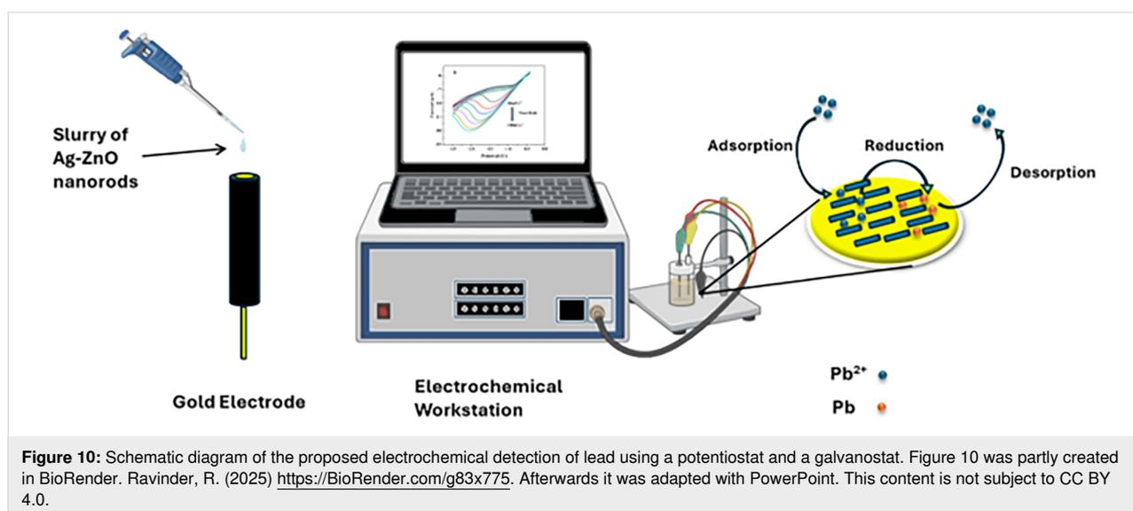
**Figure 10:** Schematic diagram of the proposed electrochemical detection of lead using a potentiostat and a galvanostat. Figure 10 was partly created in BioRender. Ravinder, R. (2025) <https://BioRender.com/g83x775>. Afterwards it was adapted with PowerPoint. This content is not subject to CC BY 4.0.
