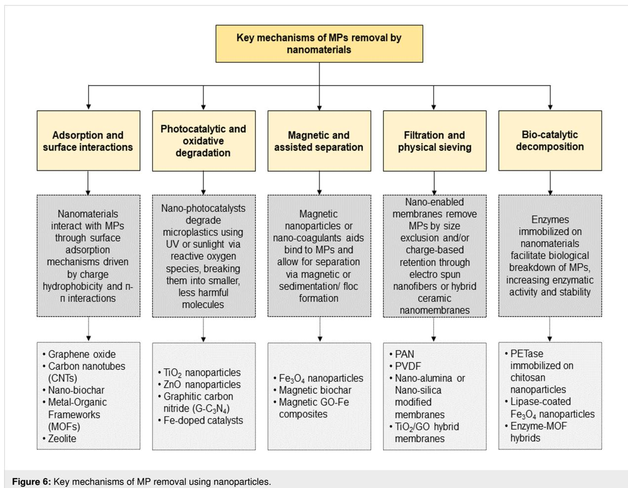
**Figure 6:** Key mechanisms of MP removal using nanoparticles.
