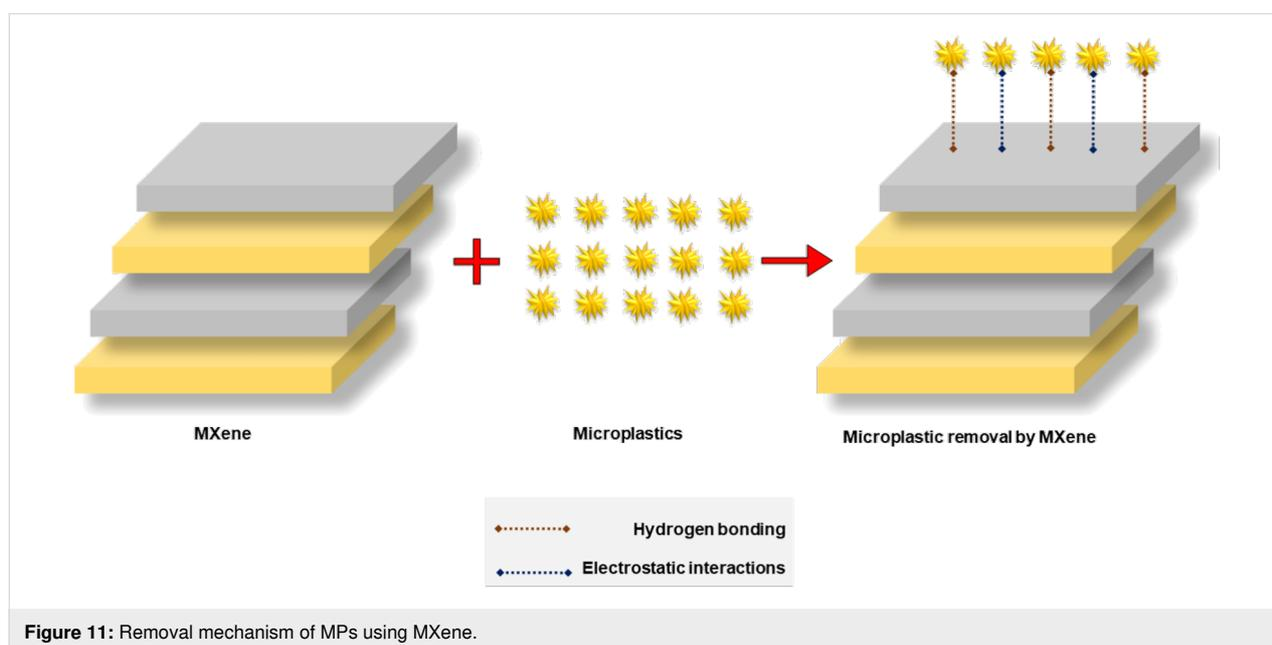
**Figure 11:** Removal mechanism of MPs using MXene.
