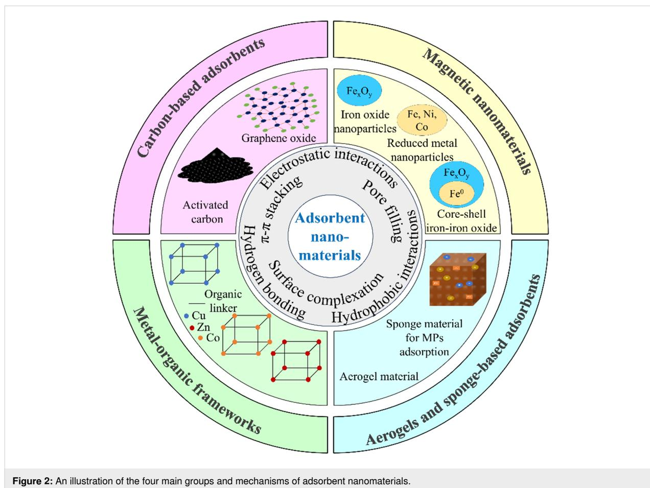
**Figure 2:** An illustration of the four main groups and mechanisms of adsorbent nanomaterials.
