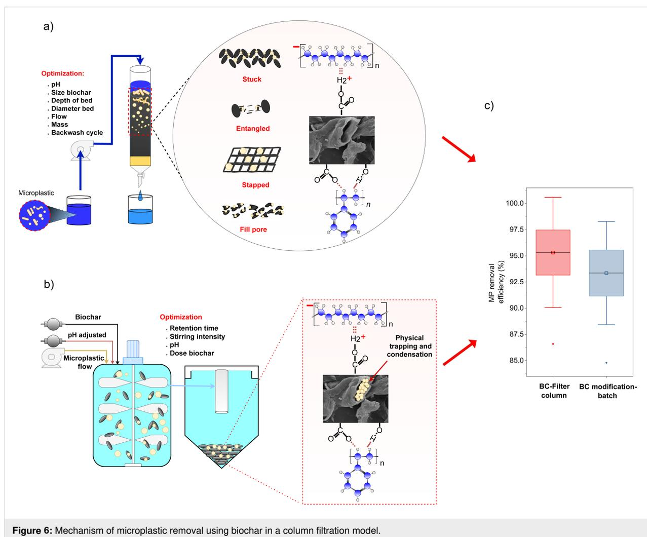
**Figure 6:** Mechanism of microplastic removal using biochar in a column filtration model.
