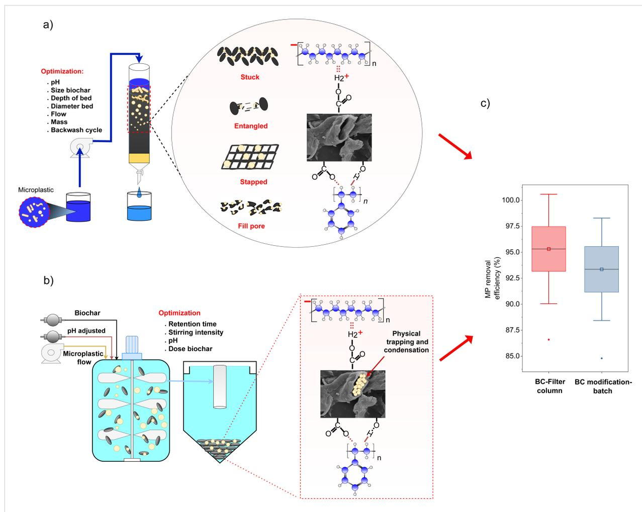
Figure 6: Mechanism of microplastic removal using biochar in a column filtration model.
