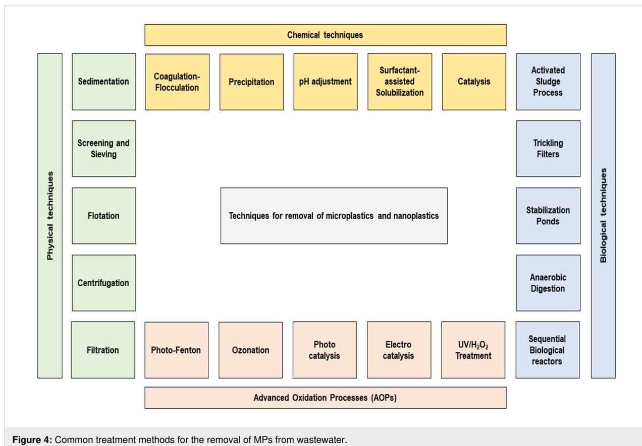
**Figure 4:** Common treatment methods for the removal of MPs from wastewater.
