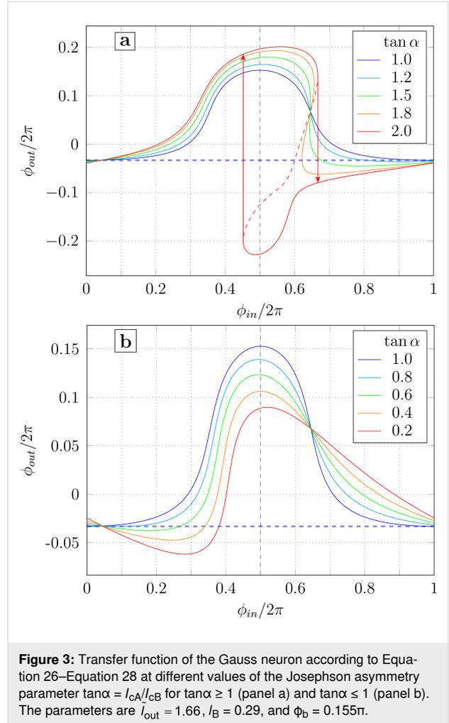
**Figure 3:** Transfer function of the Gauss neuron according to Equation 26–Equation 28 at different values of the Josephson asymmetry parameter  $\tan\alpha = I_{cA}/I_{cB}$  for  $\tan\alpha \geq 1$  (panel a) and  $\tan\alpha \leq 1$  (panel b). The parameters are  $\tilde{l}_{\text{out}} = 1.66$ ,  $l_B = 0.29$ , and  $\phi_b = 0.155\pi$ .
