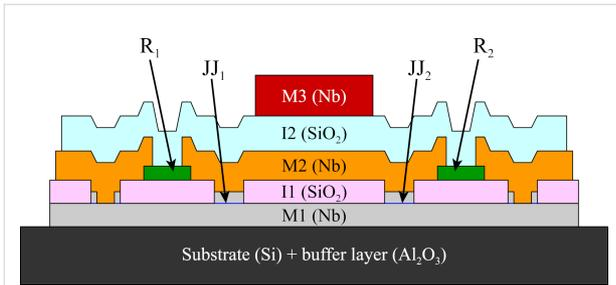
**Figure 1:** Cross-sectional diagram of a two-junction SQUID containing three superconducting layers (M1, M2, and M3) separated by insulating layers (I1 and I2). Josephson junctions are labeled as  $JJ_{1,2}$ , and their shunt resistors are  $R_{1,2}$ . Layer heights are to scale.
