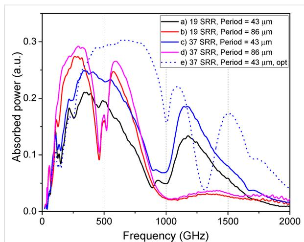
**Figure 5:** Dependence of the absorbed power on the number of elements in the SRR array.
