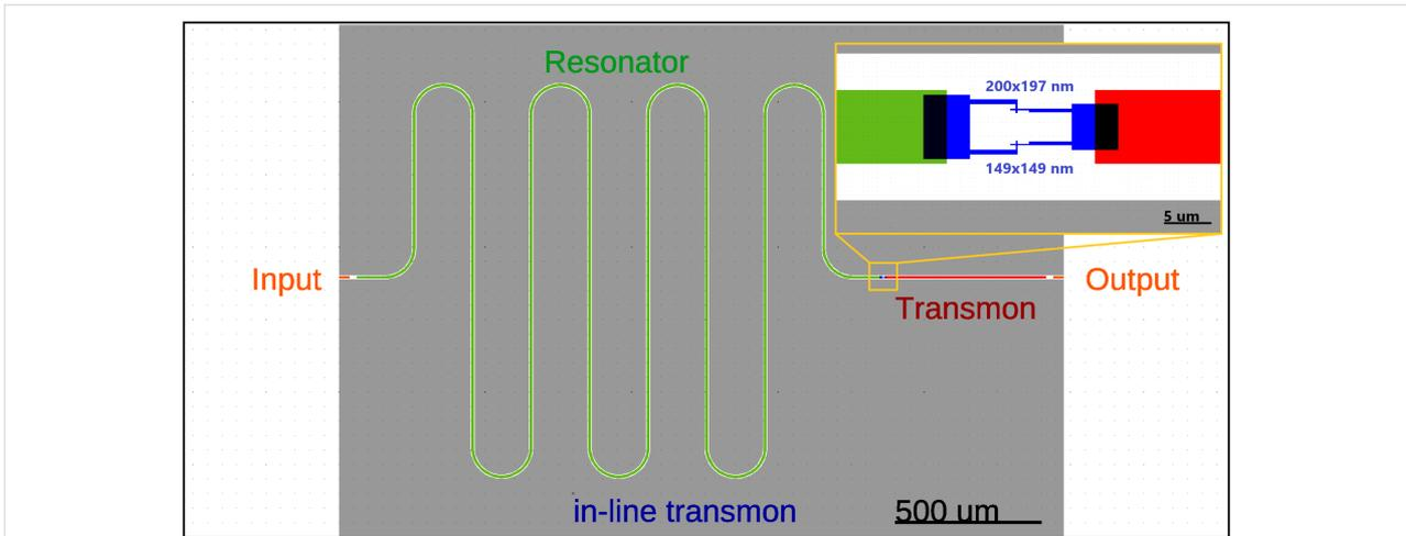
**Figure 5:** In-line transmon design for efficient transmission of the quantum state. The red part of the central conductor of the resonator and the blue SQUID form a transmon, the total length of the resonator (green and red parts) forms the main resonant mode  $\omega_0$ .
