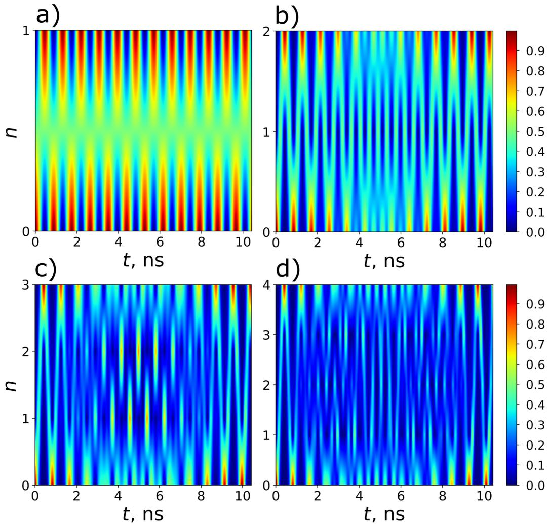
**Figure 8:** A demonstration of the rapid control of the states with  $n = 1$ –4 of the designed transmon (from (a) to (d), respectively). The panels show the time-dependent population of transmon states at the selected optimal frequency detuning. The parameters for each panel are the same as for the corresponding panels in Figure 7.
