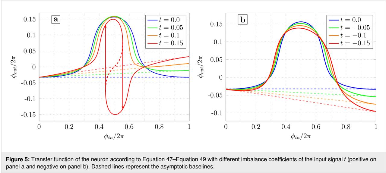
**Figure 5:** Transfer function of the neuron according to Equation 47–Equation 49 with different imbalance coefficients of the input signal  $t$  (positive on panel a and negative on panel b). Dashed lines represent the asymptotic baselines.
