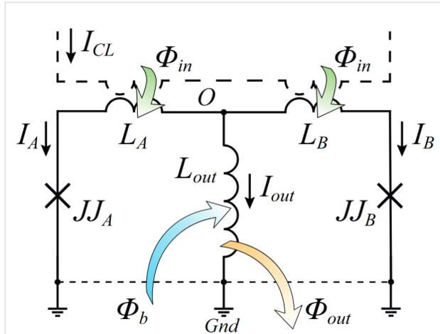
**Figure 1:** Schematic representation of a Gauss neuron, adapted from [14] (see details in the text).
