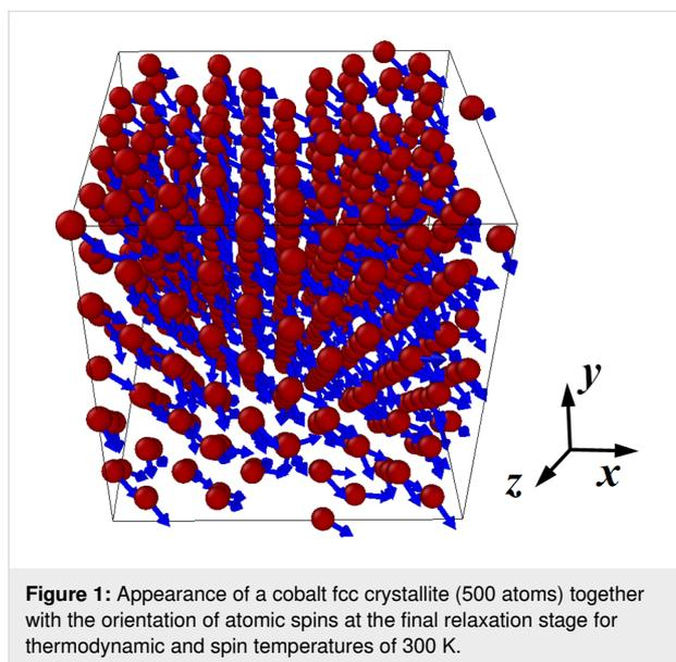
**Figure 1:** Appearance of a cobalt fcc crystallite (500 atoms) together with the orientation of atomic spins at the final relaxation stage for thermodynamic and spin temperatures of 300 K.
