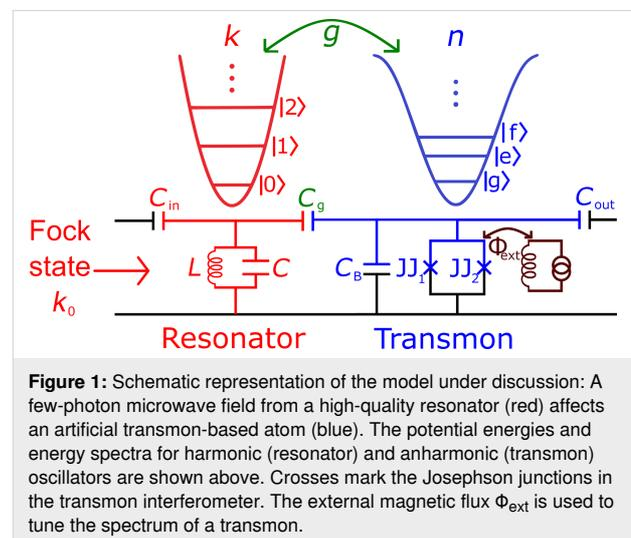
**Figure 1:** Schematic representation of the model under discussion: A few-photon microwave field from a high-quality resonator (red) affects an artificial transmon-based atom (blue). The potential energies and energy spectra for harmonic (resonator) and anharmonic (transmon) oscillators are shown above. Crosses mark the Josephson junctions in the transmon interferometer. The external magnetic flux  $\Phi_{\text{ext}}$  is used to tune the spectrum of a transmon.
