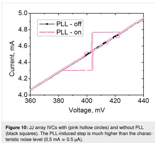
**Figure 10:** JJ array IVCs with (pink hollow circles) and without PLL (black squares). The PLL-induced step is much higher than the characteristic noise level ( $0.5 \text{ mA} \gg 0.5 \mu\text{A}$ ).
