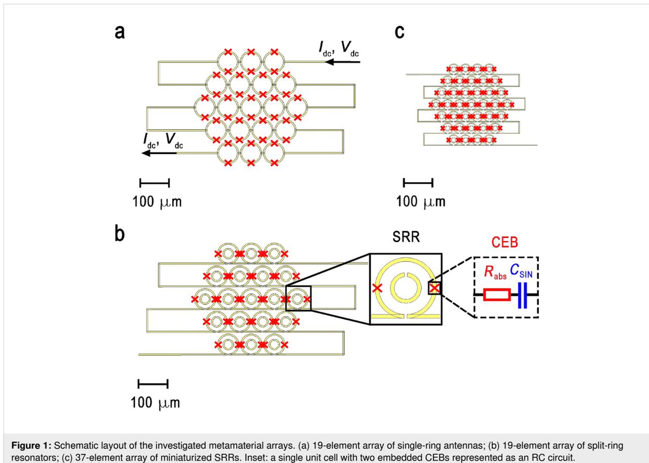
**Figure 1:** Schematic layout of the investigated metamaterial arrays. (a) 19-element array of single-ring antennas; (b) 19-element array of split-ring resonators; (c) 37-element array of miniaturized SRRs. Inset: a single unit cell with two embedded CEBs represented as an RC circuit.
