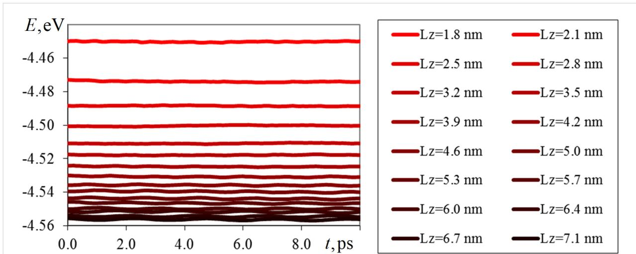
**Figure 4:** Variation of the magnetic energy of cobalt (fcc) normalized by the number of atoms in the system for nanofilms with thicknesses of 1.8–7.1 nm and thermodynamic and spin temperatures of 300 K.
