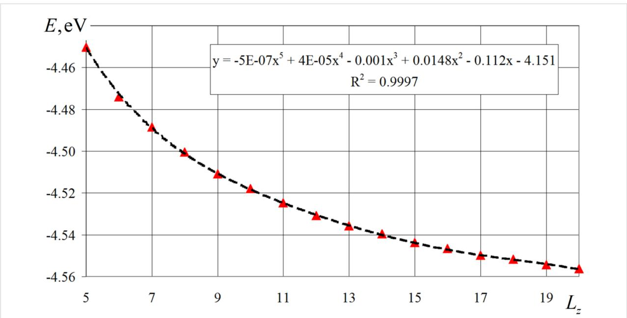
Figure 8: Variation of cobalt magnetic energy as a function of nanofilm thickness measured in crystalline layers.
