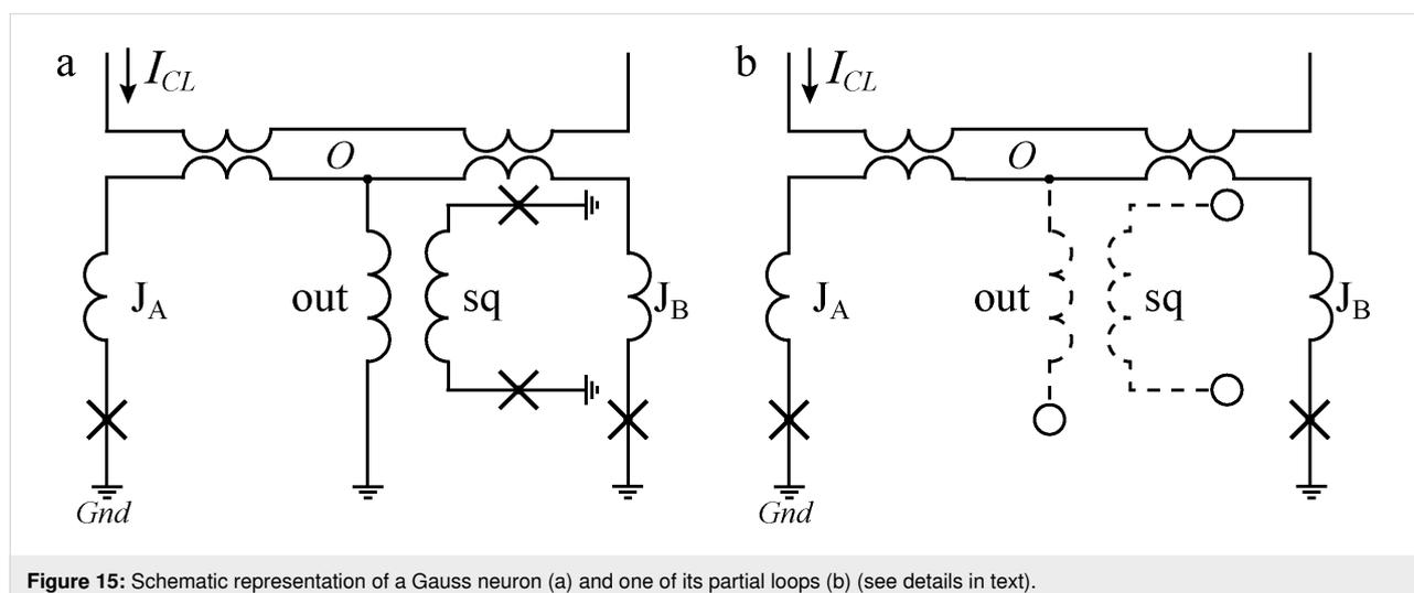
**Figure 15:** Schematic representation of a Gauss neuron (a) and one of its partial loops (b) (see details in text).
