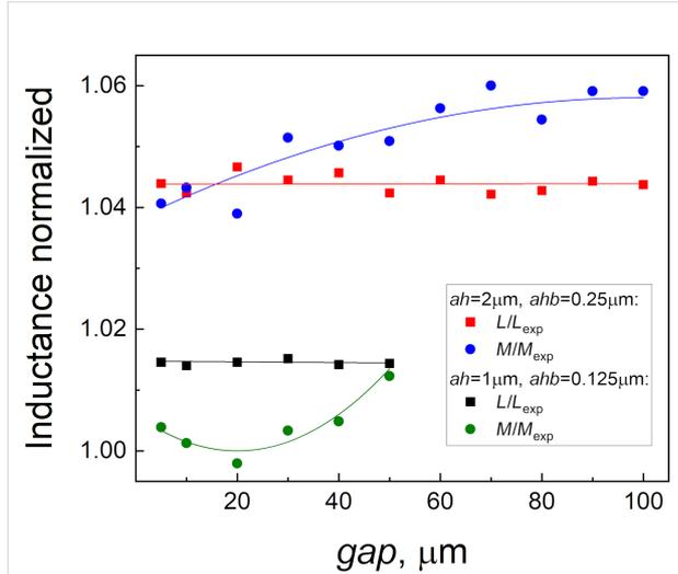
**Figure 11:** Dependence of self- and mutual inductances of the test SQUID (see Figure 2b) on the size of the superconducting screen in simulation. The horizontal axis corresponds to the distance from the outer boundaries of the structure to the truncated screen boundaries in simulation (see Figure 2c for definition).
