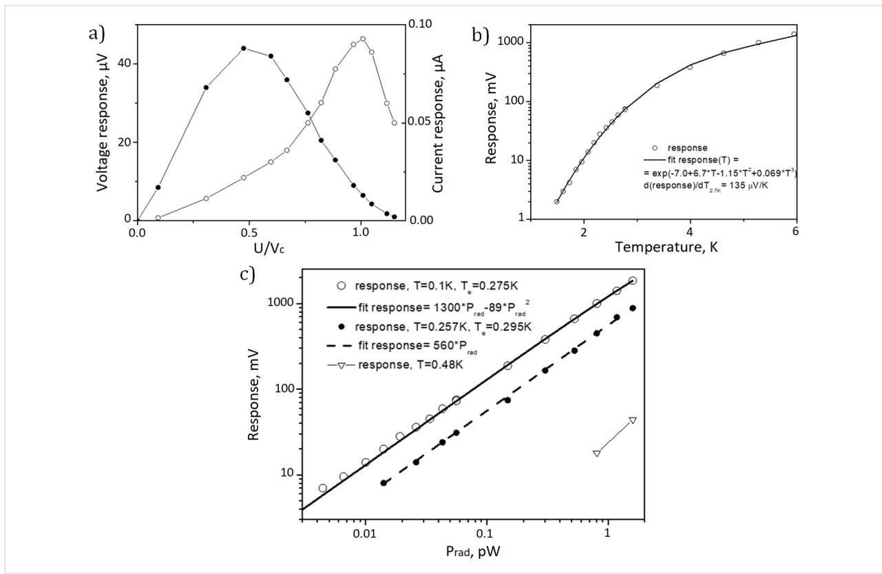
**Figure 7:** Some of SINIS detectors measured characteristics. (a) Current and voltage response for a parallel array for  $P_{\text{rad}} = 1 \text{ pW}$  and maximum current responsivity of  $dI/dP = 72000 \text{ A/W}$ . (b) Voltage response on black body temperature; at 2.7 K, it is  $dV/dT = 135 \mu\text{V}\cdot\text{K}^{-1}$ , (c) voltage response at temperatures of 0.1, 0.295, and 0.48 K; the maximum response is  $3.9 \text{ V/nW}$ .
