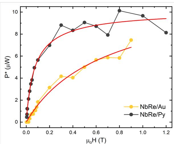
**Figure 4:** Dissipated power at the instability point as a function of the magnetic field at  $t \approx 0.5$  for NbRe/Au and NbRe/Py bilayers. The red solid lines are the fit to the data according to the BS theory [6].
