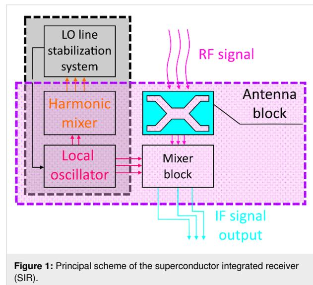
**Figure 1:** Principal scheme of the superconductor integrated receiver (SIR).
