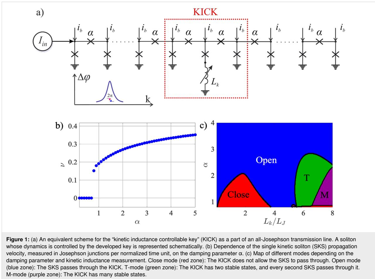
KICK functions as a T-flip-flop. It possesses two stable states, and each arriving soliton toggles the cell from its current state to the other. Every second soliton passes to the exit. (4) M-mode (Multistate mode): This regime is characterized by the formation of more than two stable states and other complex dynamics, which fall outside the scope of this study.
