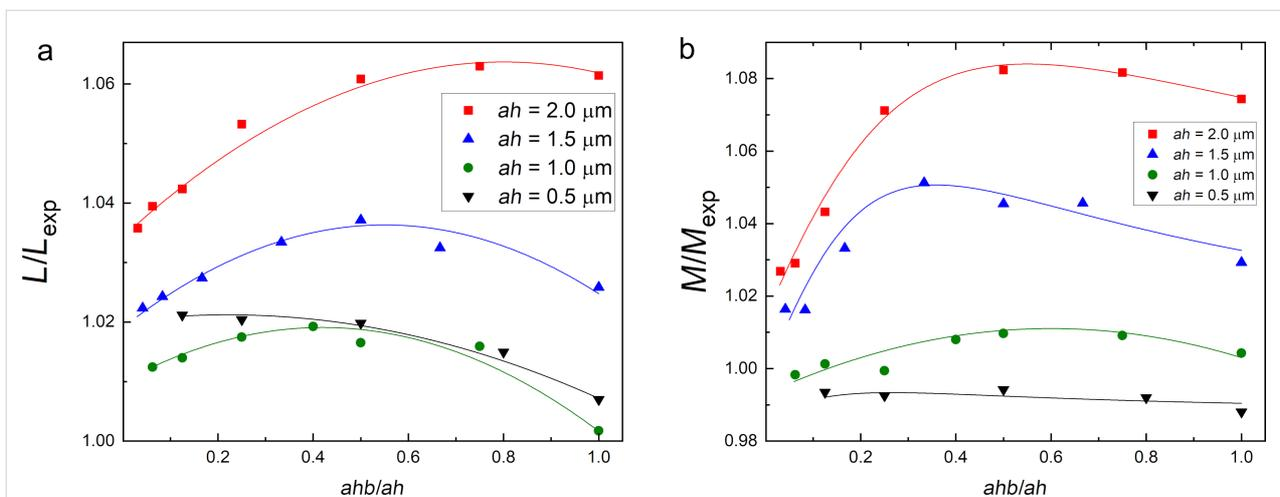
**Figure 9:** Dependence of calculated self- (a) and mutual (b) inductances of the test two-junction interferometer (see Figure 2b) on the edge discretization step  $ahb$  for several values of the general spatial discretization step  $ah$  (indicated in the Figure). Calculated values are normalized to the experimental ones.
