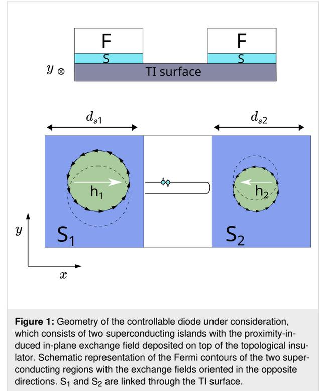
**Figure 1:** Geometry of the controllable diode under consideration, which consists of two superconducting islands with the proximity-induced in-plane exchange field deposited on top of the topological insulator. Schematic representation of the Fermi contours of the two superconducting regions with the exchange fields oriented in the opposite directions.  $S_1$  and  $S_2$  are linked through the TI surface.
