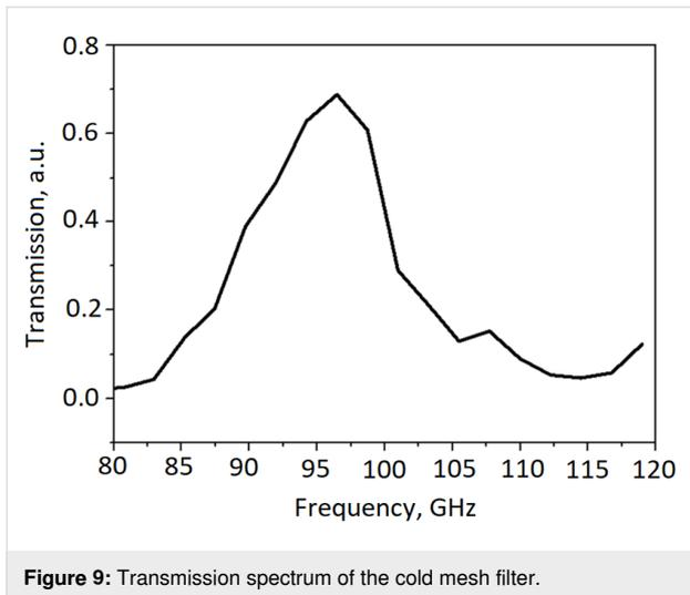
**Figure 9:** Transmission spectrum of the cold mesh filter.
