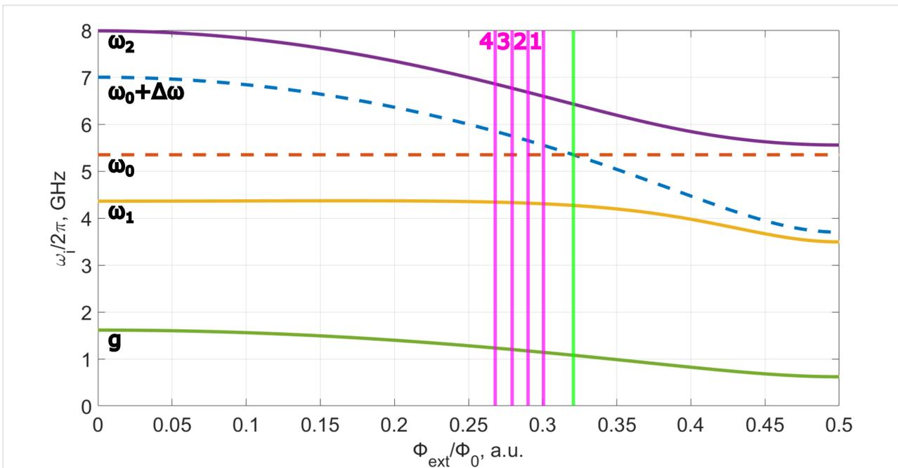
**Figure 6:** The dependence of the plasma frequency of the qubit  $\omega_p = \omega_0 + \Delta\omega$  and coupling strength  $g$  between this two systems on the external magnetic flux  $\Phi_{ext}$ . When these two systems are connected, the united system with two modes  $\omega_1$  and  $\omega_2$  appears. Anticrossing at the point when the frequencies of the two systems coincide corresponds to the green vertical line.
