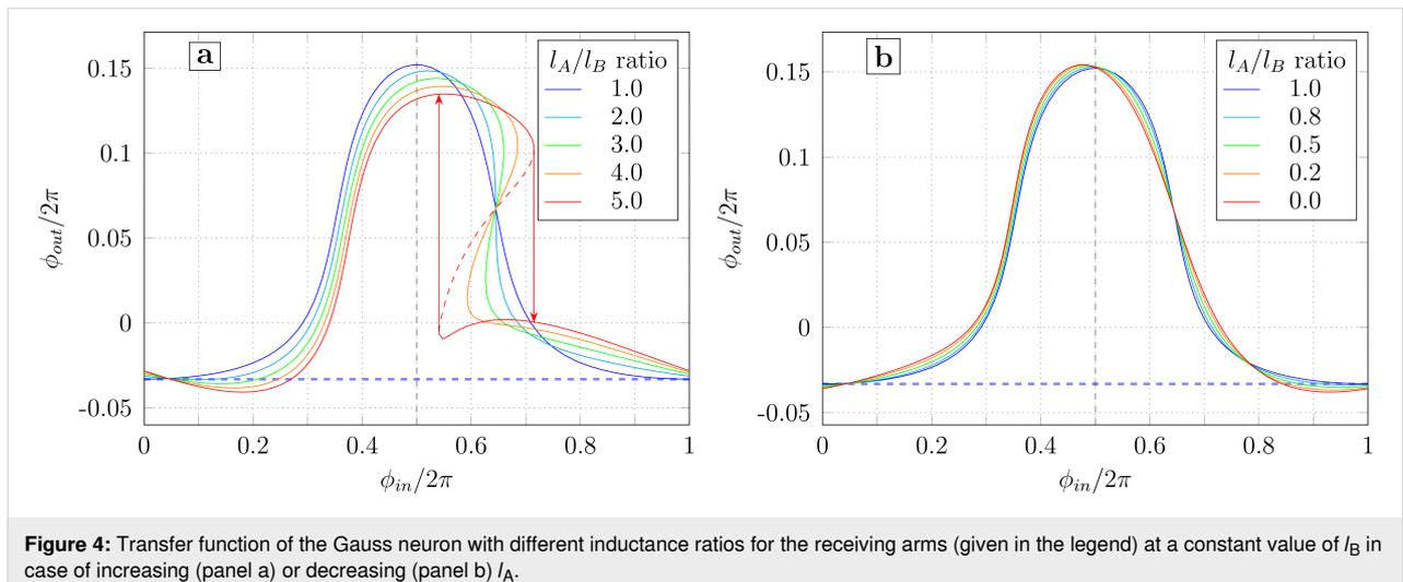
**Figure 4:** Transfer function of the Gauss neuron with different inductance ratios for the receiving arms (given in the legend) at a constant value of  $l_B$  in case of increasing (panel a) or decreasing (panel b)  $l_A$ .
