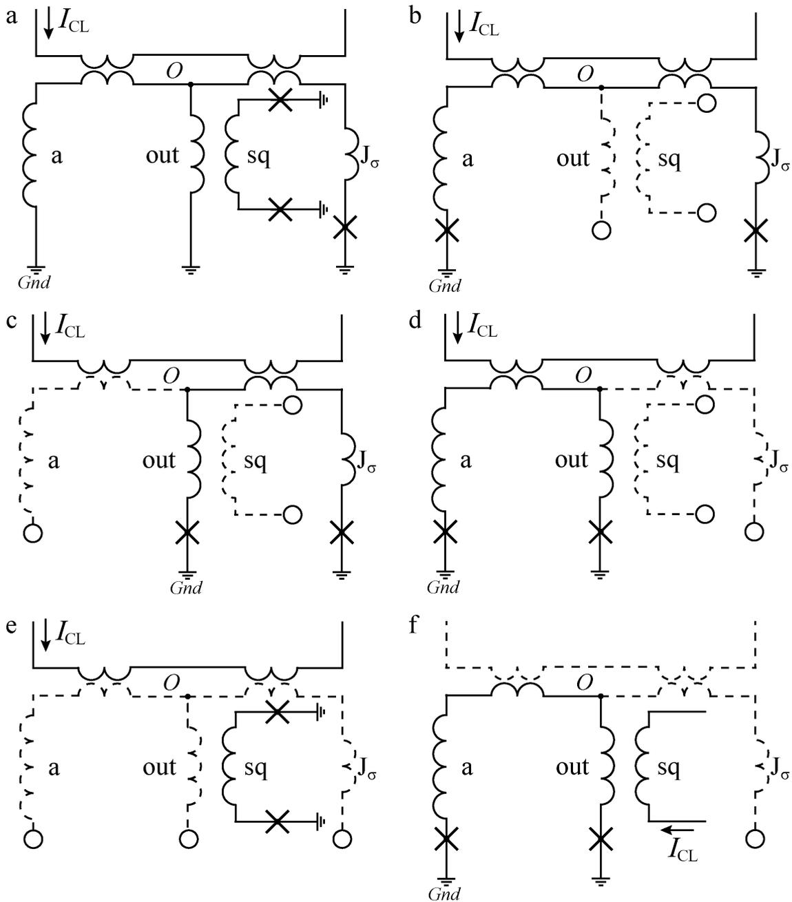
**Figure 14:** Schematic representation of a sigma neuron and examples of its partial loops (see details in text). JJs are marked with crosses, and the wavy lines stand for inductances. Circles indicate the nodes where the circuit is open, and the corresponding arms are drawn with dashed lines, as well as the elements “CL” and “sq” in case they are not used.
