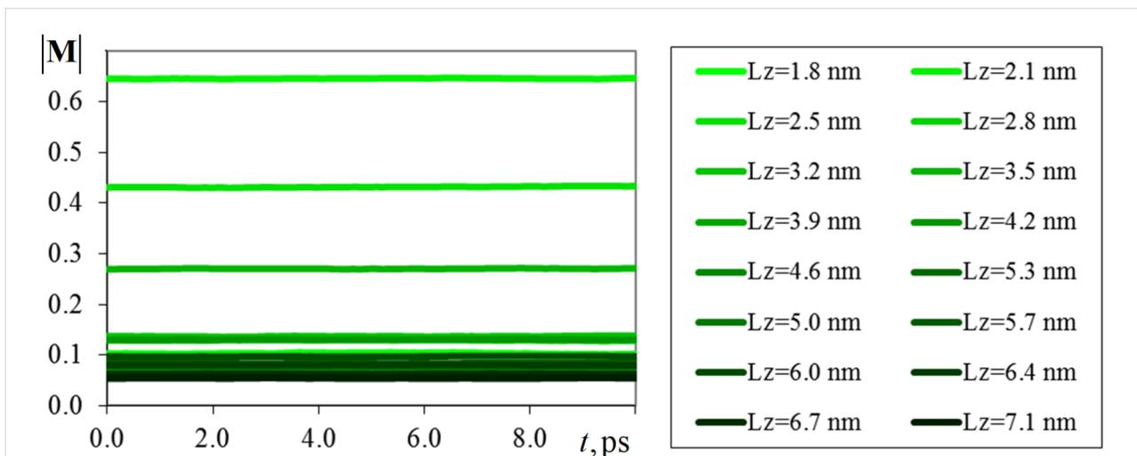
**Figure 5:** Variation of the magnetization modulus of cobalt (fcc) normalized by the number of atoms in the system, for nanofilms of thicknesses 1.8–7.1 nm and thermodynamic and spin temperatures of 300 K.
