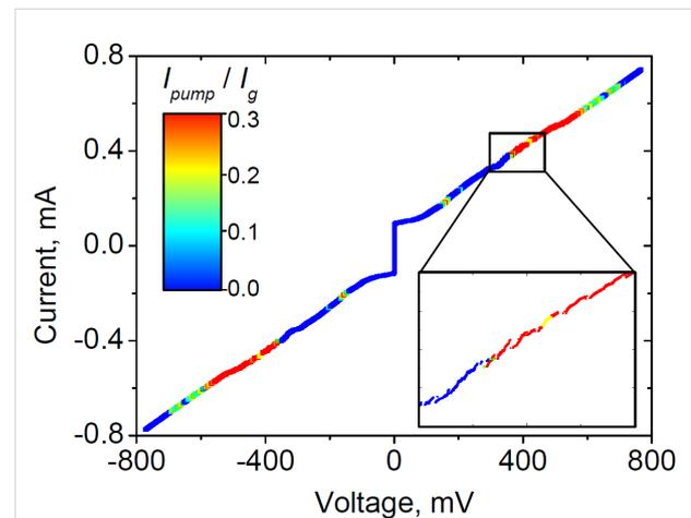
**Figure 5:** IVC of the 600 JJ array with 300–550 GHz matching circuit and matched load on the nonradiating end. The color indicates the  $I_{\text{pump}}$  of the SIS mixer in the corresponding operating point. The inset shows the enlarged part of the IVC, where the steps related to the resonances along the entire array length are observed.
