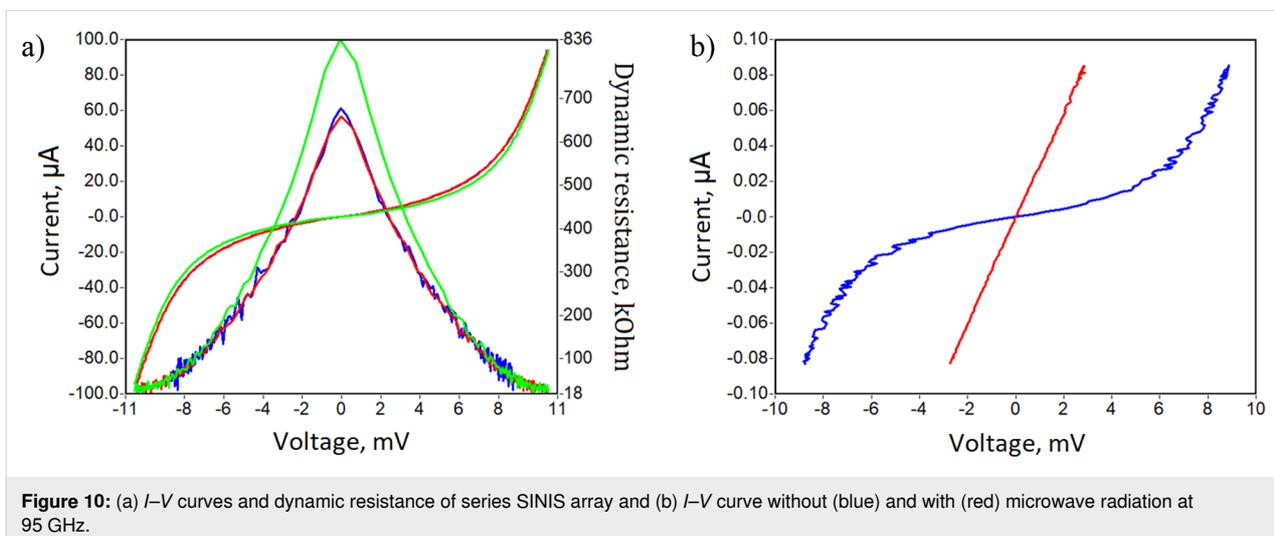
**Figure 10:** (a)  $I$ – $V$  curves and dynamic resistance of series SINIS array and (b)  $I$ – $V$  curve without (blue) and with (red) microwave radiation at 95 GHz.
