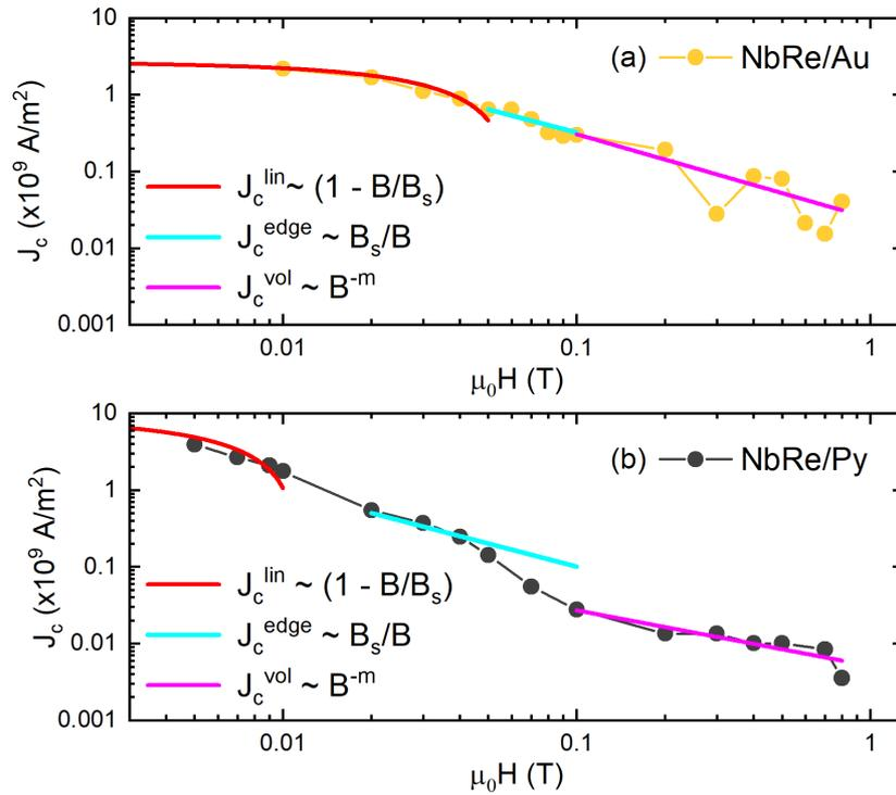
**Figure 3:** Magnetic field dependence for the critical current density at  $t \approx 0.5$  of NbRe/Au (a) and NbRe/Py (b). The red curves represent the dependence  $J_c^{\text{lin}} \sim (1 - B/B_s)$ , the cyan curves the dependence  $J_c^{\text{edge}}(B) \sim B_s/B$ , and the magenta curves the dependence  $J_c^{\text{vol}} \sim B^{-m}$ .
