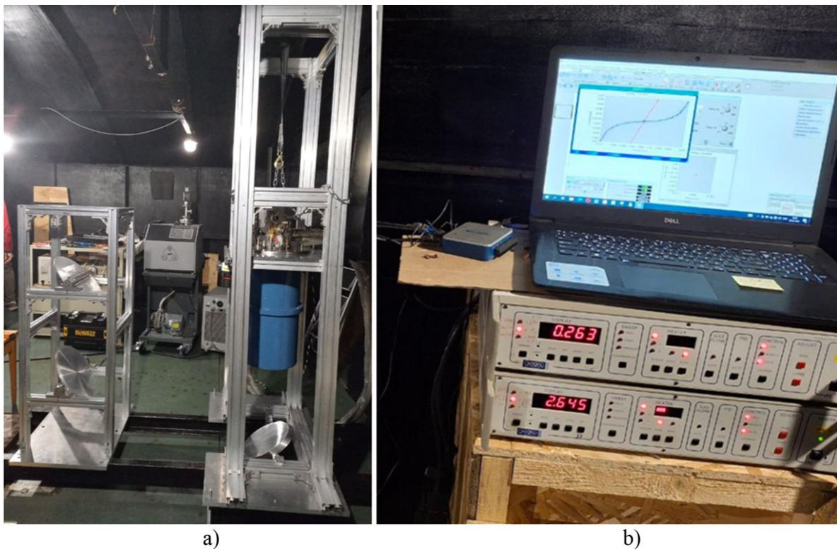
**Figure 8:** Installation and initial testing of the receiving system based on SINIS detectors at the BTA SAO RAS observatory. (a) Installed racks with a Heliox AC-V cryostat and (b) measured  $I$ – $V$  characteristics of the SINIS detector matrix installed inside the cryostat with a closed optical window and under irradiation by the source; The lower part demonstrates a PT2 temperature of 2.6 K and a <sup>3</sup>He pot temperature of 263 mK.
