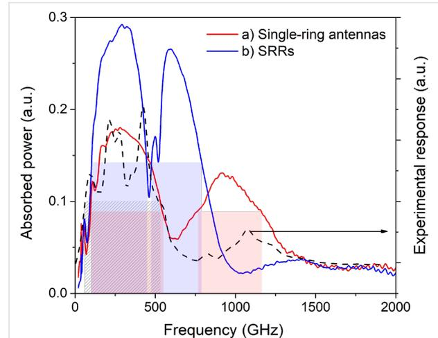
**Figure 2:** Amplitude–frequency characteristics of the metamaterial receiver. (a) 19-element array of single-ring antennas with a lattice period of  $P = 86 \mu\text{m}$  (red curve); (b) 19-element array of SRRs with  $P = 86 \mu\text{m}$  (blue curve). The dashed black curve shows the experimentally measured response of the single-ring metamaterial.
