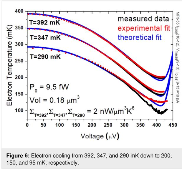
**Figure 6:** Electron cooling from 392, 347, and 290 mK down to 200, 150, and 95 mK, respectively.
