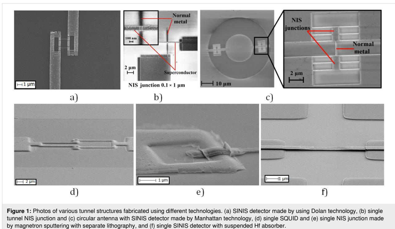
**Figure 1:** Photos of various tunnel structures fabricated using different technologies. (a) SINIS detector made by using Dolan technology, (b) single tunnel NIS junction and (c) circular antenna with SINIS detector made by Manhattan technology, (d) single SQUID and (e) single NIS junction made by magnetron sputtering with separate lithography, and (f) single SINIS detector with suspended Hf absorber.
