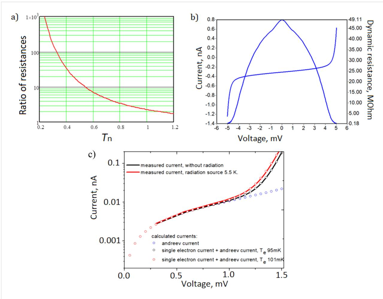
**Figure 4:** (a) Ratio of resistance at zero bias to the asymptotic resistance using Equation 7, obtained from the general relation in Equation 3. (b)  $I$ - $V$  curve and dynamic resistance for the SINIS thermometer. (c) Measured current with and without radiation. The resistance ratio is  $R_d/R_n = 15000$  at 95 mK and does not respond to radiation at 5.5 K.
