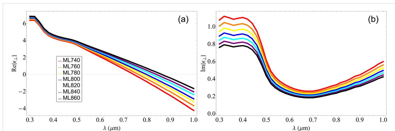
**Figure 2:** (a) Simulated real part of the perpendicular component of the permittivity of the Au/TiO<sub>2</sub> multilayered material having a fixed width of the metallic layer  $d_m = 10$  nm with varying thickness of the dielectric layer. (b) Simulated imaginary part of the perpendicular component of the permittivity of the Au/TiO<sub>2</sub> multilayered material.
