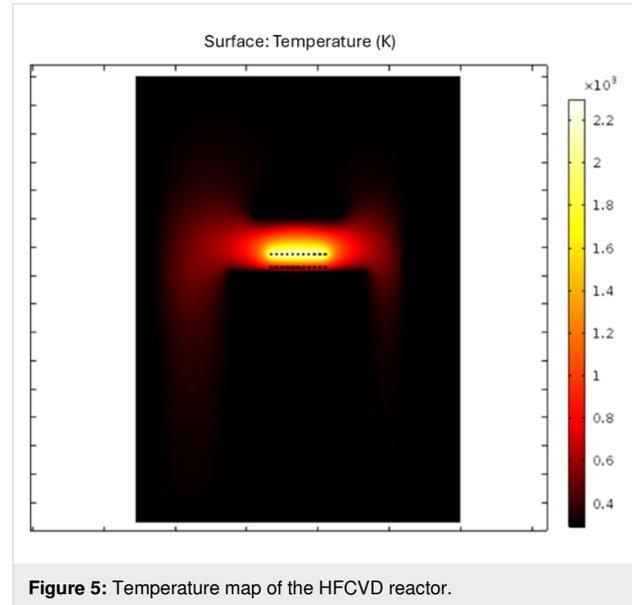
**Figure 5:** Temperature map of the HFCVD reactor.
