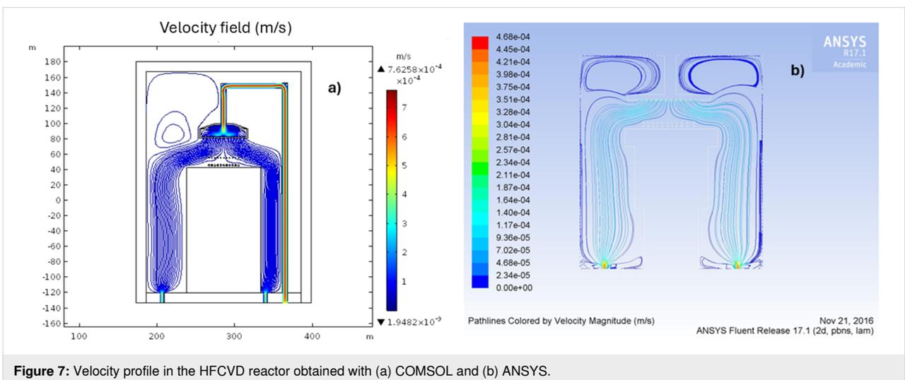
**Figure 7:** Velocity profile in the HFCVD reactor obtained with (a) COMSOL and (b) ANSYS.
