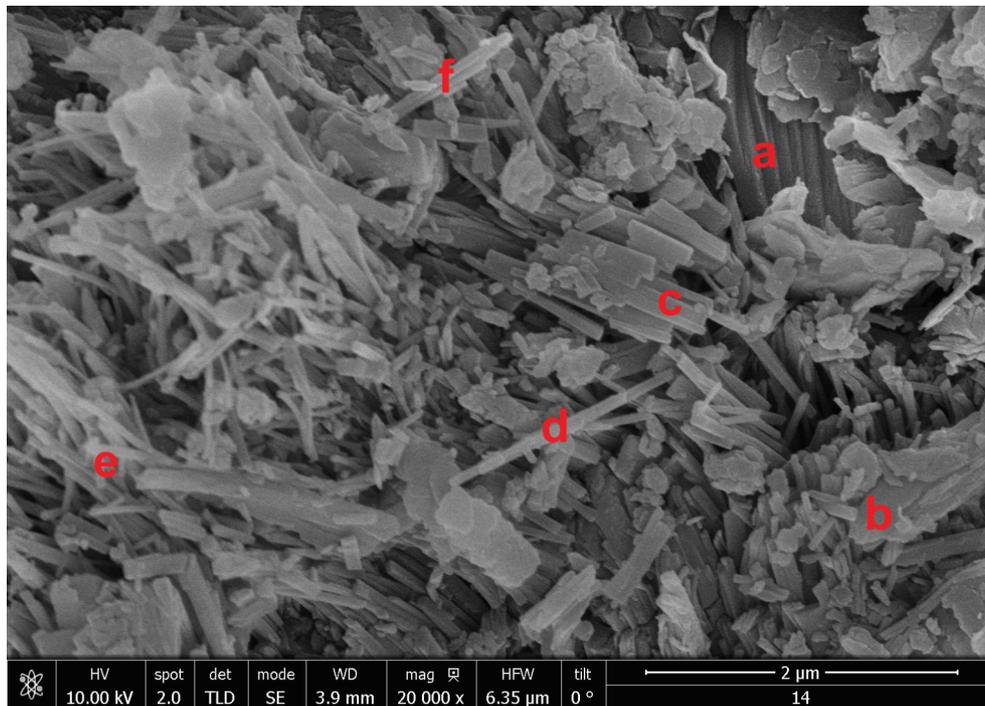
**Figure 2:** SEM micrograph of ZSA from the San Andrés deposit. Some HEU crystals are indicated by a, b, and c, where a and b exhibit tabular characteristics while c has slat morphology. Mordenite crystals, marked by d, e, and f, show acicular to fibrous shapes.
