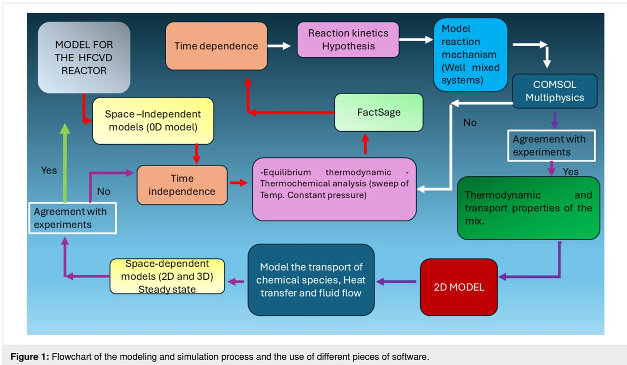
**Figure 1:** Flowchart of the modeling and simulation process and the use of different pieces of software.
