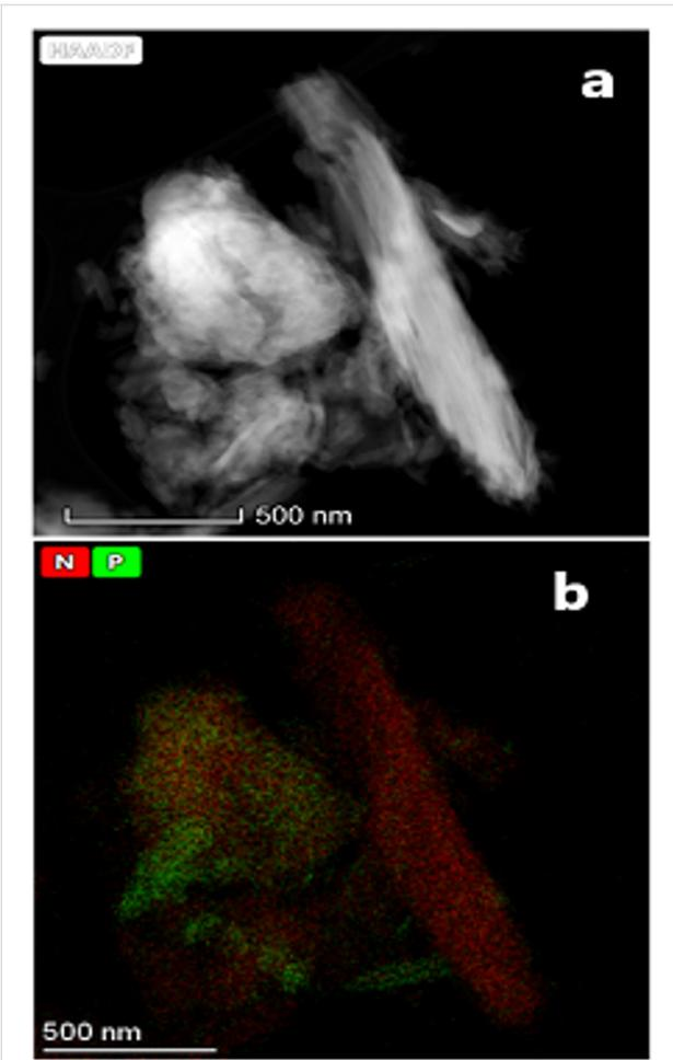
**Figure 7:** STEM micrographs of the CLIM<sub>2-U5M</sub> material (a) showing the combined elemental mapping for nitrogen and phosphorus (b).
