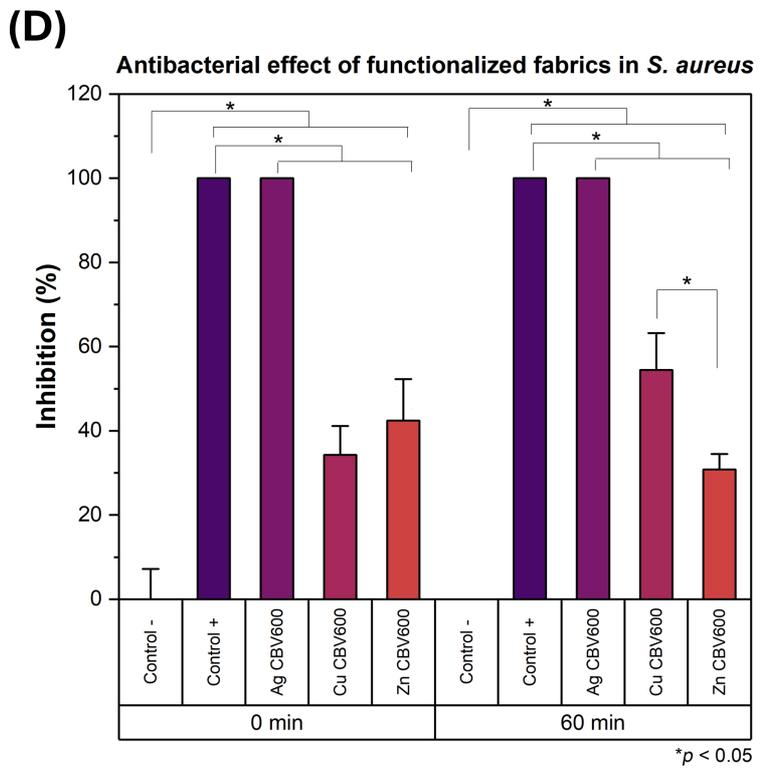
**Figure 4:** (A) *E. coli* growth on LB agar plates on fabrics exposed to 0 and 60 min of sunlight. (B) Inhibition of *E. coli* growth on fabrics after 0 and 60 min of exposure to sunlight. (C) *S. aureus* growth on LB agar plates on fabrics exposed to 0 and 60 min of sunlight. (D) Inhibition of *S. aureus* growth on fabrics after 0 and 60 min of exposure to sunlight. The asterisk (\*) indicates  $p < 0.05$ .
