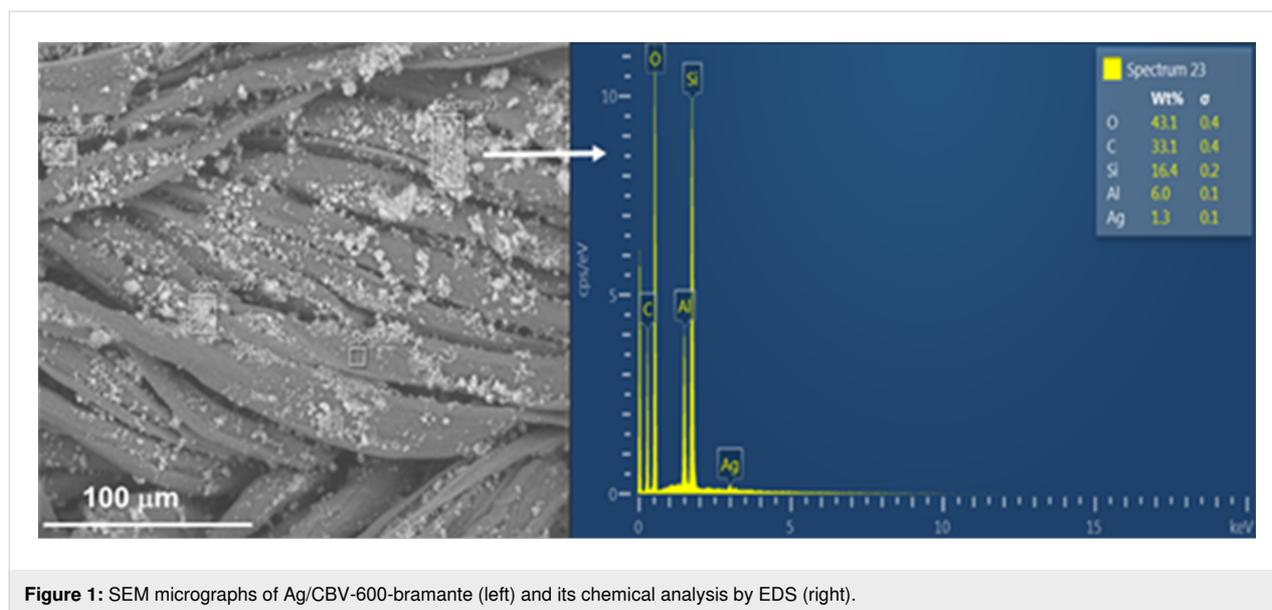
**Figure 1:** SEM micrographs of Ag/CBV-600-bramante (left) and its chemical analysis by EDS (right).
