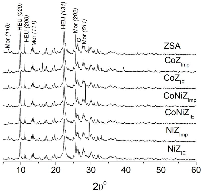
**Figure 1:** XRD pattern of the starting zeolite mineral (ZSA) and the materials obtained through traditional ion exchange (IE) and impregnation (Imp) methods. The Miller indexes (*hkl*) corresponding to the zeolite phases are shown in the pattern of the ZSA. Mor, HEU, and Q are associated to the phases of mordenite, clinoptilolite–heulandite, and quartz, respectively.
