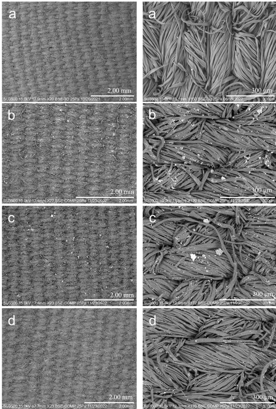
**Figure 2:** SEM micrographs of the samples. (Left column) Panoramic view and (right column) zoomed view. (a) Bramante fabric, (b) Ag/CBV-600-bramante, (c) Cu/CBV-600-bramante, and (d) Zn/CBV-600-bramante.
