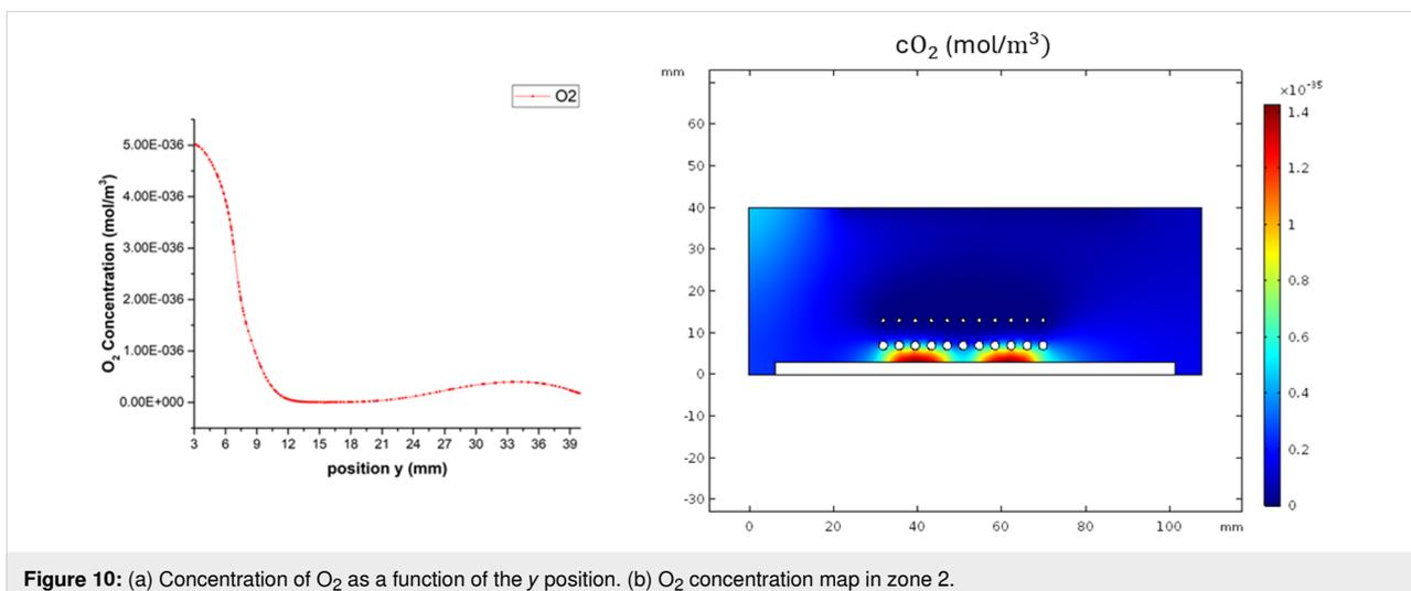
**Figure 10:** (a) Concentration of O<sub>2</sub> as a function of the y position. (b) O<sub>2</sub> concentration map in zone 2.
