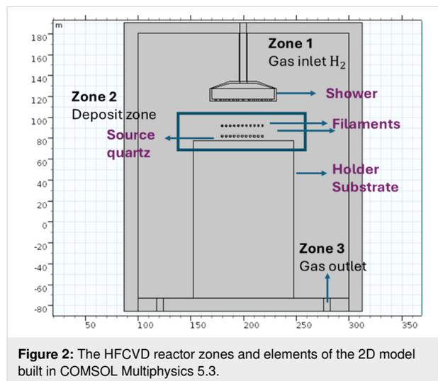
**Figure 2:** The HFCVD reactor zones and elements of the 2D model built in COMSOL Multiphysics 5.3.
