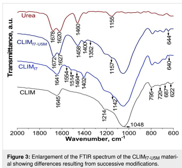
**Figure 3:** Enlargement of the FTIR spectrum of the CLIM<sub>f7-U5M</sub> material showing differences resulting from successive modifications.
