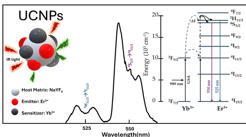
**Figure 1:** Characteristic UC fluorescent emission spectra of  $\text{NaYF}_4:\text{Er}^{3+}/\text{Yb}^{3+}$  in the green region when irradiated with 980 nm laser light. Insets: UC process scheme (right). Schematic representation of the energy transfer between  $\text{Yb}^{3+}$  and  $\text{Er}^{3+}$  ions and the UC emission in an upconversion nanoparticle UCNP (left).
