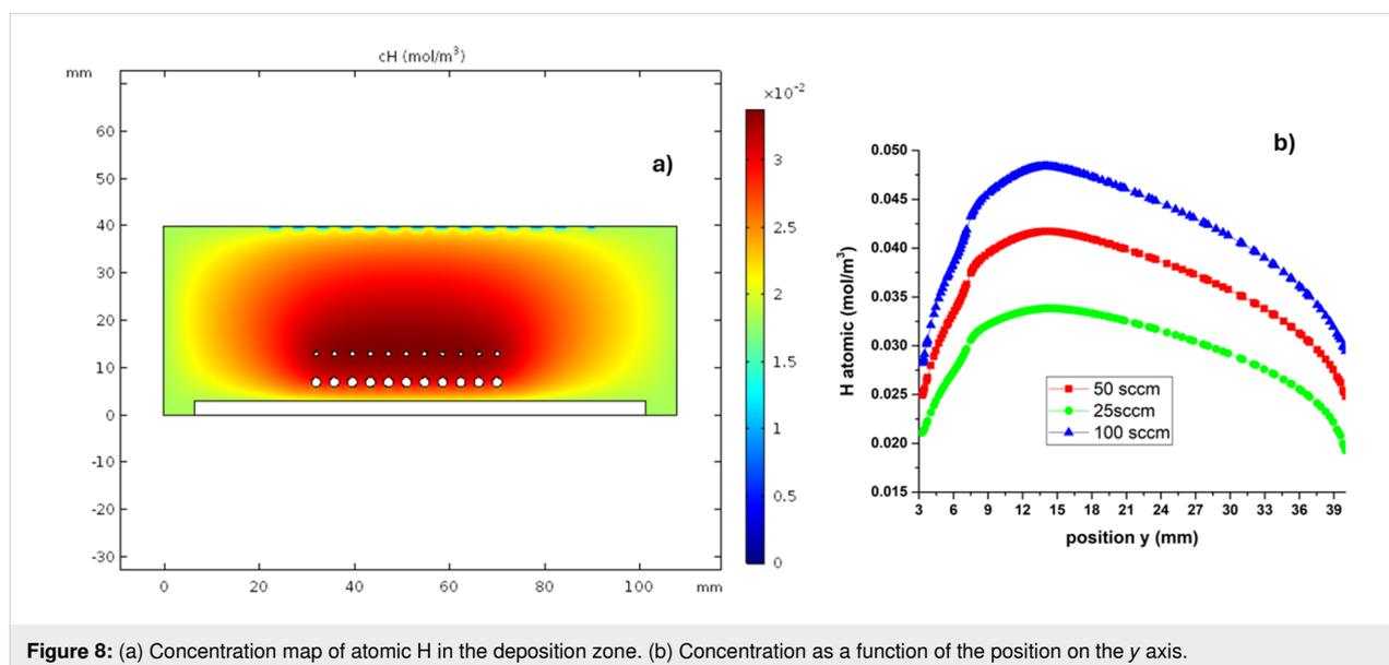
**Figure 8:** (a) Concentration map of atomic H in the deposition zone. (b) Concentration as a function of the position on the  $y$  axis.
