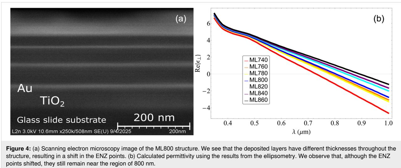
**Figure 4:** (a) Scanning electron microscopy image of the ML800 structure. We see that the deposited layers have different thicknesses throughout the structure, resulting in a shift in the ENZ points. (b) Calculated permittivity using the results from the ellipsometry. We observe that, although the ENZ points shifted, they still remain near the region of 800 nm.
