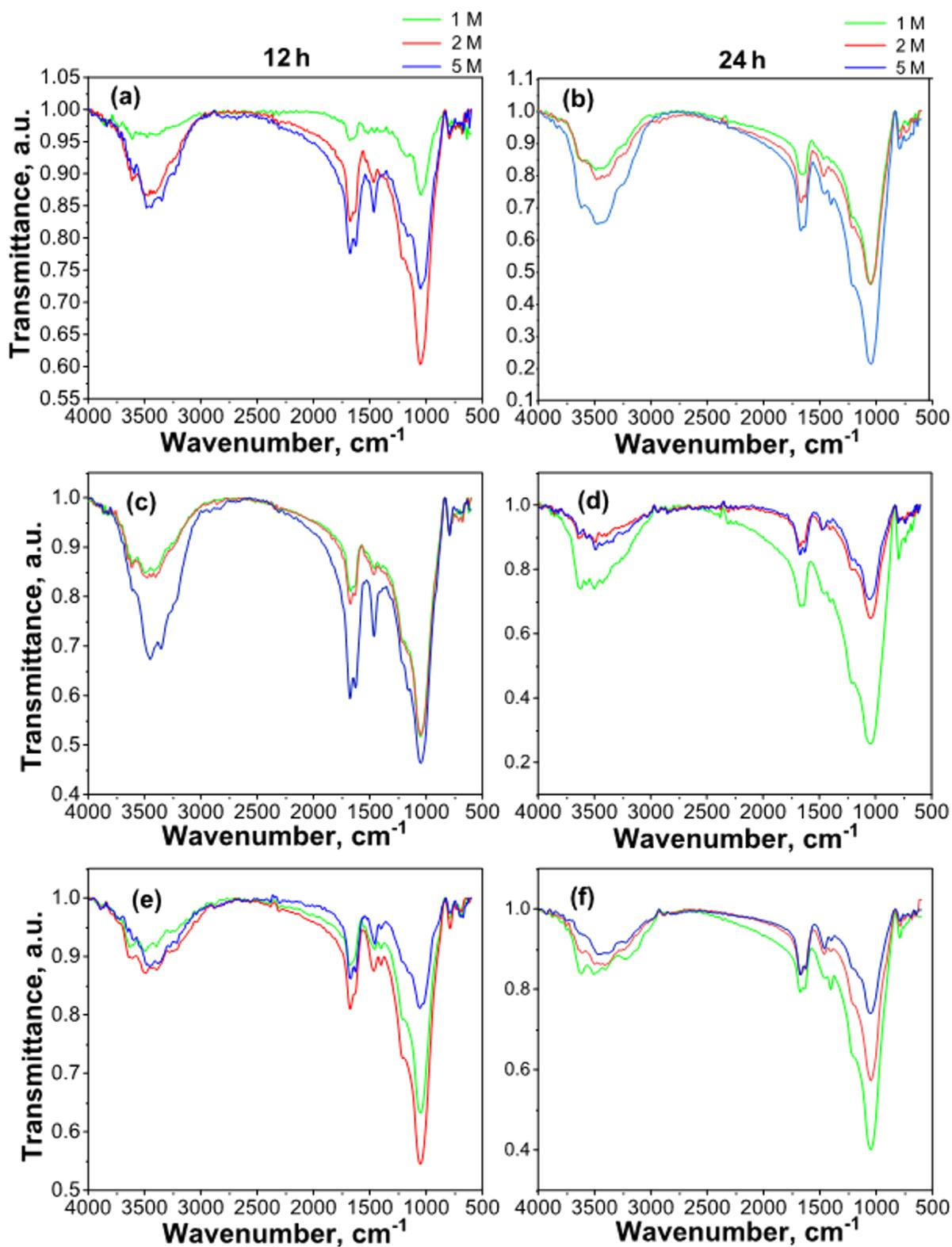
**Figure 2:** FTIR spectra of CLIM<sub>F-U</sub> materials obtained from CLIM consecutively modified with DAP and urea solutions at different concentrations (1, 2, and 5 M) for contact times of 12 and 24 h: (a, b) with 2% DAP, (c, d) with 3.5% DAP, and (e, f) with 7% DAP.
