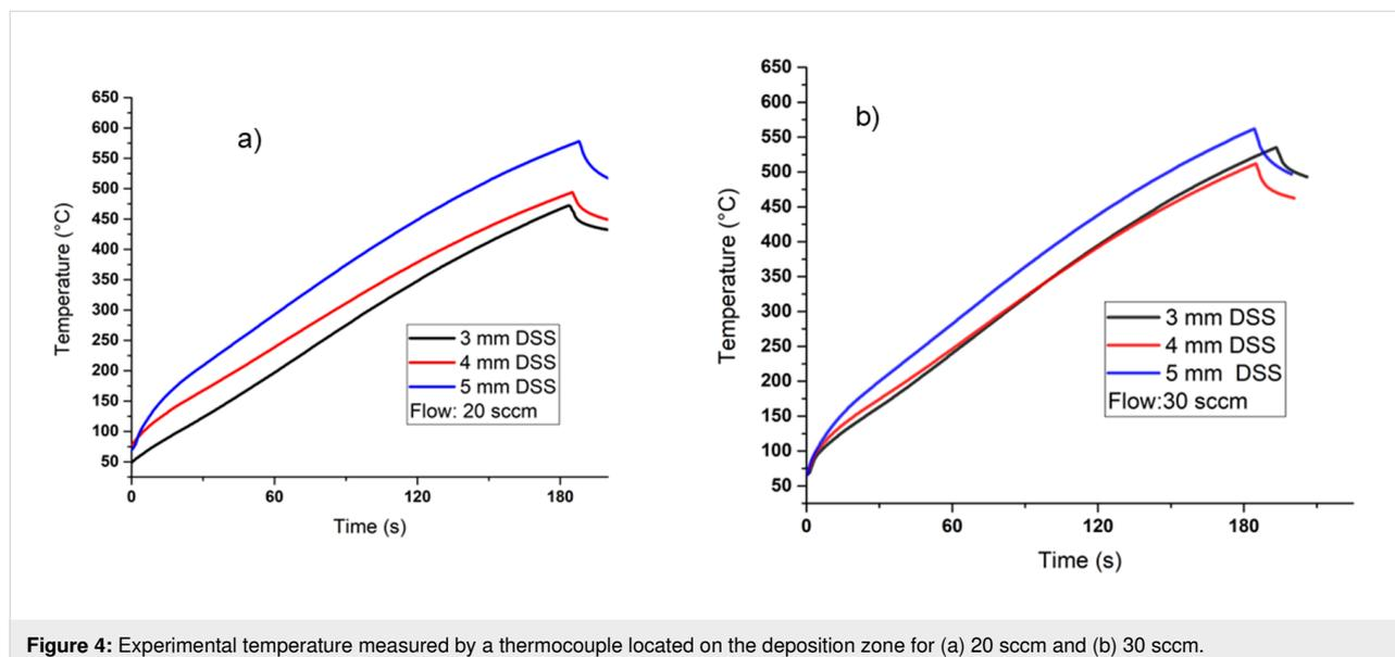
**Figure 4:** Experimental temperature measured by a thermocouple located on the deposition zone for (a) 20 sccm and (b) 30 sccm.
