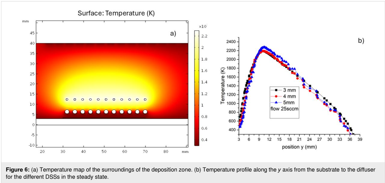
**Figure 6:** (a) Temperature map of the surroundings of the deposition zone. (b) Temperature profile along the  $y$  axis from the substrate to the diffuser for the different DSSs in the steady state.
