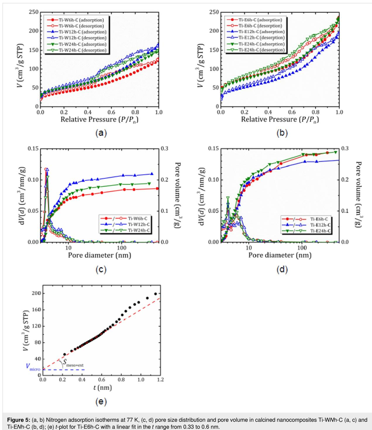
**Figure 5:** (a, b) Nitrogen adsorption isotherms at 77 K, (c, d) pore size distribution and pore volume in calcined nanocomposites Ti-WNh-C (a, c) and Ti-ENh-C (b, d); (e)  $t$ -plot for Ti-E6h-C with a linear fit in the  $t$  range from 0.33 to 0.6 nm.
