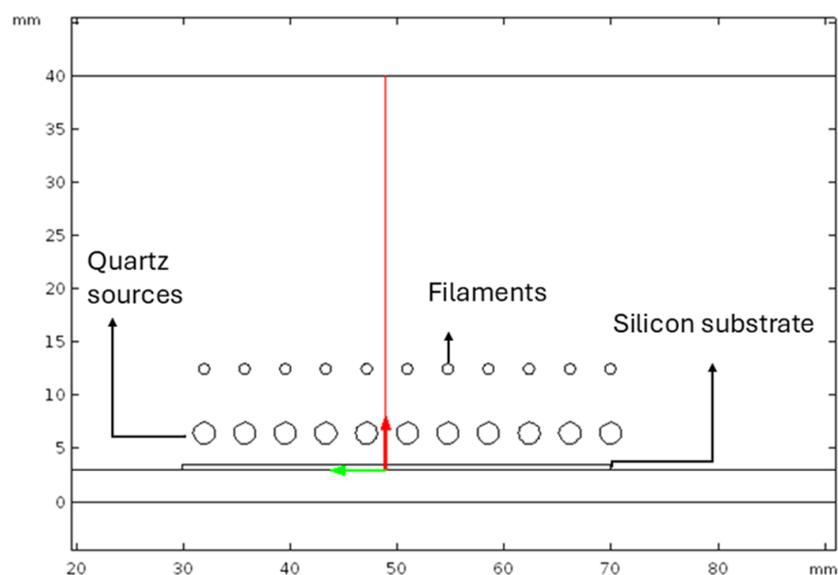
**Figure 3:** The red line along the  $y$  direction in the deposition area (zone 2) built in COSMOL Multiphysics.
