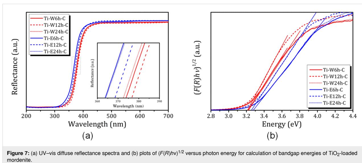
**Figure 7:** (a) UV–vis diffuse reflectance spectra and (b) plots of  $(F(R)hv)^{1/2}$  versus photon energy for calculation of bandgap energies of TiO<sub>2</sub>-loaded mordenite.
