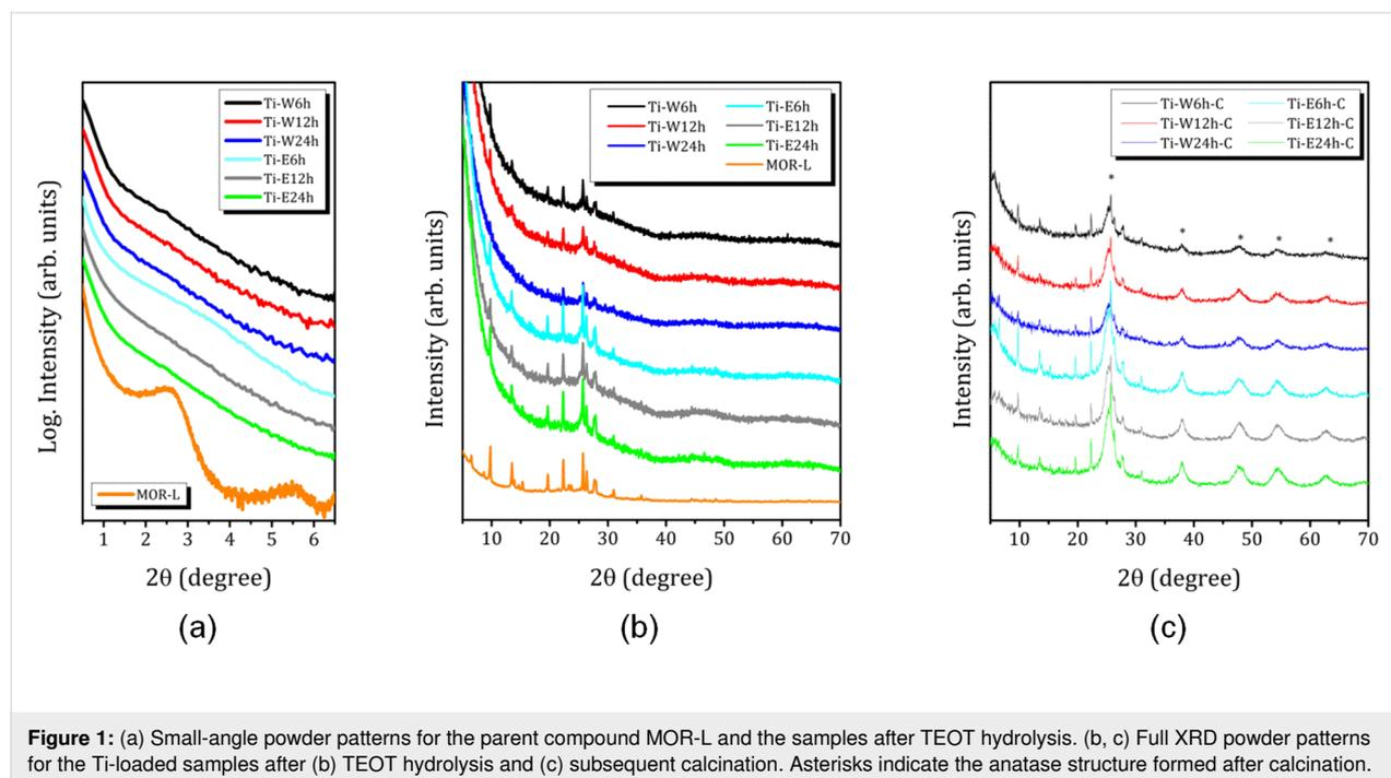
**Figure 1:** (a) Small-angle powder patterns for the parent compound MOR-L and the samples after TEOT hydrolysis. (b, c) Full XRD powder patterns for the Ti-loaded samples after (b) TEOT hydrolysis and (c) subsequent calcination. Asterisks indicate the anatase structure formed after calcination.
