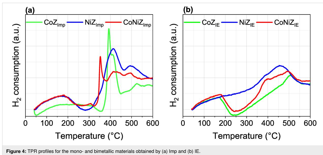
**Figure 4:** TPR profiles for the mono- and bimetallic materials obtained by (a) Imp and (b) IE.
