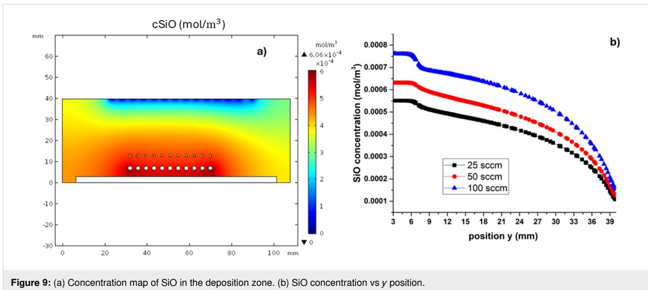
**Figure 9:** (a) Concentration map of SiO in the deposition zone. (b) SiO concentration vs y position.
