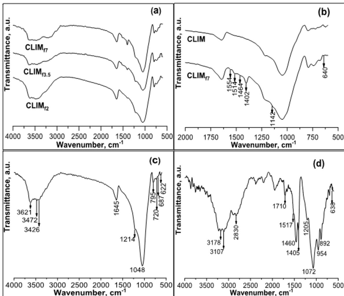
**Figure 1:** FTIR spectra of modified samples (CLIM<sub>f</sub>) and raw material (CLIM). (a) CLIM<sub>f</sub> obtained as a result of modification using different amounts of DAP (2.0%, 3.5% and 7.0% corresponding to CLIM<sub>f2</sub>, CLIM<sub>f3.5</sub> and CLIM<sub>f7</sub>, respectively). (b) Magnification in the range from 600 to 2000 cm<sup>-1</sup> for spectrum “CLIM<sub>f7</sub>” of Figure 1a compared to CLIM. (c) CLIM. (d) DAP.
