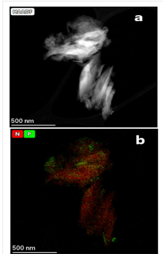
**Figure 8:** STEM micrographs of CLIM<sub>3.5-U5M</sub> material (a) showing the combined elemental mapping for nitrogen and phosphorus (b).
