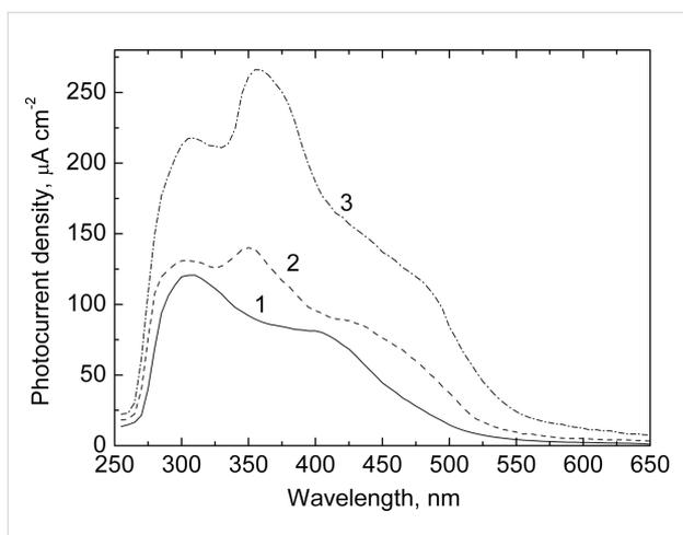
**Figure 9:** Photocurrent spectra of  $\text{In}_2\text{O}_3(400)/\text{CdS}$  film electrodes in  $0.1 \text{ M Na}_2\text{S} + 0.1 \text{ M Na}_2\text{SO}_3 + 0.1 \text{ M NaOH}$  solution. The spectra were measured at a potential of  $-0.1 \text{ V}$  versus  $\text{Ag}/\text{AgCl}$ . The number of the SILAR cycles of CdS deposition was 10 (1), 30 (2) and 50 (3).
