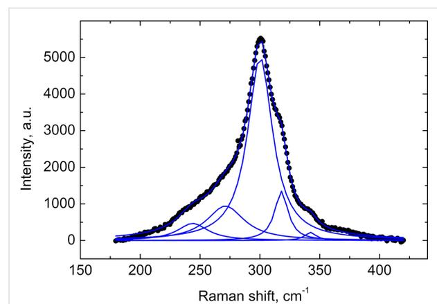
**Figure 5:** Raman spectrum of the  $\text{In}_2\text{O}_3(400)/\text{CdS}$  system prepared by using 40 SILAR cycles of CdS deposition after background subtraction (circles) and its fitting by the superposition of five Lorentz lines.
