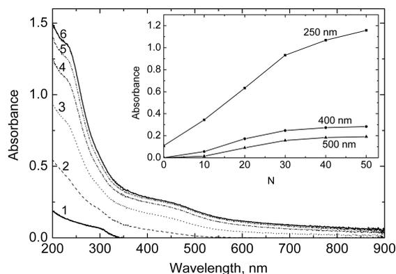
**Figure 4:** Absorption spectra of the In<sub>2</sub>O<sub>3</sub>(400) and In<sub>2</sub>O<sub>3</sub>(400)/CdS films deposited onto a quartz substrate. The number of SILAR cycles of the CdS deposition are as follows: 0 (1); 10 (2); 20 (3); 30 (4); 40 (5); 50 (6). The inset shows the dependencies of the absorbance at different wavelengths on the number of SILAR cycles.
