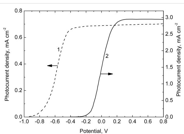
**Figure 7:** Photocurrent versus electrode-potential curves recorded under UV illumination of the mesoporous  $\text{In}_2\text{O}_3$  electrodes annealed at 200 °C (1) and 400 °C (2). Electrolyte: 0.1 M KOH solution.
