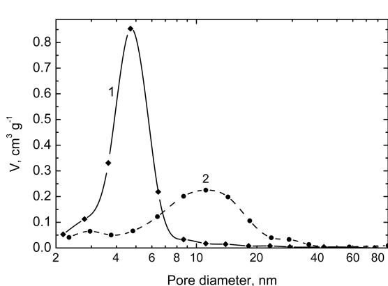
**Figure 3:** Barrett–Joyner–Halenda desorption-model pore-volume distribution of the  $\text{In}_2\text{O}_3(400)$  mesoporous films prepared with (1) and without (2) Pluronic F127.
