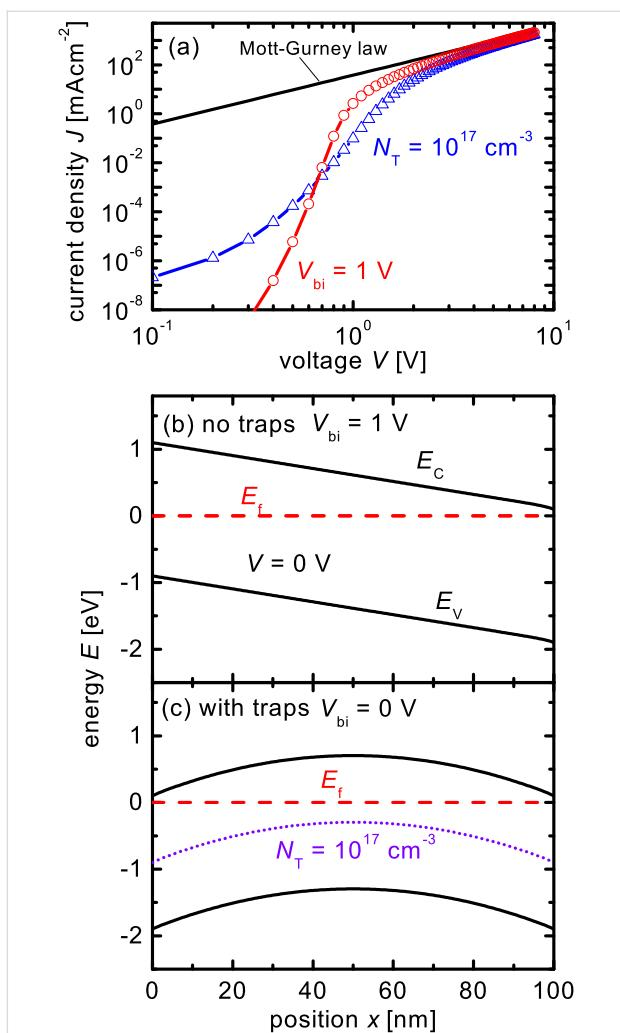
**Figure 2:** (a) Current–voltage curves of a device with charged acceptor-like defects and a built-in voltage  $V_{bi} = 0$  V (as in Figure 1a) and a device with no defects but a built-in voltage  $V_{bi} = 1$  V are compared to the Mott–Gurney law (Equation 1). Band diagram of the device (b) without charged defects and  $V_{bi} = 1$  V and (c) with charged defects and  $V_{bi} = 0$  V. Both band diagrams are depicted at short circuit.
