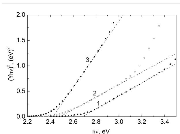
**Figure 10:** Analysis of the photocurrent spectra shown in Figure 9 in coordinates of  $(Y \cdot hv)^2$  versus  $hv$  typical for direct optical transitions for  $\text{In}_2\text{O}_3(400)/\text{CdS}$  film electrodes. The number of the SILAR cycles of CdS deposition was 10 (1), 30 (2) and 50 (3).
