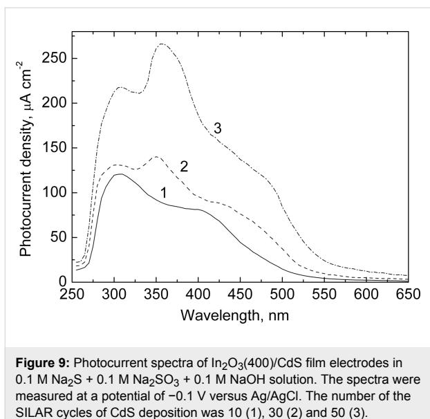
**Figure 9:** Photocurrent spectra of  $\text{In}_2\text{O}_3(400)/\text{CdS}$  film electrodes in  $0.1 \text{ M Na}_2\text{S} + 0.1 \text{ M Na}_2\text{SO}_3 + 0.1 \text{ M NaOH}$  solution. The spectra were measured at a potential of  $-0.1 \text{ V}$  versus  $\text{Ag}/\text{AgCl}$ . The number of the SILAR cycles of CdS deposition was 10 (1), 30 (2) and 50 (3).
