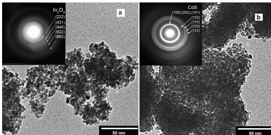
**Figure 1:** TEM images and electron diffraction patterns (insets) for In<sub>2</sub>O<sub>3</sub>(400) (a) and In<sub>2</sub>O<sub>3</sub>(400) after 30 SILAR CdS deposition cycles (b).
