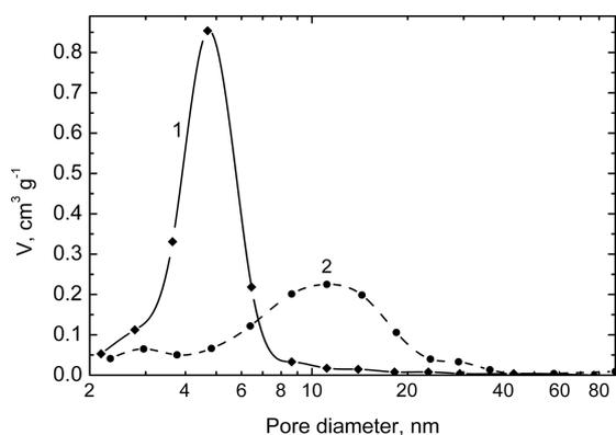
**Figure 3:** Barrett–Joyner–Halenda desorption-model pore-volume distribution of the In<sub>2</sub>O<sub>3</sub>(400) mesoporous films prepared with (1) and without (2) Pluronic F127.
