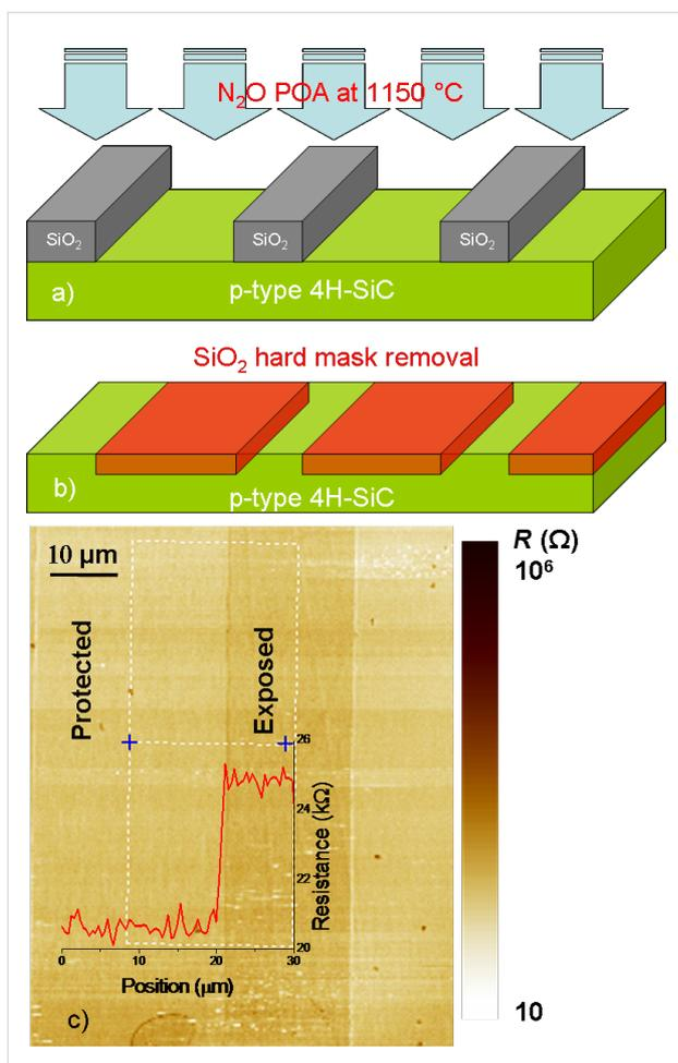
**Figure 1:** Schematic description of the POA treatment. (a) A SiO<sub>2</sub> hard mask is used to protect selectively the 4H-SiC during the POA. (b) After removal of the hard mask (by HF wet etch) on the 4H-SiC surface there are regions protected and exposed to the POA. (c) SSRM imaged on the patterned SiC surface; the two dimensional map of the substrate surface. The resistance line profile going from protected to exposed strips demonstrates a higher resistance value in the exposed region.
