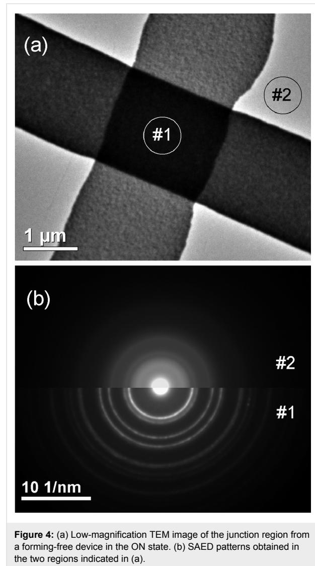
**Figure 4:** (a) Low-magnification TEM image of the junction region from a forming-free device in the ON state. (b) SAED patterns obtained in the two regions indicated in (a).
