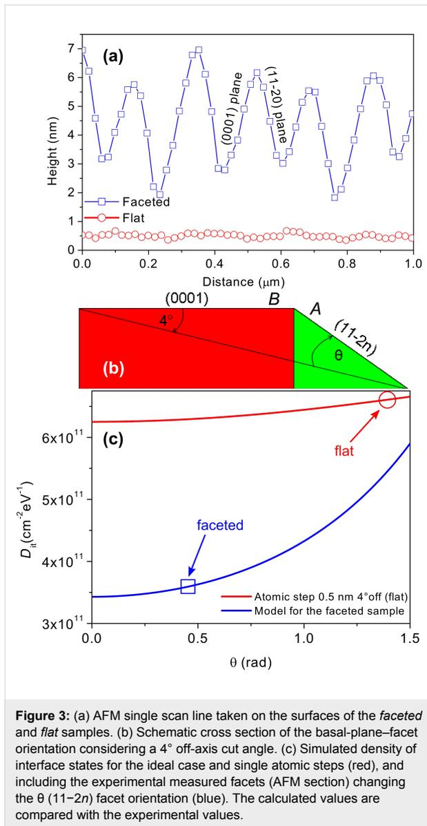
In fact, for our MOS capacitors fabricated on a faceted surface as in Figure 3a, a significant fraction of the total SiO<sub>2</sub>/4H-SiC interface area is formed on (11–2n) planes, with lower  $D_{it}$  than the basal plane (0001). This latter can justify the reduced  $D_{it}$  in the faceted sample.
