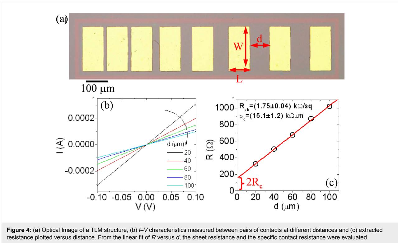
resistance  $R$ , obtained from the slope of each curve, is plotted versus the contact distance. According to the TLM theory [24],  $R$  is related to the metal/graphene contact resistance  $R_c$  and to the graphene sheet resistance  $R_{sh}$  according to the relation
