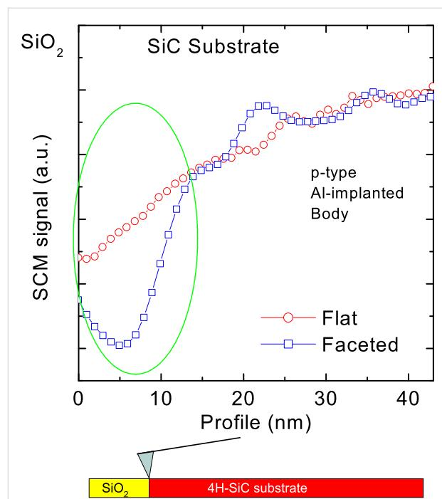
**Figure 2:** SCM profiling across the SiO<sub>2</sub>/4H-SiC interfaces on the *faceted* (blue squares) and *flat* (red circles) samples respectively.
