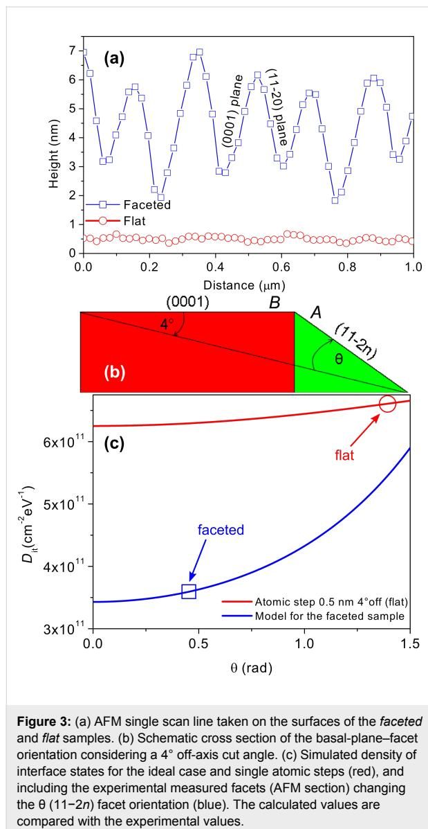
In fact, for our MOS capacitors fabricated on a faceted surface as in Figure 3a, a significant fraction of the total  $\text{SiO}_2/4\text{H-SiC}$  interface area is formed on (11–2n) planes, with lower  $D_{it}$  than the basal plane (0001). This latter can justify the reduced  $D_{it}$  in the faceted sample.
