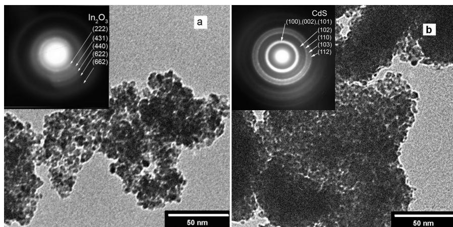
**Figure 1:** TEM images and electron diffraction patterns (insets) for  $\text{In}_2\text{O}_3(400)$  (a) and  $\text{In}_2\text{O}_3(400)$  after 30 SILAR CdS deposition cycles (b).
