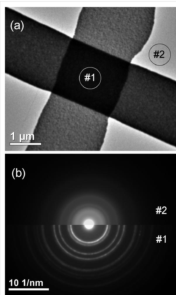
**Figure 4:** (a) Low-magnification TEM image of the junction region from a forming-free device in the ON state. (b) SAED patterns obtained in the two regions indicated in (a).
