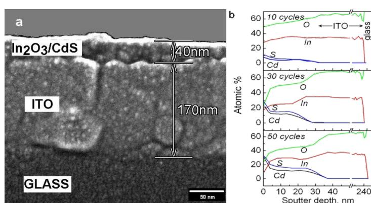
**Figure 2:** Cross-sectional SEM image of the  $\text{In}_2\text{O}_3(400)$  film after 30 SILAR CdS deposition cycles (a) and AES profiles for  $\text{In}_2\text{O}_3(400)/\text{CdS}$  structures with different numbers of SILAR cycles (b). Scaling from sputter time to depth in AES profiles was done on the basis of cross-sectional SEM data.
