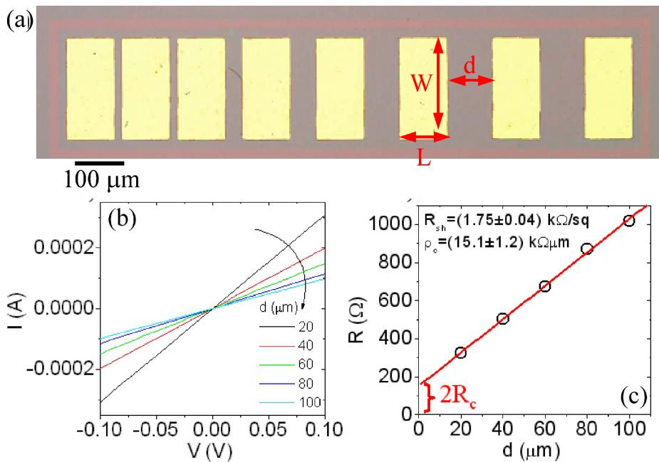
**Figure 4:** (a) Optical Image of a TLM structure, (b)  $I$ - $V$  characteristics measured between pairs of contacts at different distances and (c) extracted resistance plotted versus distance. From the linear fit of  $R$  versus  $d$ , the sheet resistance and the specific contact resistance were evaluated.
