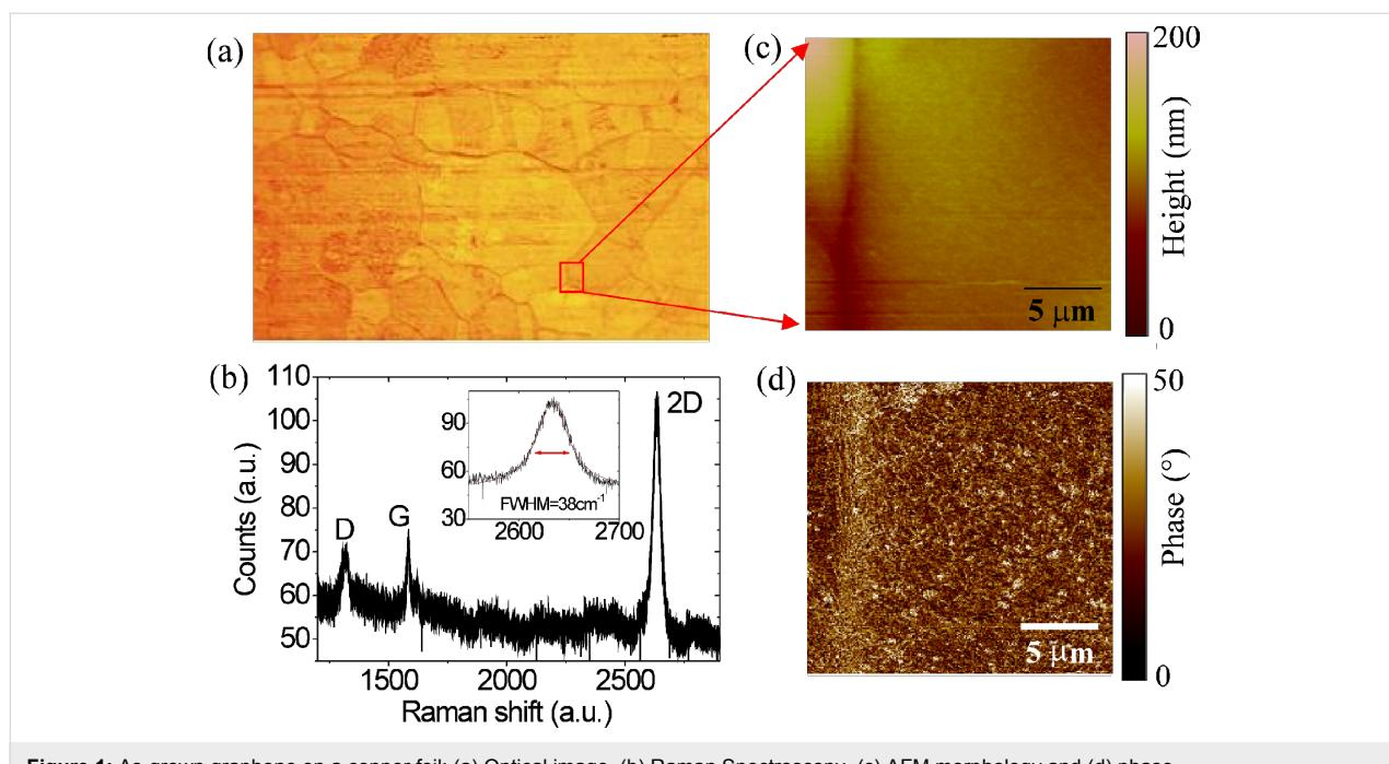
Figure 1: As-grown graphene on a copper foil: (a) Optical image, (b) Raman Spectroscopy, (c) AFM morphology and (d) phase.
