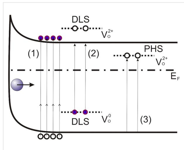
**Figure 6:** Schematic energy-level diagram of ZnO taking into account the existence of theoretically predicted [42]  $\alpha$ - and  $\beta$ -type configurations of oxygen vacancies. The processes of electron–hole pair generation via band-to-band absorption, charge carrier photoexcitation from a defect localized state (DLS) and to a perturbed host state (PHS) of an oxygen vacancy are marked as (1), (2) and (3), respectively.
