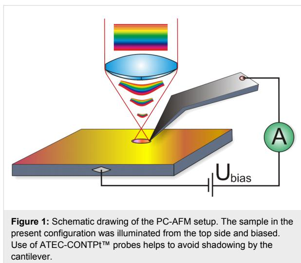
**Figure 1:** Schematic drawing of the PC-AFM setup. The sample in the present configuration was illuminated from the top side and biased. Use of ATEC-CONTPT™ probes helps to avoid shadowing by the cantilever.
