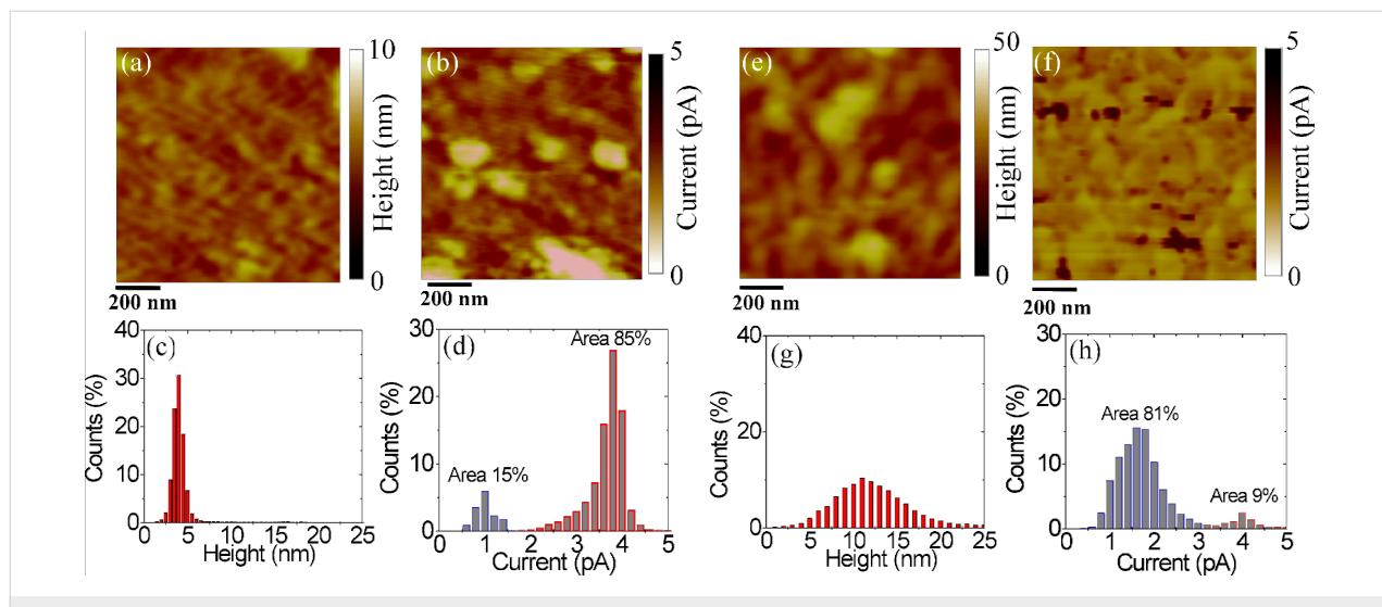
**Figure 6:** TRCAFM of Graphene on  $\text{SiO}_2$ : (a) morphology and (c) the related histogram, (b) current map and (d) the related histogram. TRCAFM of Graphene on PEN: (a) morphology and (c) the related histogram, (b) current map and (d) the related histogram.
