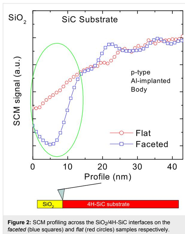
**Figure 2:** SCM profiling across the SiO<sub>2</sub>/4H-SiC interfaces on the *faceted* (blue squares) and *flat* (red circles) samples respectively.
