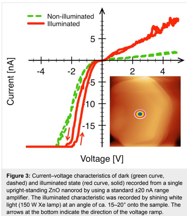
Both, illuminated and dark characteristics demonstrate rectifying behavior with a rather significant deviation of the reverse current from the zero level. Moreover, the reverse current in both cases demonstrates a linear dependence on the applied voltage, which can be attributed to the photoexcitation of charge carriers from the valence band to a defect-perturbed host state
