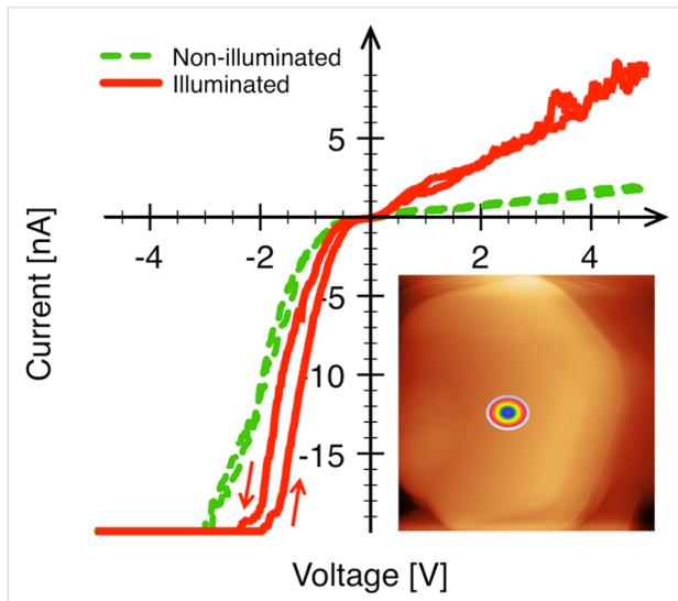
**Figure 3:** Current–voltage characteristics of dark (green curve, dashed) and illuminated state (red curve, solid) recorded from a single upright-standing ZnO nanorod by using a standard  $\pm 20$  nA range amplifier. The illuminated characteristic was recorded by shining white light (150 W Xe lamp) at an angle of ca.  $15$ – $20$ ° onto the sample. The arrows at the bottom indicate the direction of the voltage ramp.
