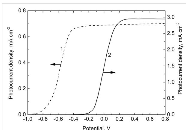
**Figure 7:** Photocurrent versus electrode-potential curves recorded under UV illumination of the mesoporous  $\text{In}_2\text{O}_3$  electrodes annealed at 200 °C (1) and 400 °C (2). Electrolyte: 0.1 M KOH solution.
