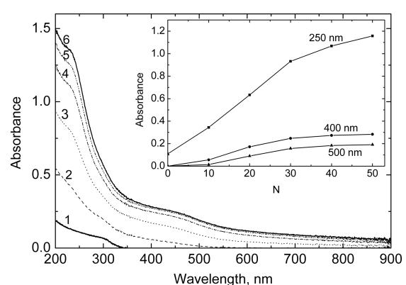
**Figure 4:** Absorption spectra of the  $\text{In}_2\text{O}_3(400)$  and  $\text{In}_2\text{O}_3(400)/\text{CdS}$  films deposited onto a quartz substrate. The number of SILAR cycles of the CdS deposition are as follows: 0 (1); 10 (2); 20 (3); 30 (4); 40 (5); 50 (6). The inset shows the dependencies of the absorbance at different wavelengths on the number of SILAR cycles.
