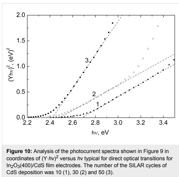
**Figure 10:** Analysis of the photocurrent spectra shown in Figure 9 in coordinates of  $(Y \cdot h\nu)^2$  versus  $h\nu$  typical for direct optical transitions for  $\text{In}_2\text{O}_3(400)/\text{CdS}$  film electrodes. The number of the SILAR cycles of CdS deposition was 10 (1), 30 (2) and 50 (3).
