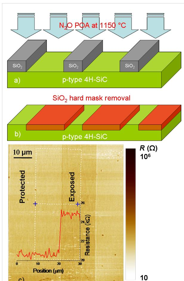
**Figure 1:** Schematic description of the POA treatment. (a) A SiO<sub>2</sub> hard mask is used to protect selectively the 4H-SiC during the POA. (b) After removal of the hard mask (by HF wet etch) on the 4H-SiC surface there are regions protected and exposed to the POA. (c) SSRM imaged on the patterned SiC surface; the two dimensional map of the substrate surface. The resistance line profile going from protected to exposed strips demonstrates a higher resistance value in the exposed region.
