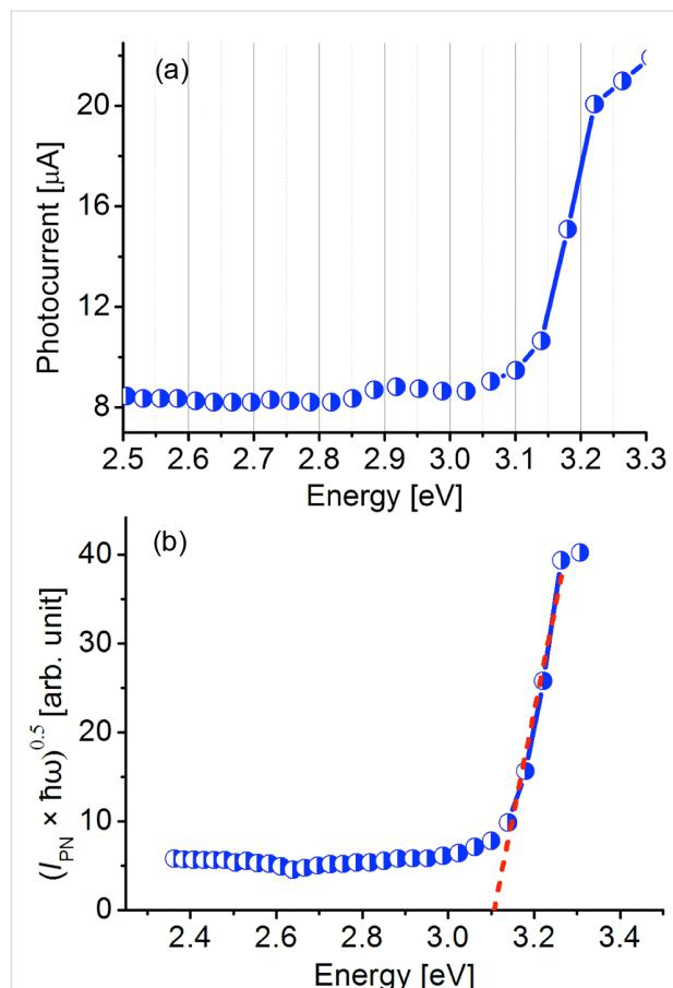
**Figure 5:** (a) The photoconductivity spectral response from a single upright standing ZnO NR recorded using a  $150$  W Xe lamp connected to the monochromator. The sample bias was  $-10$  V. (b) The quantum efficiency of light conversion linearized in coordinates  $(I_{PN}\hbar\omega)^{0.5}$  versus  $\hbar\omega$ . The dashed line represents extrapolation of the linearized region until the intersection with the x-axis.
