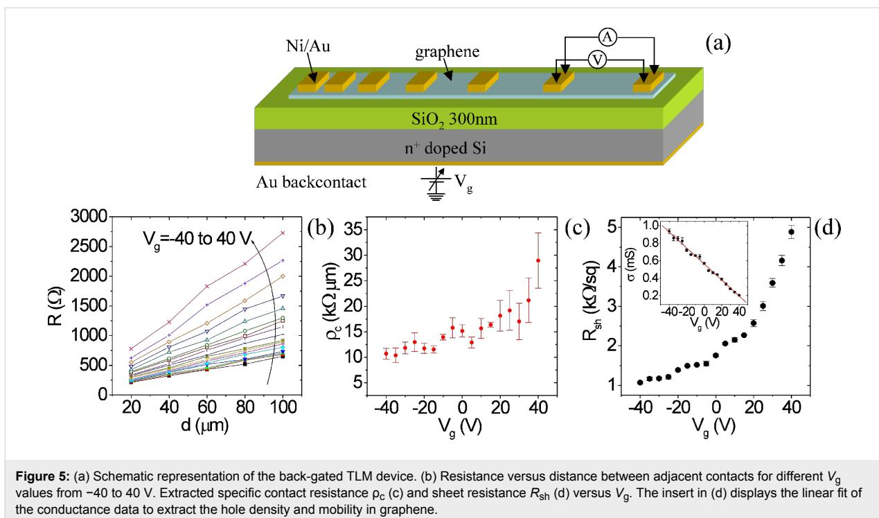
**Figure 5:** (a) Schematic representation of the back-gated TLM device. (b) Resistance versus distance between adjacent contacts for different  $V_g$  values from  $-40$  to  $40$  V. Extracted specific contact resistance  $\rho_c$  (c) and sheet resistance  $R_{sh}$  (d) versus  $V_g$ . The insert in (d) displays the linear fit of the conductance data to extract the hole density and mobility in graphene.
