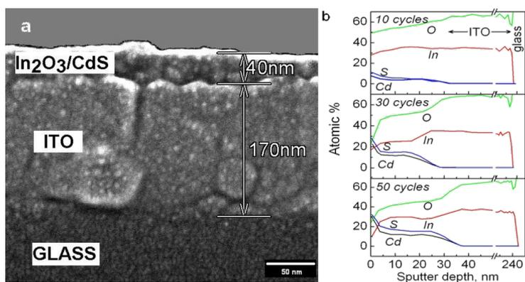
**Figure 2:** Cross-sectional SEM image of the In<sub>2</sub>O<sub>3</sub>(400) film after 30 SILAR CdS deposition cycles (a) and AES profiles for In<sub>2</sub>O<sub>3</sub>(400)/CdS structures with different numbers of SILAR cycles (b). Scaling from sputter time to depth in AES profiles was done on the basis of cross-sectional SEM data.
