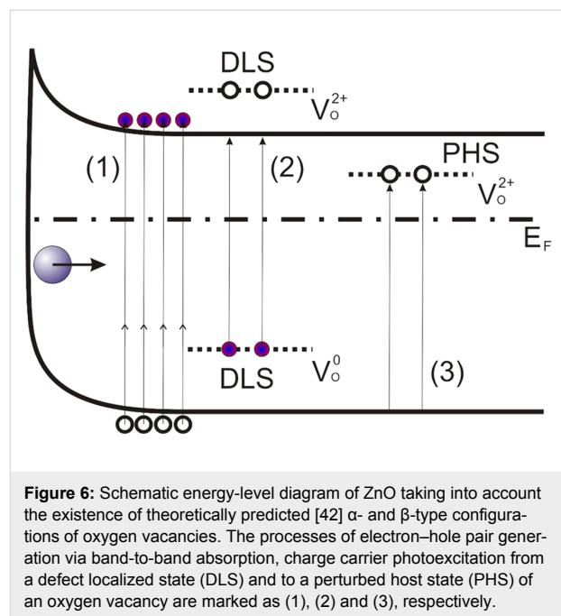
**Figure 6:** Schematic energy-level diagram of ZnO taking into account the existence of theoretically predicted [42]  $\alpha$ - and  $\beta$ -type configurations of oxygen vacancies. The processes of electron–hole pair generation via band-to-band absorption, charge carrier photoexcitation from a defect localized state (DLS) and to a perturbed host state (PHS) of an oxygen vacancy are marked as (1), (2) and (3), respectively.
