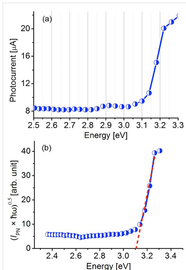
**Figure 5:** (a) The photoconductivity spectral response from a single upright standing ZnO NR recorded using a 150 W Xe lamp connected to the monochromator. The sample bias was  $-10$  V. (b) The quantum efficiency of light conversion linearized in coordinates  $(I_{PN}\hbar\omega)^{0.5}$  versus  $\hbar\omega$ . The dashed line represents extrapolation of the linearized region until the intersection with the x-axis.
