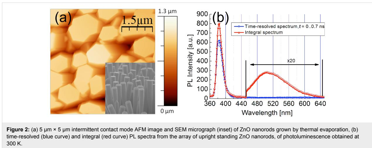
**Figure 2:** (a)  $5\text{ }\mu\text{m} \times 5\text{ }\mu\text{m}$  intermittent contact mode AFM image and SEM micrograph (inset) of ZnO nanorods grown by thermal evaporation, (b) time-resolved (blue curve) and integral (red curve) PL spectra from the array of upright standing ZnO nanorods, of photoluminescence obtained at 300 K.
