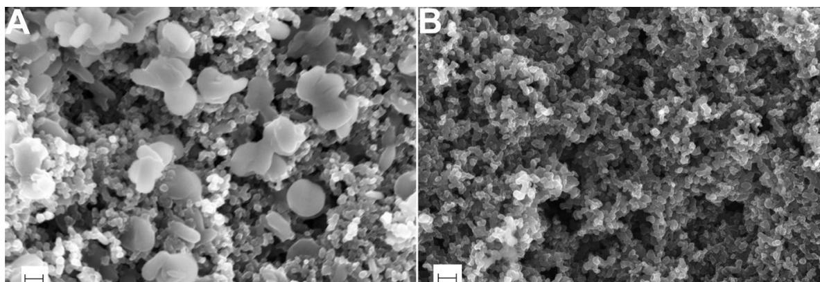
**Figure 6:** Microstructures of (A) discharged and (B) recharged electrodes. The formation of lithium peroxide crystals on the discharged electrode up to 1000 mAh·(g carbon)<sup>−1</sup> is clearly visible in (A). The scale bars correspond to 200 nm.
