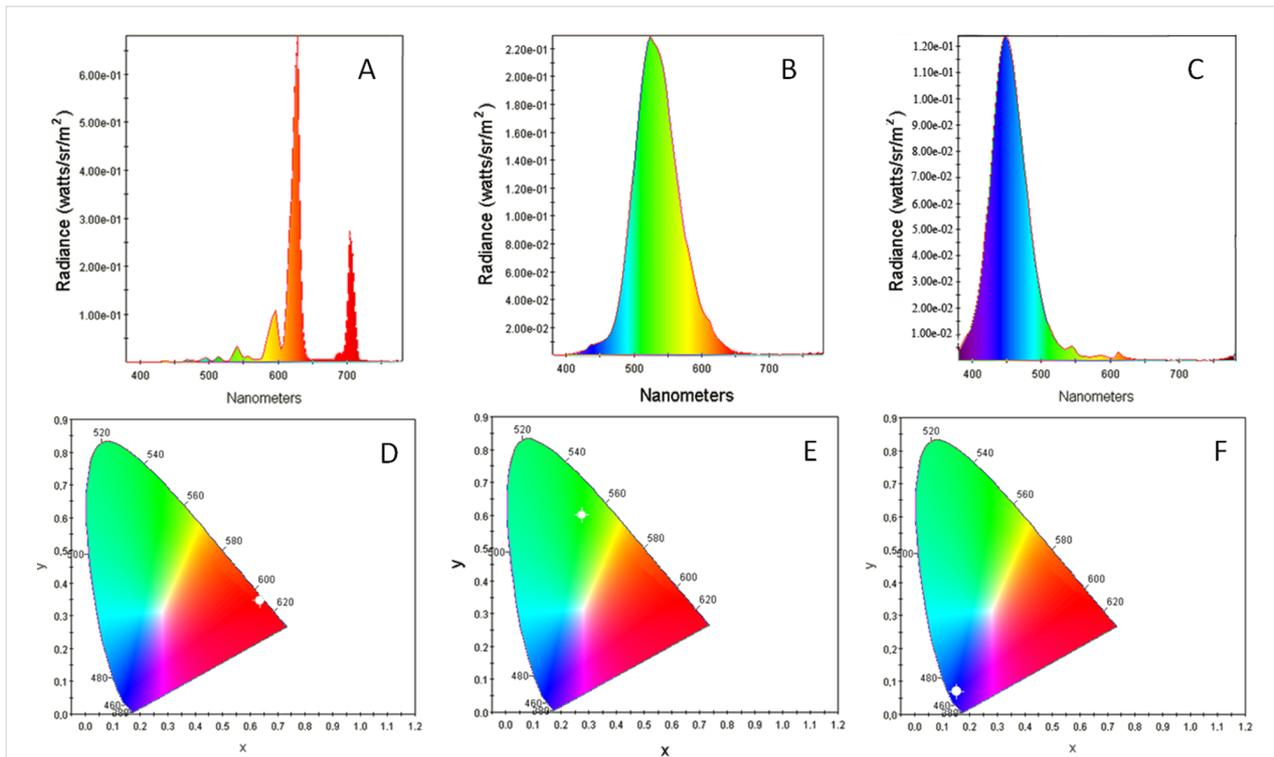
**Figure 7:** Emission spectra and color coordinates (CIE 1931 Chromaticity Diagrams) for light emitted by red (A, D), green (B, E), and blue (C, F) segments of the CL lamp shown in Figure 6, correspondingly.
