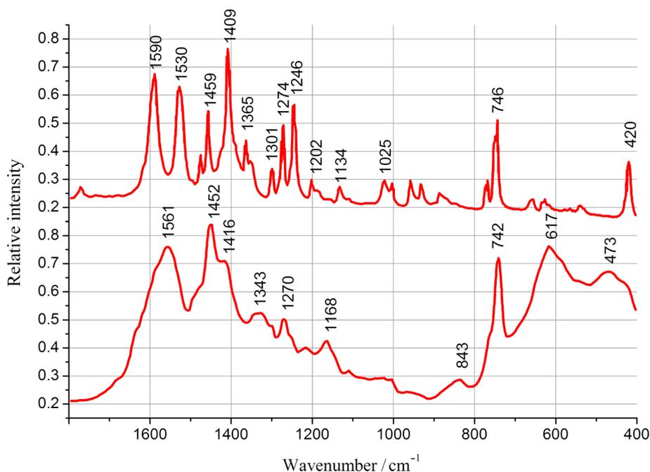
**Figure 4:** FT-IR spectra of a mixture of BI with Zr(acac)<sub>4</sub> (4:1 molar ratio, upper spectrum) and of the product of the reaction occurring after heating of this mixture to 320–350 °C (lower spectrum).
