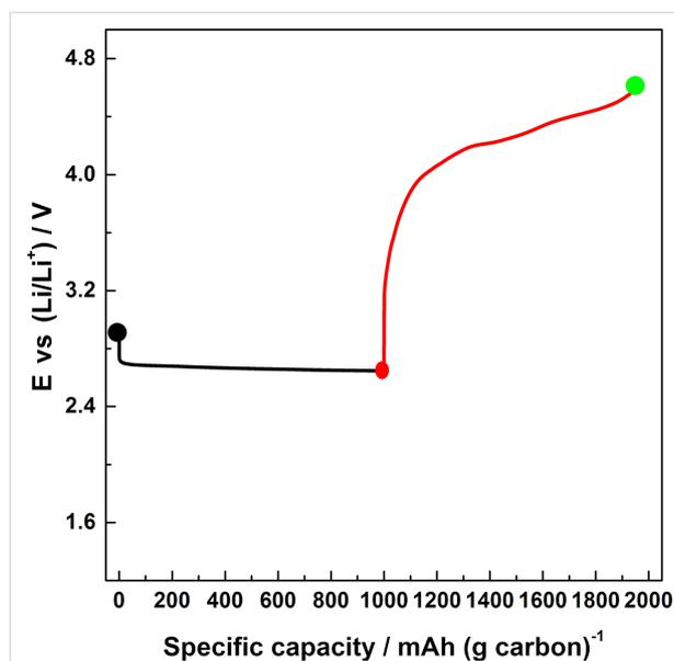
**Figure 5:** First galvanostatic curve of a Li–O<sub>2</sub> battery discharged up to 1000 mAh·(g carbon)<sup>−1</sup>.
