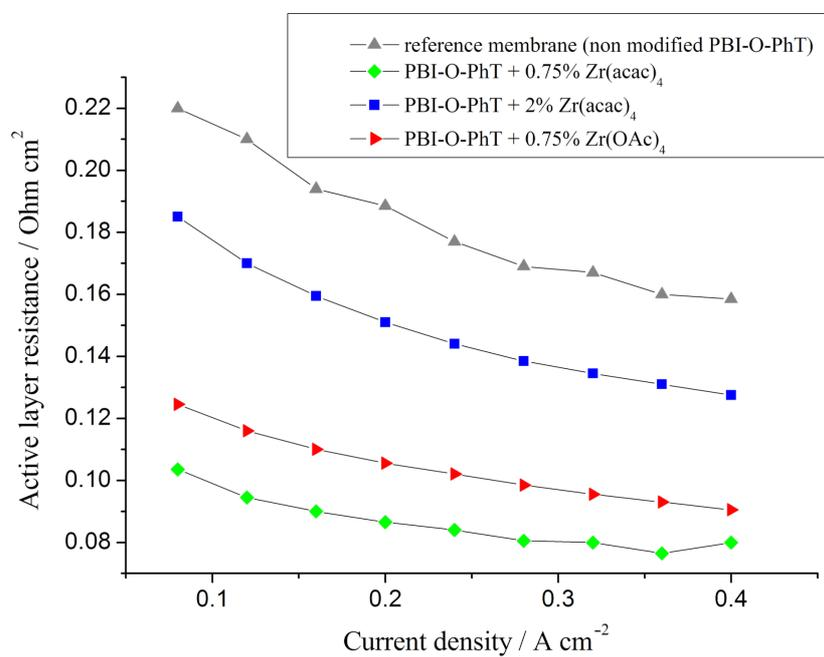
**Figure 11:** Distributed cathode active layer resistances as functions of current density for fuel cells with different PBI membranes.  $T = 160\text{ }^{\circ}\text{C}$ .
