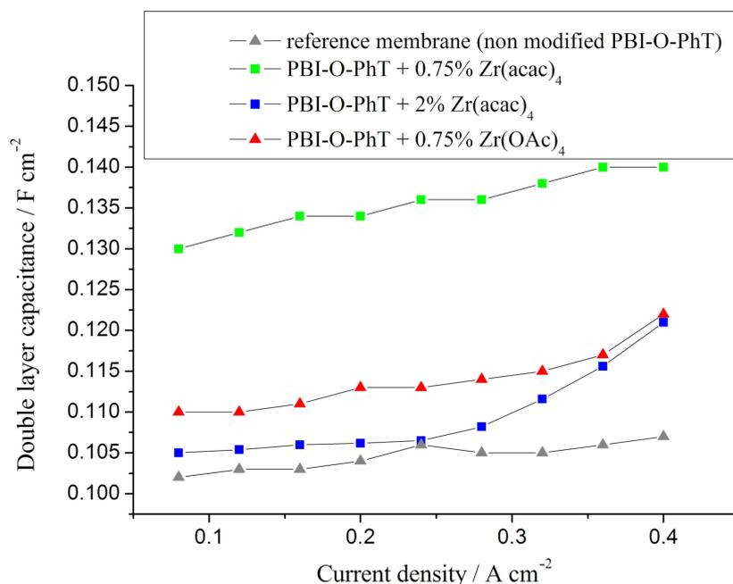
**Figure 12:** The double layer capacitance as a function of the current density for fuel cells with different PBI membranes ( $T = 160\text{ }^{\circ}\text{C}$ ). A higher capacitance indicates a higher area of interphase boundary (PA/Pt and C), which depends on the amount of PA in the active layer.
