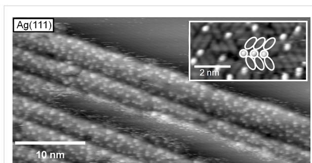
**Figure 2:** STM image of a submonolayer film of [BMP][TFSA] adsorbed on Ag(111); the narrow terraces of the surface are covered with IL islands in the 2D glass phase, the inset shows a high resolution image of the 2D glass structure resolving both the round shaped and the longish protrusions (marked with white circles and ellipsoids) ( $T = 135$  K,  $U_T = -1.14$  mV,  $I_T = 100$  pA).
