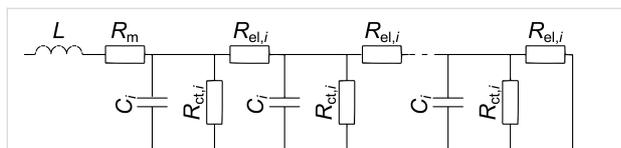
**Figure 2:** Equivalent circuit with a transmission line for modelling the impedance response of the active layers.
