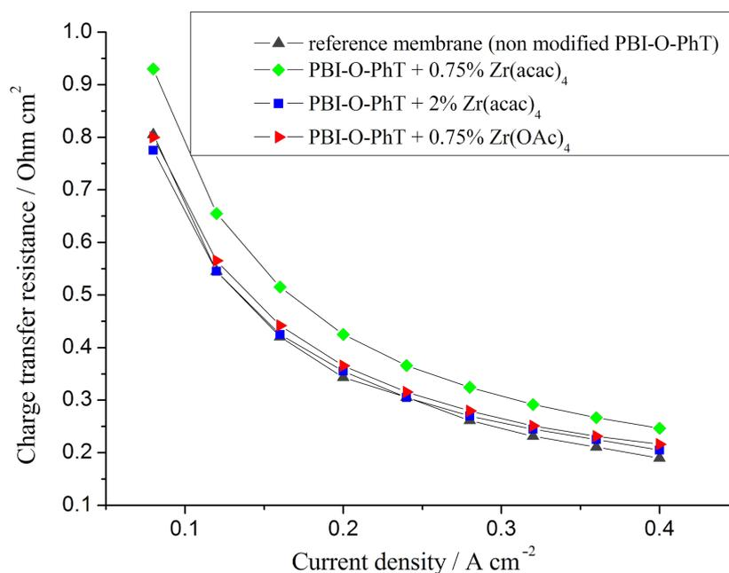
**Figure 13:** Polarization resistance (the sum of charge-transfer and mass-transfer resistances) as a function of the current density for fuel cells with different PBI membranes ( $T = 160\text{ }^{\circ}\text{C}$ ). Higher resistances indicate a lower oxygen transport in the active layer because of a higher acid content in AL.
