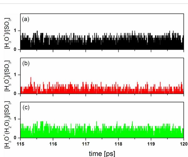
**Figure 14:** A 5-ps section of a QMD trajectory showing the change in the relative content of different hydrated proton complexes at  $\lambda = 10$ . This short time section is chosen for visibility, but the behavior shown here is typical of any time section from the same trajectory.
