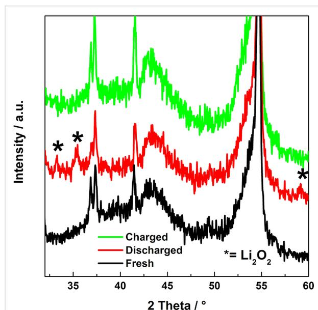
**Figure 3:** X-ray diffractograms of pristine, discharged and charged carbon cathodes. Note the additional peaks of Li<sub>2</sub>O<sub>2</sub> (marked by asterisk) for the discharged state of the cathode.
