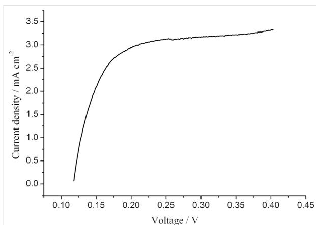
**Figure 9:** Oxidation current of hydrogen diffusing through the membrane for PBI-O-PhT with 0.75 wt %  $\text{Zr}(\text{OAc})_4$ .  $\text{H}_2/\text{N}_2$  operation,  $T = 160\text{ }^{\circ}\text{C}$ .
