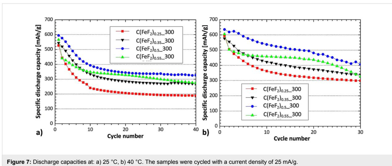
**Figure 7:** Discharge capacities at: a) 25 °C, b) 40 °C. The samples were cycled with a current density of 25 mA/g.
