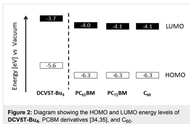
**Figure 2:** Diagram showing the HOMO and LUMO energy levels of **DCV5T-Bu<sub>4</sub>**, PCBM derivatives [34,35], and C<sub>60</sub>.
