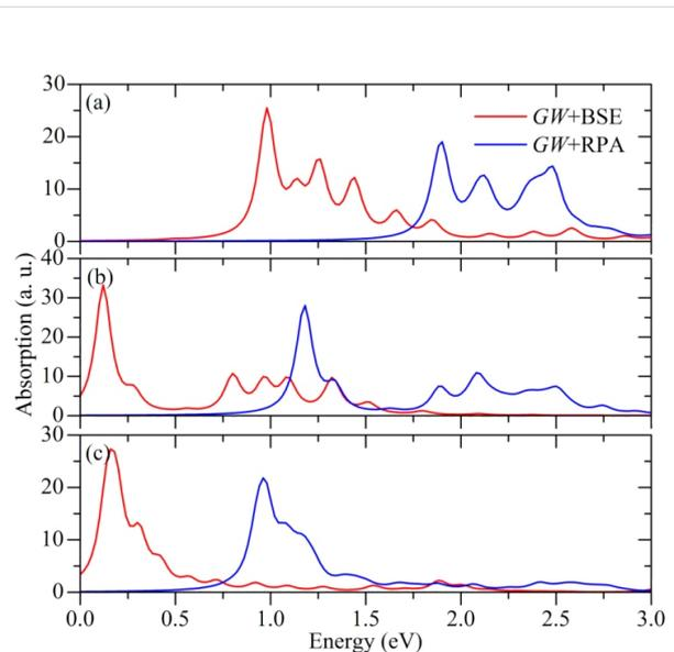
**Figure 4:** Absorption spectra of silicon nanotubes for light polarization along the tube calculated with and without the inclusion of  $e-h$  Coulomb interactions, i.e.,  $GW+BSE$  and  $GW+RPA$ , respectively: (4,4) (a), (6,6) (b) and (10,0) (c). For the  $GW+BSE$  calculation, five occupied and five empty bands and a Lorentzian broadening of 0.05 eV are used.
