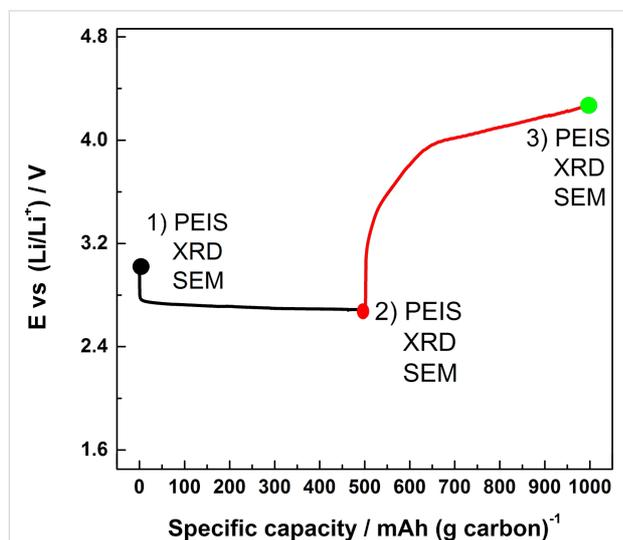
**Figure 1:** First galvanostatic discharge/charge curve of a typical Li–O<sub>2</sub> battery consisting of a carbon-based cathode, lithium metal anode and LiTFSI/tetraglyme as electrolyte.
