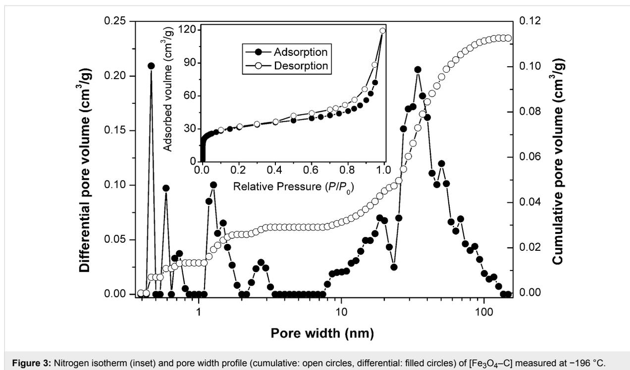
**Figure 3:** Nitrogen isotherm (inset) and pore width profile (cumulative: open circles, differential: filled circles) of  $[\text{Fe}_3\text{O}_4\text{-C}]$  measured at  $-196^\circ\text{C}$ .
