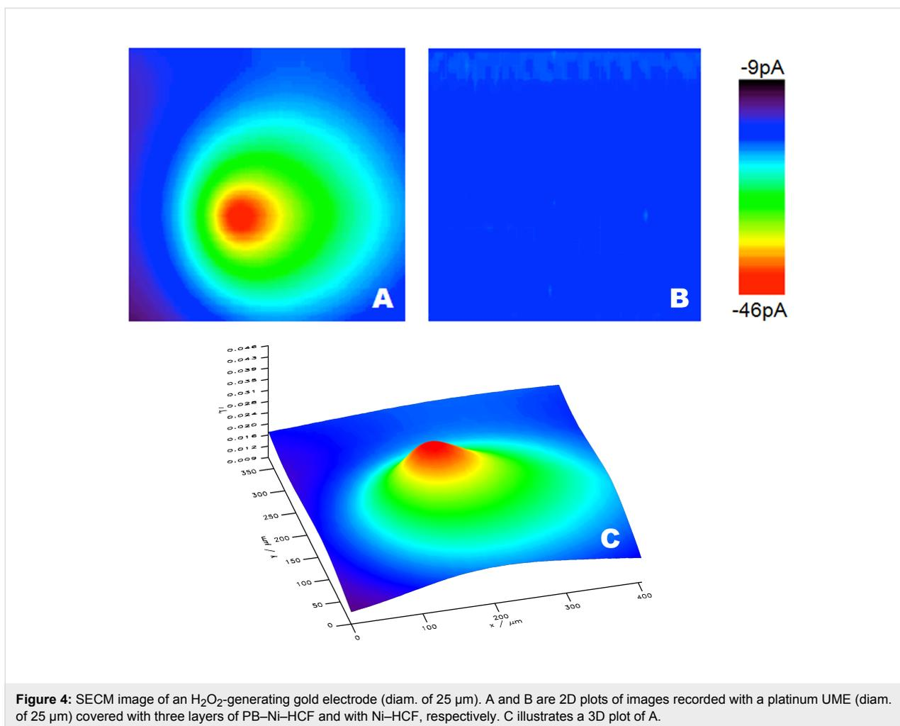
**Figure 4:** SECM image of an  $\text{H}_2\text{O}_2$ -generating gold electrode (diam. of  $25\ \mu\text{m}$ ). A and B are 2D plots of images recorded with a platinum UME (diam. of  $25\ \mu\text{m}$ ) covered with three layers of PB–Ni–HCF and with Ni–HCF, respectively. C illustrates a 3D plot of A.
