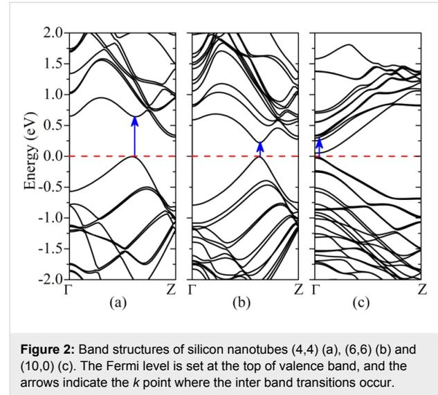
**Figure 2:** Band structures of silicon nanotubes (4,4) (a), (6,6) (b) and (10,0) (c). The Fermi level is set at the top of valence band, and the arrows indicate the  $k$  point where the inter band transitions occur.
