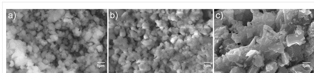
**Figure 4:** SEM images of fluorophosphate materials a) Li<sub>2</sub>CoPO<sub>4</sub>F/C, b) Li<sub>2</sub>Co<sub>0.9</sub>Mn<sub>0.1</sub>PO<sub>4</sub>F/C, c) Li<sub>2</sub>Co<sub>0.7</sub>Fe<sub>0.3</sub>PO<sub>4</sub>F.
