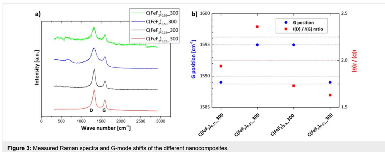
Figure 3: Measured Raman spectra and G-mode shifts of the different nanocomposites.
