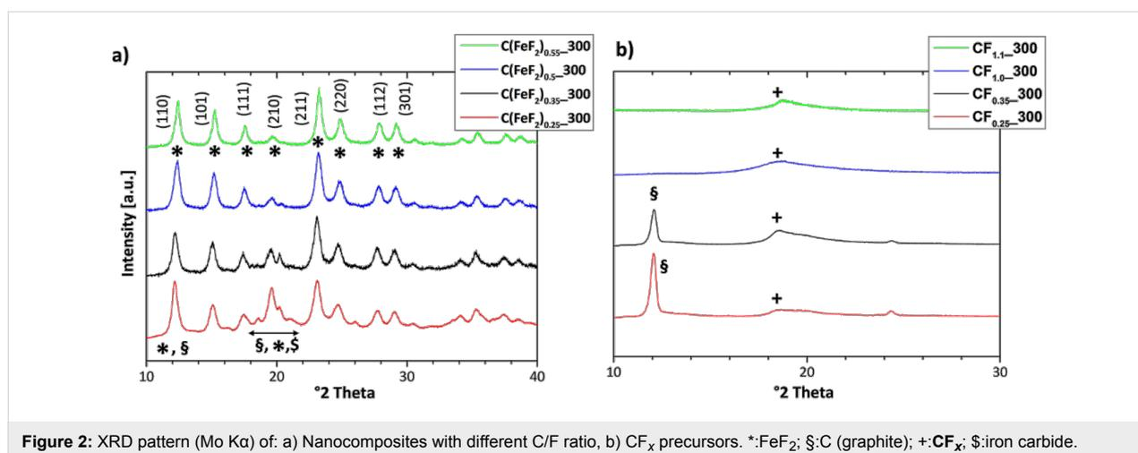
**Figure 2:** XRD pattern (Mo  $\text{K}\alpha$ ) of: a) Nanocomposites with different C/F ratio, b)  $\text{CF}_x$  precursors. \*:  $\text{FeF}_2$ ; §: C (graphite); +:  $\text{CF}_x$ ; §: iron carbide.
