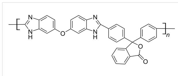
**Figure 1:** Chemical structure of poly[oxy-3,3-bis(4'-benzimidazol-2''-ylphenyl)phtalide-5''(6'')-diy] (PBI-O-PhT).
