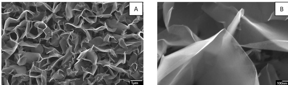
**Figure 3:** Typical SEM images of NGF material taken with different magnifications: overview of the mesoporous structure of the film (A) and a fragment of a flake transparent for secondary electrons taken with a higher resolution (B).
