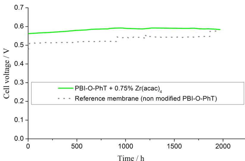
**Figure 14:** 2000-hour stability test of a composite PBI-O-PhT + 0.75 wt %  $Zr(acac)_4$  membrane and the reference membrane in an operating fuel cell.  $H_2/air$ ,  $T = 160\text{ }^\circ\text{C}$ , current density  $0.4\text{ A}\cdot\text{cm}^{-2}$ .
