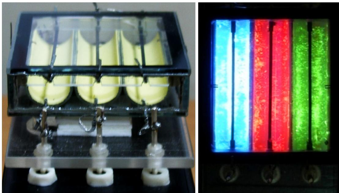
**Figure 6:** Photographs showing the general design of the CL lamp (left side) and the light emission from RGB segments (right side) with the application of a pulsed voltage (pulse duration 15  $\mu$ s, repetition rate 1 kHz, amplitude 8 kV) and with a total current per segment of about 0.25 mA. The image is an adapted version of a previously published graphic in [22] with permission from *J. Nanoelectron. Optoelectron.* © 2009.
