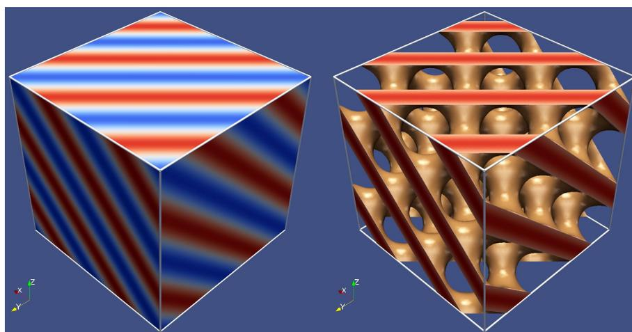
**Figure 5:** Ordered bicontinuous double diamond structure (space group 224), which contains two separate, connected, triply periodic, tetrahedrally coordinated networks comprised of the minority (A, "red") component in a matrix of the majority (B, "blue") component. Both the red and blue domains are three-dimensionally continuous. The right part of the figure shows the minority component bound by the isodensity surface.
