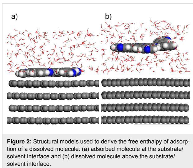
the scheme illustrated in Figure 2, i.e., it is evaluated as the difference of the free enthalpy of the molecule adsorbed at the substrate/solvent interface minus the free enthalpy of the molecule dissolved above the substrate/solvent interface:
