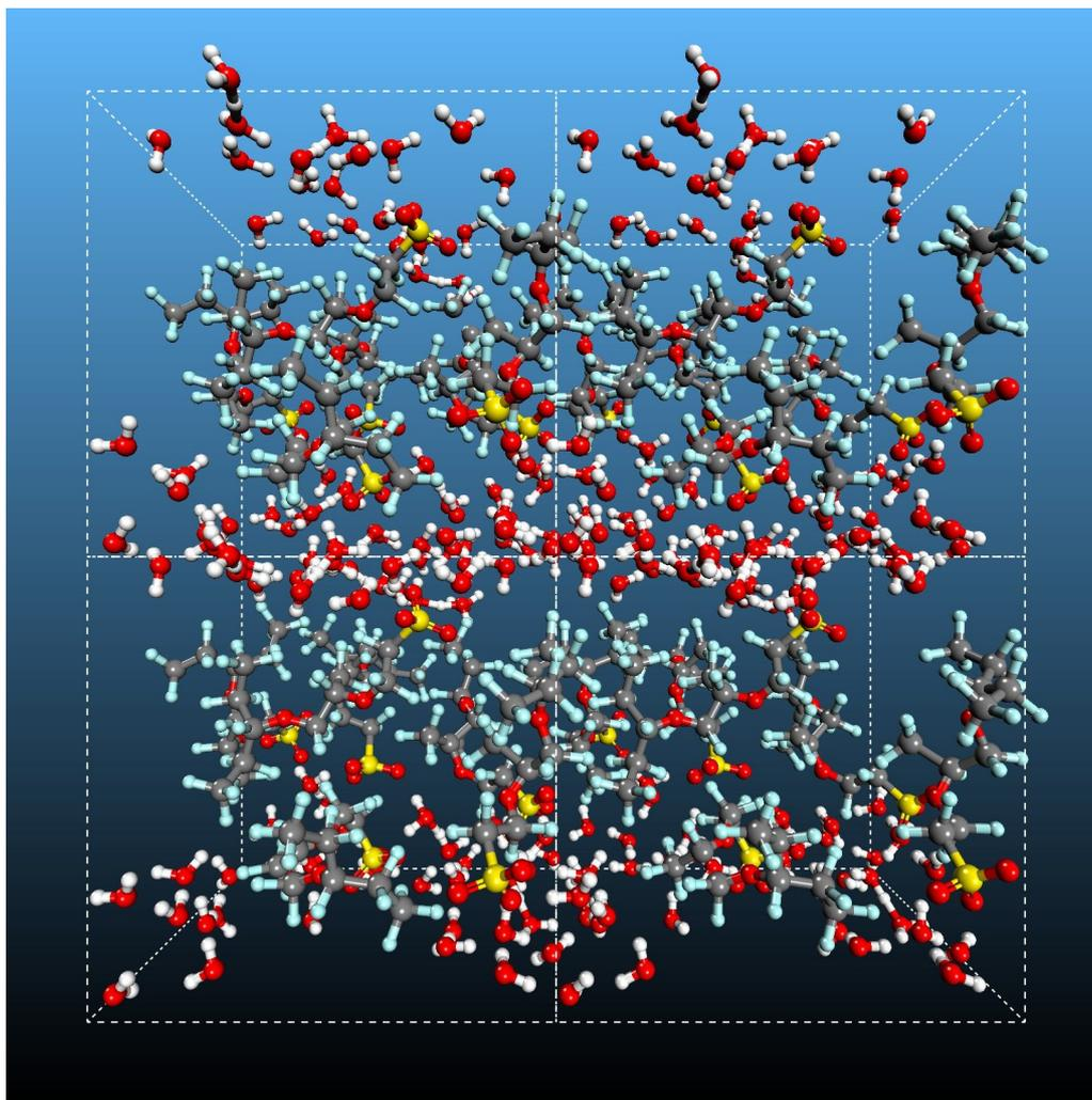
**Figure 11:** Snapshot of the water-containing Nafion structure obtained after the 200 ps QMD simulation at 298 K and  $\lambda = 10$ . The simulation box is replicated two times along the X- and Z-directions. For clarity, some of the equivalent atoms (not all) across the periodic boundaries are also depicted. Oxygen is shown in red, carbon in gray, fluorine in light blue, hydrogen in white, and sulfur in yellow.
