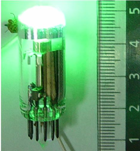
**Figure 5:** Photograph of the CL diode lamp with an NGF cathode with an emitting surface (of about 1 mm diameter) located at the center of the semispherical surface of the CL anode (of about 5 mm diameter). Applied voltage: pulses of about 15  $\mu$ s, repetition rate of about 1 kHz with 8 kV amplitude. The image is an adapted version of a previously published graphic in [22] with permission from *J. Nanoelectron. Optoelectron.* © 2009.
