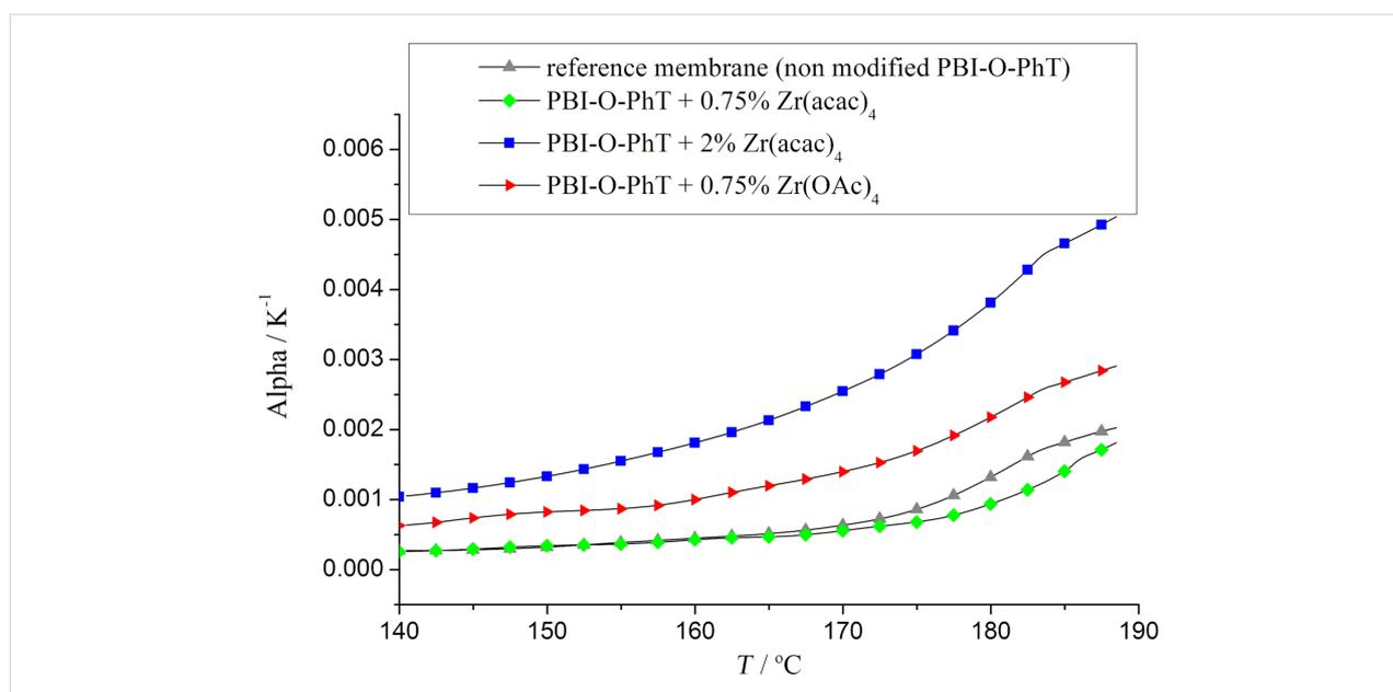
**Figure 7:** Thermal expansion coefficients of the composite membranes.
