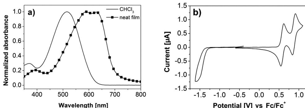
**Figure 1:** (a) Absorption spectrum of **DCV5T-Bu<sub>4</sub>** measured in chloroform and as thin film, spin-coated from chlorobenzene at 80 °C. (b) Cyclic voltammogram of **DCV5T-Bu<sub>4</sub>** in dichloromethane, TBAPF<sub>6</sub> (0.1 M) measured versus the ferrocene/ferrocenyl (Fc/Fc<sup>+</sup>) redox couple.
