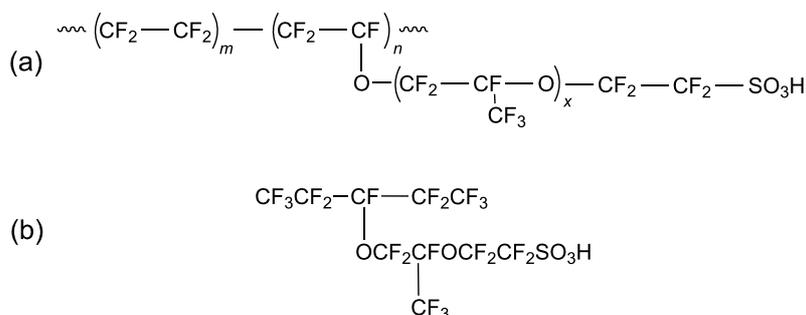
Figure 1: (a) Nafion chain. (b) Nafion sulfonated monomer.
