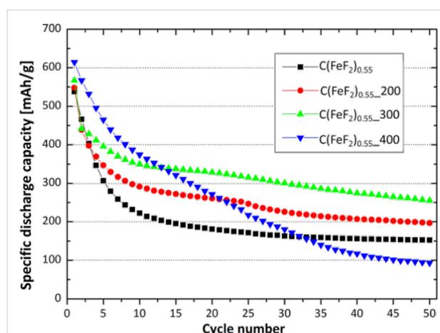
**Figure 1:** Cycling behavior of C(FeF<sub>2</sub>)<sub>0.55</sub>, C(FeF<sub>2</sub>)<sub>0.55\_200</sub>, C(FeF<sub>2</sub>)<sub>0.55\_300</sub> and C(FeF<sub>2</sub>)<sub>0.55\_400</sub>. The materials were cycled with a current density of 23 mA/g between 1.3 V and 4.3 V.
