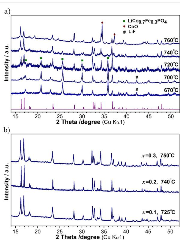
**Figure 5:** a) XRD patterns of a mixture of  $\text{LiCo}_{0.7}\text{Fe}_{0.3}\text{PO}_4$  and LiF, annealed at different temperatures, starting from 670 °C. XRD peaks that correspond to impurities are marked. b) XRD patterns of  $\text{Li}_2\text{Co}_{1-x}\text{Fe}_x\text{PO}_4\text{F}$  ( $x = 0.1, 0.2, 0.3$ ), synthesized at the denoted temperatures.
