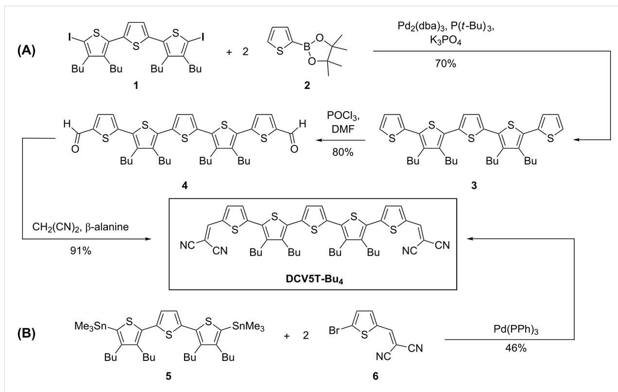
**Scheme 1:** Alternative synthetic routes used to yield **DCV5T-Bu<sub>4</sub>**.
