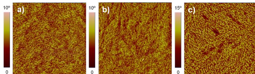
**Figure 6:** AFM phase images of samples spin-coated on ITO|PEDOT:PSS| with (a) **DCV5T-Bu<sub>4</sub>**:PC<sub>61</sub>BM from CB, (b) **DCV5T-Bu<sub>4</sub>**:PC<sub>61</sub>BM from CB:CN (0.375%), and (c) **DCV5T-Bu<sub>4</sub>**:PC<sub>71</sub>BM from ODCB. Image size: 1 × 1 μm.
