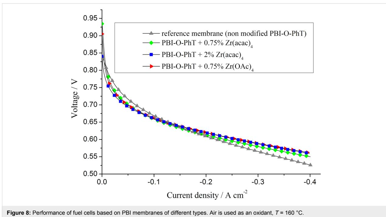
**Figure 8:** Performance of fuel cells based on PBI membranes of different types. Air is used as an oxidant,  $T = 160\text{ }^{\circ}\text{C}$ .
