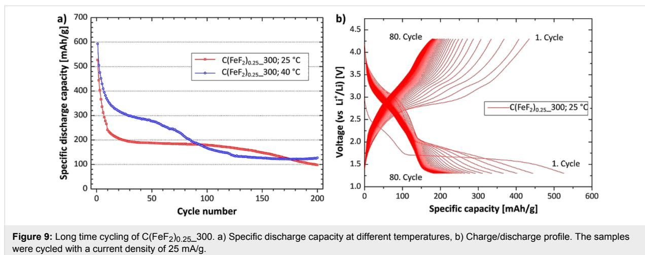
**Figure 9:** Long time cycling of C(FeF<sub>2</sub>)<sub>0.25</sub>\_300. a) Specific discharge capacity at different temperatures, b) Charge/discharge profile. The samples were cycled with a current density of 25 mA/g.
