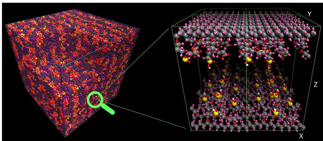
**Figure 10:** Model of the ion-conducting channel studied by quantum molecular dynamics. The initial configuration is shown. Channel walls are formed by Nafion chains oriented along the X-axis. The chains are infinite in the periodic cell. The total number of atoms in the system is 1200. Water molecules filling the channel are omitted for visual clarity. Conventional atom colors are used.
