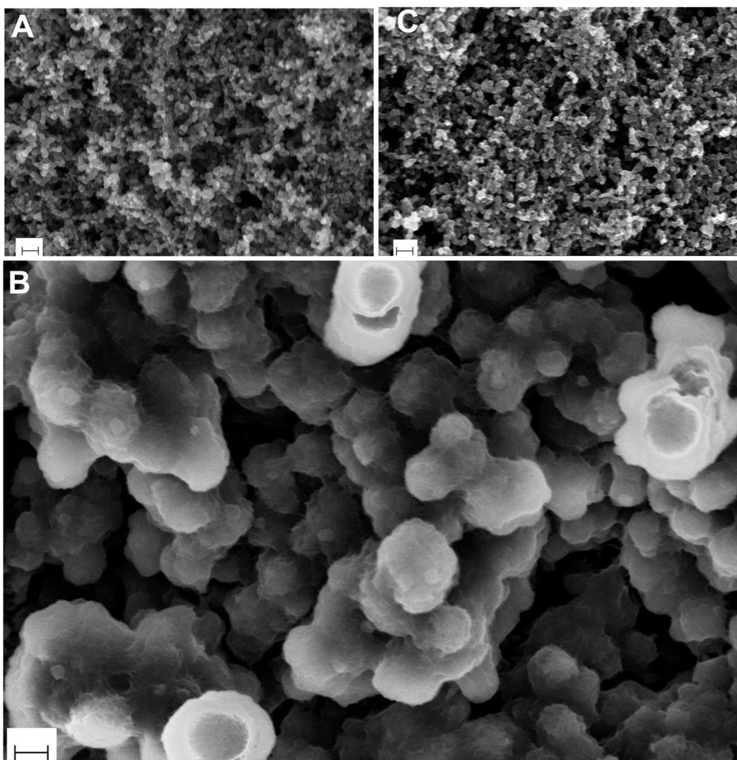
**Figure 4:** SEM micrographs of (A) pristine electrode, (B) discharged electrode for which the capacity was limited at  $500 \text{ mAh}\cdot(\text{g carbon})^{-1}$  and (C) recharged electrode of  $\text{Li}-\text{O}_2$  batteries. Note that the large  $\text{Li}_2\text{O}_2$  particles in (B) appear to have a hollow structure with a smooth surface and nodular morphology. The scale bars correspond to 200 nm.
