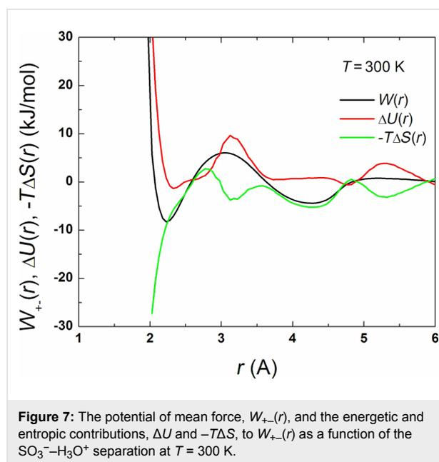
**Figure 7:** The potential of mean force,  $W_{+-}(r)$ , and the energetic and entropic contributions,  $\Delta U$  and  $-T\Delta S$ , to  $W_{+-}(r)$  as a function of the  $\text{SO}_3^- \cdot \text{H}_3\text{O}^+$  separation at  $T = 300$  K.
