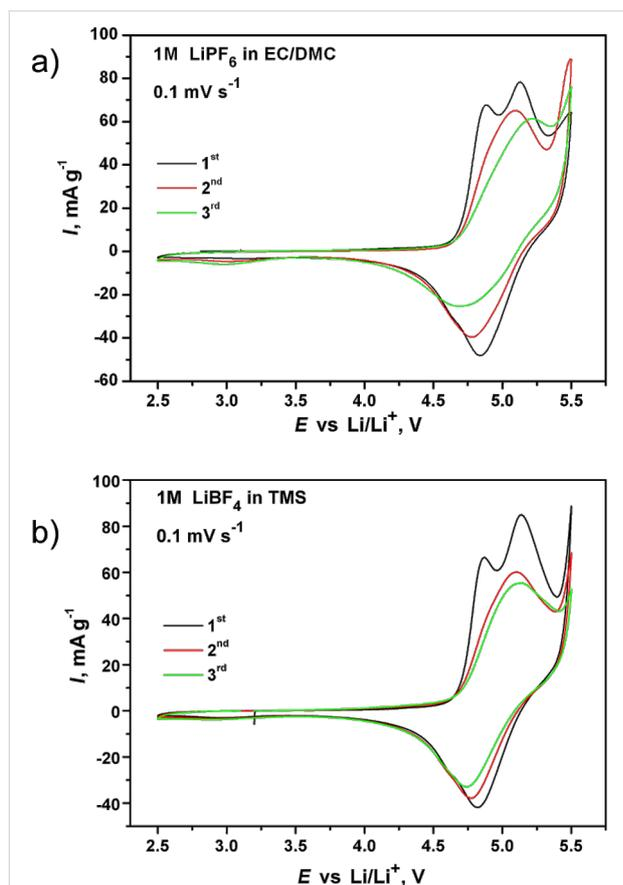
**Figure 7:** Cyclic voltammetry curves of the  $\text{Li}_2\text{Co}_{0.9}\text{Mn}_{0.1}\text{PO}_4\text{F}$  electrodes in the commercial (a) and the sulfone-based (b) electrolytes recorded at  $0.1 \text{ mV s}^{-1}$ .
