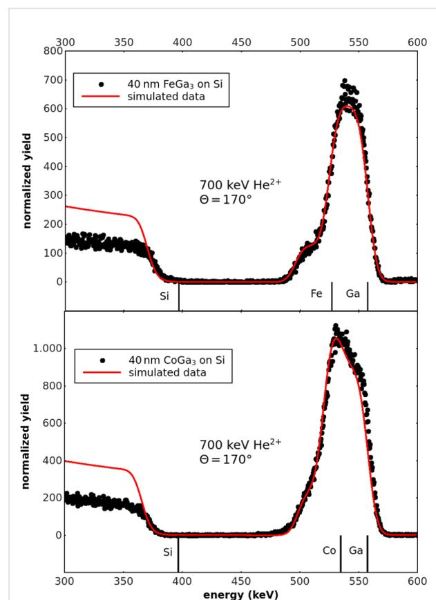
**Figure 1:** RBS spectra of FeGa<sub>3</sub> (a) and CoGa<sub>3</sub> (b) films deposited onto Si substrates. RUMP simulations (solid lines) deliver a composition of FeGa<sub>3,2</sub> with a thickness of 40 nm and a composition of CoGa<sub>3</sub> with a thickness of 43 nm. Backscattering energies of Co, Ga and Si at the sample surface are indicated by vertical marks. The displacement of the Si edge of the substrate toward lower backscattering energies is caused by the film thickness.
