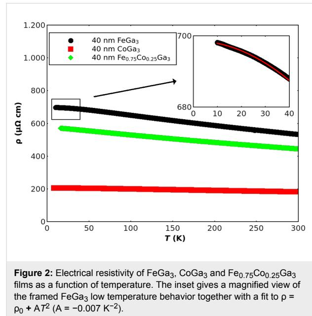
**Figure 2:** Electrical resistivity of  $\text{FeGa}_3$ ,  $\text{CoGa}_3$  and  $\text{Fe}_{0.75}\text{Co}_{0.25}\text{Ga}_3$  films as a function of temperature. The inset gives a magnified view of the framed  $\text{FeGa}_3$  low temperature behavior together with a fit to  $\rho = \rho_0 + AT^2$  ( $A = -0.007 \text{ K}^{-2}$ ).
