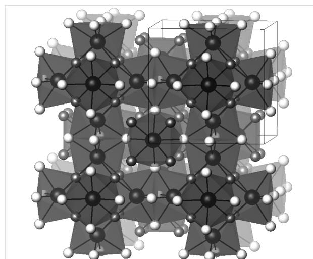
**Figure 3:** Polyhedral view of the  $\text{Re}_3\text{As}_{7-x}\text{In}_x$  crystal structure. Re is shown as black spheres inside the polyhedra, E1: white spheres, and As2: gray spheres at the vertices.
