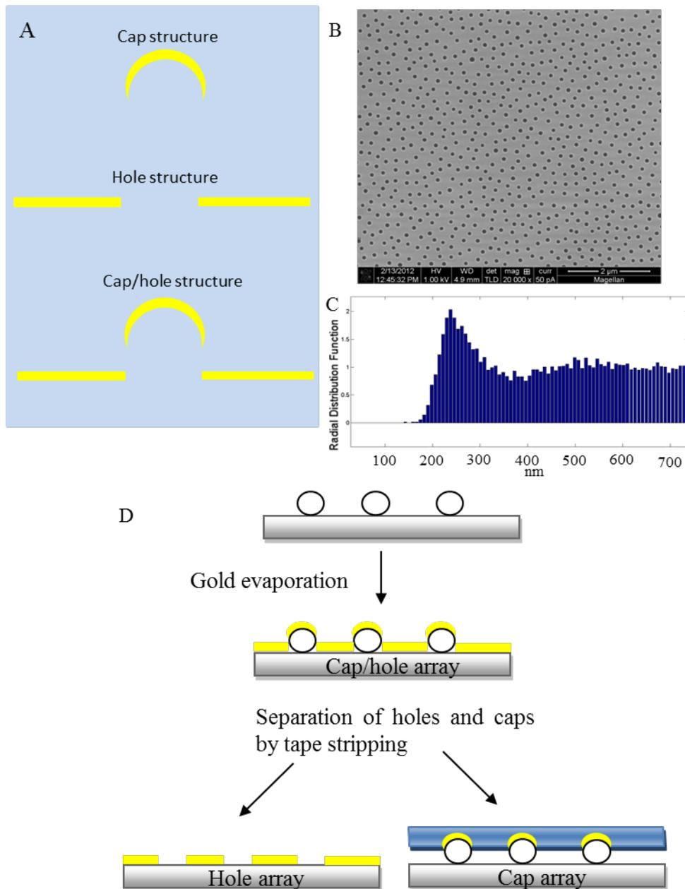
**Figure 1:** A) Schematic of the design of the plasmonic gold structures fabricated by colloidal lithography. B) SEM image showing the distribution of a 110 nm hole array in 20 nm thin Au film after removal of the gold-caps by tape stripping. C) Radial distribution function showing the characteristic average spacing between holes of the same hole array. D) Fabrication route for the plasmonic structures.
