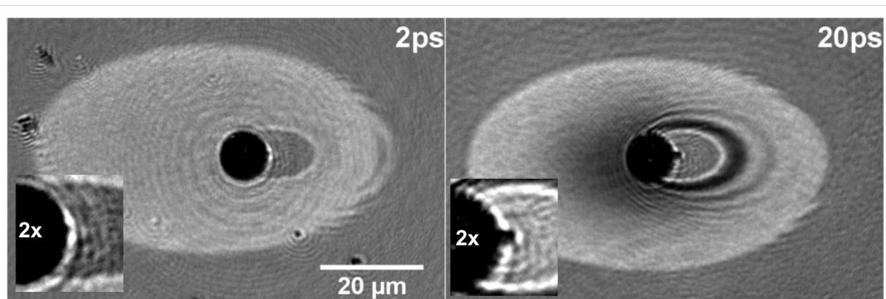
**Figure 7:** Surface reflectivity images at the particle location for two different delays (indicated), upon exposure to a 120 fs-laser pulse with a peak fluence of  $0.87 \text{ J/cm}^2$  reaching the surface at  $54^\circ$ . A zoom ( $2\times$ ) has been applied to the relevant part of the image and pasted as an inset to facilitate the description in the text.
