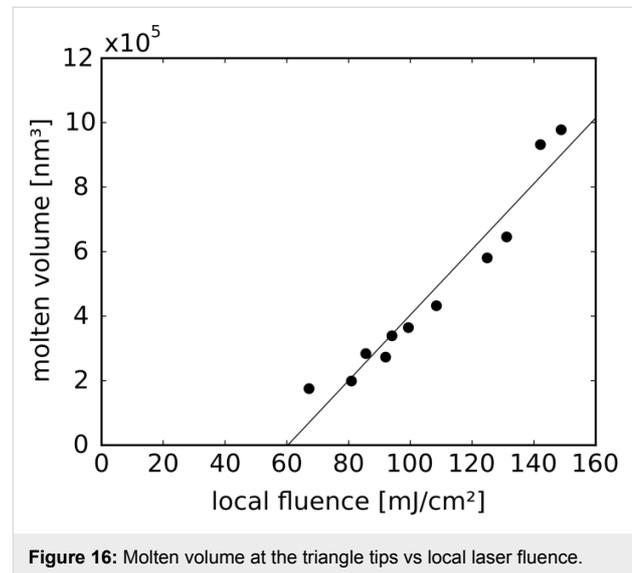
Figure 16: Molten volume at the triangle tips vs local laser fluence.
