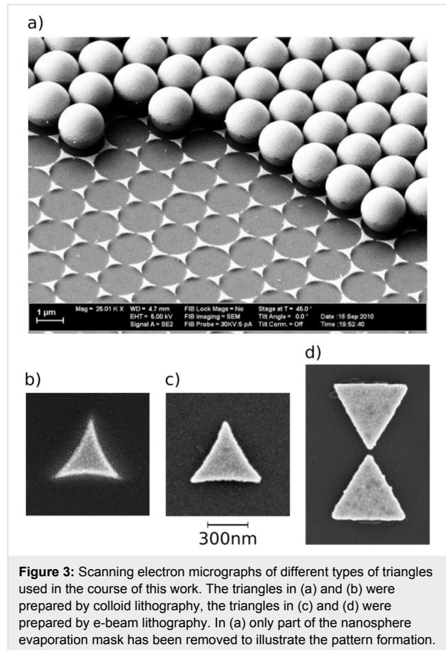
**Figure 3:** Scanning electron micrographs of different types of triangles used in the course of this work. The triangles in (a) and (b) were prepared by colloid lithography, the triangles in (c) and (d) were prepared by e-beam lithography. In (a) only part of the nanosphere evaporation mask has been removed to illustrate the pattern formation.
