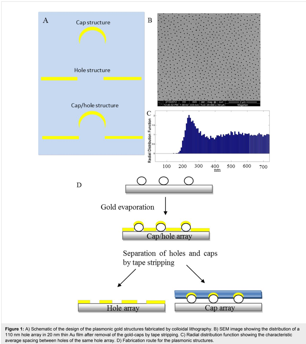
adhesive tape (90  $\mu\text{m}$  thick blue PVC Tape from Semiconductor Production Systems). The tape was subsequently placed onto a glass substrate for characterization. The tape stripped cap/hole arrays left behind hole arrays.
