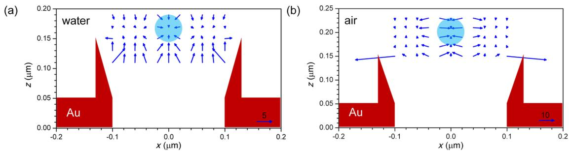
**Figure 5:** Arrow plot of the trapping force for plane-wave illumination in medium-to-substrate direction (as in Figure 4) at 760 nm wavelength for a 50-nm diameter polystyrene bead in (a) water and (b) air. The conical Au-well profile is schematically shown by the triangular shapes and the circle indicates the position of the bead in the central trap. The scale arrows at the lower right indicate forces of 5 and 10  $\text{pN/W}/\mu\text{m}^2$ .
