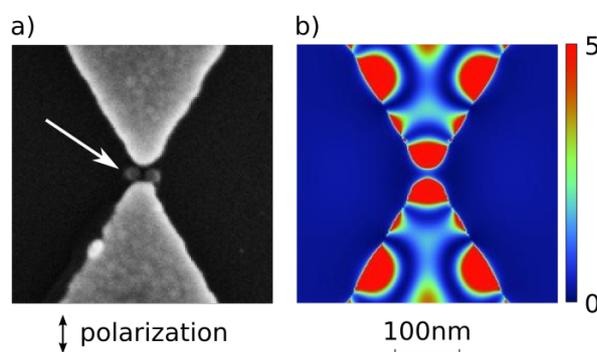
**Figure 13:** (a) SEM micrograph and (b) calculated field distribution for the center region of a bow-tie antenna with a distance of 30 nm. The structure has been irradiated with a 150 fs laser pulse (wavelength: 800 nm) with a local fluence of  $90 \text{ mJ/cm}^2$ . The arrow points towards the region in the feed gap where ablation of the Si has taken place. The color scale in (b) has been chosen such to show the field distribution in the region between the triangles.
