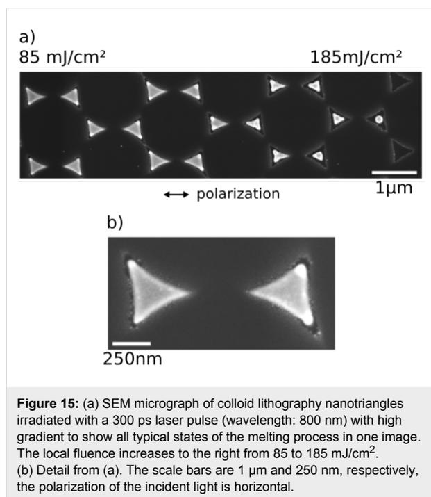
Figure 15a displays an SEM image of partly molten triangles in an intensity regime between 85 and 185 mJ/cm<sup>2</sup>, and Figure 15b shows a blow-up. Note that the intensity gradient used in this irradiation was so steep that the right triangle in Figure 15b, located less than 1 µm from the left one, exhibits considerably larger molten volumes at the tips. Plotting the molten volume, as determined from the SEM images, versus the incident intensity leads to the graph in Figure 16, from which a
