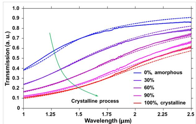
**Figure 2:** Comparison between the experimental spectra measurements (solid lines) and the simulated far-field transmission spectra (dashed lines) of a GST thin film switched at different intermediate phases. A good agreement of the spectral results shows the quantifiable phase-change modulation of a GST nano thin film at different crystalline proportions.
