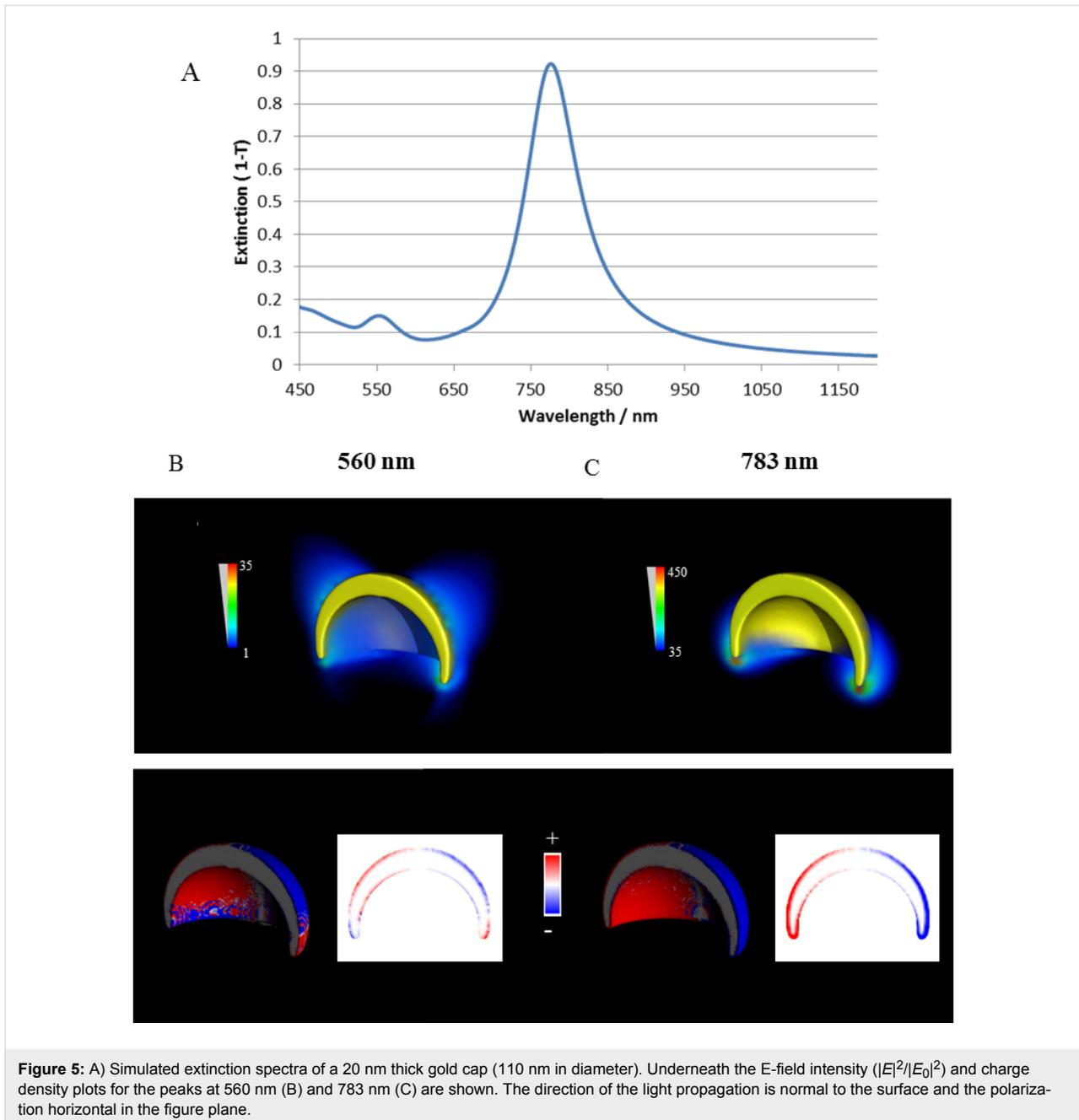
**Figure 5:** A) Simulated extinction spectra of a 20 nm thick gold cap (110 nm in diameter). Underneath the E-field intensity ( $|E|^2/E_0^2$ ) and charge density plots for the peaks at 560 nm (B) and 783 nm (C) are shown. The direction of the light propagation is normal to the surface and the polarization horizontal in the figure plane.
