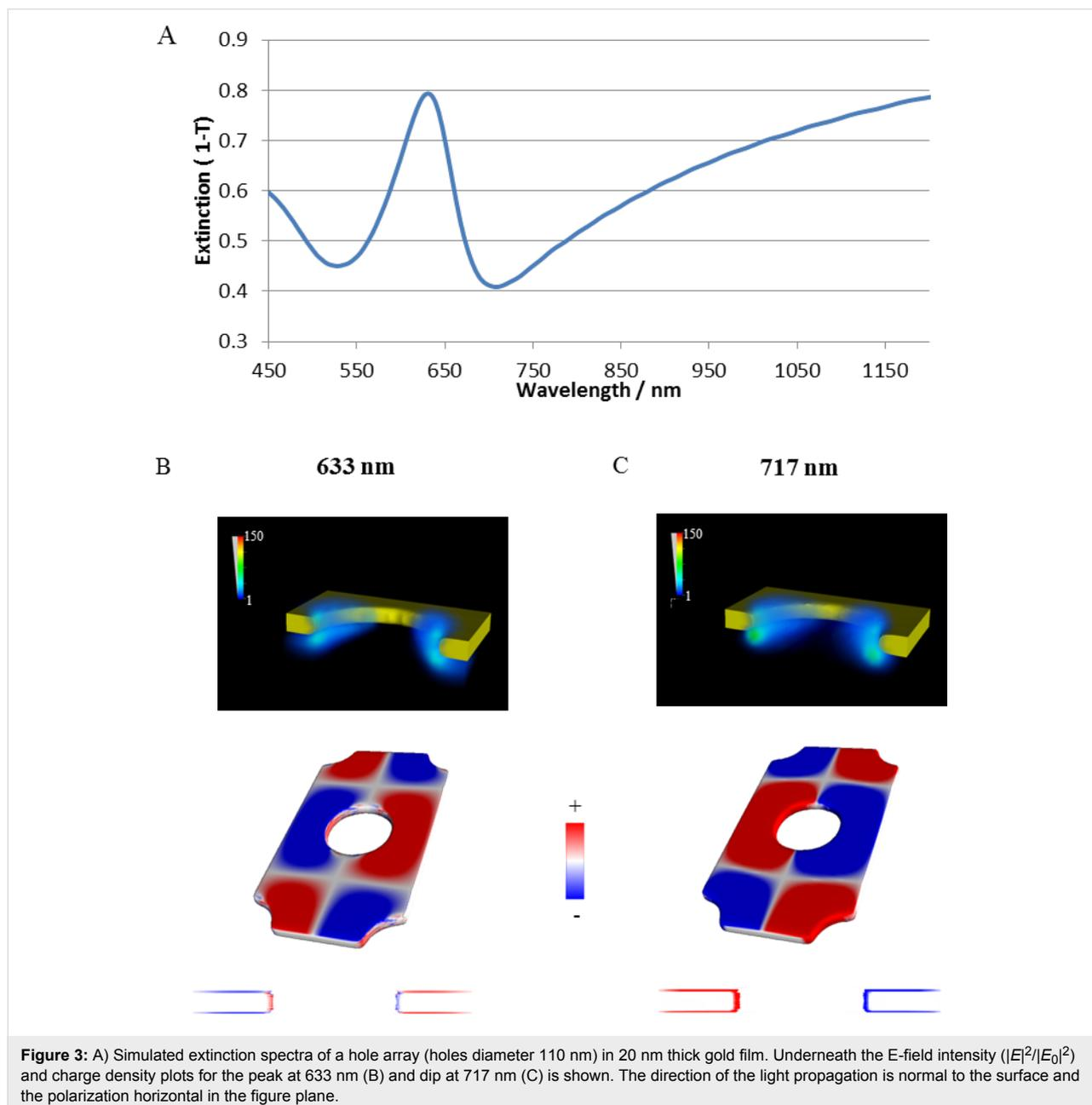
the systems used currently [33,34] in literature) as a second order SPP mode, with the localized distribution of the field arising from the abrupt presence of a hole in the metal film rather than an LSPR type character. We assign the dip to be a bonding hybridization of dipolar LSPR modes at the holes and a first order SPP mode. These assignments are consistent with the recent experimental and theoretical reports [30,33].
