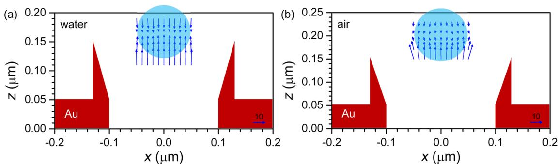
**Figure 6:** Arrow plot of the trapping force as in Figure 5 at 760 nm wavelength for a 100-nm diameter bead in (a) water and (b) air. The scale arrows at the lower right indicate a force of 10  $\text{pN/W}/\mu\text{m}^2$ .
