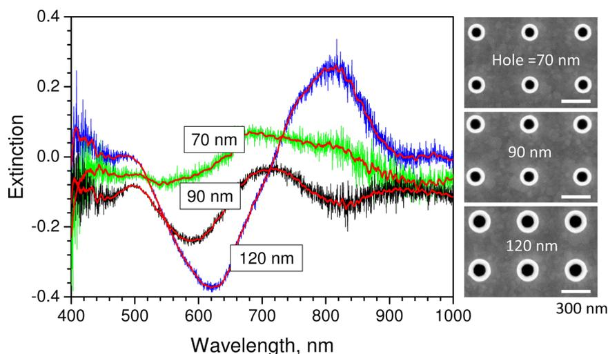
**Figure 3:** Experimentally measured extinction of the nano-well substrate for hole diameters of 70, 90, and 120 nm. The value is normalized to a continuous 100-nm Au layer, thus the negative regions offer proof of extraordinary transmission [16] through the array.
