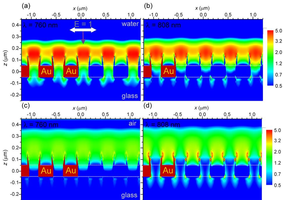
**Figure 4:** Light intensity distribution in the  $xz$ -plane simulated by 3D-FDTD at the two laser wavelengths (a,c) 760 nm and (b,d) 808 nm, in (a,b) water and (c,d) air. Incident light intensity  $|E_0|^2 = 1$ ; propagation in negative  $z$ -direction.
