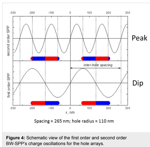
**Figure 4:** Schematic view of the first order and second order BW-SPP's charge oscillations for the hole arrays.
