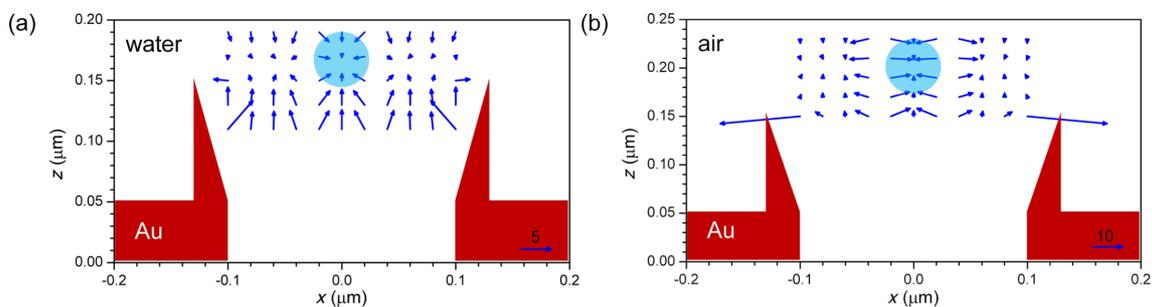
**Figure 5:** Arrow plot of the trapping force for plane-wave illumination in medium-to-substrate direction (as in Figure 4) at 760 nm wavelength for a 50-nm diameter polystyrene bead in (a) water and (b) air. The conical Au-well profile is schematically shown by the triangular shapes and the circle indicates the position of the bead in the central trap. The scale arrows at the lower right indicate forces of 5 and 10  $\text{pN/W}/\mu\text{m}^2$ .
