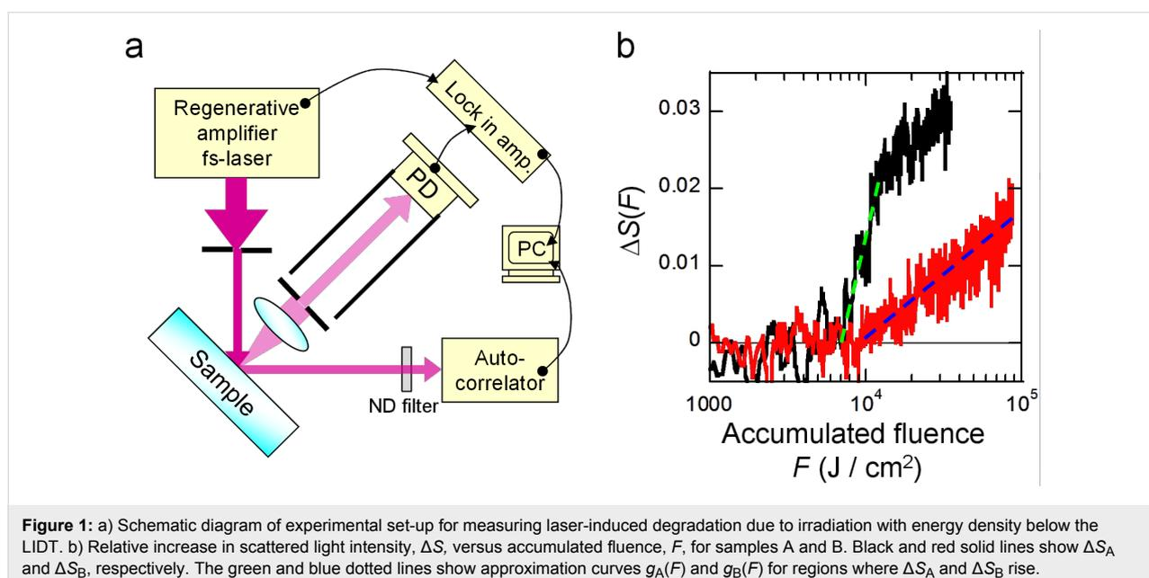
**Figure 1:** a) Schematic diagram of experimental set-up for measuring laser-induced degradation due to irradiation with energy density below the LIDT. b) Relative increase in scattered light intensity,  $\Delta S$ , versus accumulated fluence,  $F$ , for samples A and B. Black and red solid lines show  $\Delta S_A$  and  $\Delta S_B$ , respectively. The green and blue dotted lines show approximation curves  $g_A(F)$  and  $g_B(F)$  for regions where  $\Delta S_A$  and  $\Delta S_B$  rise.
