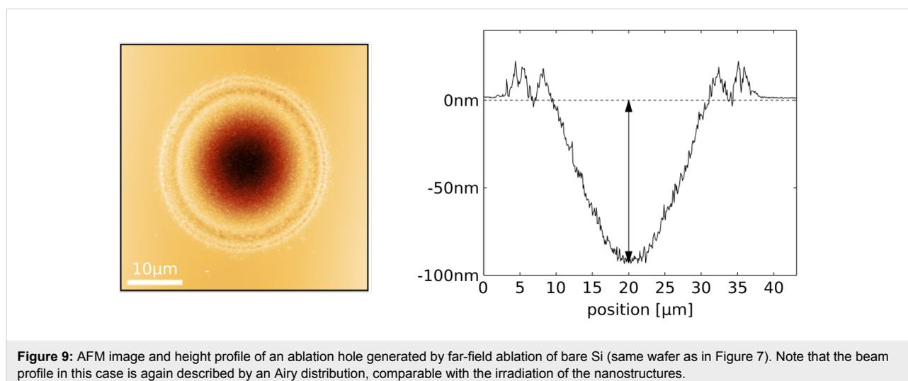
**Figure 9:** AFM image and height profile of an ablation hole generated by far-field ablation of bare Si (same wafer as in Figure 7). Note that the beam profile in this case is again described by an Airy distribution, comparable with the irradiation of the nanostructures.
