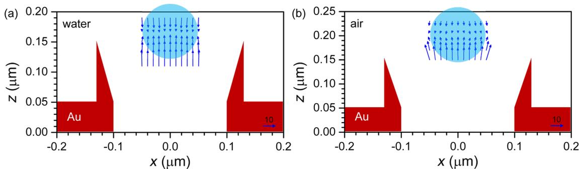
**Figure 6:** Arrow plot of the trapping force as in Figure 5 at 760 nm wavelength for a 100-nm diameter bead in (a) water and (b) air. The scale arrows at the lower right indicate a force of 10  $\text{pN/W}/\mu\text{m}^2$ .
