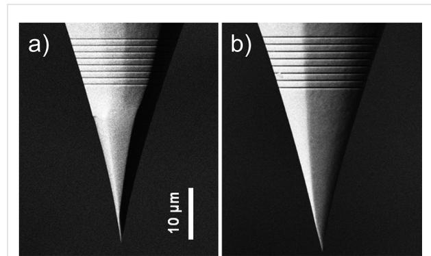
**Figure 1:** Scanning electron micrographs of two gold tapers that were obtained by electrochemical AC-etching of annealed gold wires followed by focused ion beam milling of the grating couplers. Field enhancement at the taper apex was much more pronounced for the tip shown in panel a).
