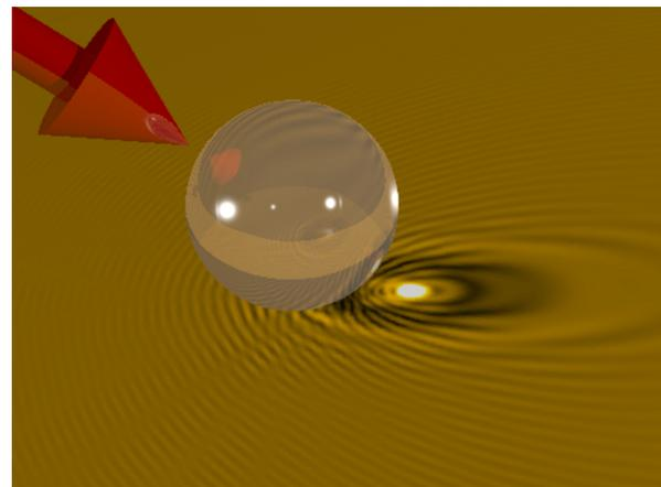
**Figure 1:** Schematic view of the spatial intensity distribution at the surface of a crystalline Si substrate in the vicinity of a 7.9  $\mu\text{m}$ -diameter  $\text{SiO}_2$  spherical particle illuminated at oblique incidence by a laser with 800 nm wavelength. The bright spot corresponds to the enhancement of the incoming field. The fine fringe structure is caused by interference of the incoming laser beam, light reflected at the substrate, and light scattered by the particle.
