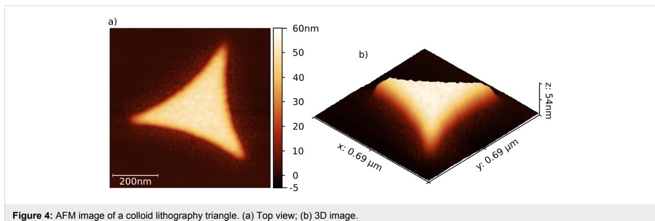
**Figure 4:** AFM image of a colloid lithography triangle. (a) Top view; (b) 3D image.
