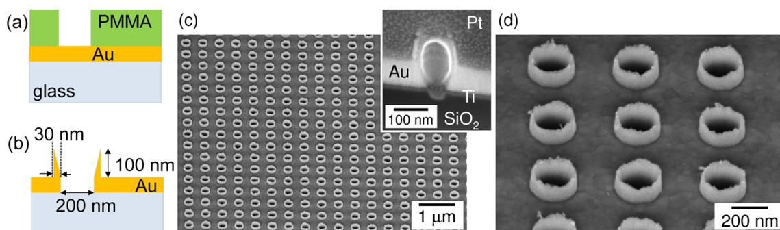
**Figure 1:** Illustration of the nano-well fabrication by (a) dry plasma etching of Au-film and PMMA mask, which results in Au re-sputtering and (b) formation of a nano-well around the rim of the hole. The experimental outcome is shown as (c) SEM image of the 3D Au nano-wells array; in (d) the magnified slanted view shows details of the nano-well edges. The inset in panel (c) shows the cross-section of a nano-well after deposition of a protective Pt layer.
