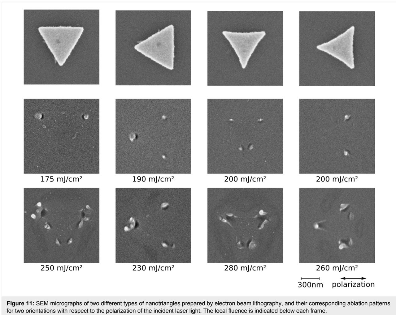
**Figure 11:** SEM micrographs of two different types of nanotriangles prepared by electron beam lithography, and their corresponding ablation patterns for two orientations with respect to the polarization of the incident laser light. The local fluence is indicated below each frame.
