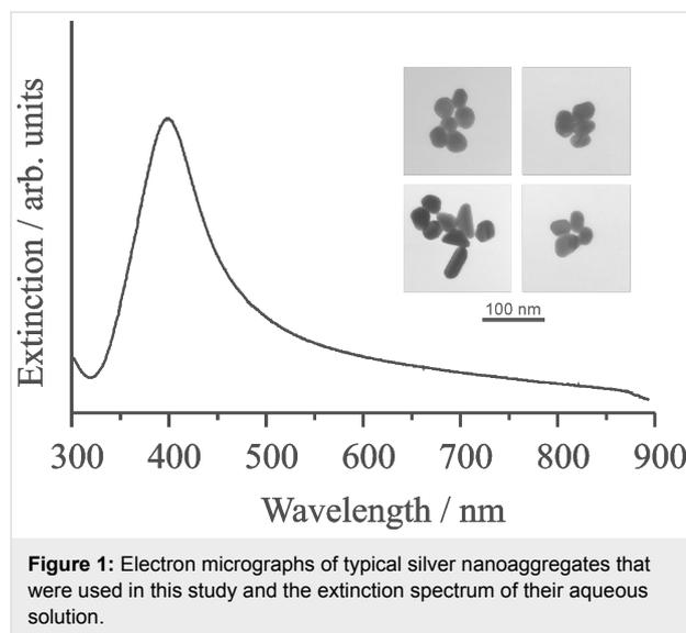
**Figure 1:** Electron micrographs of typical silver nanoaggregates that were used in this study and the extinction spectrum of their aqueous solution.
