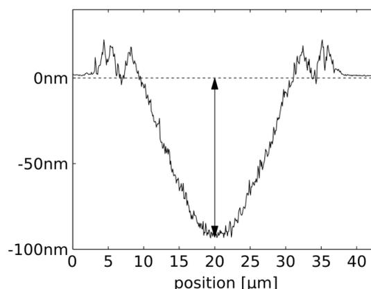
**Figure 9:** AFM image and height profile of an ablation hole generated by far-field ablation of bare Si (same wafer as in Figure 7). Note that the beam profile in this case is again described by an Airy distribution, comparable with the irradiation of the nanostructures.
