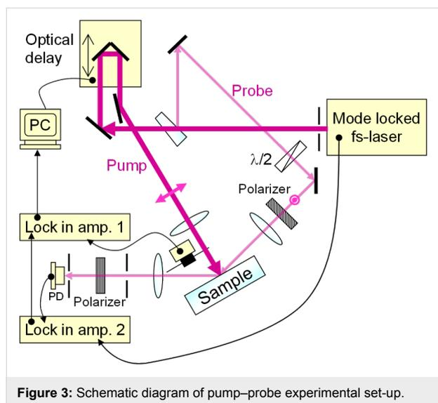
**Figure 3:** Schematic diagram of pump-probe experimental set-up.
