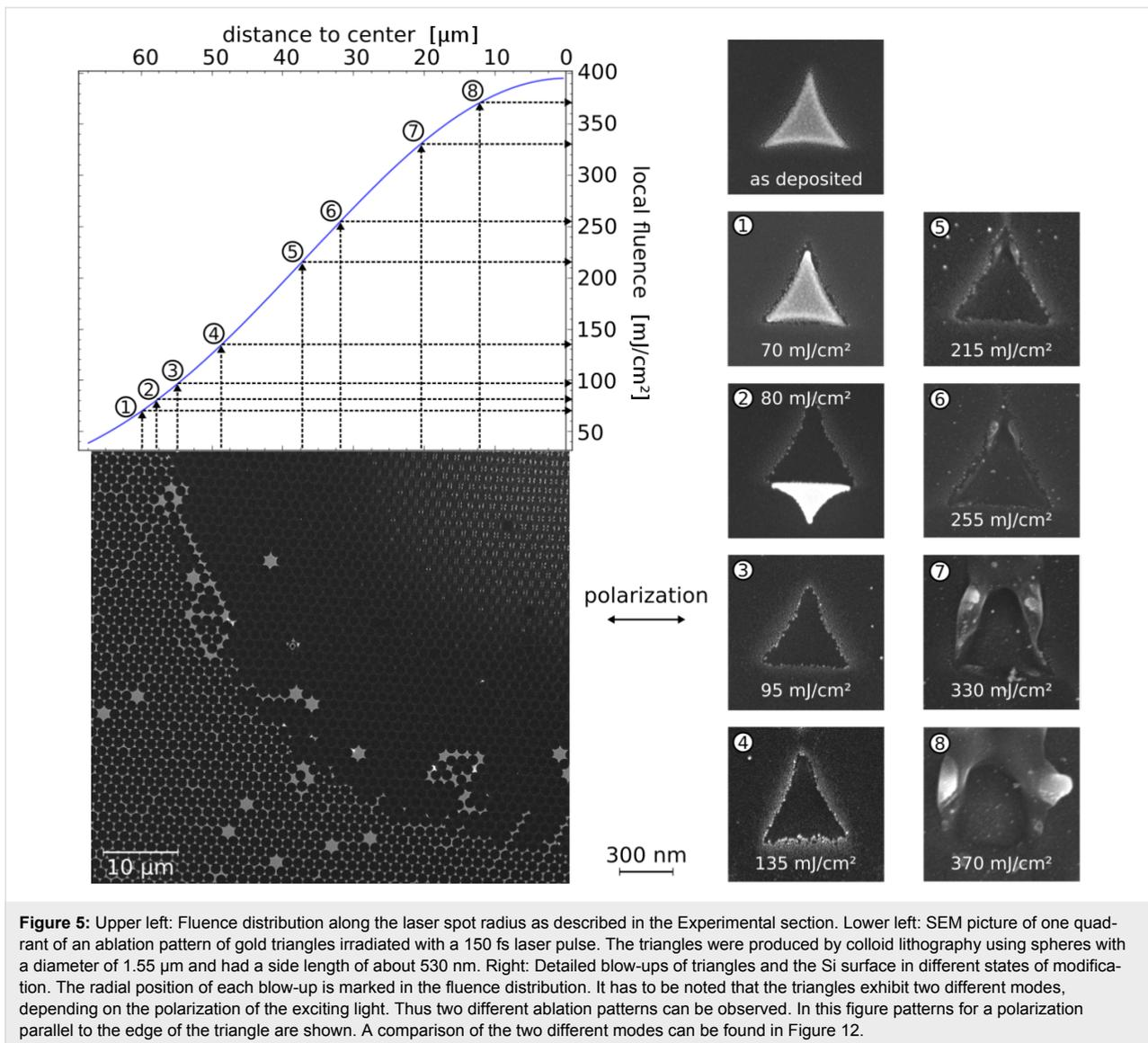
Scanning electron microscopy (SEM) and atomic force microscopy (AFM) were used for measuring the dimensions of the plasmonic structures as well as the resulting modifications of these structures and the substrate.
