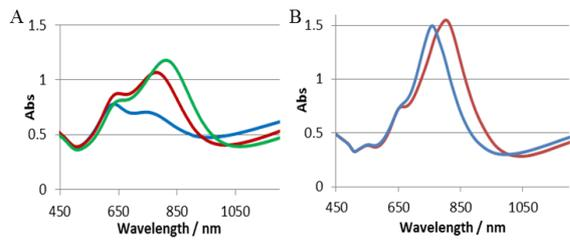
**Figure 6:** A) Extinction spectra of 110 nm PS particle gold cap/hole array with a gold film thickness of 30 nm where samples were not heated (blue) or post-heated to 116 °C (red) or 125 °C (green). B) Simulations of the non-heated structure in 6a (Blue) and with the cap lowered 10 nm (red).
