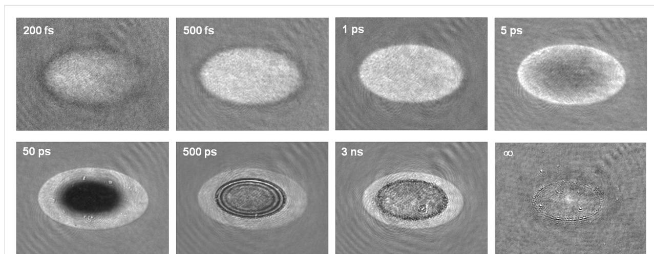
**Figure 3:** Surface reflectivity images of a particle-free c-Si surface exposed to a 120 fs laser pulse for different time delays between the excitation and illumination pulses. The peak fluence is 0.91 J/cm<sup>2</sup>. The frame size is 93 × 69 μm<sup>2</sup>. The brightness and contrast of each image have been adjusted to improve the visibility of the main features.
