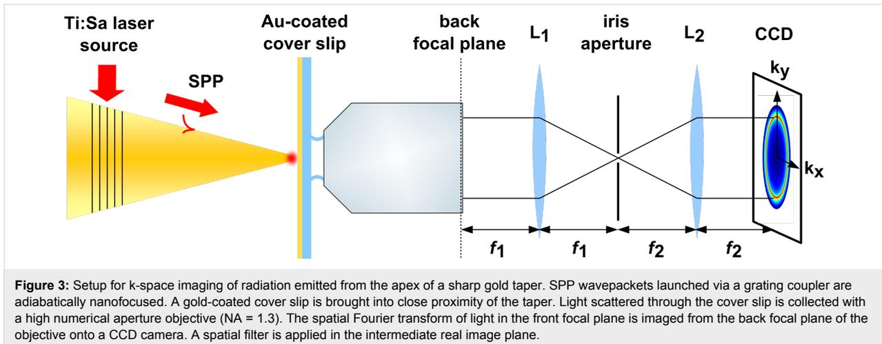
couples some fraction of the evanescent near-fields at the apex to propagating far-field modes. The angular distribution of these propagating waves is measured with an immersion objective. In the following, we describe the individual parts of the experimental setup.
