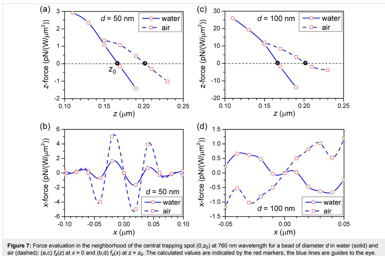
**Figure 7:** Force evaluation in the neighborhood of the central trapping spot  $(0, z_0)$  at 760 nm wavelength for a bead of diameter  $d$  in water (solid) and air (dashed): (a,c)  $f_z(z)$  at  $x=0$  and (b,d)  $f_x(x)$  at  $z=z_0$ . The calculated values are indicated by the red markers, the blue lines are guides to the eye.
