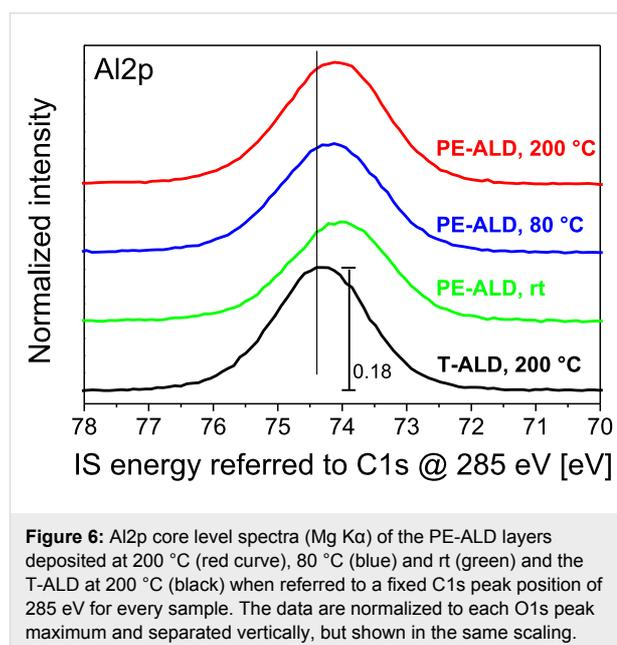
**Figure 6:** Al2p core level spectra (Mg K $\alpha$ ) of the PE-ALD layers deposited at 200 °C (red curve), 80 °C (blue) and rt (green) and the T-ALD at 200 °C (black) when referred to a fixed C1s peak position of 285 eV for every sample. The data are normalized to each O1s peak maximum and separated vertically, but shown in the same scaling.
