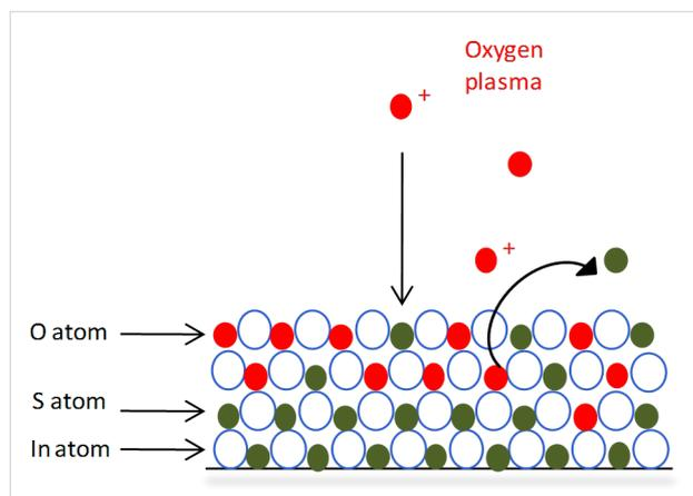
**Figure 7:** Surface mechanisms during the O<sub>2</sub> plasma pulse.
