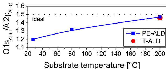
**Figure 8:** O1s to Al2p elemental ratio versus substrate temperature of PE-ALD layers (blue squares); the data point of the T-ALD film at 200 °C is included (red filled circle). Here, only the Al–O contributions were considered for the analysis. For orientation the ideal stoichiometric value is illustrated by the dashed line.
