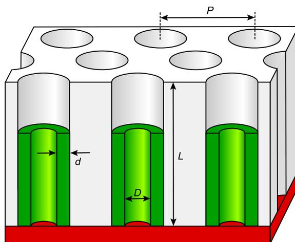
**Figure 1:** Schematic view of the proposed system, including all tunable geometric parameters. An inorganic matrix (white) defines cylindrical pores of length  $L$  and in a hexagonal order of period  $P$ . The silicon tubes (green) have a wall thickness  $d$  and an inner diameter  $D$ . The electrical contact is represented in red color.
