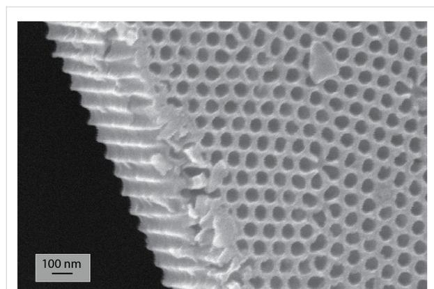
**Figure 14:** SEM micrograph of an anodic alumina oxide template. After the electropolishing, a sacrificial film was firstly grown by applying 40 V in 0.3 M  $\text{H}_2\text{C}_2\text{O}_4$  for 24 h at  $T = 8 \text{ }^\circ\text{C}$  and then dissolved in  $\text{H}_2\text{CrO}_4$  and  $\text{H}_3\text{PO}_4$  at  $50 \text{ }^\circ\text{C}$  for 12 h. The second anodization step is then carried out during 2.5 h at the same anodic conditions.
