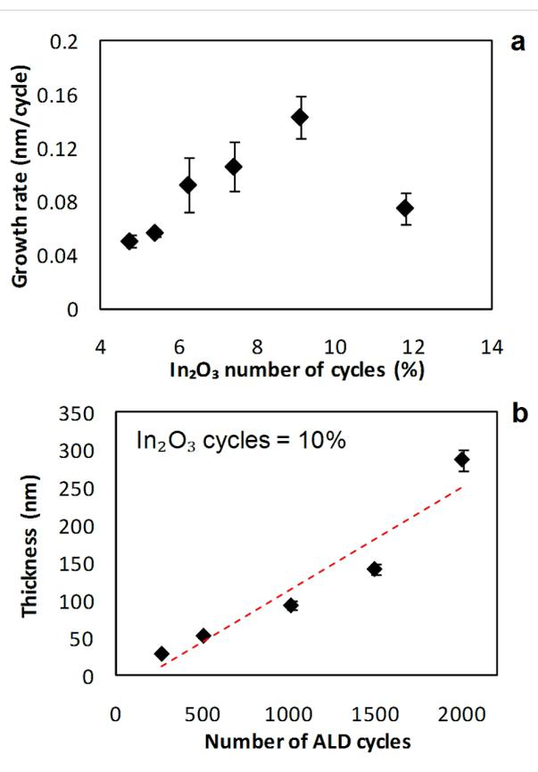
**Figure 4:** Influence of a) the number of  $\text{In}_2\text{O}_3$  cycles on the growth rate b) the number of process cycles on the film thickness when using  $\text{O}_2$  plasma as oxygen precursor. The dotted line is a guide to the eyes.
