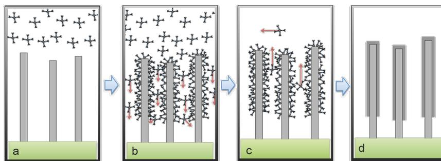
**Figure 1:** Illustration of one ALD cycle on a VACNT array. Upon exposure to the precursor gas (a: bulk gas diffusion), precursor molecules diffuse into the CNT array and adsorb onto available sites (b: confined diffusion and adsorption). After the defined precursor exposure time, purging of the ALD chamber removes unreacted precursor molecules from the chamber (c). After the oxidation pulse, a thin layer of oxide is formed on the surface (d).
