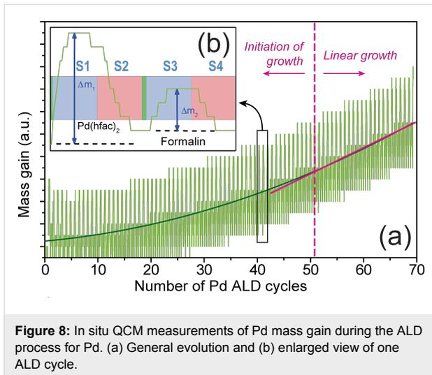
**Figure 8:** In situ QCM measurements of Pd mass gain during the ALD process for Pd. (a) General evolution and (b) enlarged view of one ALD cycle.
