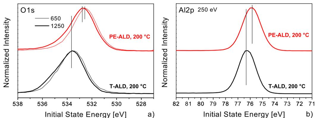
**Figure 9:** O1s (a) and Al2p (b) core level spectra of the PE-ALD (red curves) and T-ALD layers (black) deposited at 200 °C. These data were recorded with synchrotron excitation. The excitation energies were 650 eV (thick lines) and 1250 eV for the O1s and 250 eV for the Al2p, respectively. The data are normalized to each individual peak maximum and separated vertically, but shown in the same scaling. The IS energy is referred to Fermi energy.
