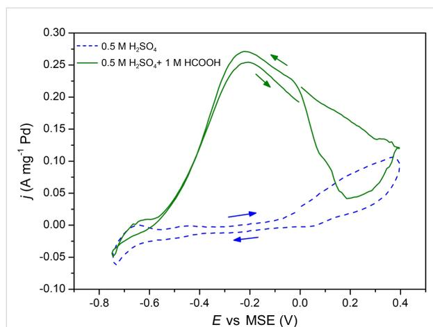
**Figure 12:** Cyclic voltammograms of Pd(100 ALD cycles)/Ni(1000 ALD cycles) catalysts in 0.5 M H<sub>2</sub>SO<sub>4</sub> without (blue dashed line) and with (continuous green line) 1 M HCOOH at 15 mV·s<sup>-1</sup>. Current densities are given per unit mass of Pd estimated from the QCM measurements.
