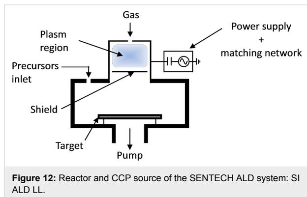
The true remote CCP source, driven by a 13.56 MHz generator, is attached to the upper flange of the reactor. During the deposition process the substrate is placed outside of the plasma generation region; the coated surface is not bombarded with destructive ions and does not see the light from plasma generation region.
