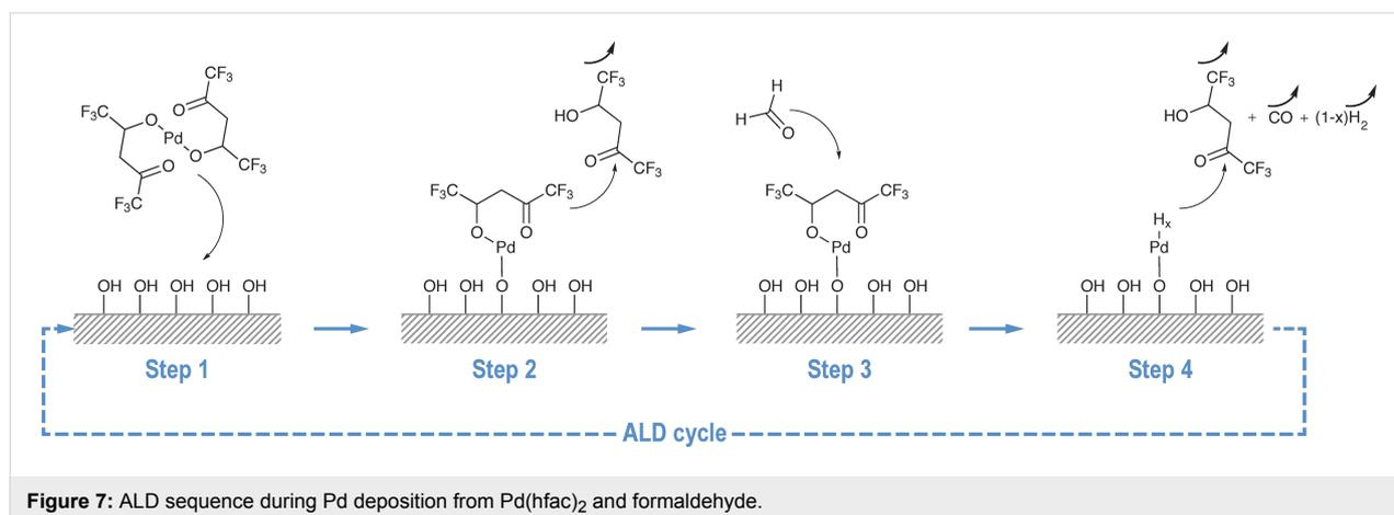
**Figure 7:** ALD sequence during Pd deposition from Pd(hfac)<sub>2</sub> and formaldehyde.
