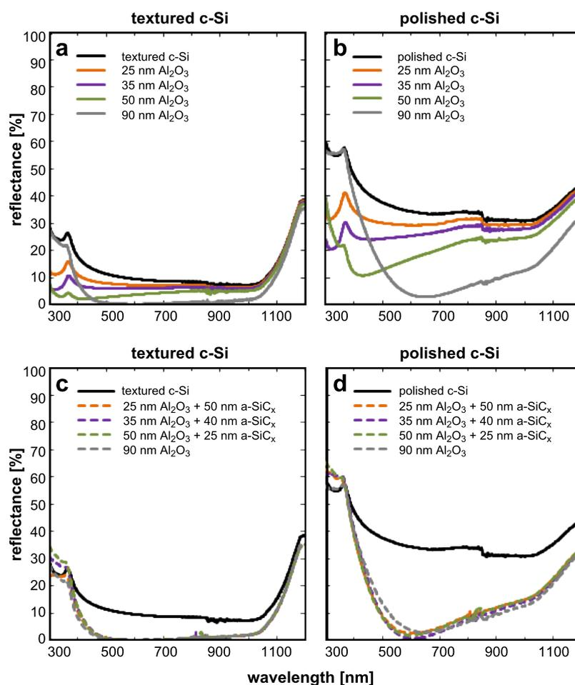
**Figure 3:** Reflectance curves of  $\text{Al}_2\text{O}_3$ -coated randomly textured c-Si (a) and polished c-Si (b) for different film thicknesses. Reflectance curves of  $\text{Al}_2\text{O}_3/\text{a-SiC}_x$  coated randomly textured c-Si (c) and polished c-Si (d). As a reference, bare polished and textured c-Si reflectances are also included (black line).
