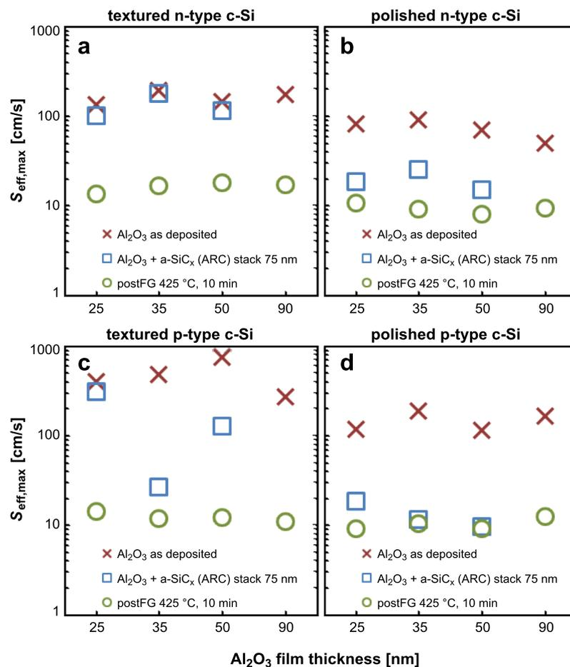
**Figure 1:** Surface recombination velocity,  $S_{\text{eff,max}}$  [cm/s]. (a) and (b)  $S_{\text{eff,max}}$  for randomly textured and polished n-type wafers respectively. (c) and (d)  $S_{\text{eff,max}}$  for randomly textured and polished p-type wafers respectively.  $S_{\text{eff,max}}$  was determined at 1-sun injection level as a function of the Al<sub>2</sub>O<sub>3</sub> thickness. The aluminum oxide layers were complemented up to 75 nm with an a-SiC<sub>x</sub> film.
