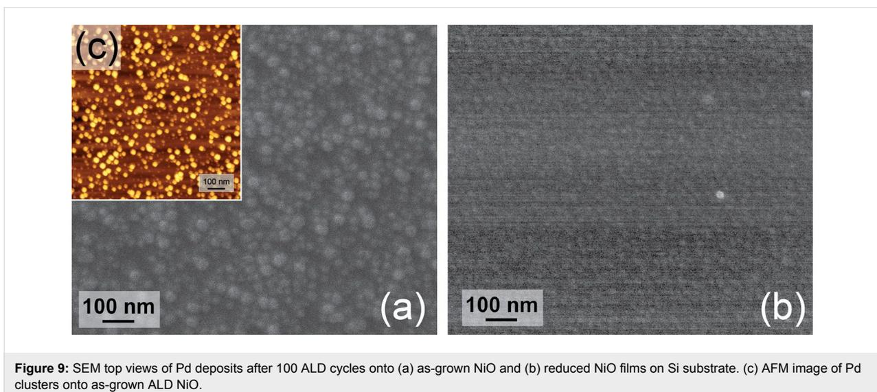
**Figure 9:** SEM top views of Pd deposits after 100 ALD cycles onto (a) as-grown NiO and (b) reduced NiO films on Si substrate. (c) AFM image of Pd clusters onto as-grown ALD NiO.
