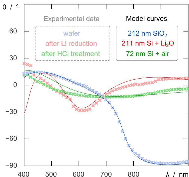
**Figure 4:** Spectroscopic ellipsometry of flat samples at various stages of preparation: initial substrate with  $\text{SiO}_2$  film (blue), after reaction with Li (red), and after acidic treatment and byproduct removal (green). The experimental data are shown as thick, light crosses, whereas the model curves calculated from the corresponding models are drawn as thin, dark lines.
