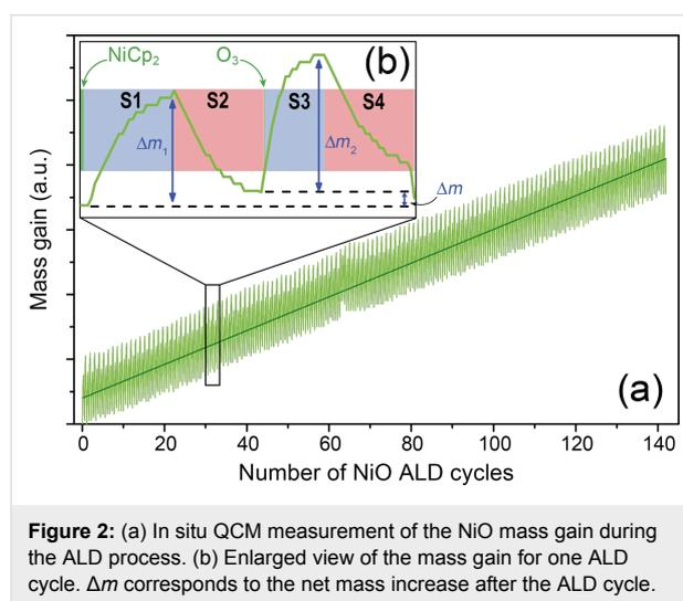
desorption of the precursors that have not reacted with active surface sites seems to occur. The net mass gain detected after the nickelocene pulse, exposure and purging could be attributed to the bonding of a –NiCp group with a surface –OH group.
