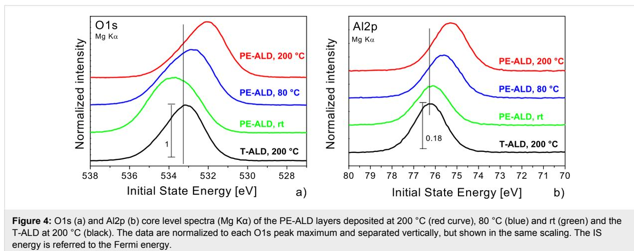
**Figure 4:** O1s (a) and Al2p (b) core level spectra (Mg K $\alpha$ ) of the PE-ALD layers deposited at 200 °C (red curve), 80 °C (blue) and rt (green) and the T-ALD at 200 °C (black). The data are normalized to each O1s peak maximum and separated vertically, but shown in the same scaling. The IS energy is referred to the Fermi energy.
