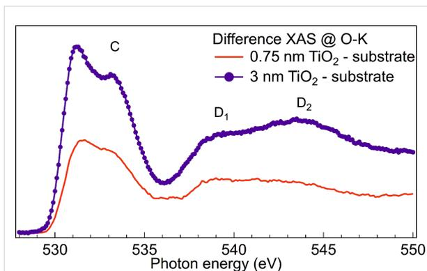
**Figure 3:** XAS difference spectra. The contribution of SiO<sub>2</sub> to the XAS at the O-K edge was subtracted from the measured spectra. Feature D of Figure 2 is now described by two features: D<sub>1</sub> and D<sub>2</sub>.
