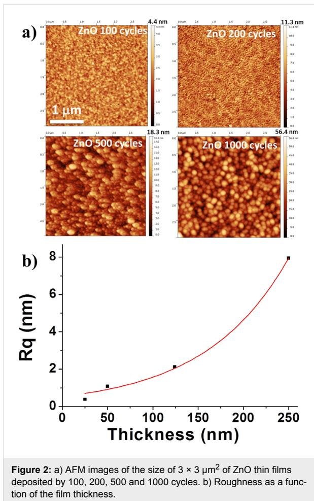
growth of vertically oriented columns with well-defined boundaries, an improvement of the crystalline structure (narrowing of XRD peaks), a crystalline growth and an alleviation of lattice strain, and an enhancement of the surface roughness and the texture coefficient.
