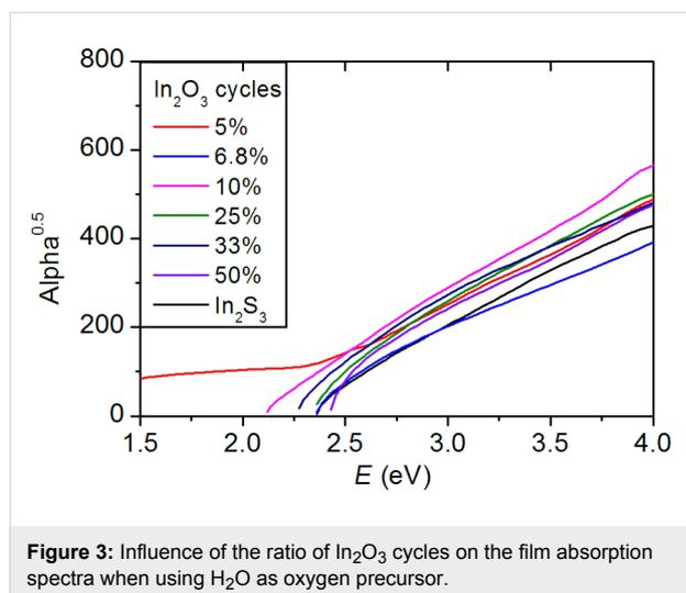
**Figure 3:** Influence of the ratio of  $\text{In}_2\text{O}_3$  cycles on the film absorption spectra when using  $\text{H}_2\text{O}$  as oxygen precursor.
