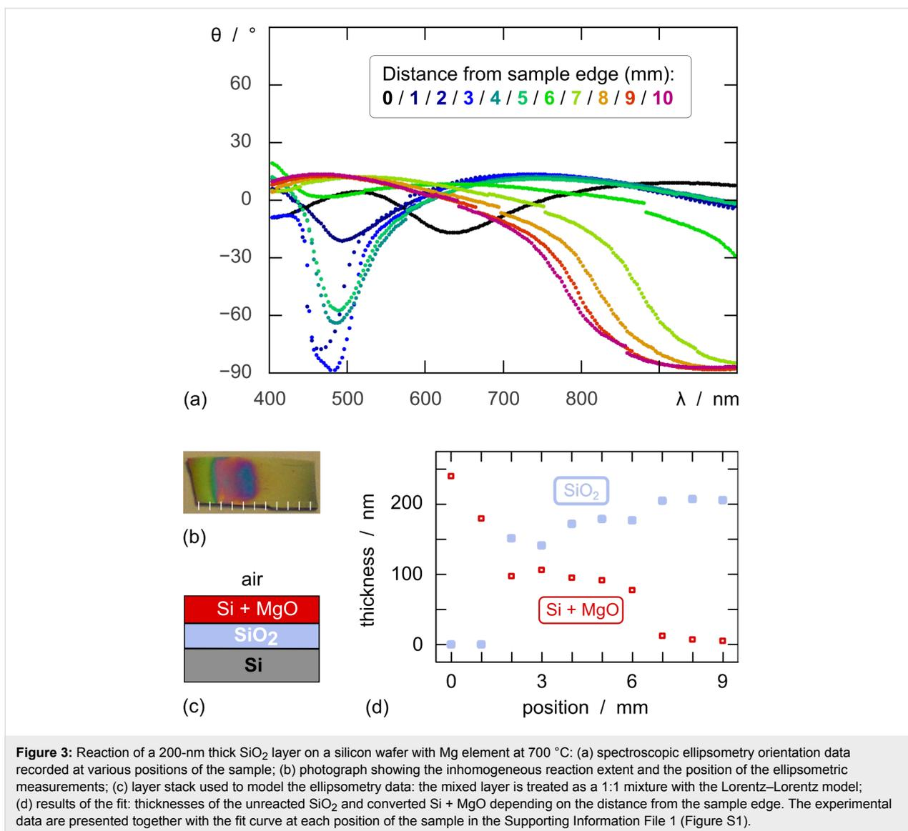
a clear picture emerges. The reaction extent transitions smoothly from 100% at position 0 to essentially 0% at a distance of 1 cm (Figure 3d and Figure S1 of Supporting Information File 1).
