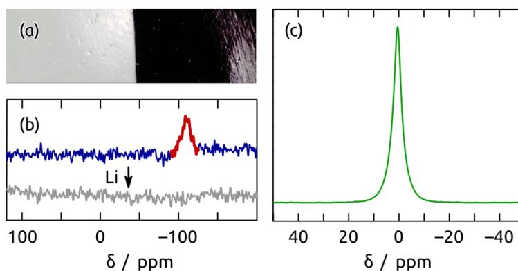
**Figure 5:** (a) Photograph of two nanoporous samples before and after the reduction by Li vapor with the subsequent acidic treatment (left and right, respectively). (b)  $^{29}\text{Si}$  MAS NMR spectra before and after reduction. (c)  $^7\text{Li}$  MAS NMR spectrum after reduction.
