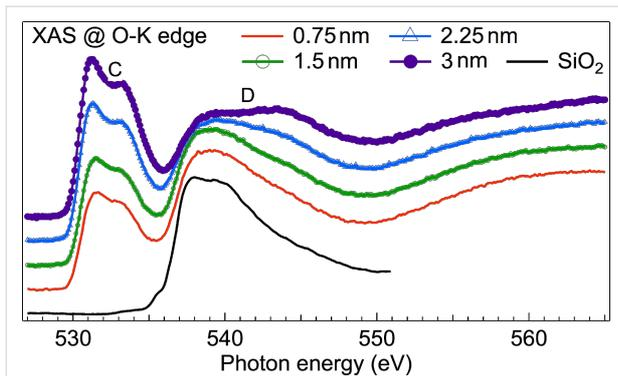
**Figure 2:** XAS at O-K edge measured for TiO<sub>2</sub> films with thicknesses of 0.75 nm, 1.5 nm, 2.25 nm and 3 nm. The XAS of native SiO<sub>2</sub> is also shown as reference. Spectra were normalized to the same intensity at 580 eV and vertically offset.
