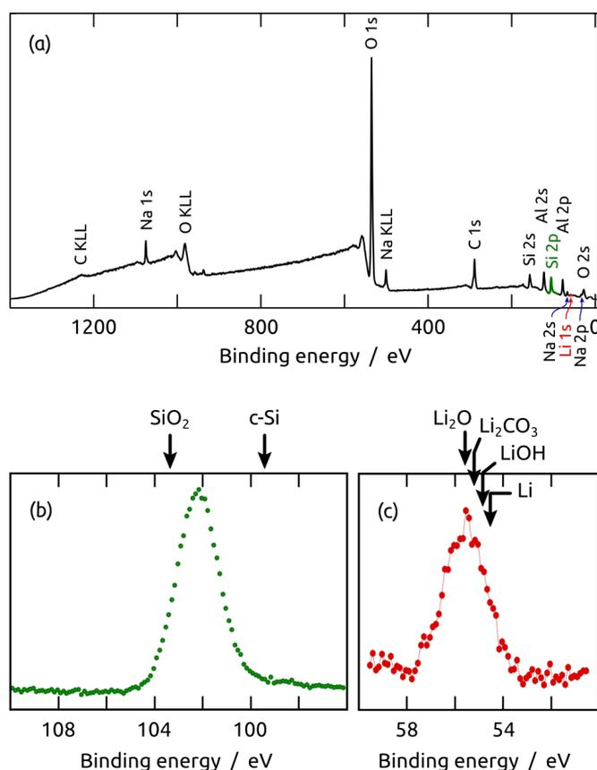
**Figure 6:** X-ray photoelectron spectrum of a Si nanotube sample at the end of the preparation: (a) survey spectrum, (b) Si 2p peak, and (c) Li 1s peak. The XPS peak positions of reference compounds are given by arrows.
