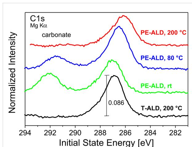
**Figure 5:** C1s core level spectra (Mg K $\alpha$ ) of the PE-ALD layers deposited at 200 °C (red curve), 80 °C (blue) and rt (green) and the T-ALD at 200 °C (black). The data are normalized to each O1s peak maximum and separated vertically, but shown in the same scaling. The energy is referred to the Fermi energy.
