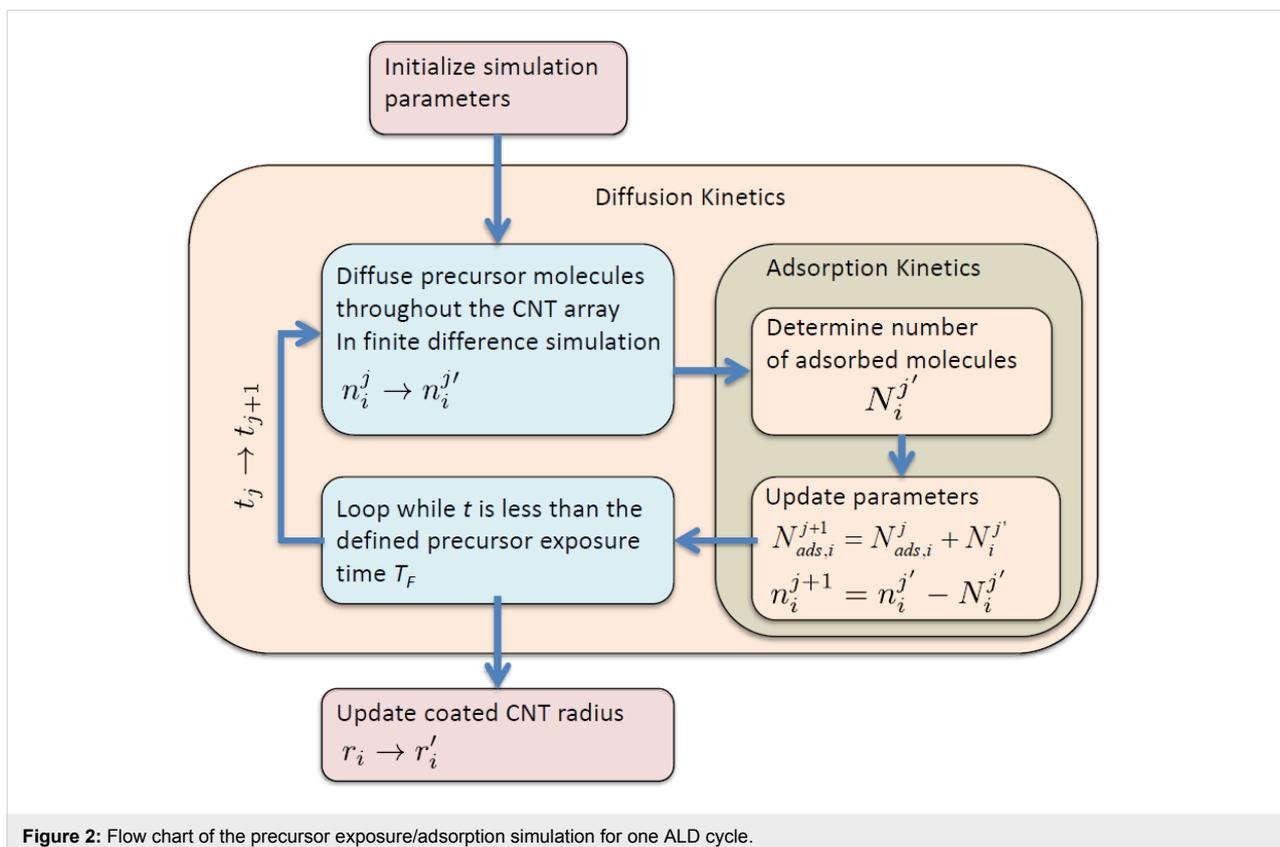
**Figure 2:** Flow chart of the precursor exposure/adsorption simulation for one ALD cycle.
