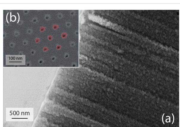
**Figure 3:** (a) SEM cross section of a NiO layer deposited in AAO membrane. (b) SEM image (obtained in backscattering electron mode) showing NiO grown by ALD within the AAO template. The NiO top layer has been removed by a short Ar sputtering in order to reveal the NiO film coating the vertical pore walls. The NiO deposit is emphasized on the picture using a red overlay.
