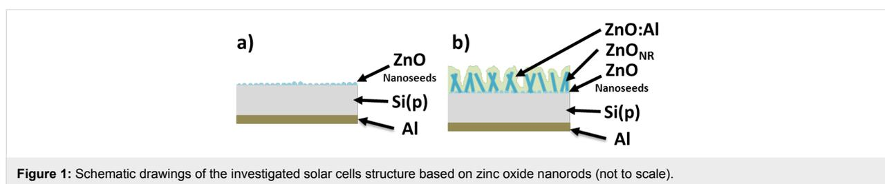
**Figure 1:** Schematic drawings of the investigated solar cells structure based on zinc oxide nanorods (not to scale).
