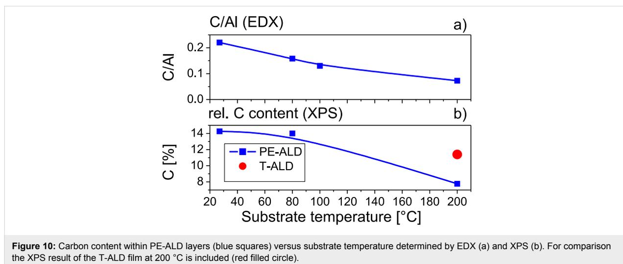
**Figure 10:** Carbon content within PE-ALD layers (blue squares) versus substrate temperature determined by EDX (a) and XPS (b). For comparison the XPS result of the T-ALD film at 200 °C is included (red filled circle).
