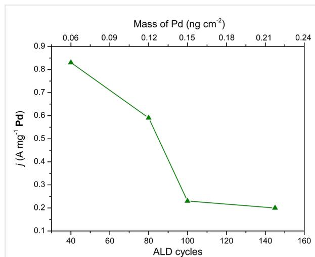
**Figure 13:** Peak current densities of the electrooxidation of 1 M HCOOH in 0.5 M H<sub>2</sub>SO<sub>4</sub> with various Pd contents in the Pd/Ni nanocatalysts, which were obtained with 40 to 145 Pd ALD cycles. The mass of Pd was estimated from the QCM measurements.
