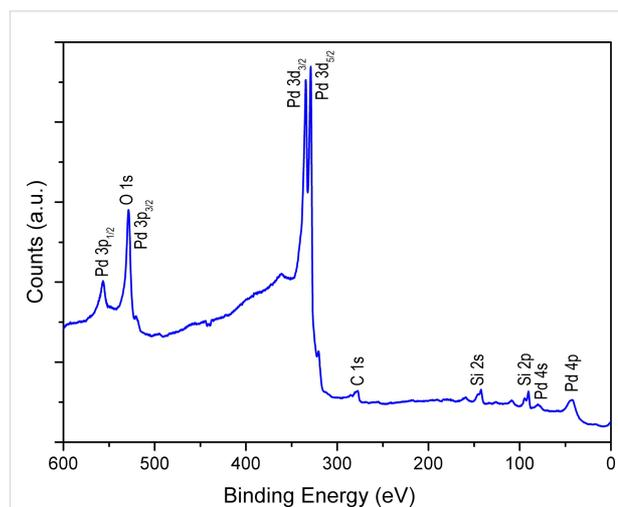
**Figure 11:** XPS survey spectrum of metallic Pd.
