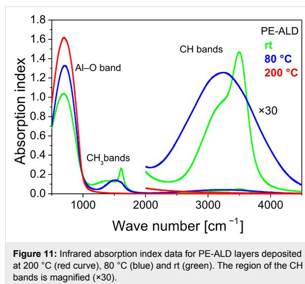
**Figure 11:** Infrared absorption index data for PE-ALD layers deposited at 200 °C (red curve), 80 °C (blue) and rt (green). The region of the CH bands is magnified ( $\times 30$ ).
