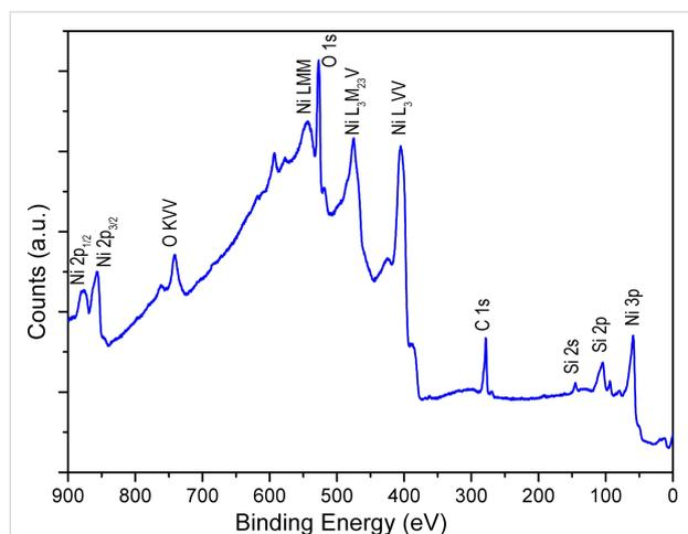
**Figure 6:** XPS survey spectrum of metallic Ni.
