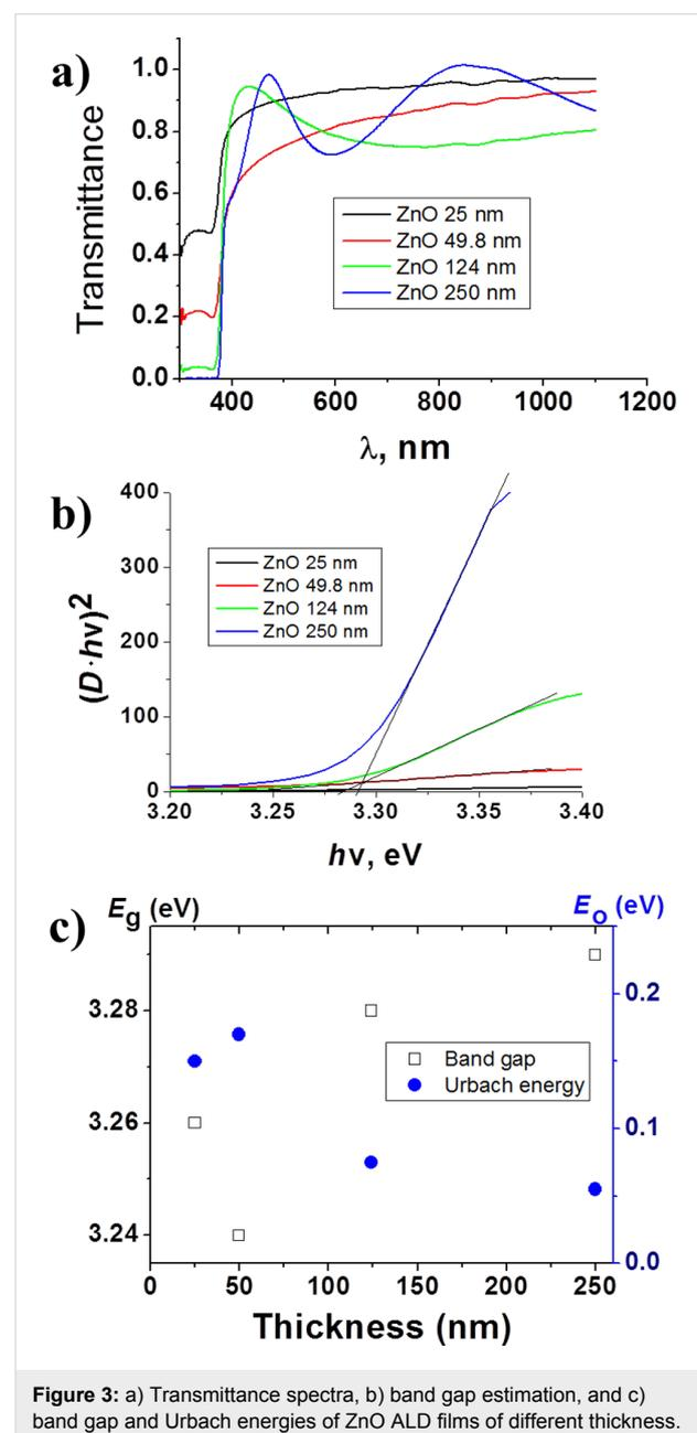
The structure of 25 nm thick films is amorphous. The films might contain crystallites with a size of less than 3 nm which are difficult to detect by XRD. In this case, a band gap broadening due to the quantum confinement effect would be expected. However, results obtained from 25 nm films do not show any significant increase of the band gap value. This hints at an absence of small crystallites in the amorphous structure of the films.
