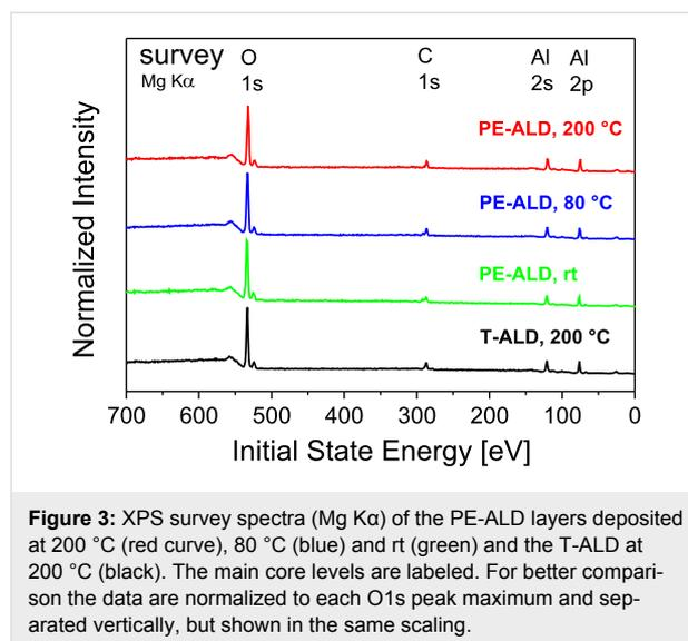
**Figure 3:** XPS survey spectra (Mg K $\alpha$ ) of the PE-ALD layers deposited at 200 °C (red curve), 80 °C (blue) and rt (green) and the T-ALD at 200 °C (black). The main core levels are labeled. For better comparison the data are normalized to each O1s peak maximum and separated vertically, but shown in the same scaling.
