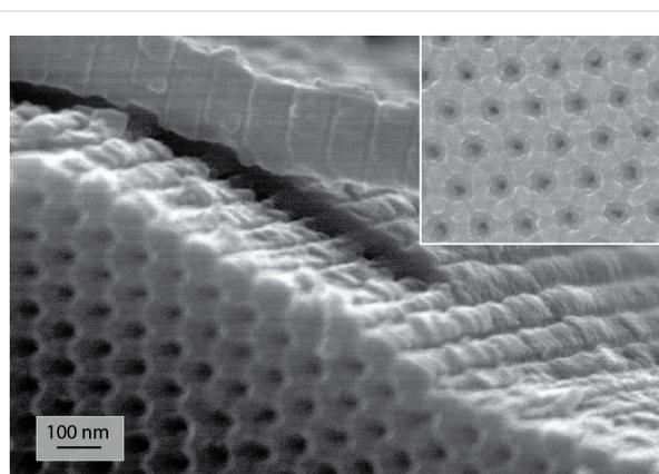
**Figure 5:** SEM image of Ni layer deposited in an AAO template after 3 h annealing in H<sub>2</sub> at 300 °C of the initially deposited NiO by ALD. The inset shows a detailed top-view of the surface.
