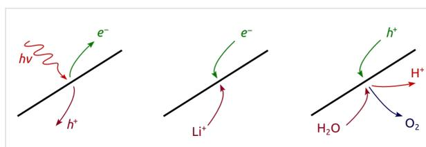
**Figure 1:** Nature of the charge carriers combining or separating at an interface in a solar cell (left), a lithium ion battery (center), and the water oxidation electrode of an electrolyzer (or the oxygen-evolving complex in photosynthesis, right).
