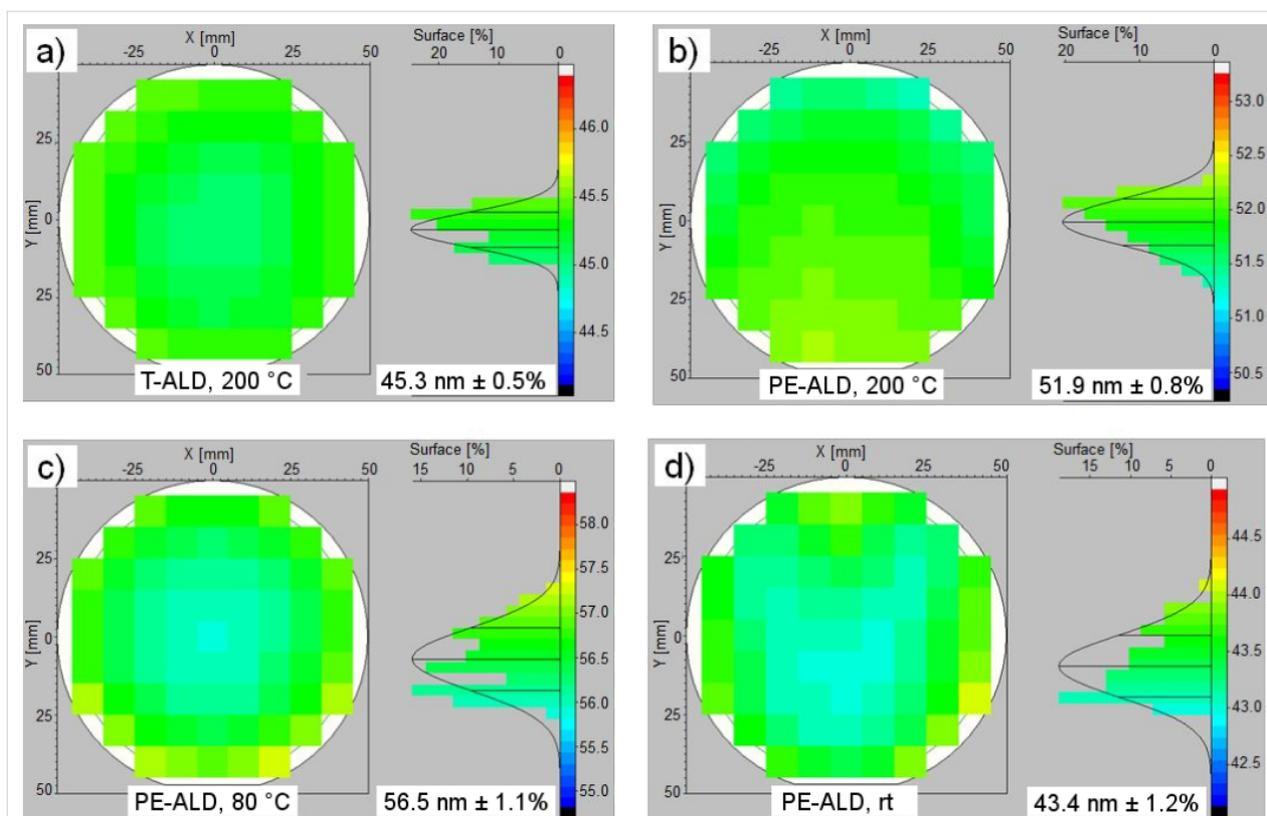
**Figure 1:** Thickness distributions of T-ALD at 200 °C (a) and PE-ALD films at 200 °C (b), 80 °C (c) and rt (d). The data were recorded by ellipsometry. The left part of every fraction shows the thickness distribution over 4 inch wafers ( $\varnothing = 100$  mm) and the right part its statistics. The thickness average and the uniformity of the layer over the 4 inch wafer are given within the graphs.
