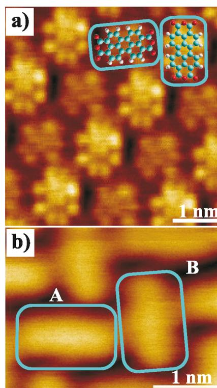
**Figure 1:** (a) STM topography scan ( $V = 0.2$  V,  $I = 0.3$  nA) of PTCDA on Ag(111). The two molecule orientations (turquoise rectangles) of the unit cell correspond to different adsorption geometries and are imaged with a different intensity. (b) NC-AFM topography scan ( $\Delta f = -0.6$  Hz) of the surface area where the 3D force spectroscopy measurement was performed. No difference between the two orientations is detectable.
