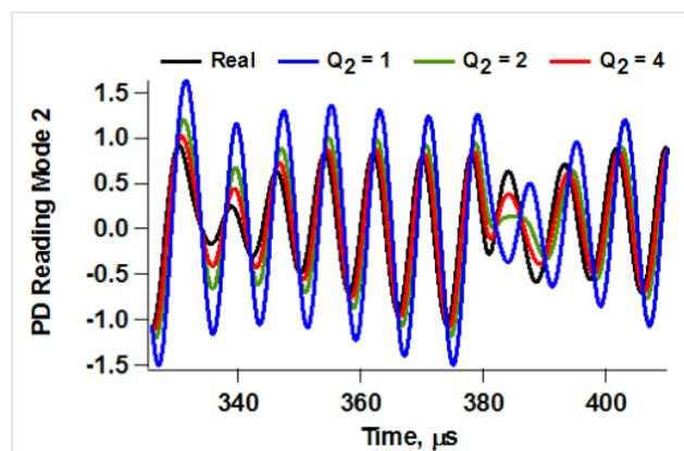
**Figure 9:** Illustration of the photodetector (PD) reading that would be obtained for a given second eigenmode trajectory (taken from a tip-excited bimodal simulation) for different values of the quality factor when the cantilever is driven using base excitation. There is a clear discrepancy between the photodetector reading and the real trajectory as  $Q$  drops.
