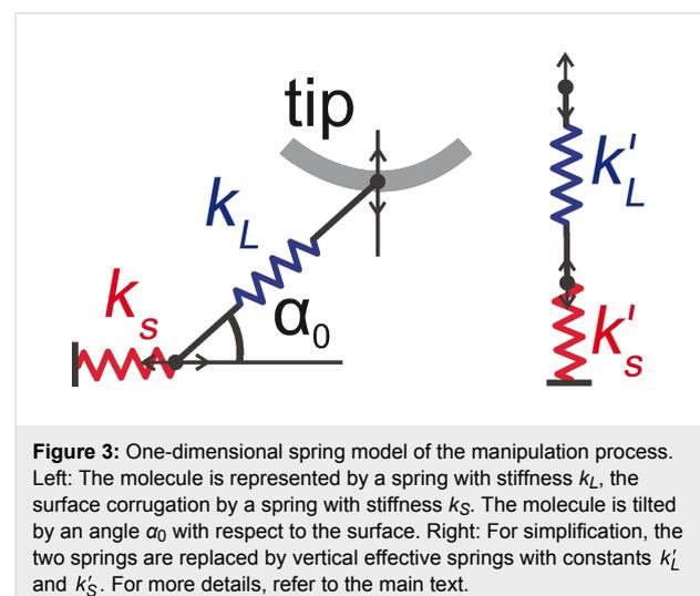
**Figure 3:** One-dimensional spring model of the manipulation process. Left: The molecule is represented by a spring with stiffness  $k_L$ , the surface corrugation by a spring with stiffness  $k_S$ . The molecule is tilted by an angle  $\alpha_0$  with respect to the surface. Right: For simplification, the two springs are replaced by vertical effective springs with constants  $k'_L$  and  $k'_S$ . For more details, refer to the main text.
