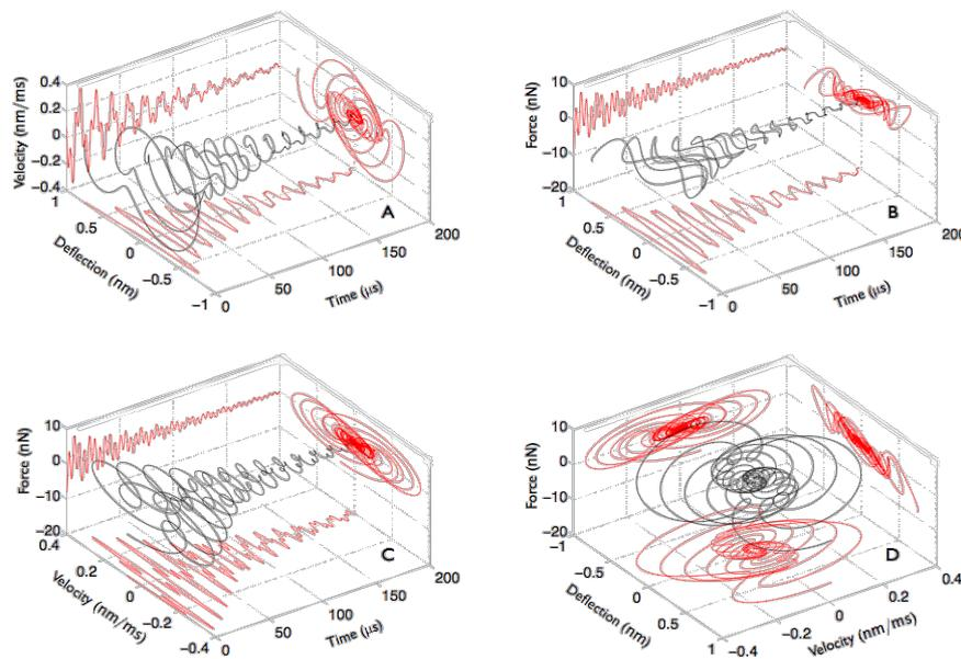
**Figure 3:** 3D-representation of the main observables describing the tip dynamics during the jump-to-contact transition. (A) deflection–velocity, (B) deflection–force and (C) velocity–force phase-spaces evolving in time. (D) Force vs velocity vs displacement phase-space representation.
