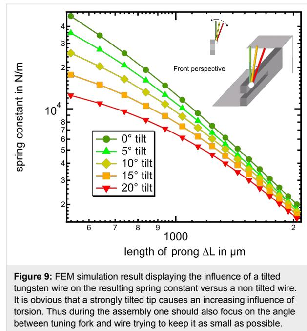
**Figure 9:** FEM simulation result displaying the influence of a tilted tungsten wire on the resulting spring constant versus a non tilted wire. It is obvious that a strongly tilted tip causes an increasing influence of torsion. Thus during the assembly one should also focus on the angle between tuning fork and wire trying to keep it as small as possible.
