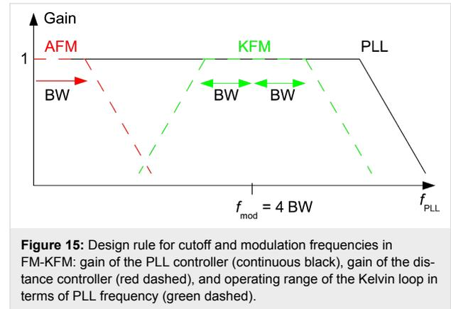
**Figure 15:** Design rule for cutoff and modulation frequencies in FM-KFM: gain of the PLL controller (continuous black), gain of the distance controller (red dashed), and operating range of the Kelvin loop in terms of PLL frequency (green dashed).
