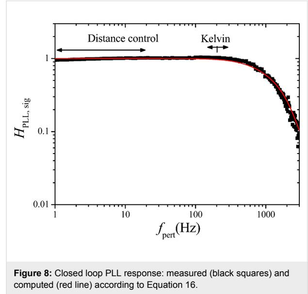
**Figure 8:** Closed loop PLL response: measured (black squares) and computed (red line) according to Equation 16.
