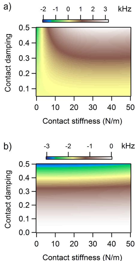
**Figure 9:** The frequency error introduced by a PLL in measuring the shift of the contact resonance frequency of (a) the first and (b) second eigenmodes in the UAFM configuration as a function of contact stiffness and contact damping. The corresponding frequency shifts over the investigated contact stiffness and contact damping ranges are shown in Figure 7a and Figure 8a for the two eigenmodes, respectively.
