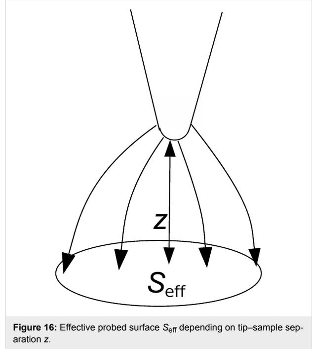
**Figure 16:** Effective probed surface  $S_{\text{eff}}$  depending on tip–sample separation  $z$ .
