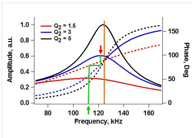
**Figure 10:** Cantilever amplitude and phase response for various levels of damping in low- $Q$  environments. The thick red and green arrows and the green line illustrate the nature of the errors made in determining the resonance frequency when a frequency modulation operation is locked to the peak frequency instead of the natural frequency (see discussion in the text).
