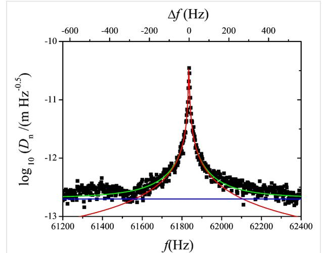
**Figure 5:** Noise PSD at the photodetector output. Fitted with Equation 9 (green) and decomposition into thermal excitation noise (red) and constant detector noise  $z_{n,S}$  (blue).
