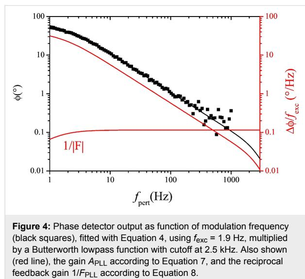
**Figure 4:** Phase detector output as function of modulation frequency (black squares), fitted with Equation 4, using  $f_{\text{exc}} = 1.9$  Hz, multiplied by a Butterworth lowpass function with cutoff at 2.5 kHz. Also shown (red line), the gain  $A_{\text{PLL}}$  according to Equation 7, and the reciprocal feedback gain  $1/F_{\text{PLL}}$  according to Equation 8.
