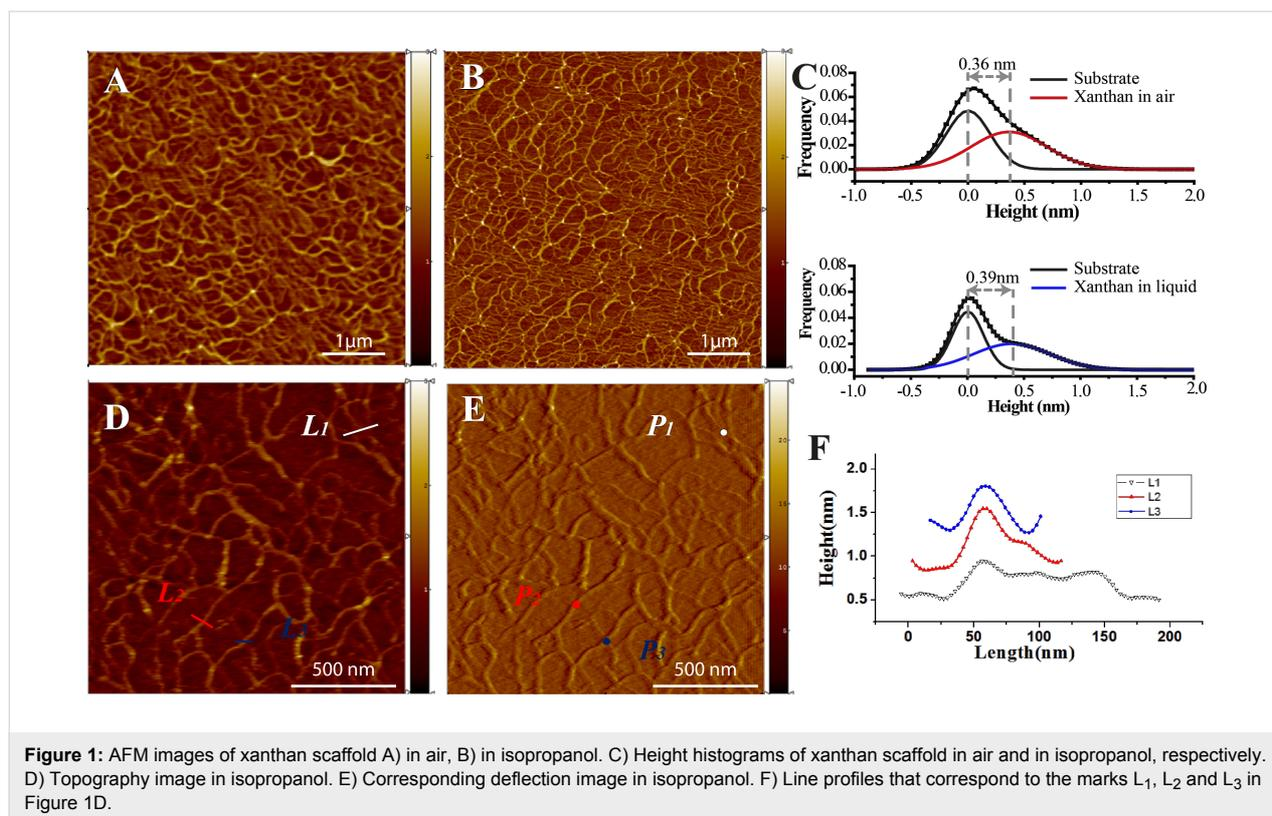
**Figure 1:** AFM images of xanthan scaffold A) in air, B) in isopropanol. C) Height histograms of xanthan scaffold in air and in isopropanol, respectively. D) Topography image in isopropanol. E) Corresponding deflection image in isopropanol. F) Line profiles that correspond to the marks  $L_1$ ,  $L_2$  and  $L_3$  in Figure 1D.
