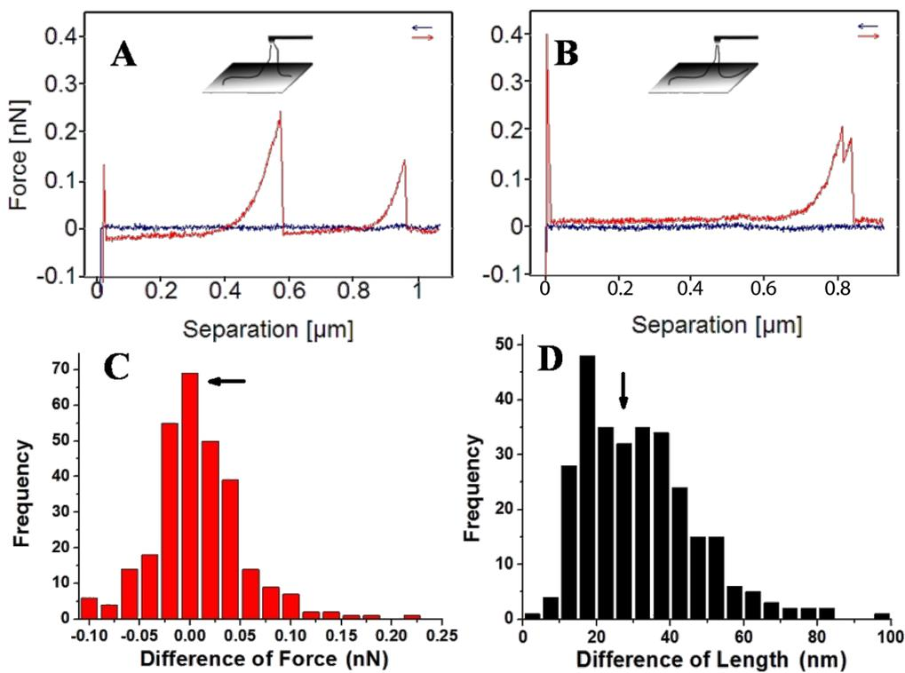
**Figure 6:** A) Typical double-peak force curve. B) "type 3" ( $t_3$ ) force curve. C,D) histograms of the differences between the rupture forces and rupture lengths of the two continuous peaks in  $t_3$  force curves.
