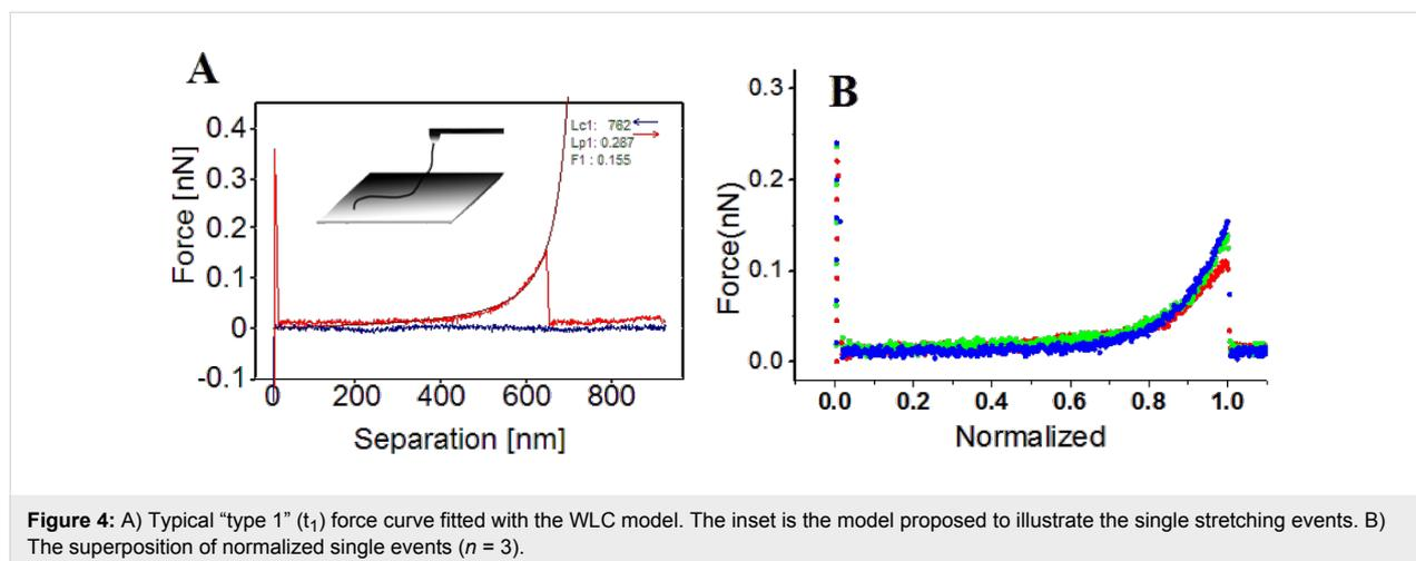
**Figure 4:** A) Typical “type 1” ( $t_1$ ) force curve fitted with the WLC model. The inset is the model proposed to illustrate the single stretching events. B) The superposition of normalized single events ( $n = 3$ ).
