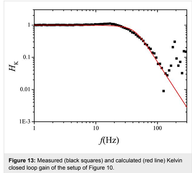
**Figure 13:** Measured (black squares) and calculated (red line) Kelvin closed loop gain of the setup of Figure 10.
