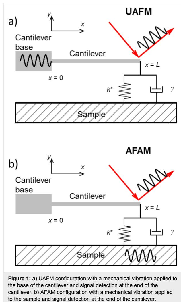
**Figure 1:** a) UAFM configuration with a mechanical vibration applied to the base of the cantilever and signal detection at the end of the cantilever. b) AFAM configuration with a mechanical vibration applied to the sample and signal detection at the end of the cantilever.
