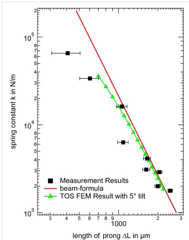
**Figure 10:** Comparison of the spring constants from experiment with FEM simulations and calculations using the beam formula (with the new origin  $L_0 = -250 \mu\text{m}$  for both). The experimental values still show a deviation from the simulations and calculation respectively. This is possibly caused by some tilt of the sensor towards the force application axis where small angles cannot be completely avoided in the fabrication procedure.
