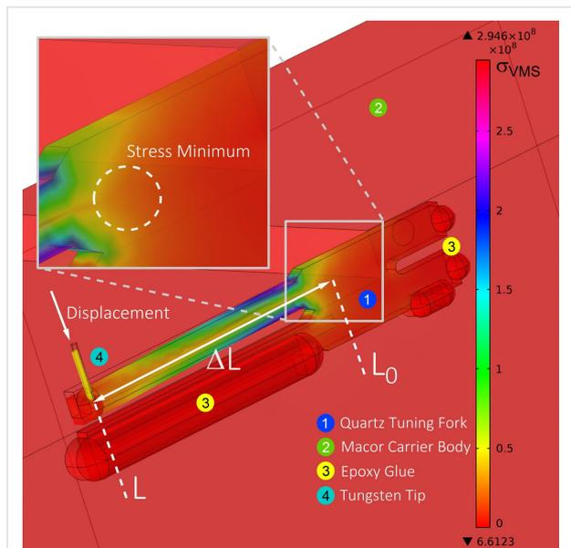
**Figure 5:** FEM simulation of von Mises stress. Analysis of the stress caused by the bending of the free prong. In contrast to the model for the beam formula, in which a cantilever is fixed at one end, the stress in the quartz tuning fork reaches beyond the end of the prong far into the basis of the tuning fork. The origin of the minimal Van Mises stress is indicated by the dashed circle (see inset).
