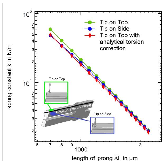
**Figure 8:** Comparison between tip on side (TOS) and tip on top (TOT) configurations as possible origin of the deviation between FEM Simulation and Experiment. The deviation was found to be larger in case of TOT than the contribution of torsion in the TOS configuration.
