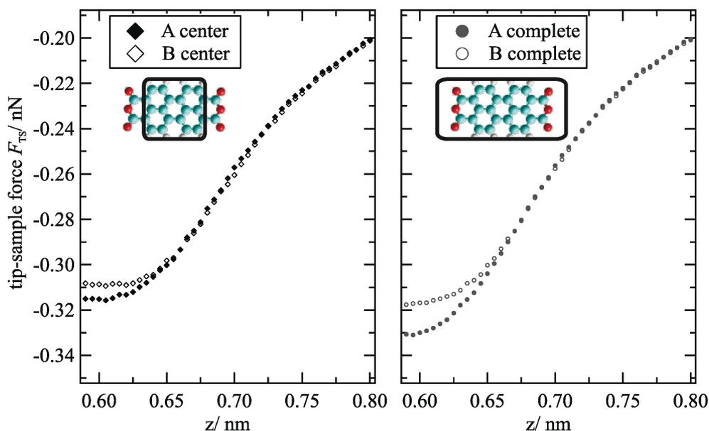
**Figure 5:** Comparison of force versus distance curves for molecule sites A and B. The forces are averaged for the perylene core (left) and the complete molecule (right) as indicated in the sketches of the molecules. At  $z$  distances below 0.65 nm, higher attractive forces are acting at molecule A.
