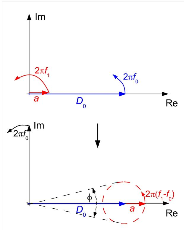
**Figure 6:** Vector diagram showing the impact of amplitude noise on phase noise in the complex plain: main vector and a small perturbation of amplitudes  $D_0$  and  $a$  and at frequencies  $f_0$  and  $f_1$  respectively (upper drawing) and their resulting sum in the reference plane rotating at  $f_0$  (lower drawing).
