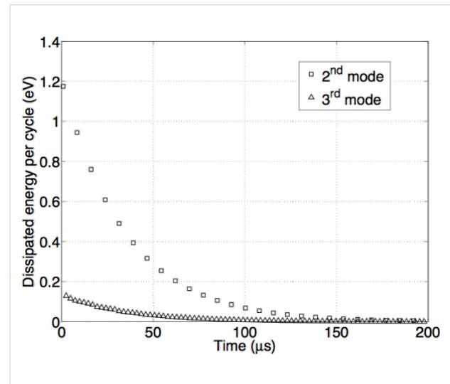
**Figure 2:** Dissipated energy per cycle vs time in each mode contributing to the dynamics described in Figure 3.
