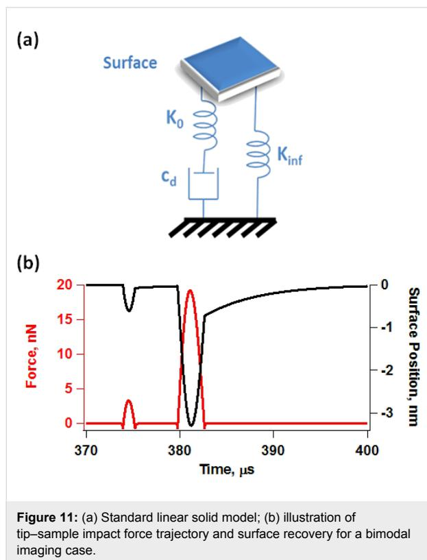
**Figure 11:** (a) Standard linear solid model; (b) illustration of tip–sample impact force trajectory and surface recovery for a bimodal imaging case.
