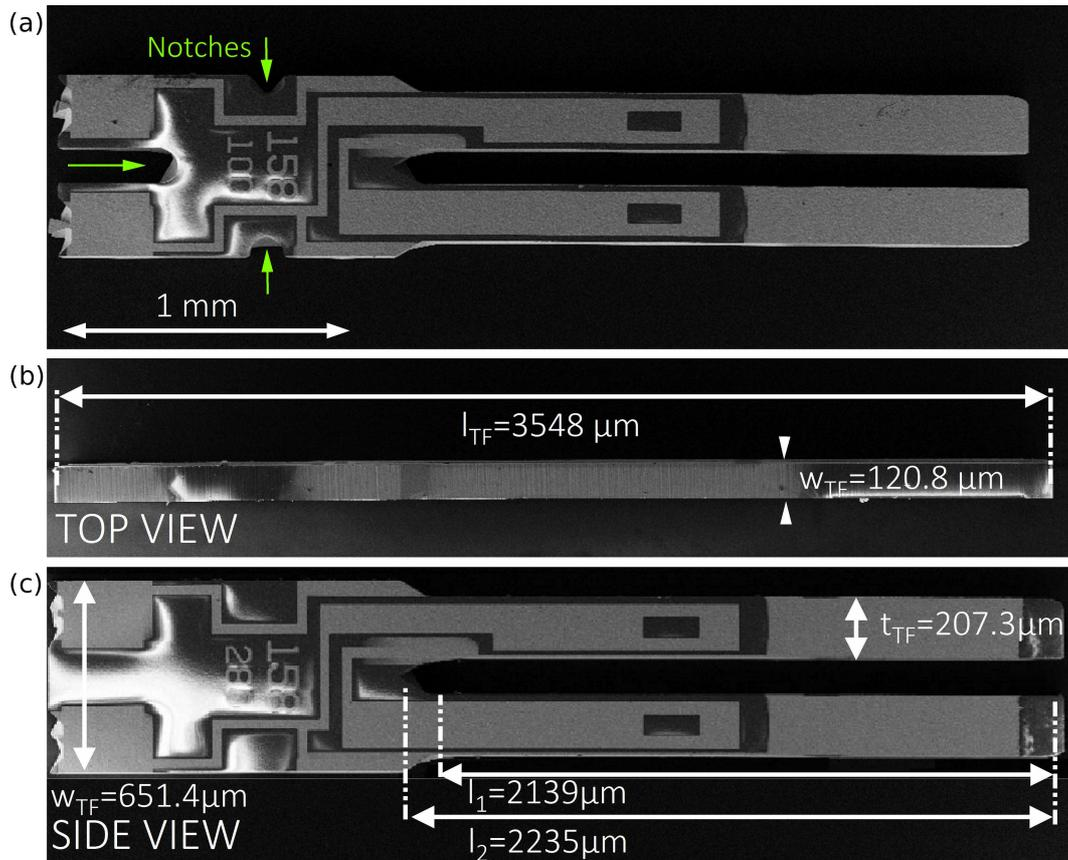
**Figure 1:** Determination of the geometric dimensions of a quartz tuning fork (Micro Crystal, type DS26 used for “qPlus”-force sensors from SEM images. (a) Sideview of tuning fork made from quartz with notches (cf. arrows) at the basis. (b) Topview of the tuning fork for measuring its width by the wafer thickness. (c) Sideview of an alternative geometric layout of DS26-type tuning fork without notches at the basis.
