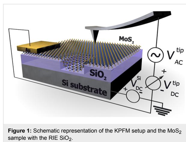
**Figure 1:** Schematic representation of the KPFM setup and the MoS<sub>2</sub> sample with the RIE SiO<sub>2</sub>.
