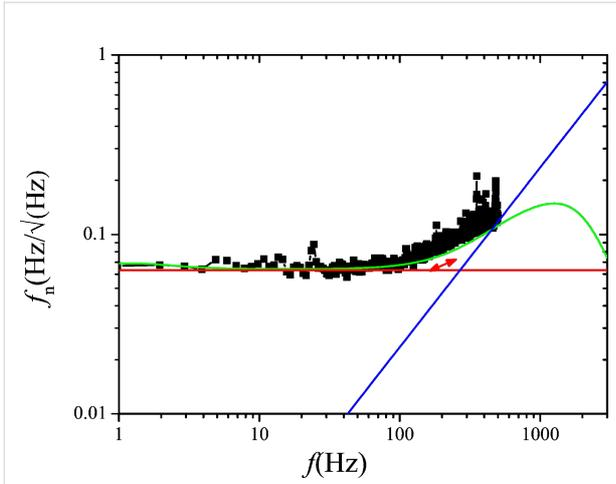
**Figure 9:** Output noise PSD of the PLL in closed loop configuration: measured (black squares) and modeled according to Equation 18 (green) from the previously determined gains and phase noise spectrum. The decomposition into thermal excitation contribution (red, constant) and detector noise (blue, rising) are also shown; the decomposed spectra were modeled with simplified noise gains  $H_{\text{noise,PLL}} \approx 1/|A_{\text{PLL}}|$ .
