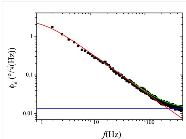
**Figure 7:** Phase noise PSD at the lock-in phase detector output in open PLL loop and under probe excitation at  $D_0 = 0.75$  nm: measured (black squares), fitted according to Equation 15 (green), and decomposed into detector noise (blue, constant) and thermal excitation contribution (red, lowpass) according to the two terms of Equation 15.
