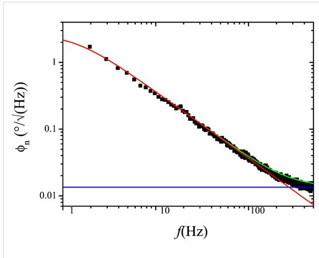
**Figure 7:** Phase noise PSD at the lock-in phase detector output in open PLL loop and under probe excitation at  $D_0 = 0.75$  nm: measured (black squares), fitted according to Equation 15 (green), and decomposed into detector noise (blue, constant) and thermal excitation contribution (red, lowpass) according to the two terms of Equation 15.
