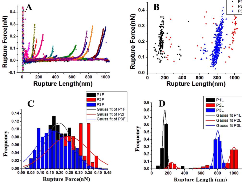
**Figure 3:** A) Schematic diagram of the superposition of force curves with single events. B) Distributions of rupture length and rupture force of various single events obtained by manipulating distinctive structures  $P_1$ ,  $P_2$  and  $P_3$ . C, D) The frequency distributions of rupture force and rupture length.
