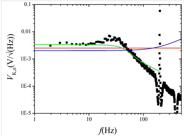
**Figure 14:** Measured (black squares) and computed (green line) Kelvin closed loop noise PSD of the setup of Figure 10. Also shown is the decomposition into thermal (red, constant) and sensor (blue, rising above 200 Hz) noise, calculated by using the approximate noise gain.
