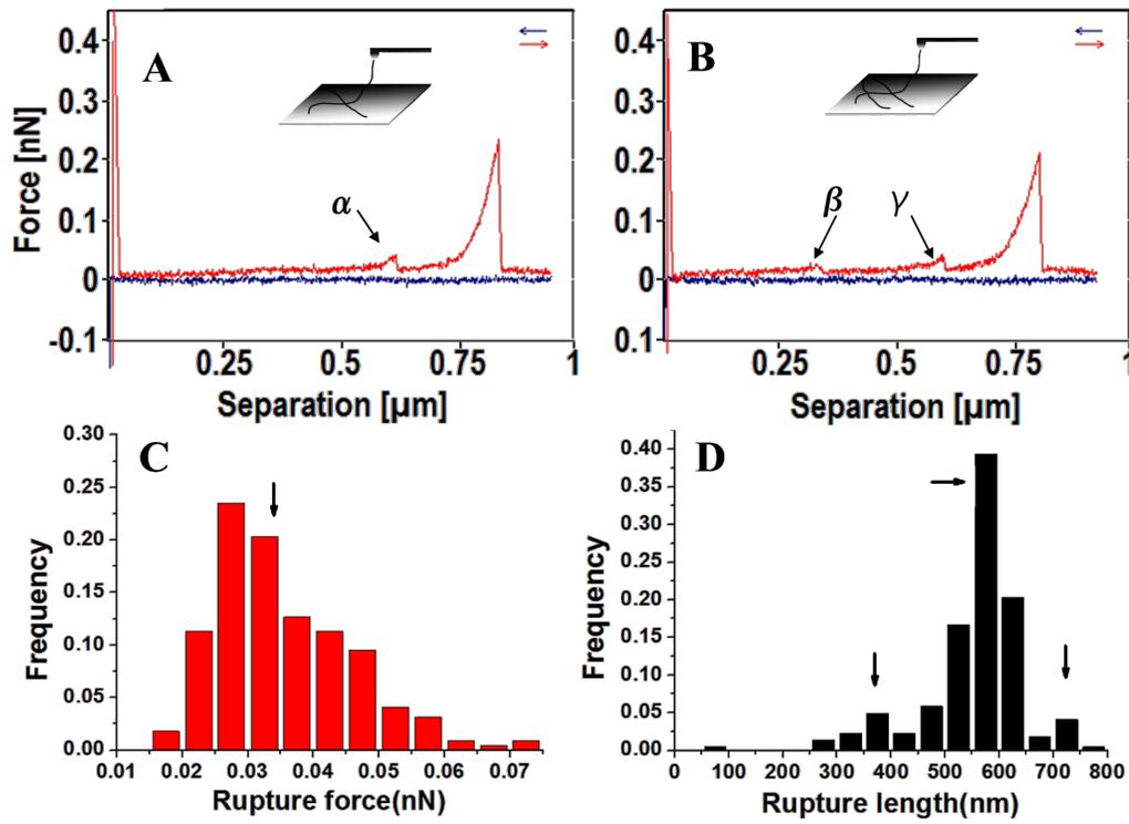
**Figure 5:** A,B) Typical single stretching event with one and two kinks (type 2), the insets are the proposed models. C,D) The frequency distributions of rupture force and rupture length of kinks in force curves with only one kink, respectively.
