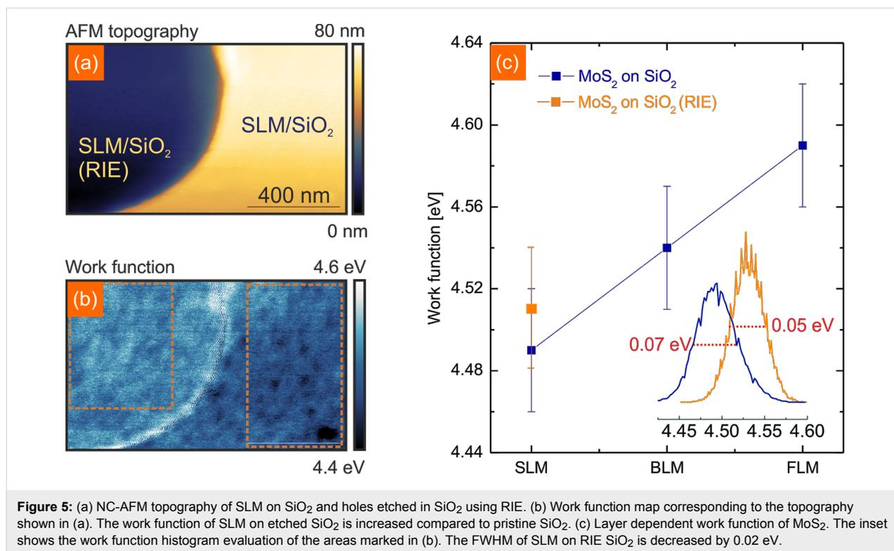
**Figure 5:** (a) NC-AFM topography of SLM on SiO<sub>2</sub> and holes etched in SiO<sub>2</sub> using RIE. (b) Work function map corresponding to the topography shown in (a). The work function of SLM on etched SiO<sub>2</sub> is increased compared to pristine SiO<sub>2</sub>. (c) Layer dependent work function of MoS<sub>2</sub>. The inset shows the work function histogram evaluation of the areas marked in (b). The FWHM of SLM on RIE SiO<sub>2</sub> is decreased by 0.02 eV.
