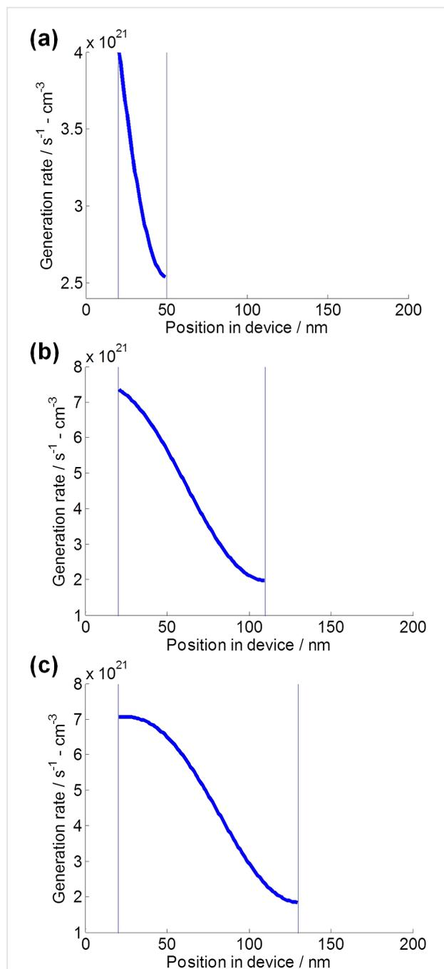
**Figure 7:** Calculated charge generation rate of the DSSCs with different TNT lengths using GTMM under 1 sun condition ( $100 \text{ mW}\cdot\text{cm}^{-2}$ ). Charge generation rate for DSSCs with (a)  $30 \text{ nm}$  thick electric field-valid layer of a  $3.3 \mu\text{m}$  long TNT array, (b)  $90 \text{ nm}$  thick electric field-valid layer of a  $11.5 \mu\text{m}$  long TNT array, and (c)  $110 \text{ nm}$  thick electric field-valid layer of a  $20.6 \mu\text{m}$  long TNT array.
