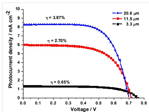
**Figure 2:** Photocurrent–voltage characteristics of N719-DSSCs fabricated by using 3.3  $\mu\text{m}$ , 11.5  $\mu\text{m}$ , and 20.6  $\mu\text{m}$  TNT arrays under an AM 1.5 solar simulator ( $100 \text{ mW}\cdot\text{cm}^{-2}$ ).
