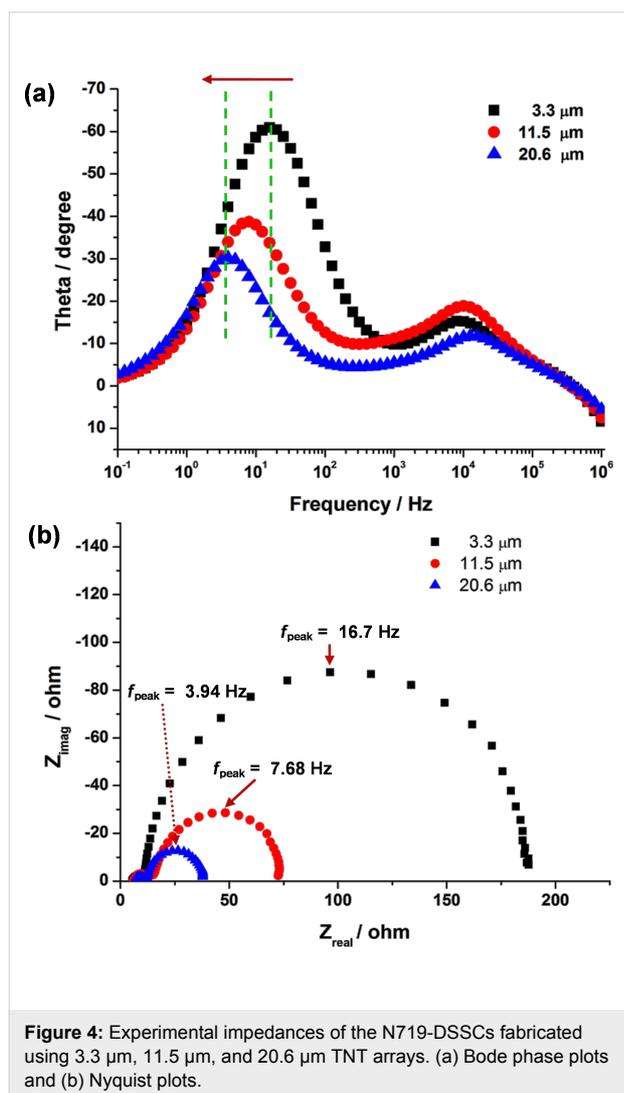
**Figure 4:** Experimental impedances of the N719-DSSCs fabricated using 3.3  $\mu\text{m}$ , 11.5  $\mu\text{m}$ , and 20.6  $\mu\text{m}$  TNT arrays. (a) Bode phase plots and (b) Nyquist plots.
