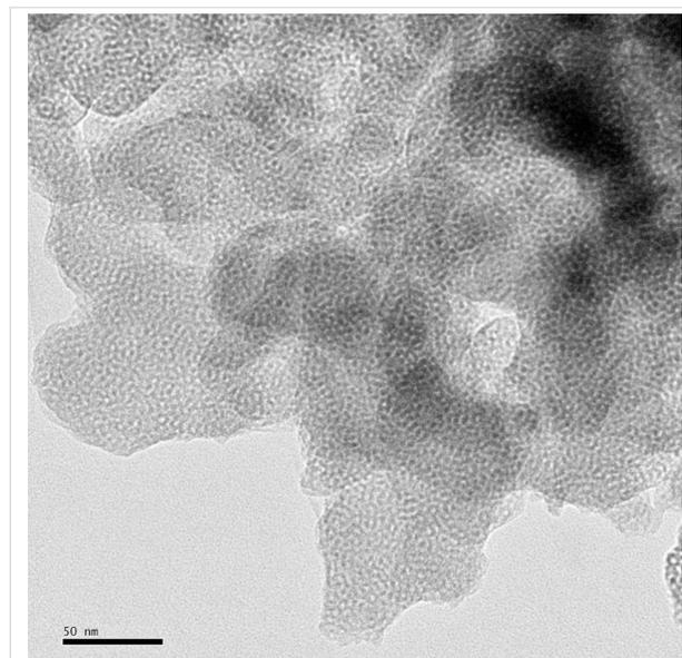
**Figure 3:** The HRTEM images of V-Ti/MCM-41 photocatalyst.
