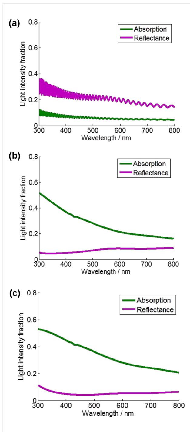
**Figure 6:** Calculated absorption and reflectance of the DSSCs with different TNT lengths by using GTMM: (a)  $3.3 \mu\text{m}$  long TNT array, (b)  $11.5 \mu\text{m}$  long TNT array, and (c)  $20.6 \mu\text{m}$  long TNT array.
