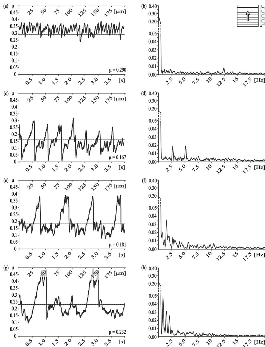
**Figure 2:** Results of frictional measurements on periodical groove-like polymer surface – PGMS perpendicular to the orientation of the microstructure. Left column, frictional signal in the spatial/time domain. Right column, frictional signal in the frequency domain after FFT; the ordinate shows the single-sided amplitude spectrum – SSAS. PGMS pitch dimension: a,b) 5  $\mu\text{m}$ , c,d) 25  $\mu\text{m}$ , e,f) 50  $\mu\text{m}$  and g,h) 100  $\mu\text{m}$ .
