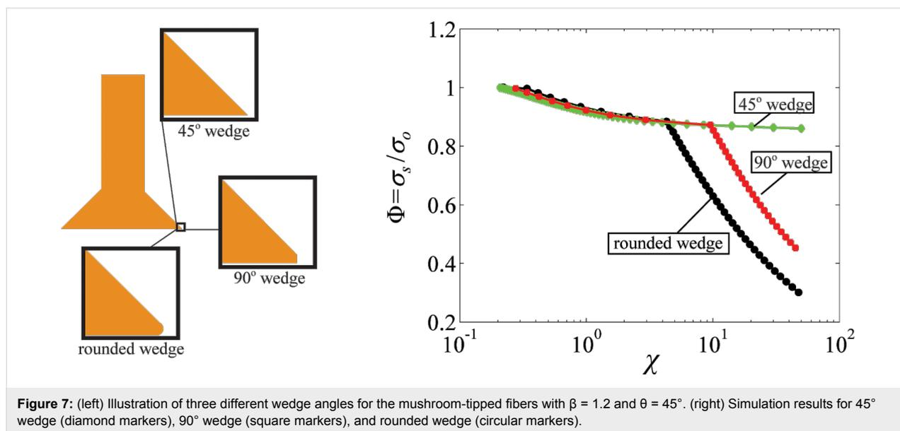
**Figure 7:** (left) Illustration of three different wedge angles for the mushroom-tipped fibers with  $\beta = 1.2$  and  $\theta = 45^\circ$ . (right) Simulation results for 45° wedge (diamond markers), 90° wedge (square markers), and rounded wedge (circular markers).
