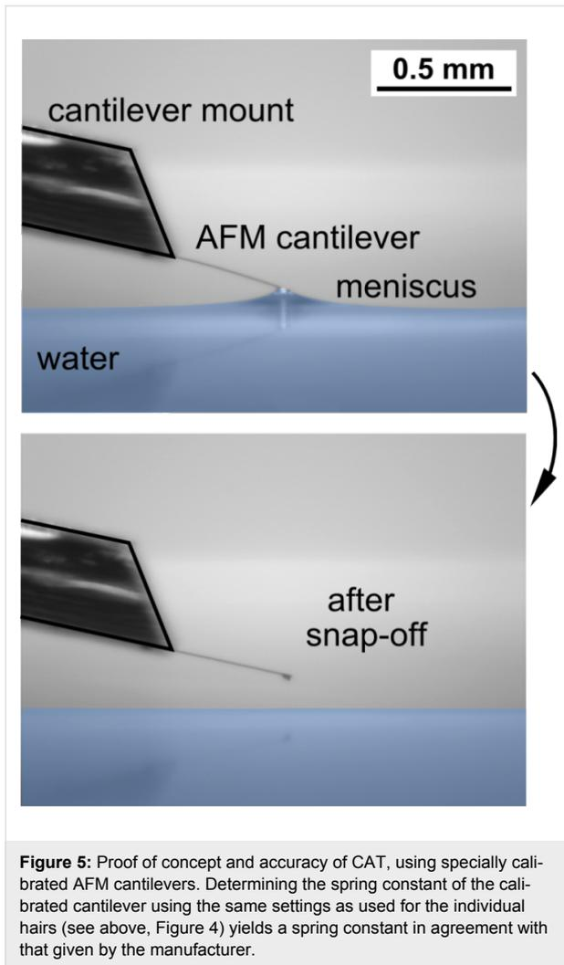
**Figure 5:** Proof of concept and accuracy of CAT, using specially calibrated AFM cantilevers. Determining the spring constant of the calibrated cantilever using the same settings as used for the individual hairs (see above, Figure 4) yields a spring constant in agreement with that given by the manufacturer.
