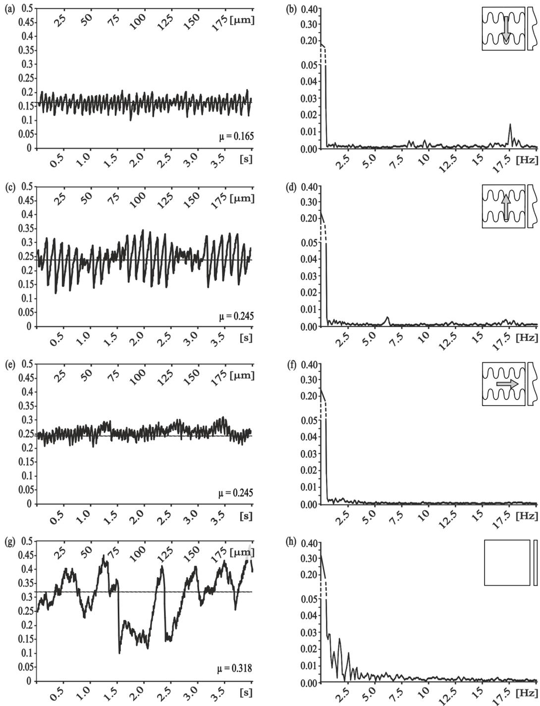
**Figure 6:** Frequency analysis of the frictional coefficient measured on snake-inspired microstructured polymer surface - SIMPS (a–f) and smooth surface (h,i). Left column, frictional signal in the spatial/time domain. Right column, frictional signal in the frequency domain after FFT; the ordinate shows the single-sided amplitude spectrum - SSAS. Measurement direction: a,b) along the microstructure, c,d) against the microstructure and e,f) lateral to the microstructure, g,h) on smooth surface.
