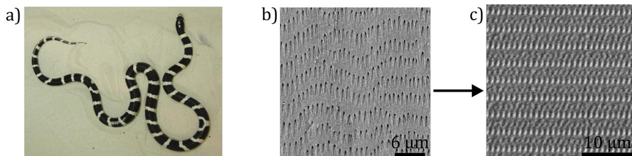
**Figure 1:** From the snake skin microstructure to the SIMPS. a) Photograph of the California King Snake (*Lampropeltis getula californicae*). SEM-micrographs of the snake skin of a ventral scale (b) and the SIMPS made of epoxy resin (c).
