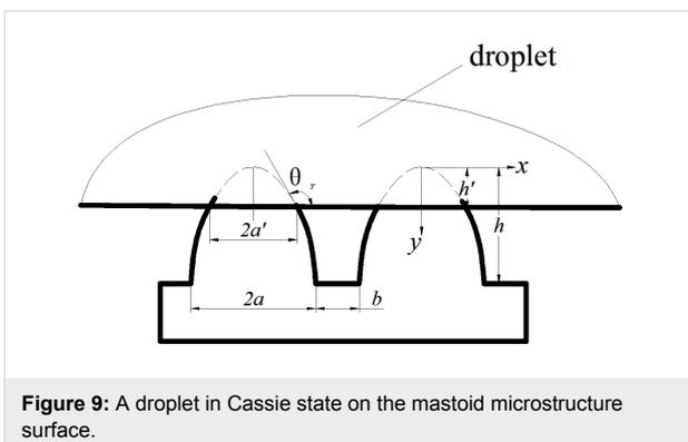
**Figure 9:** A droplet in Cassie state on the mastoid microstructure surface.
