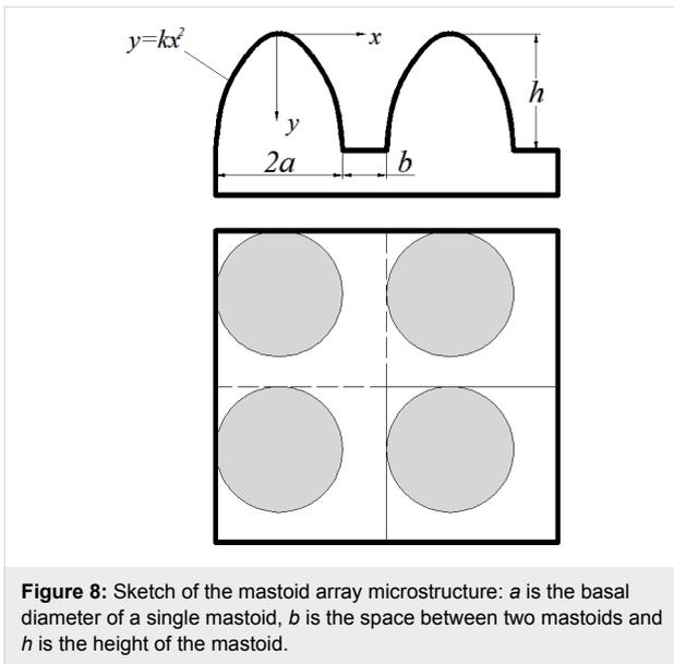
**Figure 8:** Sketch of the mastoid array microstructure:  $a$  is the basal diameter of a single mastoid,  $b$  is the space between two mastoids and  $h$  is the height of the mastoid.
