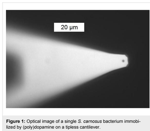
**Figure 1:** Optical image of a single *S. carnosus* bacterium immobilized by (poly)dopamine on a tipless cantilever.
