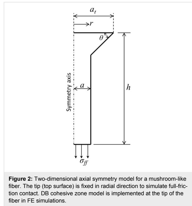
**Figure 2:** Two-dimensional axial symmetry model for a mushroom-like fiber. The tip (top surface) is fixed in radial direction to simulate full-friction contact. DB cohesive zone model is implemented at the tip of the fiber in FE simulations.
