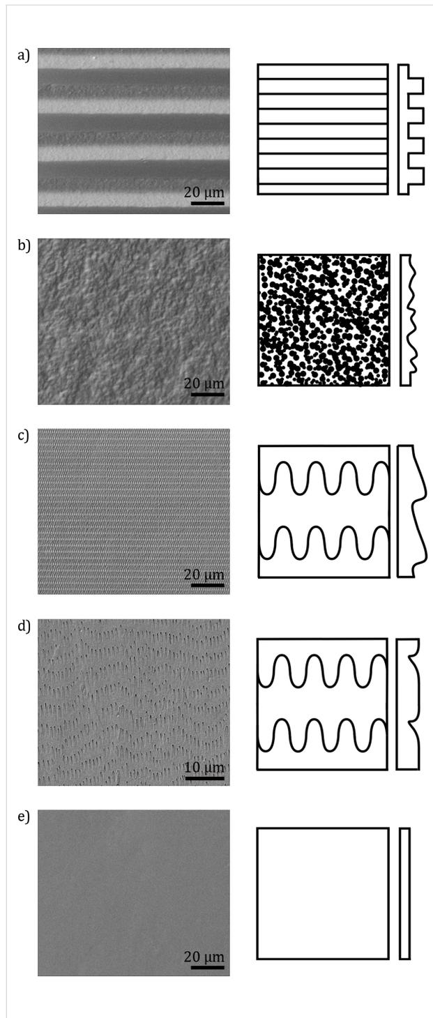
**Figure 7:** Exemplary overview of the topography of the examined polymer surfaces. Left column: SEM-micrographs. Right column: schematic top view and profile of the surface microstructure. a) Periodical groove-like polymer surface – PGMS (pitch: 25 µm). b) Randomly-rough surfaces – RRS (grain size: 1 µm). c) Snake-inspired microstructured polymer surface – SIMPS. d) Mold of the ventral scale of *L. g. californiae* - PMLG. e) Smooth surface.
