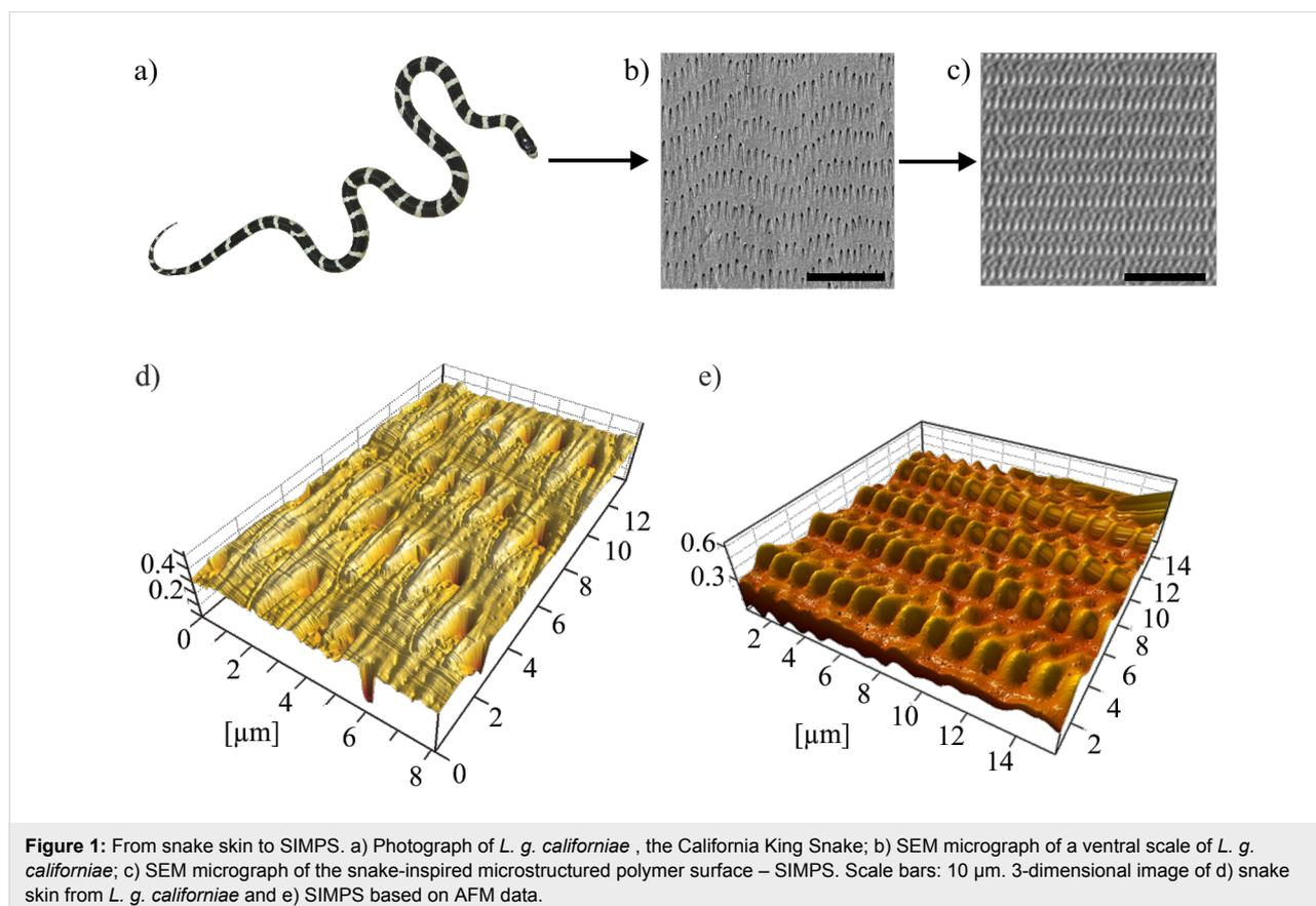
**Figure 1:** From snake skin to SIMPS. a) Photograph of *L. g. californiae*, the California King Snake; b) SEM micrograph of a ventral scale of *L. g. californiae*; c) SEM micrograph of the snake-inspired microstructured polymer surface – SIMPS. Scale bars: 10  $\mu\text{m}$ . 3-dimensional image of d) snake skin from *L. g. californiae* and e) SIMPS based on AFM data.
