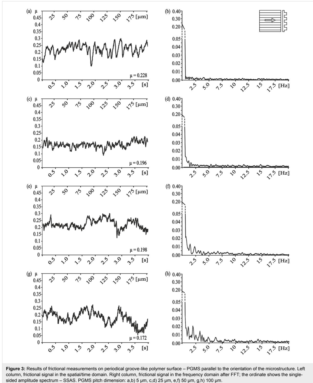
frequency was found (Figure 3b,d). A correlation to the pitch dimension was found for the PGMS with a structural wavelength of 50  $\mu\text{m}$ , nevertheless the amplitude of the frequency spectrum was quite low (Figure 3f). Similar low amplitudes were found for the PGMS 100  $\mu\text{m}$ , but the observed frequencies do not directly correlate with the microstructure dimension (Figure 3h).
