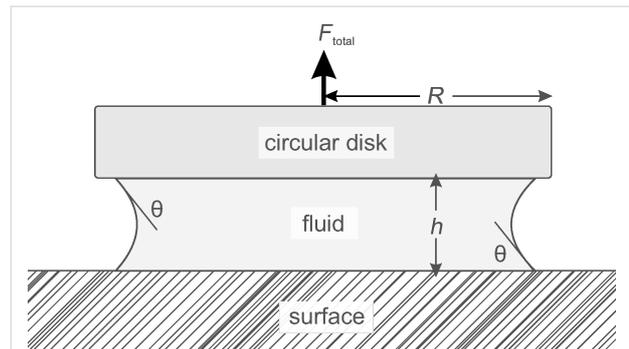
**Figure 2:** Schematic illustration of a simple fluid-mediated attachment model. The contact of a circular rigid disk (radius  $R$ ) and a plane rigid surface is mediated by a thin fluid layer (height  $h$ ). The contact angle of the fluid to the surface and the disk  $\theta$  is assumed to be identical in this case.
