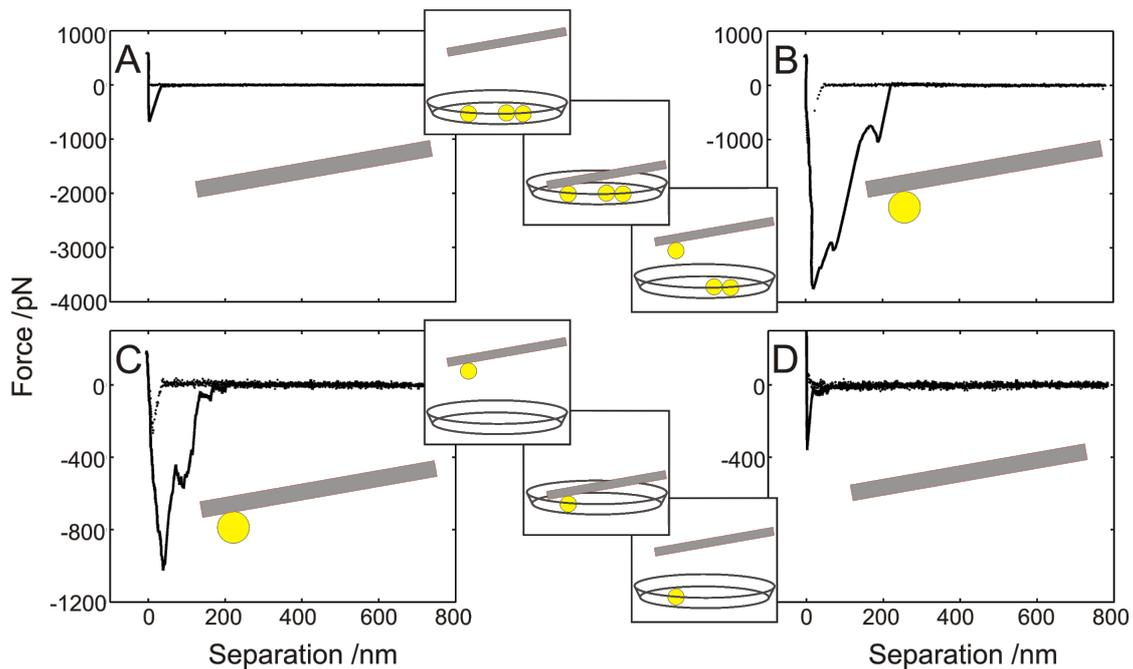
**Figure 3:** Test of artifacts of AFM force/distance curve with and without bacterium, each taken under the same conditions: (A) Bare (poly)dopamin-coated cantilever force/distance curve. (B) The same cantilever as in (A), yet after attachment of a bacterium. (C) A second cantilever with bacterium and its characteristic force/distance curve. (D) Force/distance curve after detaching the bacterium of the experiment shown in (C).
