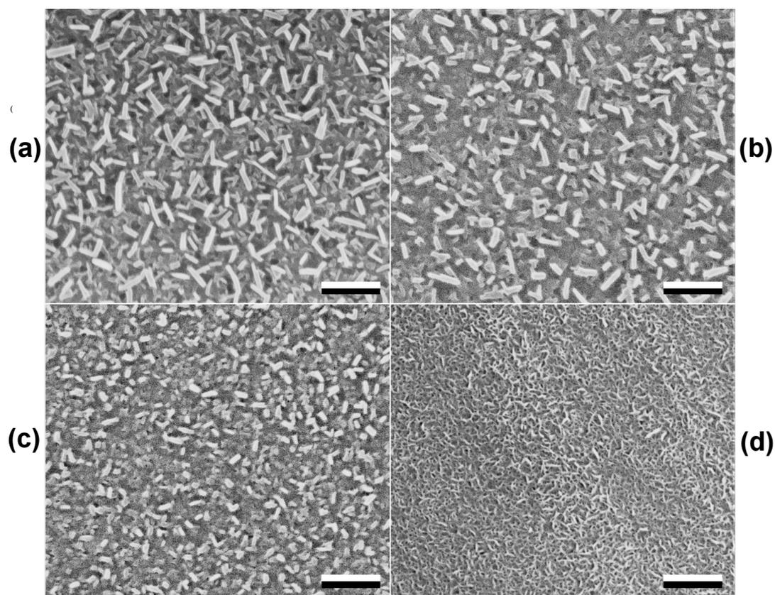
**Figure 1:** Scanning electron microscopy (SEM) micrographs of wax surfaces formed by alkanes of varying chain lengths:  $C_{36}H_{74}$  (a),  $C_{40}H_{82}$  (b),  $C_{44}H_{90}$  (c), and  $C_{50}H_{102}$  (d). Scale bars = 2  $\mu\text{m}$ .
