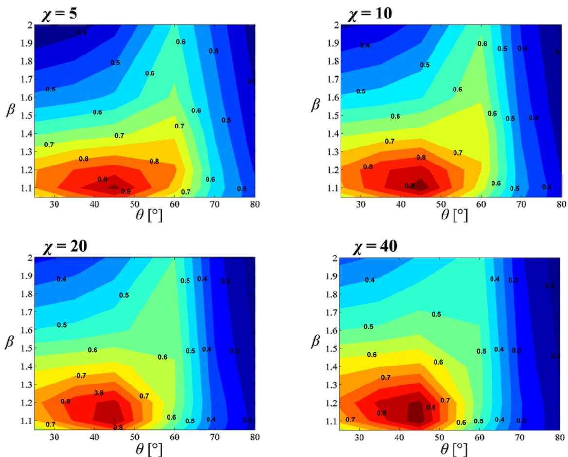
**Figure 4:** Normalized pull-off stress  $\Phi$  contour plots for  $\chi = 5$  (top left),  $\chi = 10$  (top right),  $\chi = 20$  (bottom left), and  $\chi = 40$  (bottom right) as a function of  $\beta$  and  $\theta$ . The peak  $\Phi$  for each case lies within  $\beta = 1.1\text{--}1.2$  and  $\theta = 45^\circ$ .
