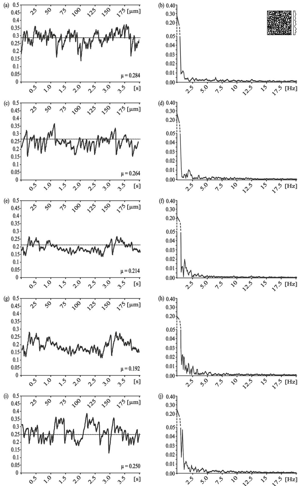
**Figure 4:** Results of frictional measurements on randomly-rough surfaces – RRS. Left column, frictional signal in the spatial/time domain. Right column, frictional signal in the frequency domain after FFT; the ordinate shows the single-sided amplitude spectrum - SSAS. Grain size of RRS: a,b) 0.3  $\mu\text{m}$ , c,d) 1  $\mu\text{m}$ , e,f) 3  $\mu\text{m}$ , g,h) 9  $\mu\text{m}$ , i,j) 12  $\mu\text{m}$ .
