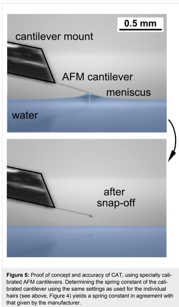
of the capillary adhesion technique (CAT) was given by the measurement of the elastic force constant of 0.195 N/m for a calibrated atomic force microscopy cantilever.
