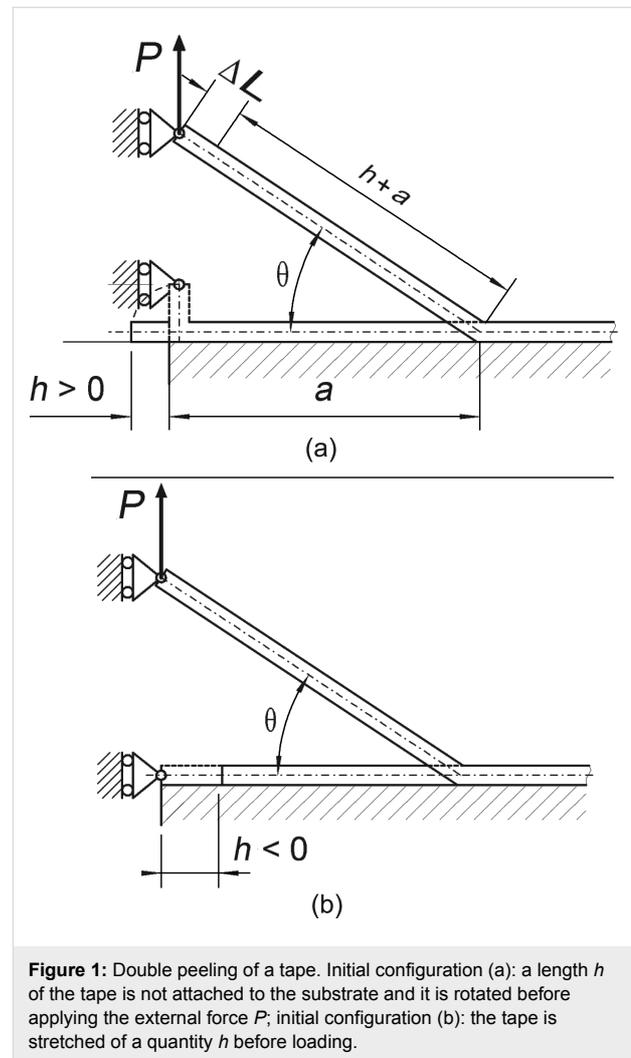
**Figure 1:** Double peeling of a tape. Initial configuration (a): a length  $h$  of the tape is not attached to the substrate and it is rotated before applying the external force  $P$ ; initial configuration (b): the tape is stretched of a quantity  $h$  before loading.
