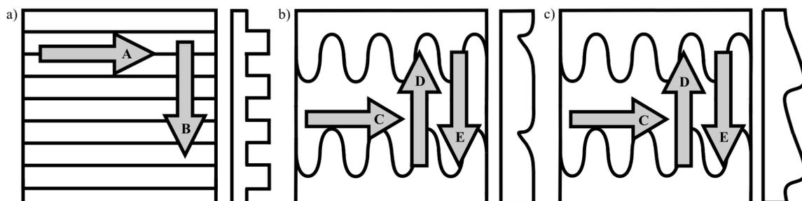
**Figure 8:** Scheme of surface geometry and sliding directions of friction measurement, top view (left) and side view (right). a) Periodical groove-like polymer surface - PGMS, b) Polymeric mould of *L. g. californiae* – PMLG, c) Snake-inspired microstructured polymer surface – SIMPS. Directions of measurement: A: parallel to microstructure, B: perpendicular to microstructure, C: lateral to microstructure, D: against microstructure, E: along microstructure.
