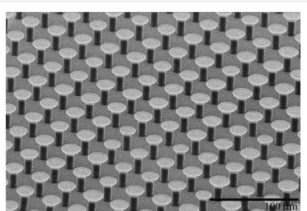
**Figure 1:** Scanning electron microscope image of polyurethane mushroom-like fibers with 4  $\mu\text{m}$  stalk radius, 8  $\mu\text{m}$  tip radius, and 20  $\mu\text{m}$  height.
