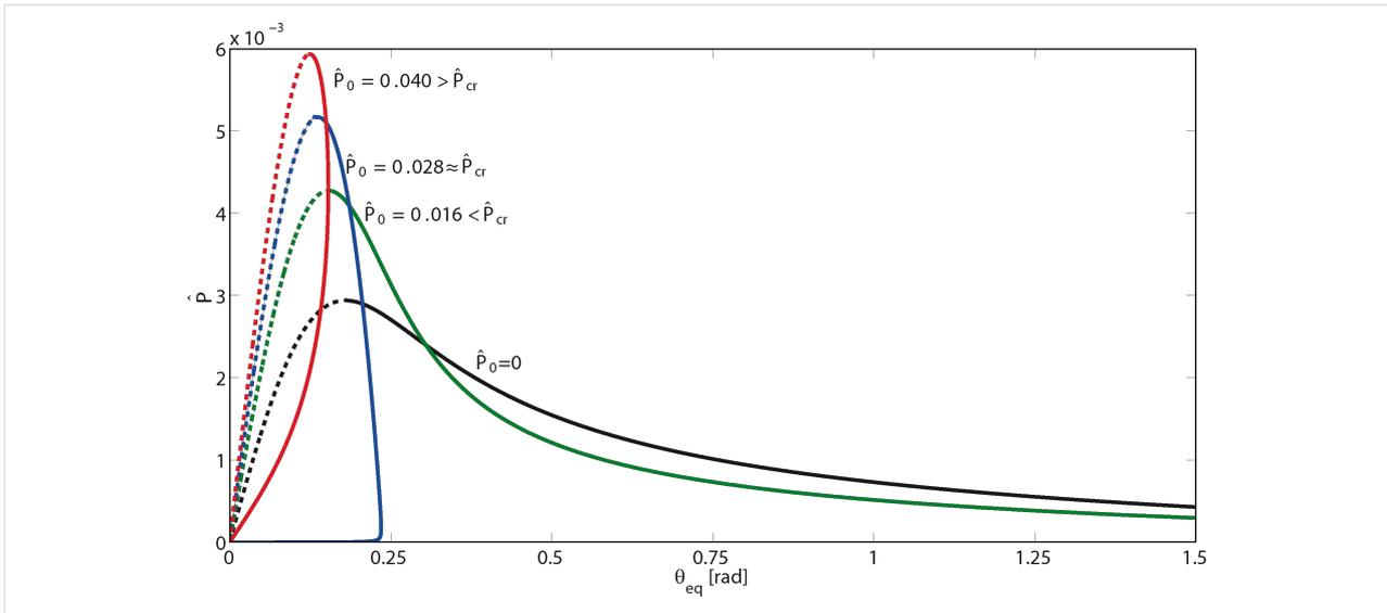
**Figure 3:** The dimensionless peeling force  $\hat{P}$  as a function of the peeling angle  $\theta_{eq}$  at equilibrium, for different values of the dimensionless pre-tension  $\hat{P}_0$ . The pre-tension generally increases the pull-off force at low peeling angles.
