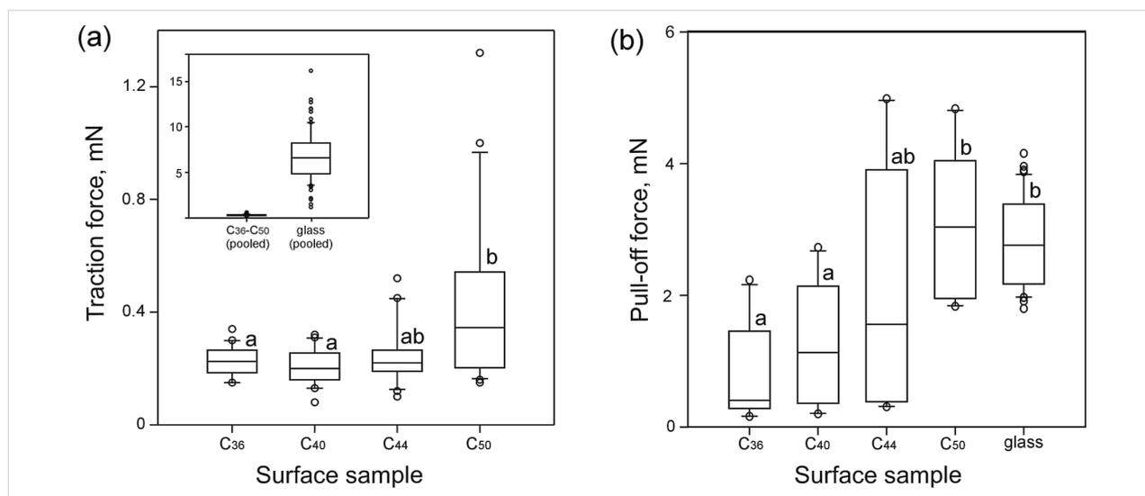
**Figure 3:** Traction forces of male beetles *Coccinella septempunctata* (a) and pull-off forces of PDMS semi-spheres (b) on different surfaces. According to the *t*-test and Mann–Whitney rank sum test (Table 3 and Table 4), means/medians with different letters differ significantly from each other.
