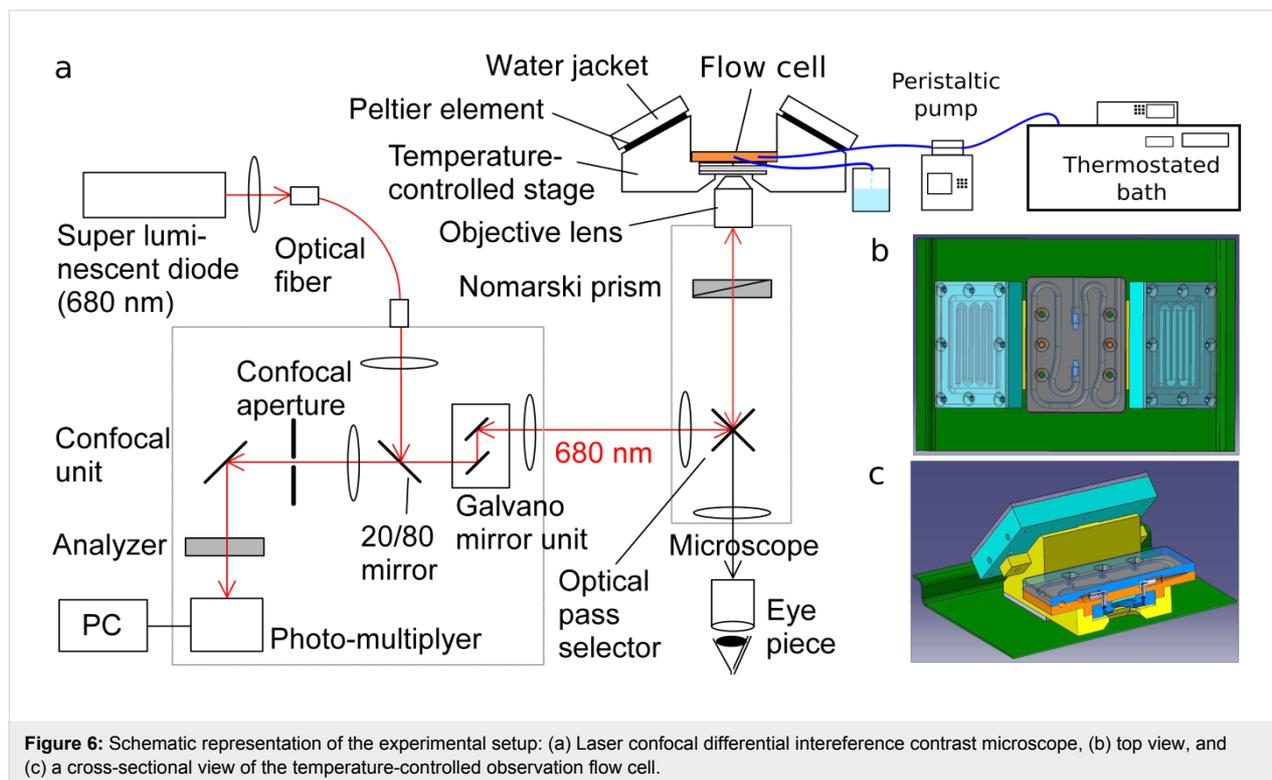
**Figure 6:** Schematic representation of the experimental setup: (a) Laser confocal differential interference contrast microscope, (b) top view, and (c) a cross-sectional view of the temperature-controlled observation flow cell.
