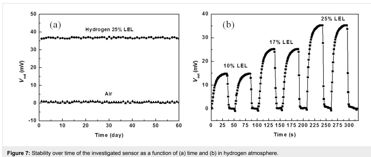
**Figure 7:** Stability over time of the investigated sensor as a function of (a) time and (b) in hydrogen atmosphere.
