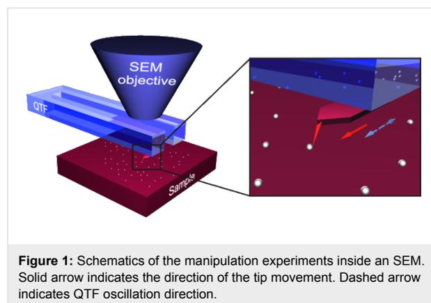
**Figure 1:** Schematics of the manipulation experiments inside an SEM. Solid arrow indicates the direction of the tip movement. Dashed arrow indicates QTF oscillation direction.
