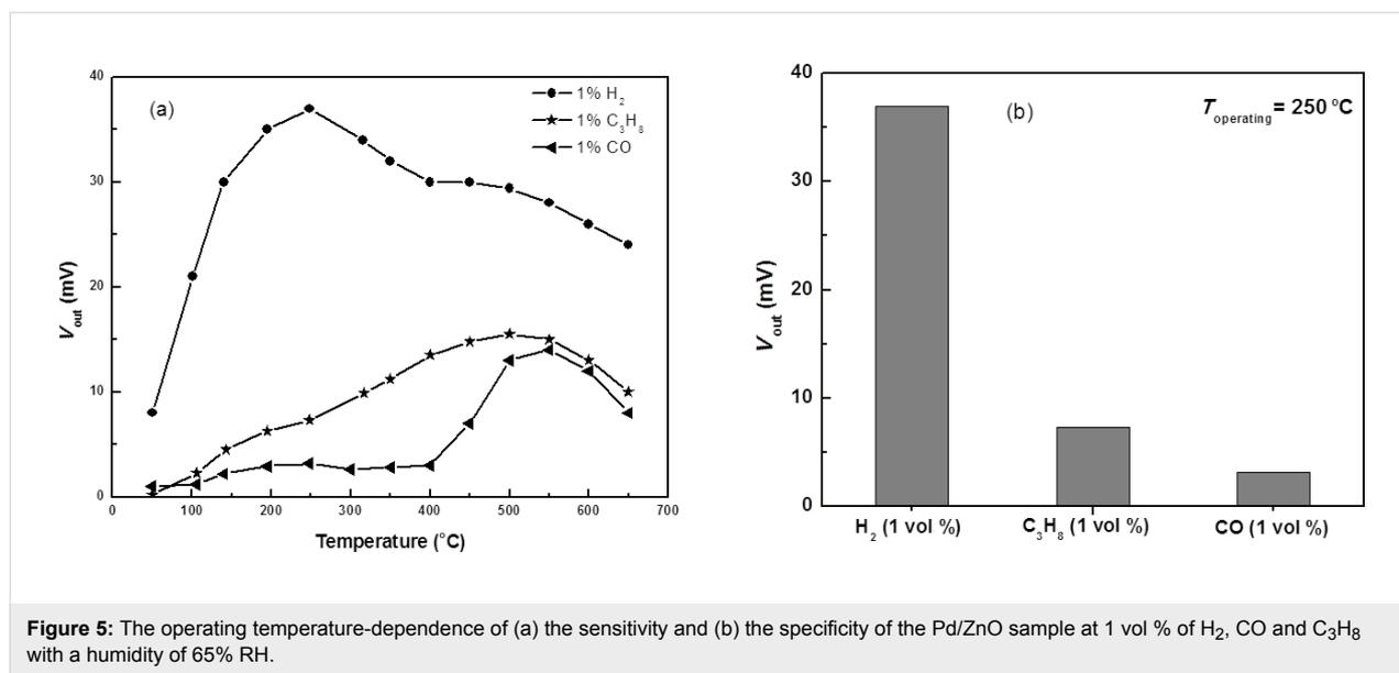
**Figure 5:** The operating temperature-dependence of (a) the sensitivity and (b) the specificity of the Pd/ZnO sample at 1 vol % of  $H_2$ , CO and  $C_3H_8$  with a humidity of 65% RH.
