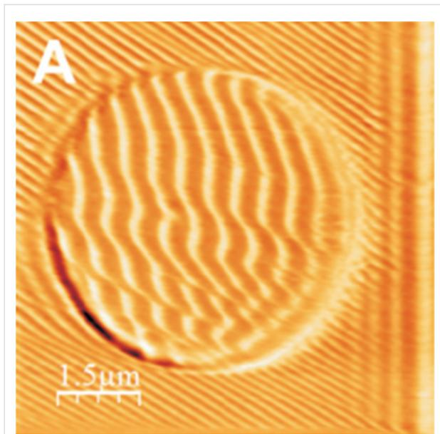
**Figure 11:** A topographical image of nanoripple patterns on a circular area. The color scale covers a range of 30 nm. The parallel lines on the right hand side are due to an instrumental artefact. Reproduced with permission from [24]. Copyright 2012 IOP Publishing.
