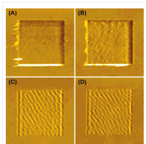
**Figure 3:** Topographical images ( $1.5 \times 1.5 \mu\text{m}^2$ ) of surfaces scratched in the multiple line mode. The PS films analyzed have different  $M_w$  values: (A) 8 kDa, (B) 15.8 kDa, (C) 58 kDa, and (D) 164 kDa. The applied load is constant and equal to 10 nN. Adapted with permission from [31]. Copyright 2001 American Chemical Society.
