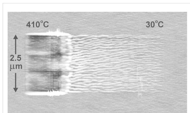
**Figure 5:** The worn area is the result of scanning a given surface with a variably heated tip, increasing  $T$  from 30 (right) to 410 °C (left). The PS film has a  $M_w$  of 70 kDa. The scan velocity is 50  $\mu\text{m/s}$ . The gray scale covers 17 nm. Reprinted with permission from [20]. Copyright 2003 American Chemical Society.
