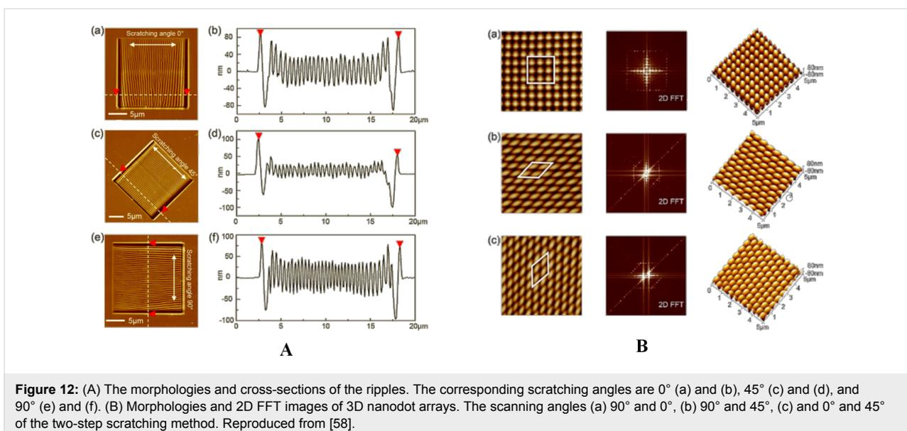
**Figure 12:** (A) The morphologies and cross-sections of the ripples. The corresponding scratching angles are 0° (a) and (b), 45° (c) and (d), and 90° (e) and (f). (B) Morphologies and 2D FFT images of 3D nanodot arrays. The scanning angles (a) 90° and 0°, (b) 90° and 45°, (c) and 0° and 45° of the two-step scratching method. Reproduced from [58].
