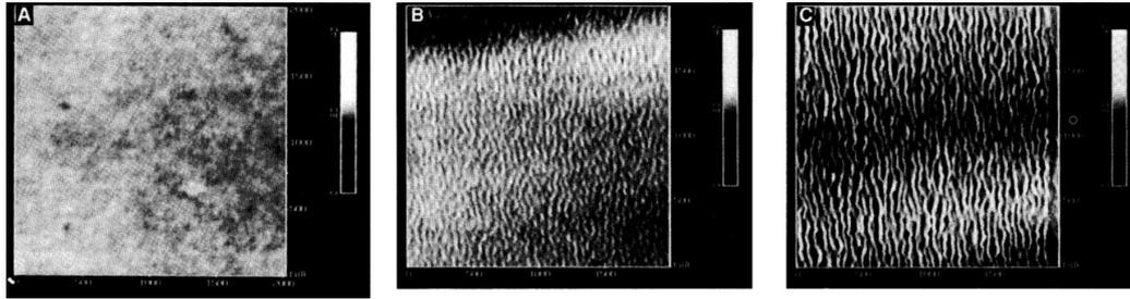
**Figure 1:** First experimental observations of the nanoripple formation on polymer films ( $2 \times 2 \mu\text{m}^2$ ): from a pristine surface of PS (A), through the initial stages of deformation (B), to a fully developed pattern (C). The gray scale covers a height difference of 10 nm. Reprinted with permission from [14]. Copyright 1992 AAAS.
