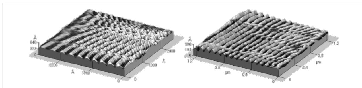
**Figure 4:** Solvent-enriched polymer films. Examples of 3D ripple structures on PCL (left) and PET (right). The images were obtained in air (relative humidity 40%), with a silicon conical shape tip with a nominal radius of 10 nm, a cantilever stiffness of 0.24 N/m, an applied load in the range between 2 and 10 nN, and scan velocity of 0.25  $\mu\text{m/s}$  on 80 nm thick films. Reproduced with permission from [23]. Copyright 2007 Elsevier.
