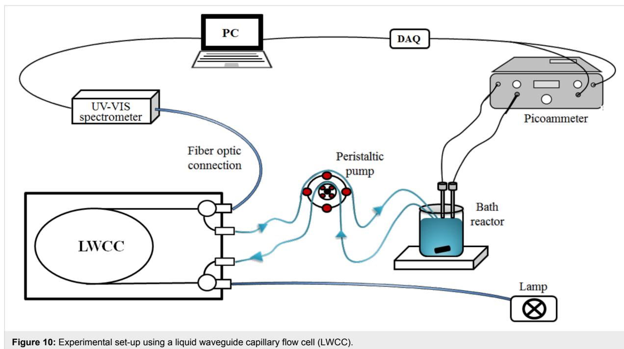
**Figure 10:** Experimental set-up using a liquid waveguide capillary flow cell (LWCC).
