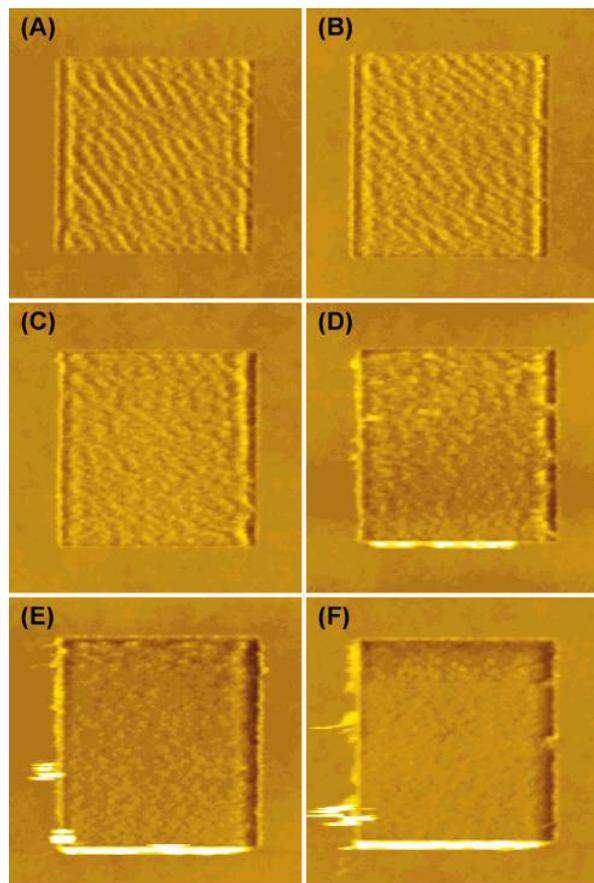
**Figure 6:** Topographical images ( $1.5 \times 1.5 \mu\text{m}^2$ ) of patterns induced on films obtained from blending two PS solutions with  $M_w$  of 8 and 164 kDa. The ratio of the two solutions is (8 kDa/164 kDa): (A) 0/100, (B) 10/90, (C) 30/70, (D) 50/50, (E) 70/30, (F) 90/10, and (G) 100/0. The applied load is constant and equal to 10 nN. Reproduced with permission from [31]. Copyright 2001 American Chemical Society.
