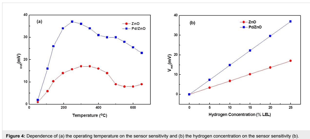
**Figure 4:** Dependence of (a) the operating temperature on the sensor sensitivity and (b) the hydrogen concentration on the sensor sensitivity (b).
