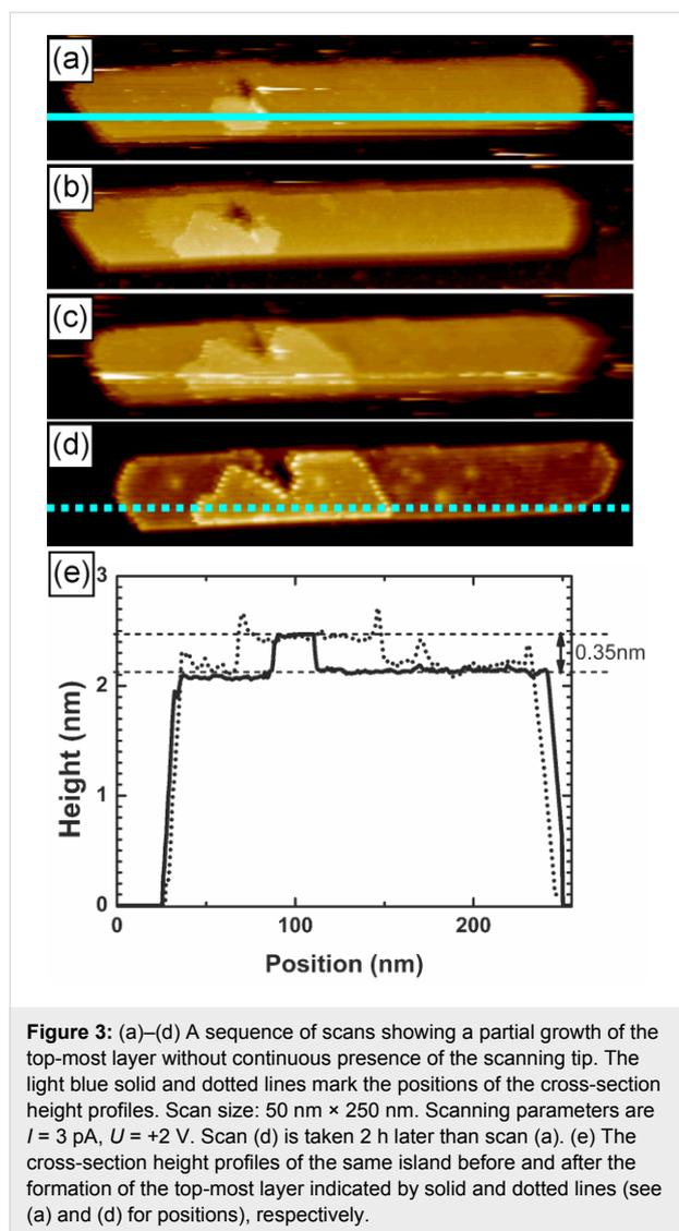
average speed of growth of the observed structure in this case is approximately  $13 \text{ nm}^2/\text{min}$ .
