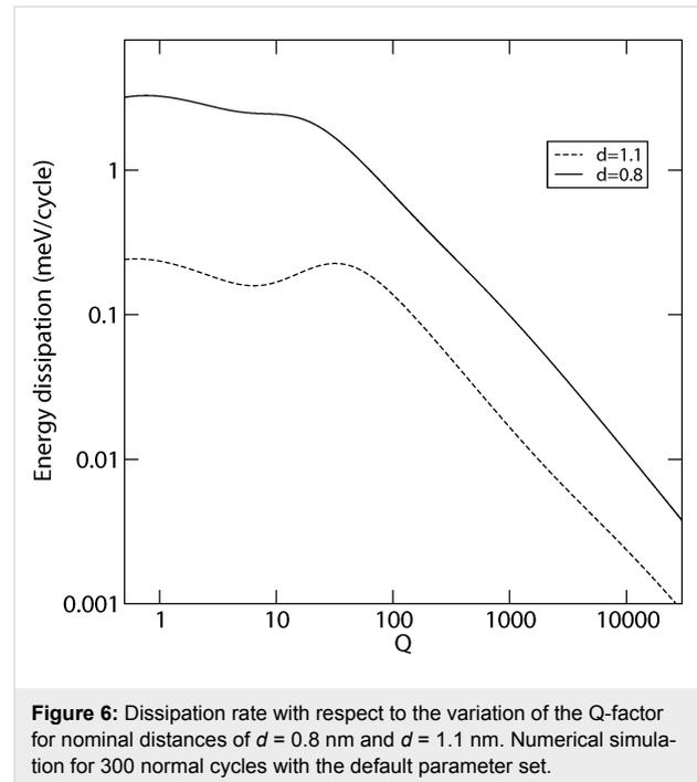
**Figure 6:** Dissipation rate with respect to the variation of the  $Q$ -factor for nominal distances of  $d = 0.8$  nm and  $d = 1.1$  nm. Numerical simulation for 300 normal cycles with the default parameter set.
