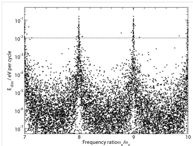
**Figure 5:** Dissipation rate depending on frequency ratio  $\omega_x/\omega_z$  for different systems. Dashed line indicates the lower bound of experimentally observed values. Dissipation rate is averaged over 300 cycles.
