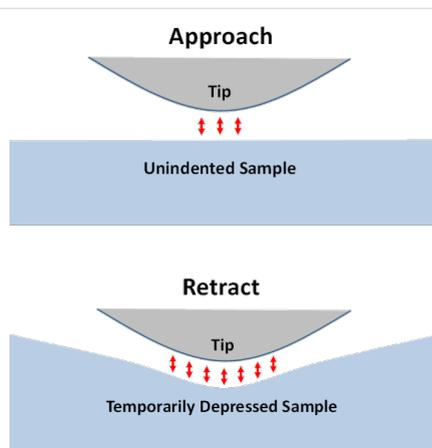
**Figure 3:** Illustration of tip–sample physical adhesion. In this case the interaction area between tip and sample is greater during the retract than during the approach, due to a change in the non-bonded attractive forces, leading to additional dissipation as the cantilever breaks free from the surface.
