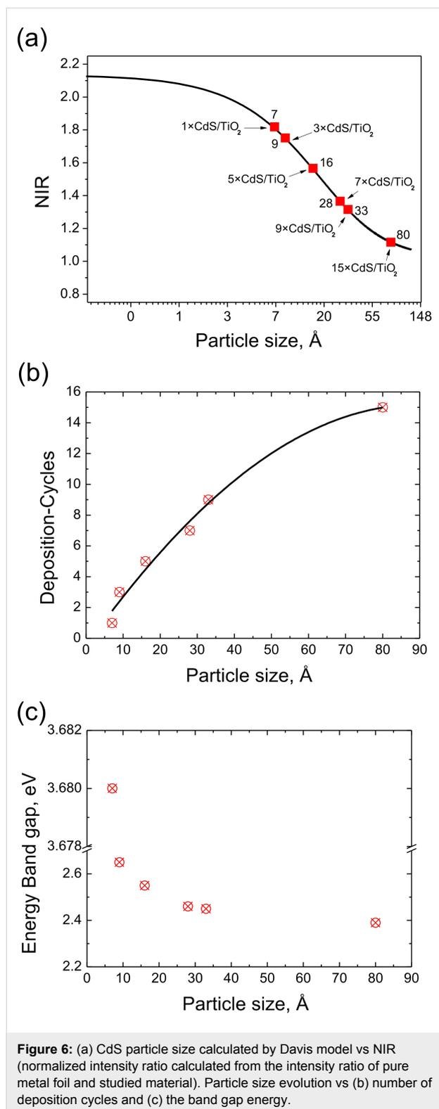
size on the number of successive deposition cycles. Moreover, a very good correlation was observed between results obtained from XPS, AFM and UV-vis. It confirms that XPS is a powerful method for the estimation of the average particle size
