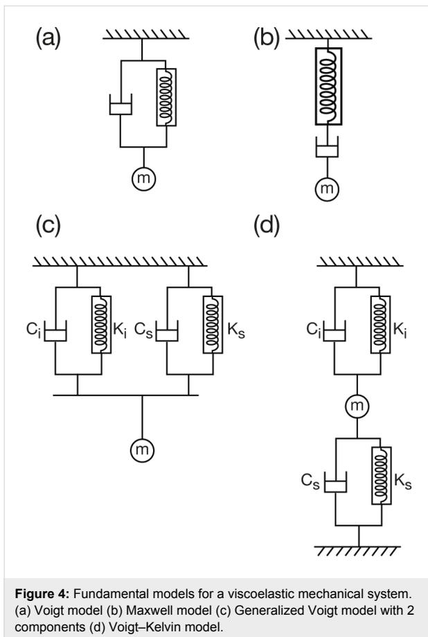
Combinations of the different models are also used. A comparison of three different models (Maxwell, Voigt–Kelvin, and combined Maxwell and Voigt–Kelvin) revealed that the latter gave the best fit to experimental data and also displayed a predictive power for experimentally-obtained indentation curves [65].
