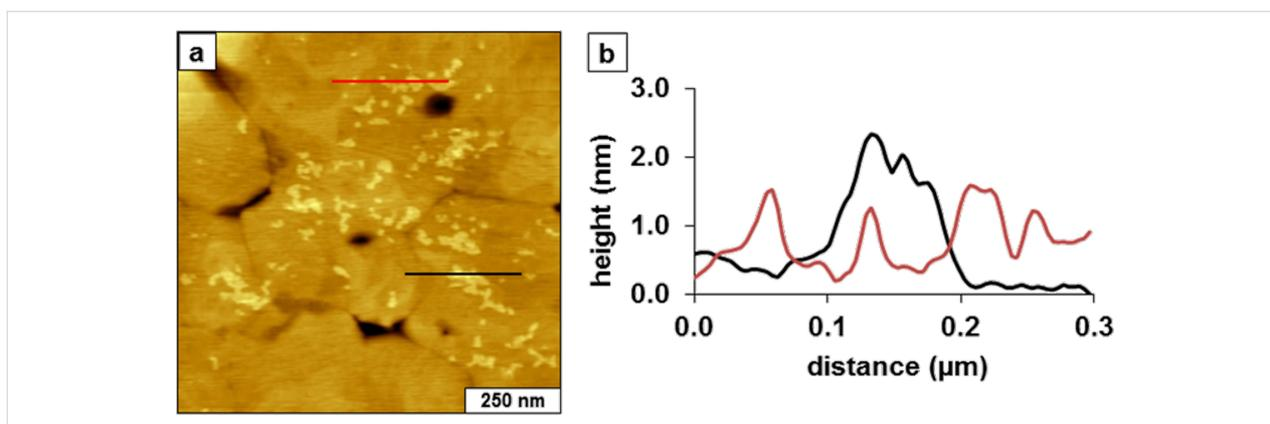
**Figure 2:** Representative cursor profiles of the side-on and standing phases of TMMH measured after 2 h of immersion.
