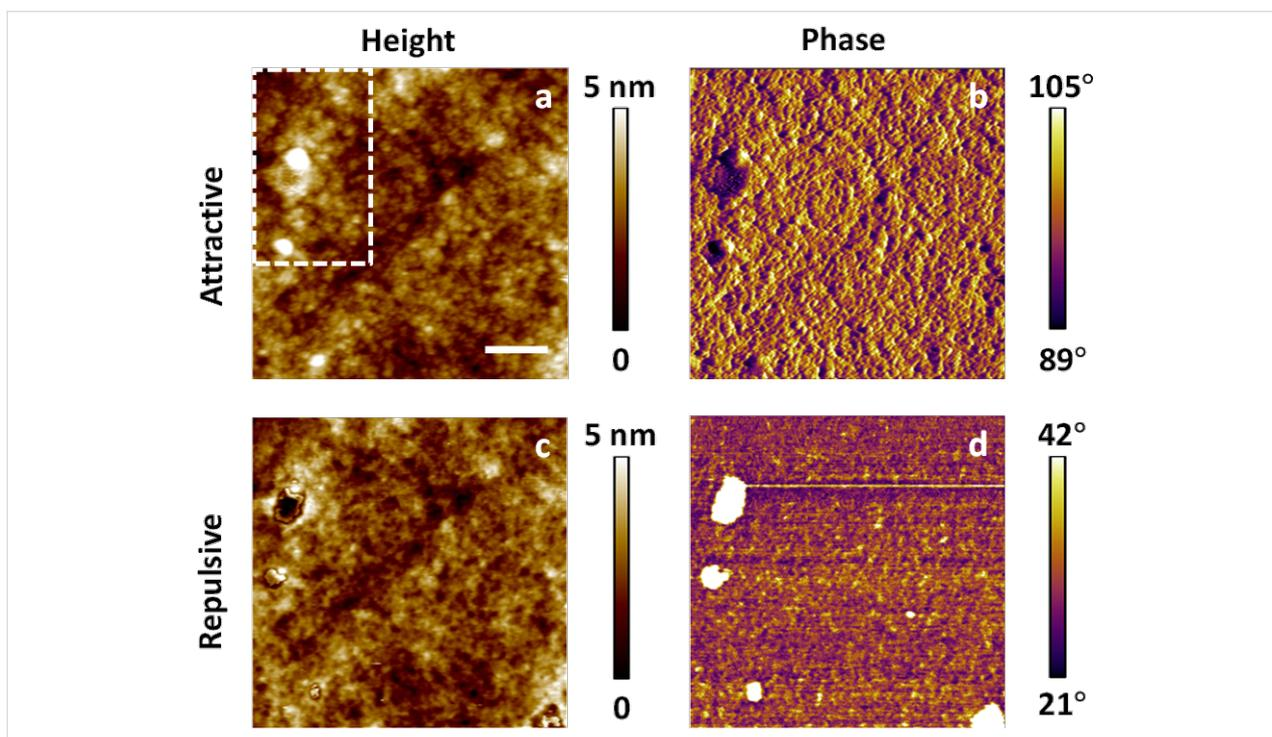
**Figure 1:** (a) and (b) topography and phase images, respectively, of a Nafion<sup>®</sup> membrane acquired in the attractive regime; (c) and (d) corresponding images acquired in the repulsive regime. The scale bar is 100 nm. The morphology of the region in the dashed rectangle in (a) is discussed below in Figure 6. The free oscillation amplitude in both cases was 17 nm, with an amplitude setpoint of 80% for attractive regime imaging and 50% for repulsive regime imaging.
