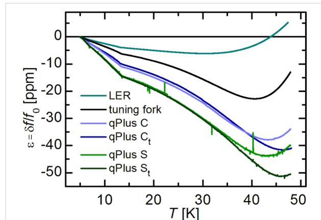
**Figure 2:** (Color online). Relative frequency change of quartz based AFM sensors from 4.8–48 K. The coupled oscillators show less relative frequency change with temperature as the qPlus sensors. For custom made qPlus sensors  $\varepsilon$  is smaller as for the standard ones. The spikes in the curves of the qPlus sensors arise from mechanical excitations of the sensors due to external vibrations or sound.
