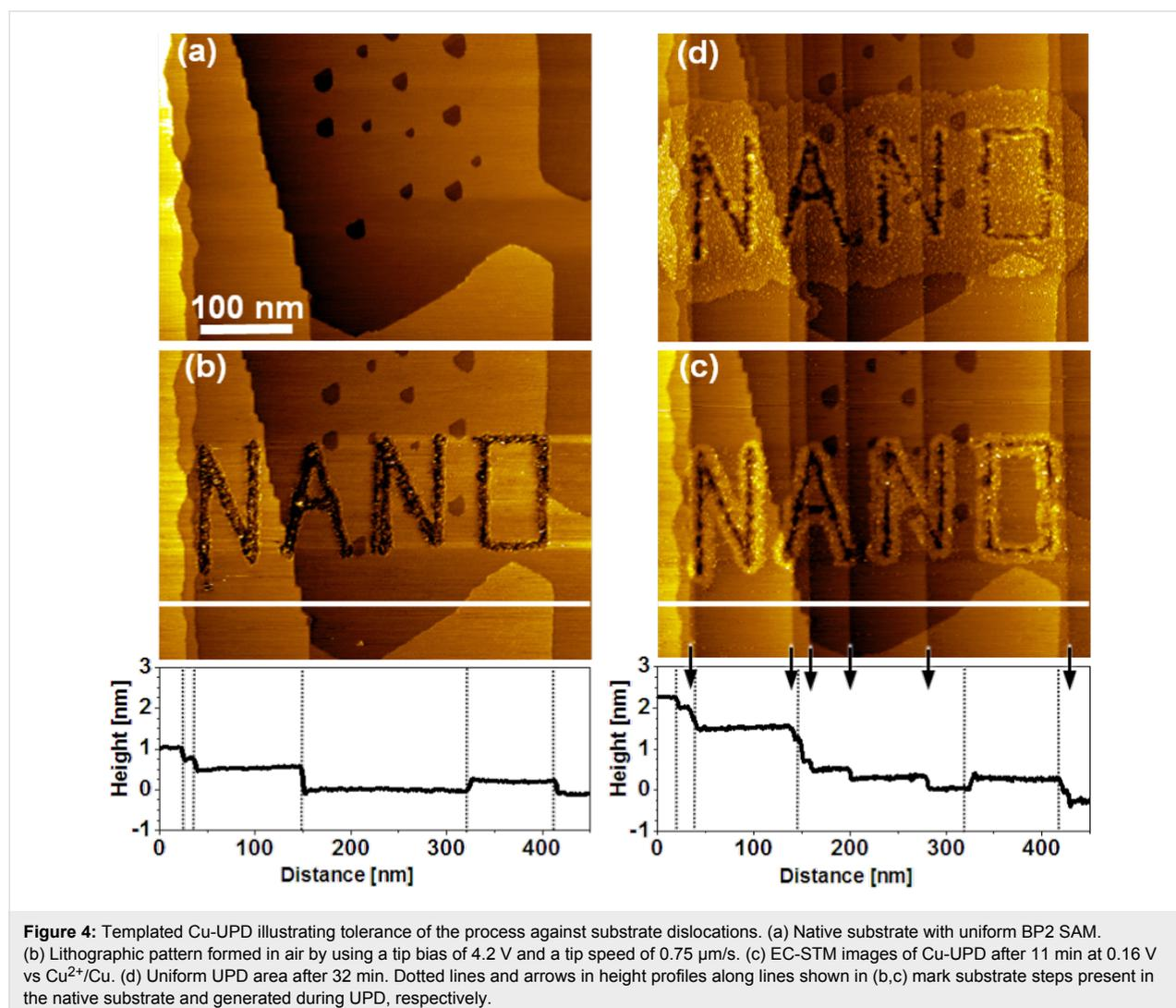
tial diffusion of UPD metal along those steps. Thus, possible structural differences between a BP2 SAM that covers a native step in the initial preparation procedure and one being generated during the UPD process are too small to alter the UPD mechanism. This is essential for the exploitation of this process on the nanoscale as the UPD pattern and, thus, its spatial resolution is not impeded by processes that cannot be eliminated.
