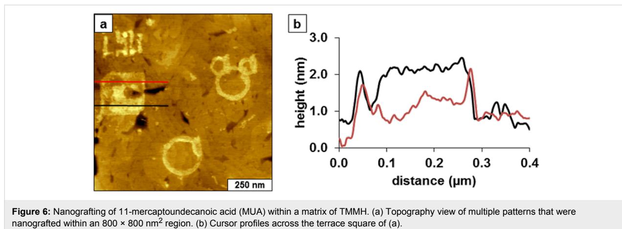
with a double layer (Figure 6b, black line) are  $2 \pm 0.2 \text{ nm}$  taller than the TMMH matrix. Since a double layer of MUA would be  $3.0 \text{ nm}$  thick, this analysis likewise indicates a height of  $\sim 1 \text{ nm}$  for the SAM derived from TMMH.
