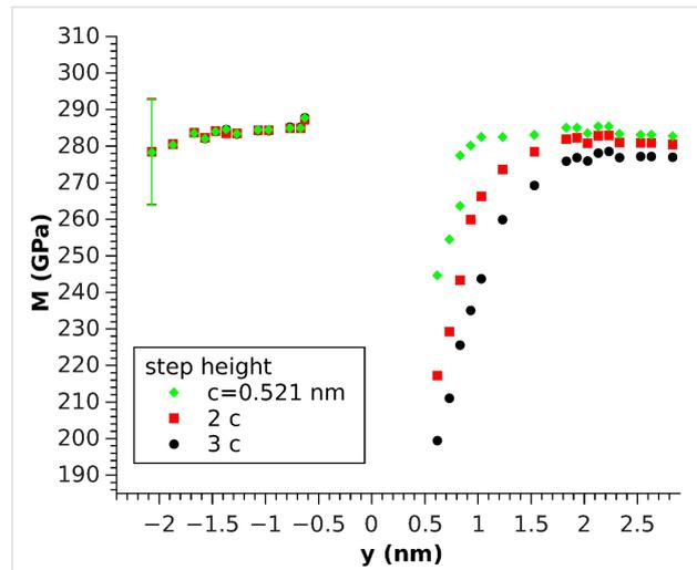
**Figure 4:** [001]-oriented indentation modulus for three different step heights along  $y$ . Measured by indenting a circular region of surface atoms ( $A_2 = 1.232 \text{ nm}^2$ ). The error bars denote the standard deviation of the displacement and apply to all data points.
