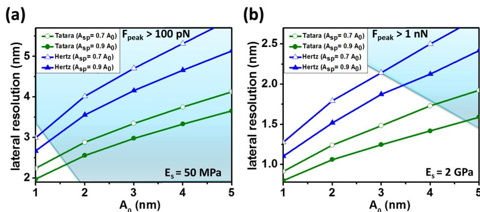
**Figure 5:** Lateral resolution maps for Hertz and Tataro contact mechanics. (a)  $E_s = 50$  MPa. (b)  $E_s = 2$  GPa. Filled symbols for  $A_{\text{sp}} = 0.9 A_0$ ; empty symbols for  $A_{\text{sp}} = 0.7 A_0$ . Circles for Tataro and triangles for Hertz. Simulation inputs:  $k = 0.1$  N/m,  $f_0 = 25$  kHz,  $Q = 2$ ,  $A_{\text{sp}} = 0.65 A_0$ ,  $R_t = 5$  nm,  $R_s = 4$  nm, and two different  $A_{\text{sp}}$  of 0.9 and  $0.7 A_0$ , respectively.
