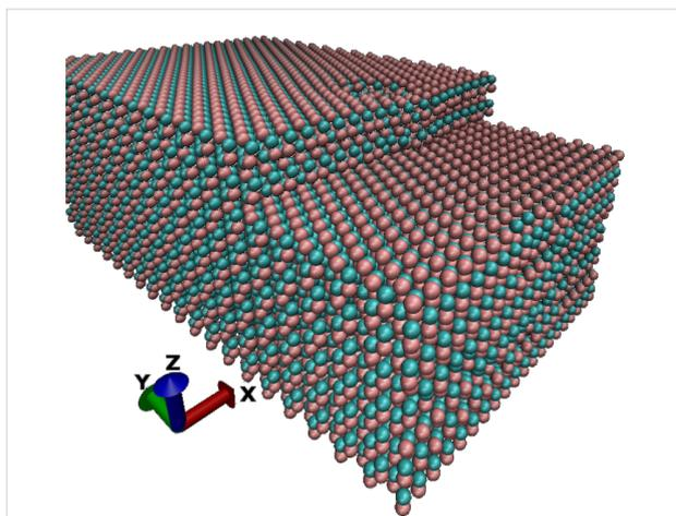
**Figure 1:** MD configuration of a GaN step with a step height of  $h = 2c$  during indentation of surface atoms within a circular area of  $A_2 = 1.232$  nm<sup>2</sup>. The red spheres denote the gallium and blue spheres the nitrogen atoms.
