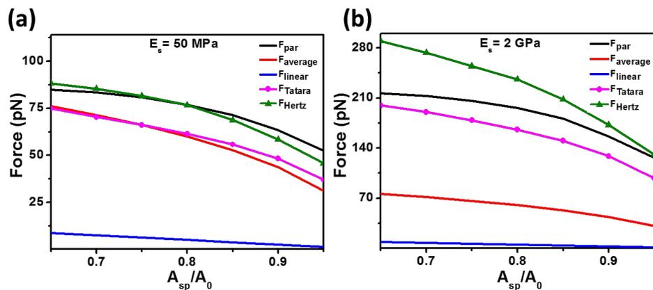
**Figure 3:** Dependence of the peak force on the set-point amplitude for different numerical simulations (Hertz and Tatara) and force analytical approximations (parametrized, average and linear). (a)  $A_0 = 1$  nm and  $E_s = 50$  MPa. (b)  $A_0 = 1$  nm and  $E_s = 2$  GPa. Simulation inputs are:  $k = 0.1$  N/m,  $f_0 = 25$  kHz,  $Q = 2$ ,  $R_t = 5$  nm, and  $R_s = 4$  nm.
