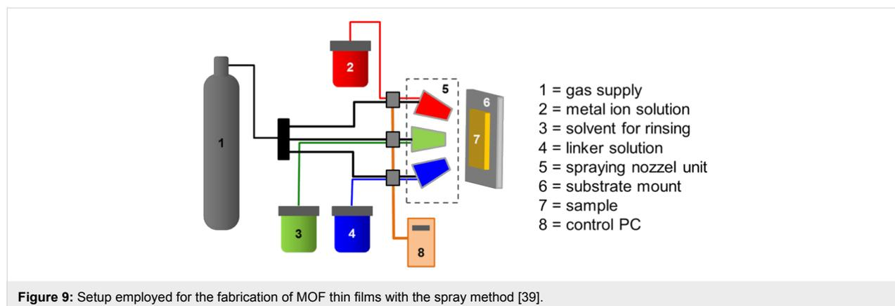
**Figure 9:** Setup employed for the fabrication of MOF thin films with the spray method [39].
