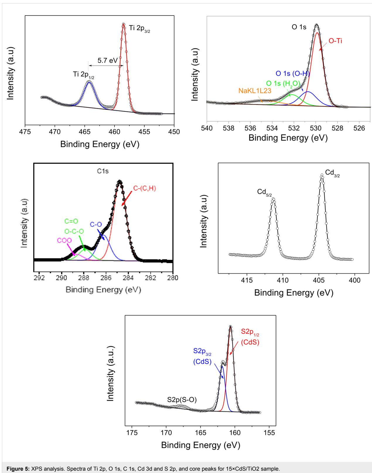
**Figure 5:** XPS analysis. Spectra of Ti 2p, O 1s, C 1s, Cd 3d and S 2p, and core peaks for 15x CdS/TiO<sub>2</sub> sample.
