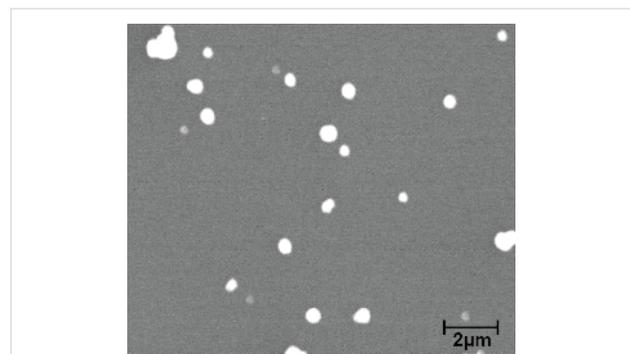
**Figure 4:** SEM image of spherical Au nanoparticles approximately 500 nm in diameter which are referred to as Au 500.
