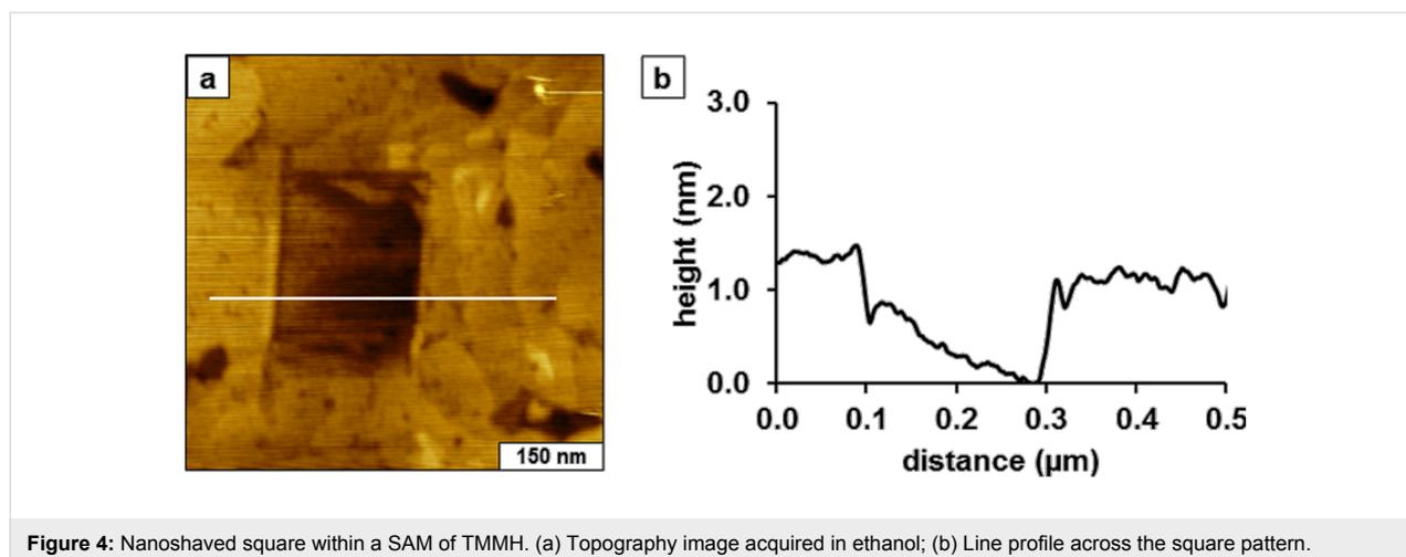
**Figure 4:** Nanoshaved square within a SAM of TMMH. (a) Topography image acquired in ethanol; (b) Line profile across the square pattern.
