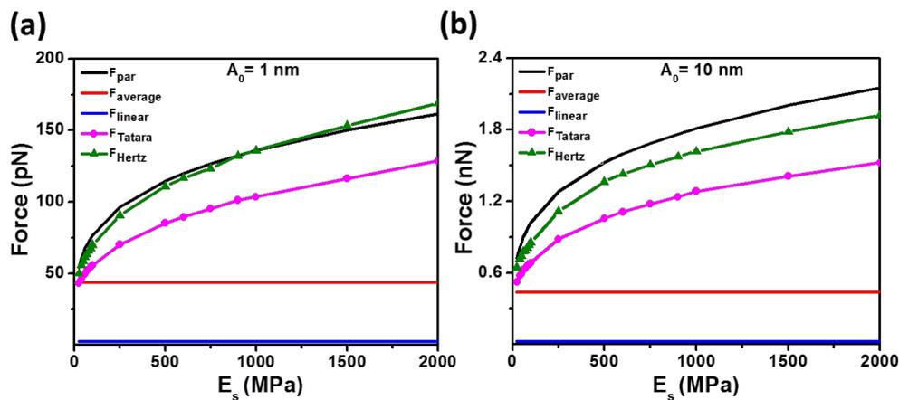
**Figure 2:** Peak force dependence on the Young modulus of the sample for different numerical simulations (Hertz and Tataru) and force analytical approximations (parametrized, average and linear). (a)  $A_0 = 1$  nm,  $R_t = 5$  nm and (b)  $A_0 = 10$  nm,  $R_t = 5$  nm. Other simulation inputs are:  $k = 0.1$  N/m,  $f_0 = 25$  kHz,  $Q = 2$ ,  $R_s = 4$  nm, and  $A_{\text{sp}} = 0.9 A_0$ .
