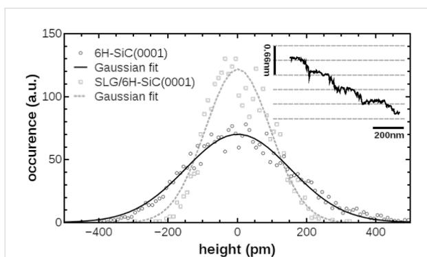
**Figure 2:** Roughness analysis of NC-AFM images taken on a single terrace within  $70 \times 70$  nm<sup>2</sup> on the 6H-SiC(0001) substrate (standard deviation  $\sigma = 304$  pm) and on the SLG ( $\sigma = 189$  pm). The inset shows a line profile taken on the SLG flake perpendicular to substrate step edges measured by Kelvin-compensated NC-AFM.
