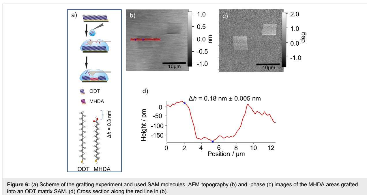
**Figure 6:** (a) Scheme of the grafting experiment and used SAM molecules. AFM-topography (b) and -phase (c) images of the MHDA areas grafted into an ODT matrix SAM. (d) Cross section along the red line in (b).
