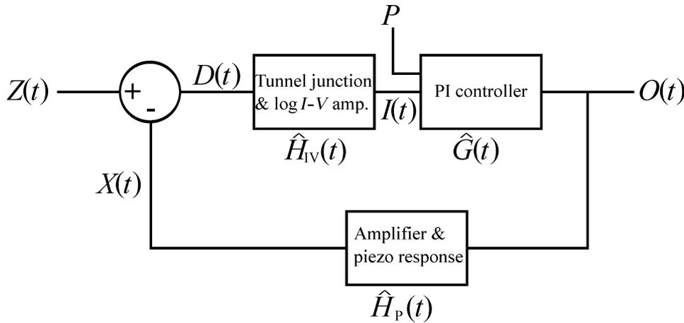
**Figure 3:** Schematic of an STM feedback loop.  $Z(t)$  and  $X(t)$  represent the sample height and  $z$ -piezo extension at time  $t$  respectively, and  $P$  is the set-point current. Other SPM systems can be modelled using the same feedback system by replacing the operator  $\hat{H}_{IV}$ , with an operator that describes the tip-sample interaction and signal amplification of the SPM to be modelled.
