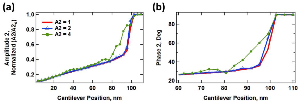
**Figure 9:** Simulated amplitude and phase spectroscopy curves for realistic cantilever trajectories calculated using parameters similar to those of Figure 7 for AM-OL operation. (a) Normalized amplitude ( $A_2/A_{2-free}$ ) vs cantilever position; (b) phase vs cantilever position.
