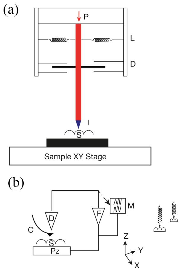
**Figure 2:** (a) Schematic of instrumented nanoindenter, including P - calibrated force; L - support springs; D - Position sensor; I - indenter tip supported by shaft; S - sample. (b) Schematic of AFM showing Pz - piezoelectric motion transducer; S -sample; C - integrated cantilever and tip; D - cantilever motion detector; F - feedback; M - monitor for display. To right the working of AFM is shown schematically: extension of spring changes before and after applying load. From [42].
