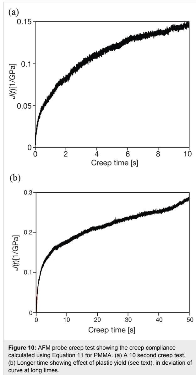
**Figure 10:** AFM probe creep test showing the creep compliance calculated using Equation 11 for PMMA. (a) A 10 second creep test. (b) Longer time showing effect of plastic yield (see text), in deviation of curve at long times.
