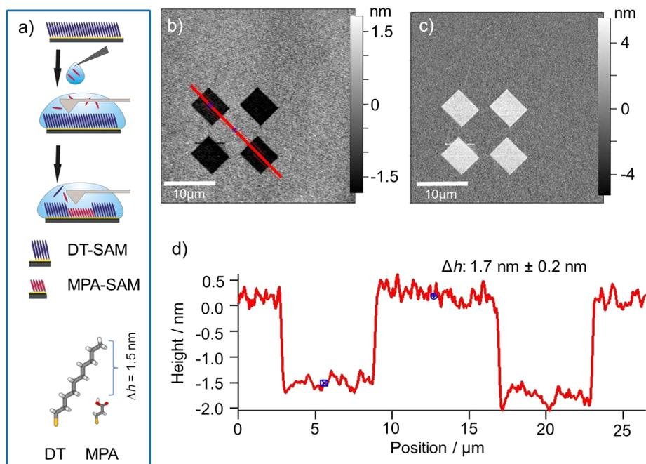
**Figure 3:** (a) Scheme of the grafting experiment and used SAM molecules (without H-atoms). AFM-topography (b) and -phase (c) image of MPA structures grafted in a DT SAM matrix. (d) Cross section along the red line in (b).
