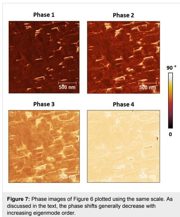
using the same scale. Clearly the highest modes exhibit the smallest phase shift from 90°. In contrast, the phase images acquired driving the fundamental eigenmode in the attractive regime almost always exhibited partial contrast inversion with respect to one another. For example, some bright spots in the
