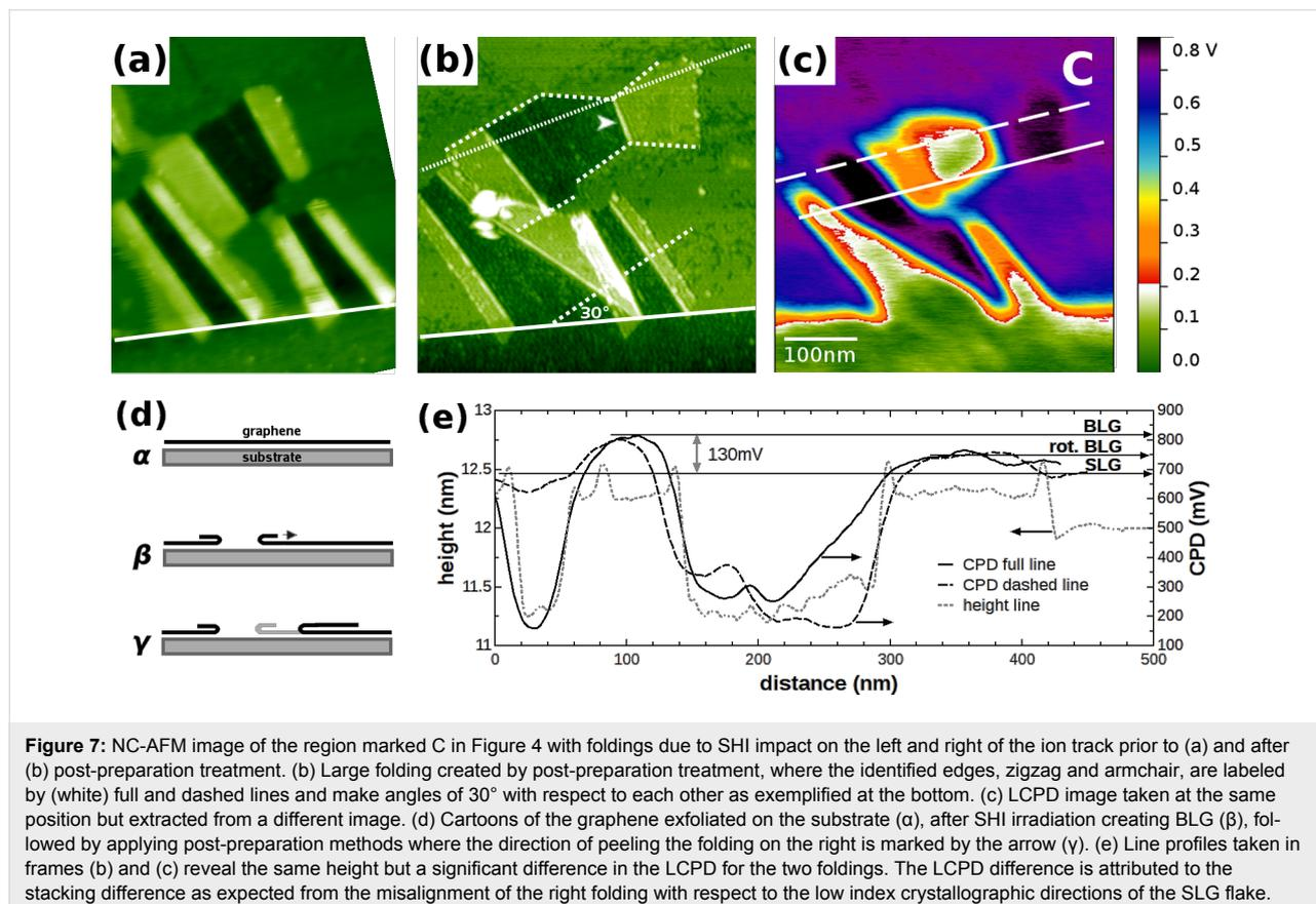
for both foldings is in agreement with the values found in Figure 5 and Figure 6. Within the error of several angstroms for the height measurement, we are unable to discriminate between the AA- and AB-stacking interlayer distance difference of 10% [42,45-47].
