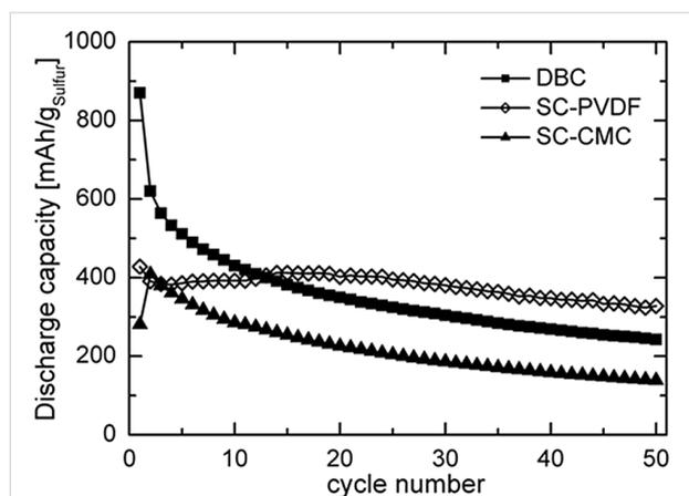
**Figure 1:** Comparison of the cycling performances of non-optimised Li-S batteries prepared with different binders. The batteries were tested in the range of 2.8–1.5 V vs Li/Li<sup>+</sup> at a current density of 533 mA·g<sup>-1</sup> sulfur.
