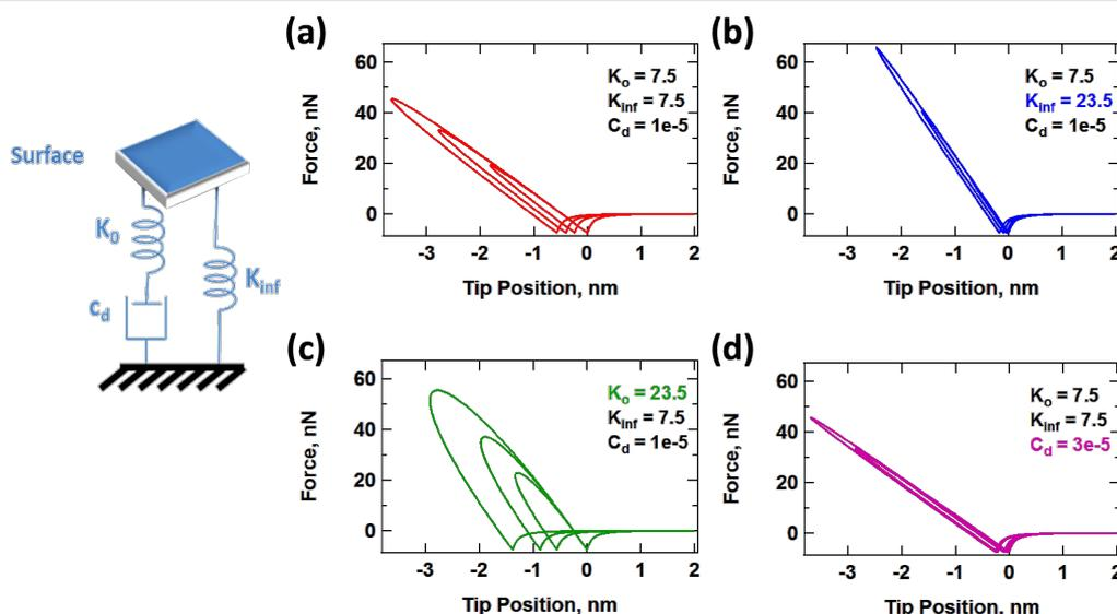
**Figure 10:** Example of the evolution of force–distance trajectories with changes in the SLS surface parameters: (a) baseline; (b) increase in  $K_{inf}$ ; (c) increase in  $K_0$ ; (d) increase in  $C_{diss}$ . The parameters are similar to those given for Figure 7, except for  $A_{2-free} = 5$  nm and any other parameters indicated in the figures.
