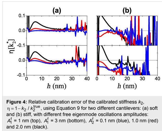
Finally, the linear method is dependent on the unknown higher eigenmode free amplitude,  $A_n^f$ , which must be small for the linear approximation to be valid. Since  $A_n^f$  is not known a priori, one can use the following formula to try to make a rough guess given the known free amplitude of the first mode for the particular drive voltage amplitude
