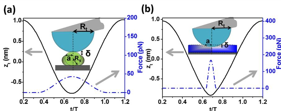
**Figure 1:** Peak forces, tip motion and contact time for two materials. (a) Soft sample ( $E_s = 50$  MPa) simulated with the Tataro interaction force (Equation 4). (b) Rigid sample ( $E_s = 2$  GPa) simulated with the Hertz interaction force (Equation 3). Simulation inputs:  $k = 0.1$  N/m,  $f_0 = 25$  kHz,  $Q = 2$ ,  $A_0 = 1$  nm,  $R_t = 5$  nm,  $R_s = 4$  nm and  $A_{sp} = 0.9 A_0$ .
