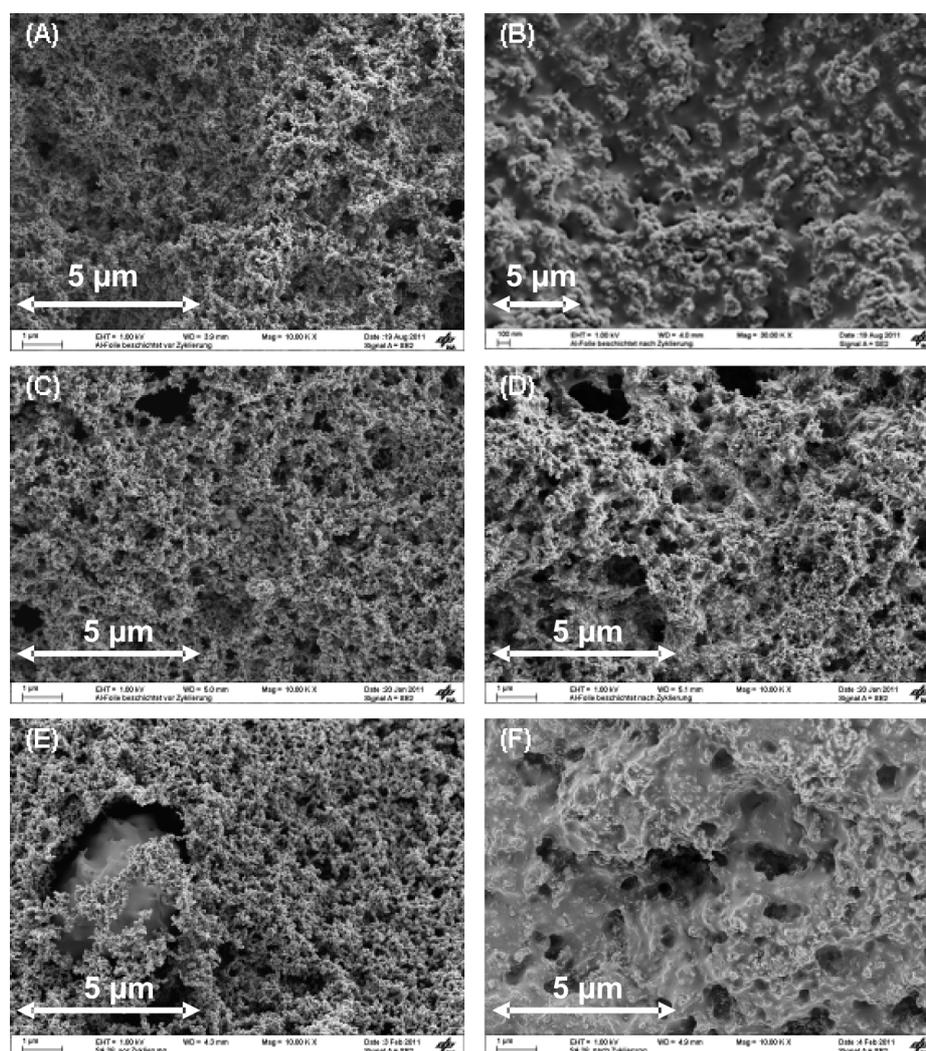
**Figure 2:** SEM images of (a) DBC-PVDF before cycling, (b) DBC-PVDF after the 50th discharge, (c) SC-PVDF before cycling, (d) SC-PVDF after the 50th discharge, (e) SC-CMC before cycling, (f) SC-CMC after the 50th discharge.
