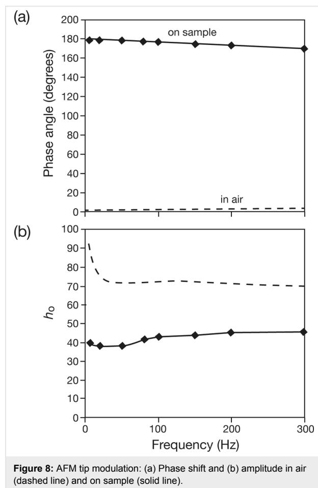
**Figure 8:** AFM tip modulation: (a) Phase shift and (b) amplitude in air (dashed line) and on sample (solid line).
