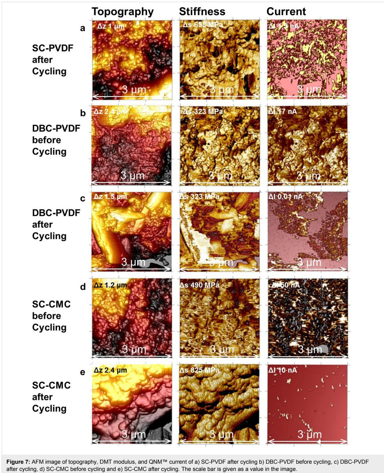
After cycling (Figure 7e) the grains are enlarged, the surface is much smoother, finer particles are lost, and flat terraces are visible in the topography image. However, the total height difference has not changed significantly. The steep (almost
