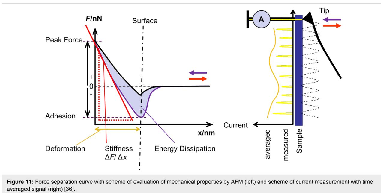
force–separation curve is recorded at every image point and the topography mechanical properties (e.g., adhesion force, energy dissipation, deformation, DMT modulus or stiffness, peak force, phase shift) are simultaneously evaluated. In case of a conductive tip, the current during the contact of the tip with the sample can be recorded. A scheme of a force–distance curve is given in Figure 11 [21].
