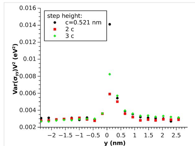
**Figure 2:** Stress fluctuation multiplied by the squared per-atom volume  $\text{Var}(\sigma_{yy})V^2 = V^2(\langle \sigma_{yy}\sigma_{yy} \rangle - \langle \sigma_{yy} \rangle^2)$  along the  $y$ -axis of the upper Ga atoms.
