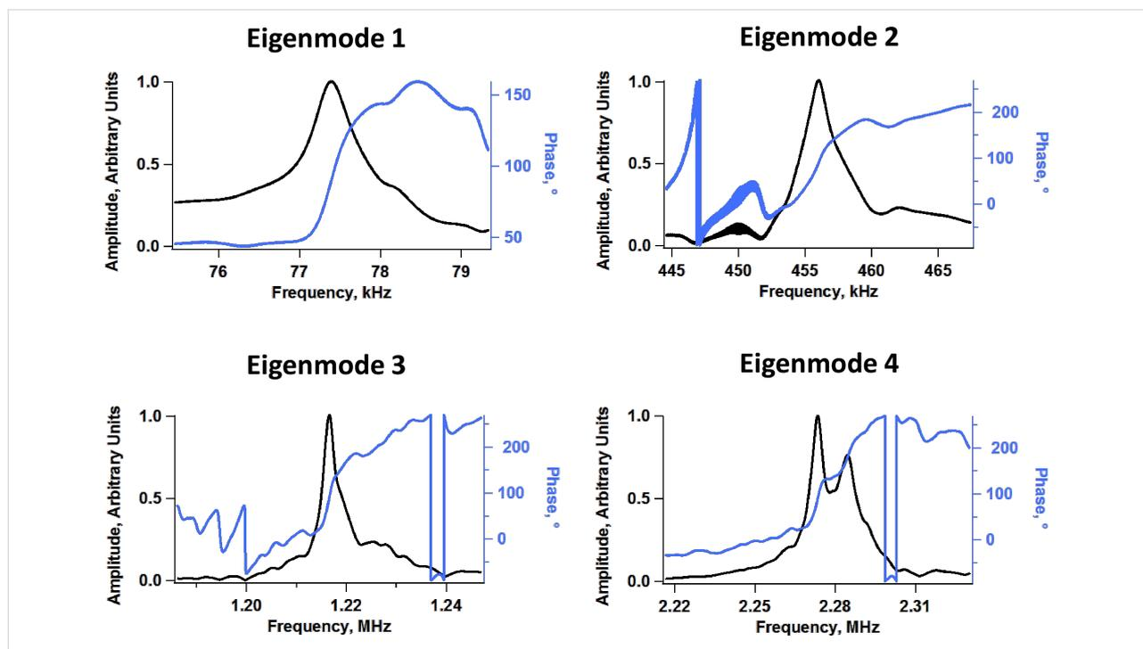
**Figure 1:** Example of measured frequency response of the first four eigenmodes of one of the rectangular cantilevers used in our experiments, which have nominal fundamental resonance frequency and force constant of 70 kHz and 2 N/m, respectively. As the mode order increases the shape of the peak increasingly deviates from the ideal response of a damped harmonic oscillator.
