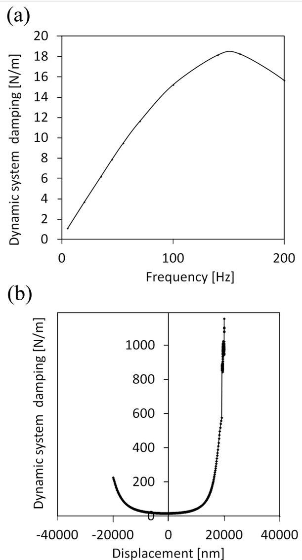
**Figure 6:** Calibration of the system damping for INI. The damping was computed for each frequency at different vertical extensions of the indenter over a range of  $\pm 30 \mu\text{m}$ . The damping is computed by using Equations 9–11 and is reported here as  $C_1\omega$ . (a) System damping as a function of the frequency for a displacement near 0. (b) System damping as a function of the displacement of the indenter head at 200 Hz frequency.
