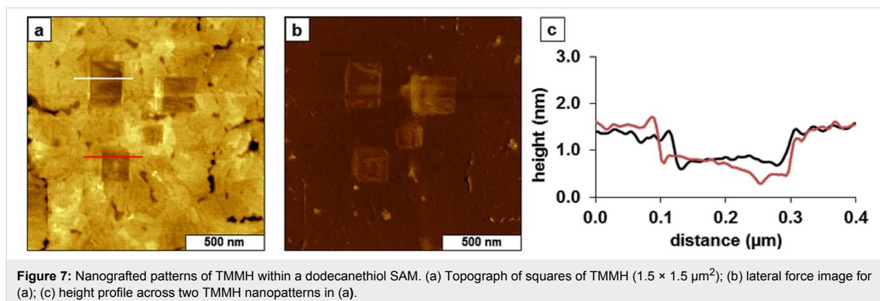
**Figure 7:** Nanografted patterns of TMMH within a dodecanethiol SAM. (a) Topograph of squares of TMMH ( $1.5 \times 1.5 \mu\text{m}^2$ ); (b) lateral force image for (a); (c) height profile across two TMMH nanopatterns in (a).
