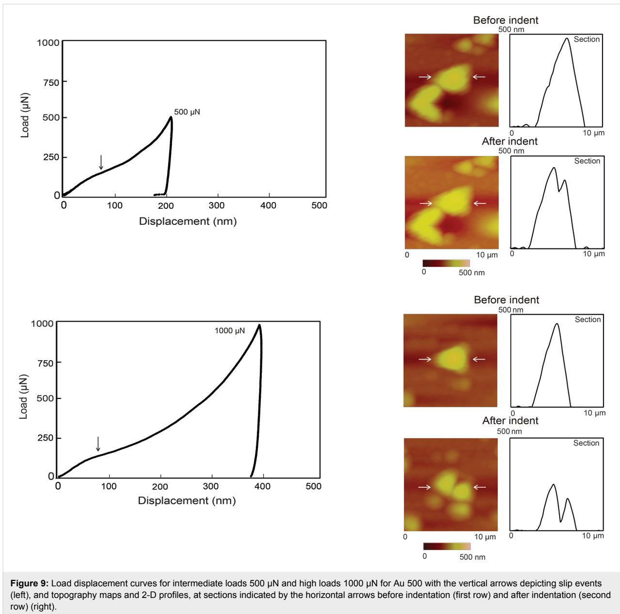
arrows in the topography maps indicate the nanoparticle of interest along with the section on which the profiles were taken. The vertical arrows shown in the load–displacement curves (left) point to slip events where the nanoparticles start to break apart during indentation leading to displacement of material below the Berkovich tip.
