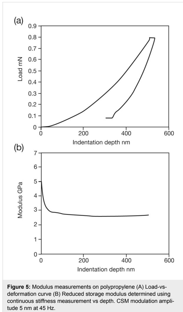
**Figure 5:** Modulus measurements on polypropylene (A) Load-vs-deformation curve (B) Reduced storage modulus determined using continuous stiffness measurement vs depth. CSM modulation amplitude 5 nm at 45 Hz.
