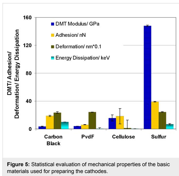
only conductive sample in this series. In the other properties, sulfur differed slightly from carbon black and binder with a smaller energy dissipation and a slightly increased adhesion. It is noted, that the measured DMT modulus has values out of the recommended range for this type of tip. Therefore, the accuracy of those values is not very high. However, the large differences allowed a good differentiation from carbon. No significant differences were found for the deformation values with the
