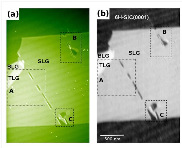
**Figure 4:** NC-AFM image (a) of an exfoliated SLG flake on 6H-SiC(0001), irradiated with SHI and subjected to post-preparation treatment, and its corresponding LCPD image (b). Folding structures, which result from post-preparation treatment labeled by A, B and C are analyzed in detail in Figure 5, Figure 6 and Figure 7.
