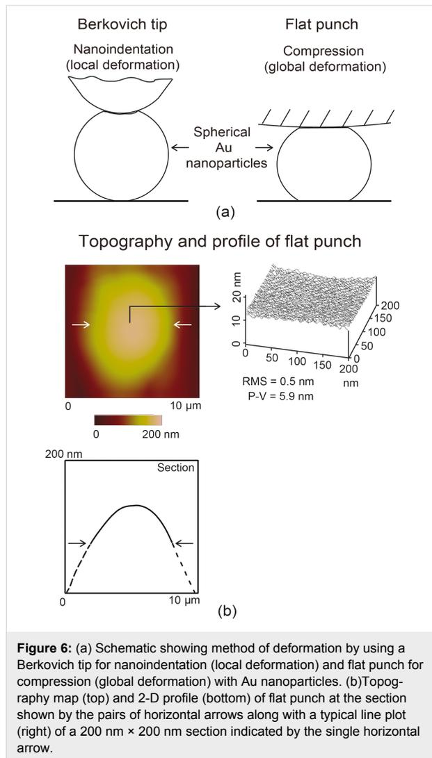
**Figure 6:** (a) Schematic showing method of deformation by using a Berkovich tip for nanoindentation (local deformation) and flat punch for compression (global deformation) with Au nanoparticles. (b) Topography map (top) and 2-D profile (bottom) of flat punch at the section shown by the pairs of horizontal arrows along with a typical line plot (right) of a 200 nm  $\times$  200 nm section indicated by the single horizontal arrow.
