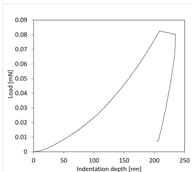
**Figure 3:** Load-vs-displacement curve taken by nanoindentation with a Berkovich indenter tip on a polyurethane sample showing negative stiffness, seen as the outward bulging of the curve, which develops in the unloading (right branch) of the curve, because of creep.
