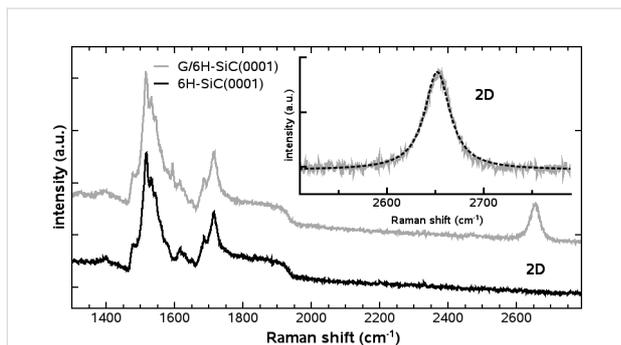
**Figure 1:** Micro-Raman spectrum for both, the substrate and the SLG flake introduced in Figure 3. The inset shows the 2D Raman peak and its Lorentzian fit.
