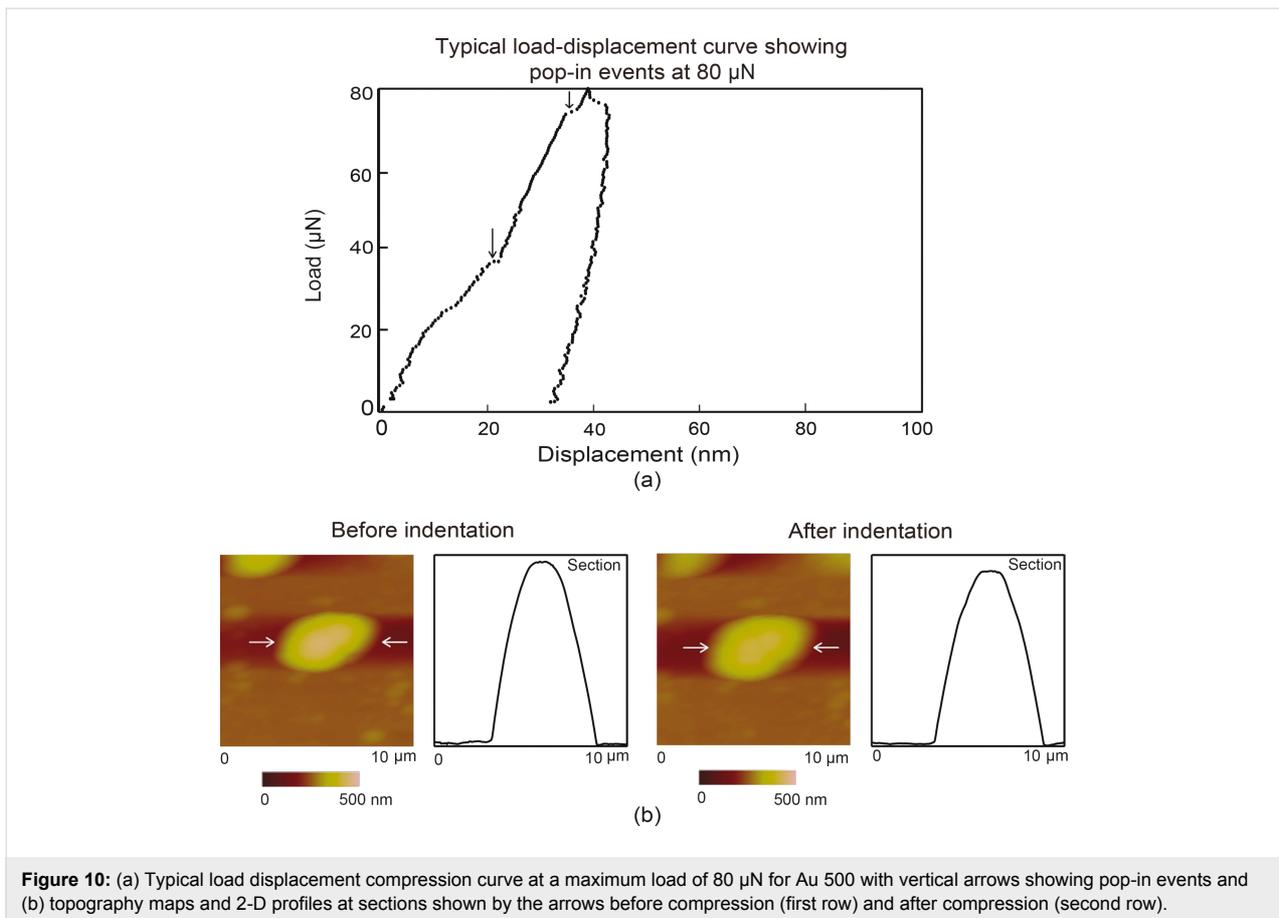
**Figure 10:** (a) Typical load displacement compression curve at a maximum load of 80  $\mu\text{N}$  for Au 500 with vertical arrows showing pop-in events and (b) topography maps and 2-D profiles at sections shown by the arrows before compression (first row) and after compression (second row).
