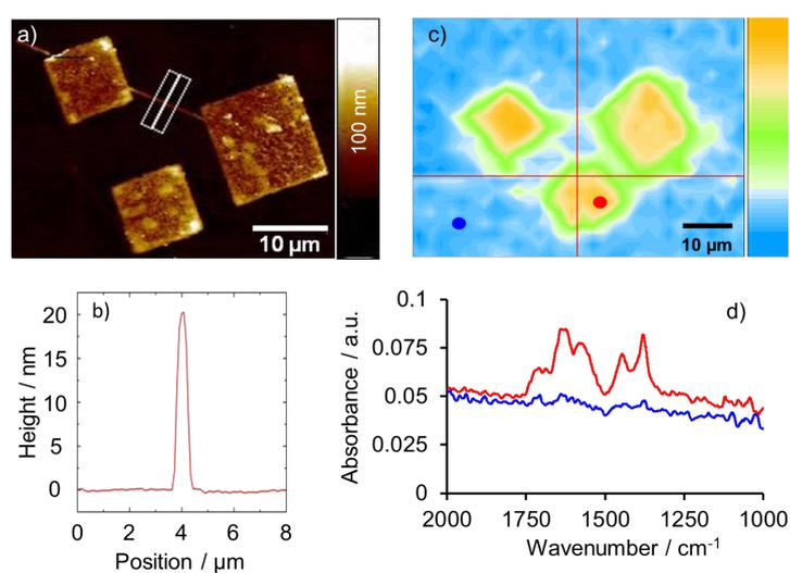
**Figure 5:** (a) AFM-topography image of HKUST-1 structures, prepared by spray coating after grafting squared areas of MPA into the DT matrix thiol. (b) Cross section along the white line of (a). (c) FT-IR imaging of the wavenumber region between  $1510\text{ cm}^{-1}$  and  $1780\text{ cm}^{-1}$ . (d) FT-IR spectra representing the area inside the squares (red line in (d) corresponding to red dot in (c)) and outside of the structures (blue line in (d), according to the blue dot in (c)).
