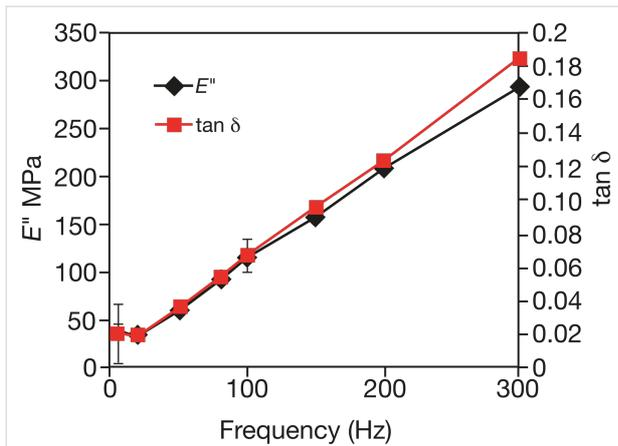
**Figure 9:** Dynamic AFM measurements of iPP as a function of the frequency. The measurements were made at a depth  $h = 50$  nm by using a probe with a spring constant  $k = 33$  N/m and a nominal tip radius of 50 nm. The oscillation amplitude was maintained at 10 nm.
