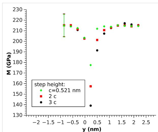
**Figure 3:** Local [001]-oriented indentation modulus for three different step heights along the  $y$ -axis. Measured by indenting a single atom ( $A_1 = 0.088 \text{ nm}^2$ ). The error bars denote the standard deviation of the displacement and apply to all data points.
