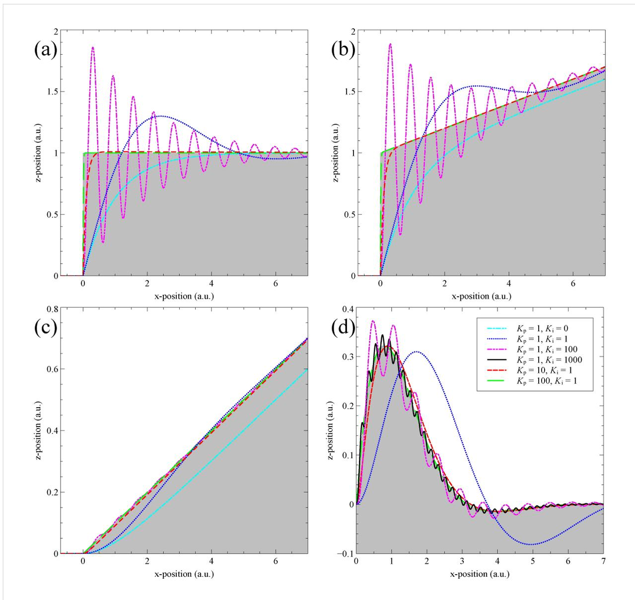
**Figure 4:** The feedback response of an SPM, without the inclusion of mechanical resonances, calculated for four different topographies, and for a range of feedback gains. Topographies in (a)–(d) correspond to Equation 16–Equation 19 respectively. Not all gains are plotted for all topographies to avoid overcrowding.
