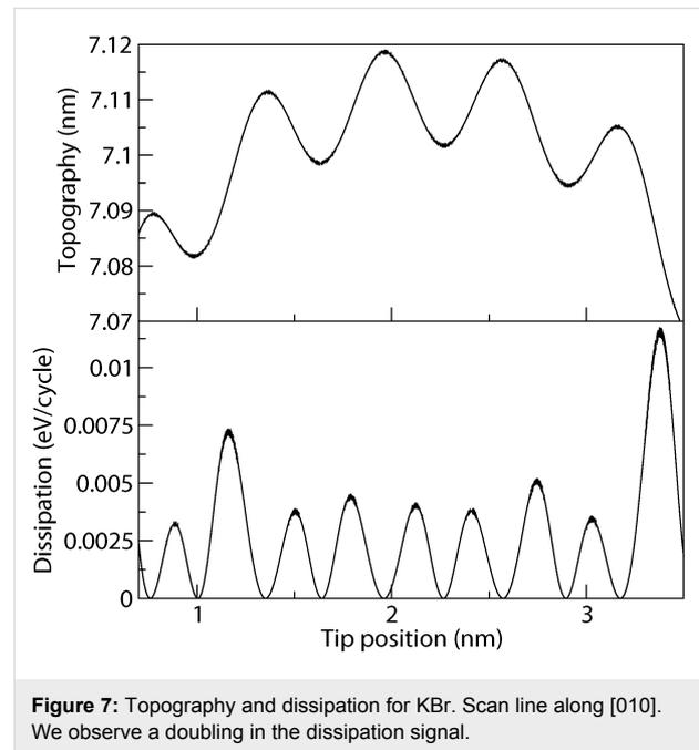
**Figure 7:** Topography and dissipation for KBr. Scan line along [010]. We observe a doubling in the dissipation signal.
