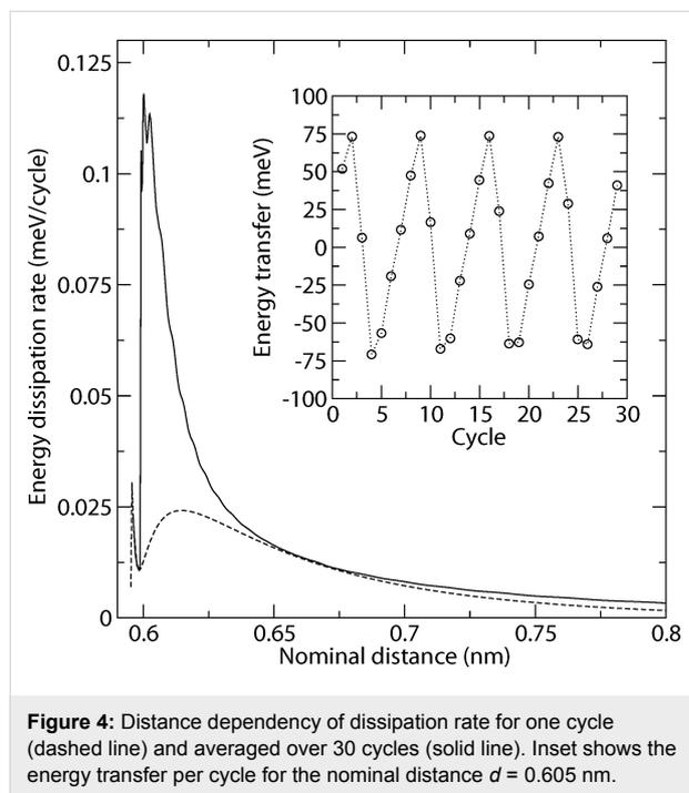
**Figure 4:** Distance dependency of dissipation rate for one cycle (dashed line) and averaged over 30 cycles (solid line). Inset shows the energy transfer per cycle for the nominal distance  $d = 0.605$  nm.
