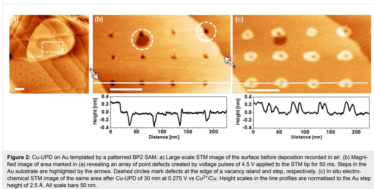
is not affected to the extent that the passivation against UPD breaks down. There is no UPD outside the damaged areas, which confirms the excellent quality of the BP2 SAM.
