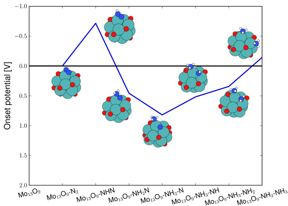
**Figure 4:** Diagram of the required applied potential to make each reaction step exergonic for electrochemical ammonia production on the  $Mo_{13}O_9$  through the associative mechanism. For all five studied reaction pathways, the highest required potential is  $-0.7$  V for the first protonation step.
