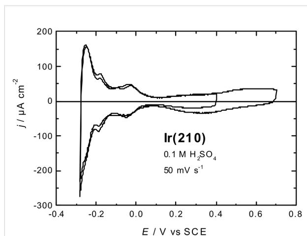
**Figure 1:** Cyclic voltammograms of Ir(210), which was annealed and cooled in a  $\text{N}_2 + \text{CO}$  mixture, after anodic stripping of the CO adlayer in  $0.1 \text{ M H}_2\text{SO}_4$ . Scan rate:  $50 \text{ mV}\cdot\text{s}^{-1}$ .
