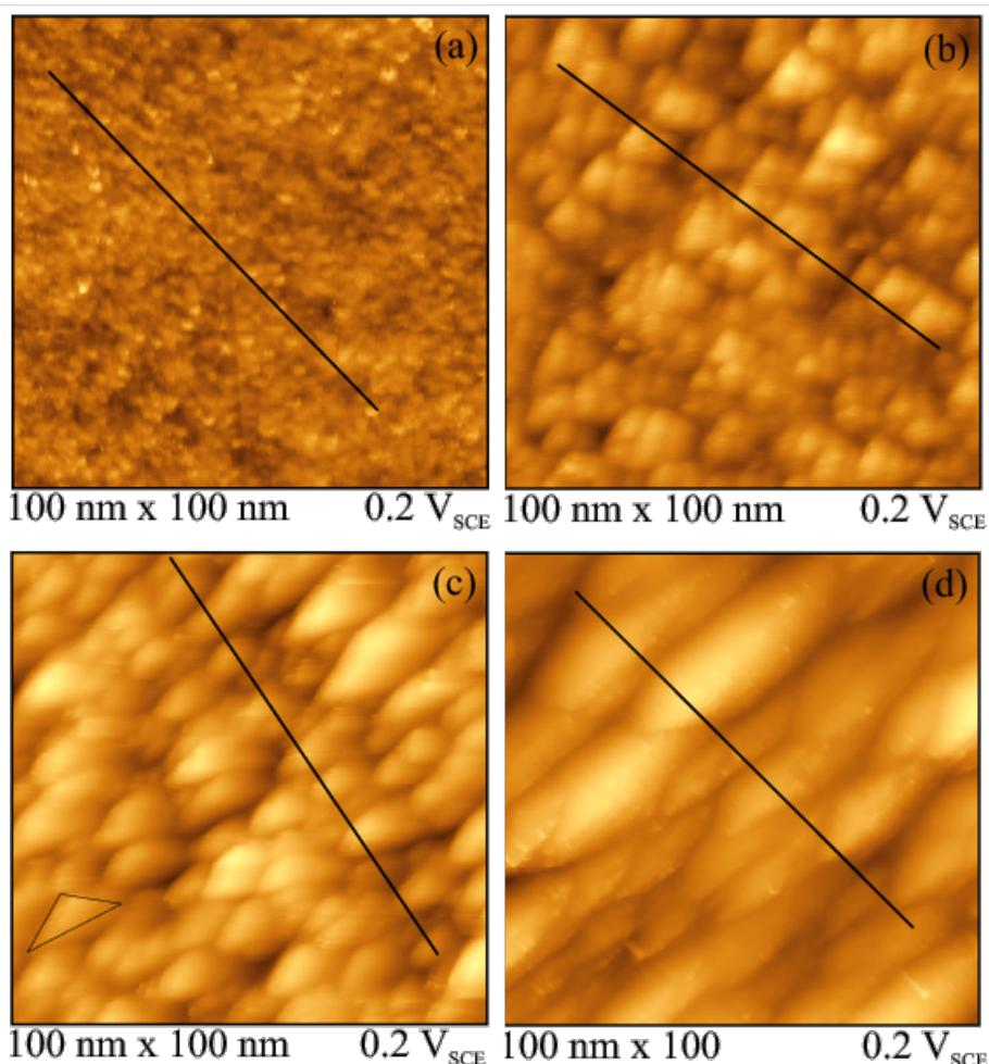
**Figure 6:** In situ STM images ( $100 \times 100 \text{ nm}^2$ ) of CO-cooled Ir(210) surface in 0.1 M  $\text{H}_2\text{SO}_4$  after cycling between  $-0.28$  and  $0.7 \text{ V}$  at  $1 \text{ V}\cdot\text{s}^{-1}$  for (a) 1, (b) 20, (c) 60 and (d) 240 min.
