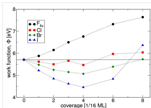
**Figure 2:** Calculated change of the work function vs coverage for the adsorption of fluorine, chlorine, bromine and iodine on Pt(111). The high value for the 0.5 ML calculation of iodine is due to a double layer structure of the adsorbates, caused by the larger size of iodine atoms.
