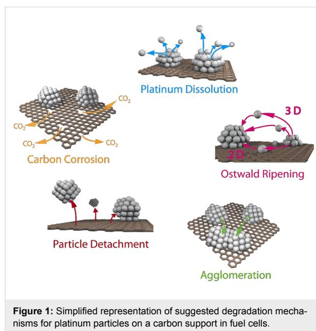
**Figure 1:** Simplified representation of suggested degradation mechanisms for platinum particles on a carbon support in fuel cells.
