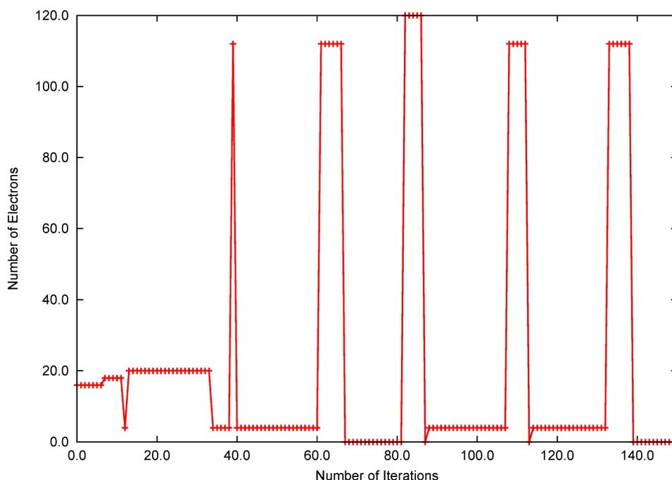
**Figure 1:** Evolution of the number of electrons with the number of iterations for O<sub>2</sub> if the potential dependent energy is computed by inserting the aspired  $\mu$  into Equation 2.
