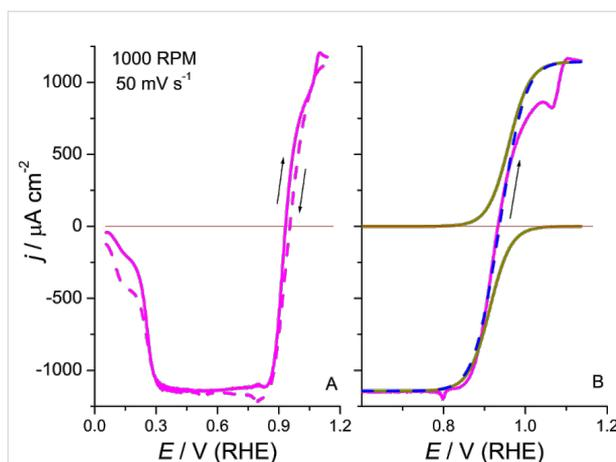
**Figure 9:** Hydrogen peroxide reduction and oxidation reactions on Pt(111) in 0.1 M  $\text{HClO}_4$  + 1 mM  $\text{H}_2\text{O}_2$ . (A) Cyclic voltammetric profile: Positively (solid line) and negatively directed (dashed line) sweeps. (B) Adjusted curves for HPOR and HPRR (dotted lines) during the positive scan. The dashed line corresponds to the sum of currents from the fitted branches and the solid line is the experimental curve after subtracting the blank.
