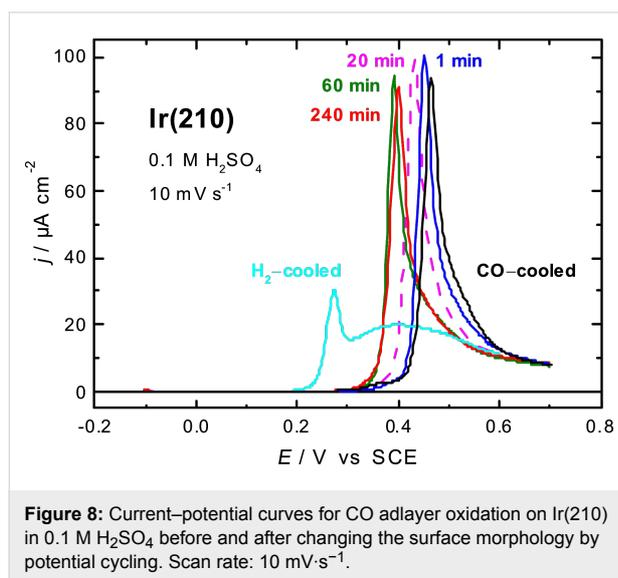
**Figure 8:** Current–potential curves for CO adlayer oxidation on Ir(210) in 0.1 M H<sub>2</sub>SO<sub>4</sub> before and after changing the surface morphology by potential cycling. Scan rate: 10 mV s<sup>-1</sup>.
