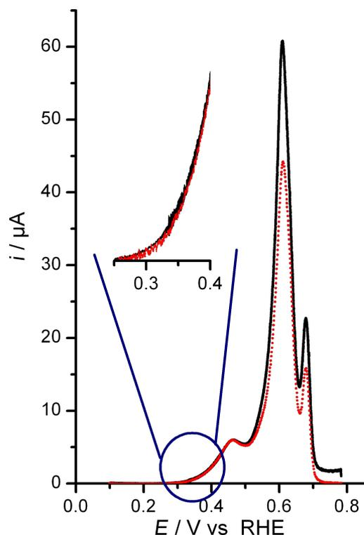
**Figure 5:** Normalized mass spectrometric current ( $m/z = 44$ ,  $\text{CO}_2$  detection, red dotted line) and Faradaic current (black solid line) acquired during the  $\text{CO}_{\text{ad}}$  stripping experiment on (111+100)-NC ( $v = 1 \text{ mV s}^{-1}$ ). The  $\text{CO}$  adlayer was formed by adsorption from  $\text{CO}$  saturated electrolyte at  $0.10 \text{ V}$  ( $0.5 \text{ M H}_2\text{SO}_4$ ).
