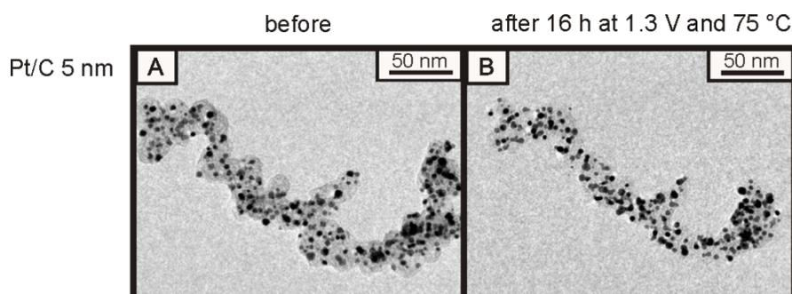
**Figure 10:** IL-TEM micrograph of Pt/C 5 nm subjected to 1.3  $V_{\text{RHE}}$  at 348 K (75 °C) for 16 h in 0.1 M  $\text{HClO}_4$ . A shrinkage of the carbon support due to carbon corrosion with successive decrease in inter-particle distances and coalescence can be observed. The images were reprinted with permission from [49]. Copyright 2011 Elsevier.
