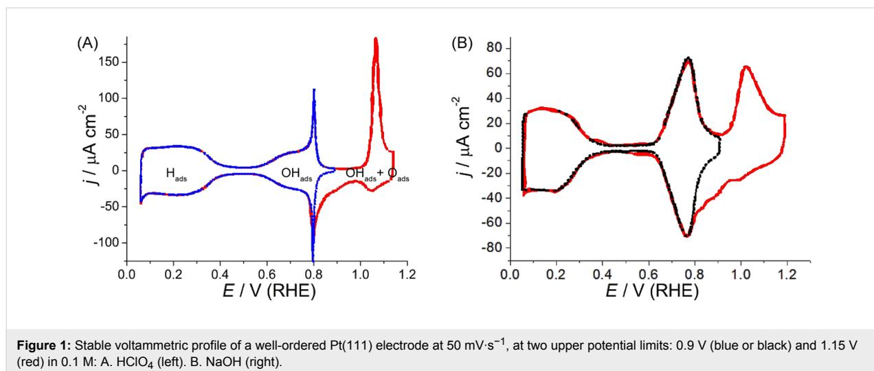
**Figure 1:** Stable voltammetric profile of a well-ordered Pt(111) electrode at  $50 \text{ mV}\cdot\text{s}^{-1}$ , at two upper potential limits: 0.9 V (blue or black) and 1.15 V (red) in 0.1 M: A.  $\text{HClO}_4$  (left). B.  $\text{NaOH}$  (right).
