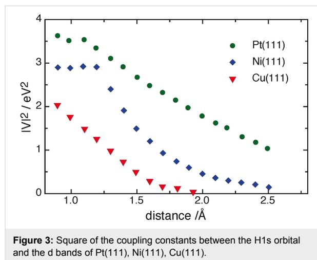
**Figure 3:** Square of the coupling constants between the H1s orbital and the d bands of Pt(111), Ni(111), Cu(111).
