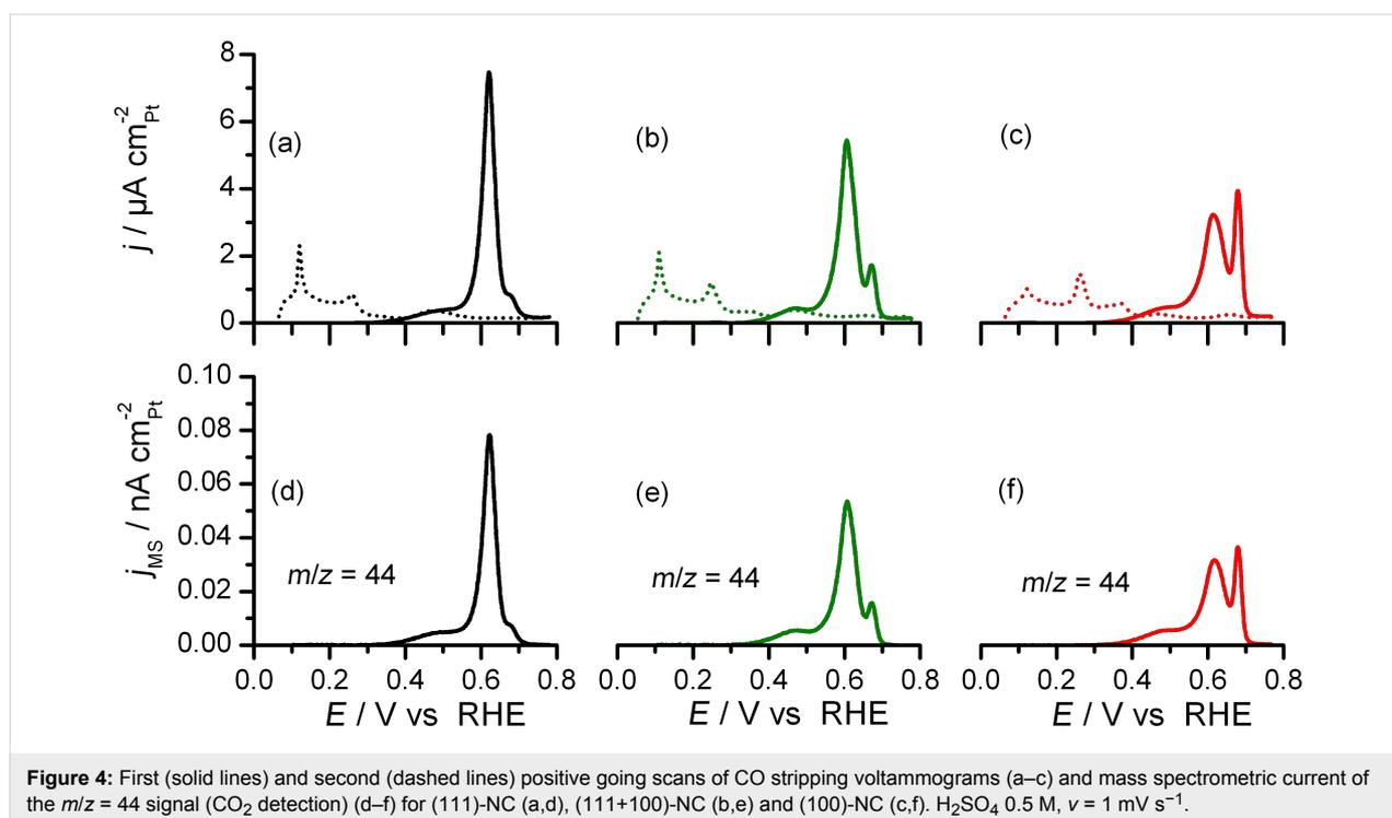
**Figure 4:** First (solid lines) and second (dashed lines) positive going scans of CO stripping voltammograms (a–c) and mass spectrometric current of the  $m/z = 44$  signal (CO<sub>2</sub> detection) (d–f) for (111)-NC (a,d), (111+100)-NC (b,e) and (100)-NC (c,f). H<sub>2</sub>SO<sub>4</sub> 0.5 M,  $\nu = 1 \text{ mV s}^{-1}$ .
