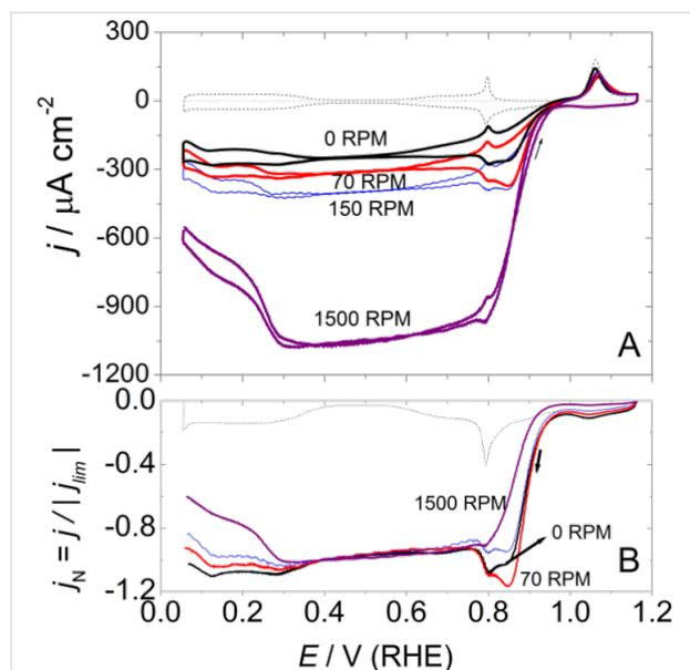
**Figure 7:** (A) Cyclic voltammograms for the ORR on a hanging meniscus rotating disc (HMCD) Pt(111) electrode from 0.06 to 1.15 V in 0.1 M HClO<sub>4</sub>, Ar/O<sub>2</sub> ratio 5:1. Scan rate  $50 \text{ mV}\cdot\text{s}^{-1}$ . (B) Negatively directed sweep normalized against the limiting currents from data in (A).
