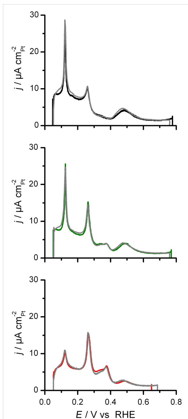
**Figure 2:** Comparison of the anodic scan of the hydrogen-region voltammograms recorded in the beaker cell (colored lines) and in the spectro-electrochemical flow cell (grey lines) at  $10 \text{ mV s}^{-1}$  in 0.5 M  $\text{H}_2\text{SO}_4$ . From top to bottom: (111)-NC, (111+100)-NC and (100)-NC.
