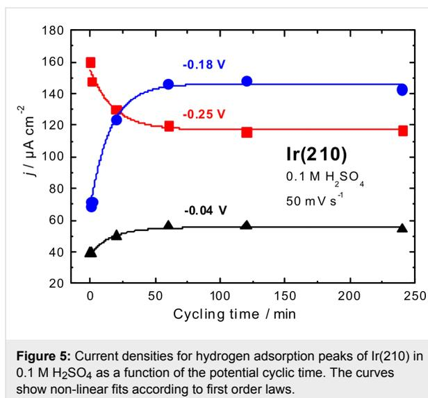
**Figure 5:** Current densities for hydrogen adsorption peaks of Ir(210) in 0.1 M H<sub>2</sub>SO<sub>4</sub> as a function of the potential cyclic time. The curves show non-linear fits according to first order laws.
