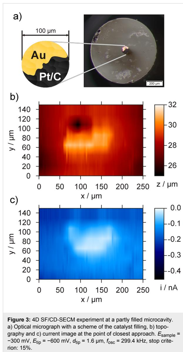
**Figure 3:** 4D SF/CD-SECM experiment at a partly filled microcavity. a) Optical micrograph with a scheme of the catalyst filling, b) topography and c) current image at the point of closest approach.  $E_{\text{sample}} = -300$  mV,  $E_{\text{tip}} = -600$  mV,  $d_{\text{tip}} = 1.6$   $\mu\text{m}$ ,  $f_{\text{osc}} = 299.4$  kHz, stop criterion: 15%.
