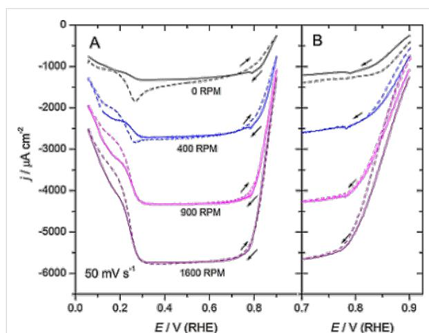
**Figure 3:** Oxygen reduction on a Pt(111) electrode in oxygen saturated 0.1 M HClO<sub>4</sub>. (A): Cyclic voltammetric profile: Positively (dashed line) and negatively directed (solid line) sweeps. The electrode was kept at the initial potential  $E_i = 0.06$  V for 10 s before each measurement. (B): Negatively directed sweeps when the electrode was kept at  $E_i = 0.06$  V (solid line) and at  $E_i = 0.90$  V (dashed line) for 10 s before each measurement [18].
