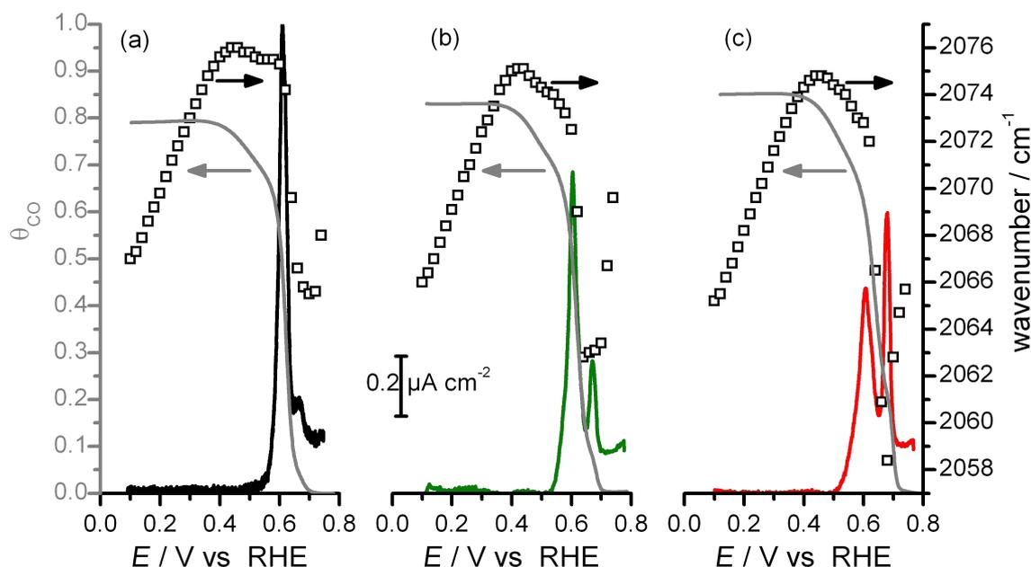
**Figure 6:** Plots of the currents from (bi)sulfate anions re-adsorption (colored traces), absolute  $\text{CO}_{\text{ad}}$  coverages ( $\theta_{\text{CO}}$ , grey traces) and IR band frequencies for linearly adsorbed  $\text{CO}$  (open square) as function of the electrode potential for (111)-NC (a), (111+100)-NC (b) and (100)-NC (c) ( $0.5 \text{ M H}_2\text{SO}_4$ ,  $v = 1 \text{ mV s}^{-1}$ ).
