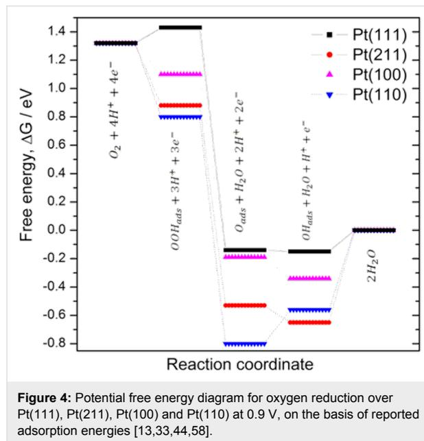
**Figure 4:** Potential free energy diagram for oxygen reduction over Pt(111), Pt(211), Pt(100) and Pt(110) at 0.9 V, on the basis of reported adsorption energies [13,33,44,58].
