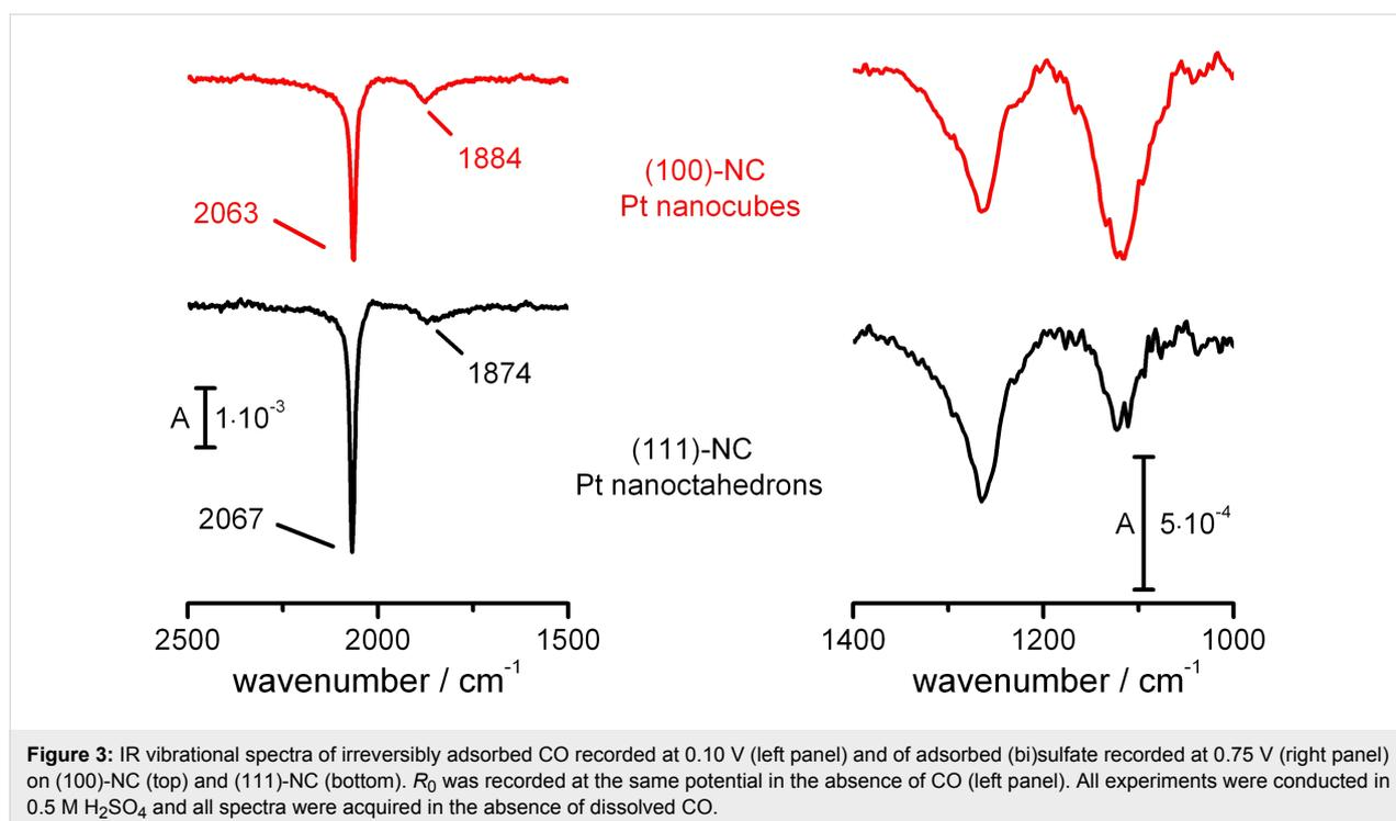
**Figure 3:** IR vibrational spectra of irreversibly adsorbed CO recorded at 0.10 V (left panel) and of adsorbed (bi)sulfate recorded at 0.75 V (right panel) on (100)-NC (top) and (111)-NC (bottom).  $R_0$  was recorded at the same potential in the absence of CO (left panel). All experiments were conducted in 0.5 M  $\text{H}_2\text{SO}_4$  and all spectra were acquired in the absence of dissolved CO.
