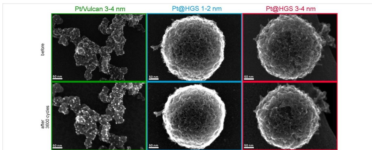
**Figure 4:** IL-SEM of Pt/Vulcan 3–4 nm (green), Pt@HGS 1–2 nm (blue) and Pt@HGS 3–4 nm (red) after 0 (top) and after 3600 (bottom) potential cycles between 0.4 and 1.4  $V_{RHE}$  in 0.1 M  $HClO_4$  at a scan rate of  $1 V \cdot s^{-1}$ . IL-SEM visualizes the surface morphology of the materials, in particular the support structure, which is demonstrated not to undergo significant changes during potential cycling at room temperature.
