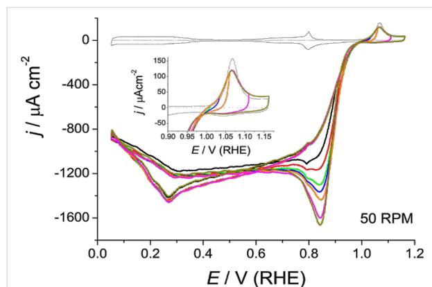
**Figure 8:** Cyclic voltammograms in the high potential region for the ORR on a HMCD Pt(111) electrode in oxygen saturated 0.1 M HClO<sub>4</sub>, at different upper potentials and 50 rpm. Inset: Detailed view of the Pt(111) oxide formation region.
