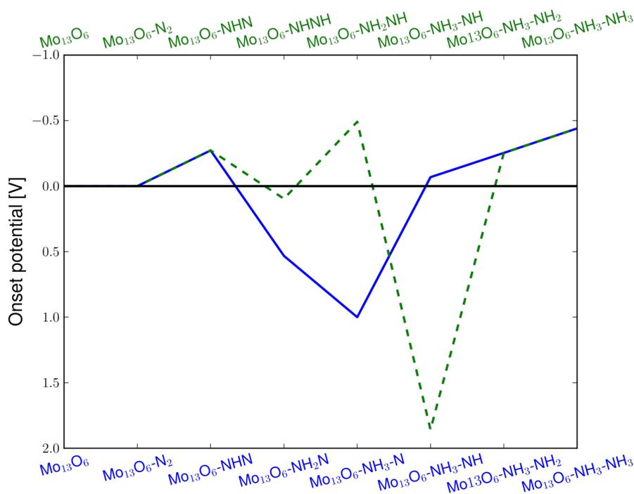
**Figure 5:** Diagram of the required applied potential to make each reaction step exergonic for electrochemical ammonia production on the  $\text{Mo}_{13}\text{O}_6$  through the associative mechanism. The limiting reaction is the last protonation to form the second ammonia on the surface requiring a potential of  $-0.45$  V to become exergonic.
