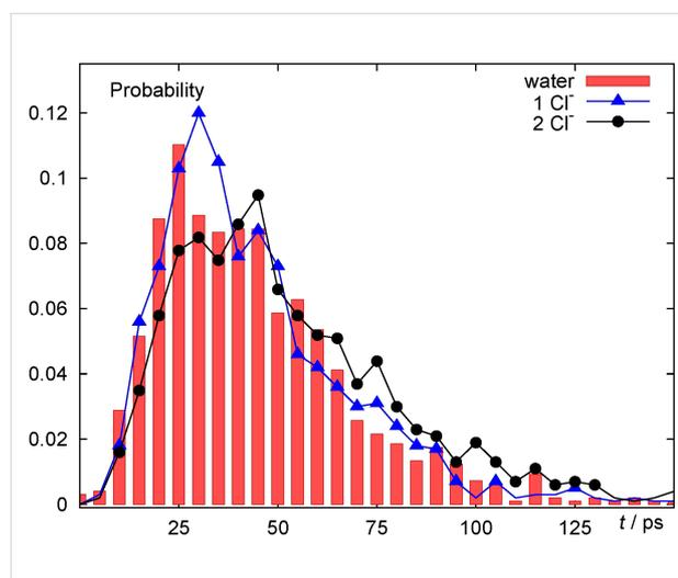
**Figure 2:** Distribution of discharge times (represented as probabilities to observe discharge within a 5 ps time interval) for a system of pure water (red boxes), of one fully charged adsorbed  $\text{Cl}^-$  ion (blue triangles) and two fully charged adsorbed  $\text{Cl}^-$  ions (black circles). In all three cases the total surface charge was  $-5e$  and, consequently, the homogeneous surface charge density corresponded to  $-5e$ ,  $-4e$  and  $-3e$ , respectively.
