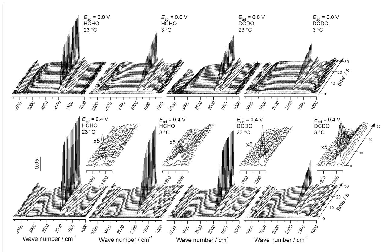
**Figure 1:** Temporal evolution of the ATR-FTIR spectra upon admission of 0.1 M H<sub>2</sub>- or D<sub>2</sub>-formaldehyde solution in 0.5 M  $\text{HClO}_4$  at 0.0 V (upper panel) or 0.4 V (lower panel) to a Pt film electrode at different temperatures (for notations see figure). Insets: five-fold magnified temporal evolution of adsorbed formate band.
