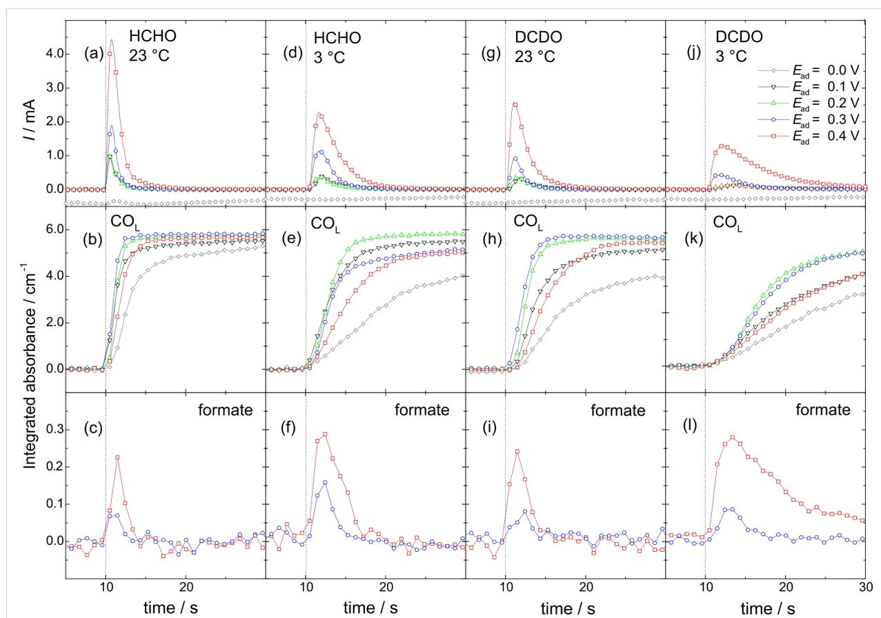
**Figure 3:** Transients of Faradaic current (upper panel) and integrated intensities of linearly bonded  $\text{CO}_{\text{ad}}$  (middle panel) and adsorbed bridge-bonded formate (for 0.3 and 0.4 V only) bands upon admission of 0.1 M H2- or D2-formaldehyde solution in 0.5 M  $\text{HClO}_4$  to a Pt film electrode biased at 0.0, 0.1, 0.2, 0.3 and 0.4 V at 23 or  $3\text{ }^{\circ}\text{C}$  temperature (see figure for notations).
