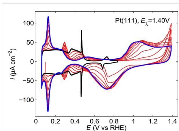
**Figure 2:** Evolution of the voltammetric profile of a Pt(111) electrode in 0.5 M  $\text{H}_2\text{SO}_4$  as the electrode is cycled at  $50 \text{ mV}\cdot\text{s}^{-1}$  between 0.06 and 1.4 V vs RHE. The black line shows the initial stable profile up to 0.85 V and the blue line the profile attained after 12 cycles (partially represented in red).
