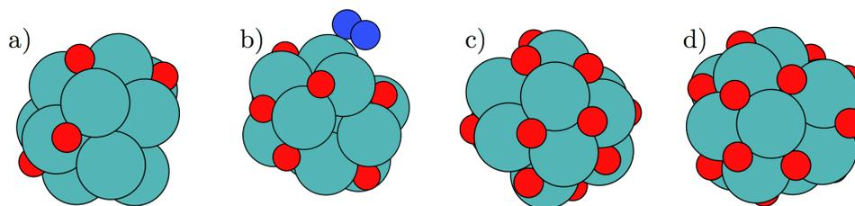
**Figure 3:** (a) The  $\text{Mo}_{13}\text{O}_6$  nanocluster, (b) the  $\text{Mo}_{13}\text{O}_9$  nanocluster with  $\text{N}_2$  adsorbed, (c) the  $\text{Mo}_{13}\text{O}_{12}$  with an almost filled oxygen skin, (d) the  $\text{Mo}_{13}\text{O}_{16}$  with a filled oxygen skin. At the  $\text{Mo}_{13}\text{O}_{16}$ , the oxygen adsorption sites are a mix of three fold hollow sites and bridge sites.
