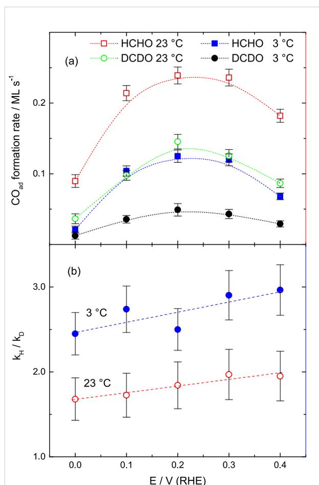
**Figure 4:** Initial CO<sub>ad</sub> formation rates (a) and kinetic isotope effects for the CO<sub>ad</sub> formation (b) upon admission of 0.1 M H<sub>2</sub>- or D<sub>2</sub>-formaldehyde to a Pt film electrode in 0.5 M HClO<sub>4</sub> at different potentials and temperatures (see figure for notations). Lines are included to guide the eye.
