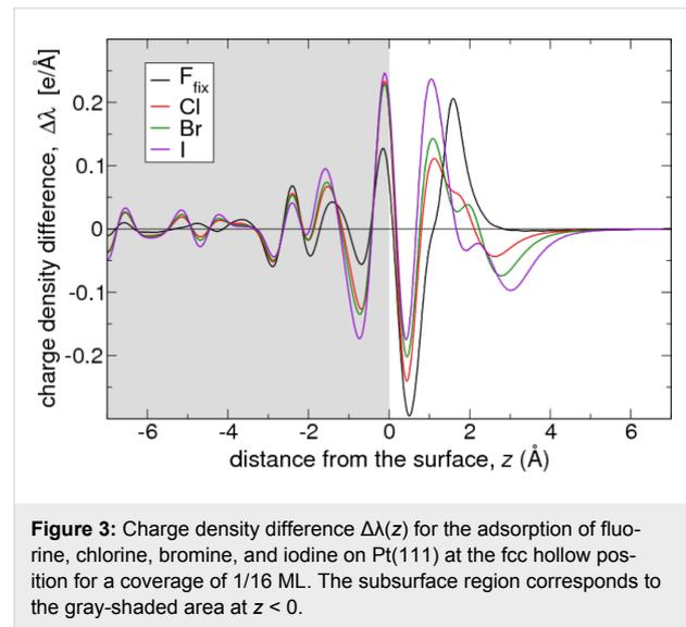
**Figure 3:** Charge density difference  $\Delta\lambda(z)$  for the adsorption of fluorine, chlorine, bromine, and iodine on Pt(111) at the fcc hollow position for a coverage of 1/16 ML. The subsurface region corresponds to the gray-shaded area at  $z < 0$ .
