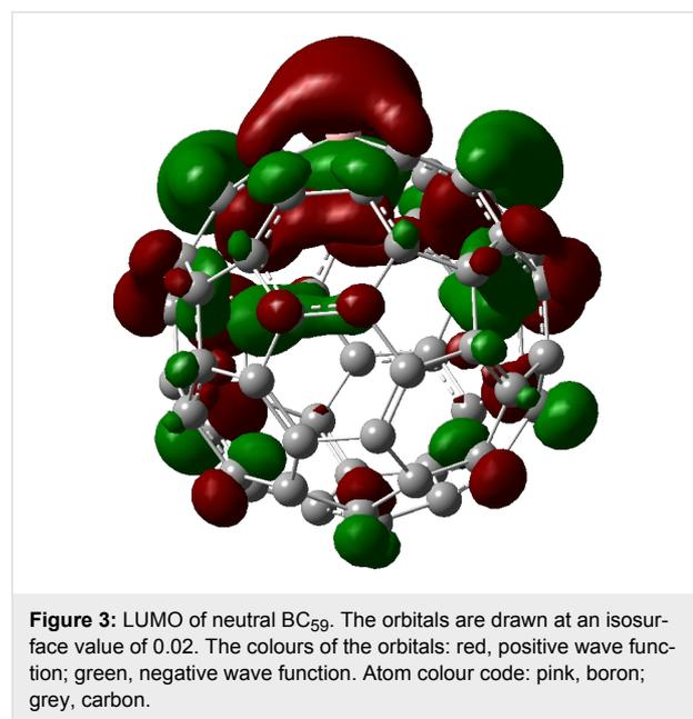
**Figure 3:** LUMO of neutral BC<sub>59</sub>. The orbitals are drawn at an isosurface value of 0.02. The colours of the orbitals: red, positive wave function; green, negative wave function. Atom colour code: pink, boron; grey, carbon.
