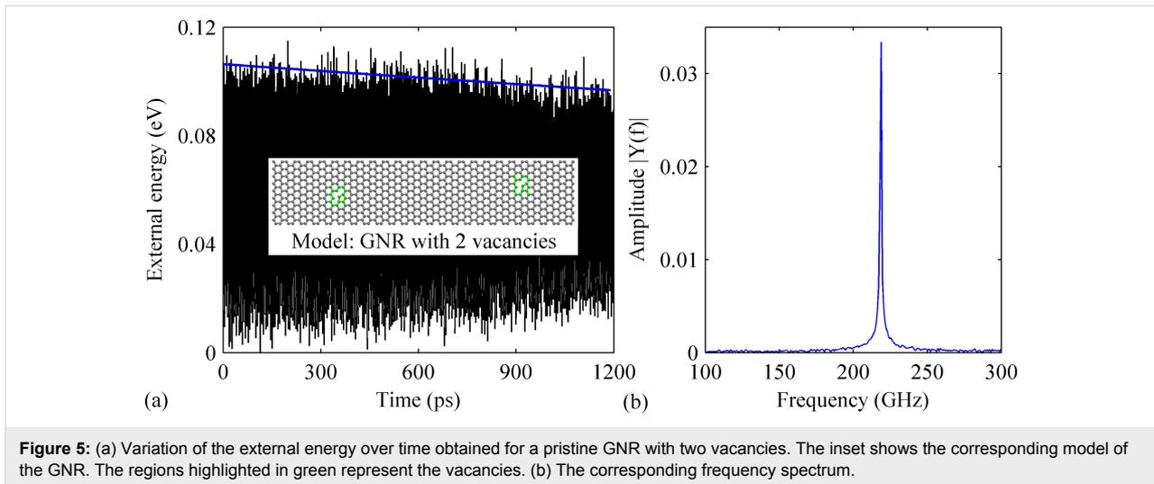
**Figure 5:** (a) Variation of the external energy over time obtained for a pristine GNR with two vacancies. The inset shows the corresponding model of the GNR. The regions highlighted in green represent the vacancies. (b) The corresponding frequency spectrum.
