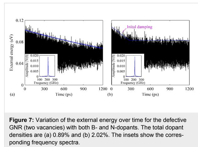
**Figure 7:** Variation of the external energy over time for the defective GNR (two vacancies) with both B- and N-dopants. The total dopant densities are (a) 0.89% and (b) 2.02%. The insets show the corresponding frequency spectra.
