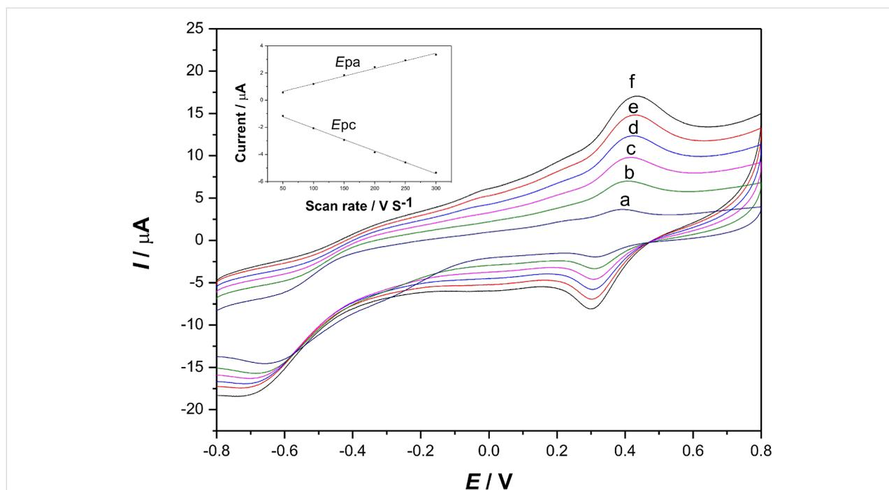
**Figure 4:** Cyclic voltammograms of the laccase–Nafion–ECNFs/GCE in acetate buffer (pH 4.0) with different scan rates ( $\text{V}\cdot\text{s}^{-1}$ ): (a) 0.05; (b) 0.1; (c) 0.15; (d) 0.2; (e) 0.25; (f) 0.3. Inset: Calibration plot of anodic and cathodic peak currents vs scan rates.
