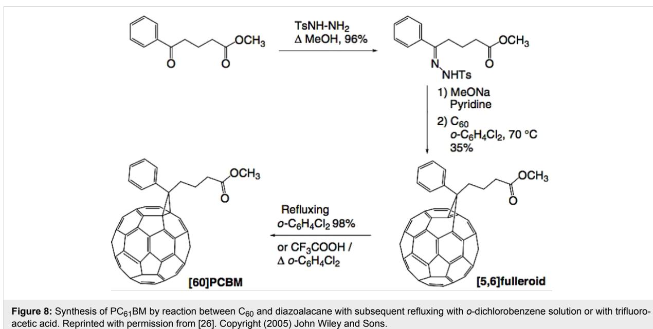
**Figure 8:** Synthesis of PC<sub>61</sub>BM by reaction between C<sub>60</sub> and diazoalane with subsequent refluxing with *o*-dichlorobenzene solution or with trifluoroacetic acid. Reprinted with permission from [26]. Copyright (2005) John Wiley and Sons.
