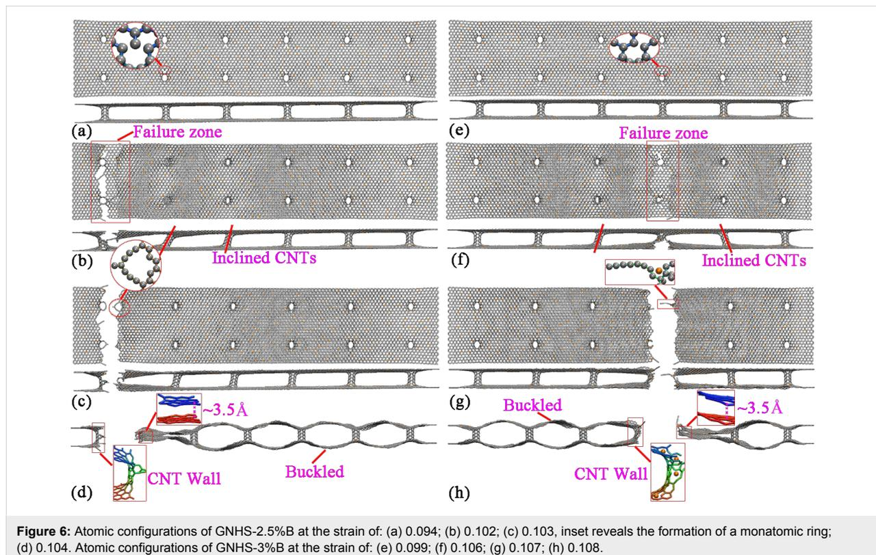
**Figure 6:** Atomic configurations of GNHS-2.5%B at the strain of: (a) 0.094; (b) 0.102; (c) 0.103, inset reveals the formation of a monatomic ring; (d) 0.104. Atomic configurations of GNHS-3%B at the strain of: (e) 0.099; (f) 0.106; (g) 0.107; (h) 0.108.
