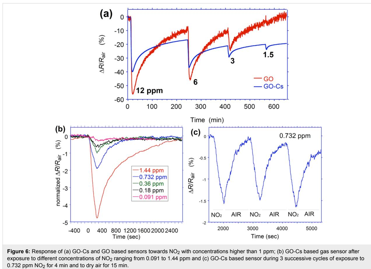
between the sensitivity and recovery time. This is in agreement with what observed by other researchers [25,46]. As shown in Figure 6c, the GO-Cs sensor exhibits a good repeatability, even if a slight drift in the baseline is observed. This may be due to the presence of gas molecules not yet desorbed from the sensor surface. An average time of 540 s is needed to recover after 240 s exposure to 0.732 ppm of NO<sub>2</sub>.
