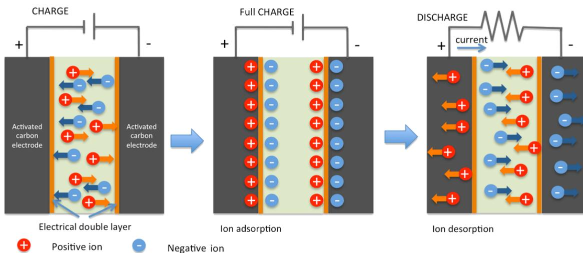
**Figure 50:** Charge and discharge processes of an EDLC.
