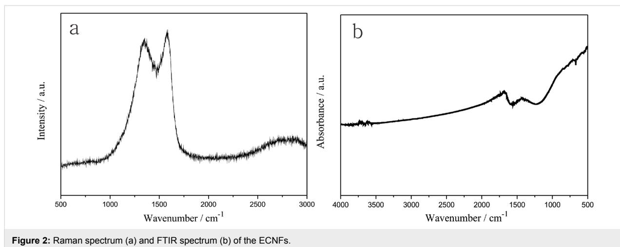
**Figure 2:** Raman spectrum (a) and FTIR spectrum (b) of the ECNFs.
