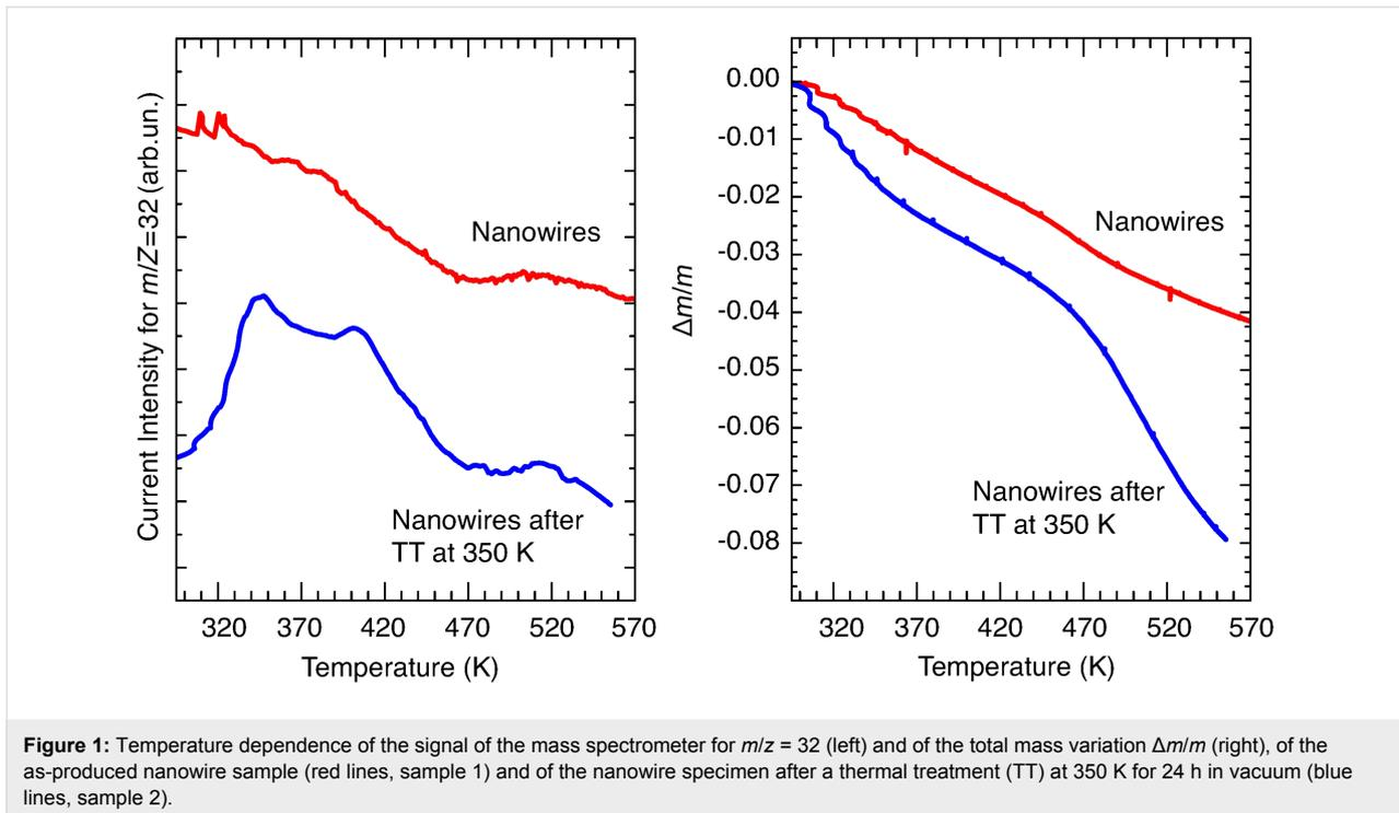
**Figure 1:** Temperature dependence of the signal of the mass spectrometer for  $m/z = 32$  (left) and of the total mass variation  $\Delta m/m$  (right), of the as-produced nanowire sample (red lines, sample 1) and of the nanowire specimen after a thermal treatment (TT) at 350 K for 24 h in vacuum (blue lines, sample 2).
