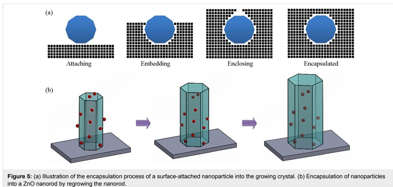
**Figure 5:** (a) Illustration of the encapsulation process of a surface-attached nanoparticle into the growing crystal. (b) Encapsulation of nanoparticles into a ZnO nanorod by regrowing the nanorod.
