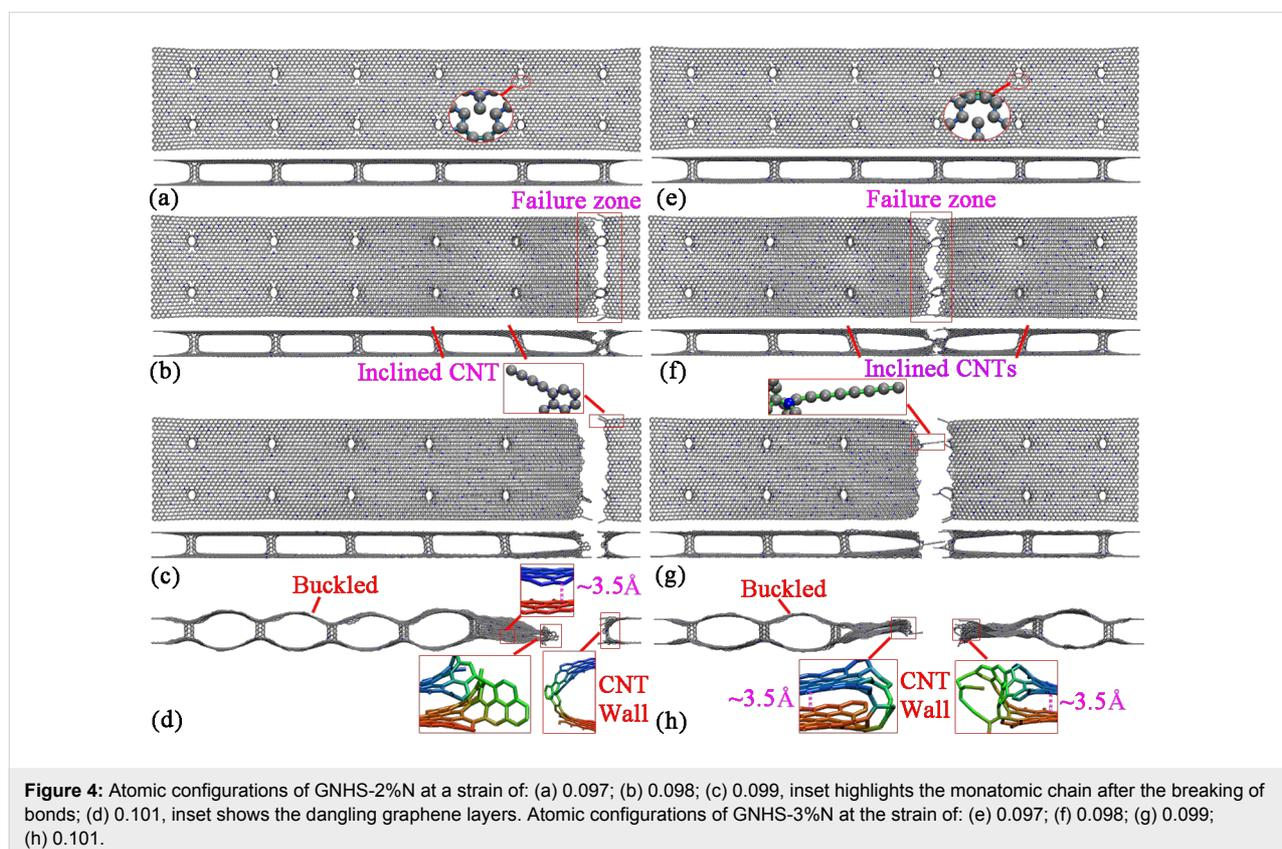
**Figure 4:** Atomic configurations of GNHS-2%N at a strain of: (a) 0.097; (b) 0.098; (c) 0.099, inset highlights the monatomic chain after the breaking of bonds; (d) 0.101, inset shows the dangling graphene layers. Atomic configurations of GNHS-3%N at the strain of: (e) 0.097; (f) 0.098; (g) 0.099; (h) 0.101.
