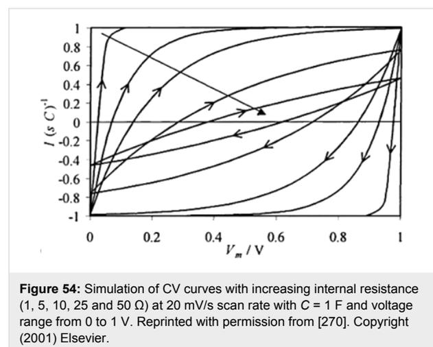
Figure 54: Simulation of CV curves with increasing internal resistance (1, 5, 10, 25 and 50  $\Omega$ ) at 20 mV/s scan rate with  $C = 1$  F and voltage range from 0 to 1 V. Reprinted with permission from [270]. Copyright (2001) Elsevier.
