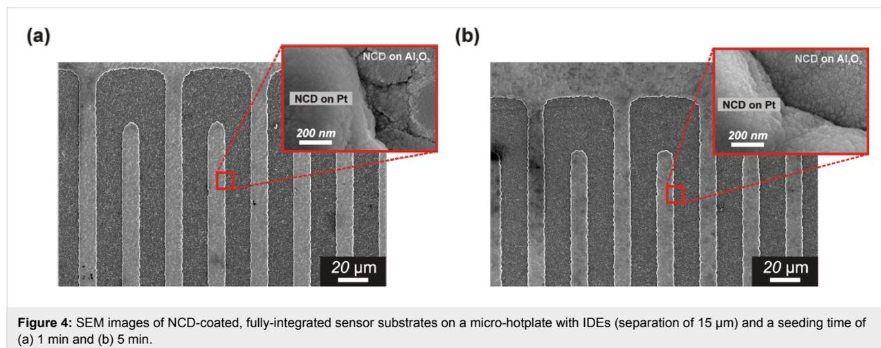
**Figure 4:** SEM images of NCD-coated, fully-integrated sensor substrates on a micro-hotplate with IDEs (separation of 15  $\mu\text{m}$ ) and a seeding time of (a) 1 min and (b) 5 min.
