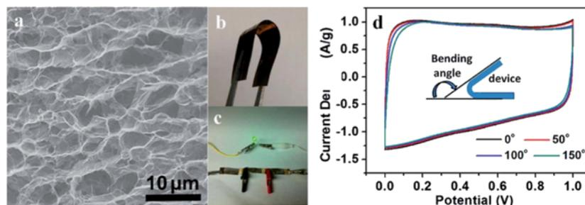
**Figure 65:** (a) SEM image of the interior microstructure of a graphene hydrogel. (b) Photograph of the flexible solid-state supercapacitor based on a graphene hydrogel film. (c) Photograph of a green LED powered by the three supercapacitors in series. (d) CV curves of the flexible solid-state device at 10 mV/s for different bending angles. Reprinted with permission from [296]. Copyright (2013) American Chemical Society.
