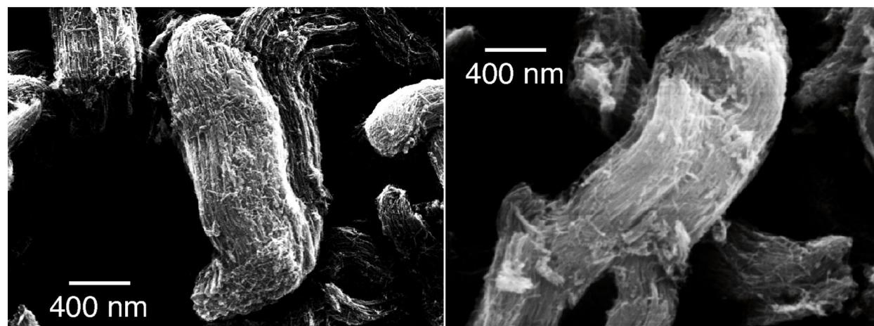
**Figure 3:** SEM images of the  $\text{Fe}_2\text{O}_3$  nanowires deposited on a Si surface before (left) and after (right) thermal treatment at 650 K.
