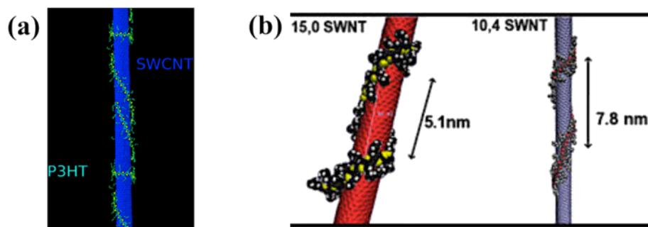
**Figure 39:** (a) Molecular dynamics simulations of P3HT wrapped around a SWNT (15,0). Reprinted with permission from [214]. Copyright (2010) American Chemical Society. (b) Helices form on (15,0) and (10,4) SWNTs during the folding of P3HT with orthogonal initialization. The chirality may affect the pitch distance to some extent. Reprinted with permission from [213]. Copyright (2010) American Chemical Society.
