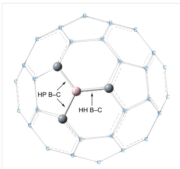
**Figure 1:** Sites for CO<sub>2</sub> adsorption on BC<sub>59</sub>. The B and C atoms of HH B–C and HP B–C sites are represented as 'ball and bond'-type and the rest of the atoms are represented as 'wireframes'. Atom colour code: grey, carbon; pink, boron.
