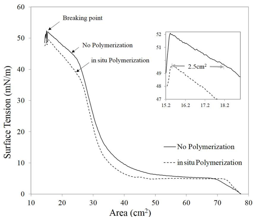
**Figure 2:** The surface tension–area isotherm of the PDA monolayer with and without in situ polarization in the trough. The inset shows that the in situ polymerization of the PDA film reduces the film surface area by 2.5 cm<sup>2</sup> (making it 15% more compact), which is close to the maximum confinement before the breaking point.
