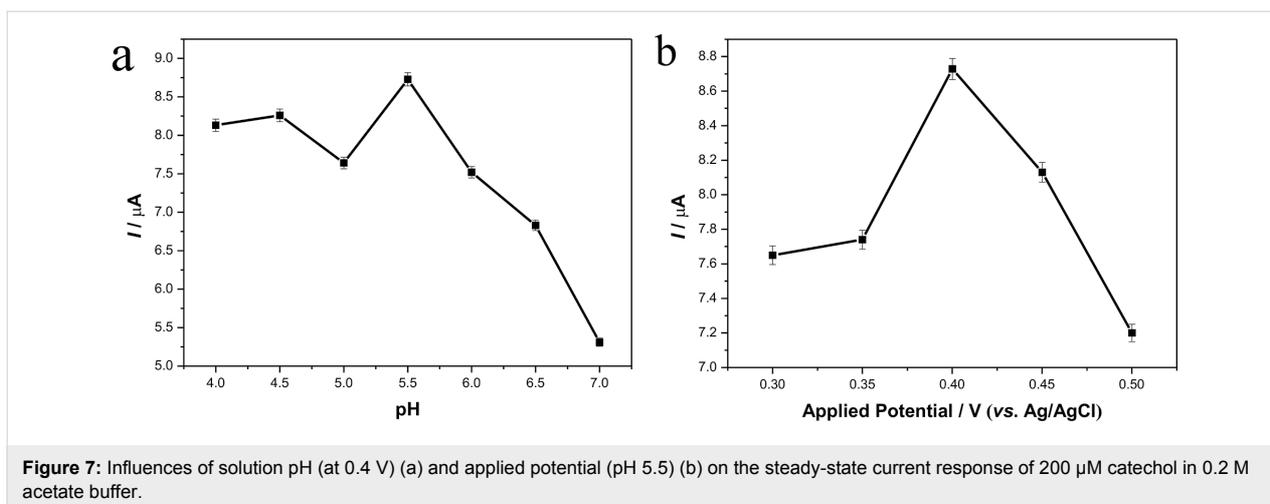
previous report [34]. Figure 7b presents the influences of different applied potentials on the amperometric responses. It can be clearly seen that the maximum current value came at 0.4 V. So the applied potential was set at 0.4 V in the following experiments.
