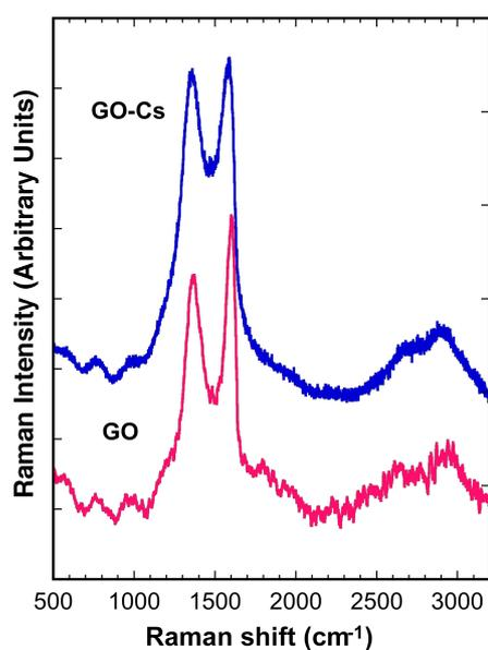
**Figure 4:** Raman spectra of GO-Cs and GO, displaying intense D and G peaks at  $\approx 1380$  and  $\approx 1600$   $\text{cm}^{-1}$ , respectively. The increase of the D peak, which is the signature of defects in graphene and GO, is clearly linked to the presence of Cs in GO-Cs.
