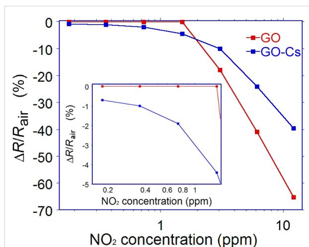
**Figure 5:** Response of the GO and GO-Cs based sensors as a function of NO<sub>2</sub> concentration. The inset shows the response at very low concentrations.
