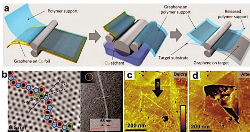
**Figure 22:** CVD graphene. (a) Schematic of the transfer of graphene produced on Cu using the roll-to-roll method. (b) Two types of graphene boundaries: aperiodic heptagon/pentagon pairs and overlapped bilayer regions. (c,d) Tears along the graphene grain boundaries after indentation. Reprinted with permission from [135]. Copyright (2014) American Chemical Society.
