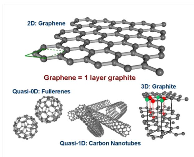
**Figure 12:** Honeycomb lattice of graphene. Graphene layers can be stacked into graphite or rolled up into carbon nanotubes. The formation of fullerenes requires the incorporation of five-membered rings. Reprinted with permission from [61]. Copyright (2008) John Wiley and Sons.
