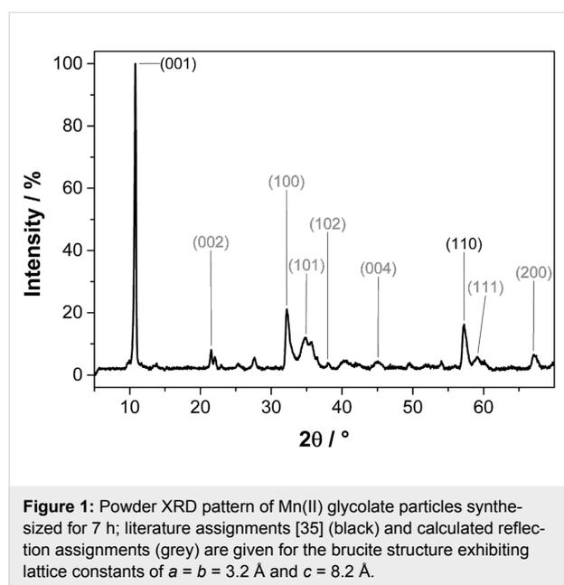
**Figure 1:** Powder XRD pattern of Mn(II) glycolate particles synthesized for 7 h; literature assignments [35] (black) and calculated reflection assignments (grey) are given for the brucite structure exhibiting lattice constants of  $a = b = 3.2$  Å and  $c = 8.2$  Å.
