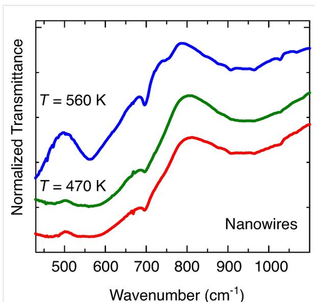
**Figure 2:** Infrared spectrum (normalized transmittance signal) of the nanowire sample (sample 2, red line), and of the specimen obtained from sample 2 after a thermal treatment at 470 K (sample 3, green line) and at 560 K (sample 4, blue line). In order to compare the transmission of different oxide powders, the transmittance spectra have been normalized. Data are vertically stacked, for the sake of clarity.
