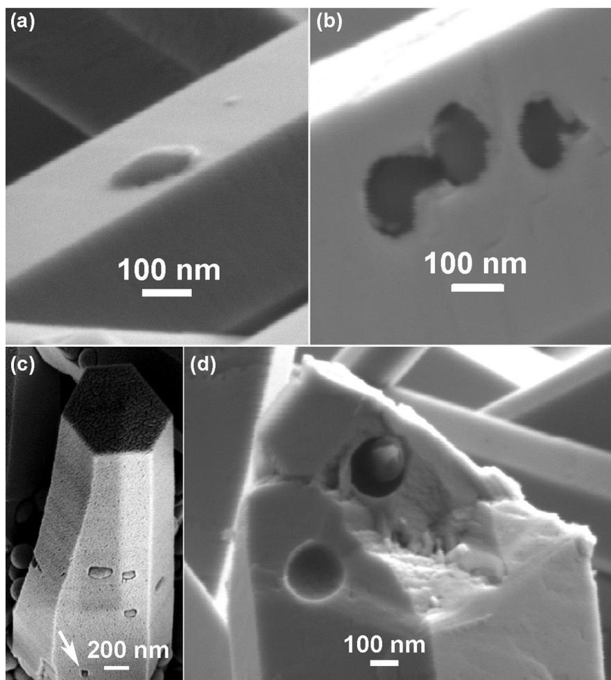
**Figure 4:** FE-SEM Images showing the encapsulation of nanobeads into ZnO nano/microrods after different regrowth processes. (a) Most part of the nanobead is embedded into a nanorod. (b) Nanobeads are deeper embedded into a nanorods, leaving holes in the surface. (c) A thick microrod showing that the embedded nanobeads are slightly exposed. (d) A fractured microrod showing a completely encapsulated nanobead inside.
