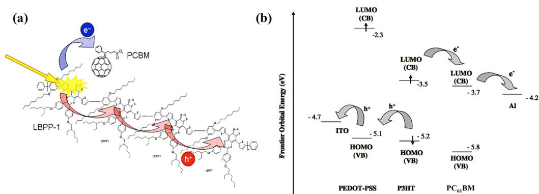
**Figure 33:** (a) Electron transfer from P3HT to PCBM after generation of the exciton at the interface of the two materials. (b) HOMO and LUMO levels of the different materials in an organic solar cell structure ITO/PEDOT-PSS/P3HT-PCBM/LiF/Al. Reprinted with permission from [26]. Copyright (2005) John Wiley and Sons.
