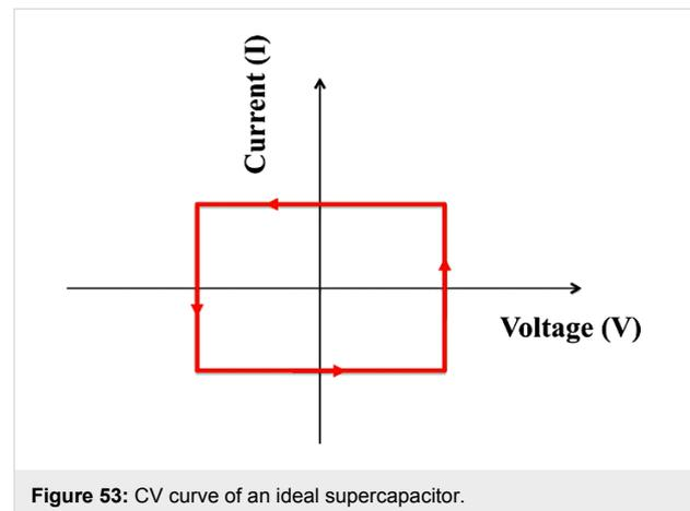
Figure 53: CV curve of an ideal supercapacitor.
