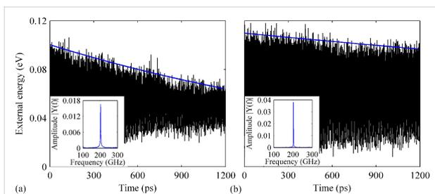
**Figure 6:** Variation of the external energy over time for a defective GNR (two vacancies) with B-dopant. The density of the dopant is (a) 1.64% and (b) 1.89%. The insets show the corresponding frequency spectra.
