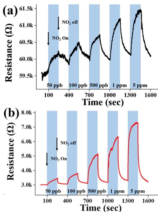
**Figure 3:** Electrical responses of the gas sensors fabricated from ZnSe nanowires to 50 ppb, 100 ppb, 500 ppb, 1 ppm and 5 ppm NO<sub>2</sub> gas at room temperature (a) in the dark and (b) under UV (365 nm) illumination at 1.2 mW/cm<sup>2</sup>.
