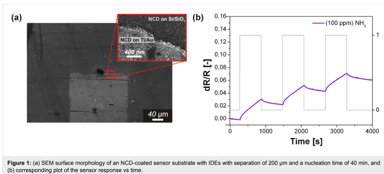
**Figure 1:** (a) SEM surface morphology of an NCD-coated sensor substrate with IDEs with separation of 200 μm and a nucleation time of 40 min, and (b) corresponding plot of the sensor response vs time.
