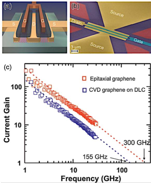
**Figure 30:** High frequency graphene transistor. (a) and (b) Structure of a graphene-based FET for an analogue radio frequency device. (c) Current gain as a function of frequency, showing a cut-off frequency of 300 GHz for epitaxial graphene on SiC. Reprinted with permission from [173]. Copyright (2012) MRS Bulletin.
