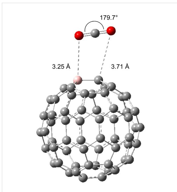
**Figure 2:** Configuration of physisorbed CO<sub>2</sub> on neutral BC<sub>59</sub>. Atom colour code: grey, carbon; pink, boron; red, oxygen.
