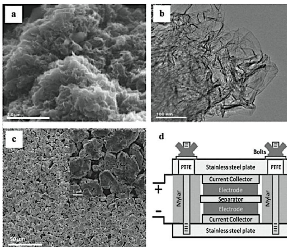
**Figure 61:** Graphene-based EDLCs utilizing chemically modified graphene as electrode materials. (a) Scanning electron microscopy (SEM) image of the material. (b) Transmission electron microscopy (TEM) image showing individual graphene sheets. (c) Low- and high- (inset) magnification SEM images of the electrode. (d) Schematic of test cell assembly. Reprinted with permission from [68]. Copyright (2008) American Chemical Society.
