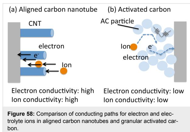
MWNTs were the first to be proposed as an electrode for an EDLC, showing a capacitance of  $\approx 100$  F/g, a low surface area of  $\approx 400$  m<sup>2</sup>/g and a low power density value of 8 kW/kg [282]. However, apart from their high volumetric capacitance values [283] obtained by optimizing the growth process, SWNTs are preferred because they exhibit a higher surface area and consequently better overall performance [284].
