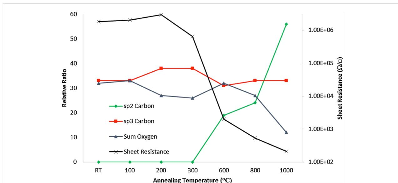
**Figure 21:** Plot of sheet resistance against annealing temperature with a comparison to key carbon and oxygen ratios. It should be noted that the sheet resistance has been plotted on a logarithmic scale. Reprinted with permission from [119]. Copyright (2015) Elsevier.
