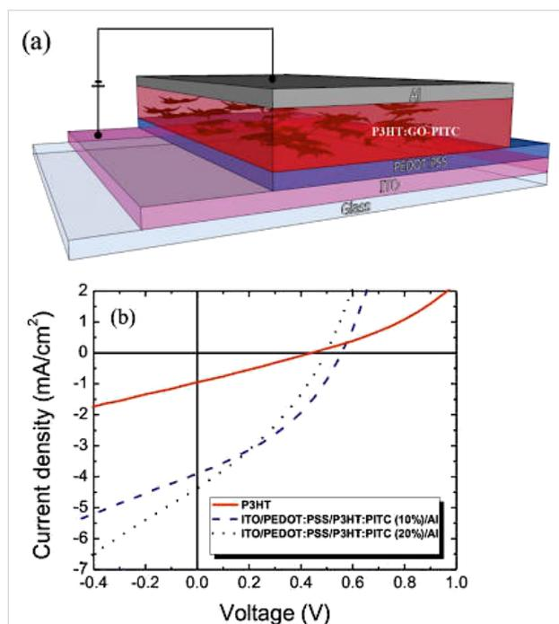
**Figure 42:** (a) Schematic of a photovoltaic device with a P3HT/GO-PITC thin film as the active layer and the structure ITO-PEDOT/PSS(30 nm)-P3HT/GO-PITC(110 nm)/Al(80 nm). (b) Experimental  $J$ - $V$  curves of the photovoltaic devices based on P3HT (red curve) and P3HT/GO-PITC composites (dashed curve, 10 wt %; dotted curve, 20 wt %) after post fabrication thermal annealing at 160 °C for 20 min. Reprinted with permission from [236]. Copyright (2012) American Chemical Society.
