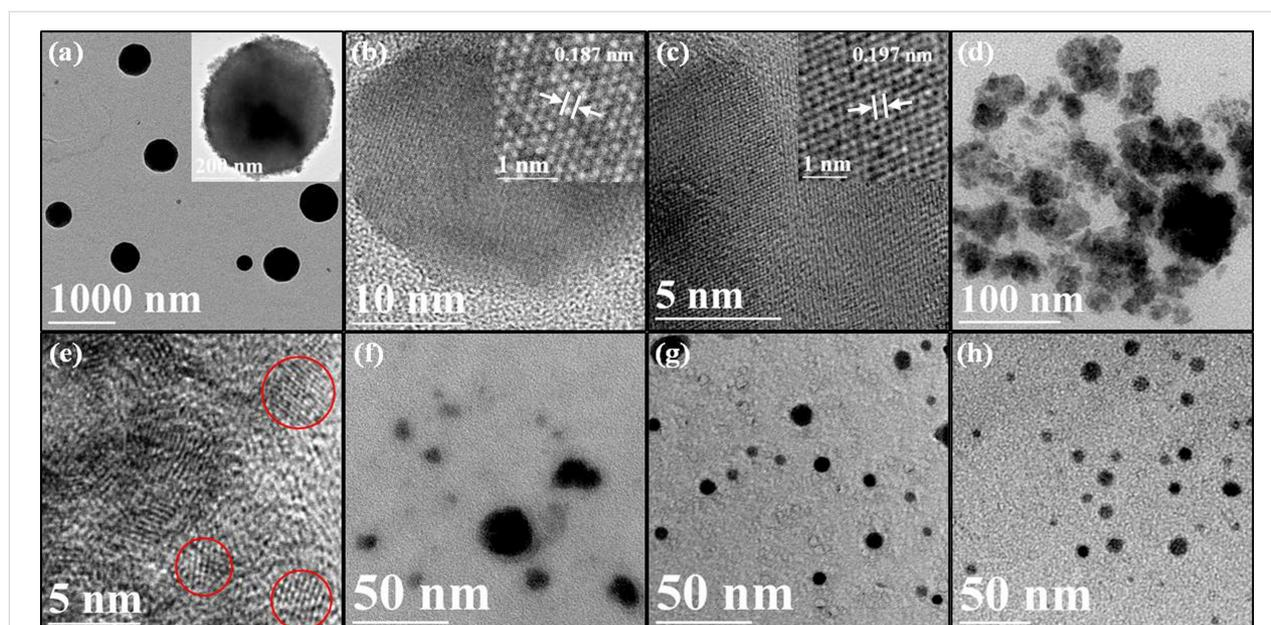
**Figure 6:** TEM images of (a, b, c)  $\text{Cu}_7\text{S}_4$  and  $\text{Cu}_{1.8}\text{S}$  nanocrystals collected prior to hydrothermal reaction and CZTS nanocrystals synthesized at different reaction duration: (d, e) 0.5 h, (f) 2 h, (g) 8 h, and (h) 24 h respectively.
