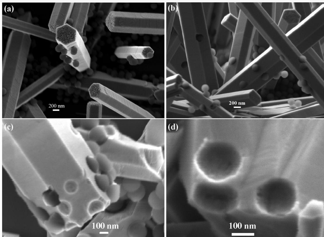
**Figure 3:** FE-SEM images showing the embedment of 200-nm-diameter polymer nanobeads in ZnO nanorods. (a) ZnO nanorods with polymer nanobeads attached to their surfaces. (b) Nanobeads were embedded in nanorods after a second growth process. These nanobeads were about half-volume exposed. (c) Intentionally fractured nanorods. (d) Close-view of the vacant sites where the nanobeads were broken off.
