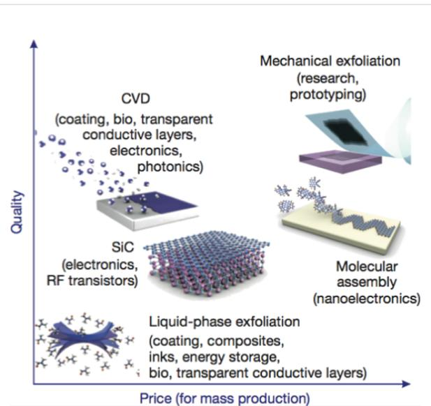
**Figure 14:** Several methods for the mass production of graphene that allow a wide choice in terms of size, quality and price for any particular application. Reprinted with permission from [81]. Copyright (2012) Nature Publishing Group.
