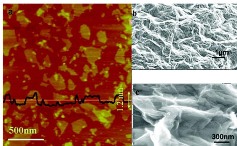
**Figure 62:** Morphology of graphene oxide and graphene-based materials. (a) Tapping-mode AFM image of graphene oxide and height profile plot. (b) and (c) SEM images at lower and higher magnification respectively of the graphene oxide reduced by a gas–solid reduction process. Reprinted with permission from [291]. Copyright (2009) American Chemical Society.
