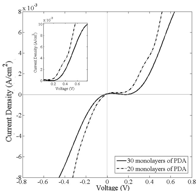
**Figure 8:** Current density–voltage characteristics for Ni–20 and 30 PDA monolayers–Ni junctions.
