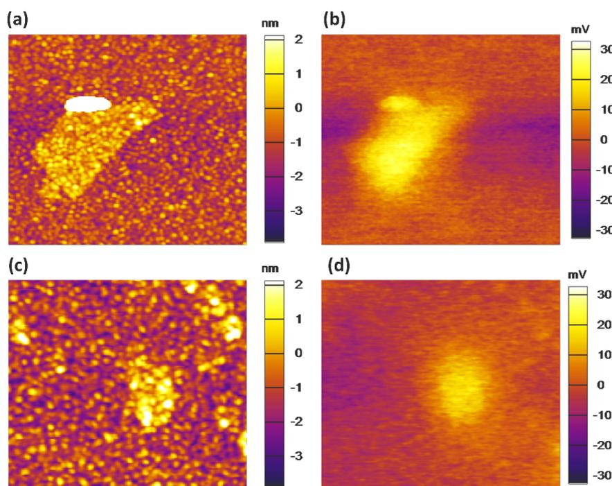
**Figure 2:** AFM and KPFM images of (a) and (b) a GO flake ( $2 \times 2 \mu\text{m}$ ); (c) and (d) a GO-Cs flake ( $1.4 \times 1.4 \mu\text{m}$ ).
