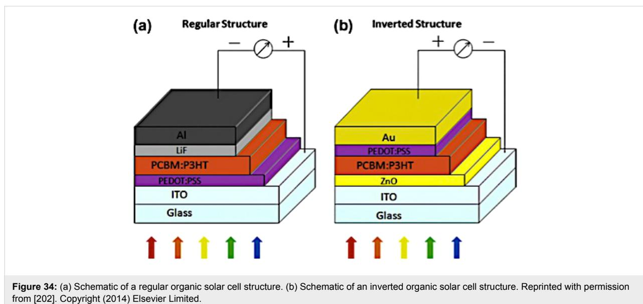
Figure 34: (a) Schematic of a regular organic solar cell structure. (b) Schematic of an inverted organic solar cell structure. Reprinted with permission from [202]. Copyright (2014) Elsevier Limited.
