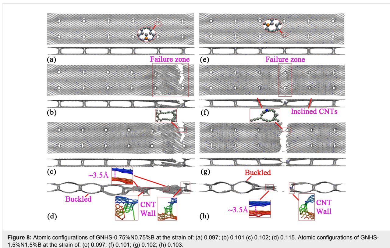
**Figure 8:** Atomic configurations of GNHS-0.75%N0.75%B at the strain of: (a) 0.097; (b) 0.101 (c) 0.102; (d) 0.115. Atomic configurations of GNHS-1.5%N1.5%B at the strain of: (e) 0.097; (f) 0.101; (g) 0.102; (h) 0.103.
