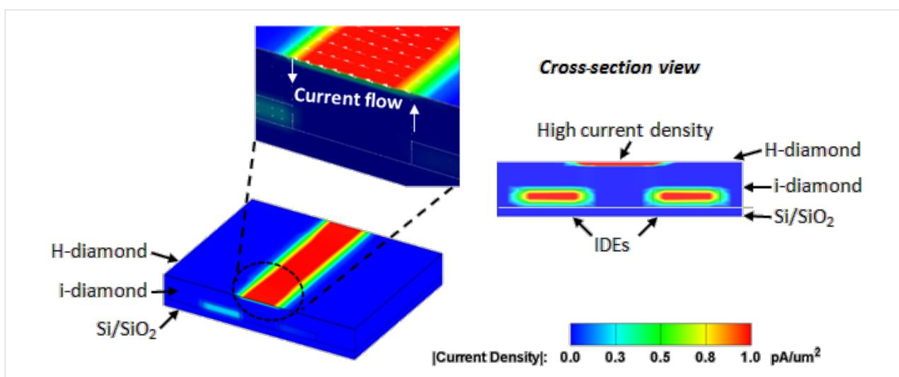
**Figure 7:** Current density profile for a single pair of IDEs covered by intrinsic diamond with a hydrogenated surface.
