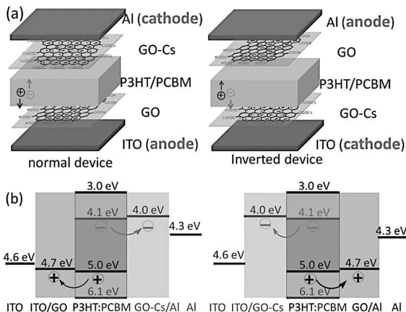
**Figure 44:** Device structures (a) and energy level diagrams (b) of the normal device and the inverted device with GO as the hole-extraction layer and GO/Cs as the electron-extraction layer. Reprinted with permission from [238]. Copyright (2012) John Wiley and Sons.
