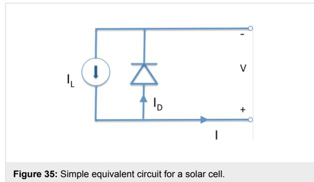
Figure 35: Simple equivalent circuit for a solar cell.
