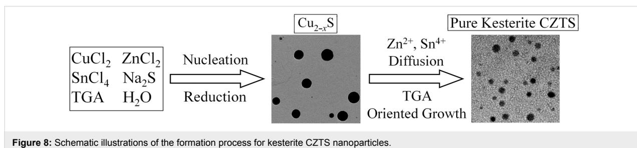
**Figure 8:** Schematic illustrations of the formation process for kesterite CZTS nanoparticles.
