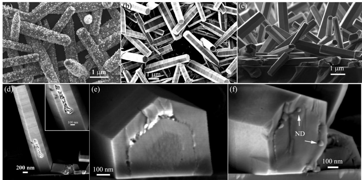
**Figure 2:** FE-SEM images showing the encapsulation of 40-nm-diameter NDs into ZnO nanorods. (a) ZnO nanorods covered with NDs. (b and c) Top- and side-view images of the nanorods after a second growth process, showing the complete encapsulation of NDs into the nanorods. (d) A nanorod shows the incomplete encapsulation of agglomerated NDs. (e and f) Cross-section images of fractured nanorods containing NDs, showing NDs inside the crystal.
