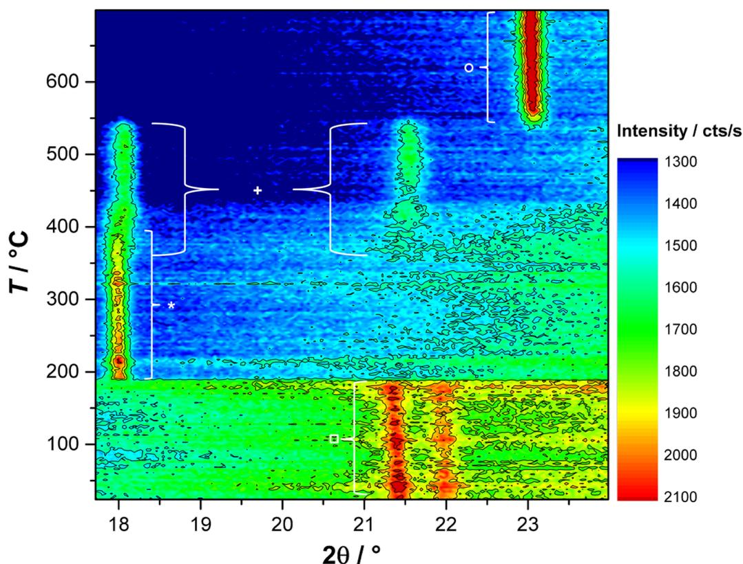
**Figure 3:** In situ XRD patterns recorded in a pure  $\text{O}_2$  flow while heating the  $\text{Mn(II)}$  glycolate precursor to  $700^\circ\text{C}$  at  $2\text{ K/min}$ ; reflexes denoted are:  $\text{Mn(II)}$  glycolate ( $\square$ ),  $\text{Mn}_3\text{O}_4$  (\*),  $\text{Mn}_5\text{O}_8$  (+) and  $\alpha\text{-Mn}_2\text{O}_3$  ( $\circ$ ).
