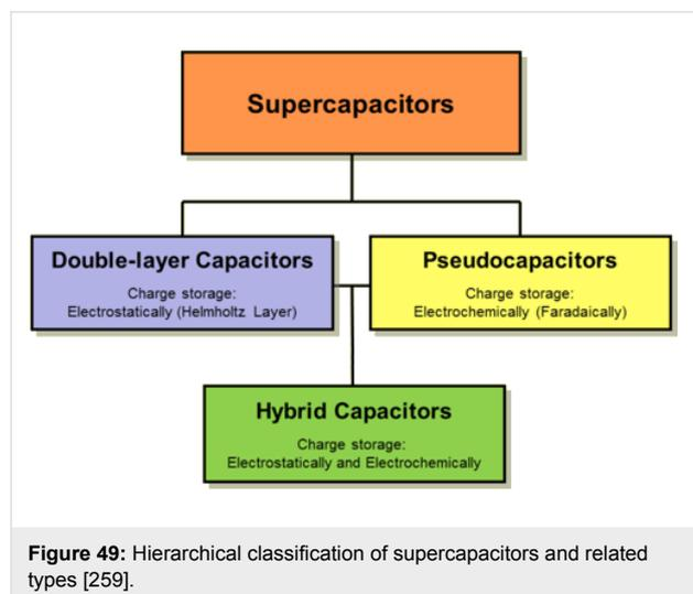
**Figure 49:** Hierarchical classification of supercapacitors and related types [259].
