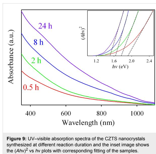
**Figure 9:** UV–visible absorption spectra of the CZTS nanocrystals synthesized at different reaction duration and the inset image shows the  $(Ah\nu)^2$  vs  $h\nu$  plots with corresponding fitting of the samples.
