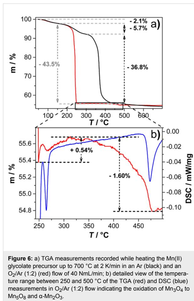
**Figure 6:** a) TGA measurements recorded while heating the Mn(II) glycolate precursor up to 700 °C at 2 K/min in an Ar (black) and an  $\text{O}_2/\text{Ar}$  (1:2) (red) flow of 40 NmL/min; b) detailed view of the temperature range between 250 and 500 °C of the TGA (red) and DSC (blue) measurements in  $\text{O}_2/\text{Ar}$  (1:2) flow indicating the oxidation of  $\text{Mn}_3\text{O}_4$  to  $\text{Mn}_5\text{O}_8$  and  $\alpha$ - $\text{Mn}_2\text{O}_3$ .
