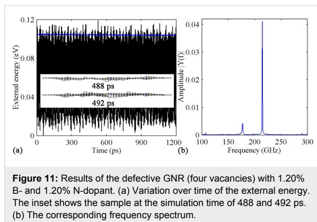
**Figure 11:** Results of the defective GNR (four vacancies) with 1.20% B- and 1.20% N-dopant. (a) Variation over time of the external energy. The inset shows the sample at the simulation time of 488 and 492 ps. (b) The corresponding frequency spectrum.
