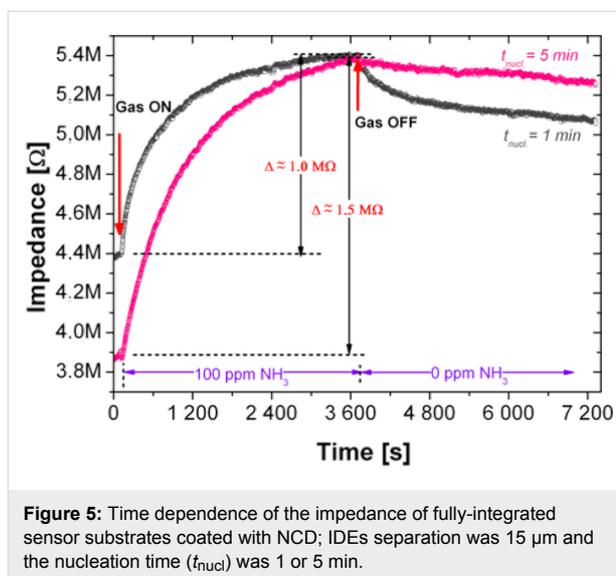
**Figure 5:** Time dependence of the impedance of fully-integrated sensor substrates coated with NCD; IDEs separation was 15  $\mu\text{m}$  and the nucleation time ( $t_{\text{nuc}}$ ) was 1 or 5 min.
