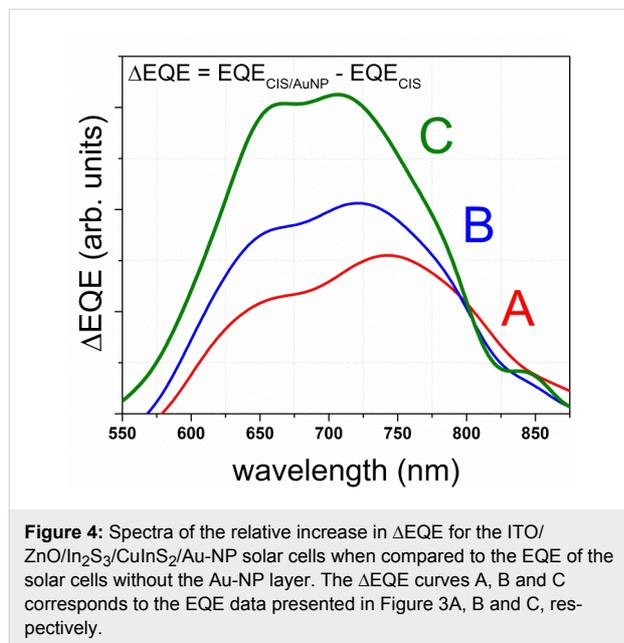
Thus, the increase in the EQE in the red/infrared region (Figure 3) is likely due to the gain in optical absorbance induced by the surface plasmon resonance effect. For this effect to occur, the scattering medium must have a lower refractive index than that of the absorbing medium. As required, the refractive index of Au is in the range 1.5–0.2 [18] and that of CuInS<sub>2</sub> is 3–2.6 [19] in the wavelength range of 400–900 nm.
