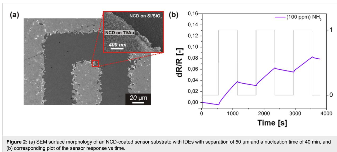
**Figure 2:** (a) SEM surface morphology of an NCD-coated sensor substrate with IDEs with separation of 50 μm and a nucleation time of 40 min, and (b) corresponding plot of the sensor response vs time.
