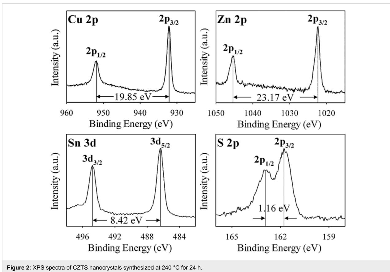
**Figure 2:** XPS spectra of CZTS nanocrystals synthesized at 240 °C for 24 h.
