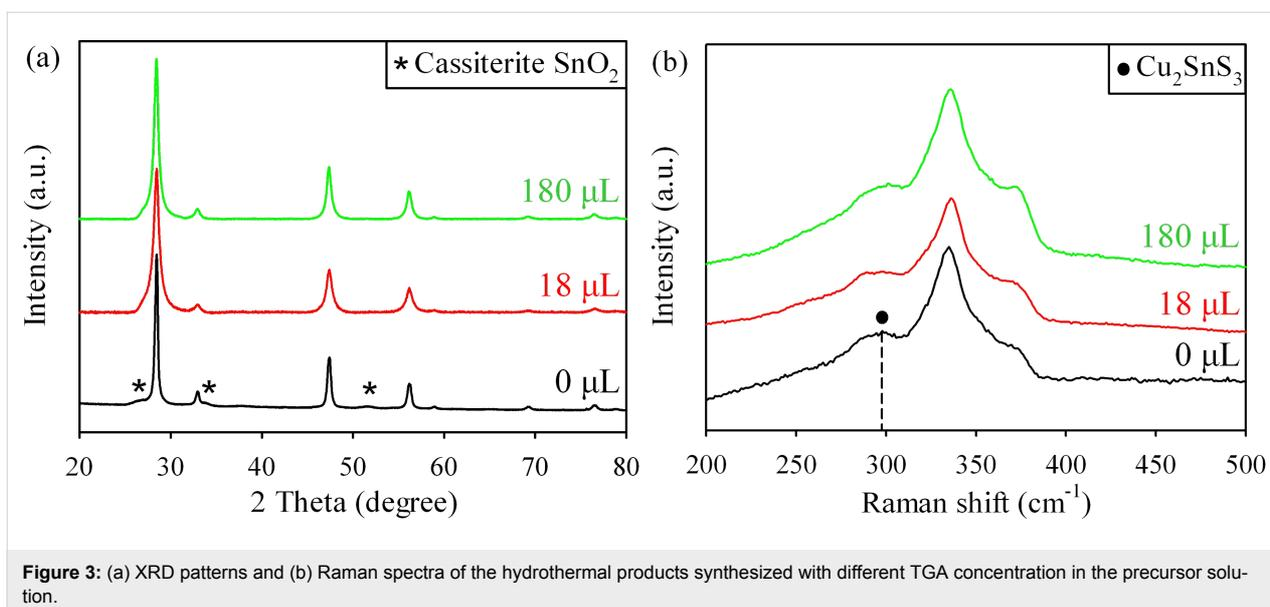
**Figure 3:** (a) XRD patterns and (b) Raman spectra of the hydrothermal products synthesized with different TGA concentration in the precursor solution.
