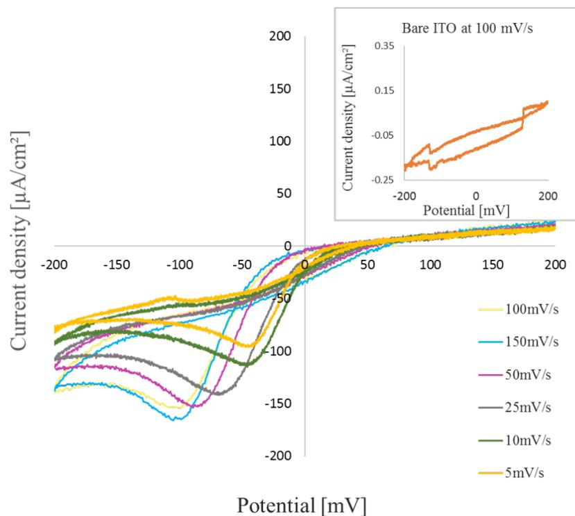
**Figure 4:** Cyclic voltammetry results with varying scan rates for a 20 monolayer PDA sample in 0.01 M HCl electrolyte. The inset shows the current density vs potential measurements for a bare ITO sample in the same measurement setup.
