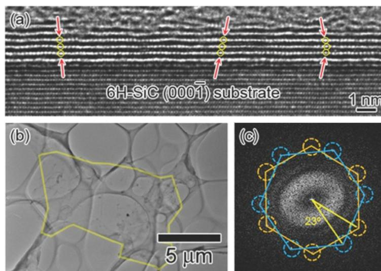
**Figure 29:** TEM images of MLG on the C-face. (a) A cross-sectional TEM image. (b) A low-magnification TEM image of graphene exfoliated from the SiC substrate. (c) FFT pattern from the area highlighted in (b). Reprinted with permission from [171]. Copyright (2012) Surface Science Society of Japan.
