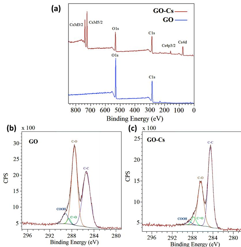
**Figure 3:** (a) XPS survey spectrum of GO (blue line) and GO-Cs (red line); High resolution XPS C1s spectra of (b) GO and (c) GO-Cs. The  $\approx 1$  eV shift towards lower binding energy of the peaks in (c) is due to the shift of the Fermi level caused by the doping.
