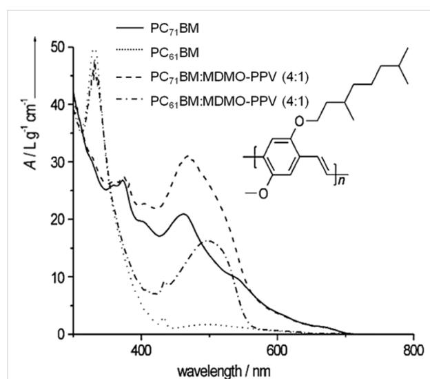
**Figure 38:** UV-vis spectra of  $PC_{71}BM$  and  $PC_{61}BM$ , both in toluene. To illustrate the contribution of MDMO-PPV to the absorption, the (normalized) spectra of  $PC_{71}BM$ /MDMO-PPV and  $PC_{61}BM$ /MDMO-PPV, also in toluene, are presented. The inset shows the structure of poly(2-methoxy-5-[3',7'-dimethyloctyloxy]-p-phenylene vinylene) (MDMO-PPV). Reprinted with permission from [207]. Copyright (2015) John Wiley and Sons.
