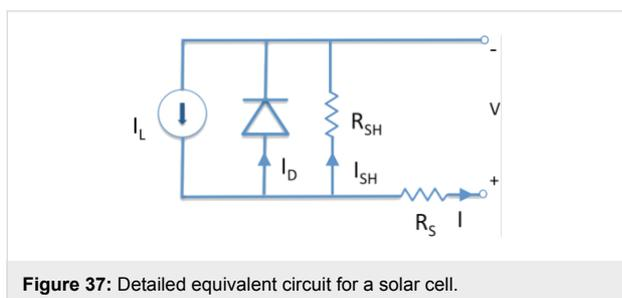
**Figure 37:** Detailed equivalent circuit for a solar cell.
