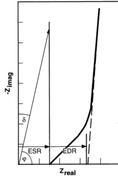
**Figure 56:** Schematic representation of the Nyquist impedance plot of an ideal capacitor (vertical thin line) and a supercapacitor with porous electrodes (thick line). Reprinted with permission from [266]. Copyright (2000) Elsevier.
