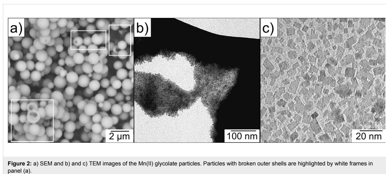
**Figure 2:** a) SEM and b) and c) TEM images of the Mn(II) glycolate particles. Particles with broken outer shells are highlighted by white frames in panel (a).
