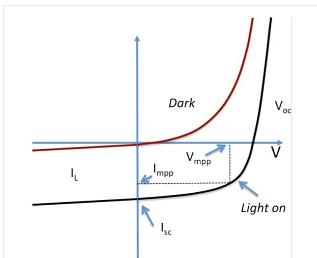
**Figure 36:**  $I$ - $V$  curves of a solar cell.  $I_L$  indicates the current under illumination.  $V_{oc}$  and  $I_{sc}$  represent the open circuit voltage and the short circuit current, respectively, while  $V_{mp}$  and  $I_{mp}$  indicate the maximum power point.
