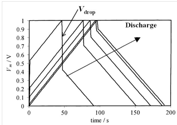
**Figure 55:** Simulation of the charge/discharge curves with increasing internal resistance (0, 1, 5, 10 and 25  $\Omega$ ) at  $I = 10$  mA. The smallest  $V_{\text{drop}}$  can be achieved with the smallest internal resistance. The longest total charging time is also achieved with the smallest internal resistance. Reprinted with permission from [270]. Copyright (2001) Elsevier.
