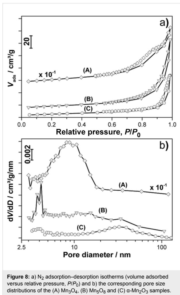
**Figure 8:** a)  $\text{N}_2$  adsorption–desorption isotherms (volume adsorbed versus relative pressure,  $P/P_0$ ) and b) the corresponding pore size distributions of the (A)  $\text{Mn}_3\text{O}_4$ , (B)  $\text{Mn}_5\text{O}_8$  and (C)  $\alpha\text{-Mn}_2\text{O}_3$  samples.
