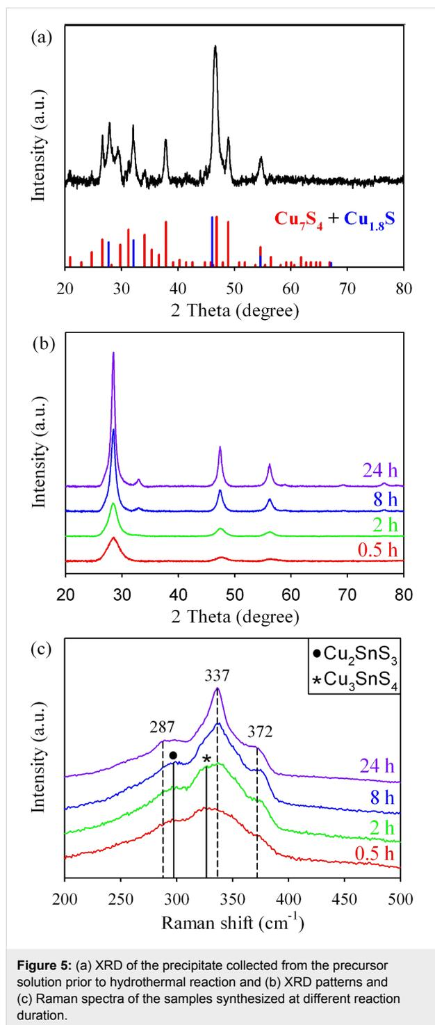
**Figure 5:** (a) XRD of the precipitate collected from the precursor solution prior to hydrothermal reaction and (b) XRD patterns and (c) Raman spectra of the samples synthesized at different reaction duration.
