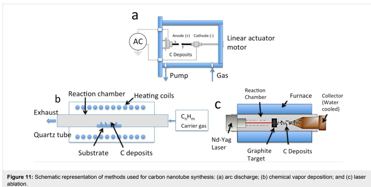
**Figure 11:** Schematic representation of methods used for carbon nanotube synthesis: (a) arc discharge; (b) chemical vapor deposition; and (c) laser ablation.
