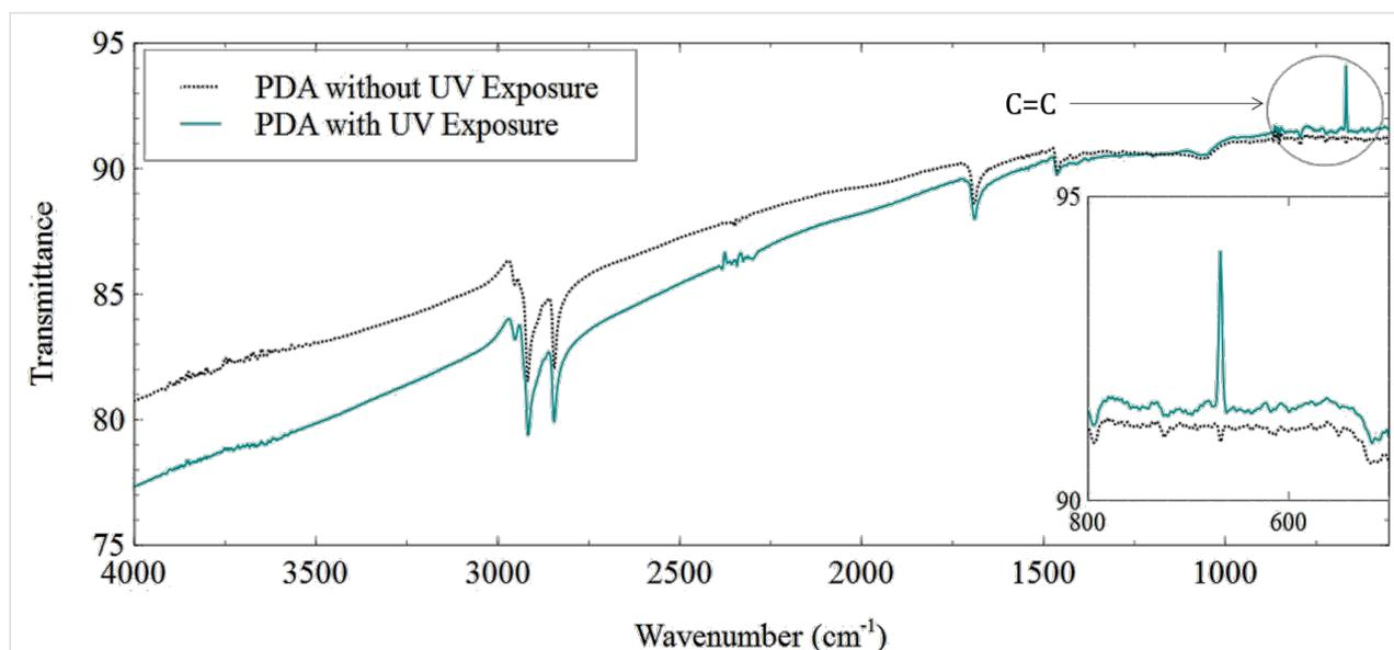
**Figure 3:** Infrared spectrum of a 20 monolayer PDA sample with and without UV exposure. The inset shows a magnified view of the C=C bending vibrations around 650–750 cm<sup>-1</sup>.
