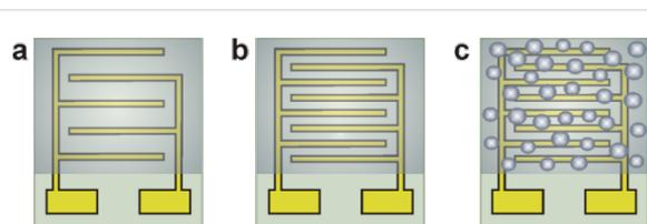
**Figure 8:** Schematic drawing of the sensor assemblies with diamond coatings: (a) continuous NCD film on IDEs with  $200\text{ }\mu\text{m}$  electrode separation, (b) continuous NCD film on IDEs with  $50\text{ }\mu\text{m}$  electrode separation, and (c) porous-like NCD film on IDEs with  $50\text{ }\mu\text{m}$  electrode separation.
