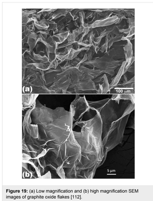
**Figure 19:** (a) Low magnification and (b) high magnification SEM images of graphite oxide flakes [112].
