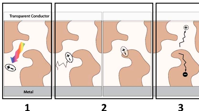
**Figure 32:** Photocurrent generation steps in an organic solar cell. Step 1: photon absorption in the conducting polymer (donor material). Step 2: creation of an exciton. Step 3: exciton separation at the interface of the heterojunction (interface between the donor and the acceptor).
