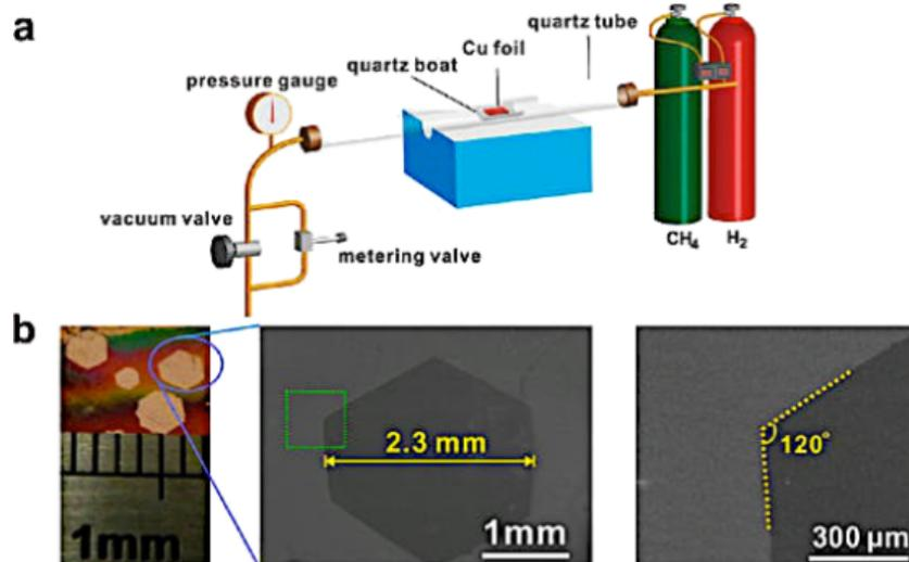
**Figure 23:** Millimeter-sized graphene grains produced on polished and annealed Cu foils. (a) Schematic of the controlled pressure CVD system. (b) Typical optical and scanning electron microscope (SEM) images of as-produced millimeter-sized graphene grains on pretreated Cu foils. Reprinted with permission from [135]. Copyright (2014) American Chemical Society.
