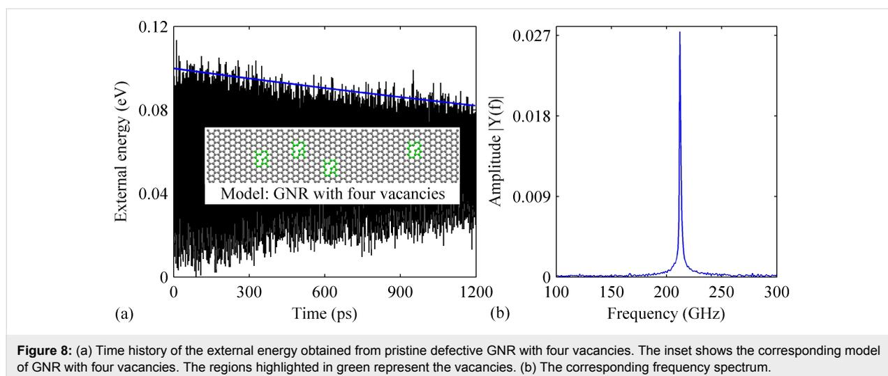
**Figure 8:** (a) Time history of the external energy obtained from pristine defective GNR with four vacancies. The inset shows the corresponding model of GNR with four vacancies. The regions highlighted in green represent the vacancies. (b) The corresponding frequency spectrum.
