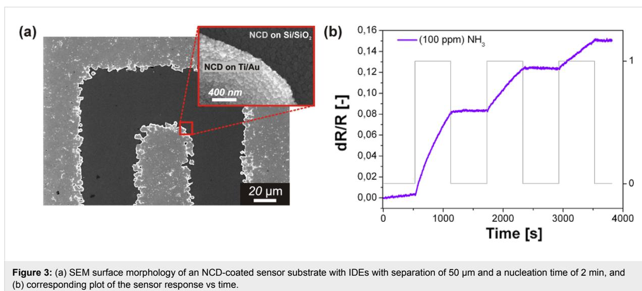
**Figure 3:** (a) SEM surface morphology of an NCD-coated sensor substrate with IDEs with separation of 50 μm and a nucleation time of 2 min, and (b) corresponding plot of the sensor response vs time.
