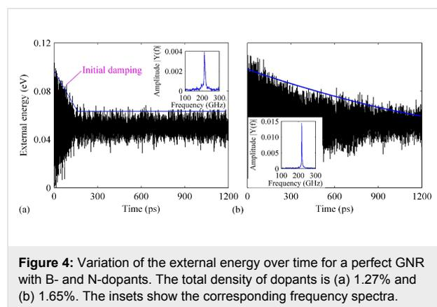
**Figure 4:** Variation of the external energy over time for a perfect GNR with B- and N-dopants. The total density of dopants is (a) 1.27% and (b) 1.65%. The insets show the corresponding frequency spectra.
