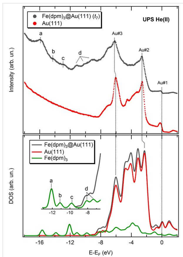
**Figure 2:** (Top panel) UPS spectra relative to the  $\text{Fe}(\text{dpm})_3$  saturation coverage (grey curve) and the clean substrate (red curve). (Bottom panel) Theoretical density of states for the system  $\text{Fe}(\text{dpm})_3@Au(111)$  (grey curve) and decomposition into Au and  $\text{Fe}(\text{dpm})_3$  contributions.
