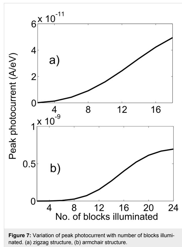
It should be mentioned here that without excitation light, the bias current through the device is in the range of  $10^{-5}$  A/eV and with light the photocurrent is in the range of  $10^{-11}$  A/eV. Thus, some kind of differential measurement is needed to detect the current in the leads. Alternatively, a high-pass frequency filter can be used at the output of the device for the detection in the variation of light.
