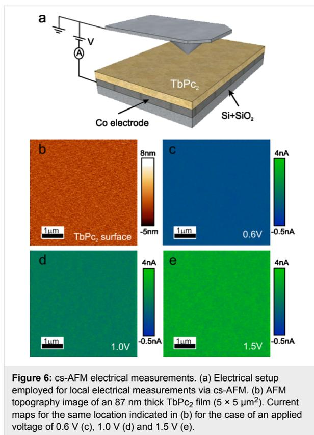
**Figure 6:** cs-AFM electrical measurements. (a) Electrical setup employed for local electrical measurements via cs-AFM. (b) AFM topography image of an 87 nm thick TbPc<sub>2</sub> film (5 × 5 μm<sup>2</sup>). Current maps for the same location indicated in (b) for the case of an applied voltage of 0.6 V (c), 1.0 V (d) and 1.5 V (e).
