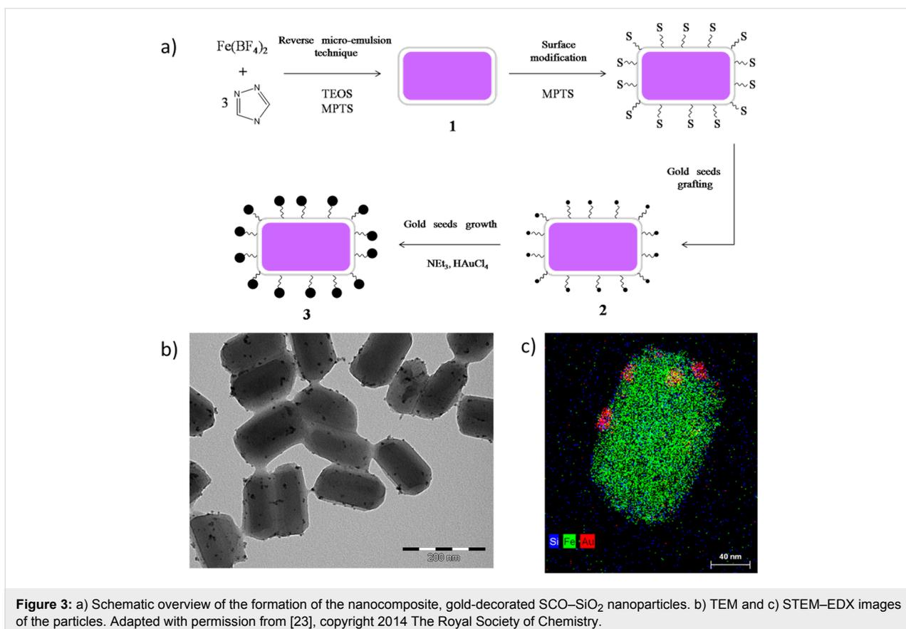
**Figure 3:** a) Schematic overview of the formation of the nanocomposite, gold-decorated SCO-SiO<sub>2</sub> nanoparticles. b) TEM and c) STEM-EDX images of the particles. Adapted with permission from [23], copyright 2014 The Royal Society of Chemistry.
