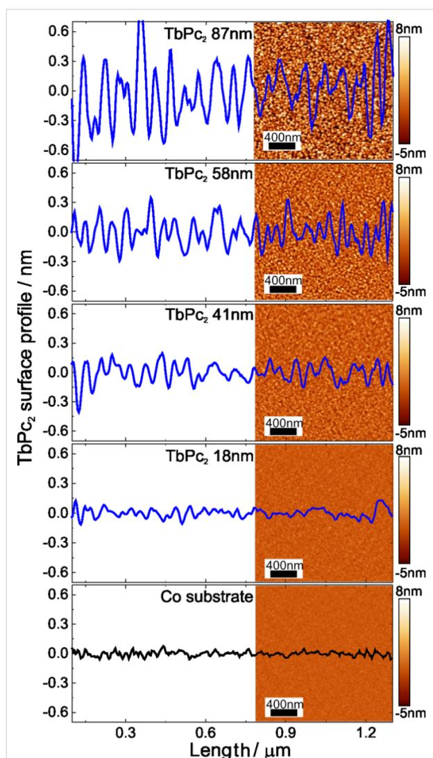
**Figure 4:** AFM topography characteristics of TbPc<sub>2</sub> thin films. Line scan profiles and AFM surface images for TbPc<sub>2</sub> films of 18, 41, 58 and 87 nm deposited on a 25 nm thick Co film.
