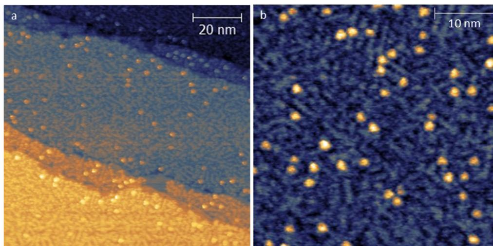
**Figure 6:** STM images for saturation coverage of  $\text{Fe}(\text{dpm})_3$  on  $\text{Au}(111)$  at  $T = 30$  K. (a)  $t_6 = 10$  min (HR); size =  $100 \times 100 \text{ nm}^2$ , bias =  $1.5$  V (filled states),  $I = 10$  pA. (b)  $t_7 = 1$  min (HR); size =  $45 \times 45 \text{ nm}^2$ , bias =  $1.5$  V (filled states),  $I = 10$  pA.
