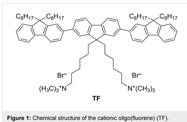
Figure 1: Chemical structure of the cationic oligo(fluorene) (TF).
