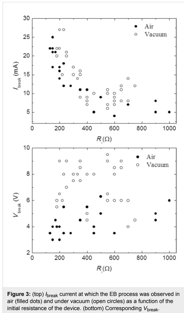
**Figure 3:** (top)  $I_{\text{break}}$  current at which the EB process was observed in air (filled dots) and under vacuum (open circles) as a function of the initial resistance of the device. (bottom) Corresponding  $V_{\text{break}}$ .
