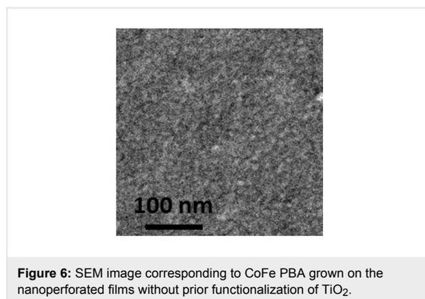
**Figure 6:** SEM image corresponding to CoFe PBA grown on the nanoporated films without prior functionalization of TiO<sub>2</sub>.
