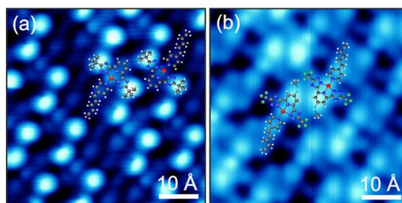
**Figure 6:** STM images of self-assembled monolayers of **C3** (a) and **C4** (b). Due to the rotational degree of freedom around the O–C bonds, the exact position of the methoxy group cannot be given here. Despite the different substituents  $\text{R}^1$  and  $\text{R}^2$  the complexes show similar packing structures indicated by the overlaid molecular models.
