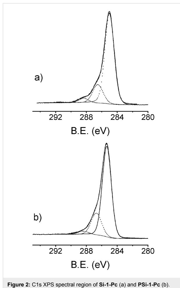
**Figure 2:** C 1s XPS spectral region of **Si-1-Pc** (a) and **PSi-1-Pc** (b).
