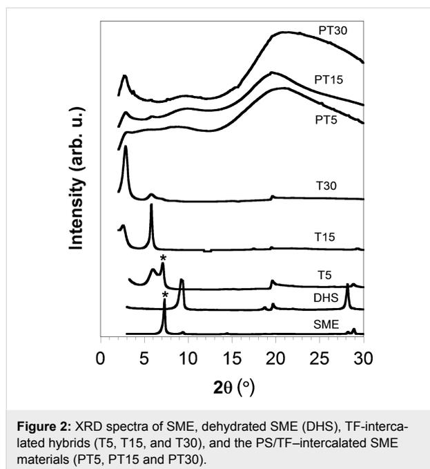
**Figure 2:** XRD spectra of SME, dehydrated SME (DHS), TF-intercalated hybrids (T5, T15, and T30), and the PS/TF-intercalated SME materials (PT5, PT15 and PT30).
