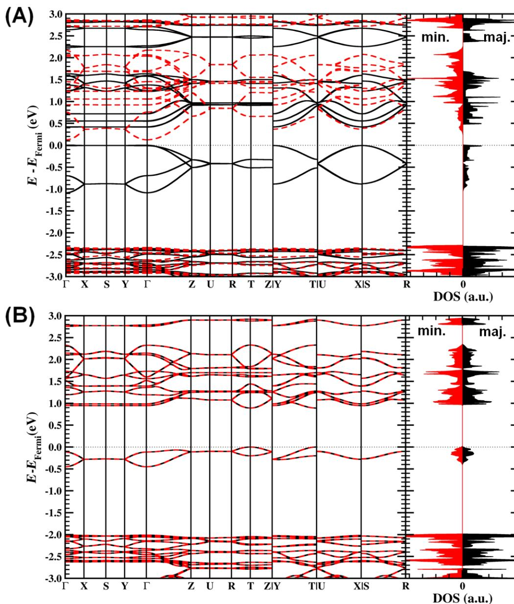
**Figure 4:** Band structure and density of states (DOS) near the Fermi level for the FM (A) and AF3 (B) spin configurations. Solid black/dashed red curves indicate the bands for the majority/minority spin components, respectively.
