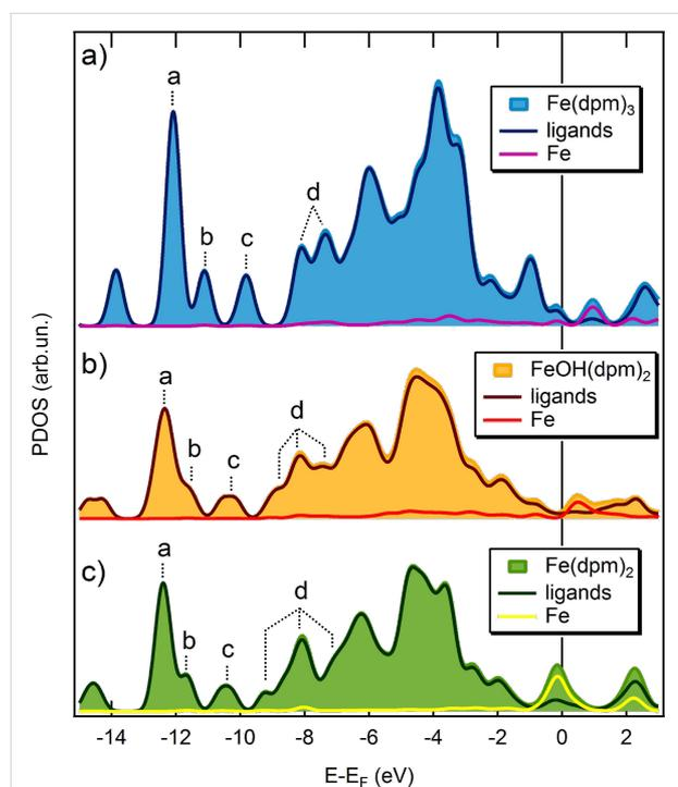
**Figure 3:** Projected DOS of the molecules in  $\text{Fe}(\text{dpm})_3@Au(111)$  (a),  $\text{FeOH}(\text{dpm})_2@Au(111)$  (b), and  $\text{Fe}(\text{dpm})_2@Au(111)$  (c), in which further separation of PDOS coming from the Fe ion and the ligands is presented.
