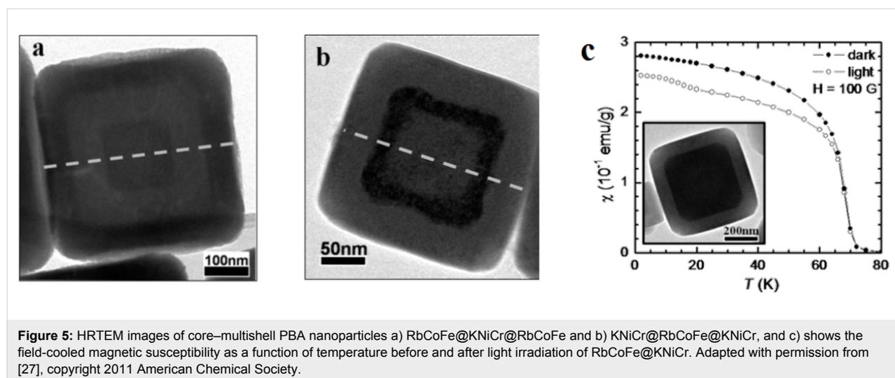
**Figure 5:** HRTEM images of core–multishell PBA nanoparticles a) RbCoFe@KNiCr@RbCoFe and b) KNiCr@RbCoFe@KNiCr, and c) shows the field-cooled magnetic susceptibility as a function of temperature before and after light irradiation of RbCoFe@KNiCr. Adapted with permission from [27], copyright 2011 American Chemical Society.
