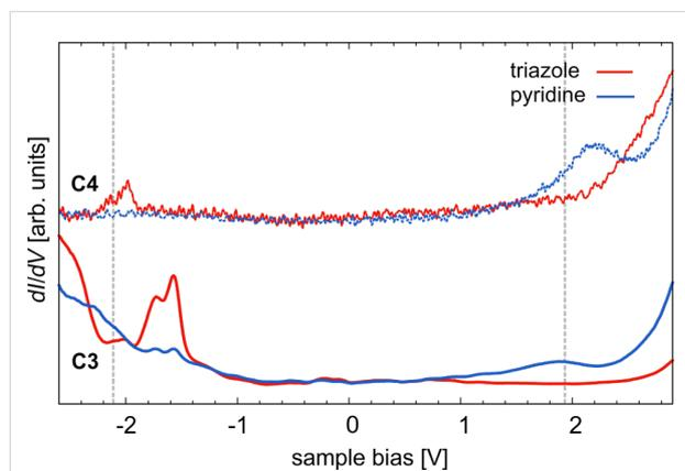
**Figure 8:** Tunneling spectra of **C3** and **C4** each acquired at the pyridine and triazole groups of the TL. For comparison, the vertical lines indicate the HOMO and LUMO levels of **C1** and **C2** [30].
