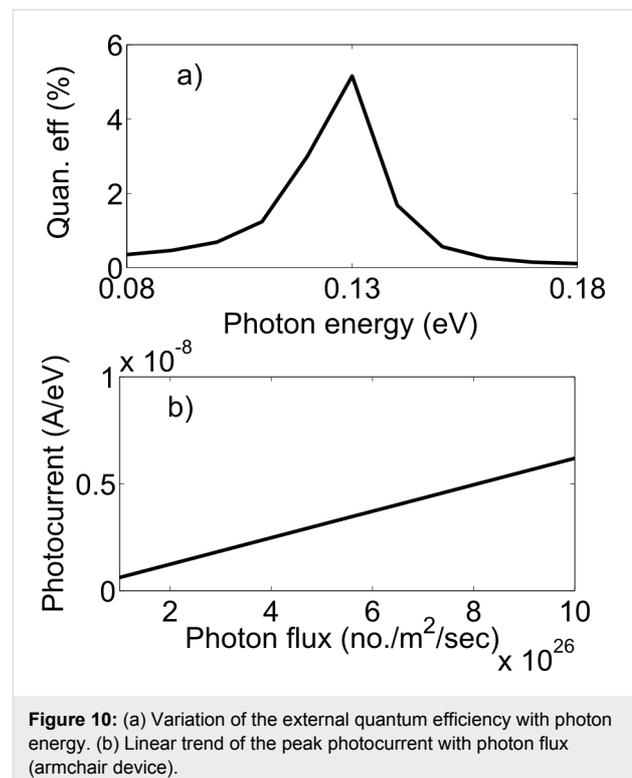
**Figure 10:** (a) Variation of the external quantum efficiency with photon energy. (b) Linear trend of the peak photocurrent with photon flux (armchair device).
