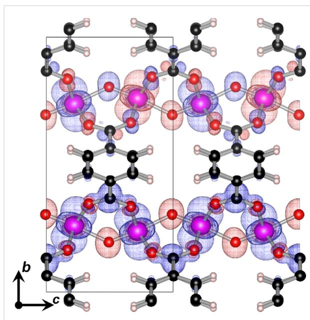
**Figure 3:** The spin density distribution of the SFM system. The upper chain has an antiferromagnetic spin configuration, while the lower chain has a ferromagnetic spin configuration. The iso-surface is taken at 0.00125, with majority spin shown in blue, and minority in red. The black rectangle indicates a single unit cell.
