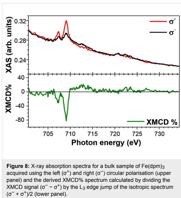
**Figure 8:** X-ray absorption spectra for a bulk sample of  $\text{Fe}(\text{dpm})_3$  acquired using the left ( $\sigma^+$ ) and right ( $\sigma^-$ ) circular polarisation (upper panel) and the derived XMCD% spectrum calculated by dividing the XMCD signal ( $\sigma^- - \sigma^+$ ) by the  $L_3$  edge jump of the isotropic spectrum ( $\sigma^- + \sigma^+$ )/2 (lower panel).
