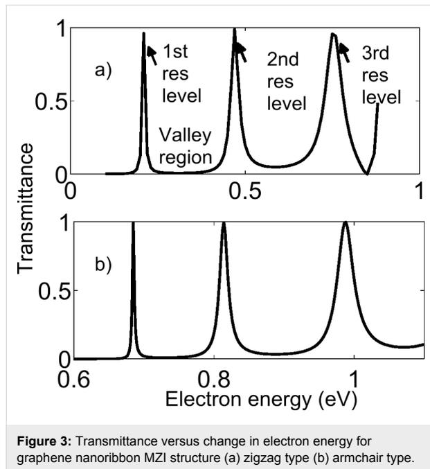
**Figure 3:** Transmittance versus change in electron energy for graphene nanoribbon MZI structure (a) zigzag type (b) armchair type.
