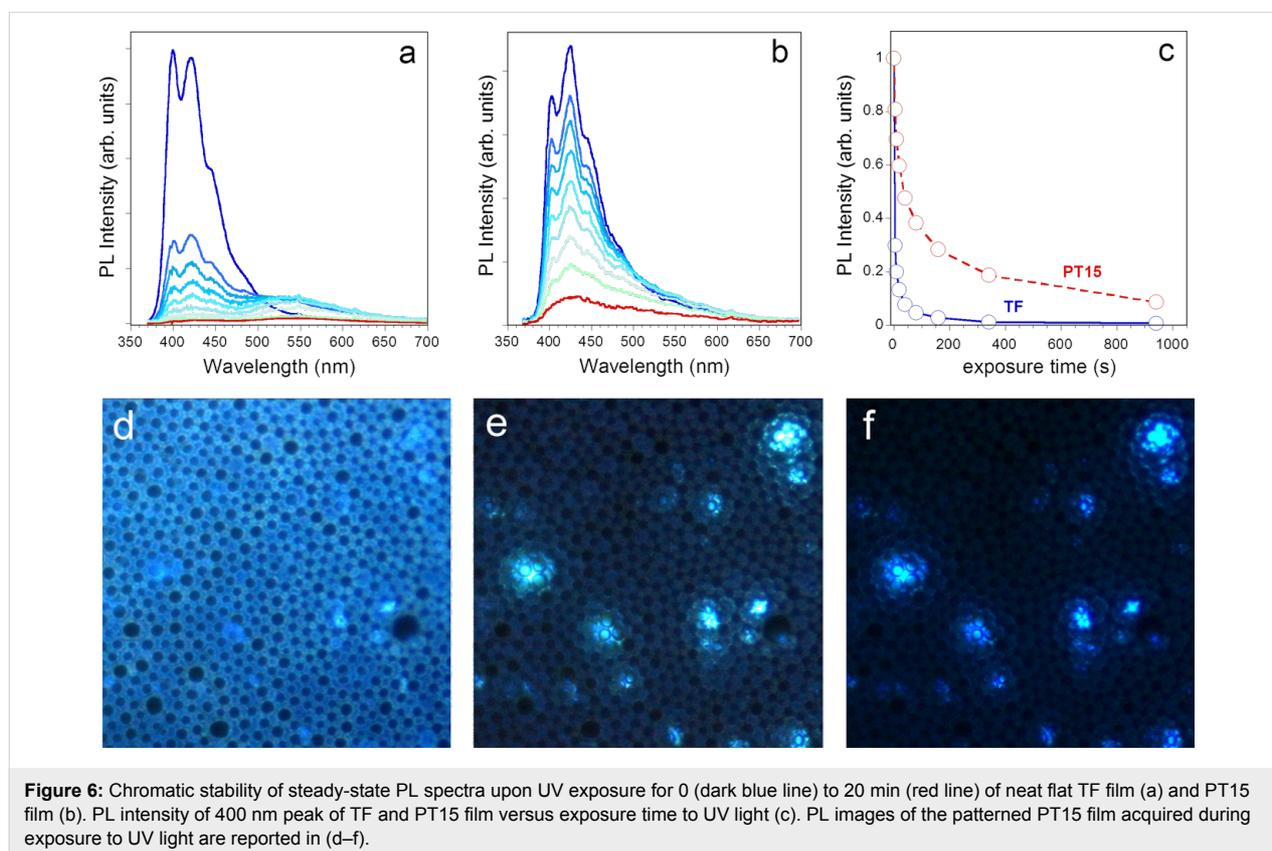
The hybrid material films exhibit ultraviolet-blue photoluminescence with a significantly enhanced photostability with respect to the bare oligo(fluorene), thanks to the intercalation of the dye in between the inorganic layers which inhibits the photochemical oxidation by blocking the oxygen penetration.
