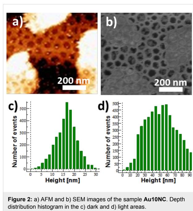
**Figure 2:** a) AFM and b) SEM images of the sample **Au10NC**. Depth distribution histogram in the c) dark and d) light areas.
