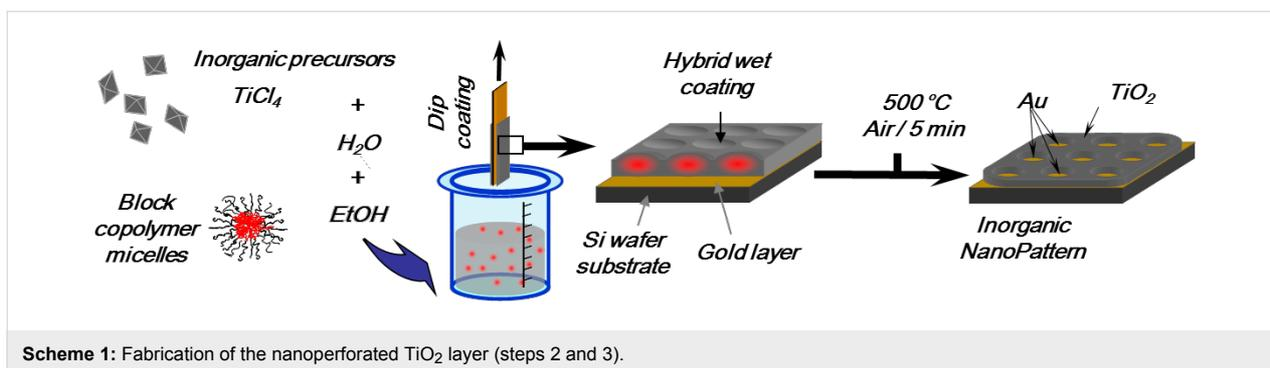
**Scheme 1:** Fabrication of the nanopatterned  $\text{TiO}_2$  layer (steps 2 and 3).
