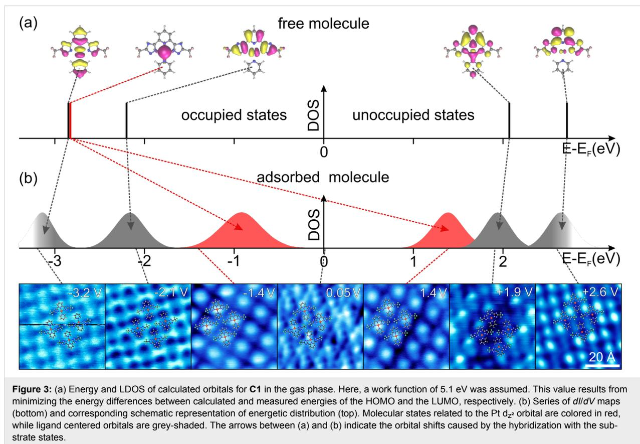
action cannot be large. This is indeed reflected in the above comparison. For the ligand orbitals, the major consequence of adsorbing the complex onto the Au substrate is a broadening of the levels due to weak hybridization with substrate states (i.e., physisorption) and only relatively small shifts in the energetic positions but no effect on the orbital order or occupancy.
