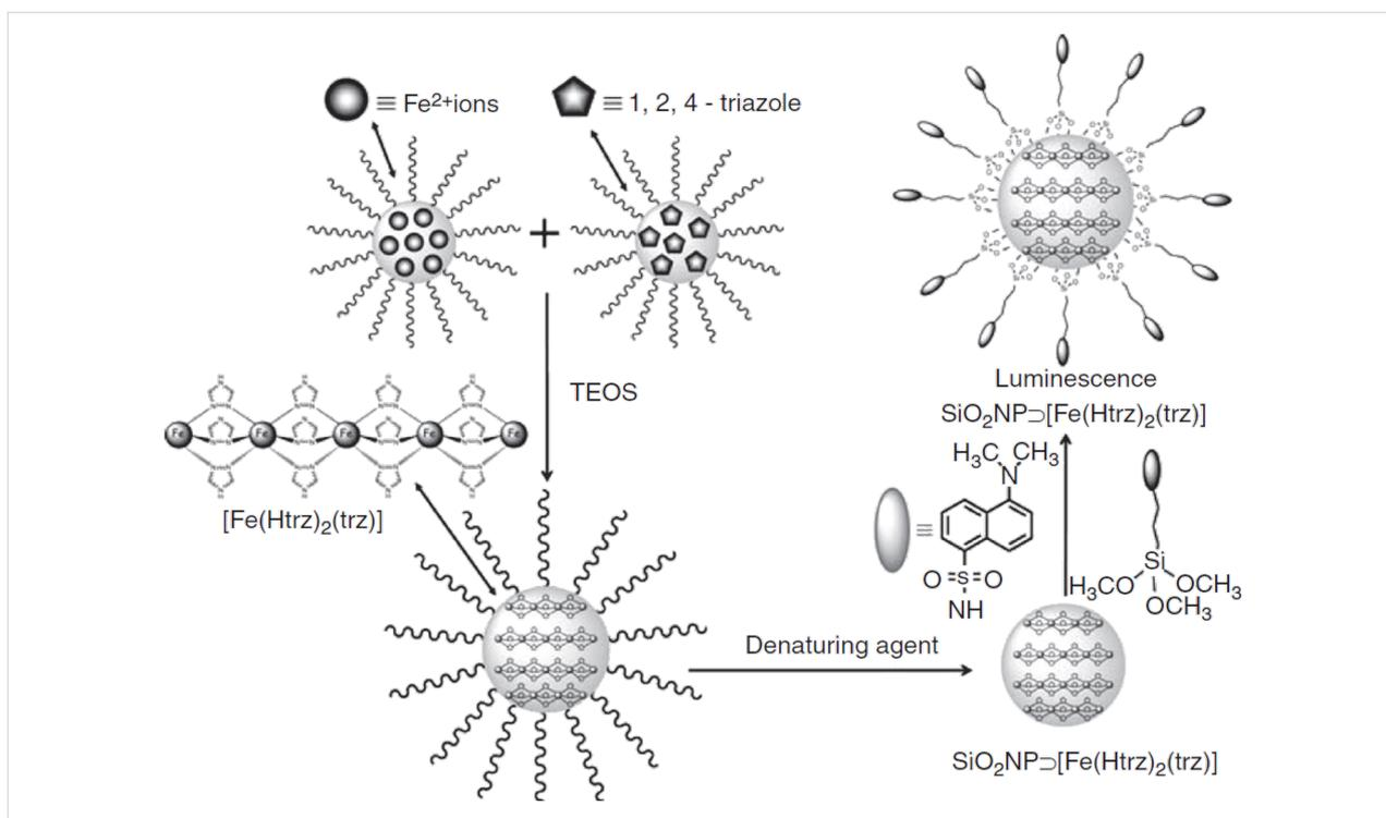
**Figure 2:** Synthesis route and schematic representation of the luminescent, SCO, SiO<sub>2</sub> nanoparticles. Reproduced with permission from [21], copyright 2011 Wiley-VCH.
