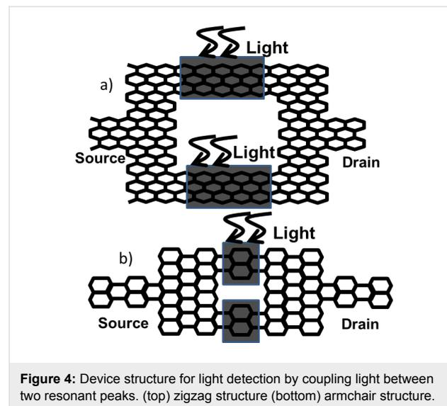
**Figure 4:** Device structure for light detection by coupling light between two resonant peaks. (top) zigzag structure (bottom) armchair structure.
