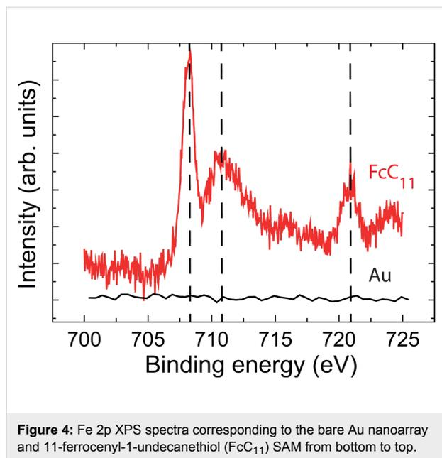
**Figure 4:** Fe 2p XPS spectra corresponding to the bare Au nanoarray and 11-ferrocenyl-1-undecanethiol (FcC<sub>11</sub>) SAM from bottom to top.
