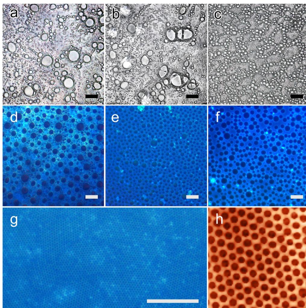
**Figure 5:** (a–c) Microscopy images of films of PT5, PT15 and PT30 cast under breath figure conditions. (d–f) Fluorescence microscopy images of PT5, PT15 and PT30 films prepared under the same conditions, after the addition of free TF (0.4% w/w). (g) Highly ordered microporous film of PT30 after optimization of parameters. (h) AFM view of a  $10 \times 10 \mu\text{m}^2$  area of the same film. All scale bars are 20  $\mu\text{m}$  long.
