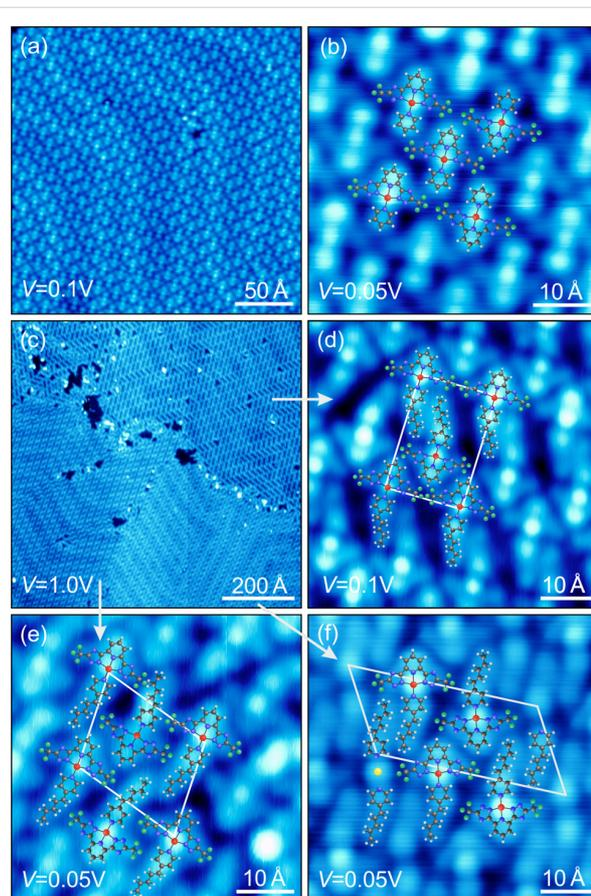
**Figure 2:** Topography analysis of a monolayer of **C1** (a,b) and **C2** (c–f) on Au(111). **C1** grows in only one close-packed structure probably due to steric packing. **C2** shows three different ordered structures, indicating the additional role of van der Waals forces between neighboring  $R^3$  alkyl chains for the self-assembly.
