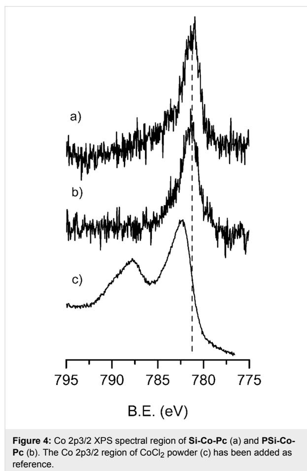
**Figure 4:** Co 2p<sub>3/2</sub> XPS spectral region of **Si-Co-Pc** (a) and **PSi-Co-Pc** (b). The Co 2p<sub>3/2</sub> region of  $\text{CoCl}_2$  powder (c) has been added as reference.
