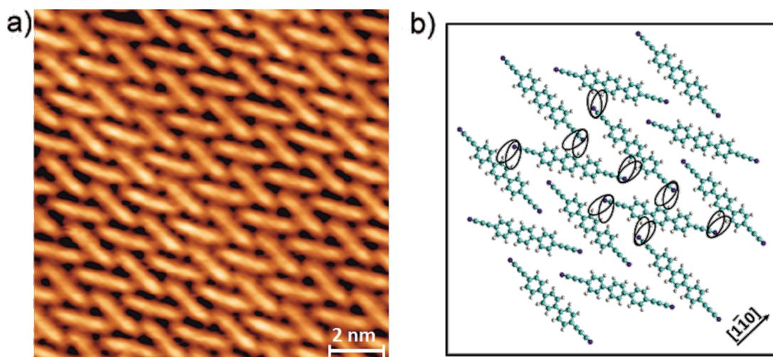
**Figure 4:** High-resolution STM image showing a) the molecular packing in chevron layers mediated by the propionitrile end groups of the NC–C≡C–Ph<sub>3</sub>–C≡C–CN (**2**) linker (data measured at 6 K; image size:  $119 \times 119$  Å<sup>2</sup>; scanning parameters:  $V_{\text{bias}} = 0.3$  V,  $I = 0.05$  nA); b) Corresponding model showing the interaction of adjacent propionitrile groups.
