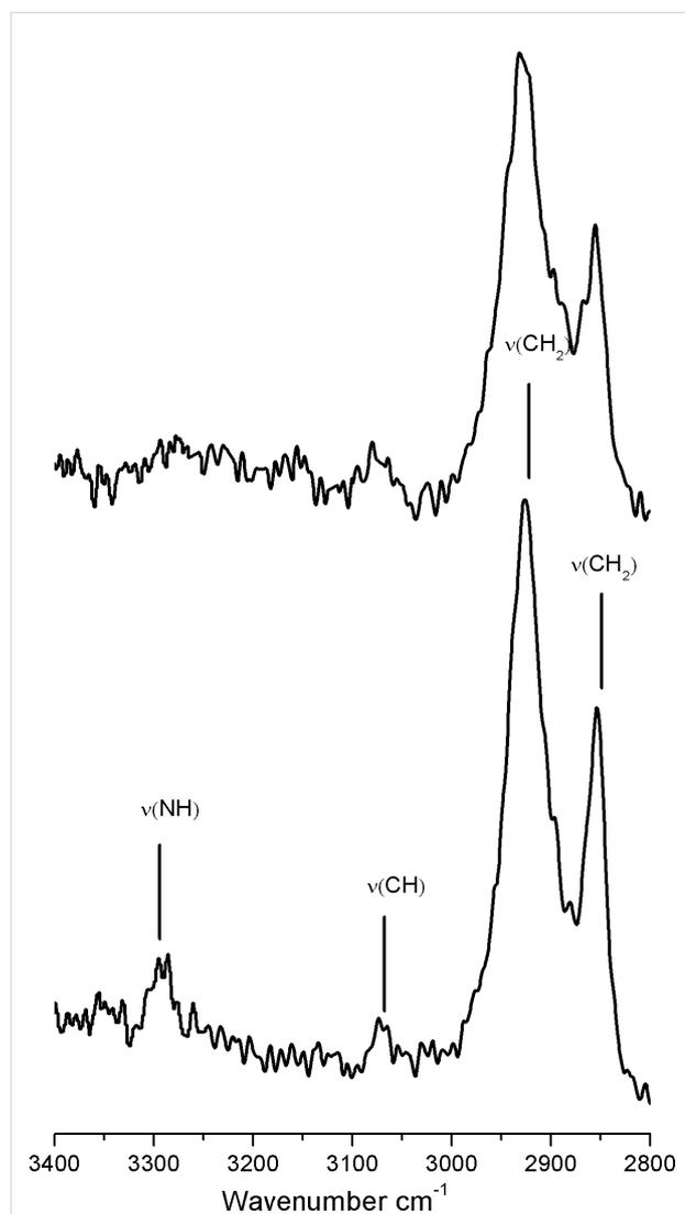
**Figure 6:** FTIR spectral region between 3400–2800  $\text{cm}^{-1}$  (CH<sub>x</sub> stretching region) of **PSi-1-Pc** (below) and **PSi-Co-Pc** (above).
