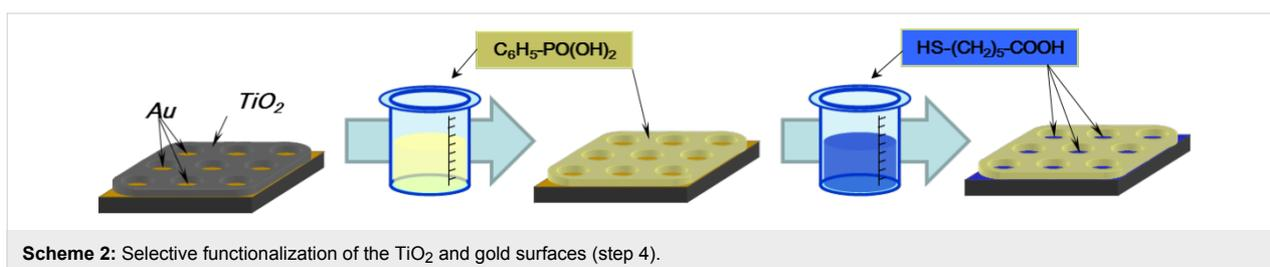
**Scheme 2:** Selective functionalization of the TiO<sub>2</sub> and gold surfaces (step 4).
