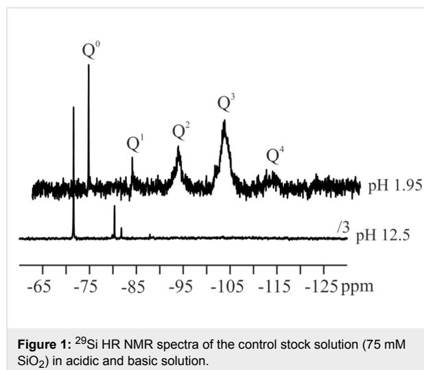
**Figure 1:**  $^{29}\text{Si}$  HR NMR spectra of the control stock solution (75 mM  $\text{SiO}_2$ ) in acidic and basic solution.
