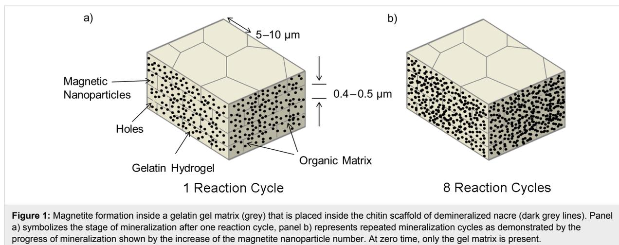
**Figure 1:** Magnetite formation inside a gelatin gel matrix (grey) that is placed inside the chitin scaffold of demineralized nacre (dark grey lines). Panel a) symbolizes the stage of mineralization after one reaction cycle, panel b) represents repeated mineralization cycles as demonstrated by the progress of mineralization shown by the increase of the magnetite nanoparticle number. At zero time, only the gel matrix is present.
