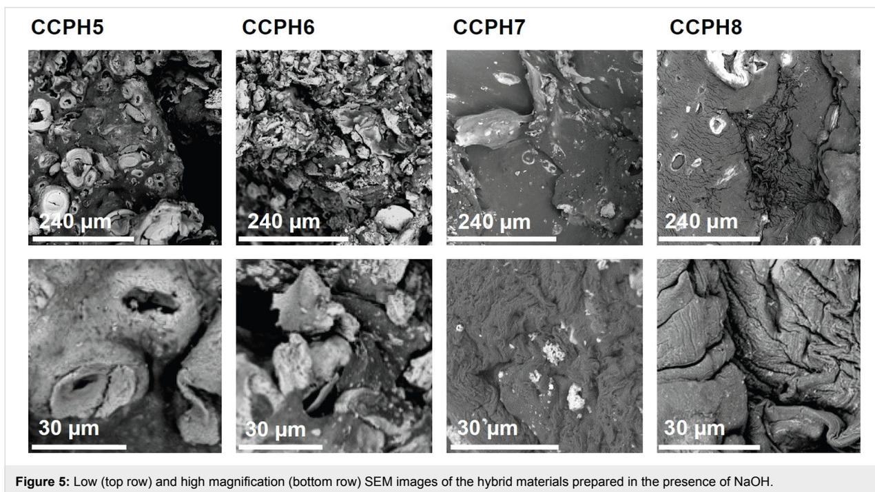
**Figure 5:** Low (top row) and high magnification (bottom row) SEM images of the hybrid materials prepared in the presence of NaOH.
