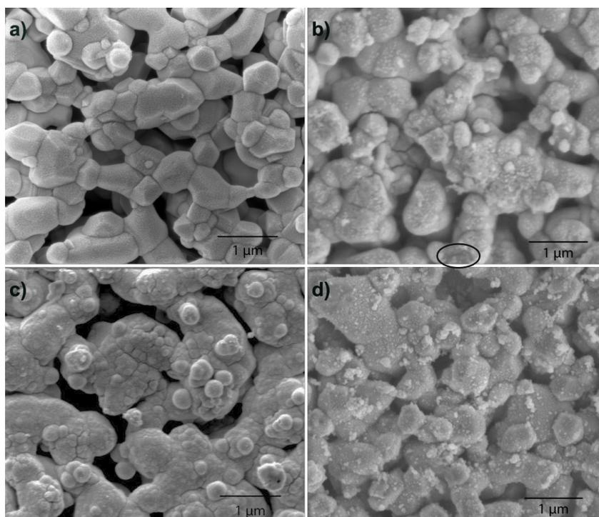
**Figure 5:** Top views of ceria deposition on NiO/GDC anodes. a) Treatment 1 (no coating). b) Treatment 2 (direct-treated). The ellipse indicates a gap in the coating. c) Treatment 3 (thiol-treated). d) Treatment 4 (sulfonate-treated).
