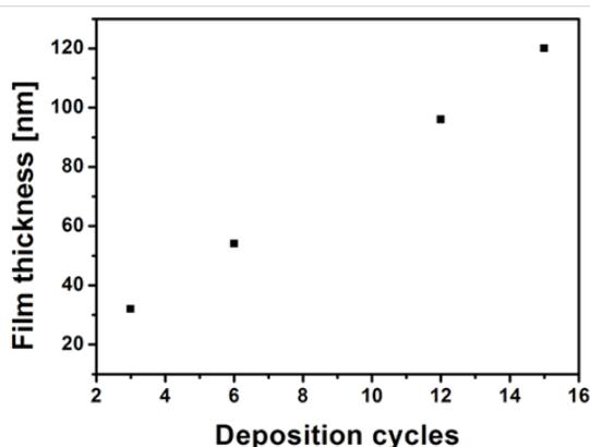
**Figure 4:** Overall thickness of the wt TMV/ZnO hybrid material as a function of the number of deposition cycles as determined by optical profilometry. ZnO was deposited onto the wt TMV template with an increasing number of deposition cycles from the precursor solution.
