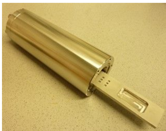
Figure 5: The tube reactor used for the chemical conversion of the golden algae.
