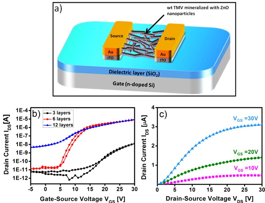
**Figure 5:** Schematic representation of the wt TMV/ZnO based FET device (a). Performance of the FET device fabricated by increasing the number of ZnO deposition cycles on the wt TMV template; (b) Transfer characteristics for constant drain–source voltage at 30 V; (c) output characteristics of TMV/ZnO hybrid after 6 deposition cycles, obtained at drain–source voltage of 30 V, for gate–source voltage varied from 0–30 V in 10 V steps.
