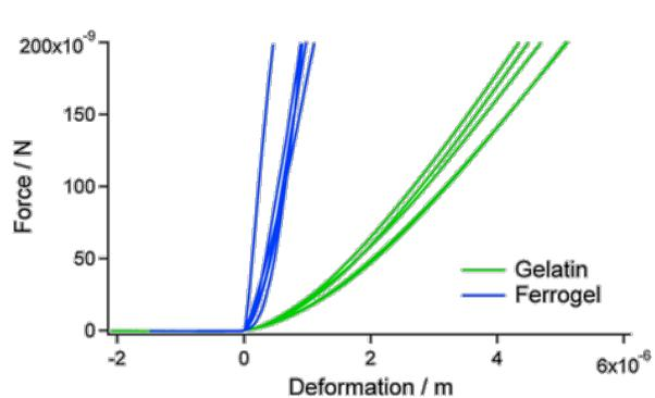
**Figure 12:** Force vs deformation characteristic of pure gelatin and gelatin with ferromagnetic particles. Introduction of nanoparticles leads to a significant increase of the stiffness of the material.
