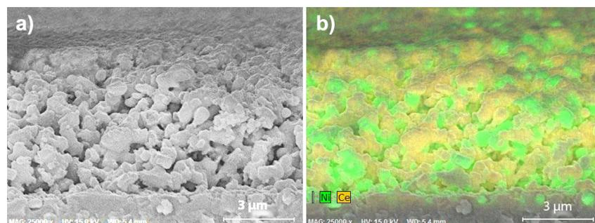
**Figure 8:** Cross-sectional view of a direct-treated anode (treatment 2) after cell operation. a) SEM image; b) EDXS mapping of Ni (green) and Ce (yellow).
