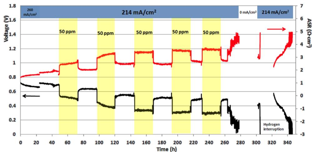
**Figure 2:** Output voltage and ASR, showing typical effects of partially reversible sulfur poisoning. Yellow bands denote periods of H<sub>2</sub>S exposure in the anode stream at the concentration indicated. (Treatment 3 cell, no interlayer.)
