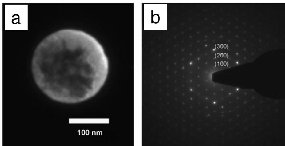
**Figure 7:** Dark-field TEM micrograph (a) and corresponding electron diffraction pattern (b) of hydroxyapatite/gelatin particles. Reprinted with permission from [87]. Copyright 2008 John Wiley & Sons.
