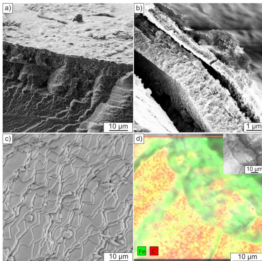
**Figure 4:** SEM micrographs of a) and b) fracture surfaces of artificial nacre and c) fracture surface of original nacre *Haliotis laevis*. d) EDX mapping analysis of artificial nacre fracture surface.
