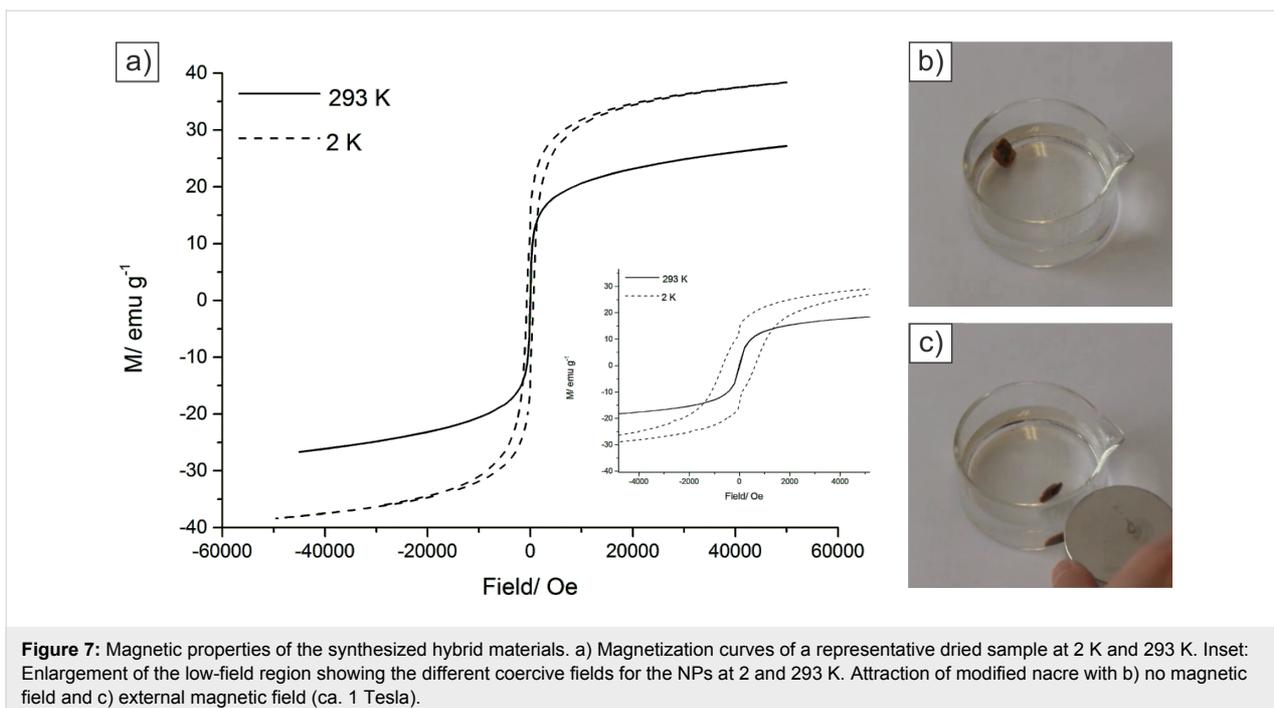
**Figure 7:** Magnetic properties of the synthesized hybrid materials. a) Magnetization curves of a representative dried sample at 2 K and 293 K. Inset: Enlargement of the low-field region showing the different coercive fields for the NPs at 2 and 293 K. Attraction of modified nacre with b) no magnetic field and c) external magnetic field (ca. 1 Tesla).
