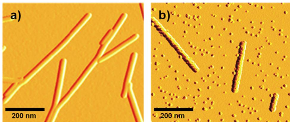
**Figure 3:** AFM micrographs of (a) the bare wt TMV template immobilized on a Si/SiO<sub>2</sub> substrate as well as (b) the wt TMV template after 1 cycle of ZnO mineralization.
