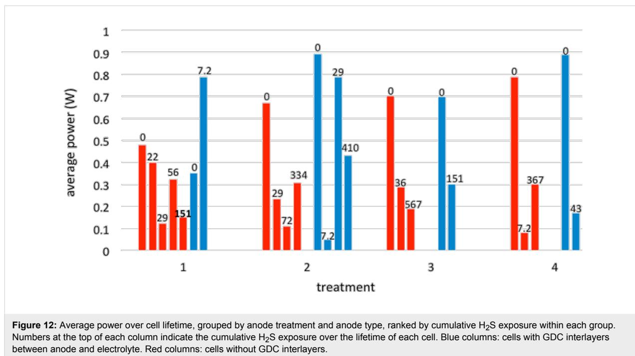
**Figure 12:** Average power over cell lifetime, grouped by anode treatment and anode type, ranked by cumulative H<sub>2</sub>S exposure within each group. Numbers at the top of each column indicate the cumulative H<sub>2</sub>S exposure over the lifetime of each cell. Blue columns: cells with GDC interlayers between anode and electrolyte. Red columns: cells without GDC interlayers.
