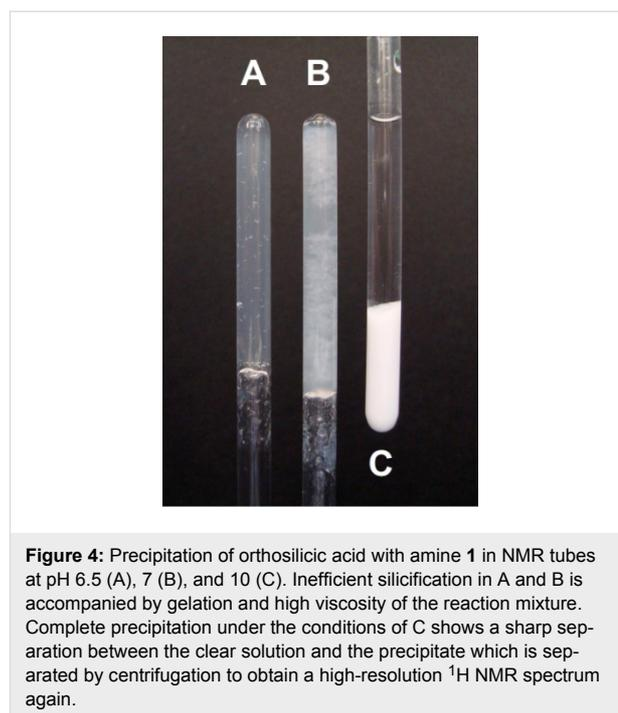
**Figure 4:** Precipitation of orthosilicic acid with amine 1 in NMR tubes at pH 6.5 (A), 7 (B), and 10 (C). Inefficient silicification in A and B is accompanied by gelation and high viscosity of the reaction mixture. Complete precipitation under the conditions of C shows a sharp separation between the clear solution and the precipitate which is separated by centrifugation to obtain a high-resolution  $^1\text{H}$  NMR spectrum again.
