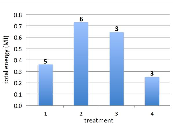
**Figure 11:** Average lifetime energy output of SOFCs (with and without GDC interlayers) tested in sulfur-containing fuel streams, grouped by treatment: 1, no coating; 2, direct ceria coating; 3, ceria coating after thiol treatment; 4, ceria coating after sulfonate treatment. The numeral above each column is the number of cells tested for each type of treatment.
