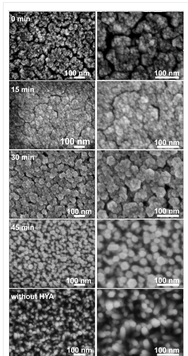
**Figure 4:** SEM micrographs of ZnO films after the first CBD. Growth was performed for 1 h in total with and without the addition of HYA. HYA was supplied after specific time intervals during the growth process as indicated.
