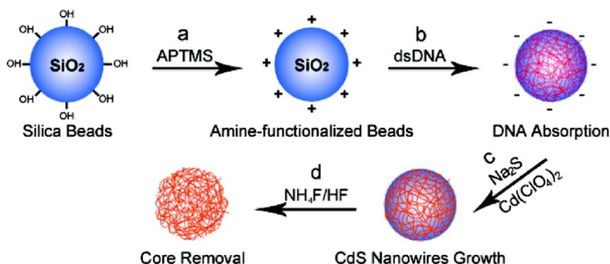
**Figure 3:** DNA-templated preparation of porous CdS shells on the surface of silica beads: (a) surface modification with (3-aminopropyl)trimethoxysilane (APTMS), (b) DNA deposition on the cationic particle surface, (c) CdS precipitation, and (d) dissolution of the  $\text{SiO}_2$  core to form hollow structures. Reprinted with permission from [52]. Copyright 2011 American Chemical Society.
