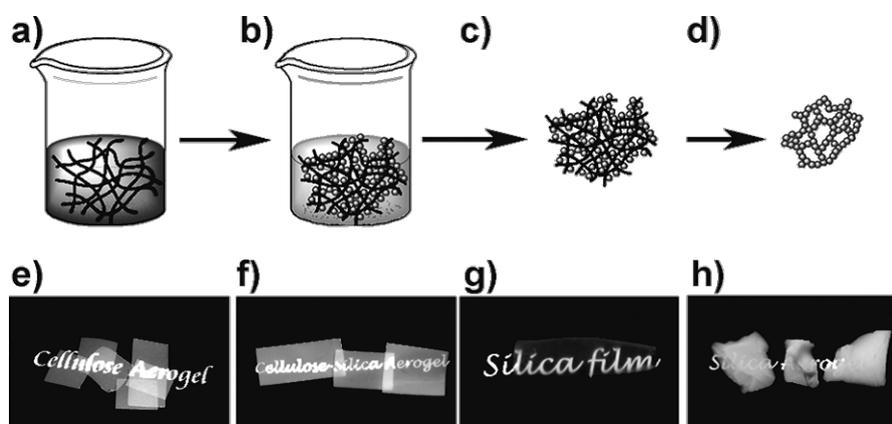
**Figure 8:** Schematic representation of aerogel preparation. A nanoporous cellulose gel is impregnated with the silica precursor TEOS (a). Afterwards, the silica formation takes place by sol–gel process (hydrolysis and condensation), yielding a cellulose–silica composite gel (b). Drying with supercritical  $\text{CO}_2$  gives a composite aerogel (c). Macroscopic views of the prepared samples are shown in panels (e–h). Reprinted with permission from [90]. Copyright 2012 John Wiley & Sons.
