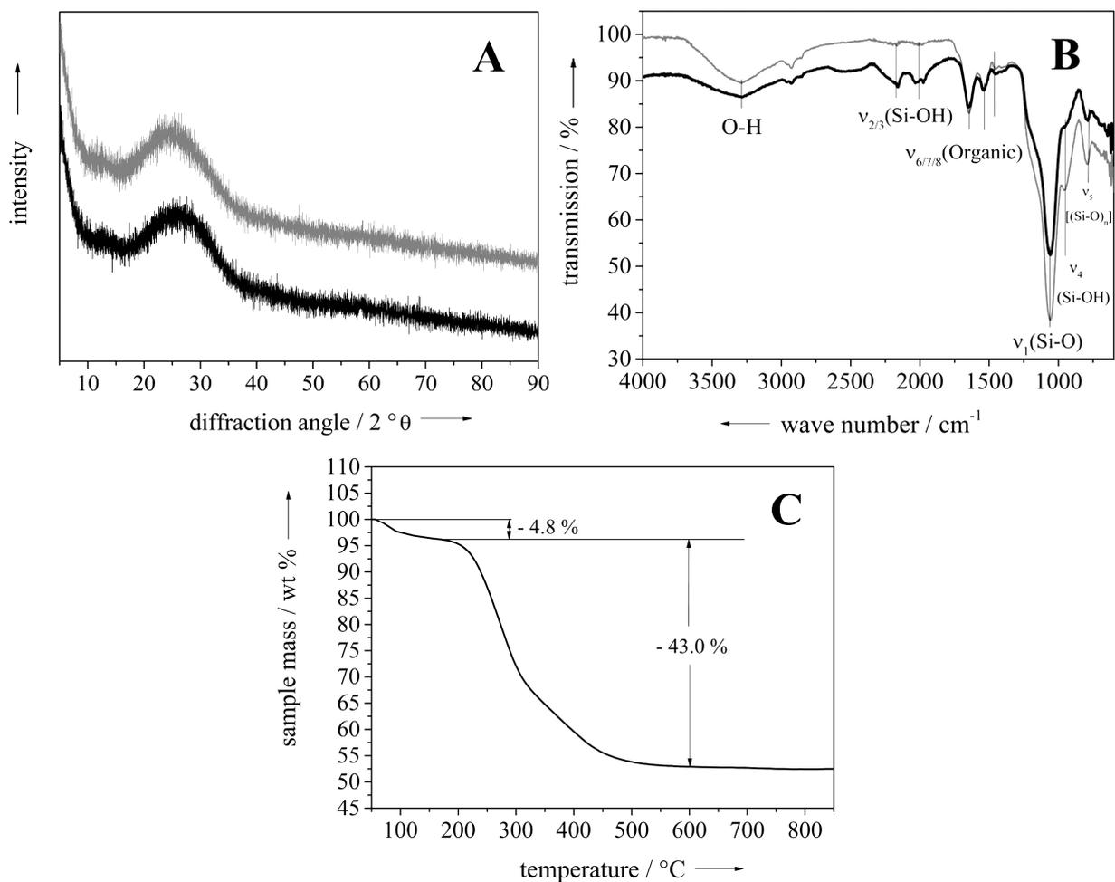
**Figure 3:** Characterization of the golden algae before the conversion. (A) shows powder diffractograms of *Synura petersenii* (black) and *Mallomonas caudata* (grey), (B) shows IR spectra of *Synura petersenii* (black) and *Mallomonas caudata* (grey), and (C) shows a thermogravimetric analysis of *Synura petersenii* in dynamic air atmosphere.
