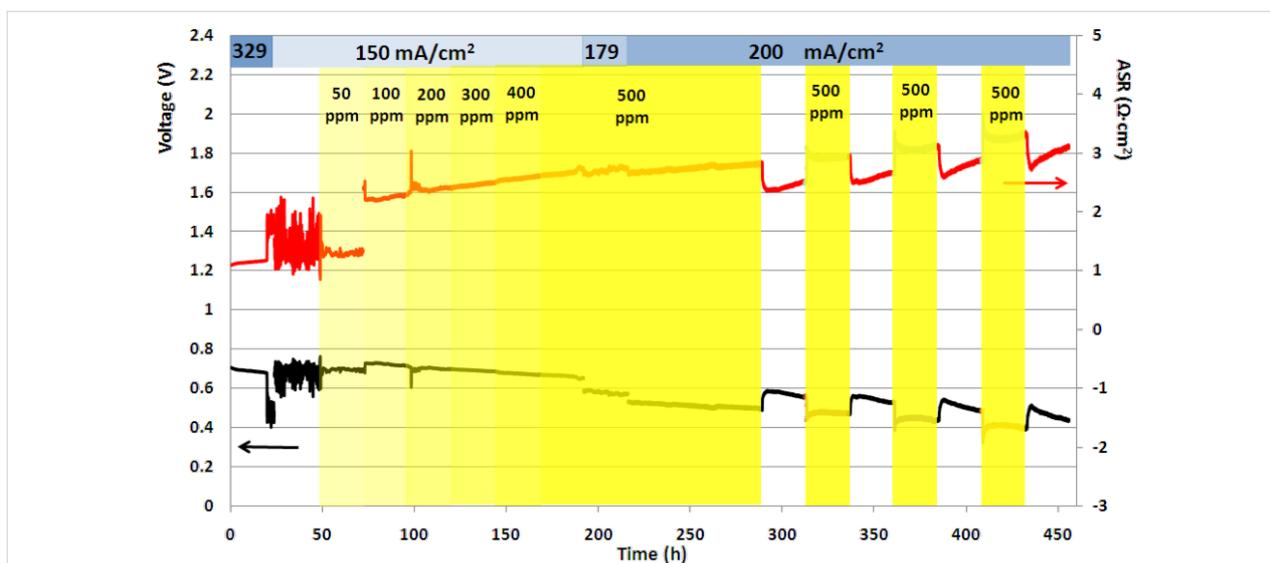
**Figure 3:** Output voltage and ASR, showing sulfur tolerance at a current density below  $200 \text{ mA}\cdot\text{cm}^{-2}$  (24–192 h) and partially reversible sulfur poisoning at  $200 \text{ mA}\cdot\text{cm}^{-2}$  (192–456 h). (Treatment-4 cell, no interlayer.)
