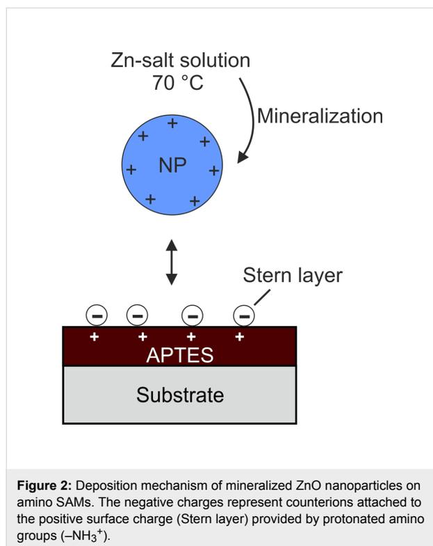
**Figure 2:** Deposition mechanism of mineralized ZnO nanoparticles on amino SAMs. The negative charges represent counterions attached to the positive surface charge (Stern layer) provided by protonated amino groups ( $-\text{NH}_3^+$ ).
