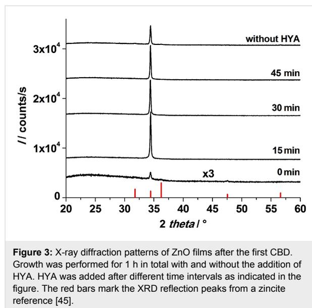
**Figure 3:** X-ray diffraction patterns of ZnO films after the first CBD. Growth was performed for 1 h in total with and without the addition of HYA. HYA was added after different time intervals as indicated in the figure. The red bars mark the XRD reflection peaks from a zincite reference [45].
