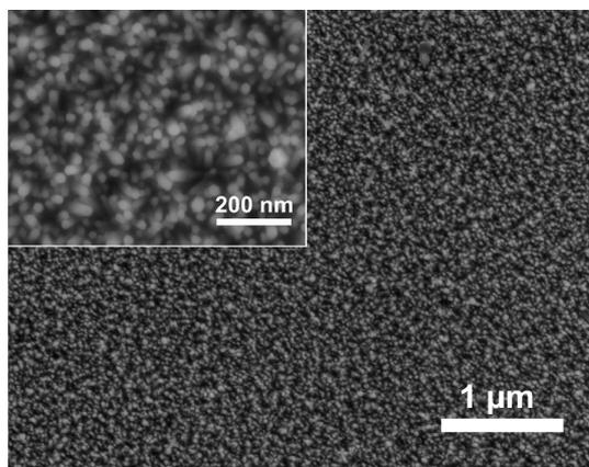
**Figure 2:** SEM micrographs of a ZnO nanorod array grown on a seeded glass slide for 1 h without the addition of HYA; the inset shows a higher magnification image.
