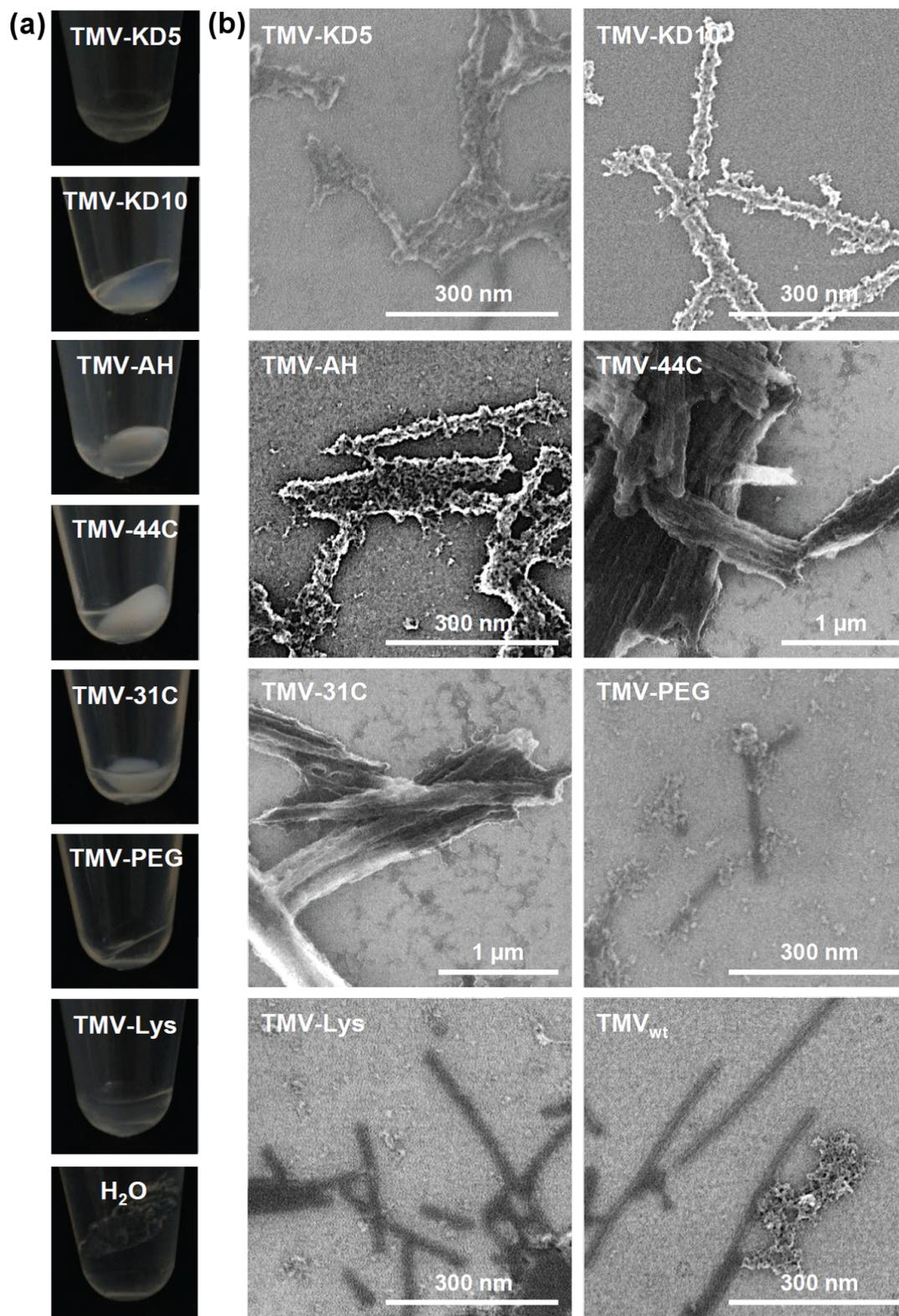
**Figure 4:** SiO<sub>2</sub> deposition reactions using functionalized and non-modified TMV templates, as indicated. (a) Images of sedimented products, and (b) corresponding SEM analysis. TMV-Lys-template (or water control) solutions were mixed with absolute EtOH (99.9%) and TEOS in a 4:4:1 volume ratio. Reaction products were sedimented by centrifugation (after 7 days of incubation in (a) or 10 days in (b)), resuspended in ddH<sub>2</sub>O and prepared for SEM (for details, refer to text).
