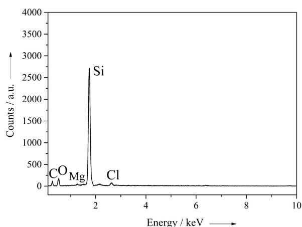
**Figure 7:** EDX spectra of *Synura petersenii* after conversion into silicon. The EDX spectra of *Mallomonas caudata* shows almost identical signals.
