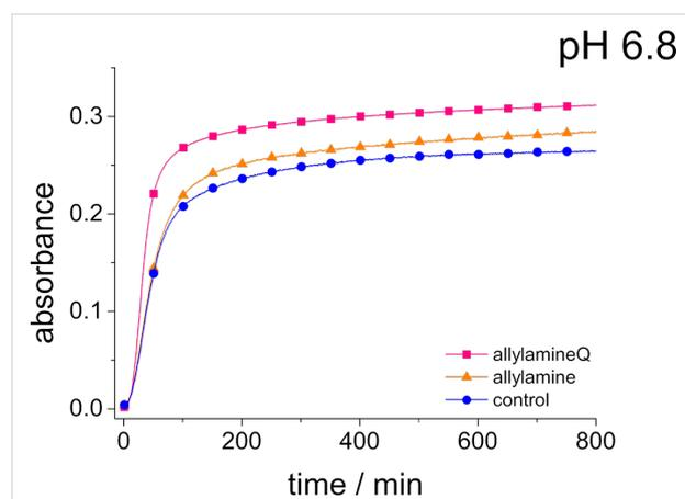
**Figure 5:** Absorbance of a 90 mM sodium metasilicate solution with 10 mM allylamine (orange triangles), 10 mM allylamineQ (pink squares) and of a sodium metasilicate solution (control, blue circles) measured as a function of time up to 800 minutes.
