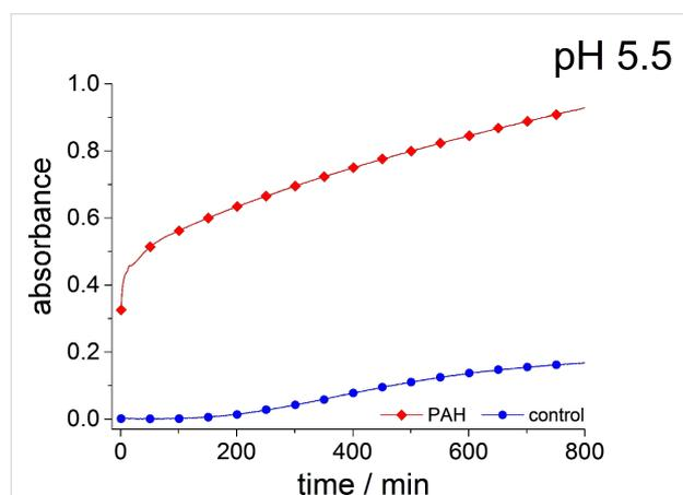
**Figure 4:** Absorbance of a 90 mM sodium metasilicate solution with 31.25  $\mu$ M PAH and 180 mM hydrogen phosphate (red rhombuses) and of a sodium metasilicate solution 90 mM containing 180 mM hydrogen phosphate (control, blue circles) measured as a function of time up to 800 min.
