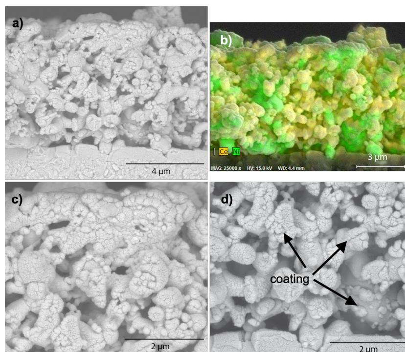
**Figure 9:** Cross-sectional views of the thiol-treated anode (treatment 3) of the cell shown in Figure 2 after operation. a) Whole anode thickness; b) EDXS mapping of Ni (green) and Ce (yellow); c) and d) higher magnification, c) near the anode surface and d) near the electrolyte (electrolyte is visible at bottom). Images c) and d) show that the ceria coating persisted throughout the anode. (Arrows in d) point to coating edges or cracks).
