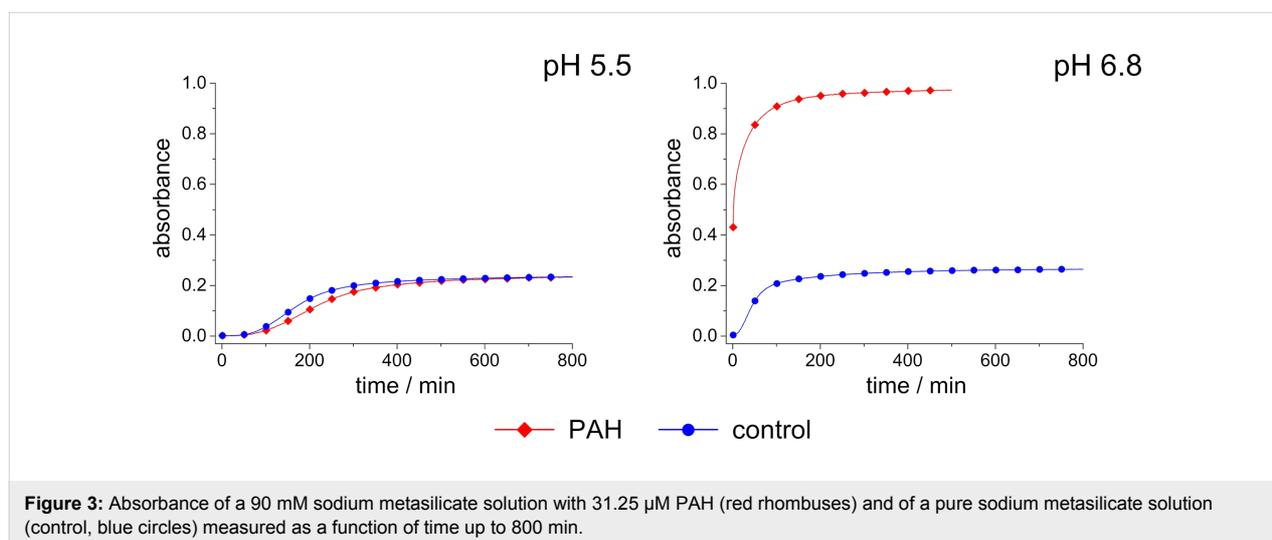
**Figure 3:** Absorbance of a 90 mM sodium metasilicate solution with 31.25  $\mu\text{M}$  PAH (red rhombuses) and of a pure sodium metasilicate solution (control, blue circles) measured as a function of time up to 800 min.
