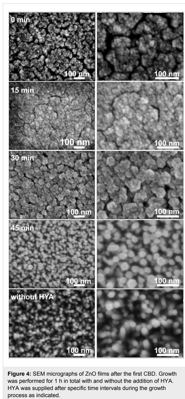
**Figure 4:** SEM micrographs of ZnO films after the first CBD. Growth was performed for 1 h in total with and without the addition of HYA. HYA was supplied after specific time intervals during the growth process as indicated.
