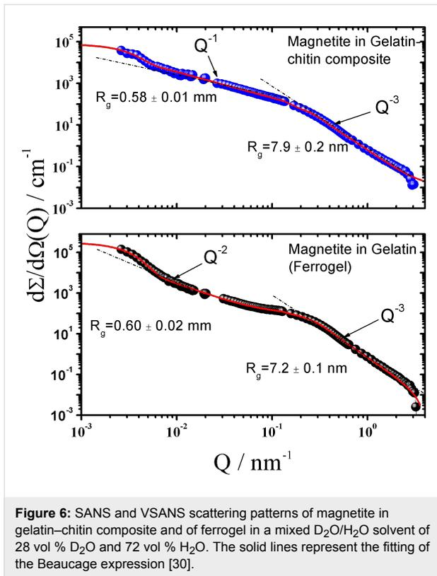
**Figure 6:** SANS and VSANS scattering patterns of magnetite in gelatin-chitin composite and of ferrogel in a mixed  $D_2O/H_2O$  solvent of 28 vol %  $D_2O$  and 72 vol %  $H_2O$ . The solid lines represent the fitting of the Beaucage expression [30].
