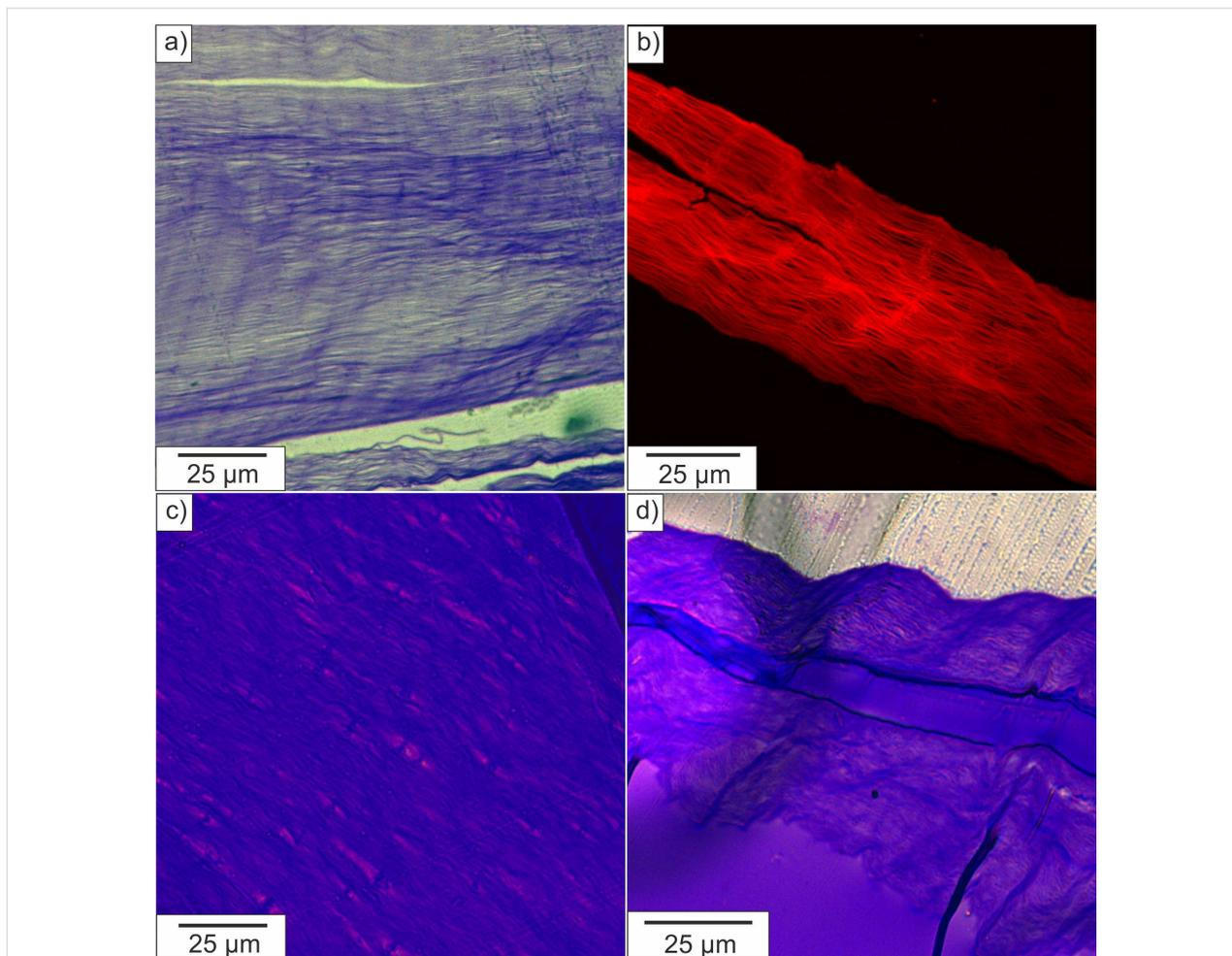
**Figure 3:** Light microscopy image of thin cuts of embedded and Coomassie stained samples. a) Demineralized nacre matrix, b) confocal laser scanning microscopy of embedded demineralized nacre matrix stained with rhodamine B ITC, c) and d) demineralized nacre matrix (blue) with infiltrated gelatin (purple).
