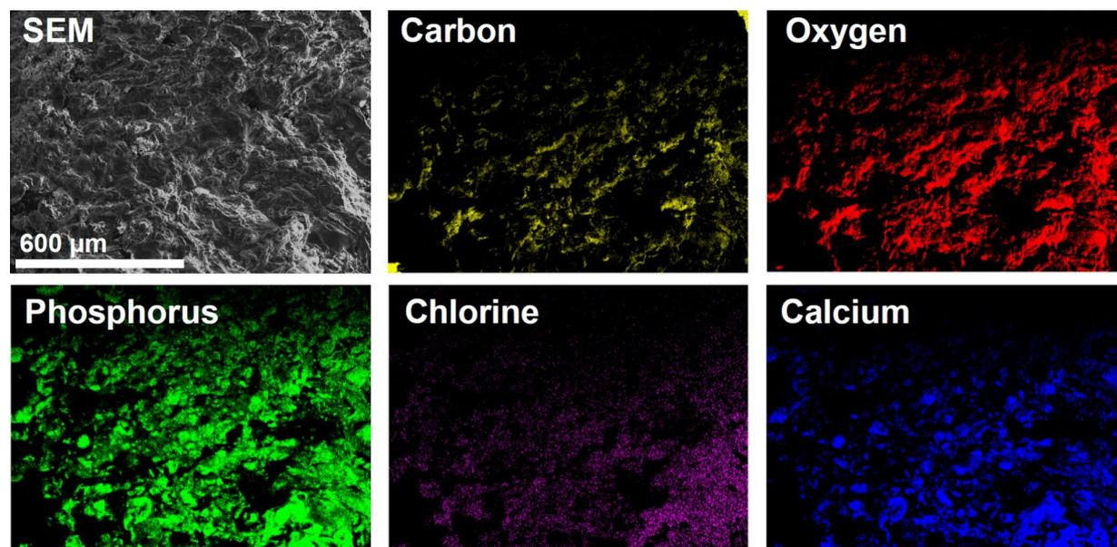
**Figure 7:** SEM image and elemental map of CCPH6.
