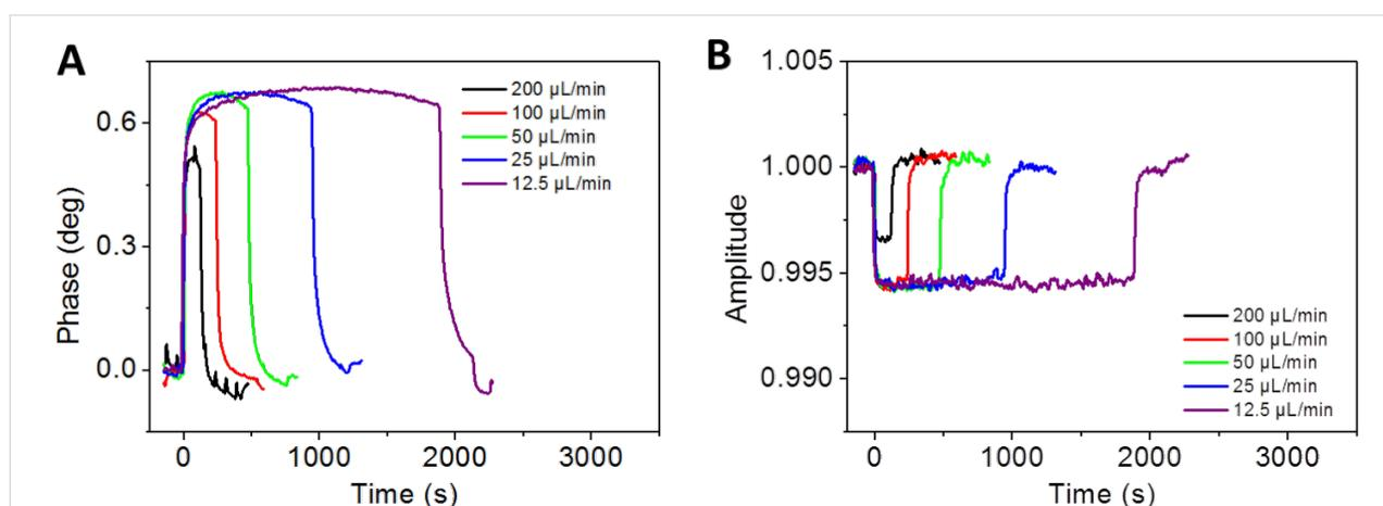
**Figure 2:** Flow-rate dependency of calcium carbonate interactions with COO-SAM chip. Phase vs time plot (A) and corresponding amplitude vs time plot (B) for different flow rates. A constant volume of 400  $\mu\text{L}$  calcium carbonate in pure water (140  $\mu\text{mol}/\text{L}$ ) was injected, followed by pure water for 5 minutes.
