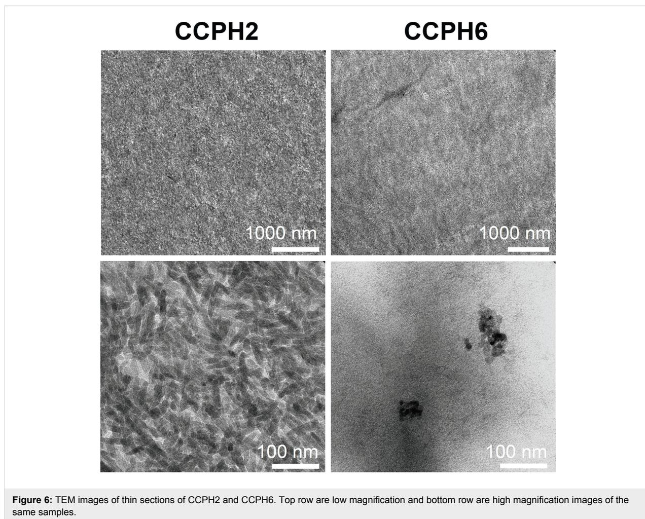
**Figure 6:** TEM images of thin sections of CCPH2 and CCPH6. Top row are low magnification and bottom row are high magnification images of the same samples.
