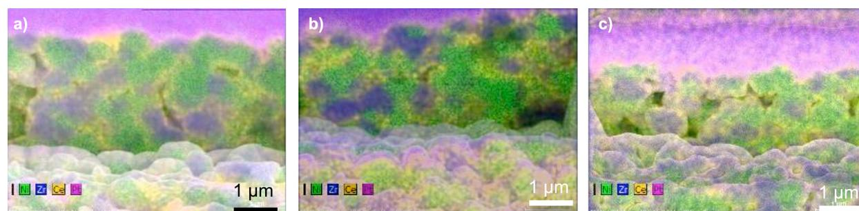
**Figure 6:** FIB cross-sections halfway through ceria-coated NiO/YSZ anodes, with superimposed EDXS maps (Ni: green; Zr: blue; Ce: yellow). a) Direct deposition (treatment 2). b) Deposition after thiol treatment (treatment 3). c) Deposition after sulfonate treatment (treatment 4). (Pink regions are the protective Pt layer applied as part of the FIB sectioning technique.)
