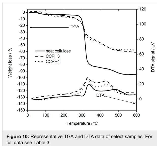
**Figure 10:** Representative TGA and DTA data of select samples. For full data see Table 3.
