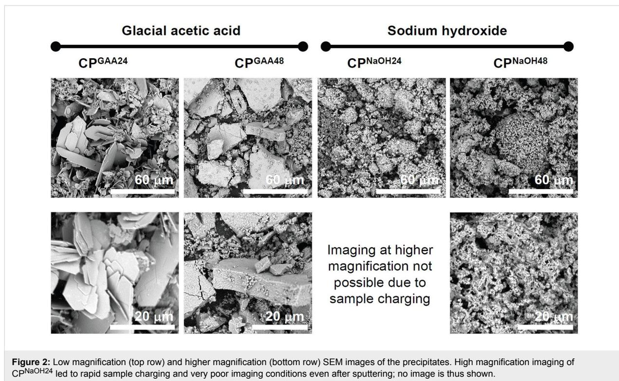
**Figure 2:** Low magnification (top row) and higher magnification (bottom row) SEM images of the precipitates. High magnification imaging of  $\text{CP}^{\text{NaOH}24}$  led to rapid sample charging and very poor imaging conditions even after sputtering; no image is thus shown.
