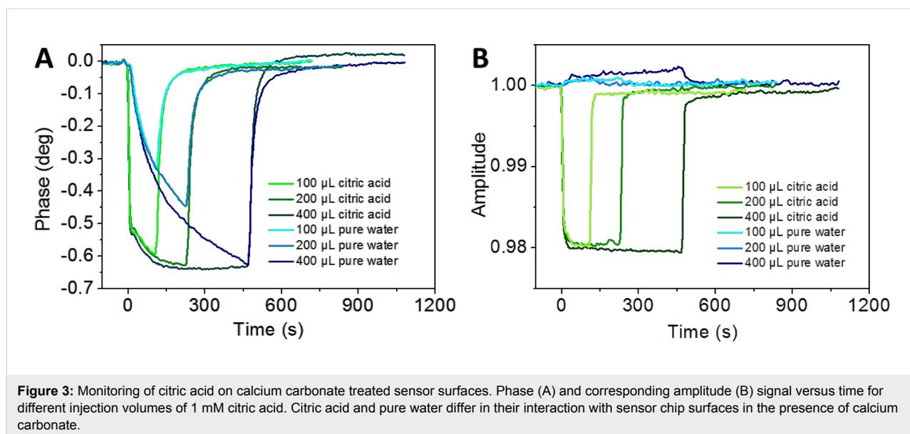
**Figure 3:** Monitoring of citric acid on calcium carbonate treated sensor surfaces. Phase (A) and corresponding amplitude (B) signal versus time for different injection volumes of 1 mM citric acid. Citric acid and pure water differ in their interaction with sensor chip surfaces in the presence of calcium carbonate.
