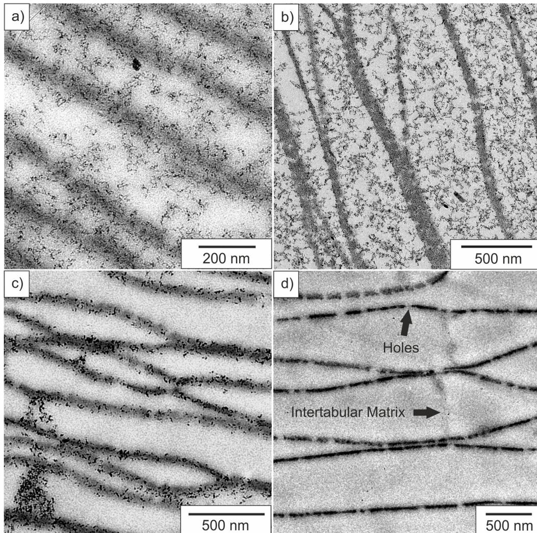
**Figure 5:** TEM micrographs of a) artificial nacre after one reaction cycle and b) after four reaction cycles, c) reference chitin–magnetite composite sample without gelatin, and d) completely demineralized matrix.
