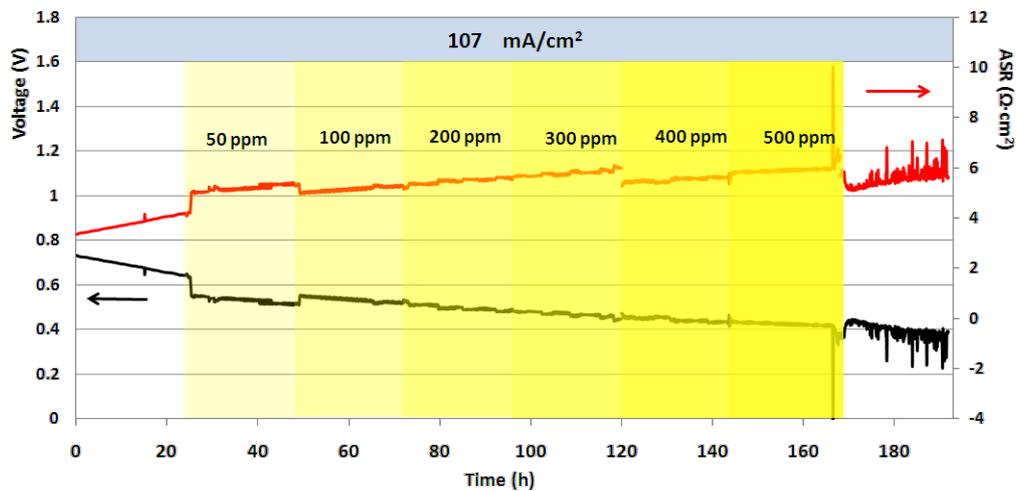
**Figure 1:** Output voltage and ASR at low current density, showing sulfur tolerance. Yellow shading denotes 24 h periods of H<sub>2</sub>S exposure in the anode stream at the concentration indicated. (Treatment-1 cell (no ceria coating) with no interlayer.)
