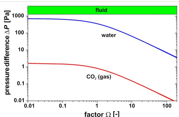
**Figure 9:** Pressure difference  $\Delta P$  of a circular membrane at  $t = 0.5$  s as a function of factor  $\Omega$  for a water-filled and CO<sub>2</sub>-filled cavity. IR power density 10 W/m<sup>2</sup>, diameter and height of the cavity: 0.5 mm.
