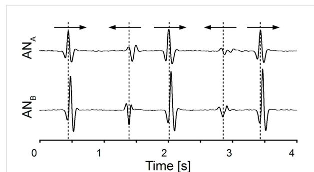
**Figure 1:** Responses of sensor platform I to a human finger that moved alongside the ALLC with a velocity of about 20 cm/s. Arrows indicate direction of finger motion. Responses of  $AN_A$  (upper graph) and  $AN_B$  (lower graph) are shown. Note that the responses were inverted if the direction of finger motion was reversed.
