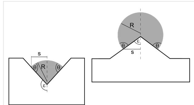
**Figure 1:** Sphere like droplets of fluid #1 (grey) attached to an axially symmetric solid cone (the broken line represents the symmetry axis).  $\theta$ : contact angle,  $R$ : droplet radius,  $s$ : radius of contact circle (= line where solid, fluid #1 and fluid #2 are in contact),  $\varepsilon$ : apex half-angle of protrusion (for  $0^\circ < \varepsilon < 90^\circ$ , right) or cavity (for  $90^\circ < \varepsilon < 180^\circ$ , left).
