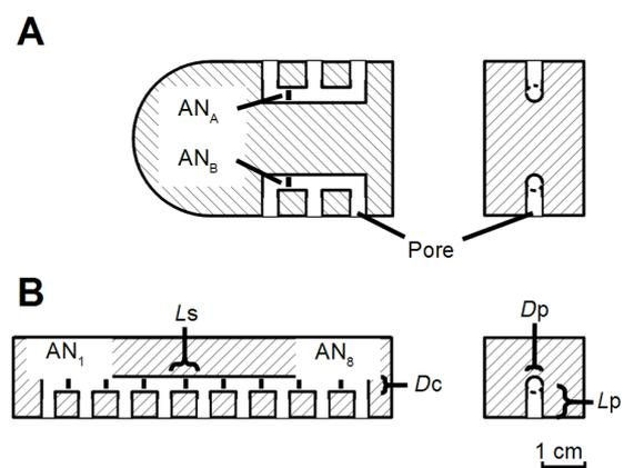
**Figure 6:** Horizontal (left) and vertical (right) cross sections of platforms III (A) and IV (B) that were used for the present study. Black squares indicate the positions of the ANs inside artificial lateral line canals. Platform III housed two and platform IV housed eight ANs. The length of pores ( $L_p$ ) was 1 cm, the inter pore distance ( $L_s$ ) was 1 cm and the diameter of the canal ( $D_c$ ) as well as the pore diameter ( $D_p$ ) was 3 mm in both devices.
