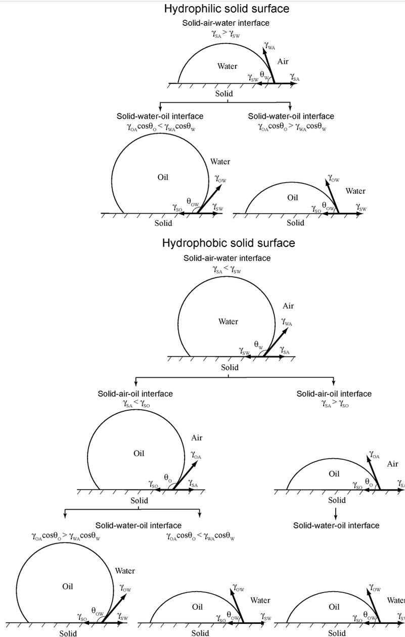
**Figure 11:** Schematics of a droplet of liquid showing philic/phobic nature in three different phase interface on the surface –  $\theta_W$ ,  $\theta_O$ , and  $\theta_{OW}$  are the static contact angles of a water droplet, an oil droplet, and an oil droplet in water, respectively [20].
