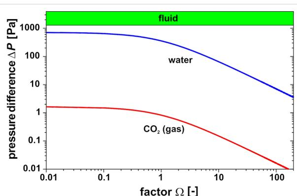
**Figure 9:** Pressure difference  $\Delta P$  of a circular membrane at  $t = 0.5 \text{ s}$  as a function of factor  $\Omega$  for a water-filled and  $\text{CO}_2$ -filled cavity. IR power density  $10 \text{ W/m}^2$ , diameter and height of the cavity:  $0.5 \text{ mm}$ .
