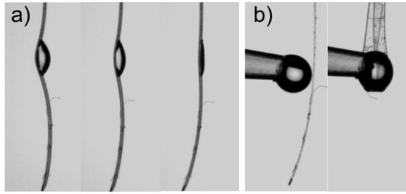
**Figure 2:** Effect of droplets of water on a thin polydimethylsiloxane (PDMS) membrane ribbon substrate hanging vertically: a) droplet causing a bending of the substrate which disappears as evaporation proceeds (three frames), b) spontaneous wrapping as a droplet touches a membrane ribbon (initial and final states).
