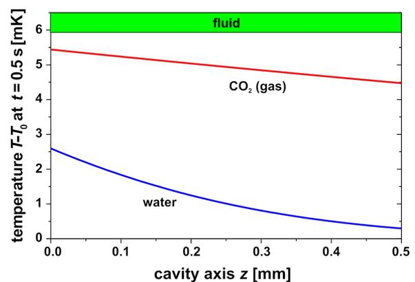
**Figure 8:** Temperature distribution along the cavity axis  $z$   $0.5 \text{ s}$  after the onset of irradiation for a water-filled and a  $\text{CO}_2$ -filled cavity with an IR power density at the outer window surface of  $10 \text{ W/m}^2$ . In the case of gas, a thin IR absorber film is assumed on the inner glass surface where all the IR energy is absorbed.
