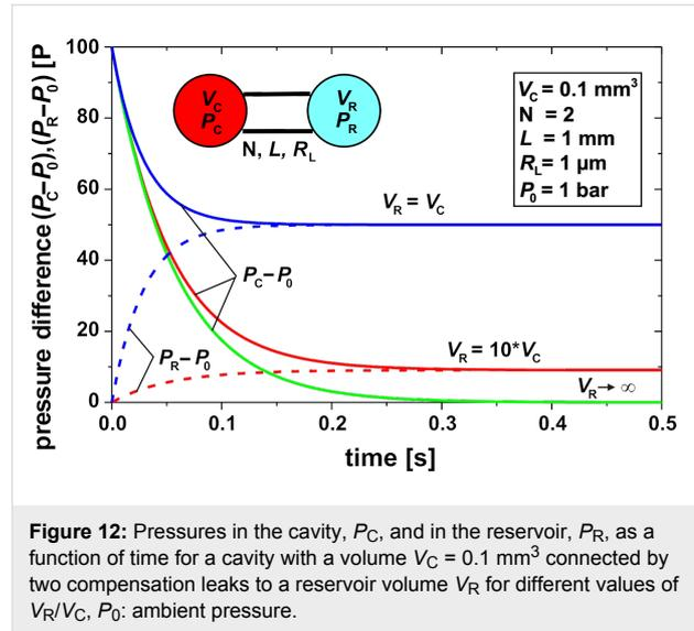
**Figure 12:** Pressures in the cavity,  $P_C$ , and in the reservoir,  $P_R$ , as a function of time for a cavity with a volume  $V_C = 0.1 \text{ mm}^3$  connected by two compensation leaks to a reservoir volume  $V_R$  for different values of  $V_R/V_C$ ,  $P_0$ : ambient pressure.
