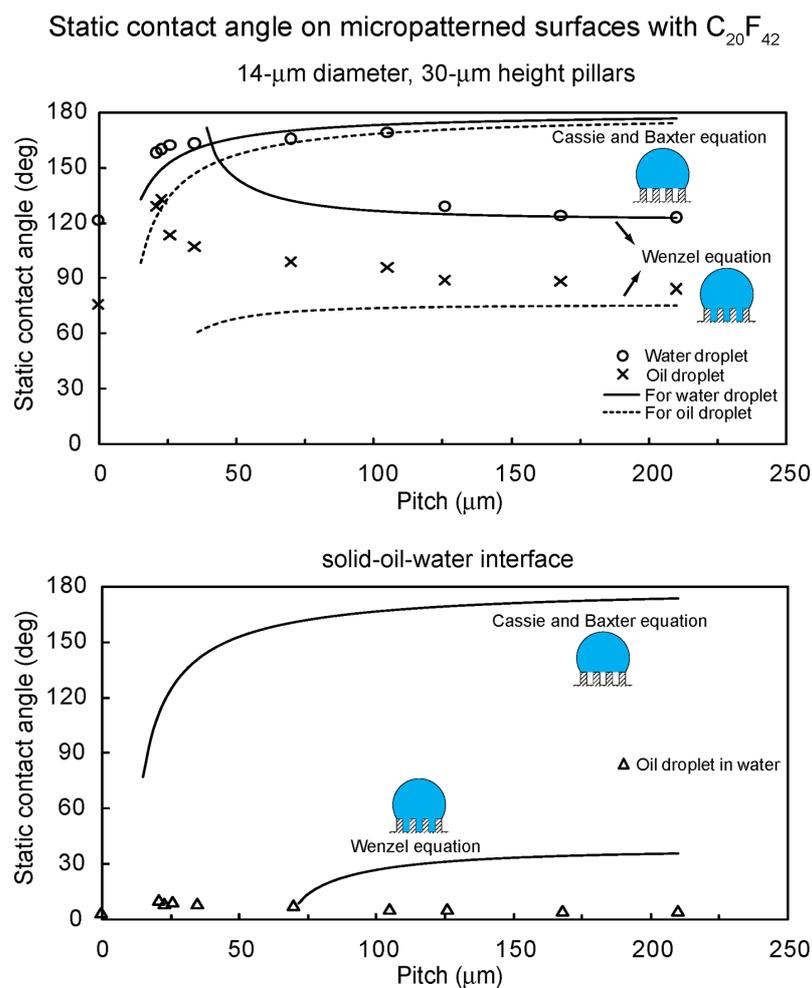
**Figure 16:** Static contact angle as a function of geometric parameters for water droplet (circle) and oil droplet (cross) in air, and oil droplet in water (triangles) compared with predicted static contact angle values obtained using the Wenzel and Cassie–Baxter equations (solid lines) with a measured value of  $\theta_0$  for the micropatterned surfaces with  $C_{20}F_{42}$  [20].
