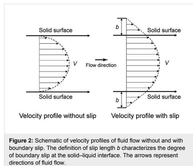
**Figure 2:** Schematic of velocity profiles of fluid flow without and with boundary slip. The definition of slip length  $b$  characterizes the degree of boundary slip at the solid–liquid interface. The arrows represent directions of fluid flow.
