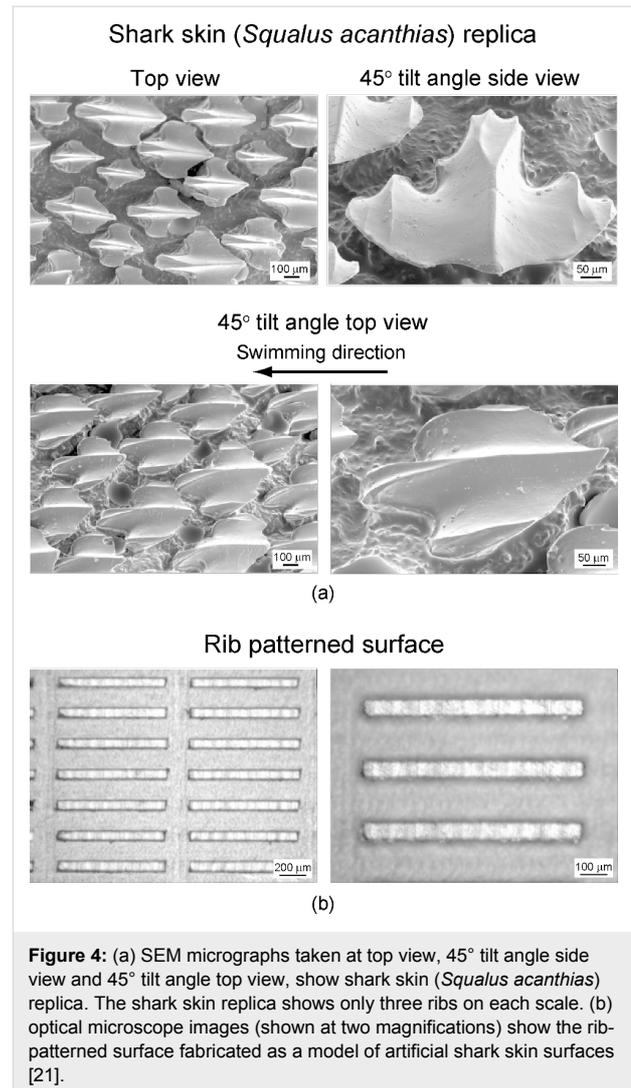
**Figure 4:** (a) SEM micrographs taken at top view, 45° tilt angle side view and 45° tilt angle top view, show shark skin (*Squalus acanthias*) replica. The shark skin replica shows only three ribs on each scale. (b) optical microscope images (shown at two magnifications) show the rib-patterned surface fabricated as a model of artificial shark skin surfaces [21].
