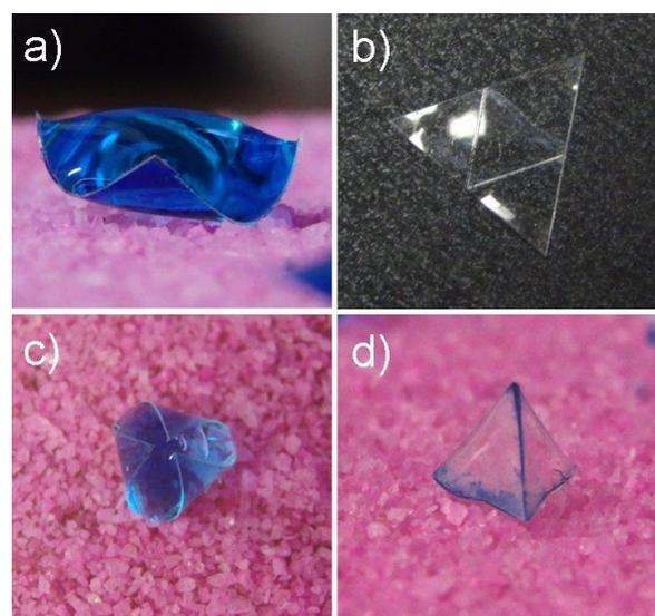
**Figure 1:** Effect of droplets of blue-dyed water on a thin polydimethylsiloxane (PDMS) membrane: a) droplet causing bending of the substrate, b) initial shaped substrate with the three score lines for folding, c) droplet induced folding, and d) three-dimensional shape left after completion of evaporation.
