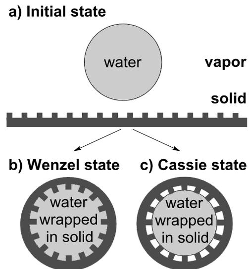
**Figure 3:** Initial and final states involved in a droplet wrapping event for a flexible ribbon membrane with rigid roughness. In the Wenzel case the liquid penetrates between features and in the Cassie case it bridges between them.
