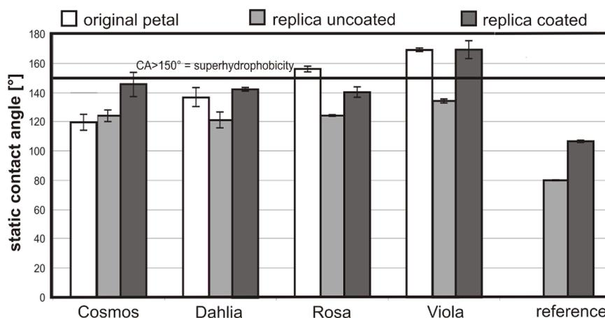
**Figure 4:** Static CAs of 5  $\mu\text{l}$  water droplets on the surfaces of fresh (original) petals, their uncoated and coated polymer replicas and of the reference (uncoated and coated flat polymer;  $n = 10$ ).
