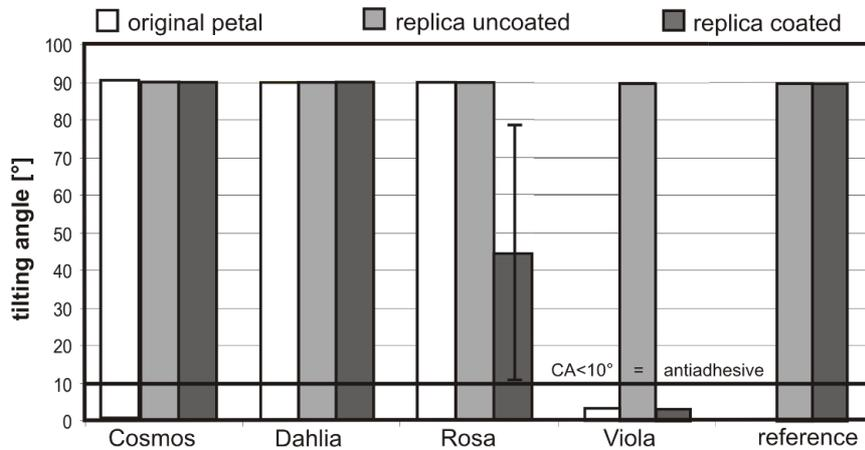
**Figure 5:** TAs of 5  $\mu\text{l}$  water droplets on the surfaces of fresh (original) *Cosmos*, *Dahlia*, *Rosa* and *Viola* flowers, their uncoated and coated polymer replicas and the TA of the reference (uncoated and coated flat polymer;  $n = 10$ ).
