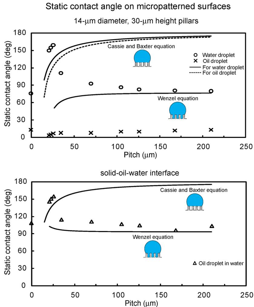
**Figure 15:** Static contact angle as a function of geometric parameters for water droplet (circle) and oil droplet (cross) in air (top), and oil droplet in water (triangle) (bottom) compared with predicted static contact angle values obtained using Wenzel and Cassie–Baxter equations (solid lines) with a measured value of  $\theta_0$  for the micropatterned surfaces [20].
