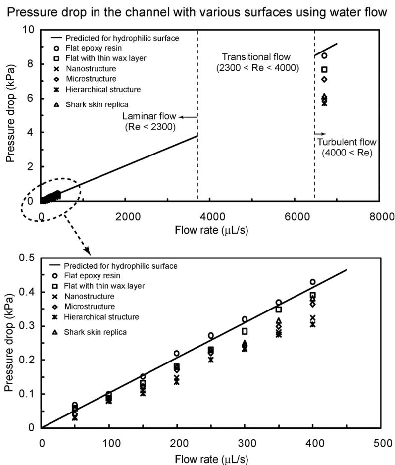
**Figure 6:** Pressure drop as a function of flow rate in the channel with various surfaces using water flow. The figure in the bottom is magnified in flow rate between 0 and 500  $\mu\text{L/s}$ . Data are compared with predicted pressure drop values for a hydrophilic surface obtained using Equation 1 for laminar and turbulent flows (solid lines) [21].
