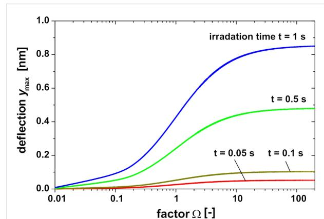
**Figure 5:** Maximum central deflection  $y_{\max}$  of a circular membrane as function of factor  $\Omega$  and irradiation time for a water-filled cavity. IR power density =  $10 \text{ W/m}^2$ , diameter and height of the cavity =  $0.5 \text{ mm}$ .
