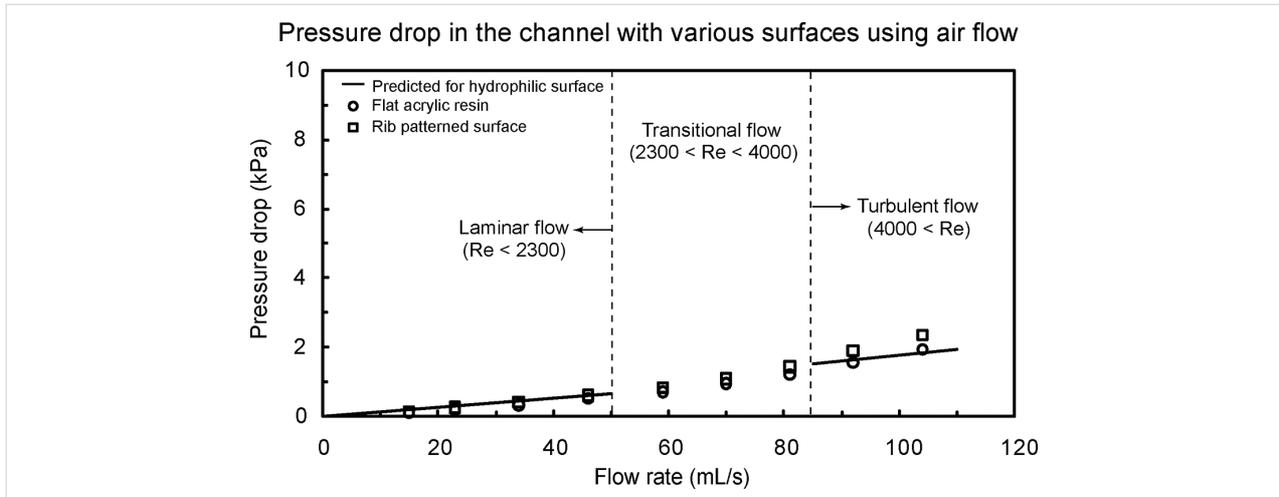
**Figure 10:** Pressure drop as a function of flow rate in the channel with flat acrylic resin and rib-patterned surface using air flow. Data are compared with predicted pressure drop values for a hydrophilic surface obtained using Equation 1 for laminar and turbulent flows (solid lines) [21].
