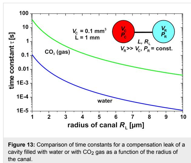
**Figure 13:** Comparison of time constants for a compensation leak of a cavity filled with water or with  $\text{CO}_2$  gas as a function of the radius of the canal.
