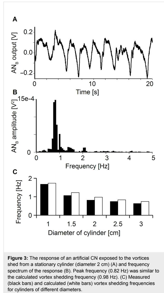
**Figure 3:** The response of an artificial CN exposed to the vortices shed from a stationary cylinder (diameter 2 cm) (A) and frequency spectrum of the response (B). Peak frequency (0.82 Hz) was similar to the calculated vortex shedding frequency (0.98 Hz). (C) Measured (black bars) and calculated (white bars) vortex shedding frequencies for cylinders of different diameters.
