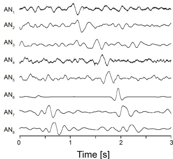
**Figure 5:** Responses of AN<sub>1</sub> to AN<sub>8</sub> (cf. Figure 6B) to bulk water flow. Note that the most prominent peak visible in the response of AN<sub>1</sub> is systematically delayed from AN<sub>1</sub> to AN<sub>8</sub>. The curves are not to scale due to the manual fabrication of each AN.
