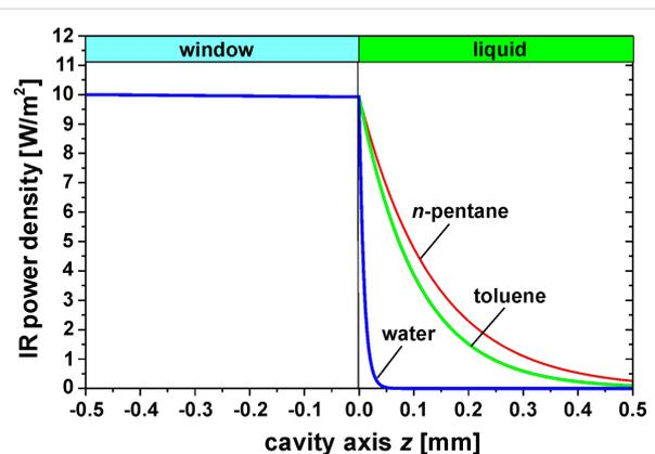
**Figure 6:** IR power density as function of the cavity axis for different liquids. Suprasil<sup>®</sup> 300 was used as the material for the window with an absorption coefficient of 0.16  $\text{cm}^{-1}$  [23]. For gas, a thin absorbing film on the inner glass surface is assumed where all the radiation is absorbed.
