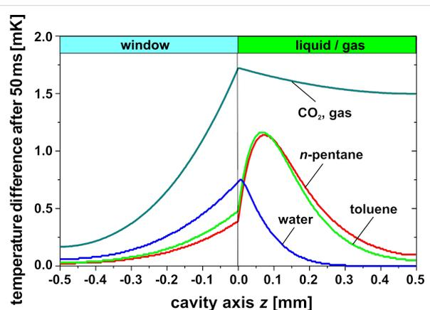
**Figure 7:** Temperature distribution along the cavity axis 50 ms after the onset of irradiation for different liquids with an IR power density at the outer window surface of 10  $\text{W}/\text{m}^2$ , see Figure 6.
