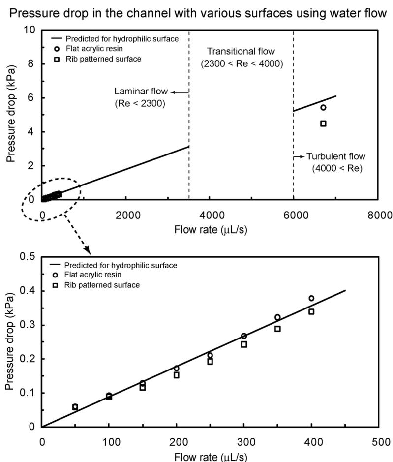
**Figure 8:** Pressure drop as a function of flow rate in the channel with flat acrylic resin and rib-patterned surface using water flow. The figure in the bottom is magnified for flow rate between 0 and 500  $\mu\text{L/s}$ . Data are compared with predicted pressure drop values for a hydrophilic surface obtained using Equation 1 for laminar and turbulent flows (solid lines) [21].
