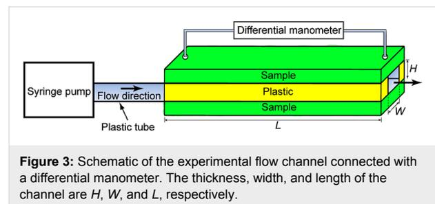
**Figure 3:** Schematic of the experimental flow channel connected with a differential manometer. The thickness, width, and length of the channel are  $H$ ,  $W$ , and  $L$ , respectively.
