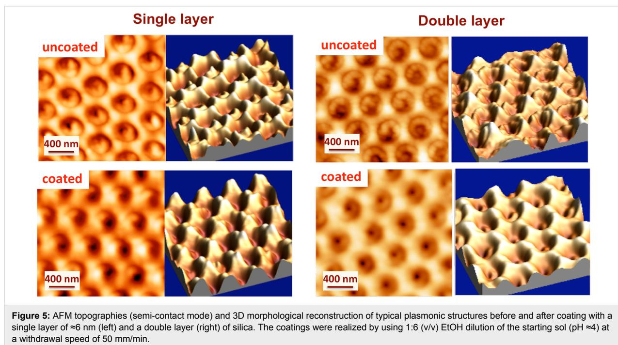
reported in Figure 5 show the topography and the 3D morphological reconstruction of typical plasmonic structures before and after coating. A regular deposition of the pillars, with a hexagonal lattice structure, is clearly observed. Similar images were obtained for samples coated with layers of different thicknesses.
