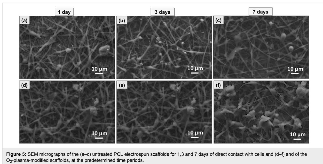
**Figure 5:** SEM micrographs of the (a–c) untreated PCL electrospun scaffolds for 1,3 and 7 days of direct contact with cells and (d–f) and of the O<sub>2</sub>-plasma-modified scaffolds, at the predetermined time periods.
