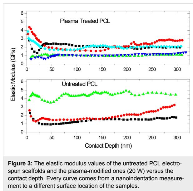
**Figure 3:** The elastic modulus values of the untreated PCL electrospun scaffolds and the plasma-modified ones (20 W) versus the contact depth. Every curve comes from a nanoindentation measurement to a different surface location of the samples.
