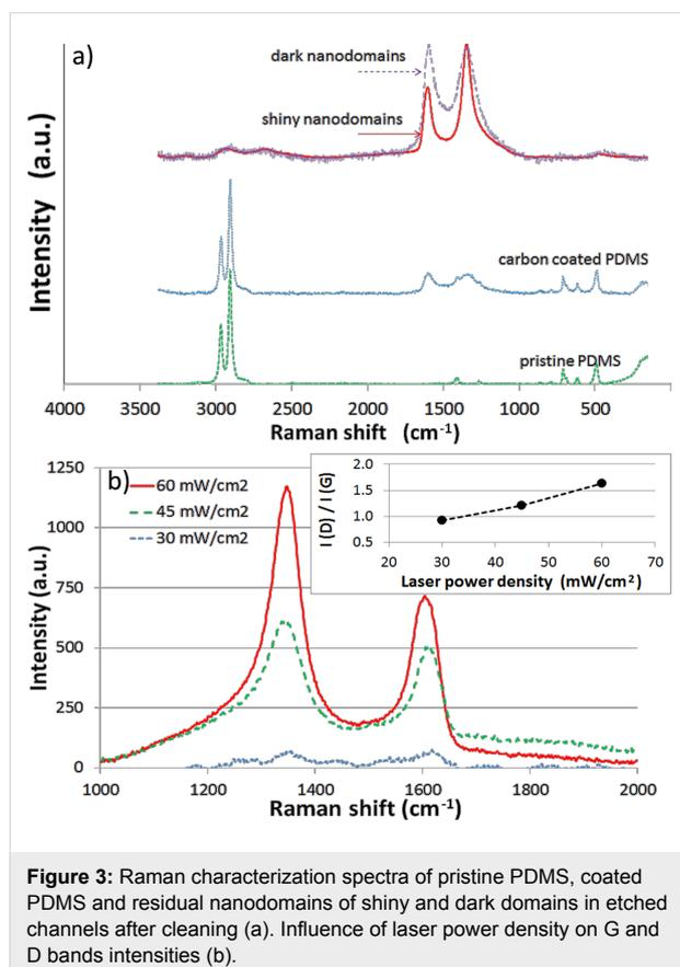
**Figure 3:** Raman characterization spectra of pristine PDMS, coated PDMS and residual nanodomains of shiny and dark domains in etched channels after cleaning (a). Influence of laser power density on G and D bands intensities (b).
