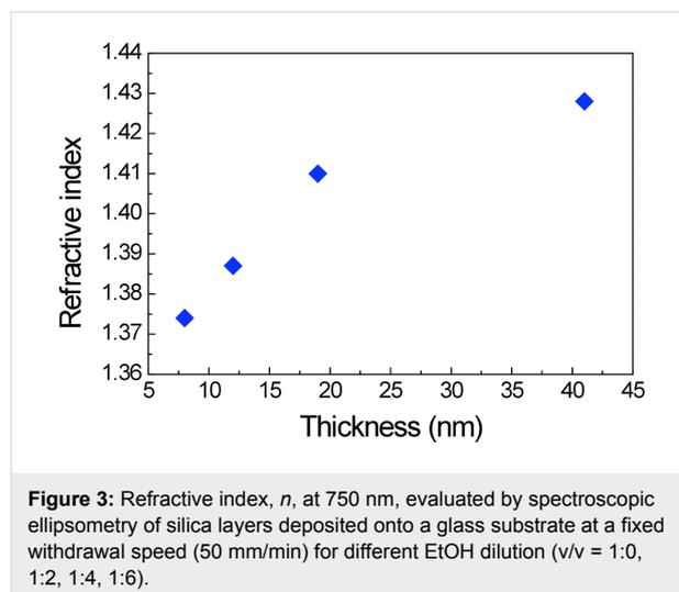
**Figure 3:** Refractive index,  $n$ , at 750 nm, evaluated by spectroscopic ellipsometry of silica layers deposited onto a glass substrate at a fixed withdrawal speed (50 mm/min) for different EtOH dilution (v/v = 1:0, 1:2, 1:4, 1:6).
