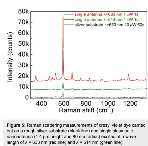
Comparing the spectrum obtained on the antenna at  $\lambda = 633$  nm (red line in Figure 5) with that on the substrate (black line in Figure 5), it is evident that the magnification of the Raman signals attributed to the antennas is much stronger than that of the silver film, thus confirming the effective capability of the hotspot at the antenna tip to act as field enhancer.
