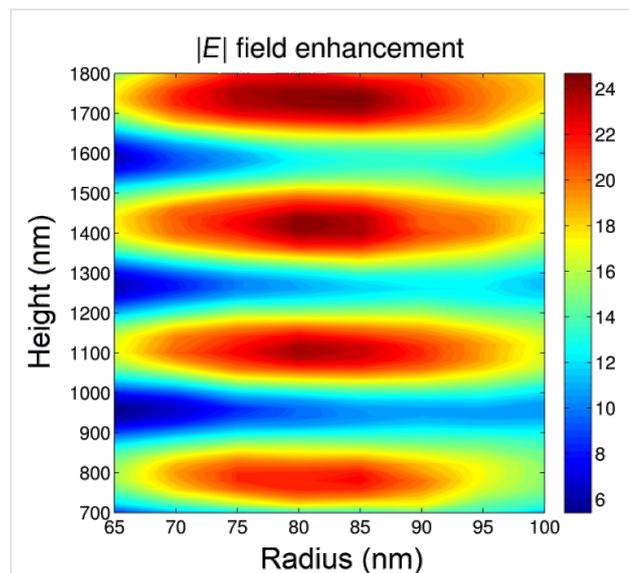
**Figure 2:** Electric field amplitude of silver antennas as a function of height and external radius. The maximum value of the field enhancement was found at an excitation wavelength of  $\lambda = 630$  nm for  $H = 1400$  and  $R = 80$  nm.
