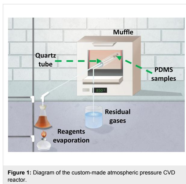
**Figure 1:** Diagram of the custom-made atmospheric pressure CVD reactor.
