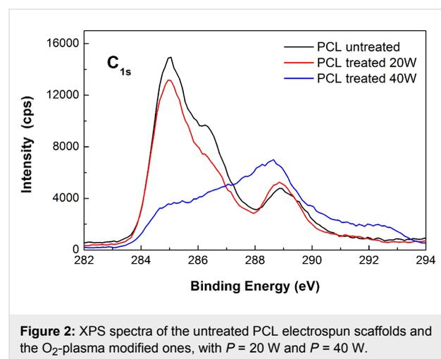
**Figure 2:** XPS spectra of the untreated PCL electrospun scaffolds and the  $O_2$ -plasma modified ones, with  $P = 20$  W and  $P = 40$  W.
