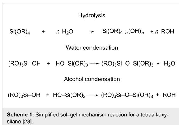
Many processing parameters can affect the rate of hydrolysis and condensation, and thus, the features of the final material. Previous studies have reported the dependence of the sol–gel film thickness on the withdrawal speed, water:precursor molar ratio, and aging time [26,28–31]. However, all processing parameters must be controlled to carefully optimize the deposition
