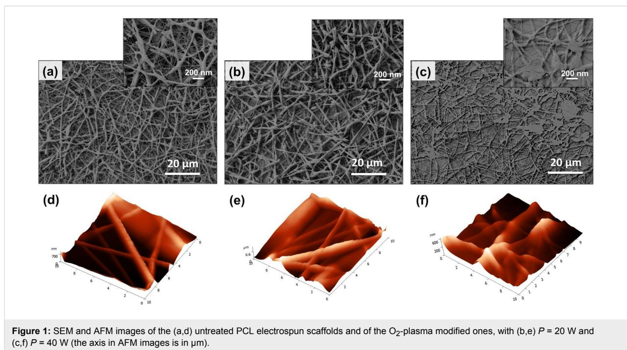
**Figure 1:** SEM and AFM images of the (a,d) untreated PCL electrospun scaffolds and of the  $O_2$ -plasma modified ones, with (b,e)  $P = 20$  W and (c,f)  $P = 40$  W (the axis in AFM images is in  $\mu\text{m}$ ).
