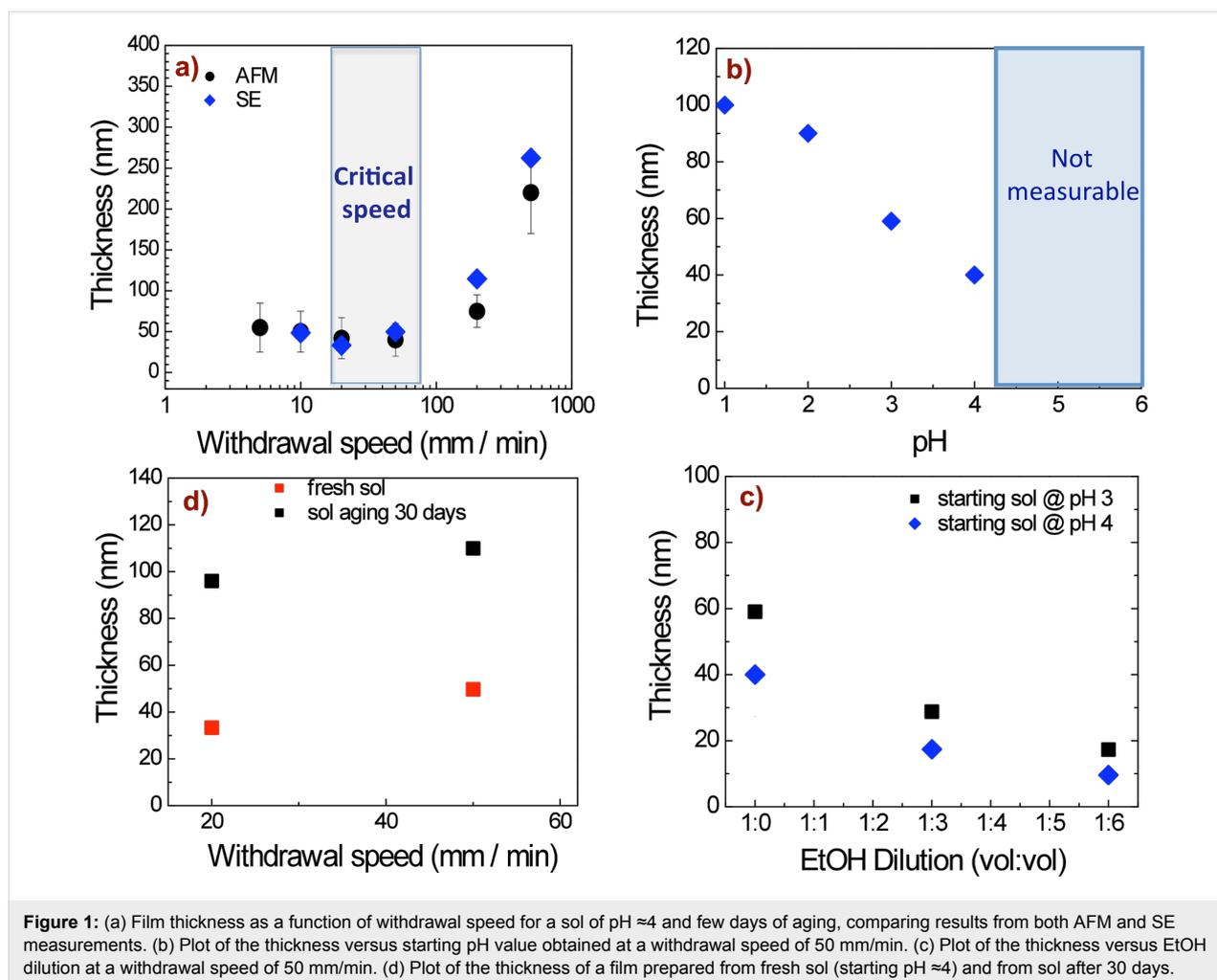
the withdrawal speed fixed (50 mm/min), while using different starting pH values. A decrease in the thickness with increasing pH (until pH 4) can be observed. These results highlight that film thickness is strongly affected by pH. From the literature [28–31] it is known that the pH value affects the hydrolysis and condensation processes, and thus, it influences the morphology and structure of the resulting final material.
