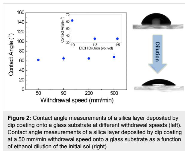
**Figure 2:** Contact angle measurements of a silica layer deposited by dip coating onto a glass substrate at different withdrawal speeds (left). Contact angle measurements of a silica layer deposited by dip coating at a 50 mm/min withdrawal speed onto a glass substrate as a function of ethanol dilution of the initial sol (right).
