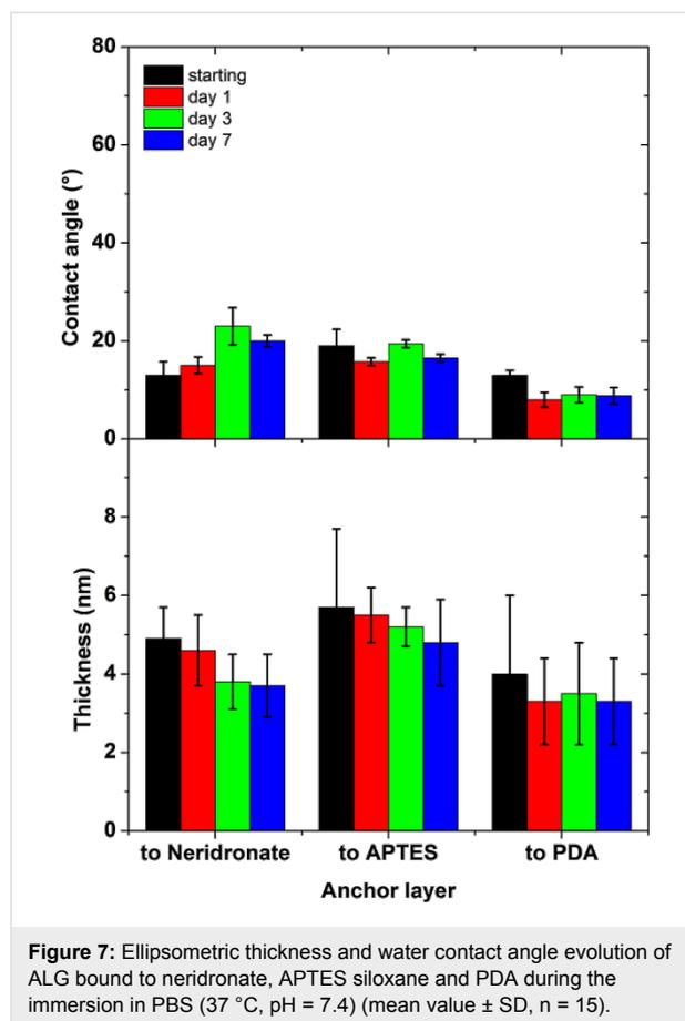
**Figure 7:** Ellipsometric thickness and water contact angle evolution of ALG bound to neridronate, APTES siloxane and PDA during the immersion in PBS (37 °C, pH = 7.4) (mean value  $\pm$  SD, n = 15).
