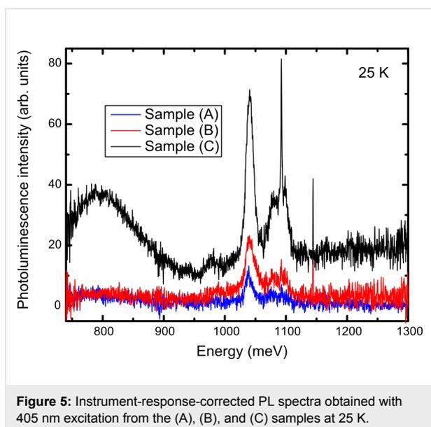
**Figure 5:** Instrument-response-corrected PL spectra obtained with 405 nm excitation from the (A), (B), and (C) samples at 25 K.
