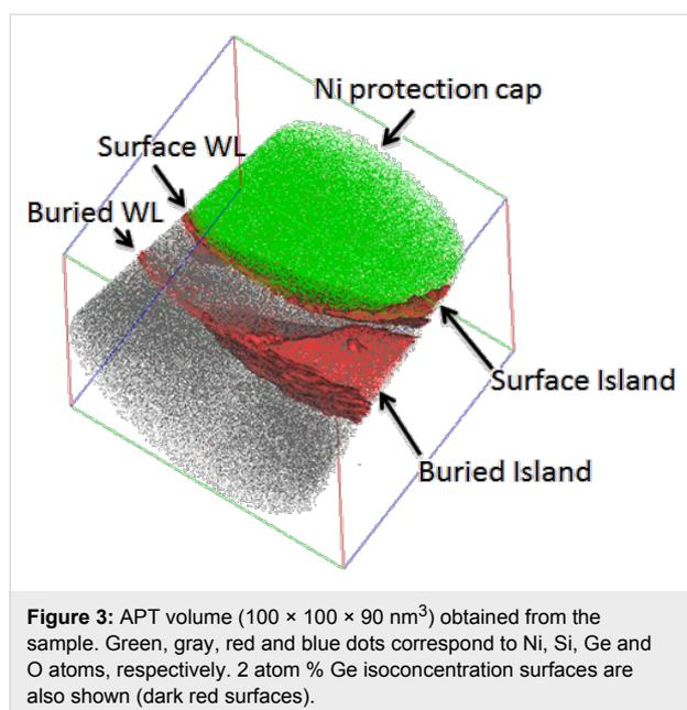
**Figure 3:** APT volume ( $100 \times 100 \times 90 \text{ nm}^3$ ) obtained from the sample. Green, gray, red and blue dots correspond to Ni, Si, Ge and O atoms, respectively. 2 atom % Ge isoconcentration surfaces are also shown (dark red surfaces).
