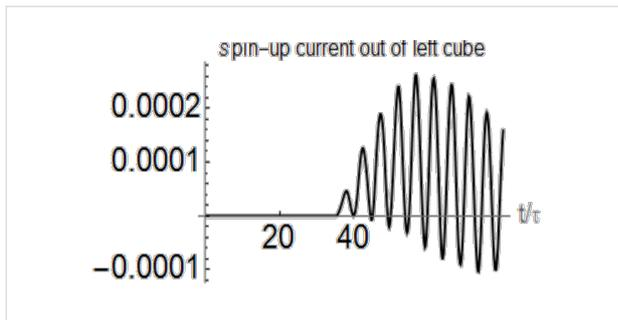
**Figure 5:** Spin-up current from the left storage cube in the cube–cube connection, when both storage cubes have eight sites. The hopping integral in the cube–cube wire is  $t_{\text{ext}} = 0.05 t_h$ . The spin-down current is opposite.
