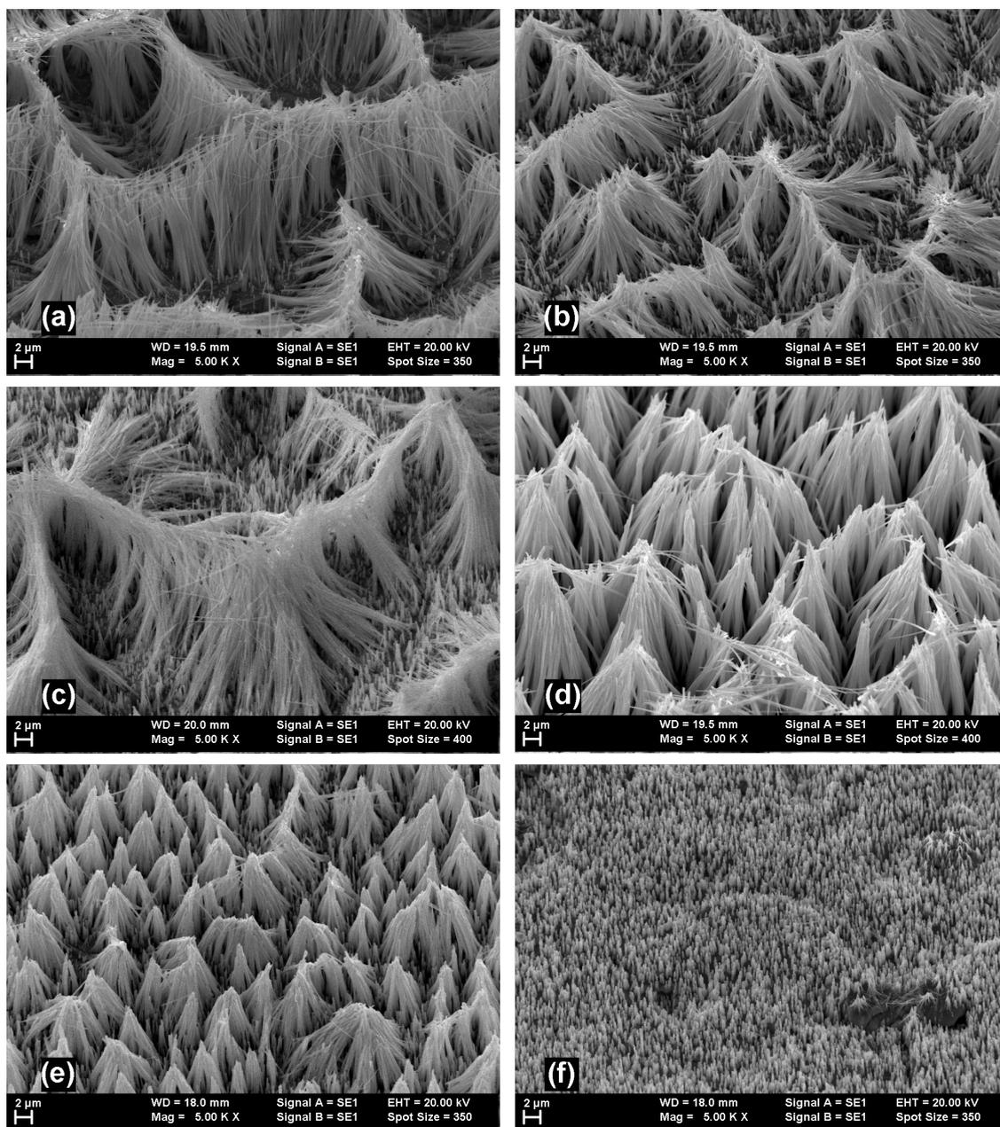
**Figure 1:** SEM micrographs of CdTe nanowires deposited at (a)  $-400$  mV; (b)  $-500$  mV; (c)  $-550$  mV; (d)  $-600$  mV; (e)  $-650$  mV; (f)  $-700$  mV.
