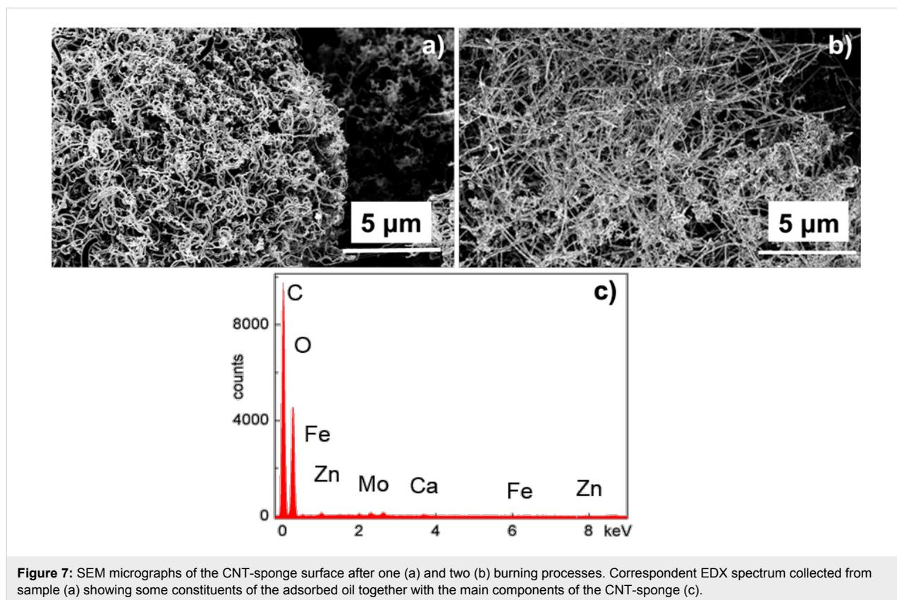
**Figure 7:** SEM micrographs of the CNT-sponge surface after one (a) and two (b) burning processes. Correspondent EDX spectrum collected from sample (a) showing some constituents of the adsorbed oil together with the main components of the CNT-sponge (c).
