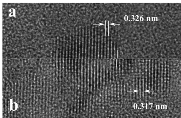
**Figure 10:** High-resolution TEM images comparing details of the initial crystallized particle (a) and the same area of the particle after the crystal growth process (b). The lattice fringe spacing in panel (b) is smaller than that in panel (a).
