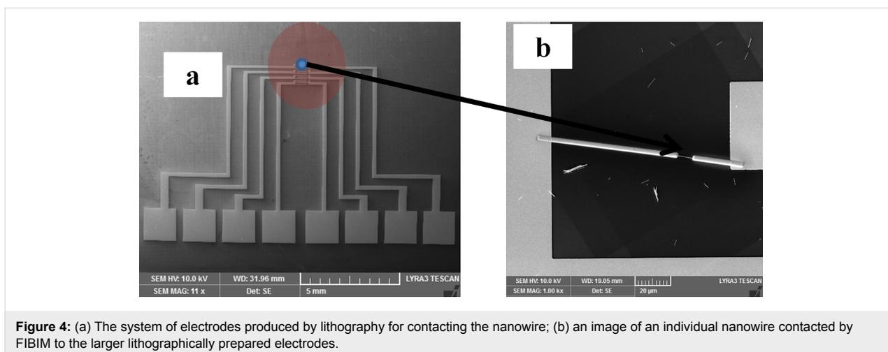
**Figure 4:** (a) The system of electrodes produced by lithography for contacting the nanowire; (b) an image of an individual nanowire contacted by FIBIM to the larger lithographically prepared electrodes.
