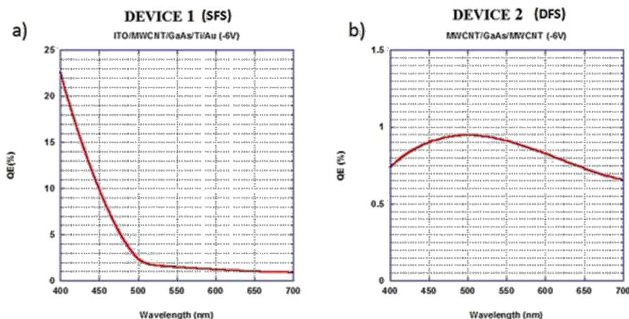
**Figure 5:** Absolute quantum efficiency trend in the visible light range, calculated at a bias voltage of  $-6$  V for the devices SFS a) and DFS b).
