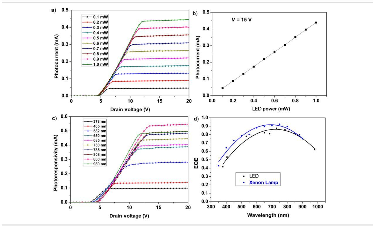
**Figure 5:** (a) Photocurrent induced by a 730 nm continuous wave, low power light source at various illumination intensities. (b) Photocurrent linearity at a drain voltage 15 V and wavelength of 730 nm. (c) Photocurrent induced at different wavelengths. (d) Comparison between the device external quantum efficiency (EQE) measured with an LD and a xenon lamp, filtered at different wavelengths.
