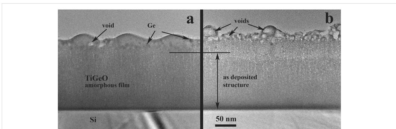
**Figure 3:** XTEM images of the amorphous GeTiO RF film after laser irradiation with 266 nm laser radiation. (a) Low fluence (15 mJ/cm<sup>2</sup>) and (b) higher laser fluence (20 mJ/cm<sup>2</sup>). The film structure morphology is transformed in a depth of about 50 nm.
