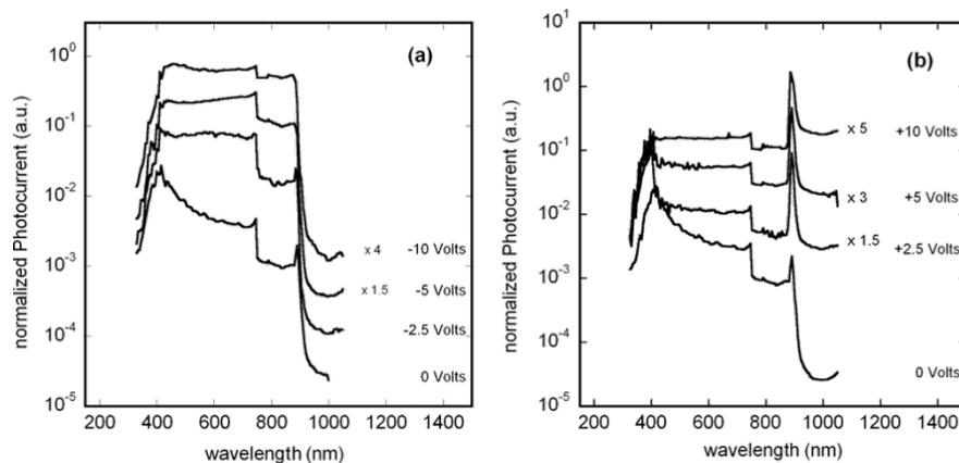
**Figure 8:** Normalized photocurrent spectra measured at: (a) negative voltages, (b) positive voltages applied to the ITO top contact with respect to the bottom Ti/Au contact. For the sake of clarity, some spectra were shifted up in the plots multiplying them by a factor, as indicated in the figure. The step shown in all the spectra at 750 nm is due to the change of the gratings of the monochromator.
