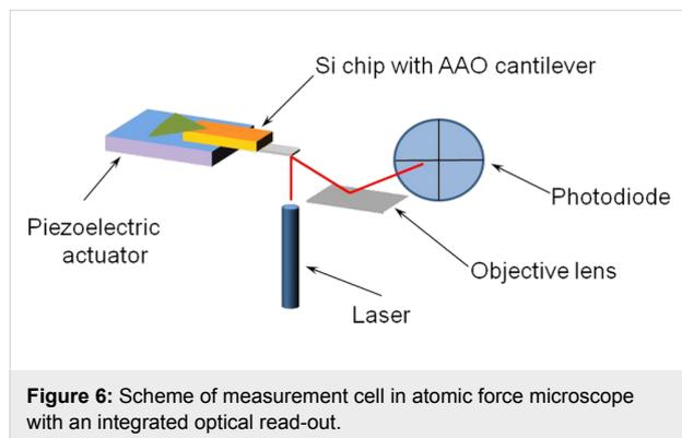
**Figure 6:** Scheme of measurement cell in atomic force microscope with an integrated optical read-out.
