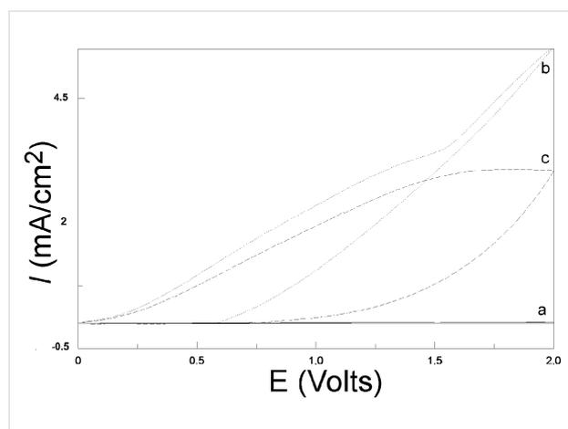
**Figure 7:** CVs of PEDOT deposition on SiNWs under various conditions. Scan rate: 100 mV/s. (a) 10 mM EDOT with 0.1 M  $\text{LiClO}_4$  in acetonitrile solution, without illumination; (b) 10 mM EDOT with 0.1 M  $\text{LiClO}_4$  in acetonitrile solution, under illumination; (c) 0.1 M  $\text{LiClO}_4$  in acetonitrile solution, under illumination.
