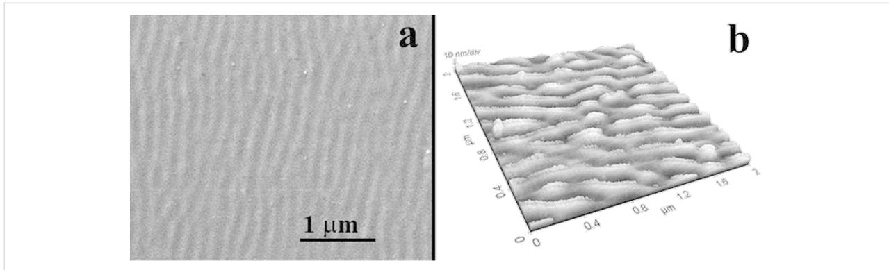
**Figure 1:** Surface relief of the GeTiO film after laser irradiation with 100 laser pulses at 15 mJ/cm<sup>2</sup> fluence. (a) SEM image and (b) AFM image.
