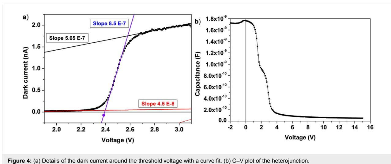
Figure 4: (a) Details of the dark current around the threshold voltage with a curve fit. (b) C–V plot of the heterojunction.
