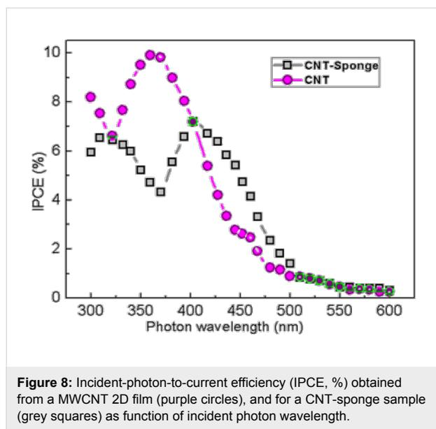
**Figure 8:** Incident-photon-to-current efficiency (IPCE, %) obtained from a MWCNT 2D film (purple circles), and for a CNT-sponge sample (grey squares) as function of incident photon wavelength.
