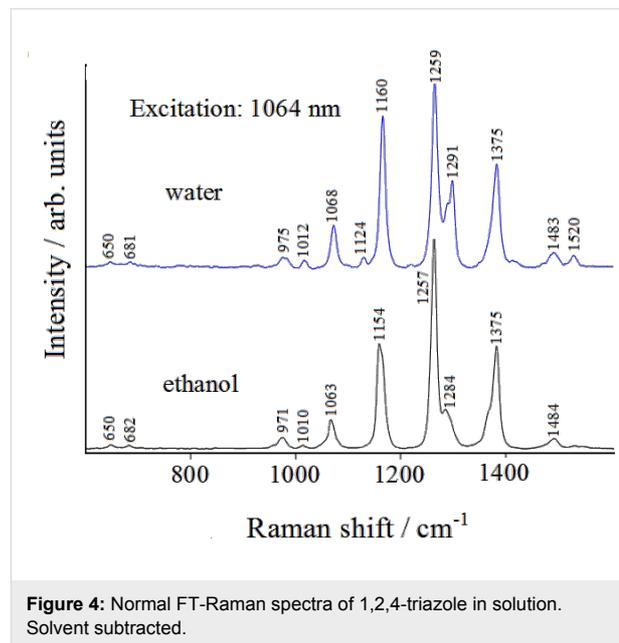
**Figure 4:** Normal FT-Raman spectra of 1,2,4-triazole in solution. Solvent subtracted.
