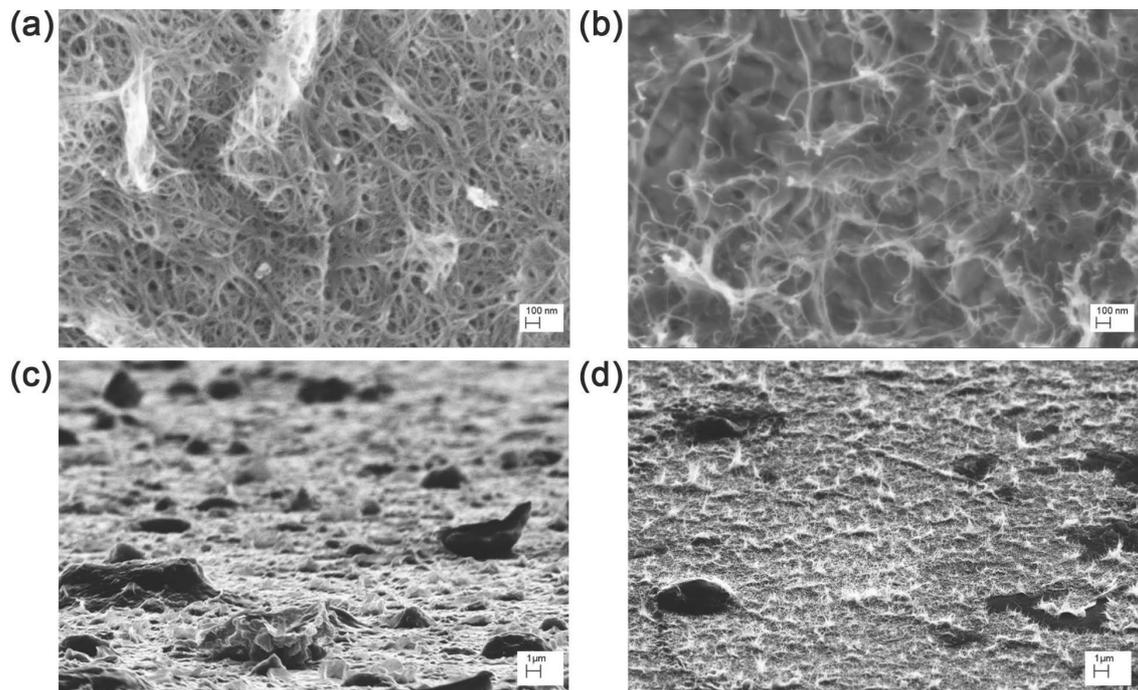
**Figure 1:** Scanning electron micrographs of SWCNT (a,c) and MWCNT (b,d) films at different magnifications 200,000 $\times$  (a,b), and 10,000 $\times$  (c,d). In the images taken at grazing incidence (c,d) it is possible to observe that SWCNTs (c) self-assemble in ripples forming several microstructures, while MWCNTs (d) just aligned in the out-of-plane vertical direction. (d) Black areas are holes in the film.
