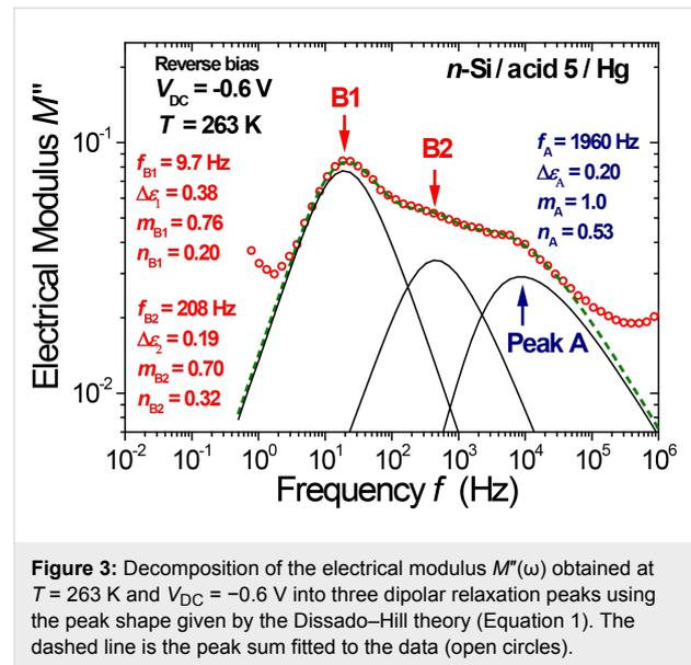
**Figure 3:** Decomposition of the electrical modulus  $M''(\omega)$  obtained at  $T = 263$  K and  $V_{\text{DC}} = -0.6$  V into three dipolar relaxation peaks using the peak shape given by the Dissado–Hill theory (Equation 1). The dashed line is the peak sum fitted to the data (open circles).
