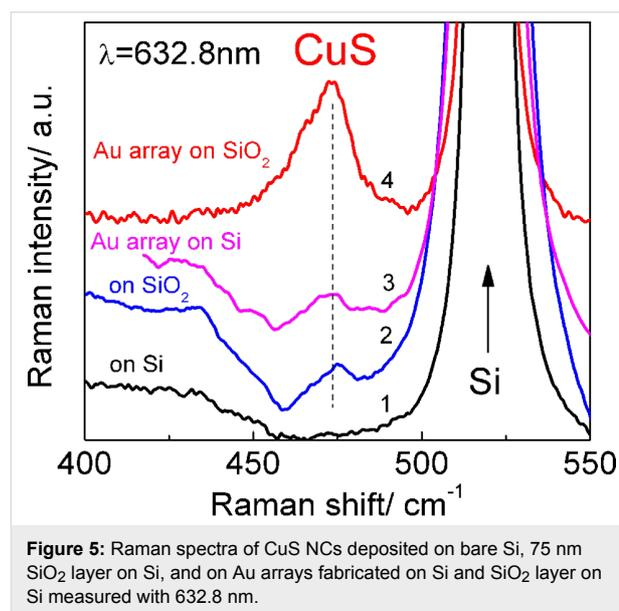
**Figure 5:** Raman spectra of CuS NCs deposited on bare Si,  $75\text{ nm}$   $\text{SiO}_2$  layer on Si, and on Au arrays fabricated on Si and  $\text{SiO}_2$  layer on Si measured with  $632.8\text{ nm}$ .
