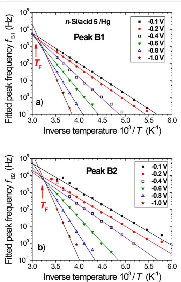
**Figure 4:** Temperature dependence of the dipolar relaxation frequencies  $f_{B1}$  (a) and  $f_{B2}$  (b) obtained for the Hg/acid 5/n-type Si junction at different reverse bias values ( $V_{DC}$  range from  $-0.1$  V to  $-1.0$  V). The lines are Arrhenius fits to the data, showing the existence of a “focal point” near  $T_F \approx 320$  K.
