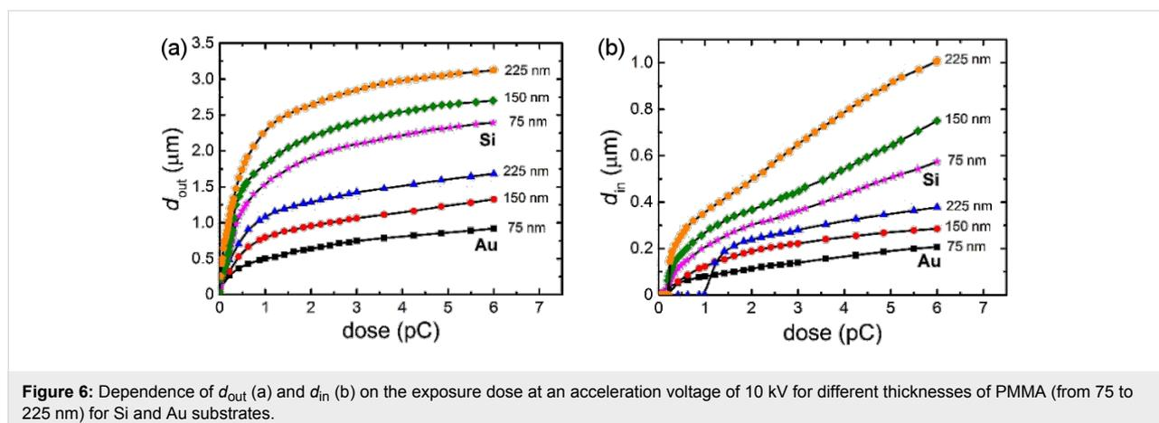
**Figure 6:** Dependence of  $d_{\text{out}}$  (a) and  $d_{\text{in}}$  (b) on the exposure dose at an acceleration voltage of 10 kV for different thicknesses of PMMA (from 75 to 225 nm) for Si and Au substrates.
