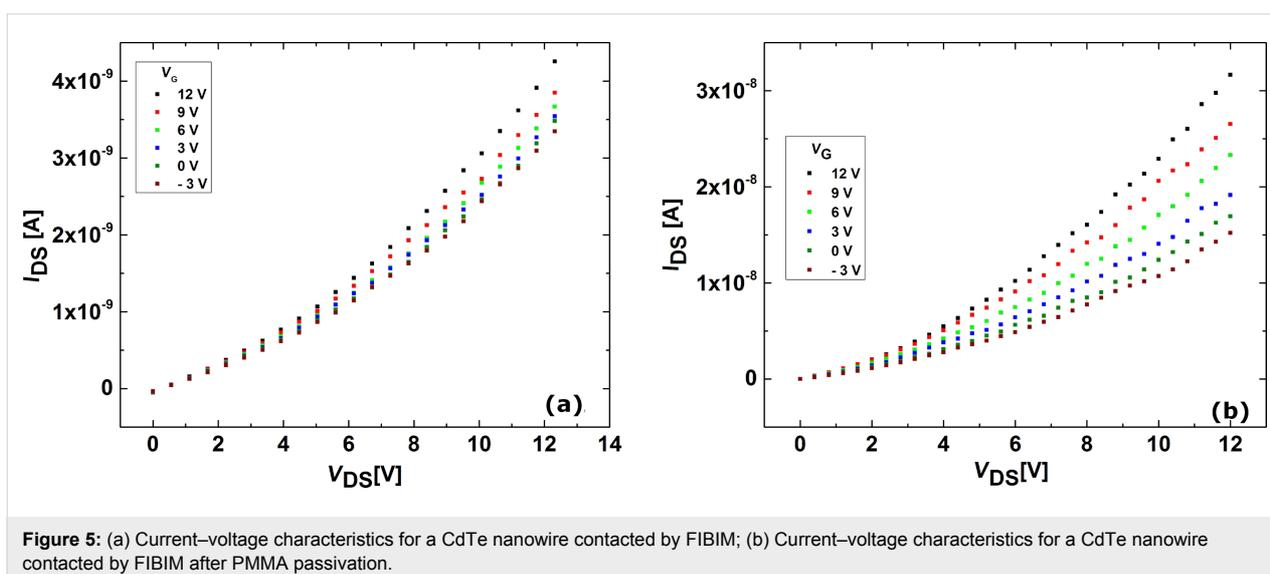
**Figure 5:** (a) Current–voltage characteristics for a CdTe nanowire contacted by FIBIM; (b) Current–voltage characteristics for a CdTe nanowire contacted by FIBIM after PMMA passivation.
