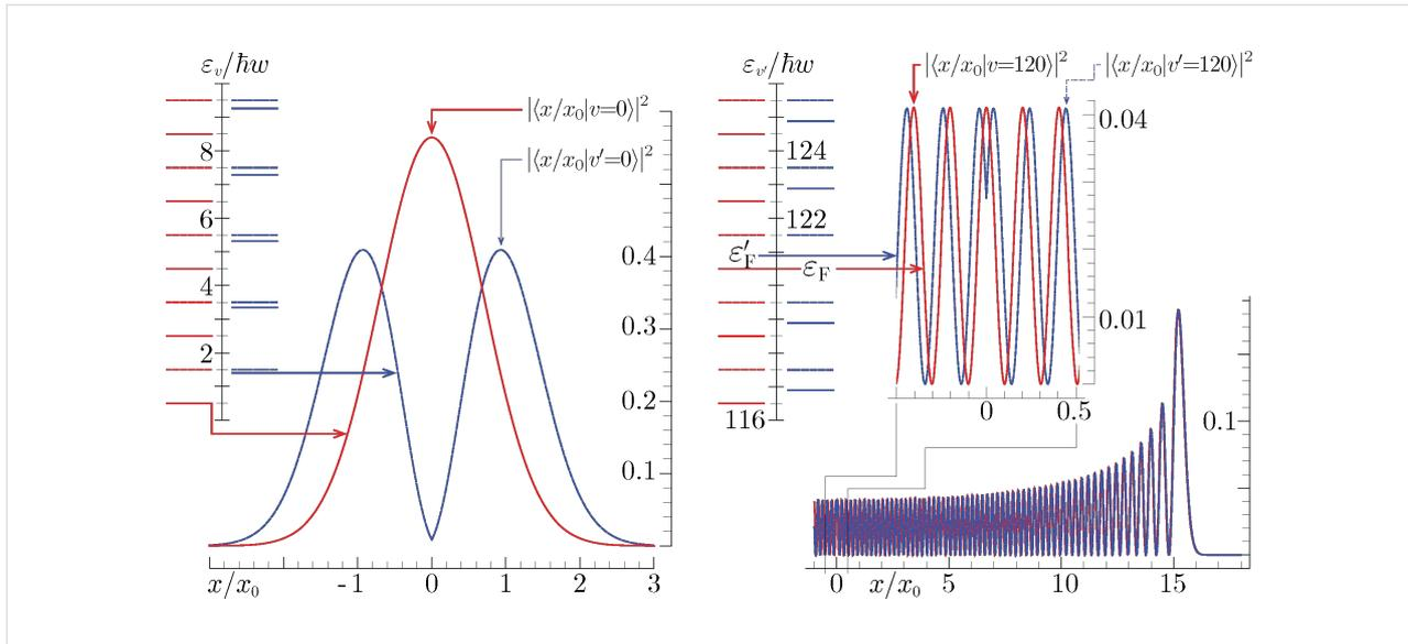
**Figure 4:** Lowest and highest occupied one-particle wave functions and levels for a harmonically trapped gas of  $N = 122$  fermions in absence and presence of the excited impurity, whose perturbation is characterized by the critical parameter  $\alpha = 0.1$  (see also Figure 3 and Table 2). The unperturbed and perturbed Fermi levels, relative to the lowest occupied one-particle state, are  $\varepsilon_F = 120.5\hbar\omega$  and  $\varepsilon'_F = 120.838\hbar\omega$ , respectively.
