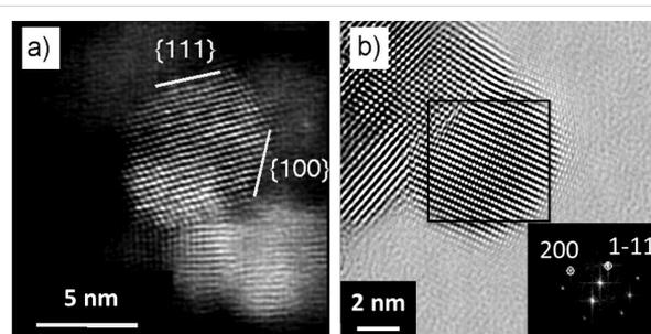
**Figure 3:** STEM (a) and HRTEM (b) images of ceria NPs corresponding to the sample with average diameter of 9 nm, the inset in (b) shows the FFT of the selected area with indicated the corresponding planes.
