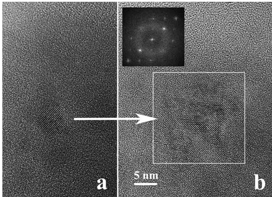
**Figure 9:** Crystallization (a) and subsequent crystal growth (b) of the Ge amorphous nanoparticle under the high density electron beam irradiation in the microscope. The FFT inserted in the (b) shows a pattern characteristic for the (GeTi)O<sub>2</sub> rutile structure.
