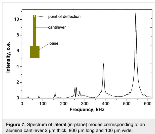
**Figure 7:** Spectrum of lateral (in-plane) modes corresponding to an alumina cantilever 2 μm thick, 800 μm long and 100 μm wide.
