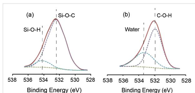
**Figure 4:** High-resolution XPS O 1s spectra of surfaces (a) thermally functionalized with ethynylbenzyl alcohol and (b) functionalized with ethynylbenzyl alcohol through UV irradiation.
