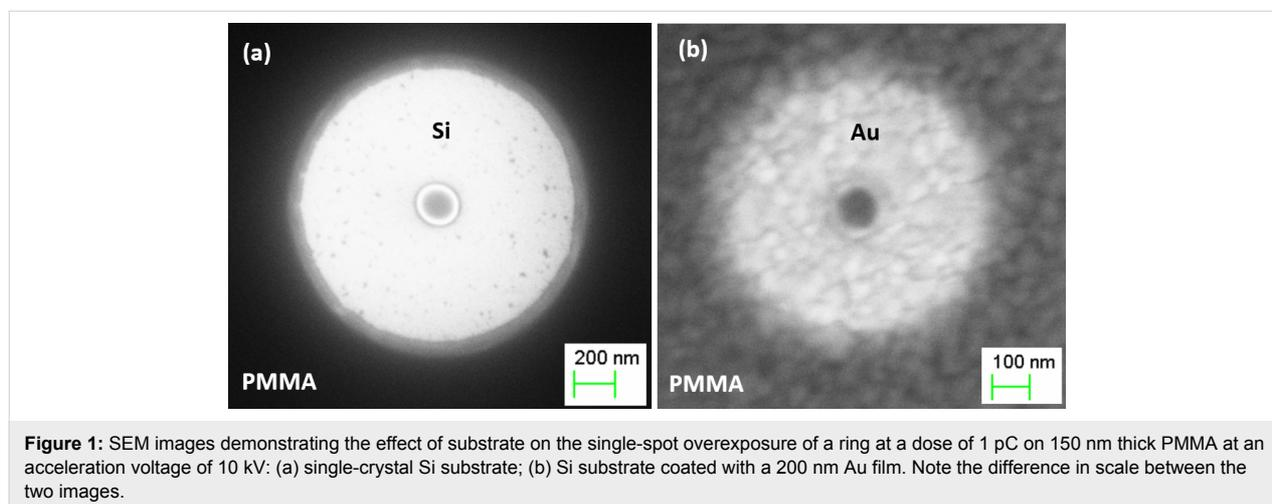
**Figure 1:** SEM images demonstrating the effect of substrate on the single-spot overexposure of a ring at a dose of 1 pC on 150 nm thick PMMA at an acceleration voltage of 10 kV: (a) single-crystal Si substrate; (b) Si substrate coated with a 200 nm Au film. Note the difference in scale between the two images.
