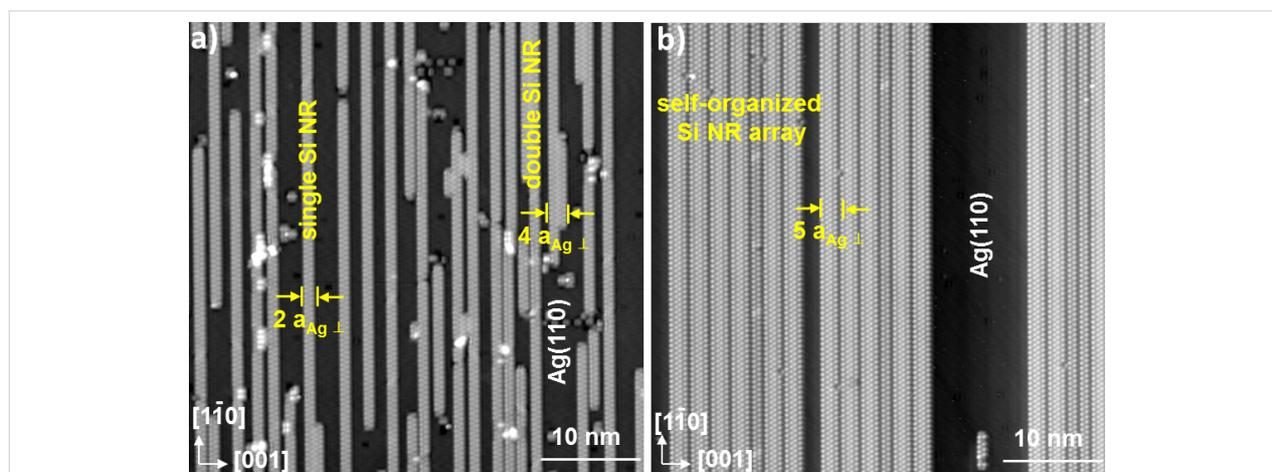
**Figure 1:** STM images recorded at 77 K at submonolayer Si coverage showing single and double Si nanoribbons (NRs) grown on Ag(110) upon Si deposition at (a)  $T_{\text{sub}} = \text{RT}$ ,  $I = 300$  pA,  $V_{\text{sample}} = 1$  V and (b)  $T_{\text{sub}} = 460$  K,  $I = 200$  pA,  $V_{\text{sample}} = 140$  mV. The pitch of the Si array is  $5 \cdot a_{\text{Ag}\perp}$  ( $a_{\text{Ag}\perp} = 0.409$  nm, the Ag(110) lattice parameter in the [001] direction).
