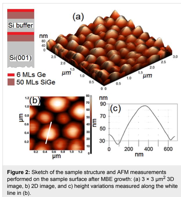
**Figure 2:** Sketch of the sample structure and AFM measurements performed on the sample surface after MBE growth: (a)  $3 \times 3 \mu\text{m}^2$  3D image, (b) 2D image, and (c) height variations measured along the white line in (b).
