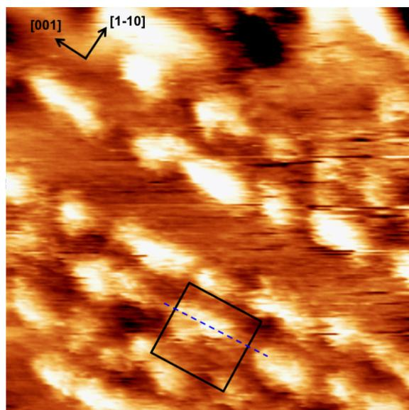
**Figure 3:** STM image in water of the  $\text{Ca}/\text{TiO}_2(110)$  surface after Ca segregation,  $27.3 \times 27.3$  nm<sup>2</sup>,  $V_{\text{bias}} = -1$  V,  $I_{\text{tunnel}} = 1$  nA. The alignment of the Ca-related rows with  $\text{TiO}_2(110)$  substrate rows (dashed, blue line) is highlighted by the black square.
