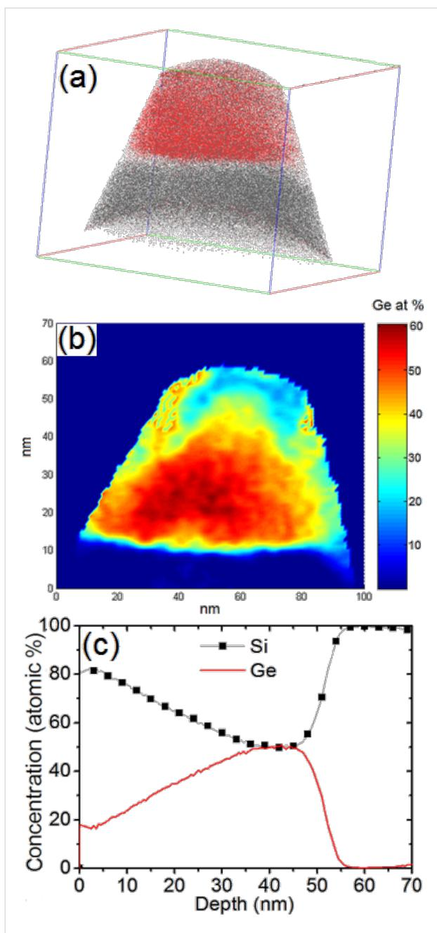
**Figure 8:** APT analysis: (a) 3D volume ( $120 \times 120 \times 100 \text{ nm}^3$ ), (b) 2D map of the Ge concentration distribution in the center of the volume presented in Figure 8a, and (c) top-down 1D Si and Ge concentration profiles measured in the volume presented in Figure 8a.
