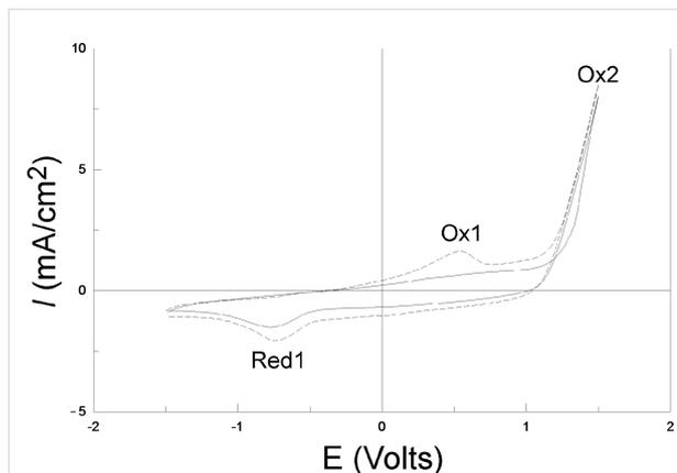
**Figure 4:** Two successive CVs performed on vitreous carbon with 10 mM EDOT and 0.1 M LiClO<sub>4</sub> in acetonitrile solution. Scan rate: 100 mV/s. The solid line corresponds to the 1st scan and the dashed line to the 2nd scan.
