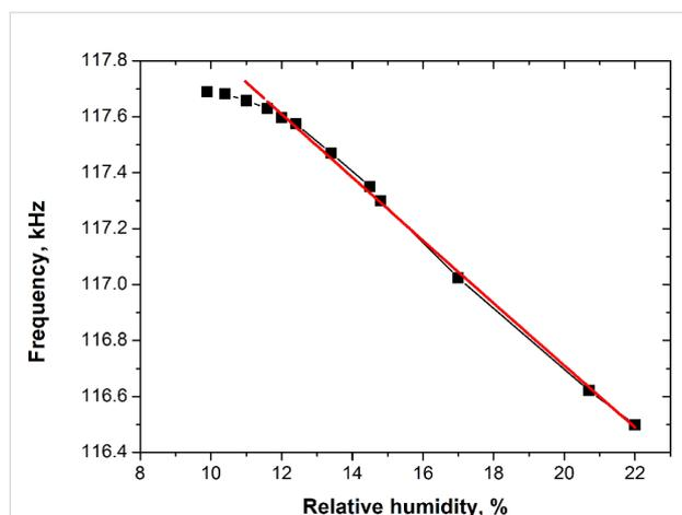
**Figure 4:** Resonance frequency of the AAO cantilevers (2  $\mu\text{m}$  thick, 800  $\mu\text{m}$  long and 100  $\mu\text{m}$  wide) as function of relative humidity from 10 to 22%. Red line: approximation of the linear part as  $f = 118.9972 \cdot (1 + 0.00198H)^{-1/2}$ . Inaccuracy of frequency detection is below the size of the symbols.
