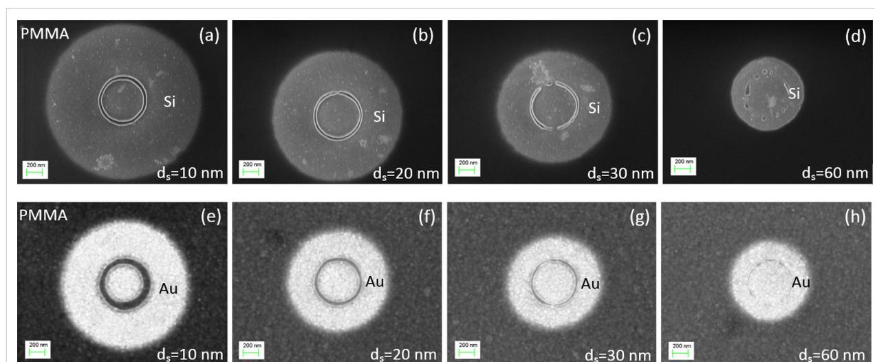
**Figure 7:** SEM images demonstrating the effect of changing the  $d_s$  between the electron beam spots with a dose of 0.1 pC on the formation of circles on Si (a–d) and Au (e–h) substrates coated with PMMA of 75 nm thickness at an acceleration voltage of 10 kV.
