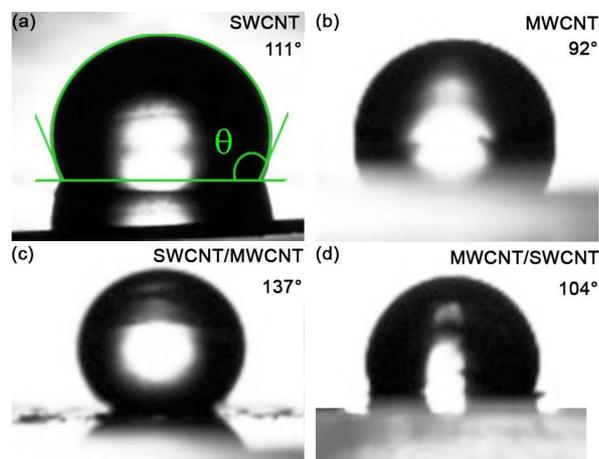
**Figure 3:** Water droplets cast on SWCNT (a), MWCNT (b), SWCNT/MWCNT (c), and MWCNT/SWCNT (d) films. Owing to the rough and porous surface of the samples, water drops exhibit different contact angle values, depending on the exact place at the surface on which they are cast. In this case, the contact angle can be only defined on average.
