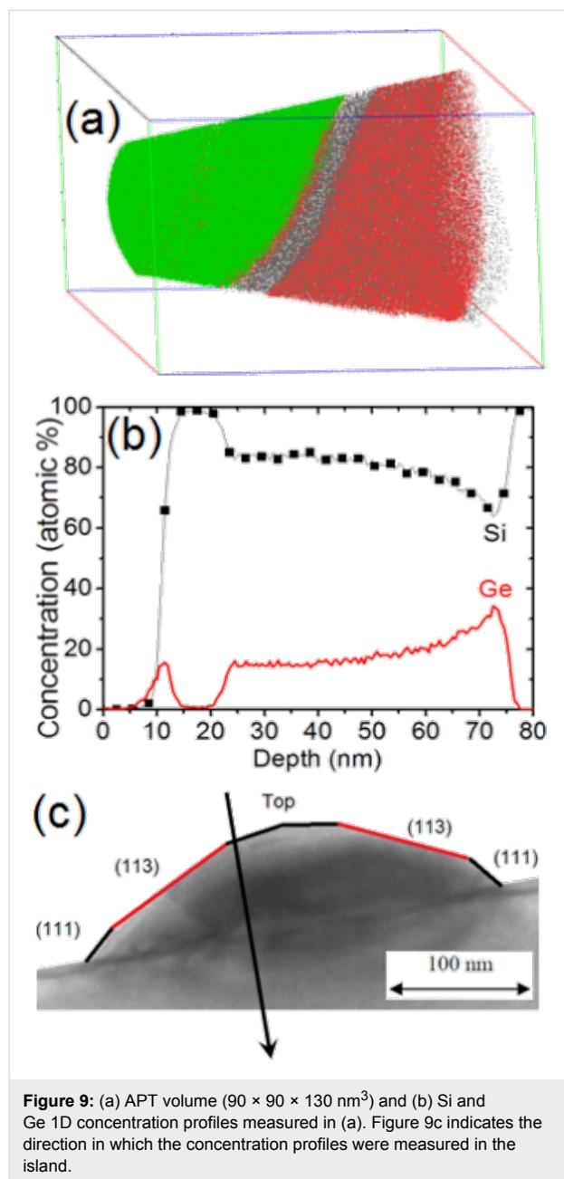
**Figure 9:** (a) APT volume ( $90 \times 90 \times 130 \text{ nm}^3$ ) and (b) Si and Ge 1D concentration profiles measured in (a). Figure 9c indicates the direction in which the concentration profiles were measured in the island.
