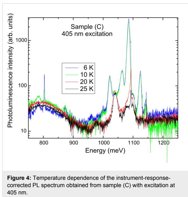
**Figure 4:** Temperature dependence of the instrument-response-corrected PL spectrum obtained from sample (C) with excitation at 405 nm.
