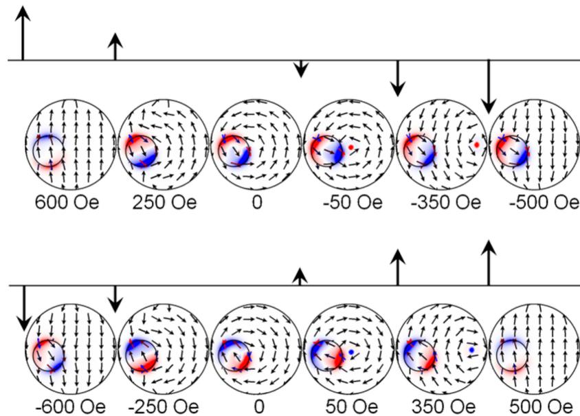
**Figure 5:** Spin configurations in the disk-on-disk nanostructure during the magnetization reversal under the applied magnetic field  $H$  oriented at  $\varphi \approx 90^\circ$ .
