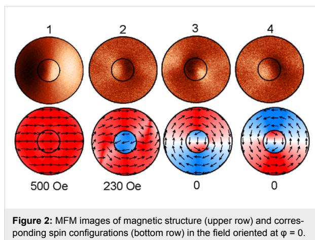
**Figure 2:** MFM images of magnetic structure (upper row) and corresponding spin configurations (bottom row) in the field oriented at  $\varphi = 0$ .
