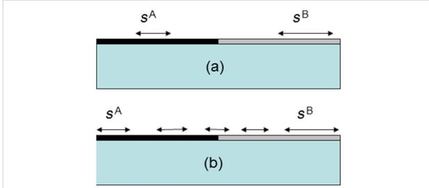
**Figure 1:** (a) Classical model in which each domain is characterized by its own supposedly constant surface stress. (b) When taking into account surface elasticity, the surface stress at mechanical equilibrium is no longer constant except far from the boundary.
