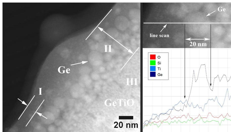
**Figure 5:** STEM-HAADF image (left) and a detail from the same image correlated with line scan EDX analyse (right) performed on the XTEM specimen prepared from the GeTiO film irradiated with 100 laser pulses at a fluence of  $15 \text{ mJ/cm}^2$ .
