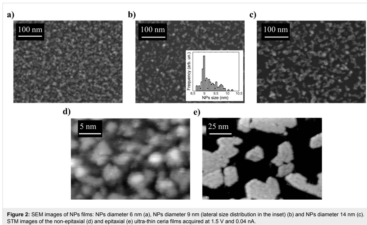
**Figure 2:** SEM images of NPs films: NPs diameter 6 nm (a), NPs diameter 9 nm (lateral size distribution in the inset) (b) and NPs diameter 14 nm (c). STM images of the non-epitaxial (d) and epitaxial (e) ultra-thin ceria films acquired at 1.5 V and 0.04 nA.
