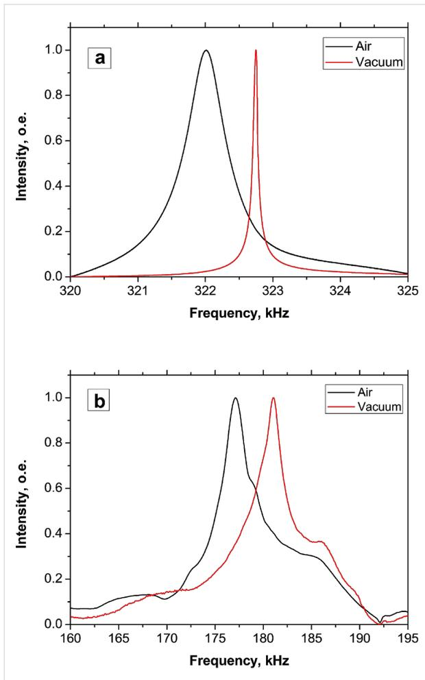
**Figure 2:** a) Frequency responses of Si rectangular cantilever (2  $\mu\text{m}$  thick, 100  $\mu\text{m}$  long and 30  $\mu\text{m}$  wide) in the air (black line) and in vacuum (red solid line). The frequency shift is 780 Hz. b) Frequency responses of AAO cantilever (2  $\mu\text{m}$  thick, 800  $\mu\text{m}$  long and 100  $\mu\text{m}$  wide) in the air (black line) and in vacuum (red solid line). The shift here is 3900 Hz.
