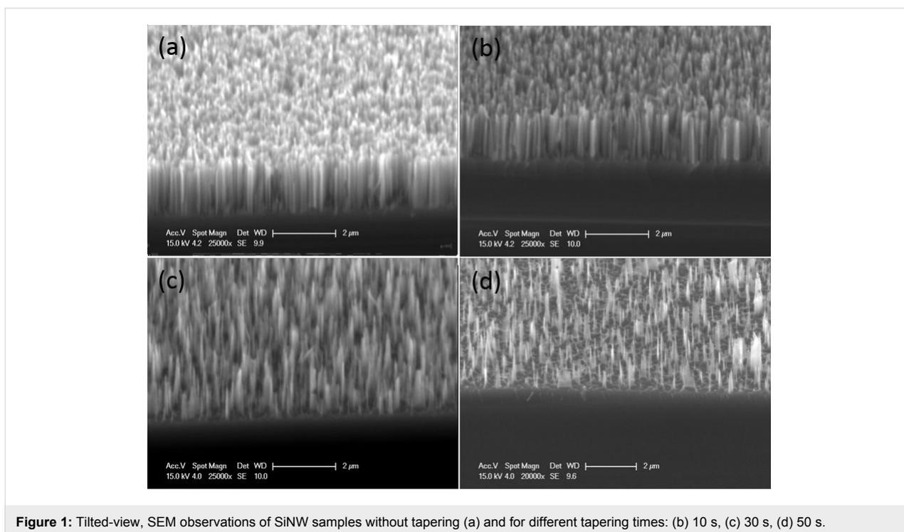
**Figure 1:** Tilted-view, SEM observations of SiNW samples without tapering (a) and for different tapering times: (b) 10 s, (c) 30 s, (d) 50 s.
