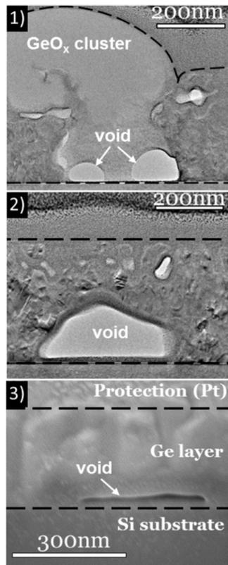
**Figure 4:** (1) and (2) TEM cross-sectional view of the Se-implanted sample after annealing with TB = 3.1  $\mu\text{m}$ . (3) SEM cross-sectional view of the Se-implanted sample after annealing with TB = 4.8  $\mu\text{m}$ .
