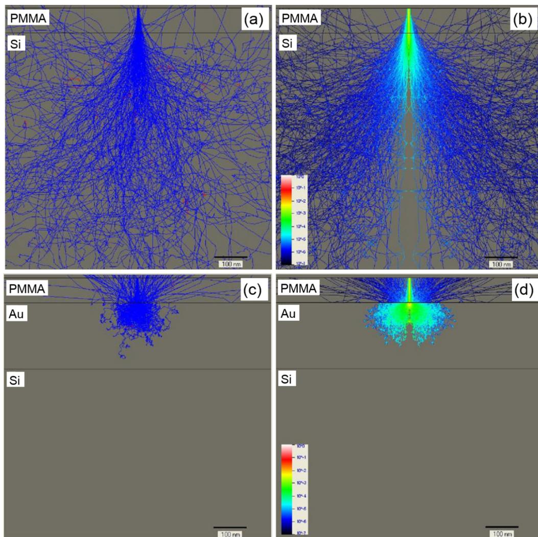
**Figure 4:** (a,c) Monte Carlo simulation of 250 electron scattering trajectories at 10 keV incident energy in a 75 nm thick PMMA layer on bulk Si and on 200 nm Au-coated substrates, respectively. (b,d) Electron energy distribution at 10 keV incident energy in a 75 nm thick PMMA layer on bulk Si and 200 nm Au-coated substrates, respectively. Trajectories that leave the sample represent backscattered electrons.
