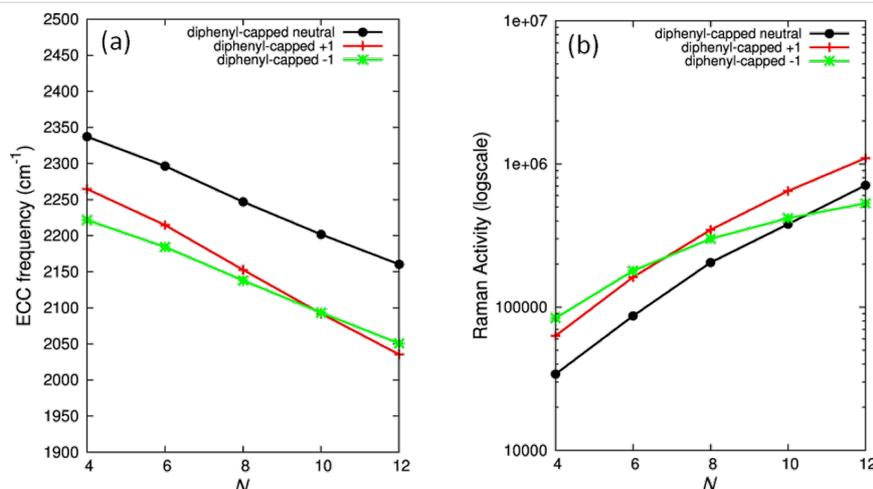
**Figure 7:** (a) Modulation of the DFT-computed [39] vibrational frequency and (b) Raman activity of the ECC band for phenyl-capped polyynes of different lengths ( $N$ ) and charge states (0, +1, -1). Figure adapted with permission from [39], copyright 2011 American Chemical Society.
