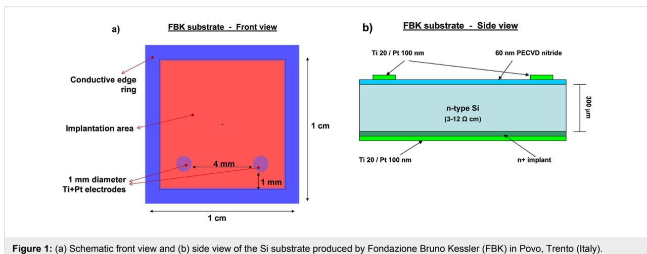
**Figure 1:** (a) Schematic front view and (b) side view of the Si substrate produced by Fondazione Bruno Kessler (FBK) in Povo, Trento (Italy).
