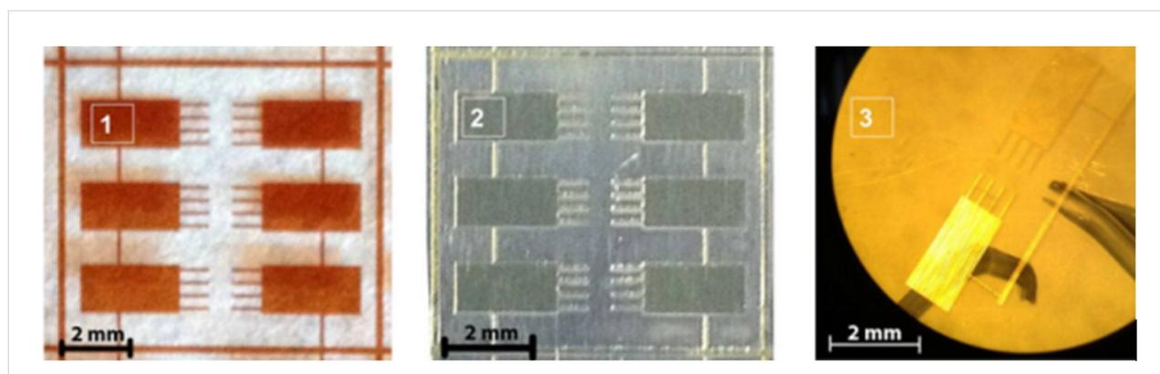
**Figure 5:** Photomask (1); cantilever arrays as formed on Al-foil (2); free-standing anodic alumina cantilevers (3).
