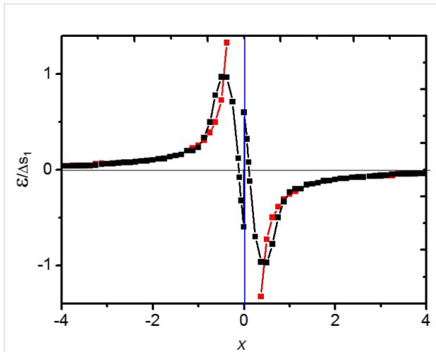
**Figure 4:** Black squares: normalised strain  $\varepsilon/\Delta s_1$  solution of Equation 8 calculated for  $\Delta s_1/S_{11} = 0.5$ , red squares: classical solution plotted from Equation 2. (arbitrary units, vertical blue line corresponds to the location of the ribbons edges sketched in grey in the upper part of the figures).
