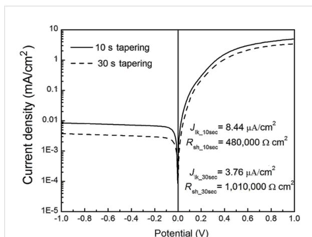
**Figure 14:** Current–potential characterization of the diodes with SiNW arrays tapered for 10 s (solid line) and 30 s (dashed line).
