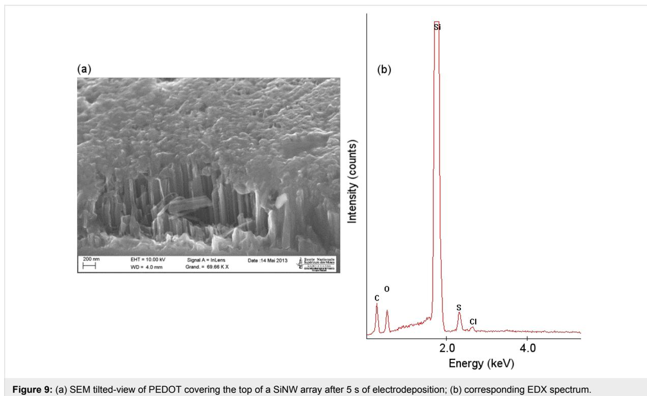
**Figure 9:** (a) SEM tilted-view of PEDOT covering the top of a SiNW array after 5 s of electrodeposition; (b) corresponding EDX spectrum.
