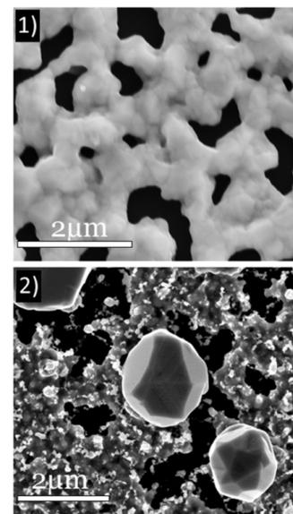
**Figure 5:** SEM plan-view image obtained after annealing a 340 nm thick Ge layer sputtered on the native Si oxide of a Si(001) substrate: (1) without implantation and TB = 0.64  $\mu\text{m}$ ; and (2) with Se implantation and TB = 8.7  $\mu\text{m}$ .
