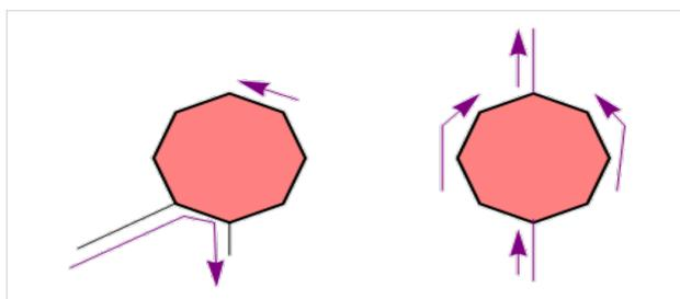
**Figure 1:** Left: Lateral connection of a quantum ring ( $N_{\text{ring}} = 8$ ) to external wires (any even number of sides greater or equal than four can be considered, since the graph is bipartite, see below.) The flow of a current in the external wire selects a chirality in the ring and produces a magnetic moment. Right: a symmetric connection to the external wire. No magnetic moment is produced.
