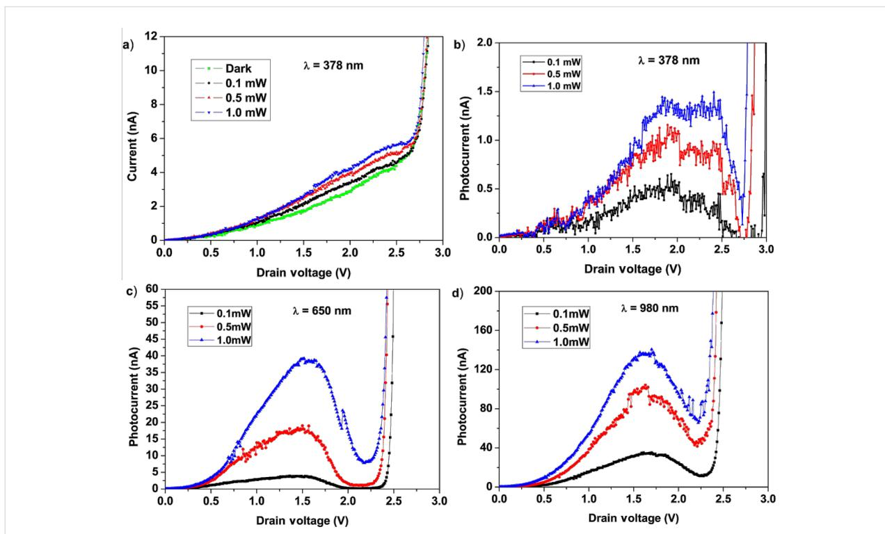
**Figure 6:** (a) Dark current and photocurrent tunneling in a CNT–Si heterojunction under 378 nm light illumination at different intensities. (b) The same as in (a) after subtracting the dark current. (c) The same as in (b) but for 650 nm and (d) 980 nm.
