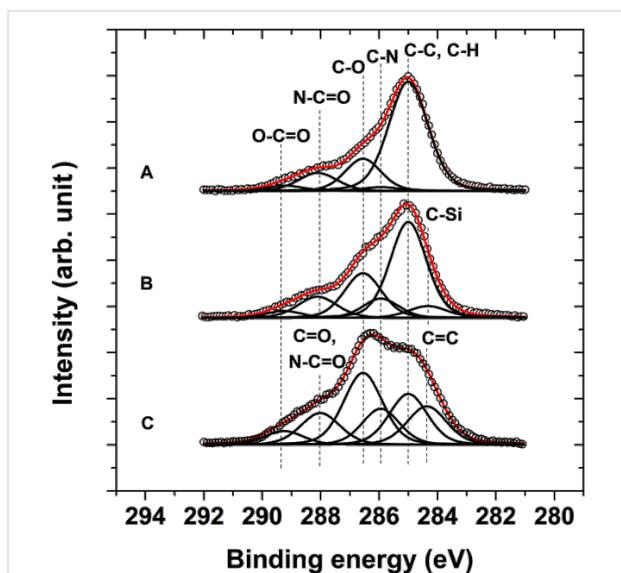
**Figure 6:** High resolution C 1s XPS spectra of alginate coatings on neridronate (A), APTES siloxane (B) and PDA (C) anchoring layers. The unfilled circles represent the measured data, while the red lines represent the fitted data. The individual contributions to the fitted data of different functional groups present in the films are represented with black lines.
