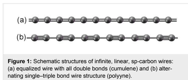
**Figure 1:** Schematic structures of infinite, linear,  $sp$ -carbon wires: (a) equalized wire with all double bonds (cumulene) and (b) alternating single–triple bond wire structure (polyynes).
