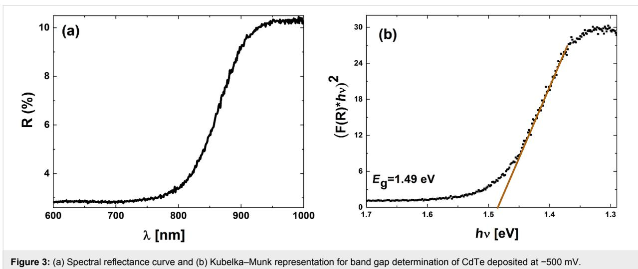
Figure 3: (a) Spectral reflectance curve and (b) Kubelka–Munk representation for band gap determination of CdTe deposited at -500 mV.
