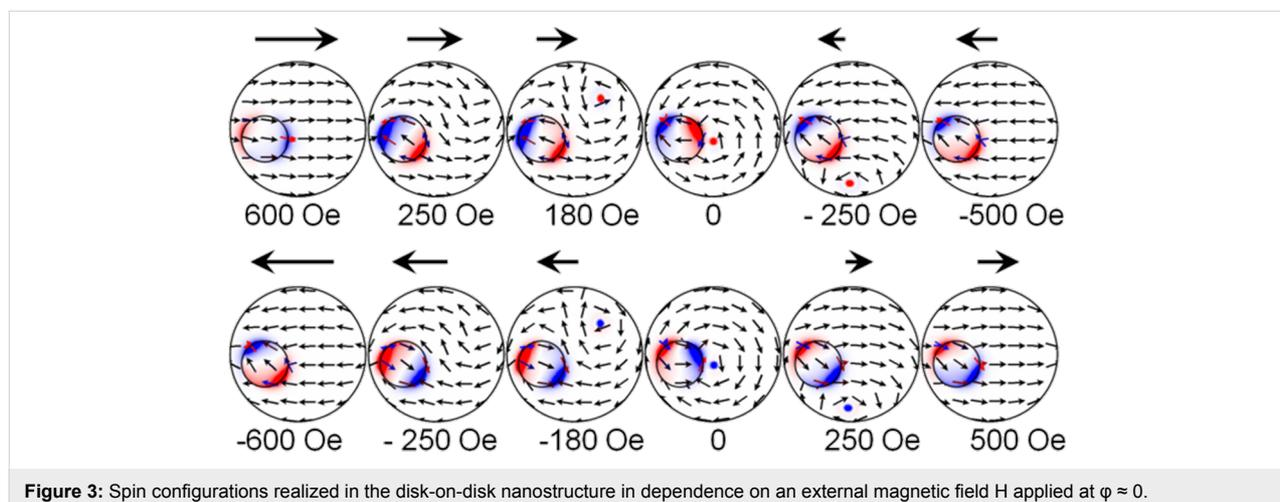
**Figure 3:** Spin configurations realized in the disk-on-disk nanostructure in dependence on an external magnetic field  $H$  applied at  $\varphi \approx 0$ .
