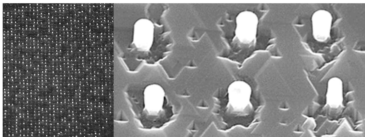
**Figure 2:** Scanning electron microscope (SEM) images of the ordered arrays of Si NWs showing (left) a NW array and (right) individual 200 nm long NWs.
