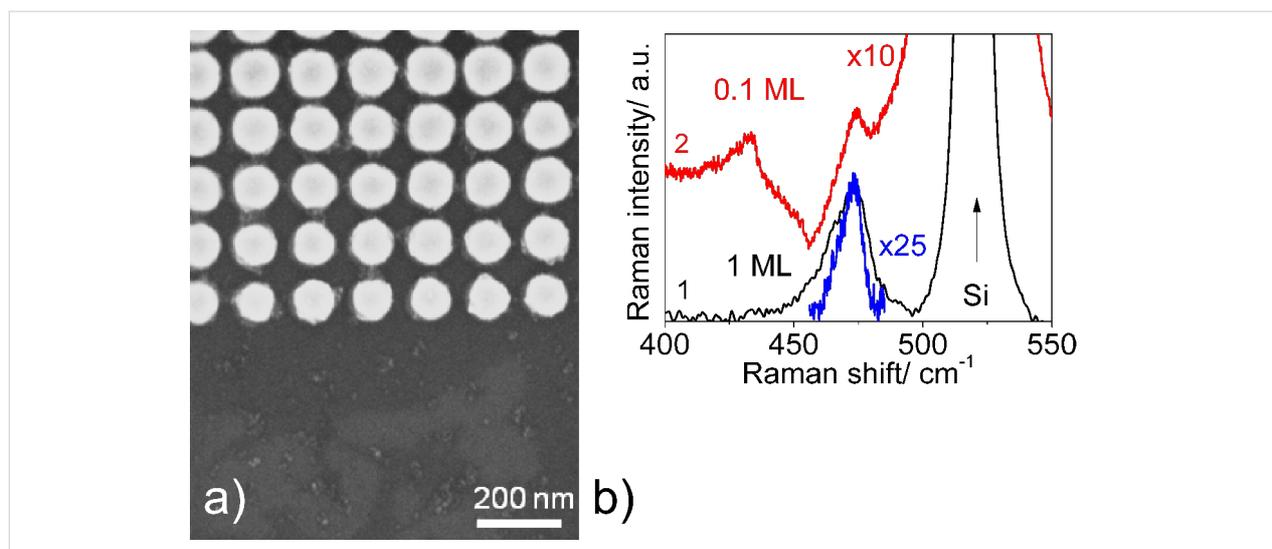
**Figure 6:** a) SEM image of CuS NCs with an ultra-low areal density deposited on Au arrays on SiO<sub>2</sub> layer and b) SERS-IERS Raman spectra measured with 632.8 nm. SERS spectrum of CuS NCs with 1 ML coverage on Au arrays formed on SiO<sub>2</sub> layer (curve 1) together with the Raman response of the CuS NCs of ultra-low areal density (denoted as 0.1 ML, curve 2). The 25 times enlarged fragment of curve 2 is shown for comparison.
