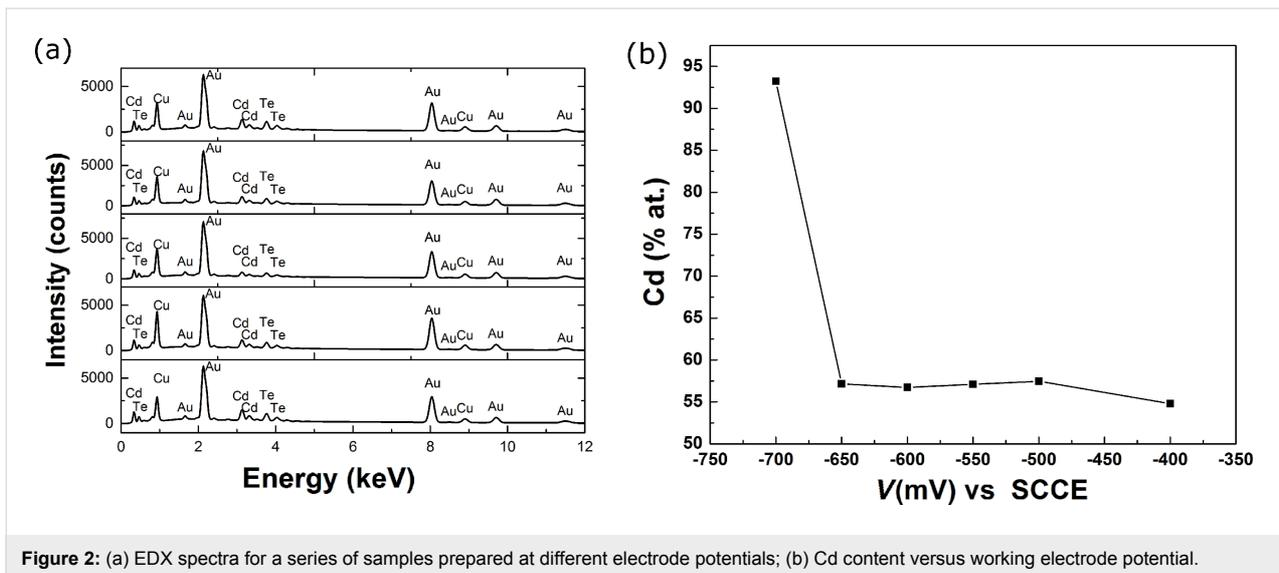
Figure 2: (a) EDX spectra for a series of samples prepared at different electrode potentials; (b) Cd content versus working electrode potential.
