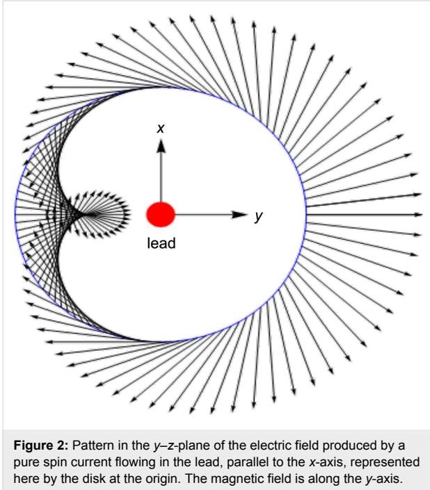
**Figure 2:** Pattern in the  $y$ - $z$ -plane of the electric field produced by a pure spin current flowing in the lead, parallel to the  $x$ -axis, represented here by the disk at the origin. The magnetic field is along the  $y$ -axis.
