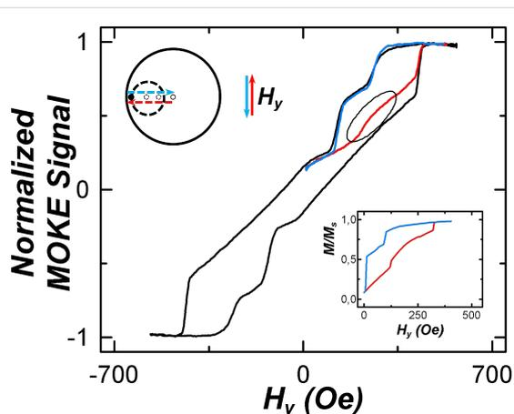
**Figure 6:** Hysteresis loops measured under a field ranging from +500 to –500 Oe (black line), as well as under an asymmetric field changing from +500 to –50 Oe (colored lines). Insets represent the schematic view of trajectories of the vortex core (top) and the result of micromagnetic simulations of the hysteresis loop (bottom).
