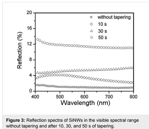
**Figure 3:** Reflection spectra of SiNWs in the visible spectral range without tapering and after 10, 30, and 50 s of tapering.
