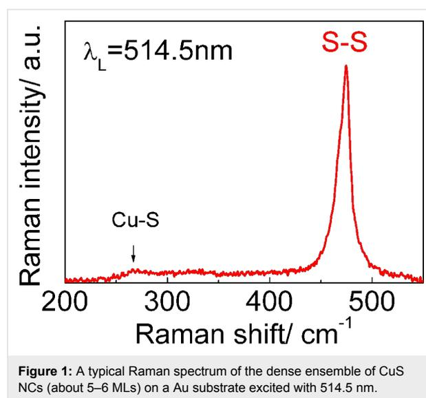
**Figure 1:** A typical Raman spectrum of the dense ensemble of CuS NCs (about 5–6 MLs) on a Au substrate excited with 514.5 nm.
