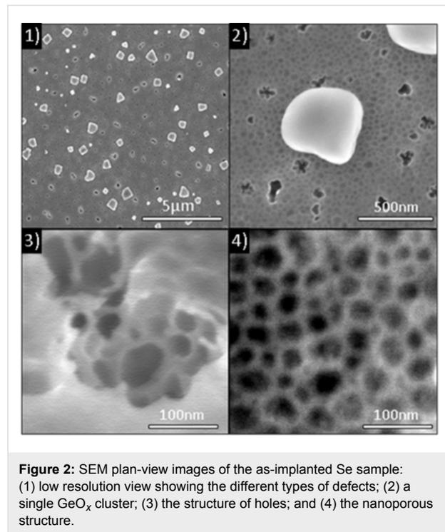
**Figure 2:** SEM plan-view images of the as-implanted Se sample: (1) low resolution view showing the different types of defects; (2) a single GeO<sub>x</sub> cluster; (3) the structure of holes; and (4) the nanoporous structure.
