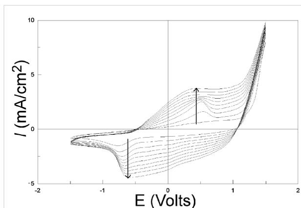
**Figure 5:** 10 successive CVs performed on vitreous carbon with 10 mM EDOT and 0.1 M LiClO<sub>4</sub> in acetonitrile solution. Scan rate: 100 mV/s. The arrow direction indicates increasing scan numbers.
