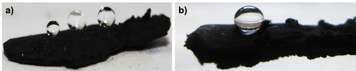
**Figure 4:** Photographs of water droplets of different volumes (a) and contact angle profile of a single drop (b) on the bulk material.
