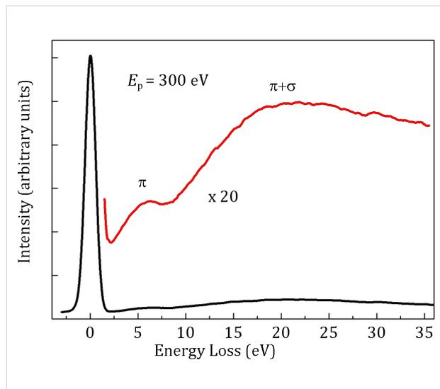
**Figure 3:** Electron energy loss spectra ( $E_p = 300$  eV) obtained on the CNT-sponge. The  $\pi$  and  $\pi + \sigma$  plasmons have been emphasized for better view (red line).
