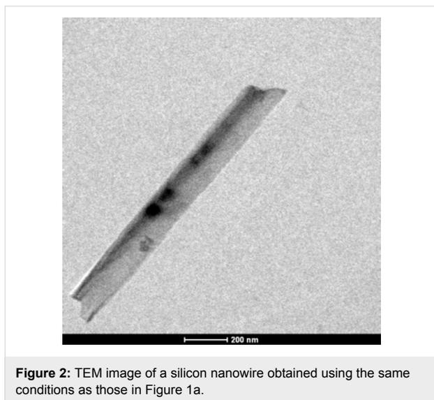
**Figure 2:** TEM image of a silicon nanowire obtained using the same conditions as those in Figure 1a.
