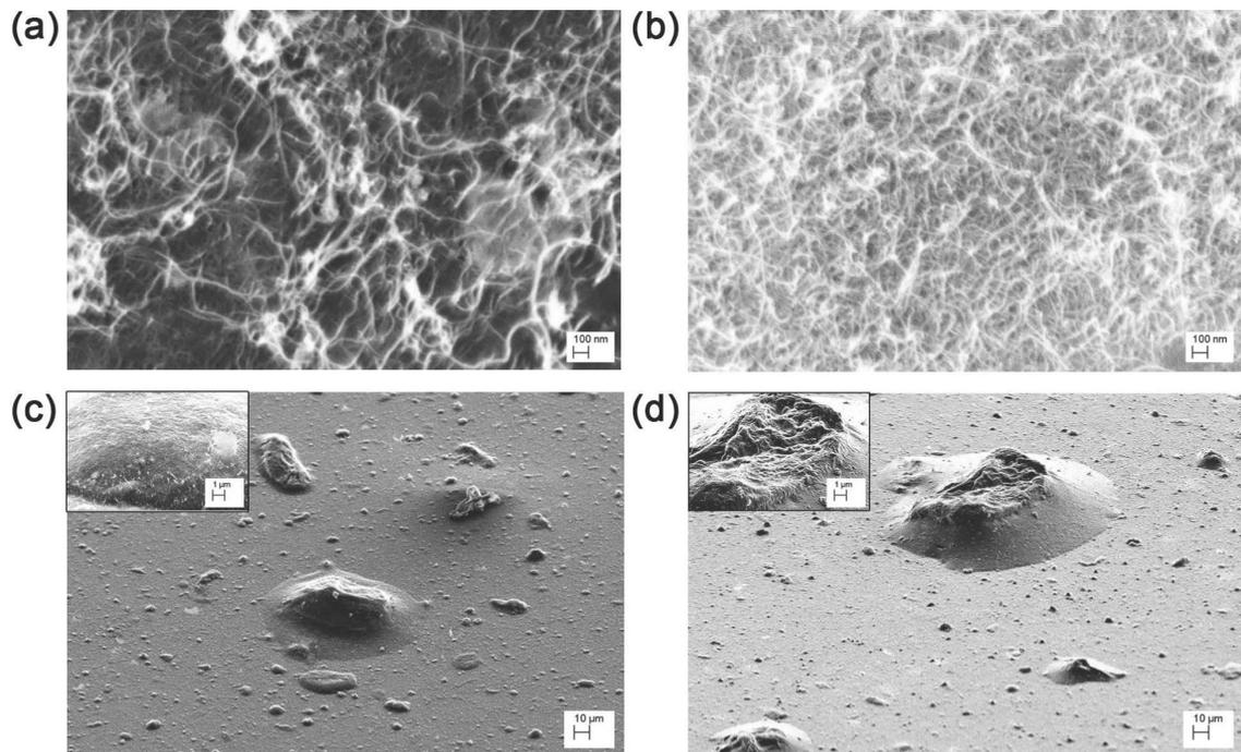
**Figure 2:** Scanning electron micrographs of SWCNT/MWCNT (a,c) and MWCNT/SWCNT (b,d) films at different magnifications 200,000 × (a,b), 1,000× (c,d), and 10,000× (c,d insets). In the images taken at grazing incidence (c,d and insets), it is possible to observe that in both cases the self-assembly forms several huge microstructures. (c,d insets) Details of the microstructures showing a hierarchical morphology very similar to that of lotus leaves and rose petals.
