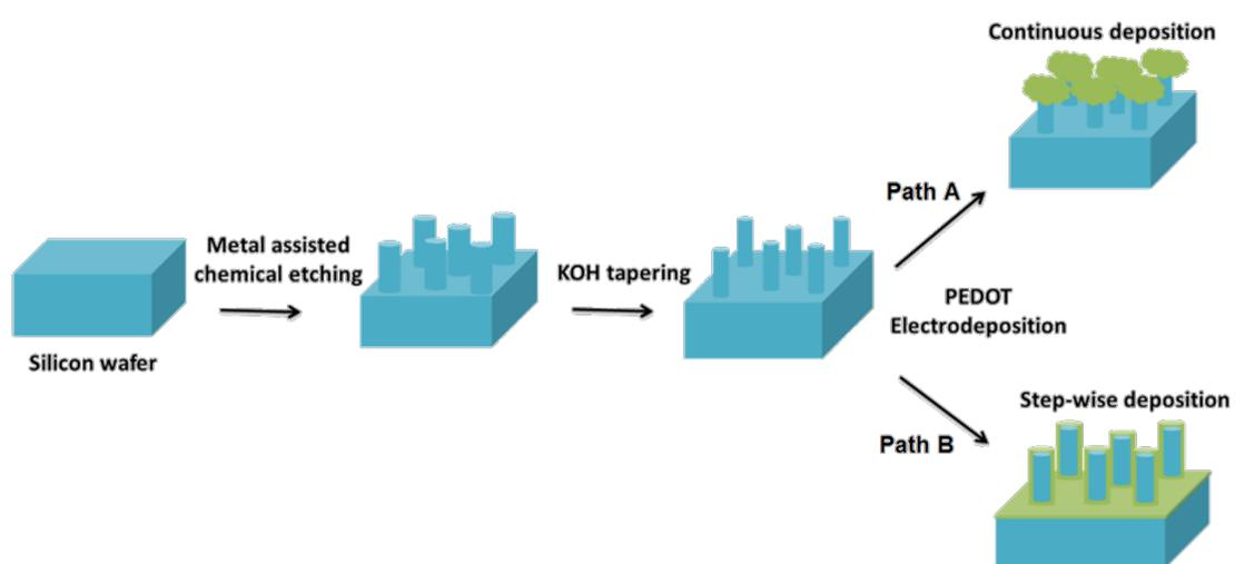
**Figure 13:** Schematic illustration of the processes resulting in PEDOT/SiNW hybrid structures. (a) Continuous electrodeposition leads to a mushroom-like morphology of PEDOT (green) on the tips of SiNW (blue), while (b) a step-wise deposition aids in the formation of a conformal PEDOT layer (green) surrounding each individual SiNW (blue).
