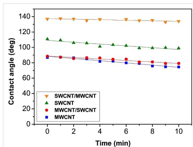
**Figure 5:** Variations of the contact angle as a function of the elapsed time from drop cast on the porous SWCNT (green triangles), MWCNT (blue squares), SWCNT/MWCNT (orange inverted triangles), MWCNT/SWCNT (red dots) films. The quite constant trend of the SWCNT/MWCNT contact angle value shows the stability in time of the carbon nanotube hydrophobic Cassie–Baxter metastable state.
