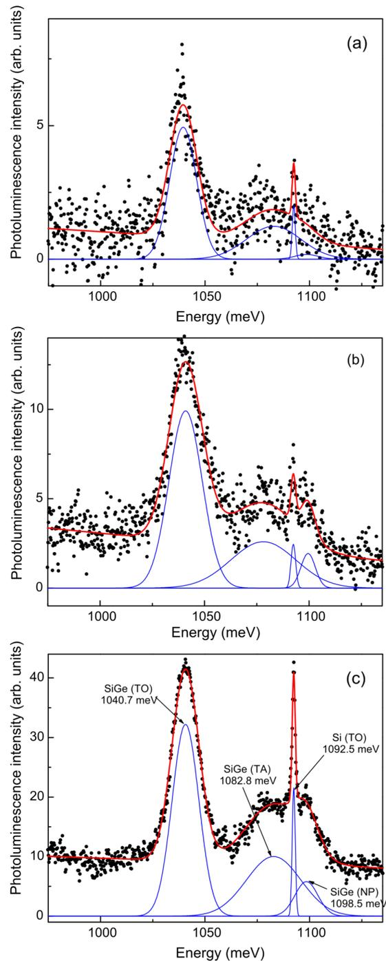
**Figure 6:** Curve-resolved PL spectrum of (a) sample (A), (b) sample (B), and (c) sample (C) at 25 K obtained with 405 nm excitation. The solid line shows the overall fit to the PL data, while the three SiGe NW component lines are shown beneath the fitted spectrum. The very sharp line at 1092.5 meV arises from the Si substrate.
