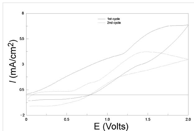
**Figure 8:** Two successive CVs performed on SiNWs under illumination with 10 mM EDOT and 0.1 M LiClO<sub>4</sub> in acetonitrile solution. Scan rate: 100 mV/s.
