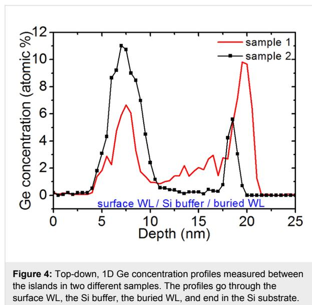
**Figure 4:** Top-down, 1D Ge concentration profiles measured between the islands in two different samples. The profiles go through the surface WL, the Si buffer, the buried WL, and end in the Si substrate.
