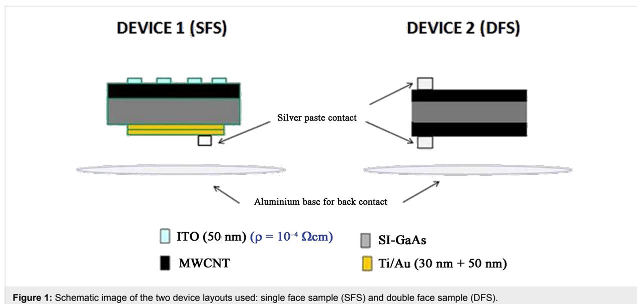
**Figure 1:** Schematic image of the two device layouts used: single face sample (SFS) and double face sample (DFS).
