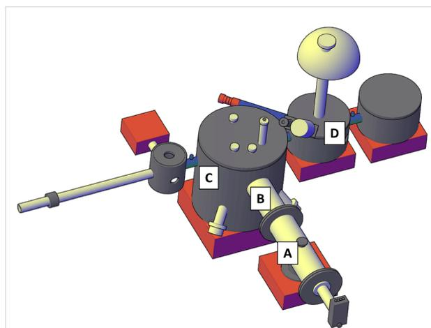
**Figure 1:** Sketch of the experimental set up: the NPs are created by the NC200 source (A), they are mass selected by the QMF (B) and they are deposited on the substrate in the deposition chamber (C). The chemical characterization is performed in situ in the XPS chamber (D).
