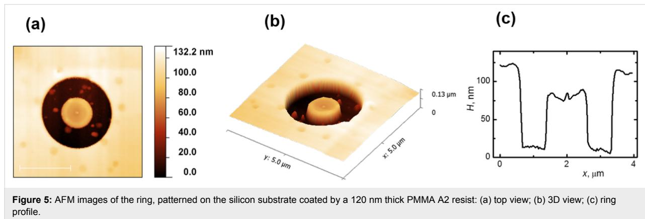
**Figure 5:** AFM images of the ring, patterned on the silicon substrate coated by a 120 nm thick PMMA A2 resist: (a) top view; (b) 3D view; (c) ring profile.
