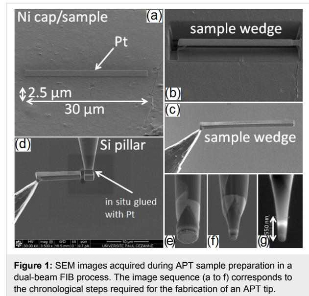
**Figure 1:** SEM images acquired during APT sample preparation in a dual-beam FIB process. The image sequence (a to f) corresponds to the chronological steps required for the fabrication of an APT tip.
