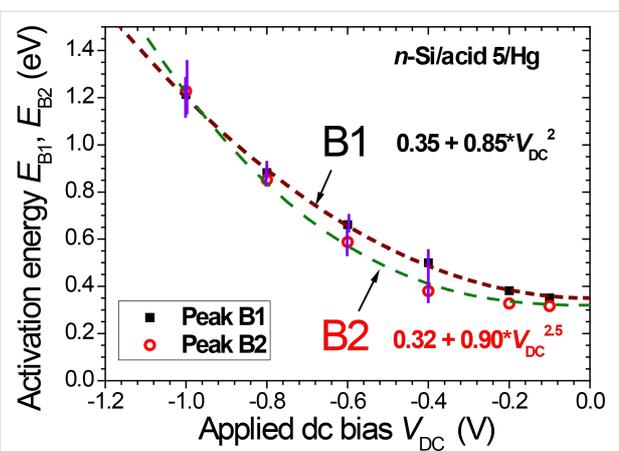
**Figure 5:** Bias dependence of dipolar relaxation activation energies,  $E_{B1}$  (squares) and  $E_{B2}$  (circles). The lines are power-law functions with forced exponent values:  $E_{B1}$  (eV) =  $0.35 + 0.85 |V_{DC}|^2$ ;  $E_{B2}$  (eV) =  $0.32 + 0.90 |V_{DC}|^{2.5}$ .
