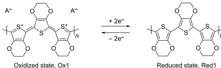
**Scheme 2:** Polymer reduction reaction scheme for PEDOT.
