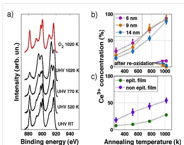
**Figure 5:** (a) Ce 3d XPS spectra for a complete reduction (black curves) and oxidation (red curve) cycle. (b) Intensity of the  $\text{Ce}^{3+}$  component at different annealing temperature and after re-oxidation on NPs of diameter of 6 nm (pink dots), 9 nm (orange dots), and 14 nm (blue dots), and (c) on the ultra-thin epitaxial (green dots) and non-epitaxial (violet dots) ceria film.
