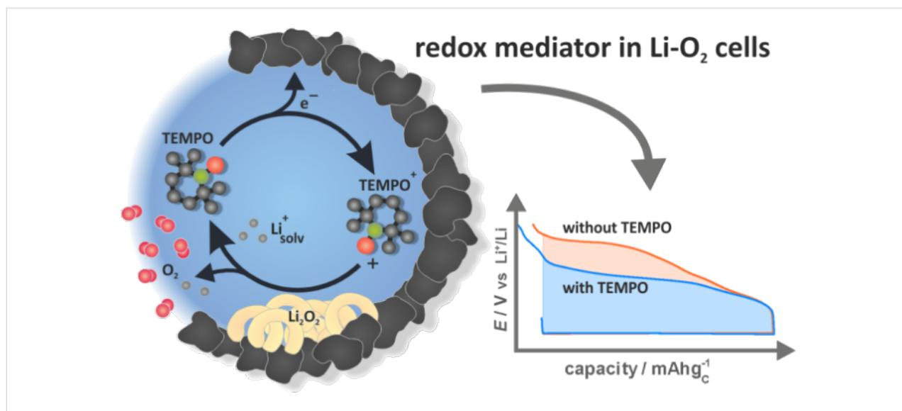
**Figure 8:** Illustration of TEMPO as a redox mediator (RM) in an  $\text{Li}/\text{O}_2$  cell reversibly catalyzing the  $\text{Li}_2\text{O}_2$  oxidation. Figure adapted with permission from [99], copyright 2014 American Chemical Society.
