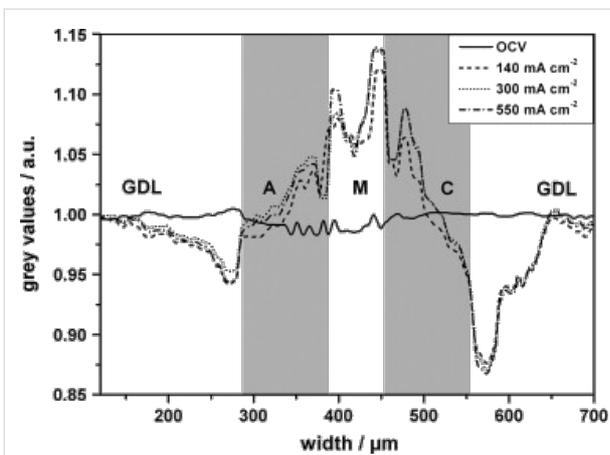
**Figure 15:** Changes of the transmission through the MEA (grey values) compared to steady-state conditions at OCV for different operating conditions: at OCV (solid line),  $140 \text{ mA}\cdot\text{cm}^{-2}$  (dashed line),  $300 \text{ mA}\cdot\text{cm}^{-2}$  (dotted line) and  $550 \text{ mA}\cdot\text{cm}^{-2}$  (dot and dash line). Reprinted with permission from [65]. Copyright 2010 Elsevier.
