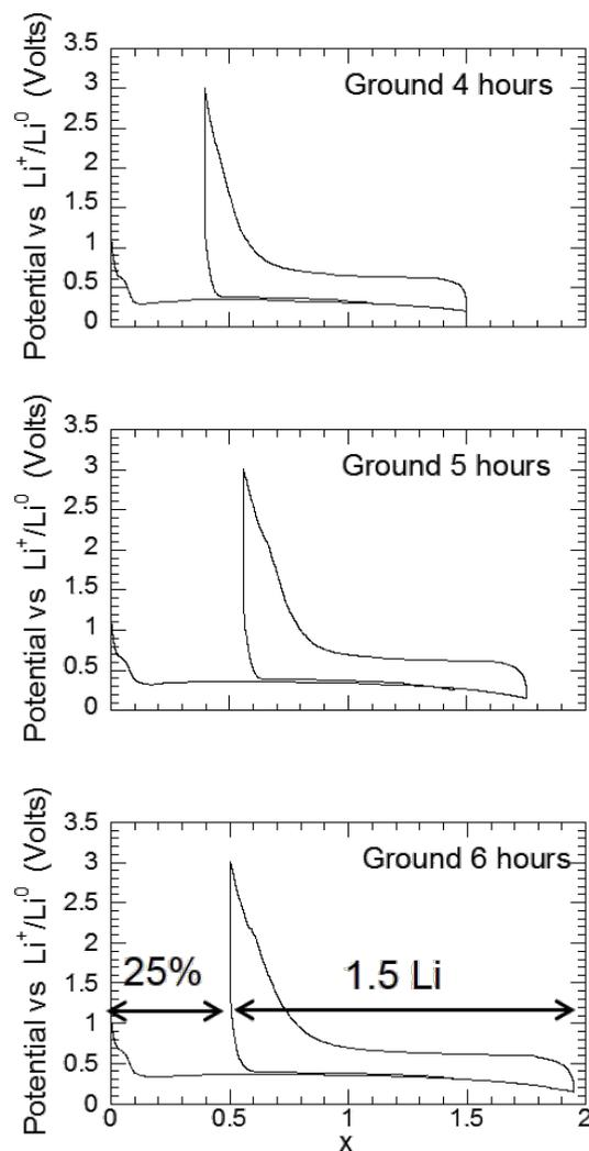
**Figure 18:** Evolution of the potential (V) as a function of  $x$  for a  $\text{Li}/\text{MgH}_2$  cell that was cycled down to 0.15 V vs  $\text{Li}^+/\text{Li}^0$  at a rate of one equivalent of lithium in 10 h. ( $\text{MgH}_2$  is obtained after three absorptions of hydrogen and then ground 4, 5 or 6 h with 10% of  $\text{C}_{t,z}$  carbon) [11].
