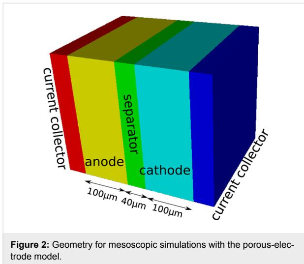
**Figure 2:** Geometry for mesoscopic simulations with the porous-electrode model.
