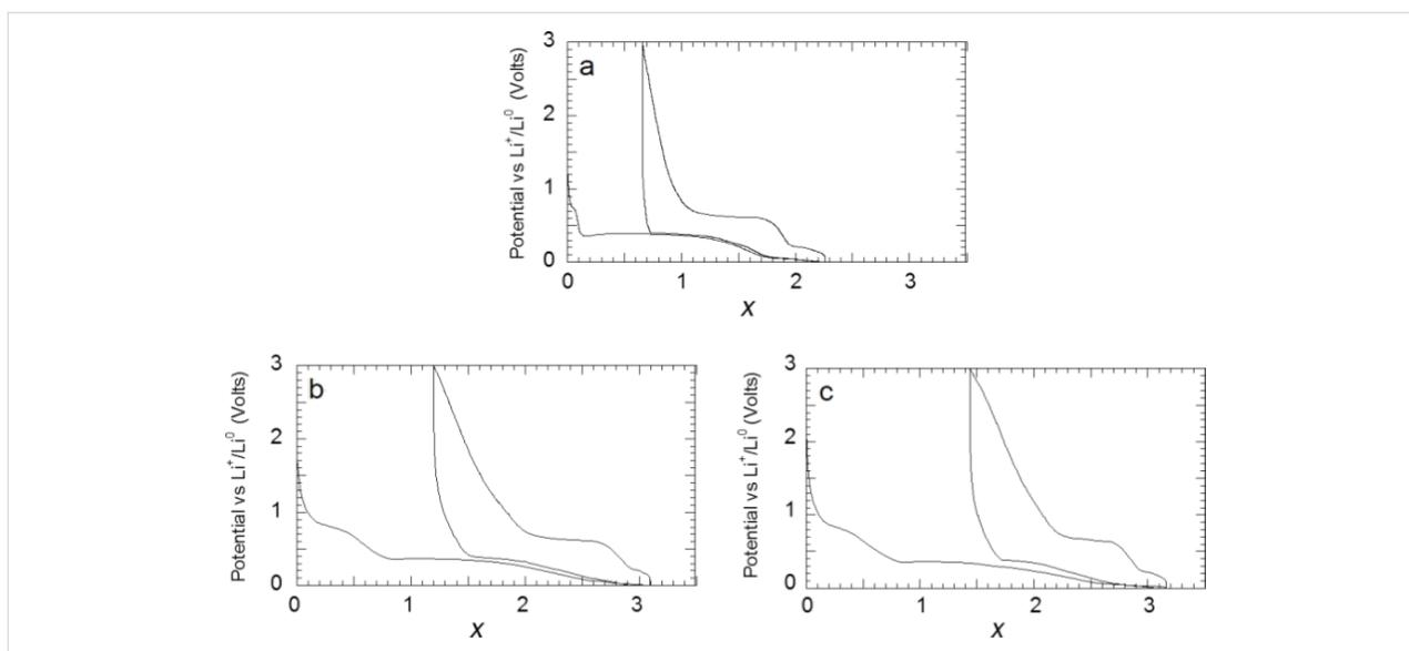
**Figure 20:** Evolution of the potential (V) as a function of  $x$  (mole fraction of Li) for  $\text{MgH}_2$  electrodes cycled between 3 and 0.005 V at a rate of one equivalent of lithium in 10 h. (a)  $\text{MgH}_2$ -18%  $\text{C}_{t,z}$ ; (b) 33.3%  $\text{MgH}_2$ -33.3% CMC-33.3%  $\text{C}_{t,z}$ ; (c) 33.3%  $\text{MgH}_2$ -33.3% CMC-f-33.3%  $\text{C}_{t,z}$ . Adapted from [46]. Copyright 2011 Elsevier.
