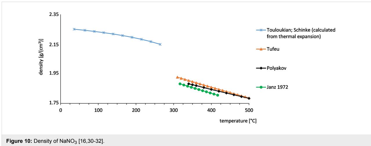
Figure 10: Density of  $\text{NaNO}_3$  [16,30-32].
