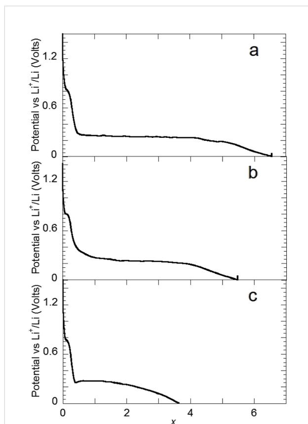
**Figure 8:** Discharge curves for a)  $\text{Mg}_2\text{FeH}_6$ , b)  $\text{Mg}_2\text{CoH}_5$  and c)  $\text{Mg}_2\text{NiH}_4$  electrodes prepared by reactive grinding as a function of Li ( $x$ ) mole fraction, recorded at a current rate of one equivalent of Li in 10 h. Adapted from [13] (copyright 2013 Elsevier) and [19].
