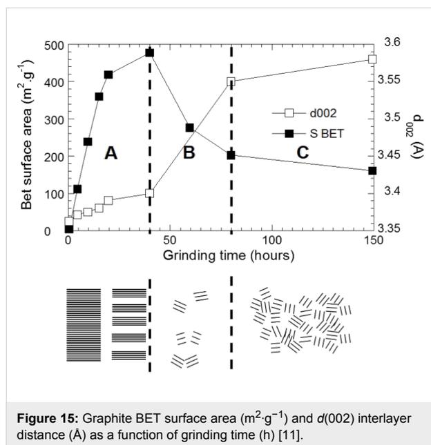
**Figure 15:** Graphite BET surface area ( $\text{m}^2\cdot\text{g}^{-1}$ ) and  $d(002)$  interlayer distance ( $\text{\AA}$ ) as a function of grinding time (h) [11].
