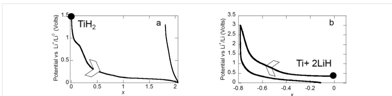
**Figure 22:** Potential profile of a)  $\text{TiH}_2$  electrode ground for 5 h with 10% of  $\text{C}_{t,z}$  carbon b)  $\text{Ti} + 2\text{LiH}$  electrode as a function of  $x$ , the mole fraction of Li (rate one equivalent of Li in 100 h). Adapted from [6]. Copyright 2009 Elsevier.
