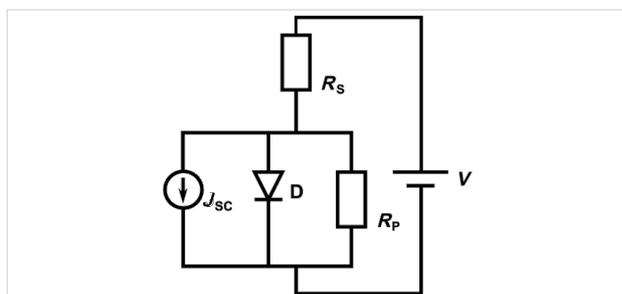
**Figure 2:** Equivalent circuit for the one diode model. The diode, D, describes the part of the circuit that represents the ideal diode equation with an ideality factor  $n = 1$ .  $R_S$  and  $R_P$  represent the parasitic resistances taking ohmic losses into account.  $J_{SC}$  represents the short circuit current density.
