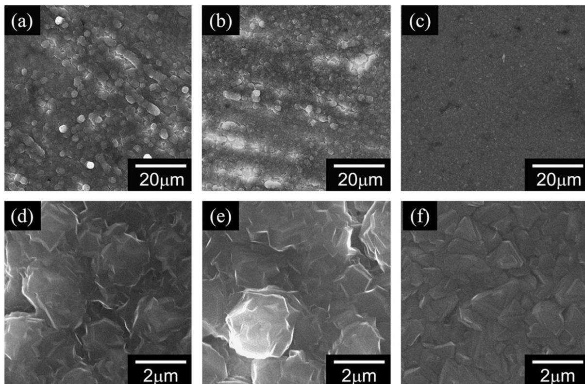
**Figure 2:** SEM images of the electrodeposited magnesium (a)  $500\times$ ,  $0.5 \text{ mA cm}^{-2}$ , (b)  $500\times$ ,  $1.0 \text{ mA cm}^{-2}$ , (c)  $500\times$ ,  $2.0 \text{ mA cm}^{-2}$ , (d)  $5000\times$ ,  $0.5 \text{ mA cm}^{-2}$ , (e)  $5000\times$ ,  $1.0 \text{ mA cm}^{-2}$ , and (f)  $5000\times$ ,  $2.0 \text{ mA cm}^{-2}$ . Reprinted with permission from [13]. Copyright 2011 Elsevier.
