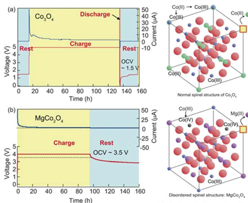
**Figure 8:** The OCV values of the test cells after constant voltage charge: positive electrode, (a) ordered  $\text{Co}_3\text{O}_4$  and (b) disordered  $\text{MgCo}_2\text{O}_4$ ; negative electrode, Mg; electrolyte,  $\text{Mg}(\text{ClO}_4)_2$  in acetonitrile. Reproduced with permission from [66]. Copyright 2011 The Royal Society of Chemistry.
