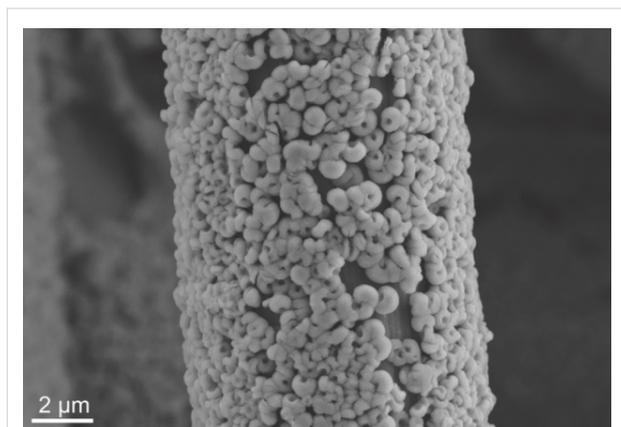
**Figure 7:** SEM image of toroidal  $\text{Li}_2\text{O}_2$  nanoparticles on a carbon fiber (10  $\mu\text{m}$  in diameter) that form as a discharge product in lithium–oxygen cells (C. L. Bender, JLU Giessen).
