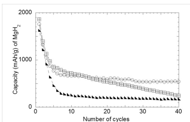
**Figure 21:** Electrochemical cycling performance for  $\text{MgH}_2$  composite electrodes:  $\text{MgH}_2$ -18%  $\text{C}_{t,z}$  (black triangles), 33.3%  $\text{MgH}_2$ -33.3% CMC-33.3%  $\text{C}_{t,z}$  (open squares) and 33.3%  $\text{MgH}_2$ -33.3% CMC-f-33.3%  $\text{C}_{t,z}$  (open circles). Cycling between 3 and 0.005 V, rate of one equivalent of lithium in 10 h. Adapted from [46]. Copyright 2011 Elsevier.
