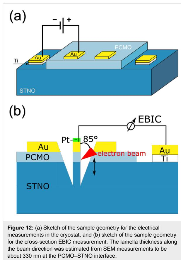
**Figure 12:** (a) Sketch of the sample geometry for the electrical measurements in the cryostat, and (b) sketch of the sample geometry for the cross-section EBIC measurement. The lamella thickness along the beam direction was estimated from SEM measurements to be about 330 nm at the PCMO–STNO interface.
