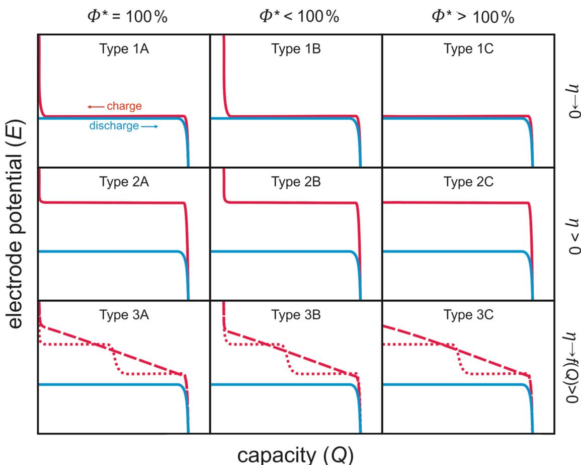
**Figure 4:** Matrix for classifying voltage profiles of metal–oxygen batteries. Type 1A is the ideal case. Frequently observed are Type 1B, 2C, 3B and 3C. The coulombic efficiency is calculated as  $\Phi = Q_{\text{charge}}/Q_{\text{discharge}} \times 100\%$ .
