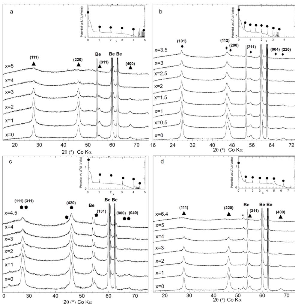
**Figure 9:** In situ XRD patterns of a) Mg<sub>2</sub>FeH<sub>6</sub>, b) Mg<sub>2</sub>CoH<sub>5</sub> and c) Mg<sub>2</sub>NiH<sub>4</sub> and d) Mg<sub>2</sub>FeH<sub>6</sub>-10% C<sub>t,z</sub> electrodes prepared by reactive grinding as a function of the mole fraction of Li (x) Inset: Potential profile of a) b) c) and d) obtained during GITT (rate: one equivalent of Li in 10 h, relaxation time: 10 h). Adapted from [13] (copyright 2013 Elsevier) and [19].
