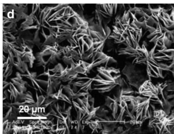
**Figure 13:** Voltage hysteresis of different carbon materials for the cathode of a sodium oxygen cell (left), figure adapted with permission from [27], copyright 2014 Wiley-VCH. SEM image of the oxygen electrode of a  $\text{Na}/\text{O}_2$  cell after discharge with  $\text{Na}_2\text{O}_2$  and  $\text{Na}_2\text{CO}_3$  as discharge product (right), figure adapted with permission from [105], copyright 2014 Elsevier.
