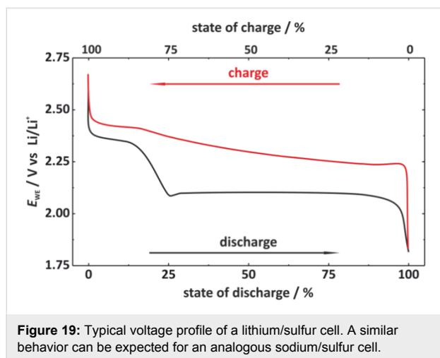
**Figure 19:** Typical voltage profile of a lithium/sulfur cell. A similar behavior can be expected for an analogous sodium/sulfur cell.
