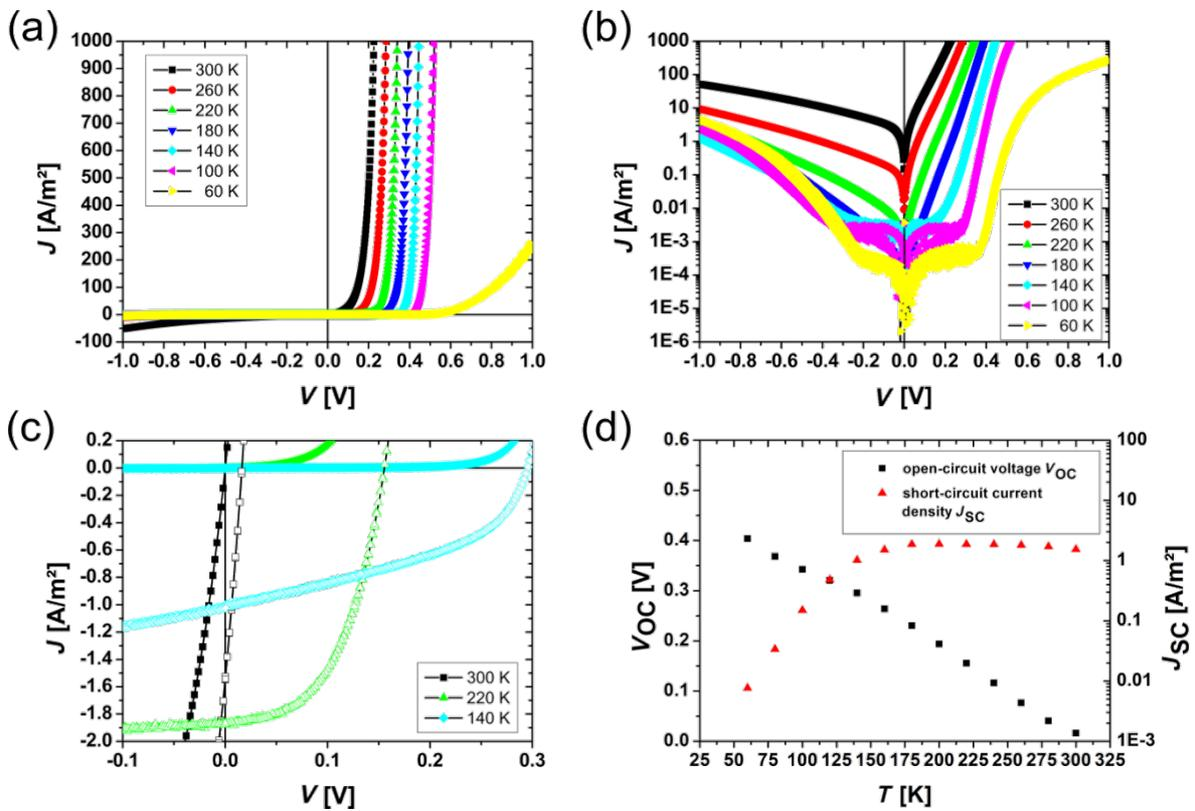
**Figure 4:** Temperature dependence of the  $J$ - $V$  characteristics for the PCMO–STNO junction: (a) in a linear and (b) in a semi-logarithmic illustration. Over the whole measured temperature range the  $J$ - $V$  curves show rectifying behavior. (c) Comparison of  $J$ - $V$  curves with and without illumination. (d) The open circuit voltage increases for decreasing temperature and the short circuit current breaks down at a temperature around 180 K.
