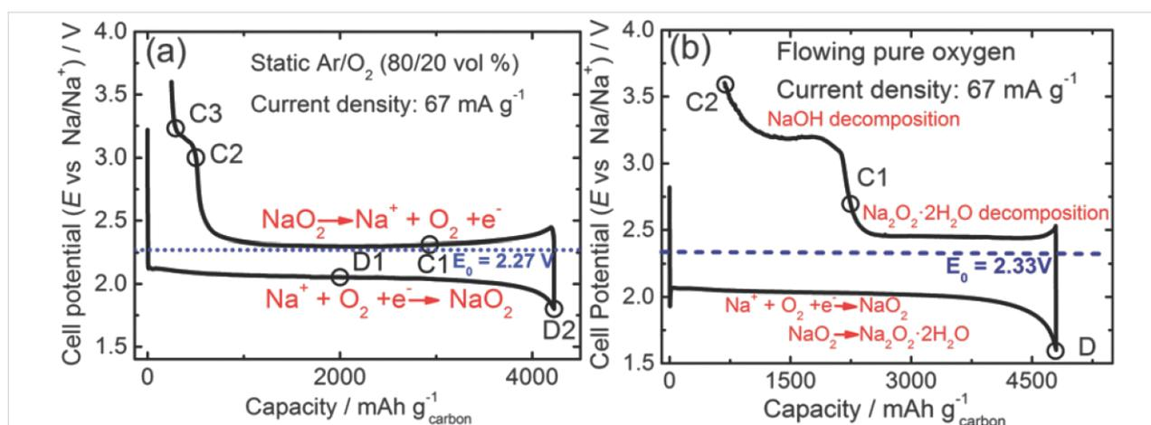
**Figure 14:** Voltage profiles of  $\text{Na}/\text{O}_2$  cells under static gas atmosphere and flowing gas atmosphere (Type 1B/3B). Figure adapted with permission from [111], copyright 2014 The Royal Society of Chemistry.
