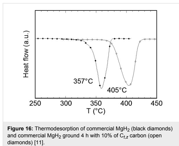
**Figure 16:** Thermodesorption of commercial  $\text{MgH}_2$  (black diamonds) and commercial  $\text{MgH}_2$  ground 4 h with 10% of  $\text{C}_{t,z}$  carbon (open diamonds) [11].
