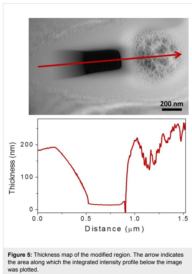
**Figure 5:** Thickness map of the modified region. The arrow indicates the area along which the integrated intensity profile below the image was plotted.
