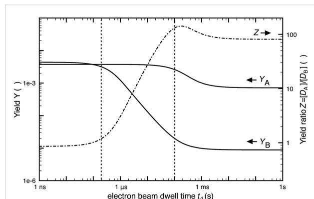
**Figure 17:** Calculated changes in dissociation yields  $Y_A$  and  $Y_B$  (per primary electron as defined in Equation 66 and Equation 67) and yield ratio  $Z$  versus electron beam dwell time. The example shown here was calculated for  $\text{Co}_2(\text{CO})_8$  and octanol as the deposition species “A” and “B”, respectively. The yield ratio  $Z$  is a measure for the ratio of non-volatile fragments of molecule “a” and “b” incorporated into the FEBID material. Taken from [78].
