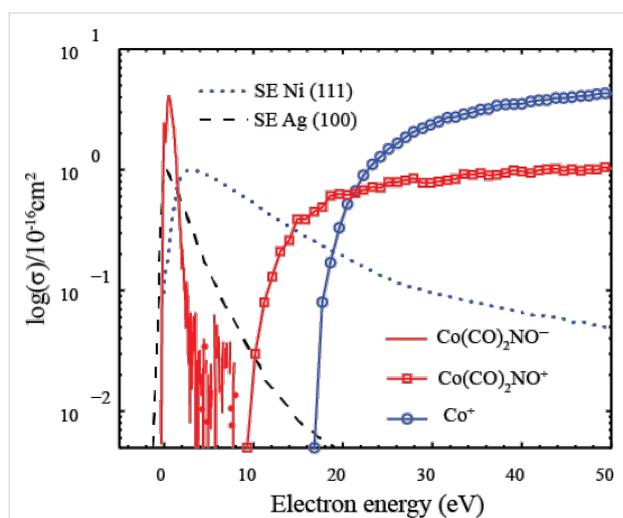
**Figure 19:** The partial cross sections for single CO loss through DEA (red solid line), for single CO loss through DI (red open squares), and for  $\text{Co}^+$  formation through DI (blue open circles), all adapted from Engmann et al. [10]. Also shown are the measured SE distributions from Ni(111) adapted from Schaefer et al. [6] (blue dotted line) and the measured SE distributions from Ag(100) adapted from Knights et al. [9] (black dashed line).
