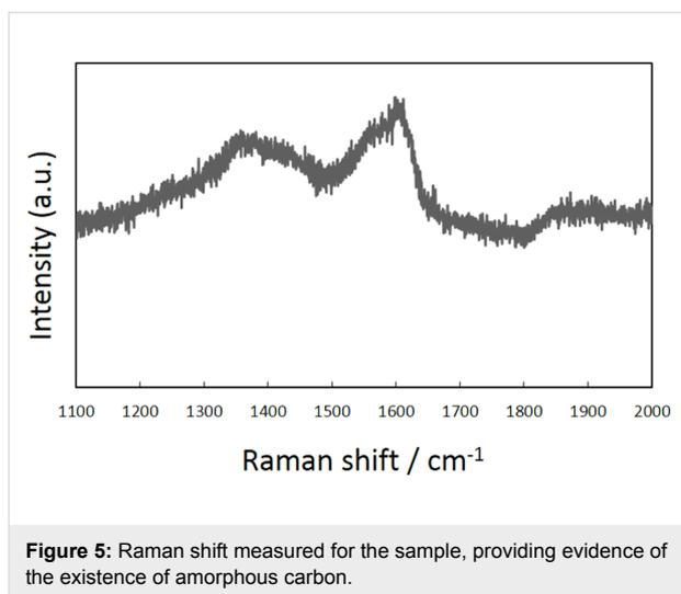
**Figure 5:** Raman shift measured for the sample, providing evidence of the existence of amorphous carbon.
