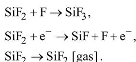
Multi-step FEBIE reactions can be modeled using a set of differential rate equations that account for each molecular species at the substrate surface, which in this case are the NF<sub>3</sub> precursor adsorbates (denoted by “a”), F radicals ( $\alpha$ ), and the reaction products SiF, SiF<sub>2</sub>, SiF<sub>3</sub>, and SiF<sub>4</sub>:
