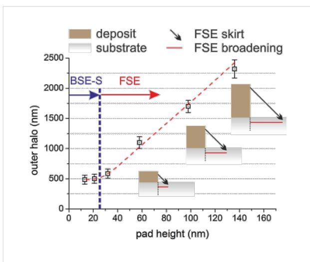
**Figure 8:** Outer-halo behavior for increasing pad thicknesses of 5 keV deposits (squares) together with an FSE-related scheme to explain the linear increase for thicker deposits (details are given in the main text).
