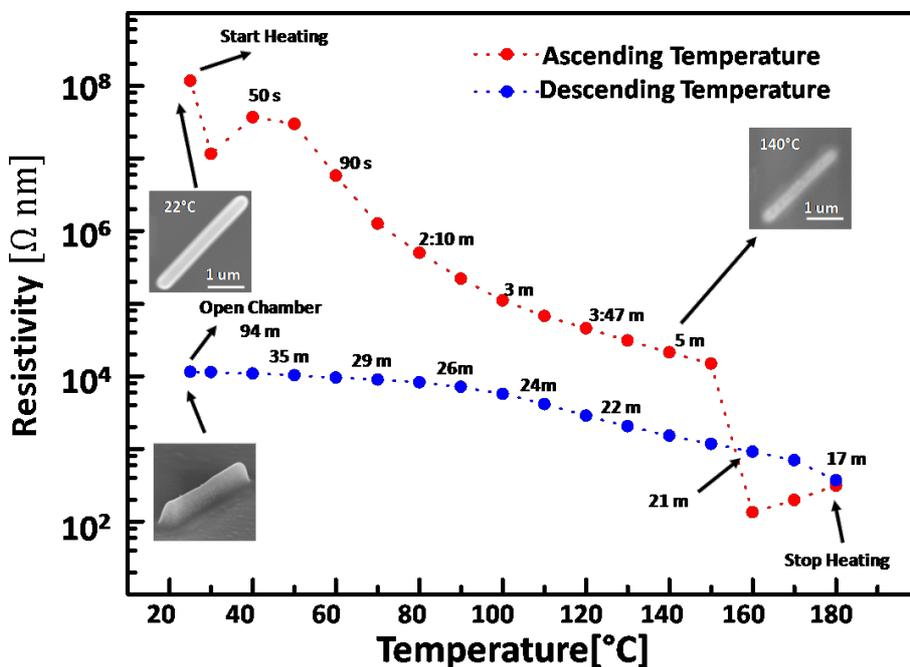
**Figure 8:** Calculated resistivity from the resistance measurement of a Cu–C line during in situ post-growth heating with a hot plate (red dots) and cooling down (blue dots) inside the SEM chamber. The resistance did not change when opening the chamber. The top SEM images show the morphology changes of an adjacent FEBID line which was observed simultaneously during the in situ resistance measurement.
