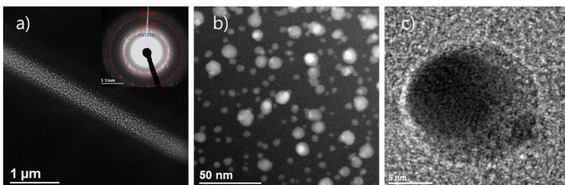
**Figure 6:** In situ TEM annealing for 10 min at 220 °C on a line deposit from Cu(hfac)<sub>2</sub> shown in Figure 2. a) STEM high angle annular dark field (STEM-HAADF) image of Cu nanocrystals forming from the deposit material. b) HAADF image showing distribution of Cu nanocrystals. c) High-resolution TEM (HR-TEM) image of 15 nm sized polycrystalline Cu precipitate. The inset shows the SAD pattern of Cu fcc nanocrystals.
