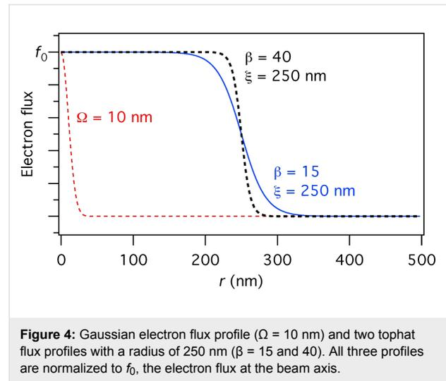
**Figure 4:** Gaussian electron flux profile ( $\Omega = 10$  nm) and two tophat flux profiles with a radius of 250 nm ( $\beta = 15$  and 40). All three profiles are normalized to  $f_0$ , the electron flux at the beam axis.
