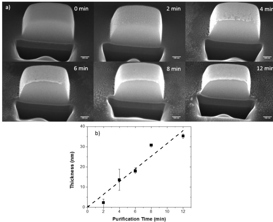
**Figure 2:** a) Cross-section SEM images of 400 nm thick Pt<sub>x</sub> deposits that were purified for 1, 2, 4, 6, 8, and 12 min (reading from left to right) demonstrating the linear, top-down nature of the purification process and b) is a plot of the purified layer thickness on the top of the pad against the total purification time.
