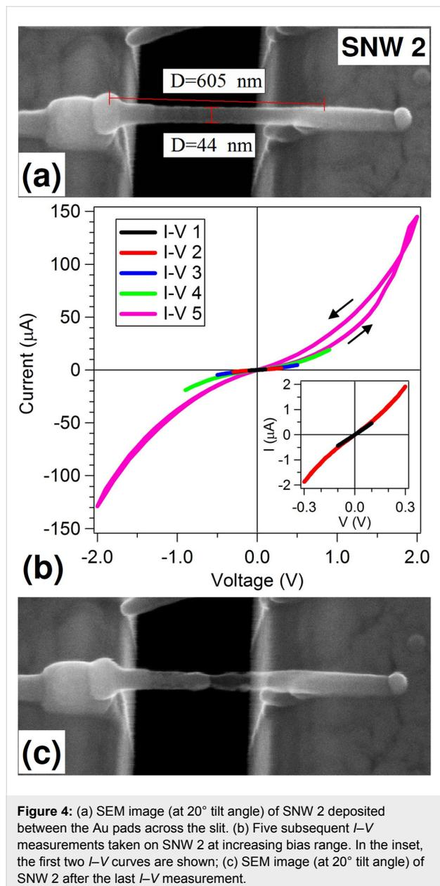
**Figure 4:** (a) SEM image (at 20° tilt angle) of SNW 2 deposited between the Au pads across the slit. (b) Five subsequent  $I$ - $V$  measurements taken on SNW 2 at increasing bias range. In the inset, the first two  $I$ - $V$  curves are shown; (c) SEM image (at 20° tilt angle) of SNW 2 after the last  $I$ - $V$  measurement.
