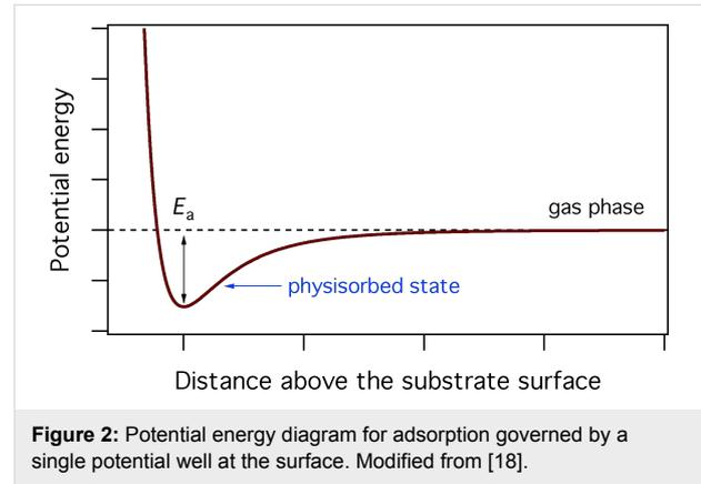
We note that Equation 2 describes non-activated Langmuir adsorption of a single molecular species ‘a’. The Langmuir model limits the surface coverage to one monolayer (hence the term  $(1 - \Theta)$  in Equation 2), and can be modified to account for other adsorption behavior such as multilayer adsorption and thermally activated chemisorption. We also note that most FEBIP models assume that  $s_a$  is independent of temperature.
