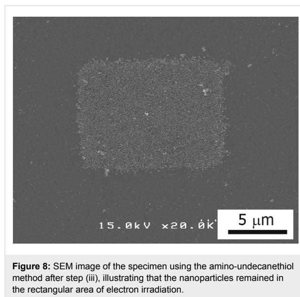
**Figure 8:** SEM image of the specimen using the amino-undecanethiol method after step (iii), illustrating that the nanoparticles remained in the rectangular area of electron irradiation.
