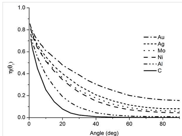
**Figure 8:** Dependence of the reflection coefficient of 35 keV He<sup>+</sup> on the grazing angle calculated with SRIM software for different materials.
