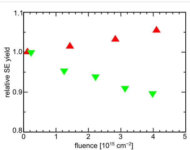
**Figure 3:** Comparison of contrast evolution in a standard HV and the used UHV HIM. The SE yield, which is proportional to the gray level in SE images, is plotted against the total dose for a HV system (green pointing down triangles) and the used UHV HIM (red pointing up triangles).
