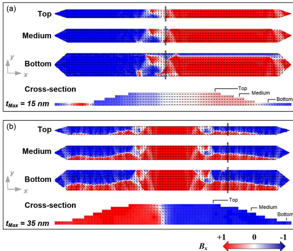
**Figure 9:** Magnetization vector-color maps extracted from the simulations for 250 nm wide Fe nanowires with bell-shaped profile (case II) and nominal thickness of (a) 10 nm and (b) 20 nm. The areas marked with black lines in the  $x,y$  plane representations have been chosen for the representation in the  $y,z$  plane (cross-section).
