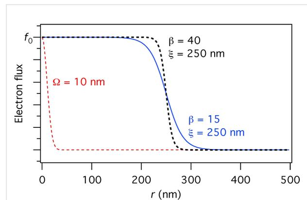
**Figure 4:** Gaussian electron flux profile ( $\Omega = 10$  nm) and two tophat flux profiles with a radius of 250 nm ( $\beta = 15$  and 40). All three profiles are normalized to  $f_0$ , the electron flux at the beam axis.
