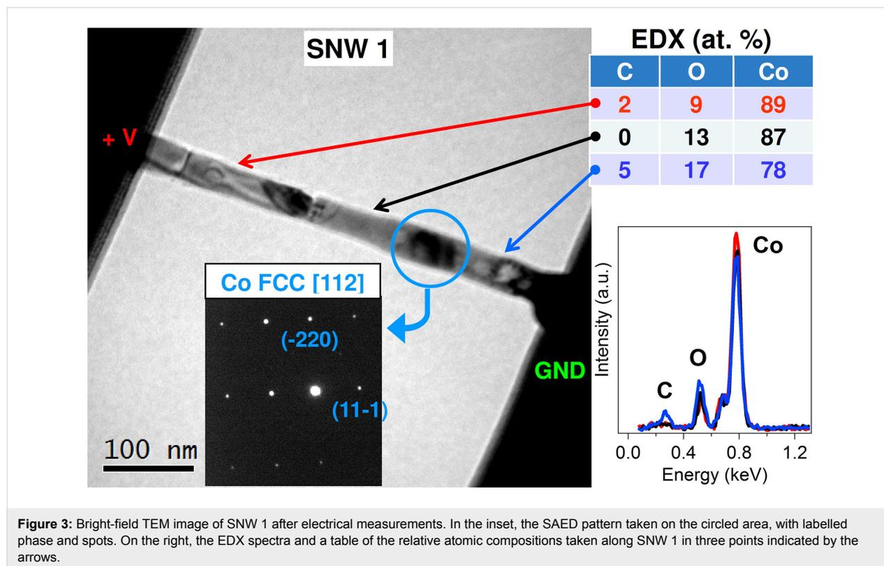
evident that a true carbon peak, above background level, remains only on the right part of SNW 1, where the graphite circles were observed.
