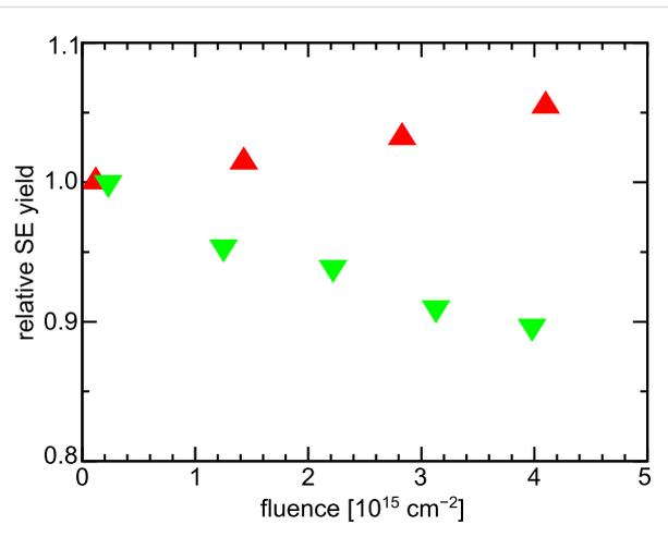
**Figure 3:** Comparison of contrast evolution in a standard HV and the used UHV HIM. The SE yield, which is proportional to the gray level in SE images, is plotted against the total dose for a HV system (green pointing down triangles) and the used UHV HIM (red pointing up triangles).
