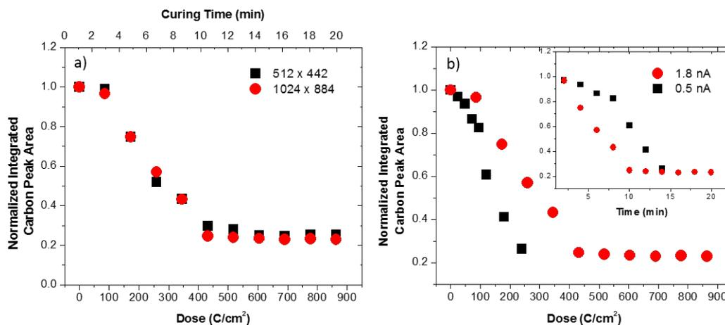
**Figure 3:** Normalized carbon peak area plotted as a function of a) curing time for the indicated pixel resolutions (note higher pixel resolution resulted in longer frame time) and b) dose for indicated beam currents. The inset depicts the same normalized carbon peak area as a function of time. The 1024 × 884 pixel resolution corresponds to ca. 0.65 nm point pitch while the 512 × 442 resolution corresponds to a point pitch of about 1.2 nm.
