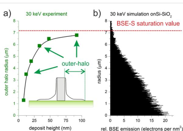
**Figure 2:** (a) Radius of the outer halo (AFM-based) of 30 keV PtC deposits as a function of the central pad thickness. (b) Simulated BSE-S radius for 30 keV electrons in Si–SiO<sub>2</sub>.
