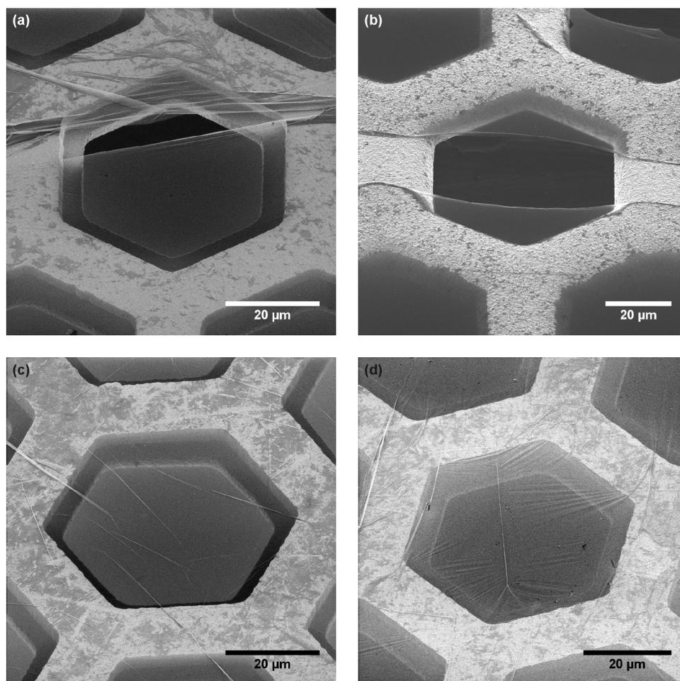
**Figure 2:** Examples of CNMs which were transferred onto copper grids with hexagonal openings. Different types of features are visible: (a) larger folds; (b) rolled CNM edges; (c) small folds; and (d) wrinkled CNMs. Detailed information on all HIM images is given in Supporting Information File 1, Tables S1 and S2.
