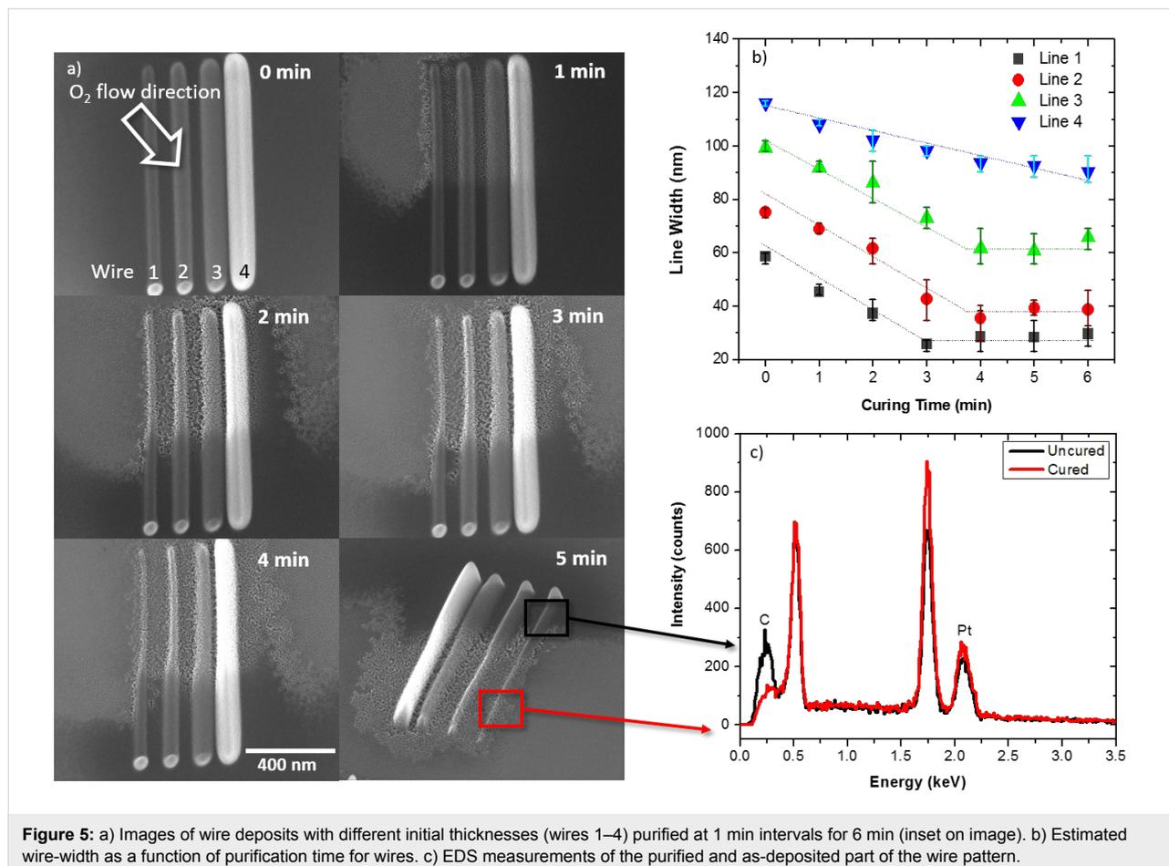
**Figure 5:** a) Images of wire deposits with different initial thicknesses (wires 1–4) purified at 1 min intervals for 6 min (inset on image). b) Estimated wire-width as a function of purification time for wires. c) EDS measurements of the purified and as-deposited part of the wire pattern.
