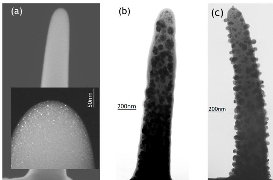
**Figure 7:** TEM in situ annealing of FEBID rods grown from (hfac)Cu(VTMS). a) Dark field image of an as-deposited freestanding rod. Inset: rod apex with small Cu nanocrystals in carbonaceous matrix. b) Bright-field image of same rod after 270 °C annealing and continuous TEM observation (200 keV). Large Cu nanocrystals form inside the rod. c) Bright field image of another rod not observed during the same annealing process. Cu nanocrystals form at the outside surface of the rod.
