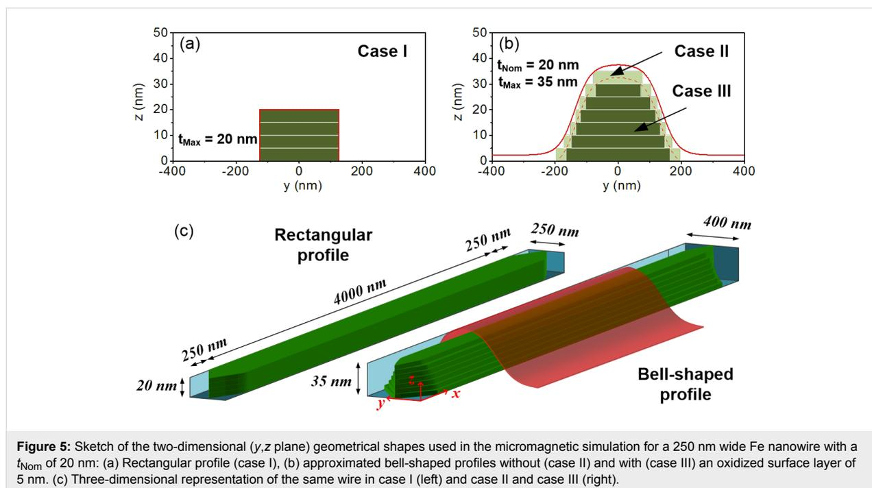
**Figure 5:** Sketch of the two-dimensional ( $y,z$  plane) geometrical shapes used in the micromagnetic simulation for a 250 nm wide Fe nanowire with a  $t_{\text{Nom}}$  of 20 nm: (a) Rectangular profile (case I), (b) approximated bell-shaped profiles without (case II) and with (case III) an oxidized surface layer of 5 nm. (c) Three-dimensional representation of the same wire in case I (left) and case II and case III (right).
