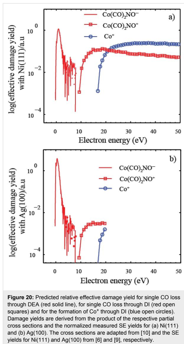
**Figure 20:** Predicted relative effective damage yield for single CO loss through DEA (red solid line), for single CO loss through DI (red open squares) and for the formation of  $\text{Co}^+$  through DI (blue open circles). Damage yields are derived from the product of the respective partial cross sections and the normalized measured SE yields for (a) Ni(111) and (b) Ag(100). The cross sections are adapted from [10] and the SE yields for Ni(111) and Ag(100) from [6] and [9], respectively.
