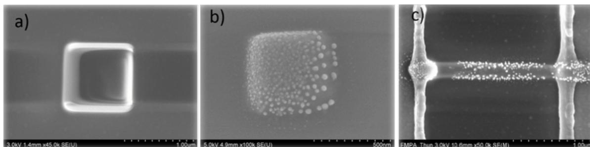
**Figure 4:** Post-growth laser annealing of FEBID deposits from  $\text{Cu}(\text{hfac})_2$ . SEM top view images of a) as-deposited square, b) Cu nanocrystals forming due to laser annealing at a power of 13.6 W over 1 min, c) laser-annealed FEBID line between two gold electrodes.
