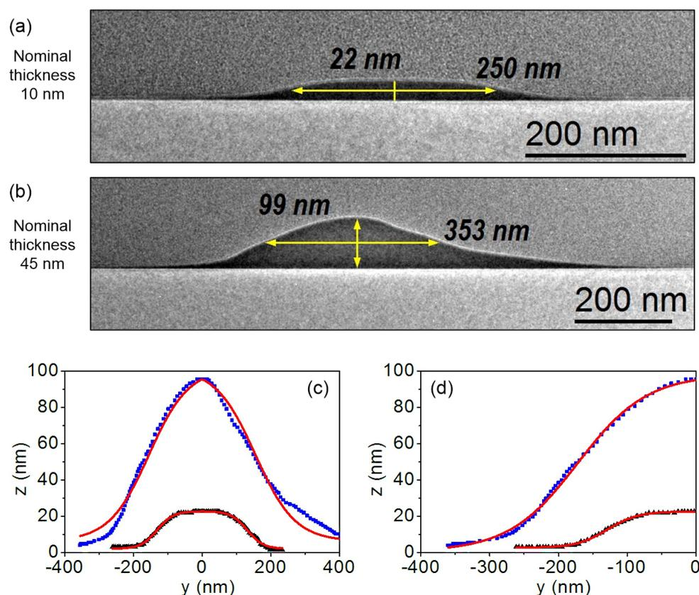
**Figure 3:** Low-magnification TEM images of the iron nanowires with width of 250 nm and nominal thickness of (a) 10 and (b) 45 nm. Fitting of the (c) full and (d) half profiles of both nanowires using Equation 2.
