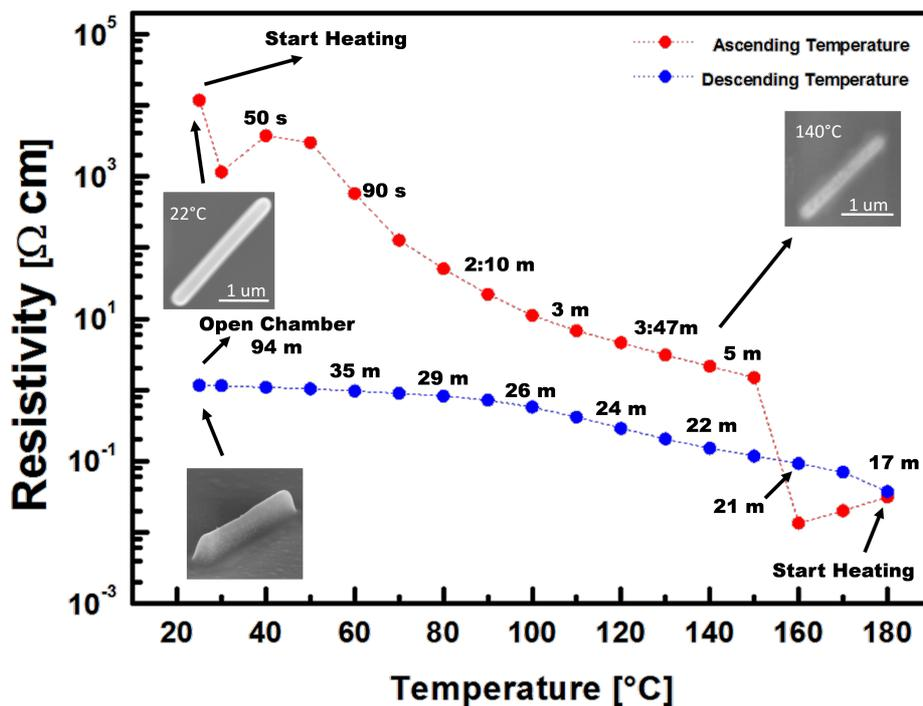
**Figure 1: Figure 8 in the original article:** Calculated resistivity from the resistance measurement of a Cu–C line during in situ post-growth heating with a hot plate (red dots) and cooling down (blue dots) inside the SEM chamber. The resistance did not change when opening the chamber. The top SEM images show the morphology changes of an adjacent FEBID line which was observed simultaneously during the in situ resistance measurement.
