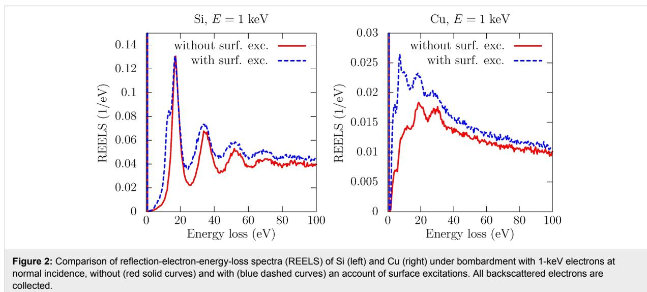
**Figure 2:** Comparison of reflection-electron-energy-loss spectra (REELS) of Si (left) and Cu (right) under bombardment with 1-keV electrons at normal incidence, without (red solid curves) and with (blue dashed curves) an account of surface excitations. All backscattered electrons are collected.
