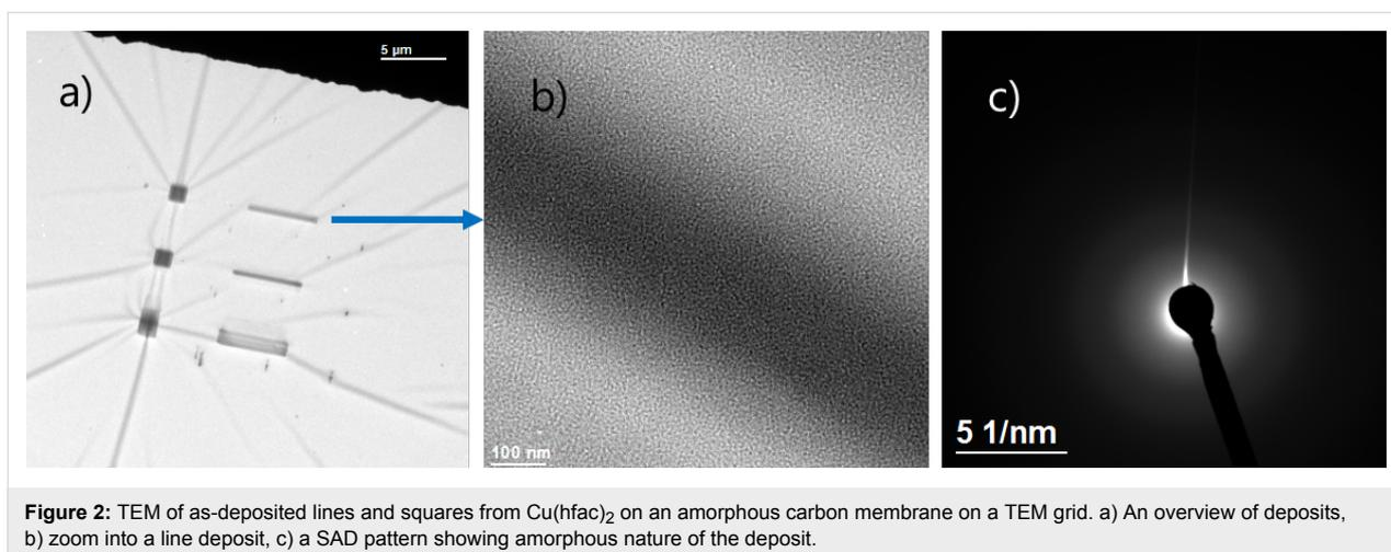
**Figure 2:** TEM of as-deposited lines and squares from  $\text{Cu}(\text{hfac})_2$  on an amorphous carbon membrane on a TEM grid. a) An overview of deposits, b) zoom into a line deposit, c) a SAD pattern showing amorphous nature of the deposit.
