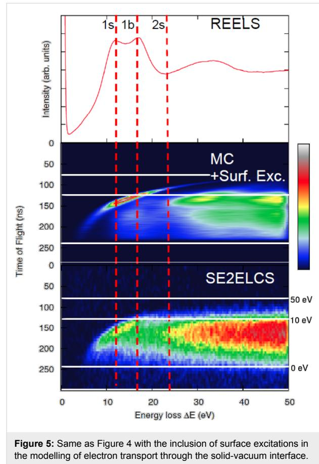
**Figure 5:** Same as Figure 4 with the inclusion of surface excitations in the modelling of electron transport through the solid-vacuum interface.
