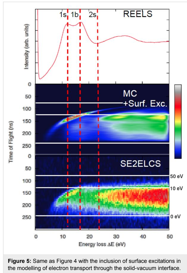
**Figure 5:** Same as Figure 4 with the inclusion of surface excitations in the modelling of electron transport through the solid-vacuum interface.
