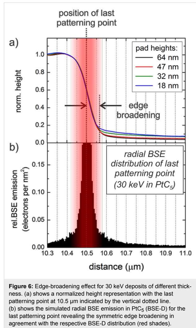
**Figure 6:** Edge-broadening effect for 30 keV deposits of different thickness. (a) shows a normalized height representation with the last patterning point at 10.5  $\mu\text{m}$  indicated by the vertical dotted line. (b) shows the simulated radial BSE emission in  $\text{PtC}_5$  (BSE-D) for the last patterning point revealing the symmetric edge broadening in agreement with the respective BSE-D distribution (red shades).
