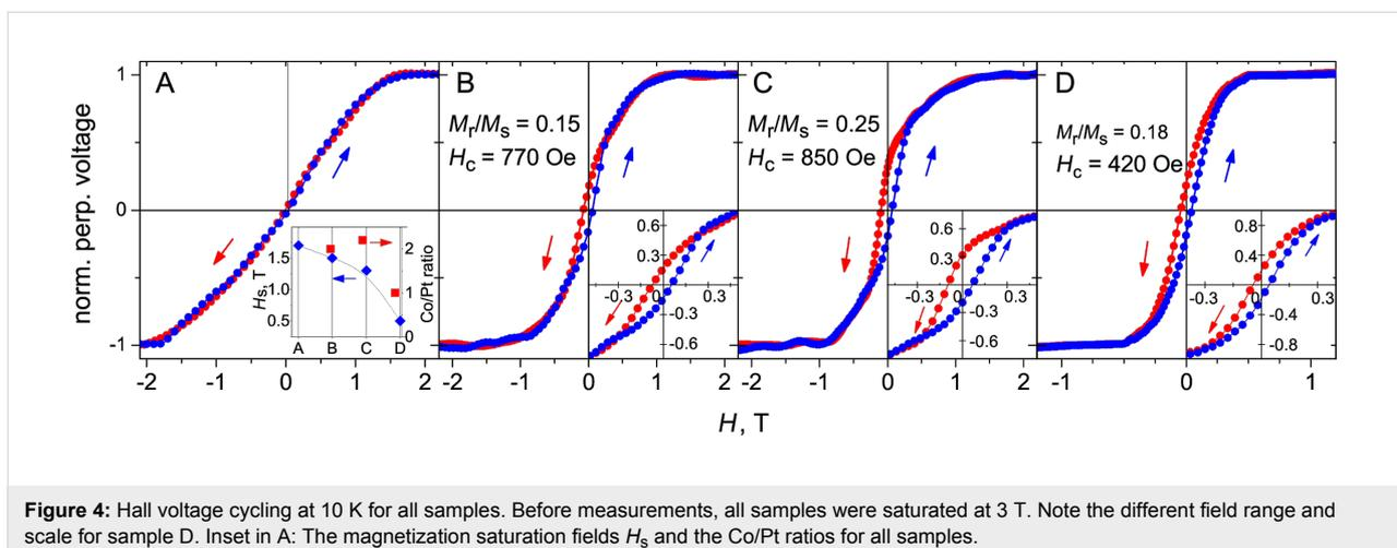
trate into the Pt layer during the Co deposition and to form a Co/Pt alloy phase. Considering the Co–Pt binary phase diagram [47], for a Co/Pt-ratio of 1:1, the CoPt L<sub>10</sub> phase can form. This phase is a hard ferromagnet whose presence can explain both, the reduction of the saturation field as well as the appearance of a hysteresis loop in samples B and C.
