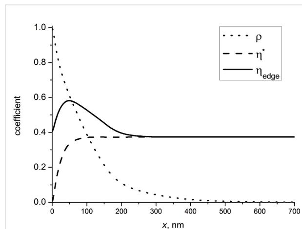
**Figure 11:** Dependence of the coefficients on the distance from the edge of the step: reflection coefficient from upper surface (dashed line), ion transmission probability (dotted line) and the total reflection coefficient calculated with Equation 11 (solid line) (angle of incidence was  $10^\circ$ ).
