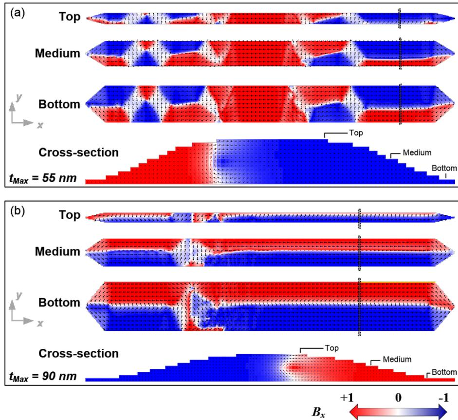
**Figure 10:** Magnetization vector-color maps extracted from the simulations for 250 nm wide Fe nanowires with bell-shaped profile (case II) and nominal thicknesses of (a) 30 nm and (b) 50 nm. The areas marked with black lines in the  $x,y$  plane representations have been chosen for the representation in the  $y,z$  plane (cross-section).
