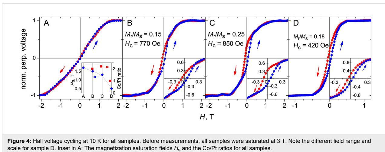
**Figure 4:** Hall voltage cycling at 10 K for all samples. Before measurements, all samples were saturated at 3 T. Note the different field range and scale for sample D. Inset in A: The magnetization saturation fields  $H_s$  and the Co/Pt ratios for all samples.
