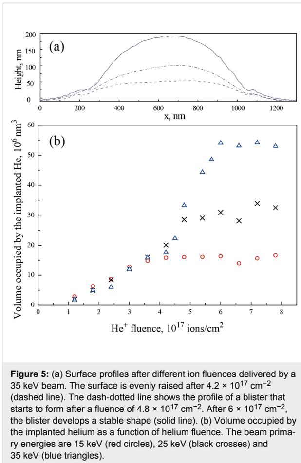
$(15.8 \pm 0.3) \times 10^6 \text{ nm}^3$ . In the case of 35 keV ions, after a fluence of  $4.2 \times 10^{17} \text{ cm}^{-2}$  a more rapid expansion begins. Later, when the fluence reaches  $6 \times 10^{17} \text{ cm}^{-2}$ , the volume saturates at  $(54.2 \pm 0.4) \times 10^6 \text{ nm}^3$ . For the energy of 25 keV the rapid expansion sets in at the same fluence, but saturates at an intermediate level of  $(30.5 \pm 0.9) \times 10^6 \text{ nm}^3$ .
