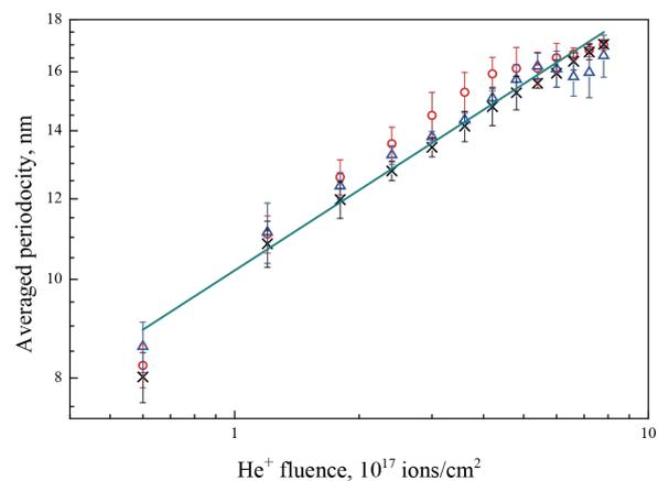
**Figure 4:** Dependence of the Au{111} average pattern periodicity on helium fluence for 15 keV (red circles), 25 keV (black crosses) and 35 keV (blue triangles) He<sup>+</sup> beams.
