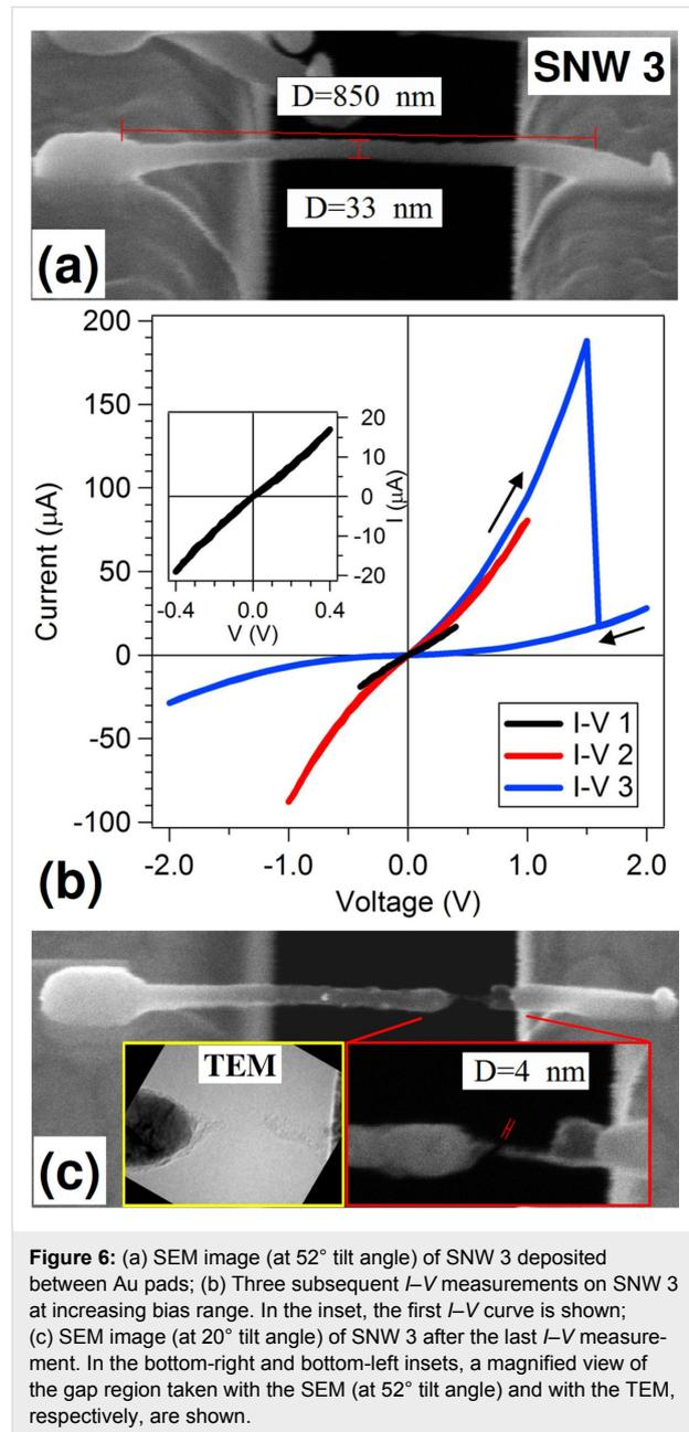
**Figure 6:** (a) SEM image (at  $52^\circ$  tilt angle) of SNW 3 deposited between Au pads; (b) Three subsequent  $I$ - $V$  measurements on SNW 3 at increasing bias range. In the inset, the first  $I$ - $V$  curve is shown; (c) SEM image (at  $20^\circ$  tilt angle) of SNW 3 after the last  $I$ - $V$  measurement. In the bottom-right and bottom-left insets, a magnified view of the gap region taken with the SEM (at  $52^\circ$  tilt angle) and with the TEM, respectively, are shown.
