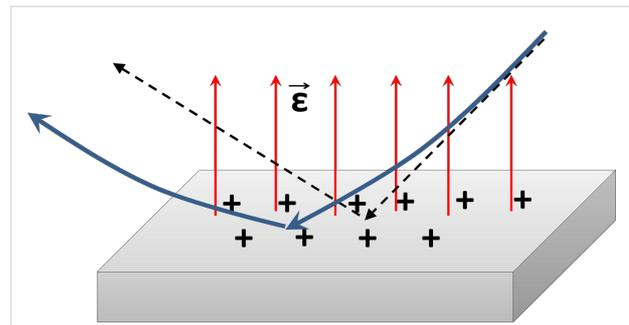
**Figure 13:** Reflection of ions from the charged surface. Trajectories of ions reflected from a charged surface (solid blue line) and trajectories of ions reflected from a neutral surface (dashed black line).
