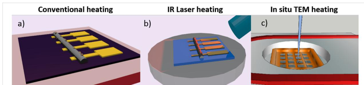
**Figure 1:** Sketch of post-growth annealing experiments: a) conventional heating using a hot plate in an SEM, b) SEM integrated laser heating; the substrate is heated by the IR laser pulses, c) post-growth thermal annealing during in situ TEM analysis. Conventional and IR laser annealing experiments were combined with in situ four-point probe resistance measurements.
