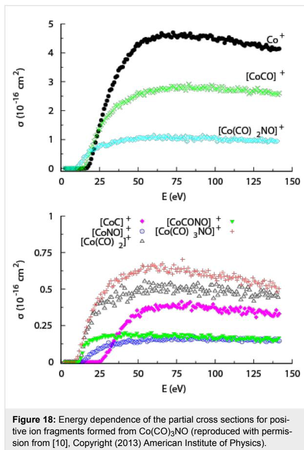
**Figure 18:** Energy dependence of the partial cross sections for positive ion fragments formed from  $\text{Co}(\text{CO})_3\text{NO}$  (reproduced with permission from [10], Copyright (2013) American Institute of Physics).
