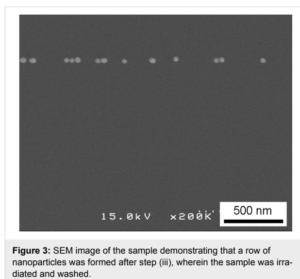
**Figure 3:** SEM image of the sample demonstrating that a row of nanoparticles was formed after step (iii), wherein the sample was irradiated and washed.
