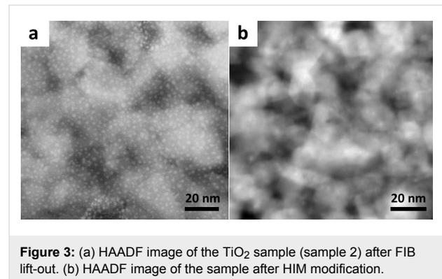
**Figure 3:** (a) HAADF image of the TiO<sub>2</sub> sample (sample 2) after FIB lift-out. (b) HAADF image of the sample after HIM modification.
