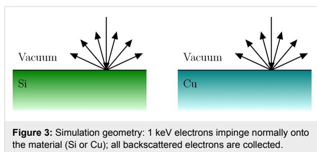
**Figure 3:** Simulation geometry: 1 keV electrons impinge normally onto the material (Si or Cu); all backscattered electrons are collected.
