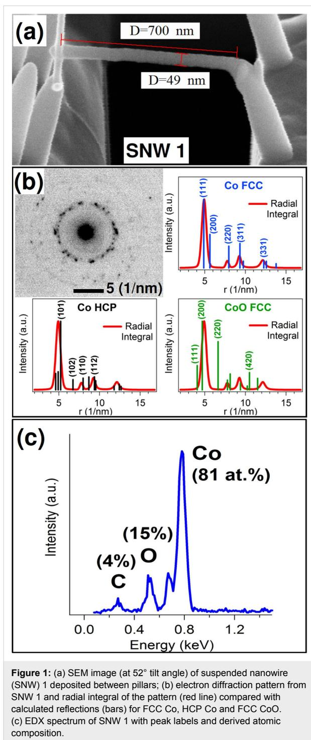
high-intensity ring with many single spots, and outer, fainter rings with spots apparently randomly arranged. This kind of pattern is typical of nanocrystalline materials with randomly oriented nanograins. To establish the structure of these nanograins the radial integral of the pattern (red curve) was compared to the main reflections calculated for face-centered cubic (FCC) Co, hexagonal close-packed (HCP) Co and FCC
