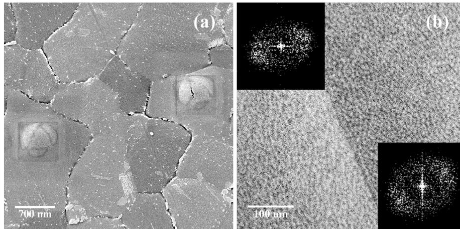
**Figure 3:** (a) Two blisters created by the 35 keV He<sup>+</sup> beam on grains with different azimuthal orientation. FOV is 4 μm. (b) HIM SE image of a Au{111} textured polycrystalline film. The insets are 2D FFTs to demonstrate the relation of the patterns to the orientation of the two grains. He<sup>+</sup> beam energy is 35 keV. FOV is 500 nm.
