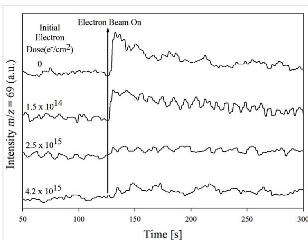
**Figure 15:** Time-resolved mass spectra of gas phase  $\text{PF}_3$  (positive  $[\text{PF}_2]^+$  ions produced by 70 eV electron impact) desorbing from films of  $\text{Pt}(\text{PF}_3)_4$  adsorbed on an Au surface at 180 K when these are irradiated with 500 eV electrons. The time at which the electron beam is turned on is represented with a vertical line. Reproduced with permission from [23], Copyright (2011) American Chemical Society.
