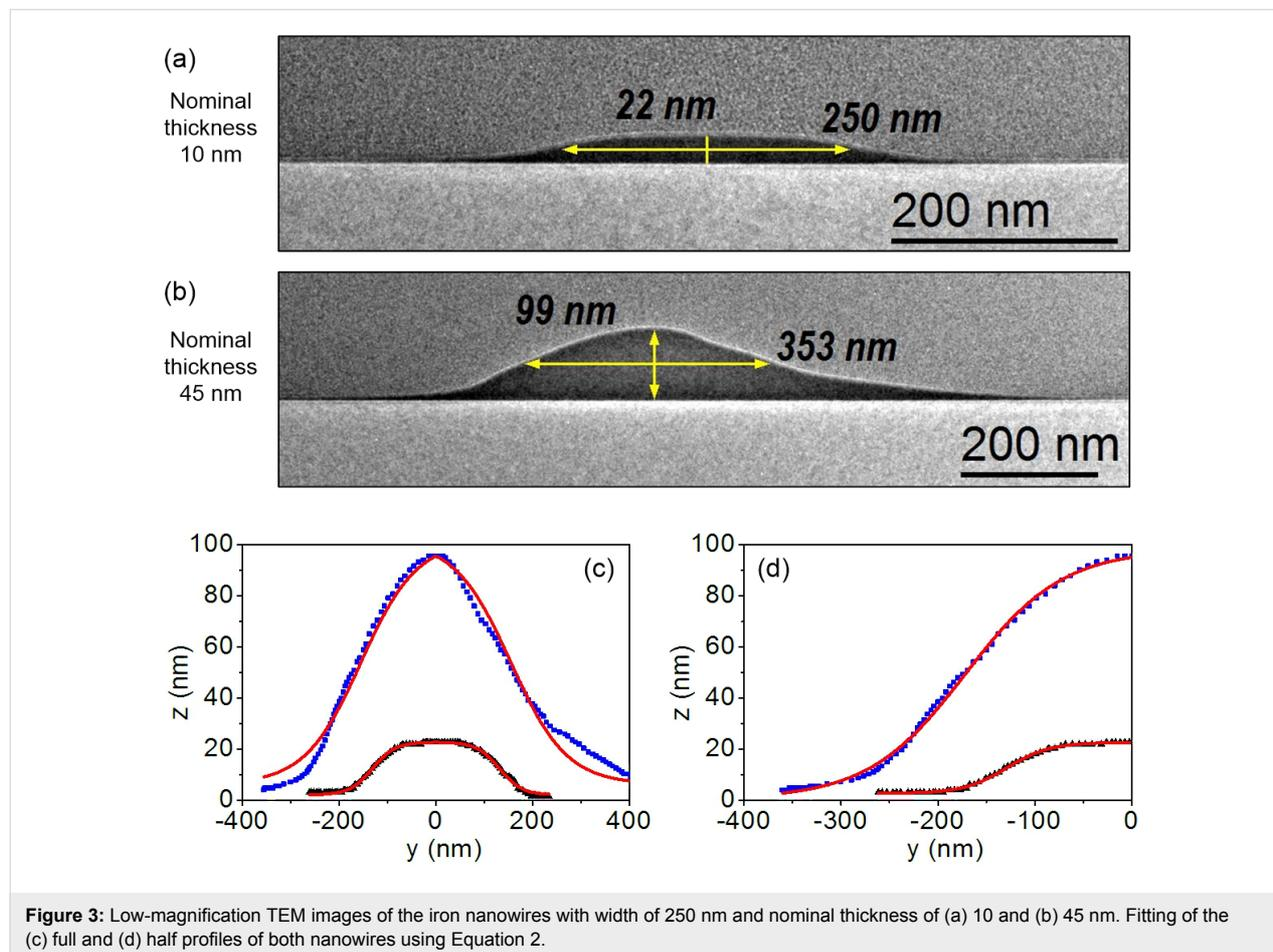
**Figure 3:** Low-magnification TEM images of the iron nanowires with width of 250 nm and nominal thickness of (a) 10 and (b) 45 nm. Fitting of the (c) full and (d) half profiles of both nanowires using Equation 2.
