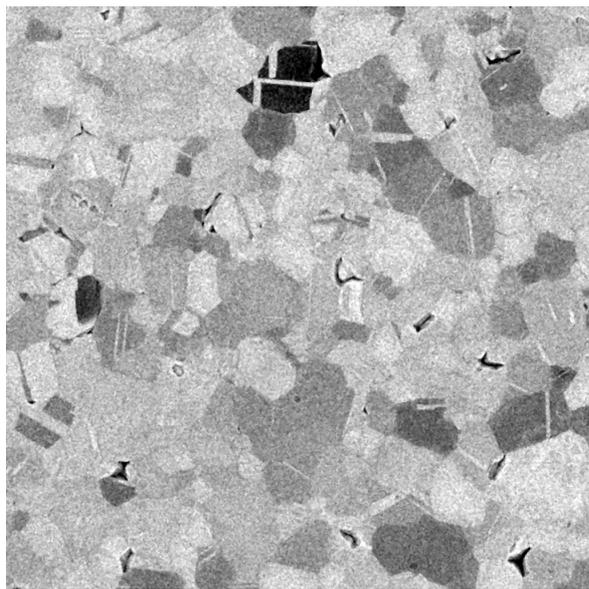
**Figure 2:** HIM BSHE images of the hydrogen-flame-annealed polycrystalline Au{111} film. A PE of 20 keV and an ion dose of  $1.11 \times 10^{15} \text{ cm}^{-2}$  has been used. The stage tilt was  $0^\circ$ . FOV:  $15 \mu\text{m}$ .
