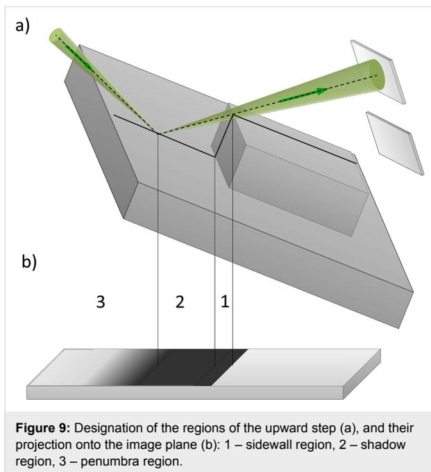
In region 1 in Figure 9 all ions are reflected by the step sidewall away from the aperture and do not contribute to the detected signal,  $S(\alpha) = 0$ . In this case, a dark area of width  $d_1 = h\cos\Theta_0$  appears in the image, where  $h$  is the step height.
