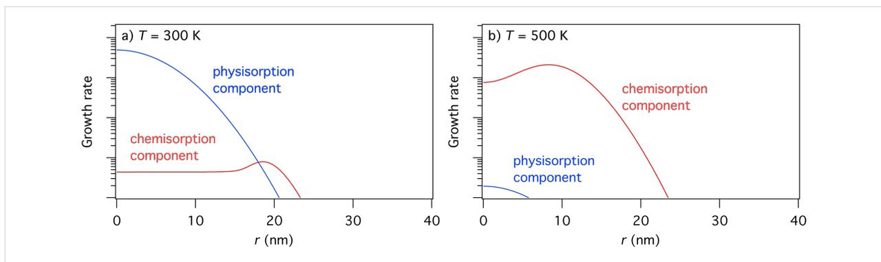
**Figure 19:** FEBID growth rates simulated using Equation 75 and Equation 76, a Gaussian electron-beam profile ( $\Omega = 5$  nm) and substrate temperatures of (a) 300 K and (b) 500 K. (Deposition precursor = TEOS,  $f_0 = 10^3 \text{ \AA}^{-2}\text{s}^{-1}$ ,  $P = 0.1$  Torr,  $T_g = 300$  K,  $E_{D_p} = 0.17$  eV,  $E_{D_c} = 0.472$  eV,  $\kappa_{D_p} = \kappa_{D_c} = 10^{11} \text{ \AA}^{-2}\text{s}^{-1}$  all other model input parameters were the same as in [5].)
