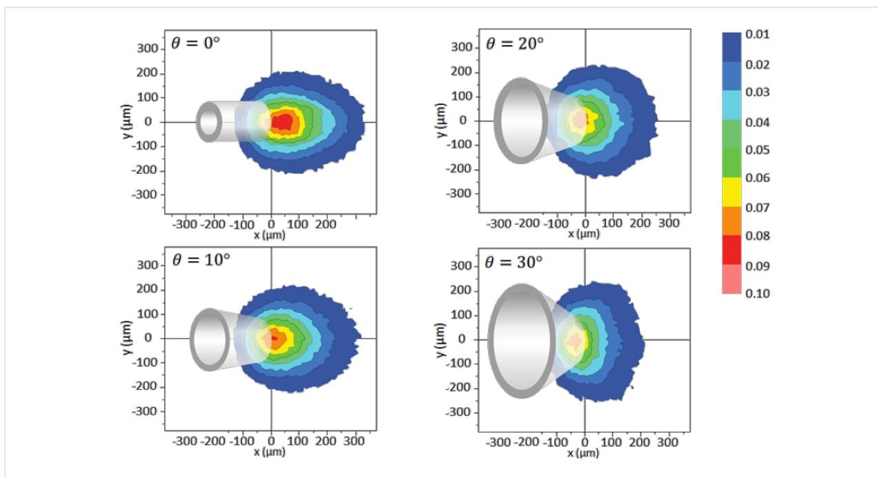
reduced capillary length  $L_r$  can be entered instead, still giving accurate results. For molecular flow conditions, the spatial distribution of impinging molecules on the substrate is not significantly altered for lengths  $L_r > 15d$ . For transient flow conditions, the reduced length depends on  $\lambda$  with  $L_r = 3\lambda$  to  $5\lambda$  [31,33].
