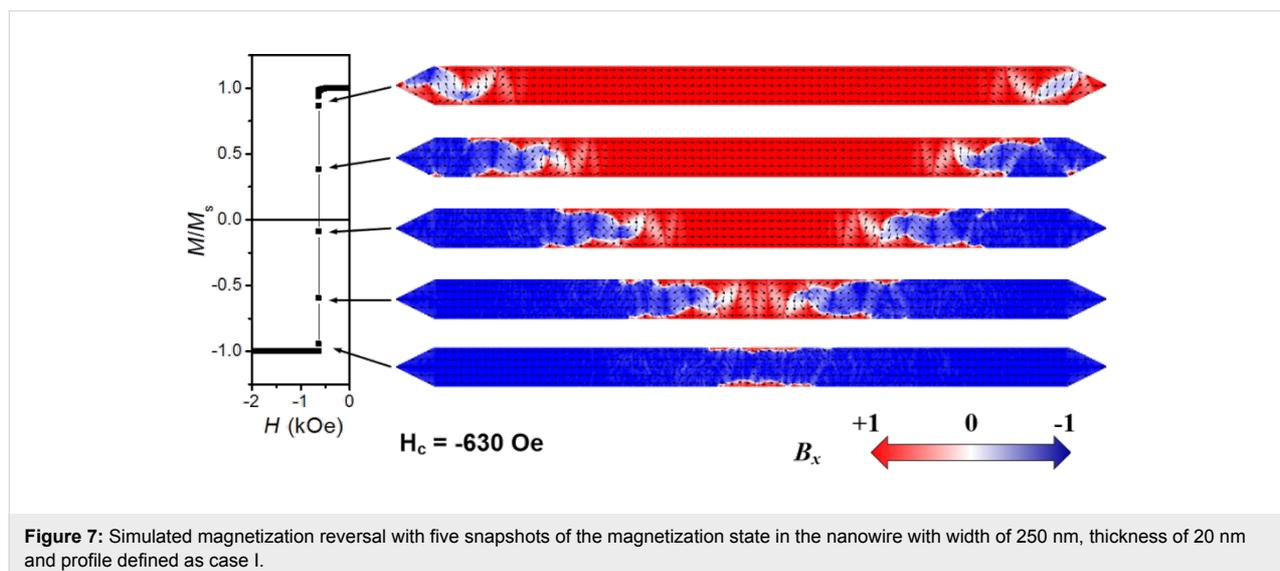
**Figure 7:** Simulated magnetization reversal with five snapshots of the magnetization state in the nanowire with width of 250 nm, thickness of 20 nm and profile defined as case I.
