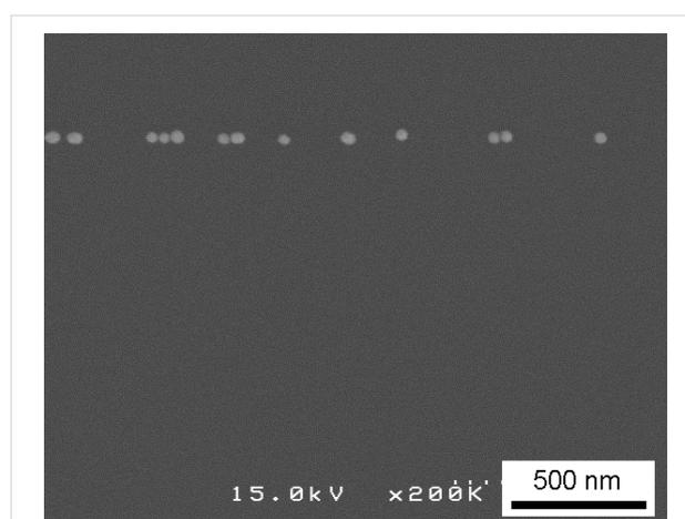
**Figure 3:** SEM image of the sample demonstrating that a row of nanoparticles was formed after step (iii), wherein the sample was irradiated and washed.
