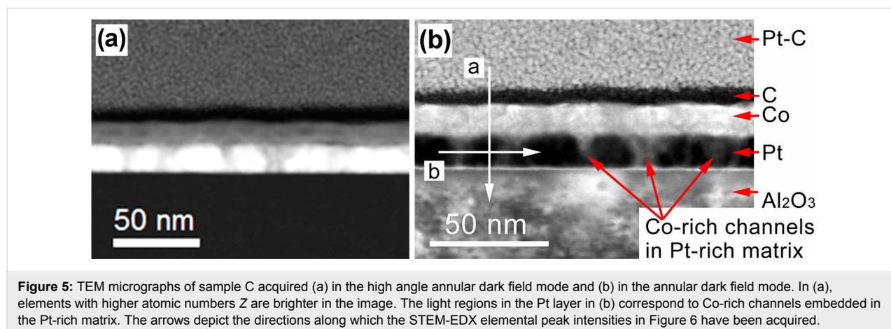
**Figure 5:** TEM micrographs of sample C acquired (a) in the high angle annular dark field mode and (b) in the annular dark field mode. In (a), elements with higher atomic numbers  $Z$  are brighter in the image. The light regions in the Pt layer in (b) correspond to Co-rich channels embedded in the Pt-rich matrix. The arrows depict the directions along which the STEM-EDX elemental peak intensities in Figure 6 have been acquired.
