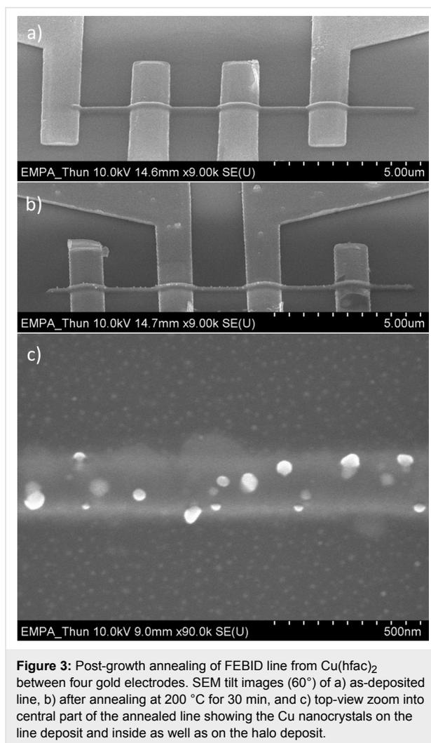
Interestingly, the size of the nanocrystals is much smaller in the thin halo region of the deposited line, yet the nanocrystal density is much larger. This may be due to the small amount of
