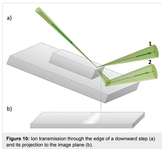
**Figure 10:** Ion transmission through the edge of a downward step (a) and its projection to the image plane (b).
