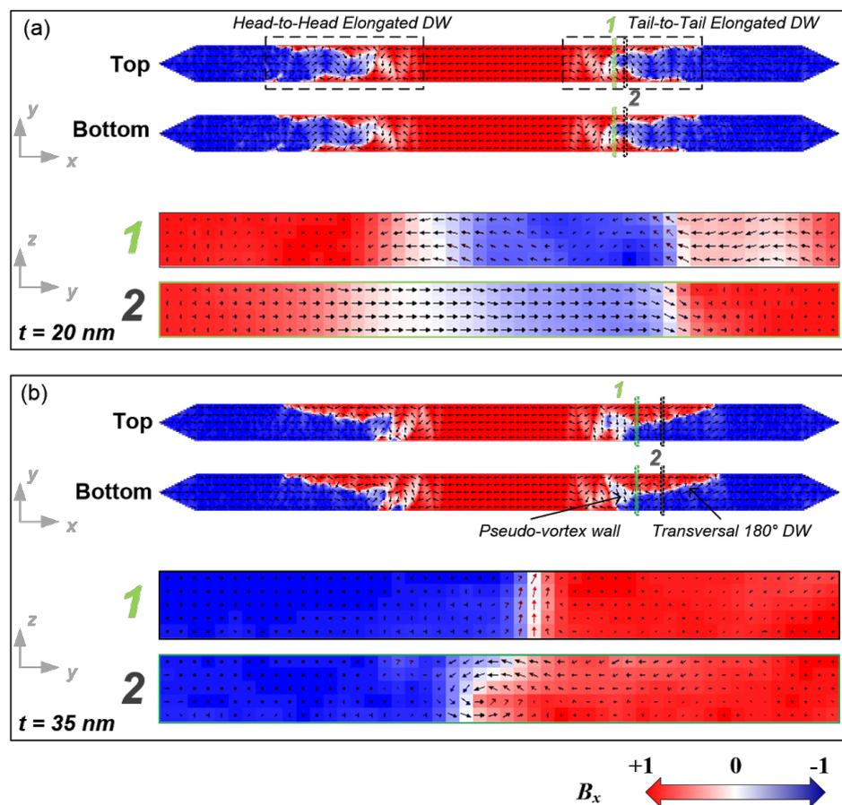
**Figure 8:** Magnetization vector-color maps extracted from the simulations for 250 nm wide Fe nanowires with rectangular profile (case I) and thickness of (a) 20 nm and (b) 35 nm. The areas named “1” (green lines) and “2” (black lines) in the  $x,y$  plane representations have been chosen for the representation in the  $y,z$  plane.
