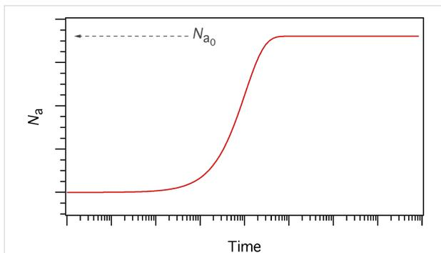
**Figure 3:** Adsorbate concentration ( $N_a$ ) versus time in the absence of electron irradiation (here,  $N_a = 0$  at  $t = 0$ ).  $N_{a_0}$  is the steady state adsorbate concentration in the absence of electron irradiation, which is used as the initial adsorbate concentration input into FEBIP models.  $N_a(t)$  and  $N_{a_0}$  are given by Equation 6 and Equation 7, respectively.
