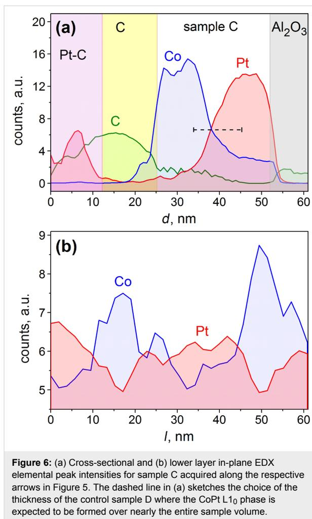
**Figure 6:** (a) Cross-sectional and (b) lower layer in-plane EDX elemental peak intensities for sample C acquired along the respective arrows in Figure 5. The dashed line in (a) sketches the choice of the thickness of the control sample D where the CoPt L<sub>10</sub> phase is expected to be formed over nearly the entire sample volume.
