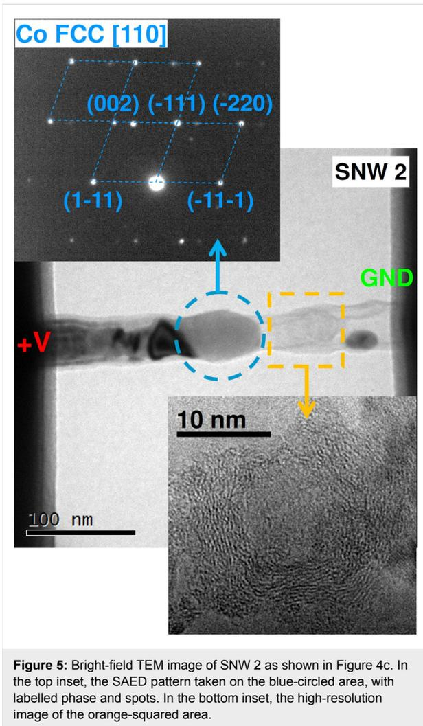
**Figure 5:** Bright-field TEM image of SNW 2 as shown in Figure 4c. In the top inset, the SAED pattern taken on the blue-circled area, with labelled phase and spots. In the bottom inset, the high-resolution image of the orange-squared area.
