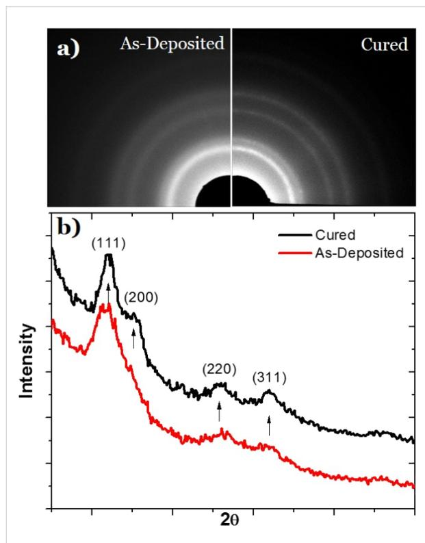
**Figure 7:** Selected area electron diffraction (SAED) patterns for O<sub>2</sub> E-beam uncured (left) and cured (right) deposit. Diffraction peaks become more pronounced after curing.
