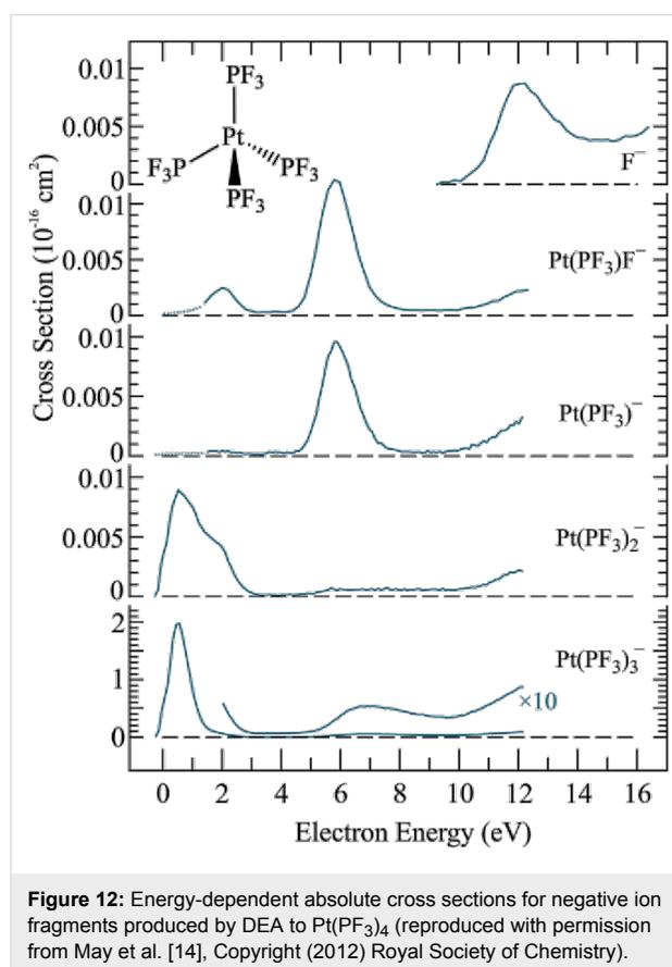
**Figure 12:** Energy-dependent absolute cross sections for negative ion fragments produced by DEA to  $\text{Pt}(\text{PF}_3)_4$  (reproduced with permission from May et al. [14], Copyright (2012) Royal Society of Chemistry).
