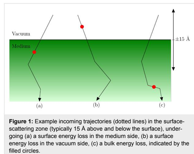
**Figure 1:** Example incoming trajectories (dotted lines) in the surface-scattering zone (typically 15 Å above and below the surface), undergoing (a) a surface energy loss in the medium side, (b) a surface energy loss in the vacuum side, (c) a bulk energy loss, indicated by the filled circles.
