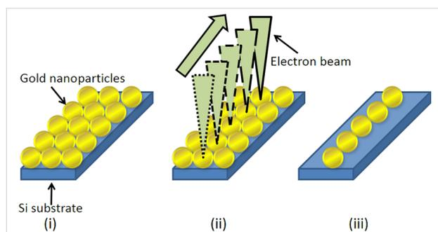
**Figure 1:** Schematic illustration of the proposed technique. (i) A two-dimensional array of gold nanoparticles is formed on a substrate. (ii) Selected nanoparticles are irradiated with the electron beam to fix these particles on the substrate. (iii) The unfixed particles are washed away, creating an array of nanoparticles.
