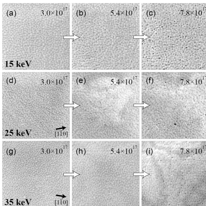
**Figure 2:** HIM SE images of the pattern that develops on the Au{111} surface as a function of ion fluence. Numbers indicate the ion fluence in helium ions per  $\text{cm}^2$ . Arrows in (d) and (g) indicate the azimuthal directions of the grains. The He<sup>+</sup> beam energies are 15, 25 and 35 keV. FOV is 500 nm, pixel spacing is 0.68 nm.
