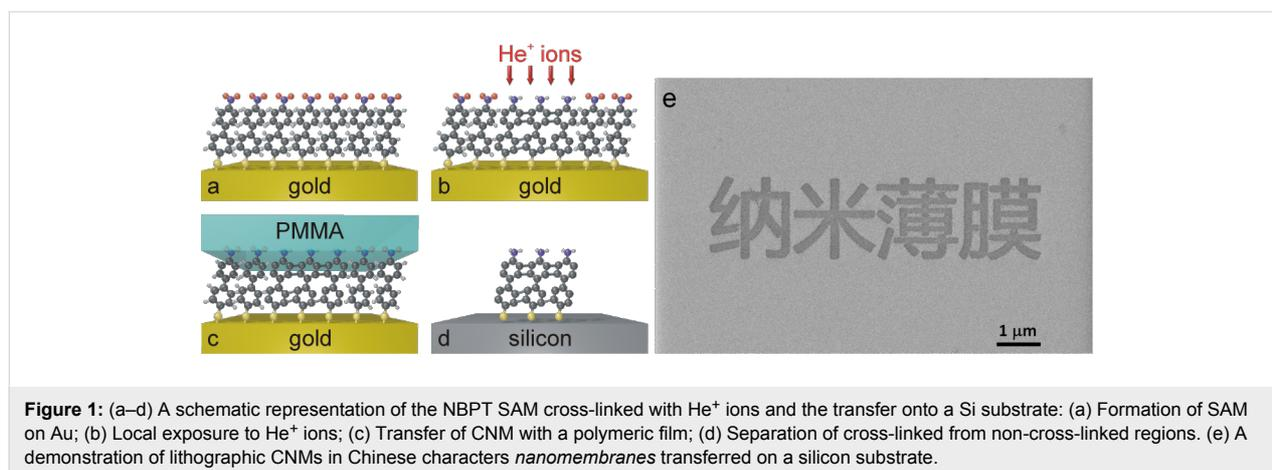
**Figure 1:** (a–d) A schematic representation of the NBPT SAM cross-linked with  $\text{He}^+$  ions and the transfer onto a Si substrate: (a) Formation of SAM on Au; (b) Local exposure to  $\text{He}^+$  ions; (c) Transfer of CNM with a polymeric film; (d) Separation of cross-linked from non-cross-linked regions. (e) A demonstration of lithographic CNMs in Chinese characters *nanomembranes* transferred on a silicon substrate.
