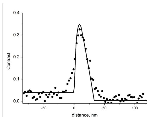
**Figure 12:** Profile of the relative contrast of a downward step: dots – experimental data, solid line – data calculated with SRIM software. Zero corresponds to the reflection from bulk  $\text{SiO}_2$ .
