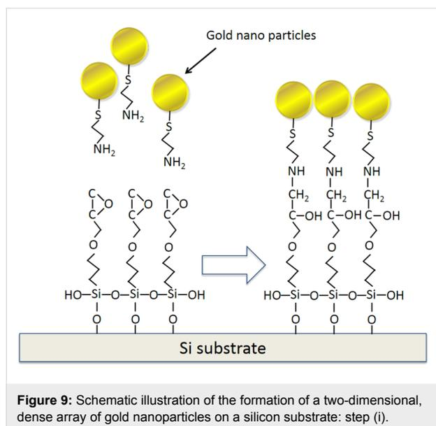
**Figure 9:** Schematic illustration of the formation of a two-dimensional, dense array of gold nanoparticles on a silicon substrate: step (i).
