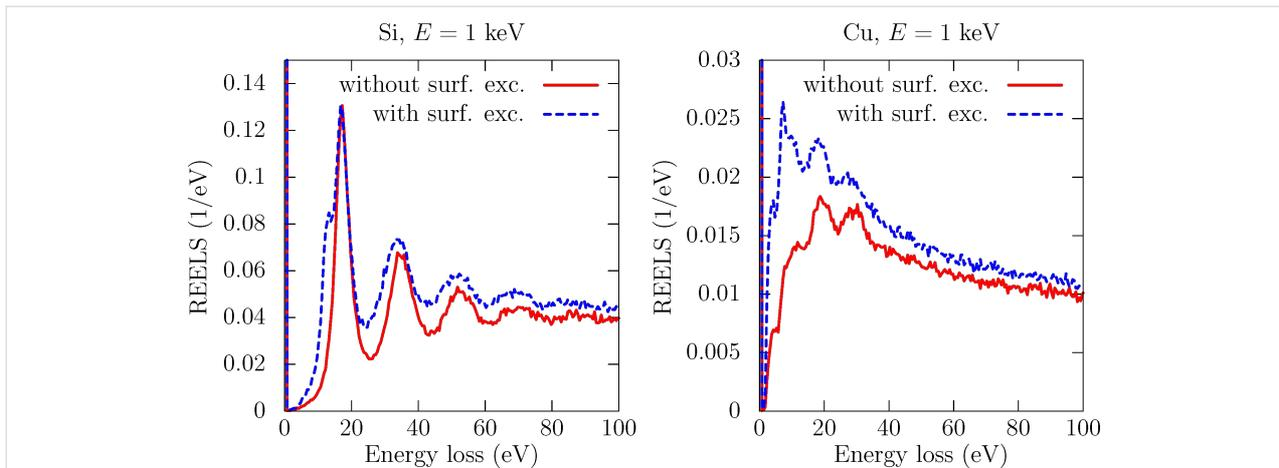
**Figure 2:** Comparison of reflection-electron-energy-loss spectra (REELS) of Si (left) and Cu (right) under bombardment with 1-keV electrons at normal incidence, without (red solid curves) and with (blue dashed curves) an account of surface excitations. All backscattered electrons are collected.
