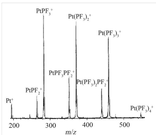
**Figure 13:** Electron ionization FT-ICR mass spectrum of  $\text{Pt}(\text{PF}_3)_4$  recorded at 20 eV incident electron energy (reproduced with permission from [22], Copyright (1997) American Chemical Society).
