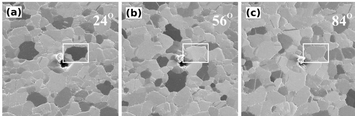
**Figure 1:** HIM SE images of the hydrogen-flame-annealed polycrystalline Au{111} film taken with a PE of 15 keV and an ion dose of  $4.9 \times 10^{14} \text{ cm}^{-2}$ . Relative sample rotation angles around the surface normal are  $24^\circ$ ,  $56^\circ$  and  $84^\circ$ . The polar angle is fixed at  $35^\circ$ . FOV:  $10 \mu\text{m}$ .
