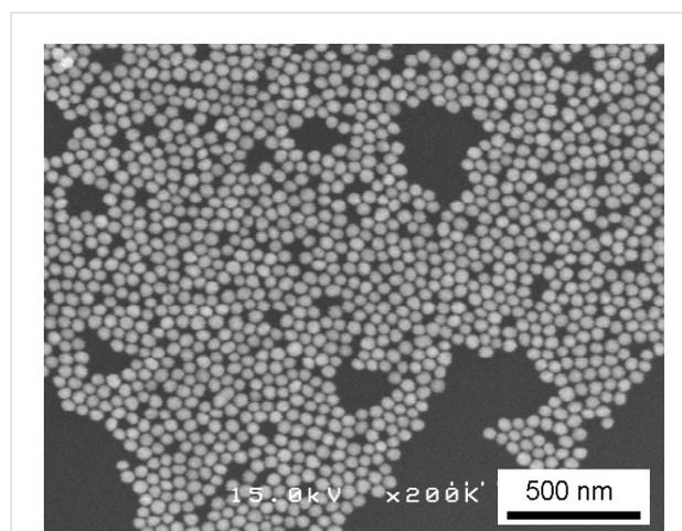
**Figure 2:** SEM image of the substrate after step (i) using the amine-epoxy method.
