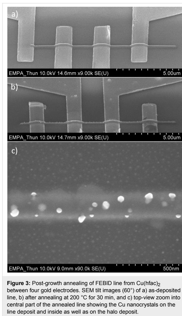
**Figure 3:** Post-growth annealing of FEBID line from  $\text{Cu}(\text{hfac})_2$  between four gold electrodes. SEM tilt images (60°) of a) as-deposited line, b) after annealing at 200 °C for 30 min, and c) top-view zoom into central part of the annealed line showing the Cu nanocrystals on the line deposit and inside as well as on the halo deposit.
