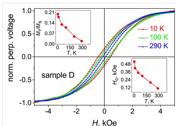
**Figure 8:** Isothermal Hall voltage cycling for sample D at a series of temperatures, as indicated. Insets: Temperature dependencies of the squareness  $M_r/M_s$  and the coercive field  $H_c$  for sample D. The lines are guides for the eye.
