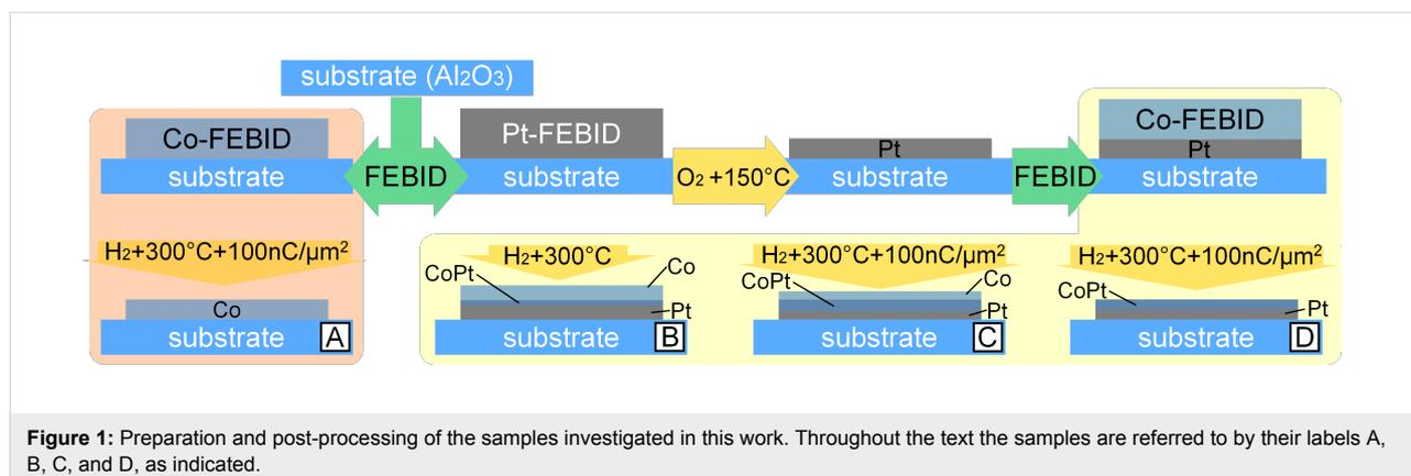
**Figure 1:** Preparation and post-processing of the samples investigated in this work. Throughout the text the samples are referred to by their labels A, B, C, and D, as indicated.
