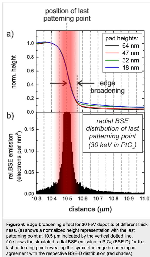
**Figure 6:** Edge-broadening effect for 30 keV deposits of different thickness. (a) shows a normalized height representation with the last patterning point at 10.5  $\mu\text{m}$  indicated by the vertical dotted line. (b) shows the simulated radial BSE emission in  $\text{PtC}_5$  (BSE-D) for the last patterning point revealing the symmetric edge broadening in agreement with the respective BSE-D distribution (red shades).
