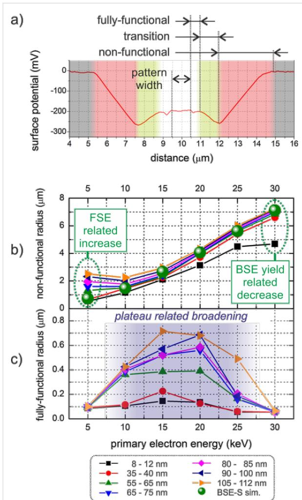
**Figure 5:** (a) Functional classification of proximity deposition based on KFM measurements. (b) and (c) show the energy- and thickness-dependent radii of the non-functional and the fully-functional radius, respectively. A detailed explanation is given in the main text.
