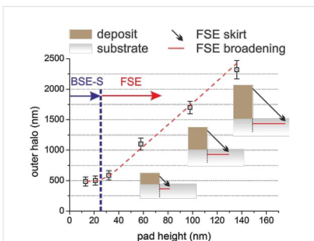
**Figure 8:** Outer-halo behavior for increasing pad thicknesses of 5 keV deposits (squares) together with an FSE-related scheme to explain the linear increase for thicker deposits (details are given in the main text).
