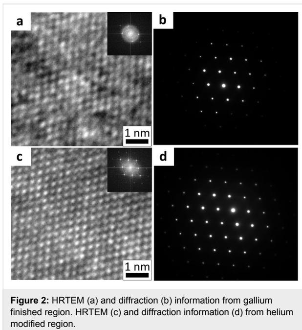
**Figure 2:** HRTEM (a) and diffraction (b) information from gallium finished region. HRTEM (c) and diffraction information (d) from helium modified region.
