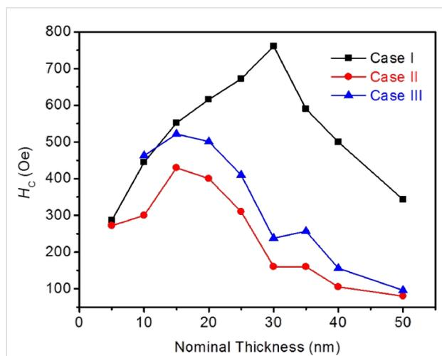
**Figure 6:** Coercive field ( $H_C$ ) obtained from the simulations of iron nanowires with nominal width of 250 nm and varying nominal thickness (from 5 to 50 nm) for the three cases discussed in the text.
