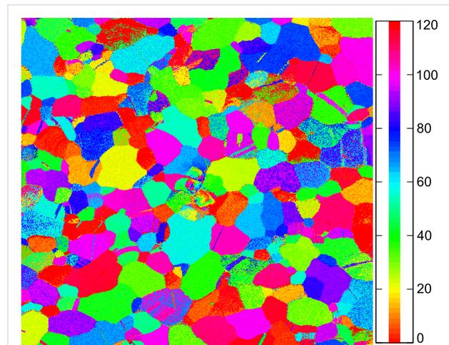
**Figure 6:** Color-coded orientation map of a polycrystalline gold film. The colors indicate the azimuthal angle around the  $[111]$  surface normal for a  $35^\circ$  sample tilt at which a  $\langle 110 \rangle$  direction is aligned with the incoming helium ion beam. Parts of the data set used are presented in Figure 1.
