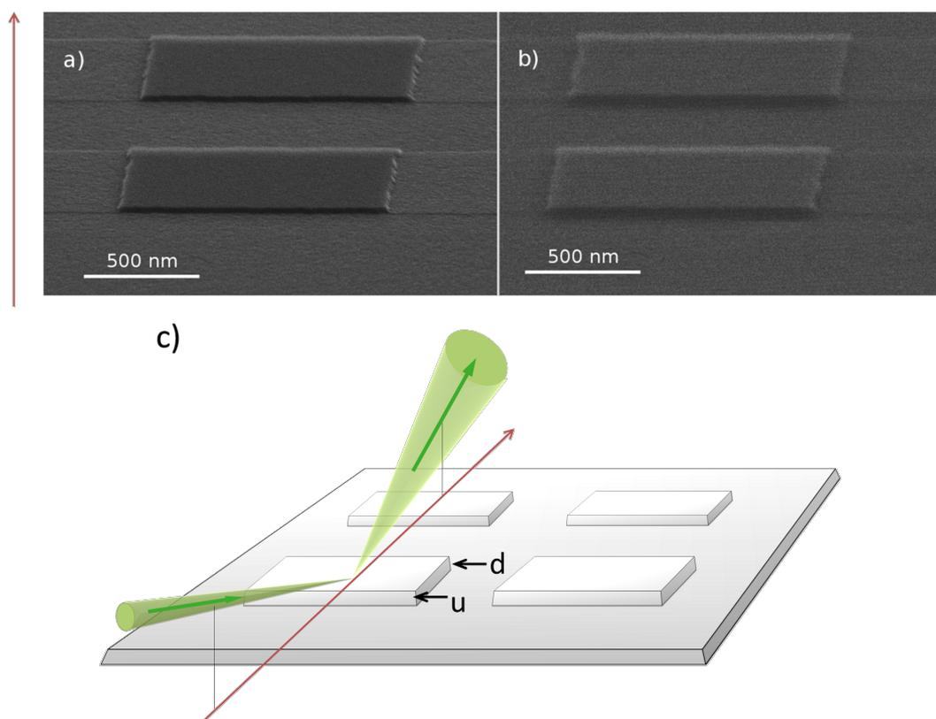
**Figure 4:** Images of silicon dioxide bars on silicon (TGQ-1 sample) obtained by detection of (a) secondary electrons, (b) reflected ions. (c) Sketch of ion beam path: green arrows correspond to the direction of the primary beam and reflected beam, the red axis corresponds to the vertical axis of the images in (a) and (b). “Upward” and “downward” steps are marked with “u” and “d”, respectively.
