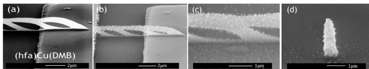
**Figure 5:** Periodic 3D FEBID line deposits from  $(\text{hfac})\text{Cu}(\text{DMB})$  between gold electrodes on  $\text{SiO}_2/\text{Si}$ . SEM tilt images: a) before annealing, b) after in situ vacuum annealing, c) zoom on Cu nanocrystals, d) tip deposit showing also Cu nanocrystal formation.
