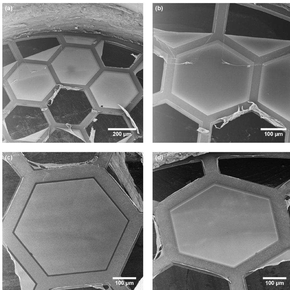
**Figure 3:** Examples of large freestanding CNMs. (a, b) Three intact CNMs are imaged at different magnifications. (c, d) Another intact CNM is imaged at different tilt angles. This comparison reveals that the intensity variation on the CNM surface originates mostly from secondary electrons emitted by the sample holder. Detailed information on all HIM images is given in Supporting Information File 1, Tables S1 and S2.
