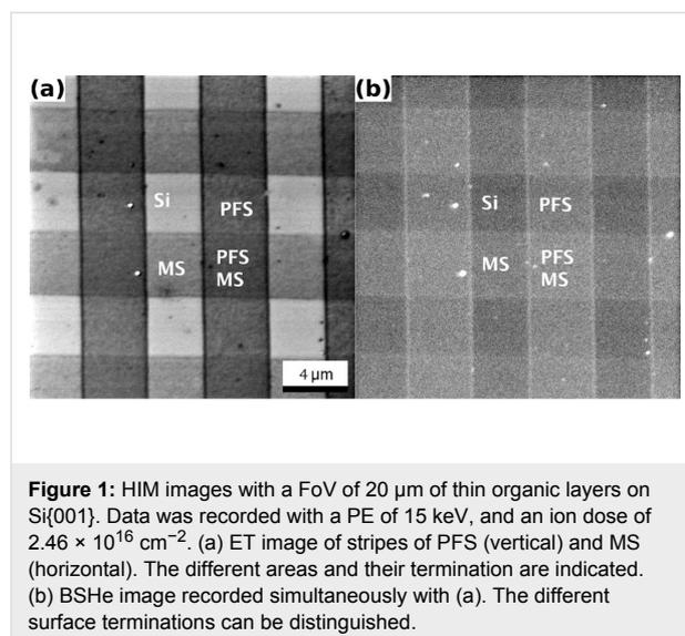
**Figure 1:** HIM images with a FoV of  $20 \mu\text{m}$  of thin organic layers on  $\text{Si}\{001\}$ . Data was recorded with a PE of 15 keV, and an ion dose of  $2.46 \times 10^{16} \text{ cm}^{-2}$ . (a) ET image of stripes of PFS (vertical) and MS (horizontal). The different areas and their termination are indicated. (b) BShe image recorded simultaneously with (a). The different surface terminations can be distinguished.
