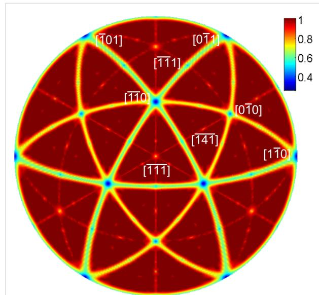
**Figure 5:** Calculated map of channeling directions for an fcc crystal. The lines connecting the nodes at low-index directions in the polar plot represent channeling directions in the used thin slab of an fcc crystal. The color coding (opaque fraction) allows a qualitative interpretation of the width and depth of the scattering minima.
