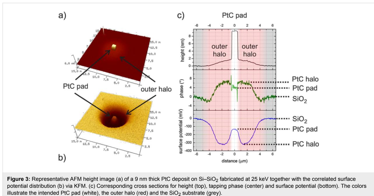
**Figure 3:** Representative AFM height image (a) of a 9 nm thick PtC deposit on Si-SiO<sub>2</sub> fabricated at 25 keV together with the correlated surface potential distribution (b) via KFM. (c) Corresponding cross sections for height (top), tapping phase (center) and surface potential (bottom). The colors illustrate the intended PtC pad (white), the outer halo (red) and the SiO<sub>2</sub> substrate (grey).
