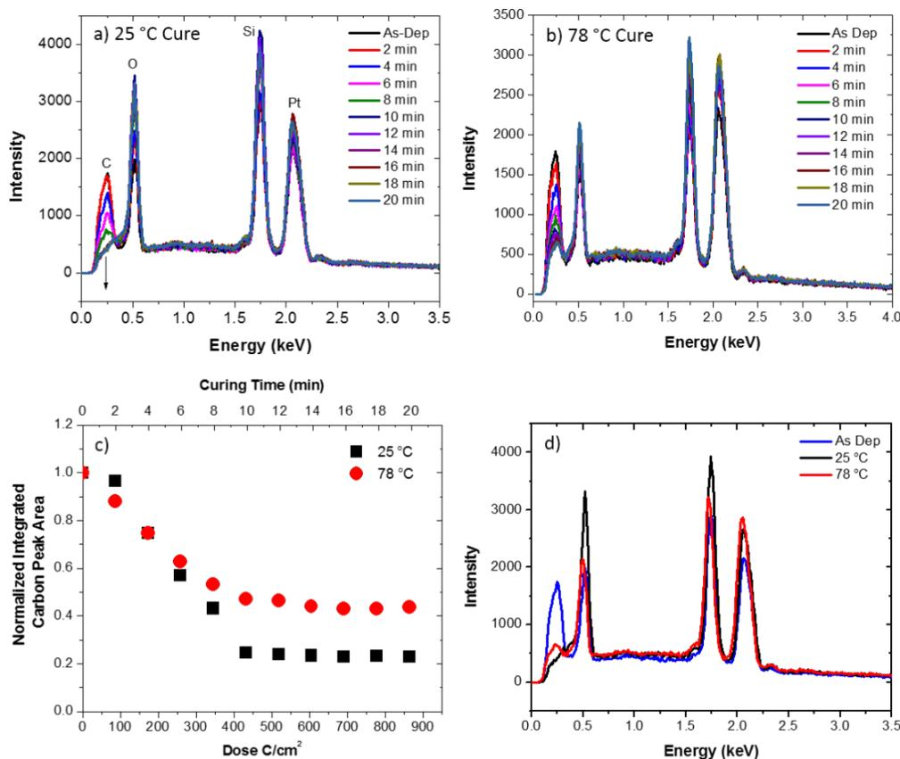
**Figure 1:** In situ EDS spectra of deposits purified using an electron beam with an energy of 5 keV, a current of 1.6 nA, a dwell time of 100 ns, and a pixel spacing of roughly 0.65 nm plotted for different purification times for the (a) 25 and (b) 78 °C O<sub>2</sub> flow studies. (c) Shows the normalized integrated Pt/C ratios as a function of purification time (top axis) and estimated received dose (bottom axis). (d) Shows the final EDS spectra after 20 min of purification.
