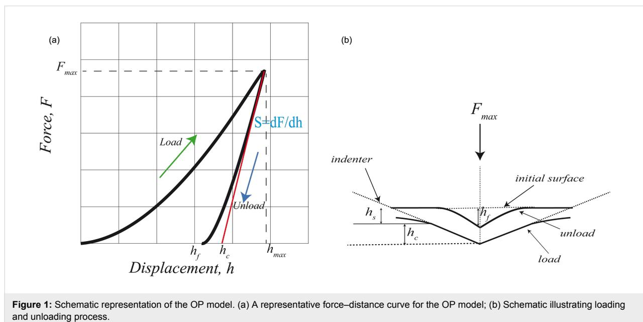
**Figure 1:** Schematic representation of the OP model. (a) A representative force–distance curve for the OP model; (b) Schematic illustrating loading and unloading process.
