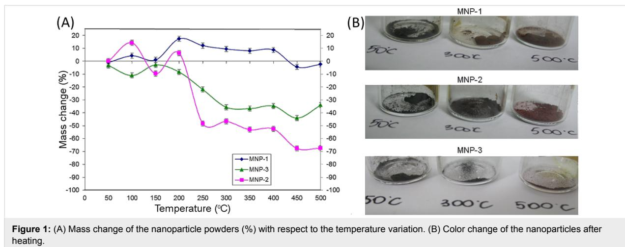
**Figure 1:** (A) Mass change of the nanoparticle powders (%) with respect to the temperature variation. (B) Color change of the nanoparticles after heating.
