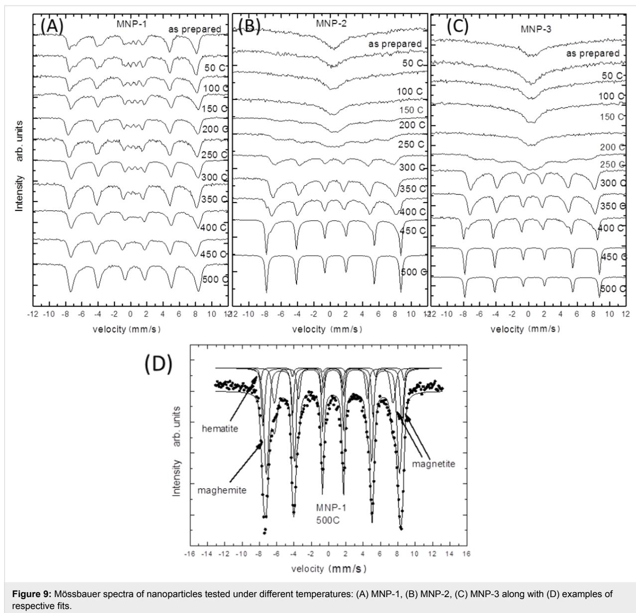
spectra consist of a sextet with a relatively wide line at half maximum, which is connected with the overlapping of the magnetite, maghemite and hematite subspectra. The quantitative analysis suggests that the relative intensity ratio of Fe in these two phases is roughly equal to 4:78:18, respectively, at 500 °C (see Figure 9D).
