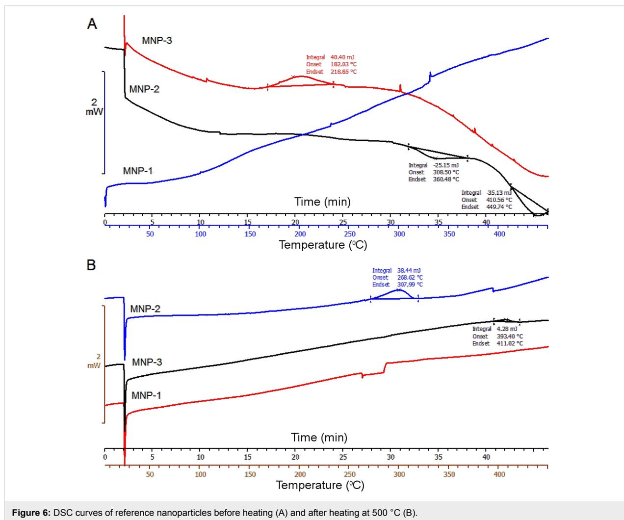
**Figure 6:** DSC curves of reference nanoparticles before heating (A) and after heating at 500 °C (B).
