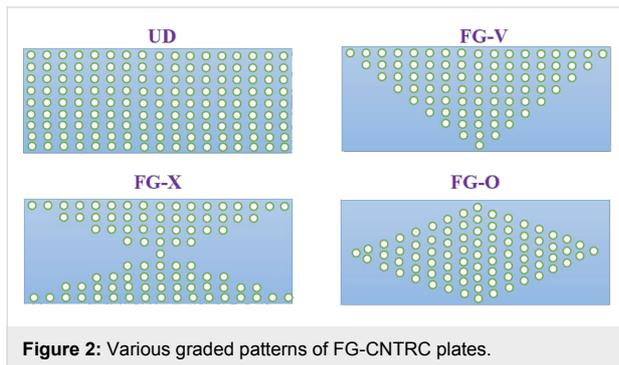
Figure 2: Various graded patterns of FG-CNTRC plates.
