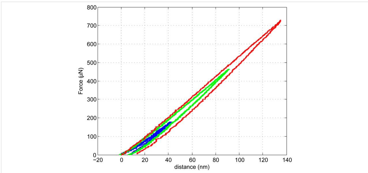
**Figure 13:** Force–distance curves on Corning Eagle Glass substrate.
