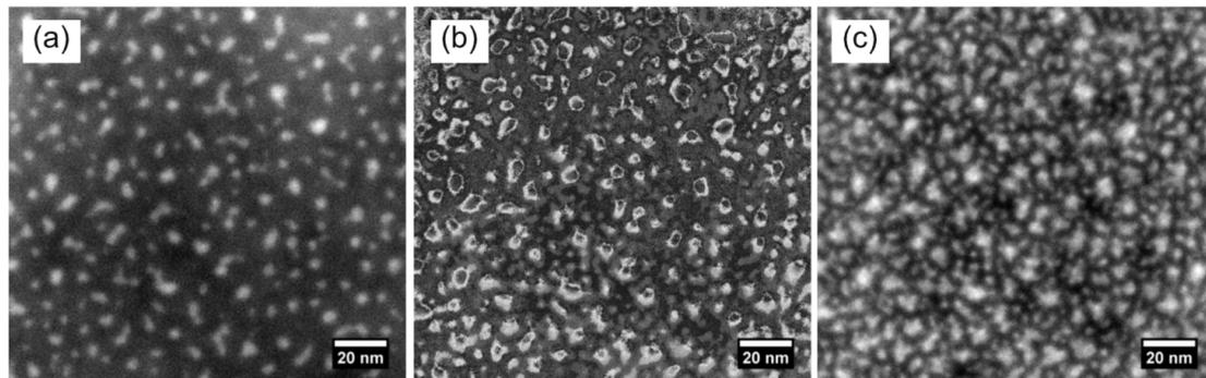
**Figure 1:** EFTEM images of S1: (a) image in fresh area, (c) after about 10 min exposure to an intense electron beam and (b) XOR image of (a) and (c) highlighting the change between the two as denoted by white regions. Nanoparticles obviously grow and even new ones are created.
