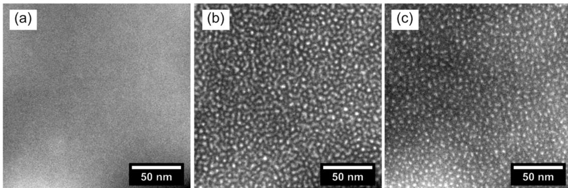
**Figure 2:** EFTEM images of reference samples S2 and S3: (a) S2 irradiated with a low dose, (b) S2 irradiated with a high dose and (c) S3 irradiated with a high dose. After low dose irradiation no Si particles are observed (cf. panel (a)), whereas high doses lead to a dense formation of tiny Si nanoparticles (cf. panels (b) and (c)).
