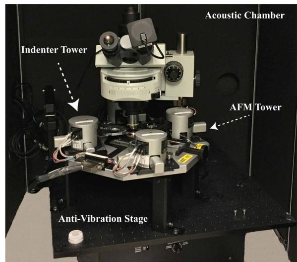
**Figure 3:** Positioning of the multi-probe system inside the acoustic chamber.
