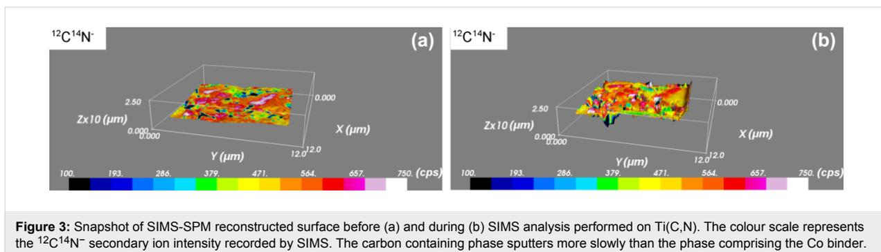
binder is sputtered at a rate of  $0.28 \text{ nm}\cdot\mu\text{m}^2\cdot\text{pA}^{-1}\cdot\text{s}^{-1}$ , compared to a sputtering rate of  $0.10 \text{ nm}\cdot\mu\text{m}^2\cdot\text{pA}^{-1}\cdot\text{s}^{-1}$  of the Ti domains. Thus, the Co binder material is sputtered 2.8 times faster than the Ti domains. The analysis was performed with a  $1.4 \text{ pA Cs}^+$  primary beam.
