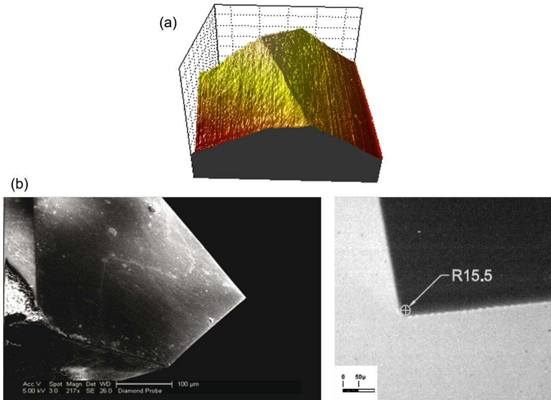
**Figure 10:** Images of cube-corner diamond tip used in nanoindentation experiments. (a) A 3D representation of AFM scan for the cube-corner diamond tip used in nanoindentation experiments. (b) SEM and TEM images of the diamond tip. The tip radius is measured as 15.5 nm.
