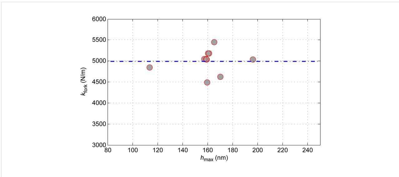
Figure 8: Spring constant vs maximum depth of penetration.
