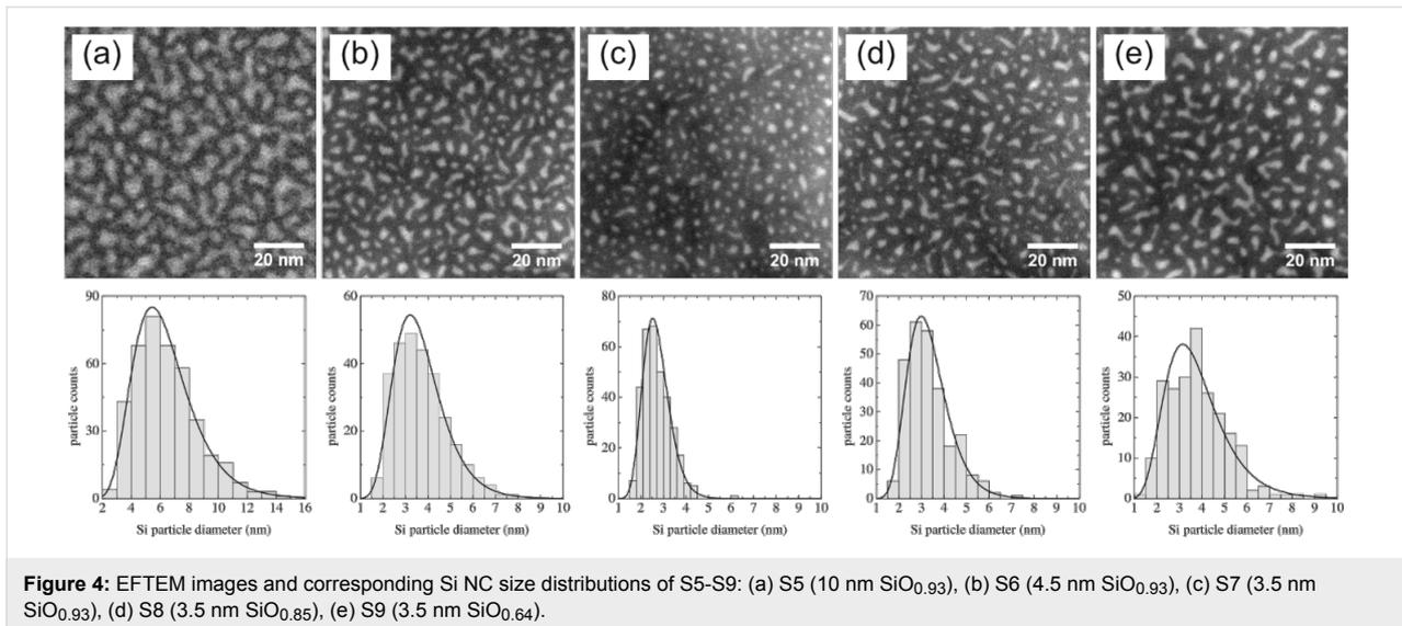
threshold for spinodal decomposition is shifted to smaller values [49,50], a fact that is experimentally demonstrated in Figure 4.
