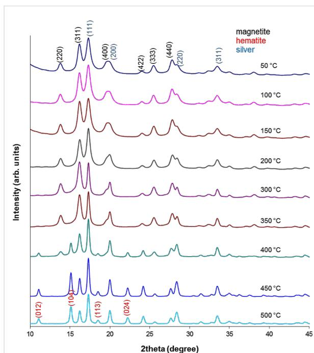
**Figure 5:** X-ray pattern of MNP-3 nanoparticles after the heating process.
