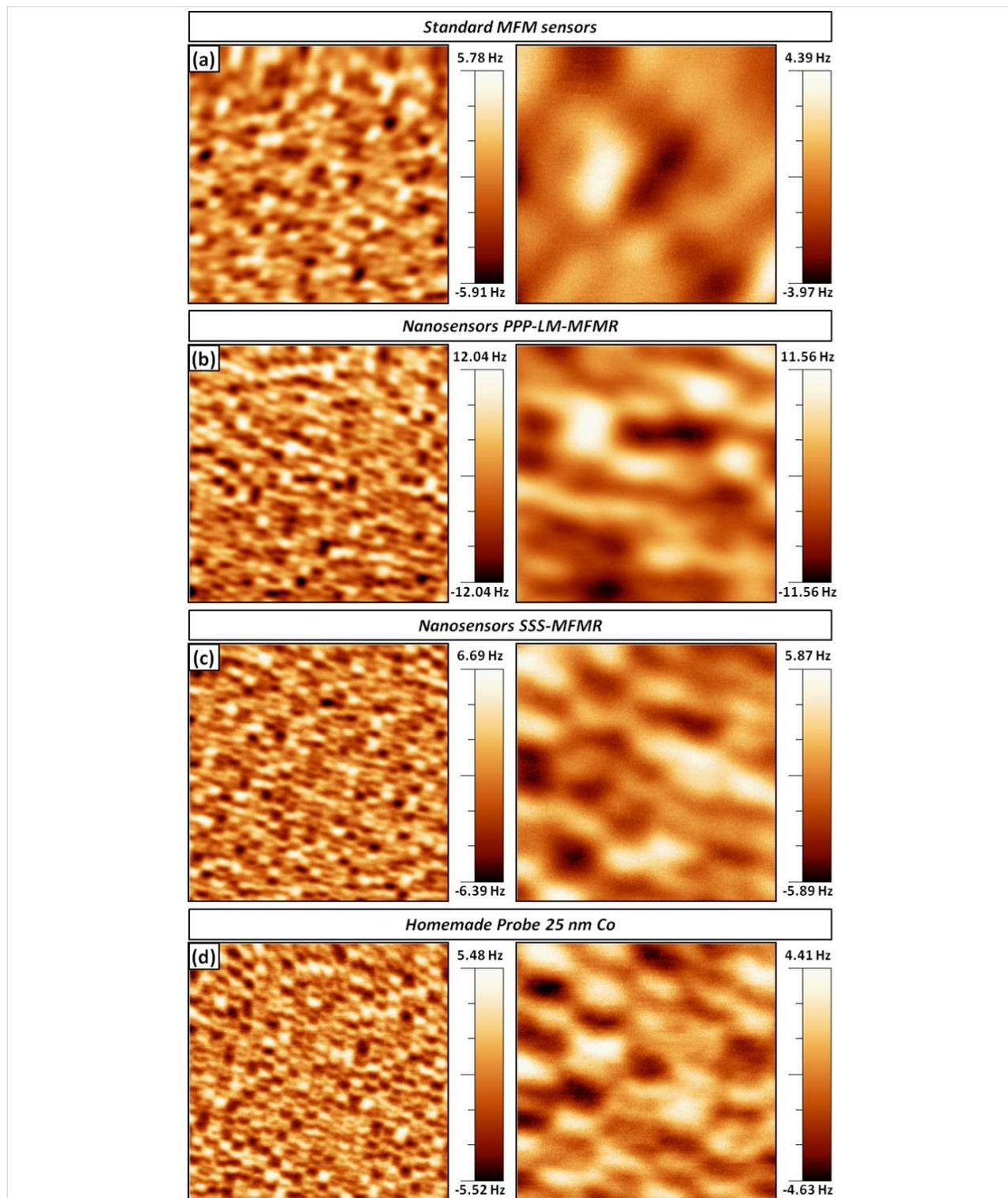
**Figure 2:** MFM images performed to show the lateral resolution obtained with commercial (a) standard, (b) low-moment and (c) super sharp probes and (d) custom-made tips with a 25 nm thick Co coating on the front sides. Images on the left/right columns are  $(2 \times 2) \mu\text{m}^2 / (500 \times 500) \text{nm}^2$ , respectively.
