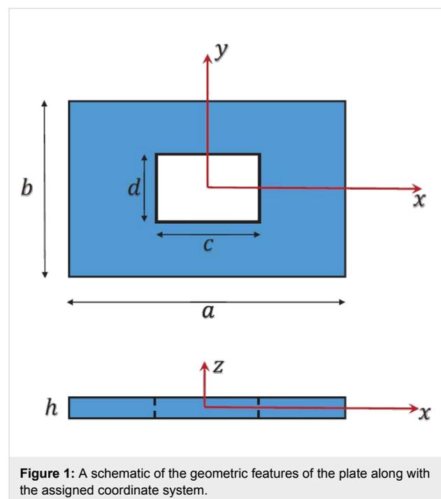
**Figure 1:** A schematic of the geometric features of the plate along with the assigned coordinate system.
