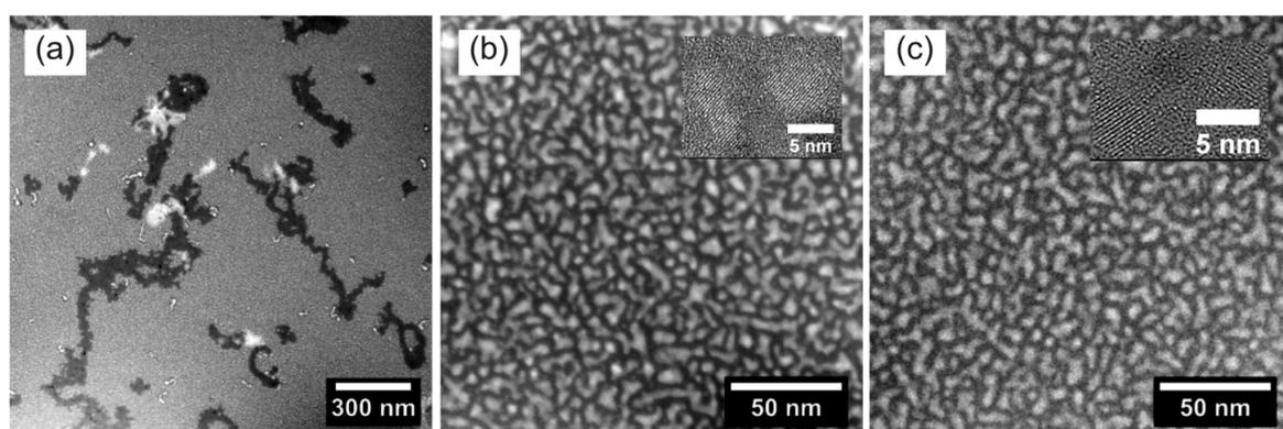
**Figure 3:** EFTEM images of S4 (a,b) and S5 (c): (a) overview image of S4 illustrating severe sample damage caused by Ar annealing, (b,c) smaller area to show that the morphology in the undamaged regions are fairly similar for both Ar and N<sub>2</sub> annealing.
