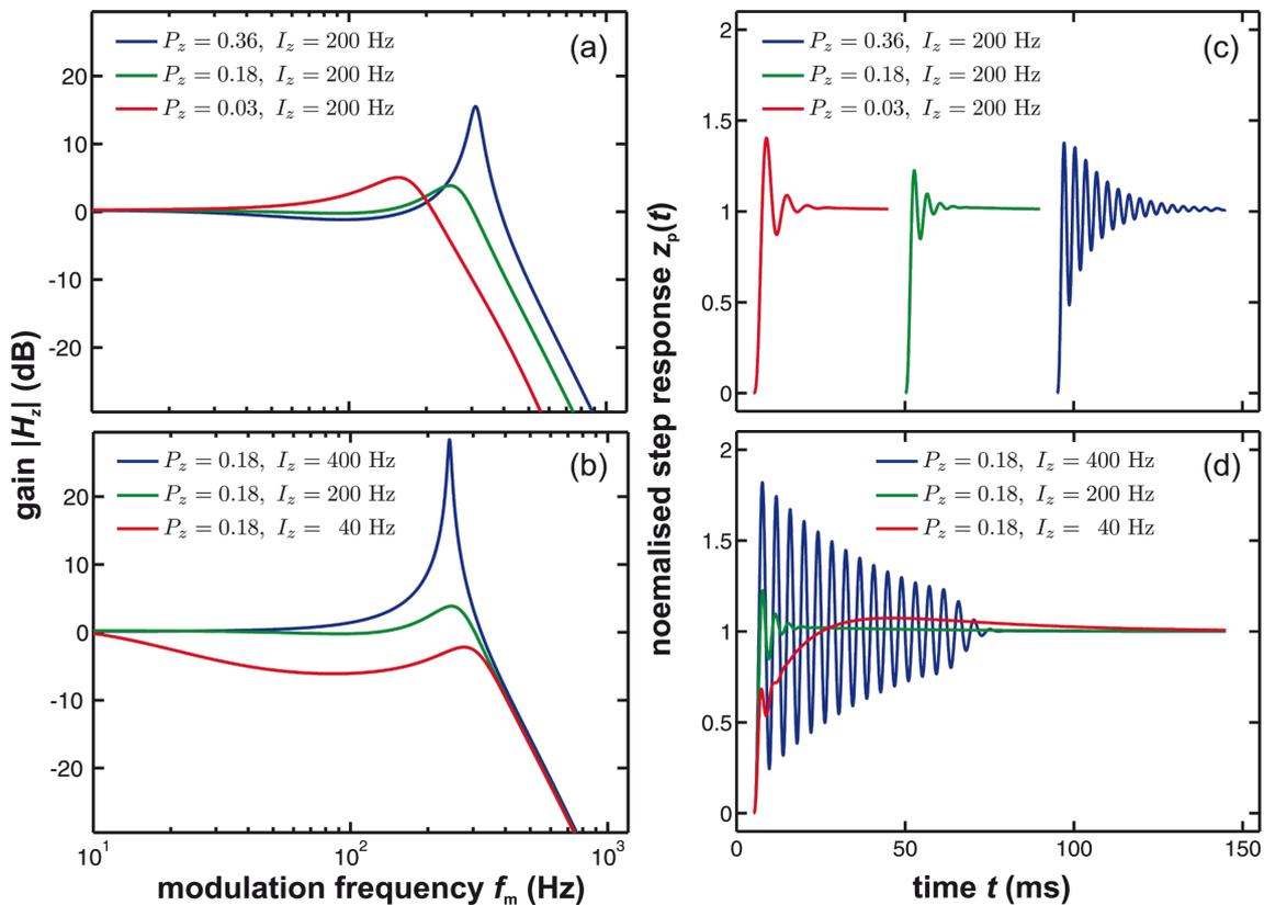
**Figure 12:** (a, b) Frequency response and (c, d) step response of the distance control loop for a given tip–sample interaction  $\beta_{ts} = 12.3$  Hz/nm and different settings of  $P_z$  and  $I_z$ . The calculations are performed using the ratio  $S_p^z / S^{\Delta f} = -0.312$  nm/Hz and for PLL settings  $P_{\text{PLL}} = -2.1$  Hz/deg,  $I_{\text{PLL}} = 1$  Hz with the loop filter  $H_{lp}$  having a 3rd-order Butterworth characteristics with a cutoff frequency of  $f_c = 500$  Hz.
