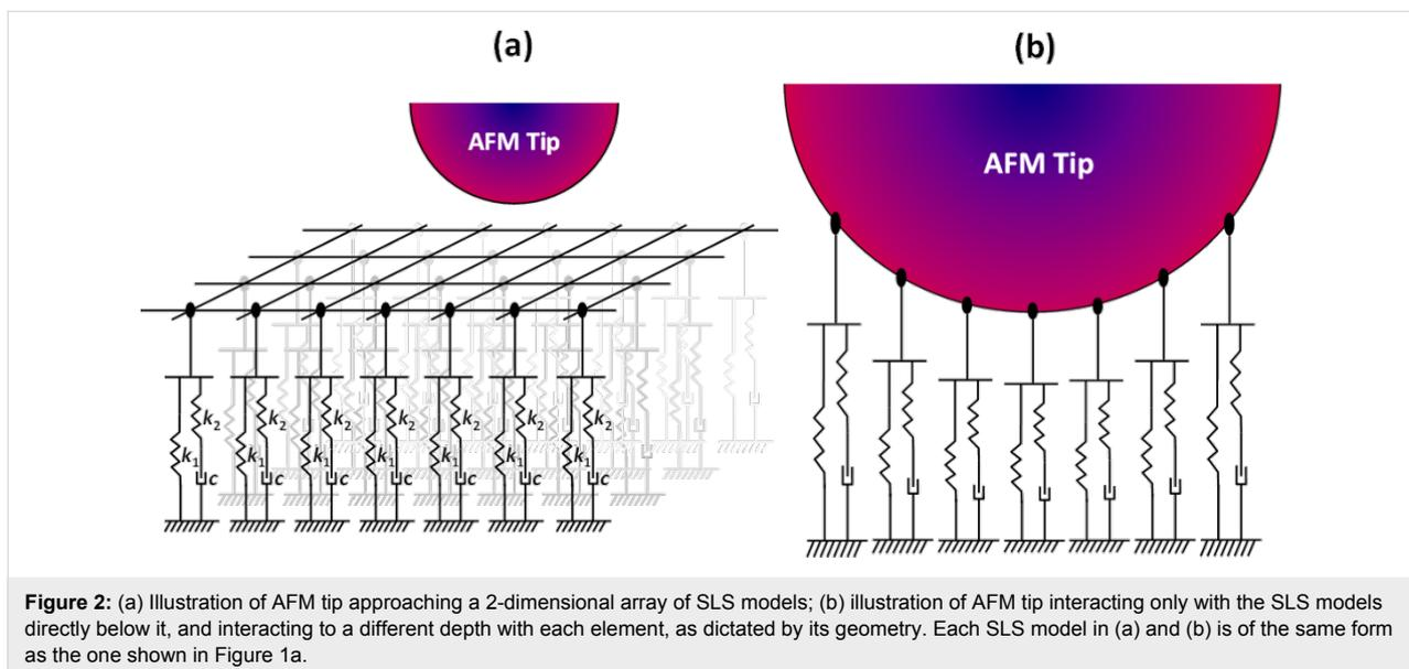
**Figure 2:** (a) Illustration of AFM tip approaching a 2-dimensional array of SLS models; (b) illustration of AFM tip interacting only with the SLS models directly below it, and interacting to a different depth with each element, as dictated by its geometry. Each SLS model in (a) and (b) is of the same form as the one shown in Figure 1a.
