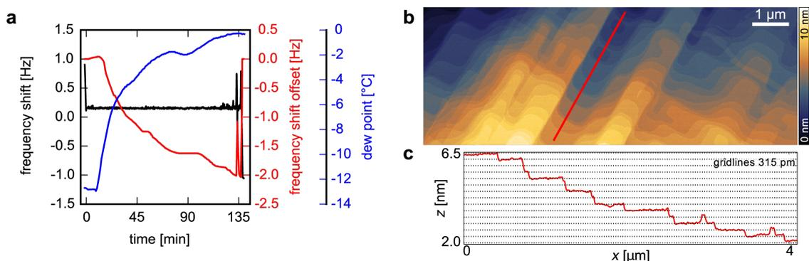
**Figure 3:** Application of the slow feedback control. a) Evolution of frequency shift  $\Delta f$  (black), frequency shift offset  $\Delta f_{\text{offset}}$  (red), and dew point  $\vartheta_{\text{dew}}$  (blue) over  $140$  min. b) Large scale topography of a KBr surface and c) corresponding height profile along the red line in b). The step height is  $315$  pm. Scan parameters:  $A = 1.1$  nm,  $\Delta f = +0.15$  Hz, scan speed  $10 \mu\text{m/s}$ .
