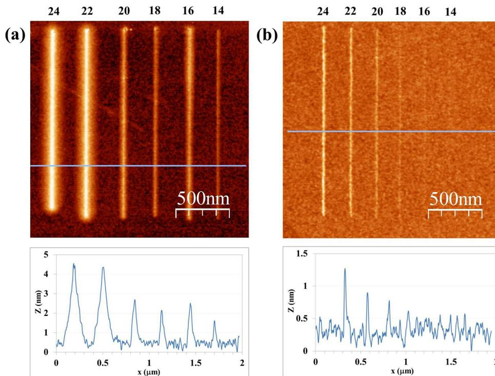
**Figure 3:** Results of LAO-AFM on Si with CNF (a) and Si (b) probes as a function of the bias voltage (in V). Writing speed is 1  $\mu\text{m/s}$ , RH is 36%.
