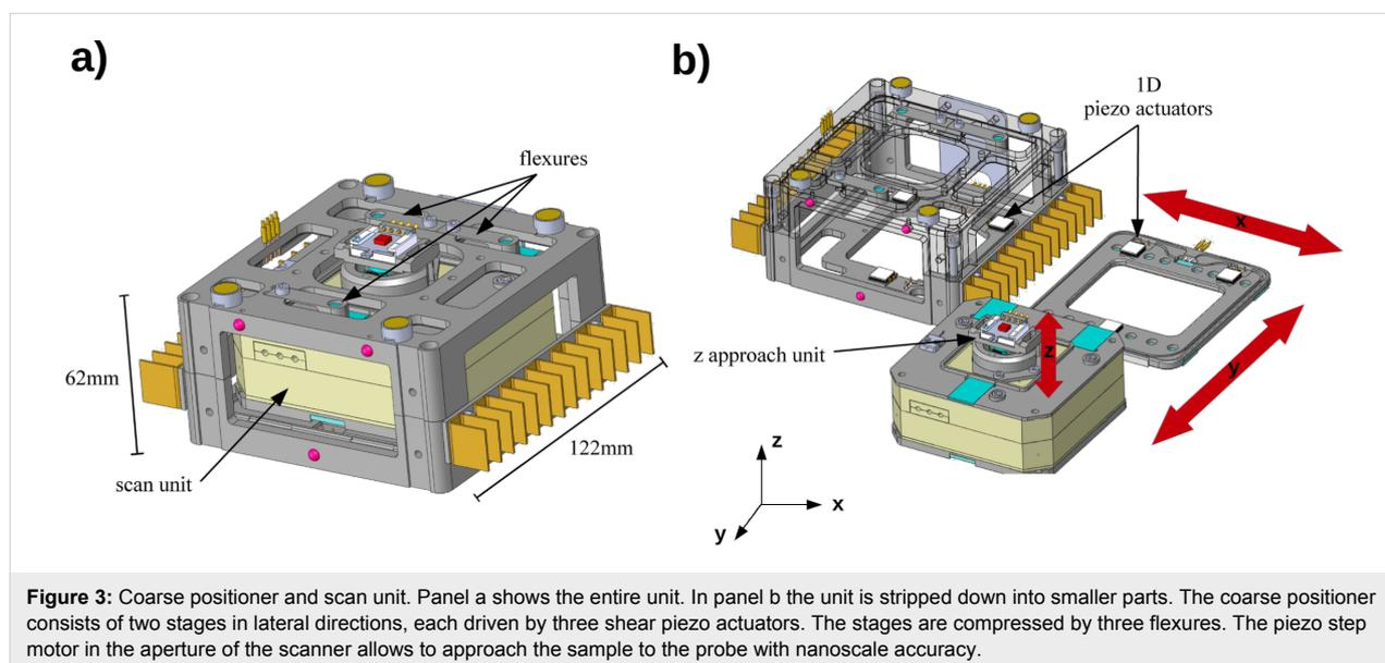
**Figure 3:** Coarse positioner and scan unit. Panel a shows the entire unit. In panel b the unit is stripped down into smaller parts. The coarse positioner consists of two stages in lateral directions, each driven by three shear piezo actuators. The stages are compressed by three flexures. The piezo step motor in the aperture of the scanner allows to approach the sample to the probe with nanoscale accuracy.
