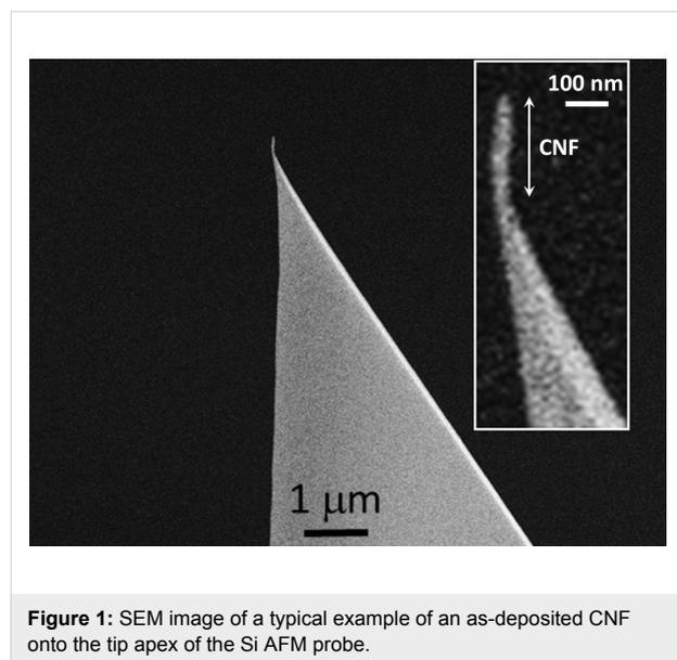
**Figure 1:** SEM image of a typical example of an as-deposited CNF onto the tip apex of the Si AFM probe.
