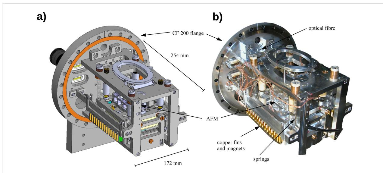
**Figure 4:** The atomic force microscope is assembled on a CF200 flange with four tension springs. Copper fins and magnets serve as an eddy current damping system to suppress vertical vibrations. In panel a, a CAD image is illustrated, whereas panel b shows a photograph of the microscope.
