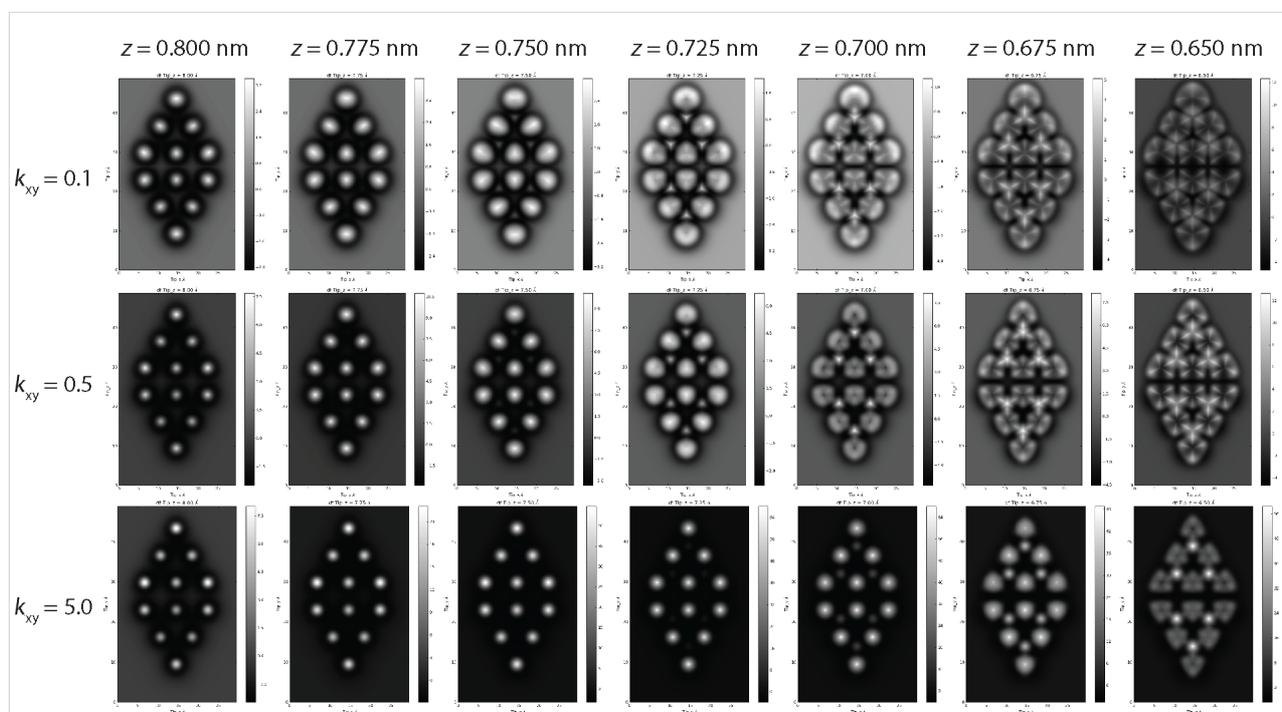
**Figure 4:** Simulated constant height images at decreasing tip-sample separation for three different probe lateral stiffness ( $k_{xy}$ ). The triangular appearance of the adatoms, and the subsequent contrast inversion, occurs at larger tip separations for lower stiffness probes. For the lowest stiffness probe the ‘hole’ produced by the contrast inversion is almost reduced to a point due to the extreme sharpening of the features caused by the deflection of the probe.
