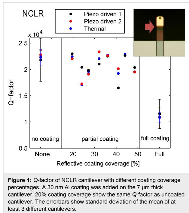
**Figure 1:**  $Q$ -factor of NCLR cantilever with different coating coverage percentages. A 30 nm Al coating was added on the 7  $\mu\text{m}$  thick cantilever. 20% coating coverage show the same  $Q$ -factor as uncoated cantilever. The errorbars show standard deviation of the mean of at least 3 different cantilevers.
