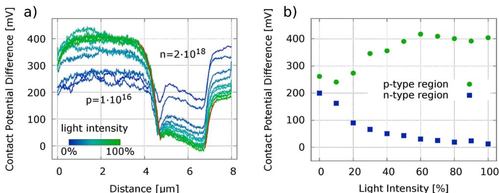
**Figure 7:** Panel a shows sections across the SiC p/n-junction (Figure 6) extracted from images taken at various light intensities. The data were averaged over five lines taken along the middle of the scan area. The averaged CPD values in the p- and n-type areas approach constant values under illumination as shown in panel b. In red are shown fits of the SCR regions of both junctions from the 100% illuminated sample calculated through Equation 2.
