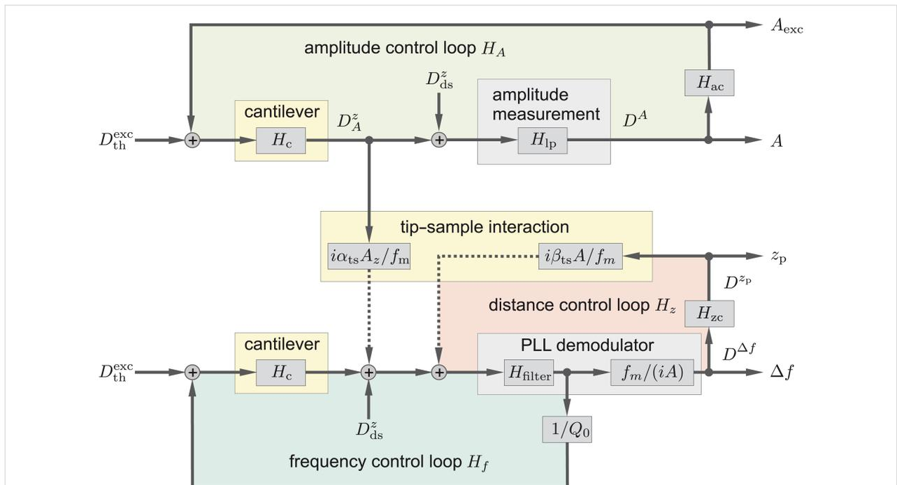
**Figure 2:** Model for signal and noise propagation in an NC-AFM, highlighting the tip-sample interaction, PLL demodulator and control loops. Signal paths indicated by dotted lines are only relevant for the case of significant tip-sample interaction.
