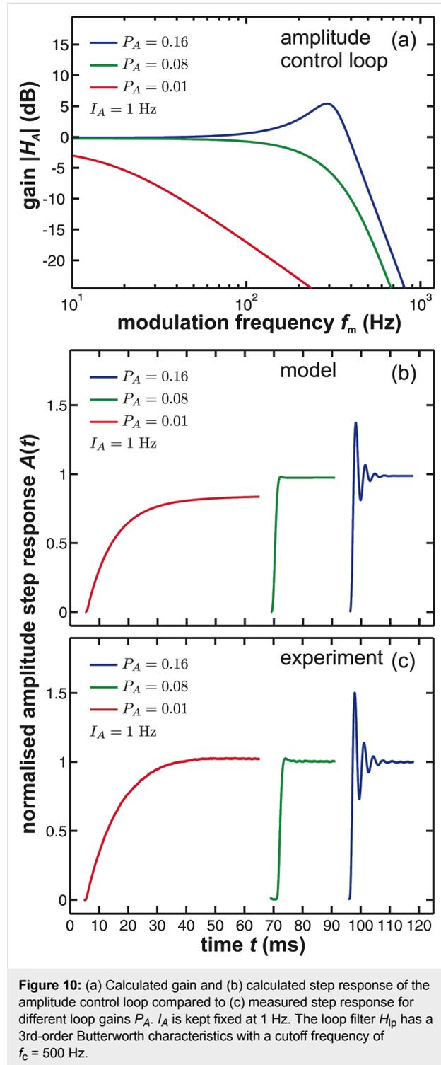
**Figure 10:** (a) Calculated gain and (b) calculated step response of the amplitude control loop compared to (c) measured step response for different loop gains  $P_A$ .  $I_A$  is kept fixed at 1 Hz. The loop filter  $H_{lp}$  has a 3rd-order Butterworth characteristics with a cutoff frequency of  $f_c = 500$  Hz.
