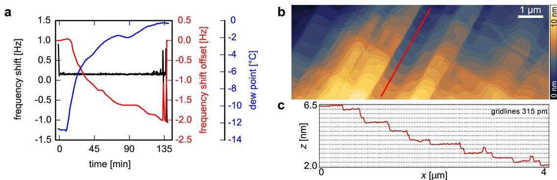
**Figure 3:** Application of the slow feedback control. a) Evolution of frequency shift  $\Delta f$  (black), frequency shift offset  $\Delta f_{\text{offset}}$  (red), and dew point  $\vartheta_{\text{dew}}$  (blue) over  $140$  min. b) Large scale topography of a KBr surface and c) corresponding height profile along the red line in b). The step height is  $315$  pm. Scan parameters:  $A = 1.1$  nm,  $\Delta f = +0.15$  Hz, scan speed  $10 \mu\text{m/s}$ .
