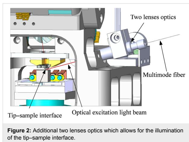
**Figure 2:** Additional two lenses optics which allows for the illumination of the tip-sample interface.
