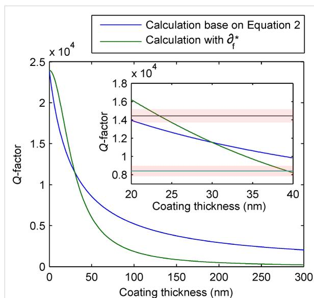
**Figure 5:** Calculation of the change of  $Q$ -factor for a fully coated NCLR cantilever with different coating thicknesses. Blue shows the predicted value according to Equation 2. Green shows the predicted  $Q$ -factor value with the added  $\delta_f^*$  term. The inset shows a zoom to 20–40 nm. The mean measured  $Q$ -factor for two sets of NCLR with a coating thickness difference of 16 nm are plotted as a horizontal line with standard error by red bands.
