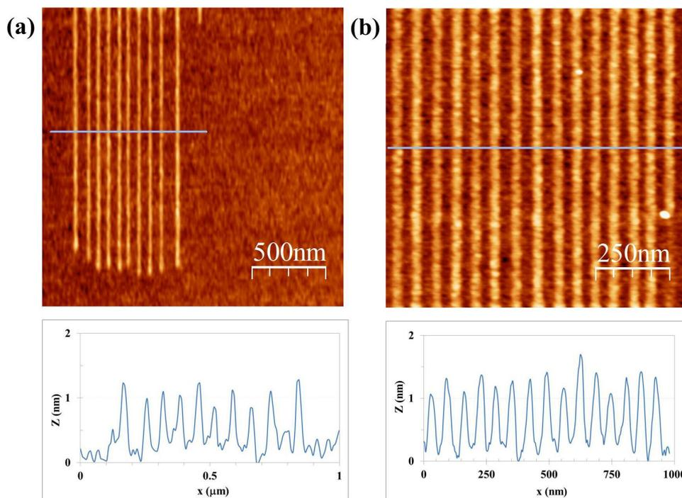
**Figure 5:** Reproducibility for patterning line arrays by using CNF probes. Array of lines written at a) 23.4 V and b) 43.2 V, having line height of ca. 0.8 nm and ca. 1.2 nm, respectively. The common writing speed is 4 μm/s, RH is 30%.
