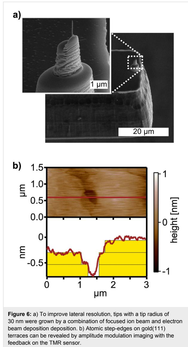
**Figure 6:** a) To improve lateral resolution, tips with a tip radius of 30 nm were grown by a combination of focused ion beam and electron beam deposition. b) Atomic step-edges on gold(111) terraces can be revealed by amplitude modulation imaging with the feedback on the TMR sensor.
