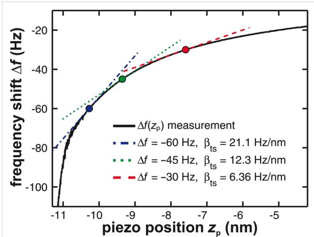
**Figure 4:** Determination of the tip–sample interaction parameter  $\beta_{ts}$  from the slope of a measured  $\Delta f(z_p)$  curve. Frequency shift data are plotted as a function of the  $z$ -piezo position  $z_p$ .
