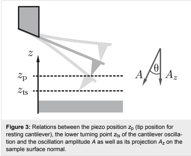
**Figure 3:** Relations between the piezo position  $z_p$  (tip position for resting cantilever), the lower turning point  $z_{ts}$  of the cantilever oscillation and the oscillation amplitude  $A$  as well as its projection  $A_z$  on the sample surface normal.
