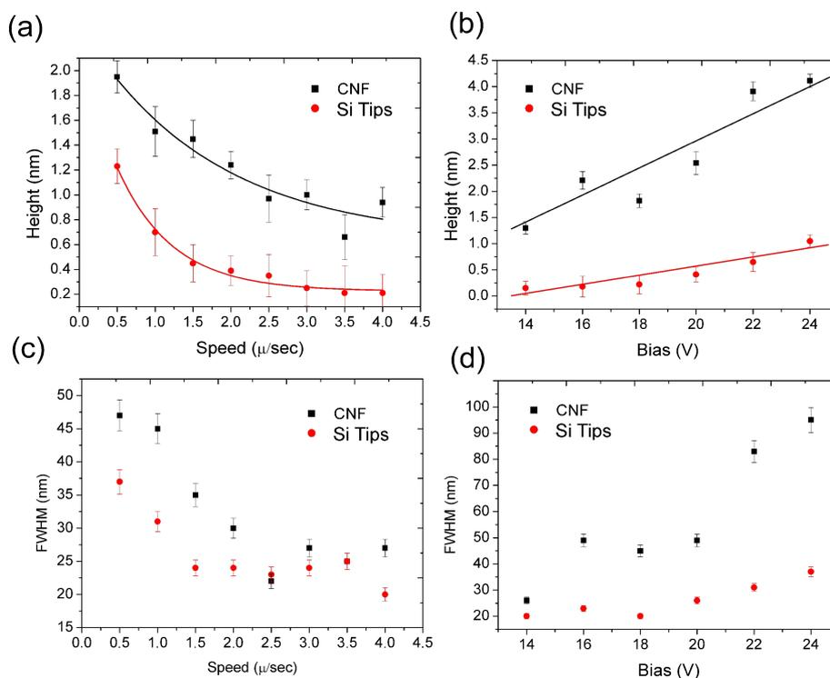
**Figure 6:** Kinetics of LAO-AFM on Si by using CNF versus Si probes. a) Line height upon writing speed for a bias voltage of 20 V. b) Line height upon bias voltage for a writing speed of 1 μm/s. Full width at half maximum (FWHM) of the same features upon writing speed (c) and upon bias voltage (d).
