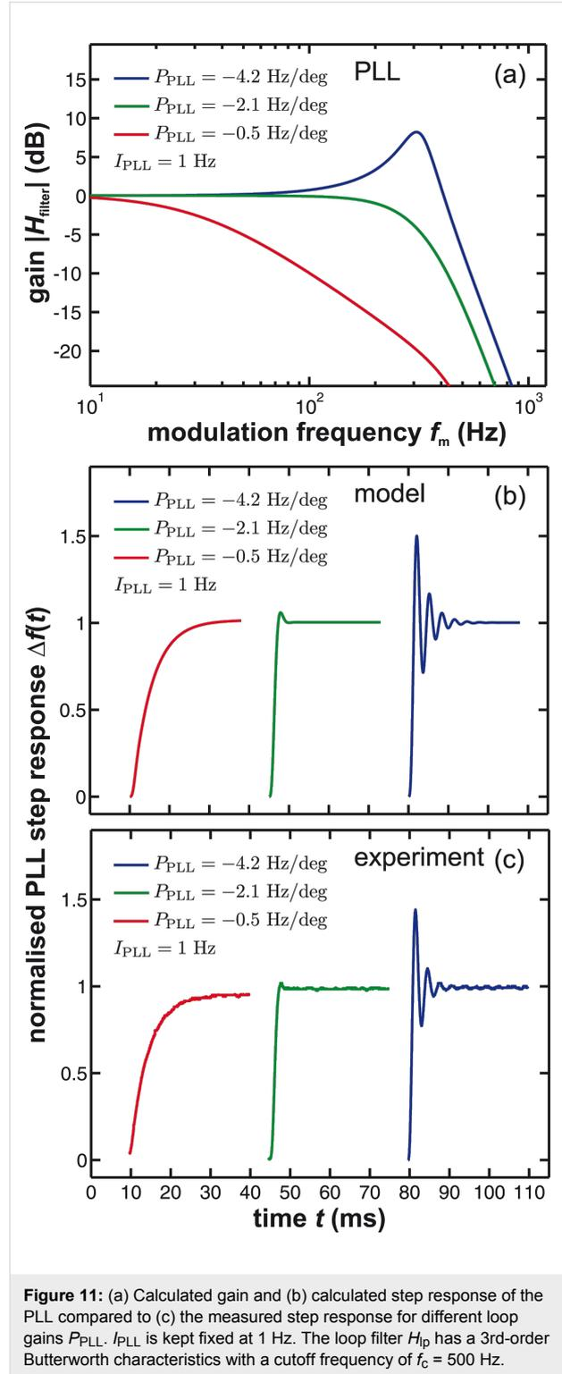
**Figure 11:** (a) Calculated gain and (b) calculated step response of the PLL compared to (c) the measured step response for different loop gain settings  $P_{\text{PLL}}$ .  $I_{\text{PLL}}$  is kept fixed at 1 Hz. The loop filter  $H_{\text{lp}}$  has a 3rd-order Butterworth characteristics with a cutoff frequency of  $f_c = 500$  Hz.
