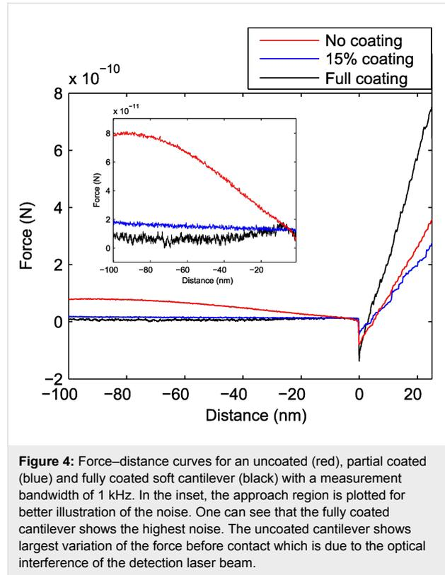
**Figure 4:** Force–distance curves for an uncoated (red), partial coated (blue) and fully coated soft cantilever (black) with a measurement bandwidth of 1 kHz. In the inset, the approach region is plotted for better illustration of the noise. One can see that the fully coated cantilever shows the highest noise. The uncoated cantilever shows largest variation of the force before contact which is due to the optical interference of the detection laser beam.
