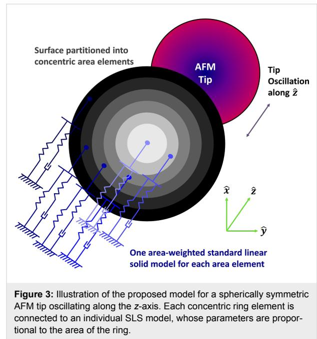
**Figure 3:** Illustration of the proposed model for a spherically symmetric AFM tip oscillating along the  $z$ -axis. Each concentric ring element is connected to an individual SLS model, whose parameters are proportional to the area of the ring.
