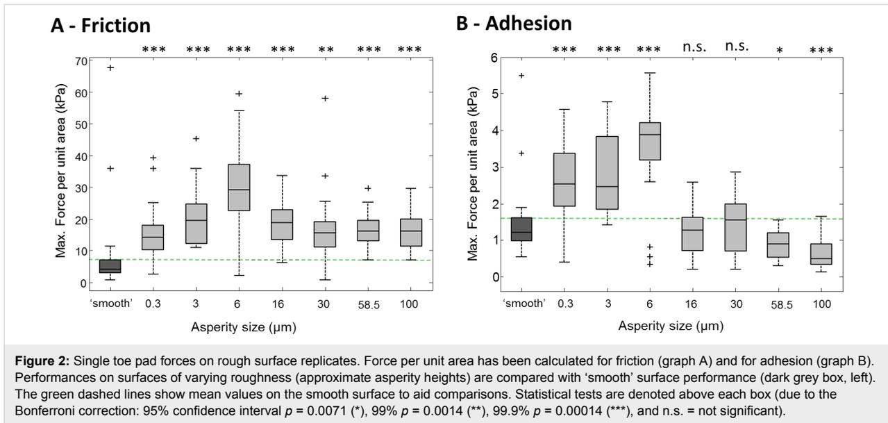
surfaces were  $18.48 \pm 6.1$  kPa, higher than the smooth values ( $z = -5.5663$ ,  $p < 0.00014$ ), but lower than the forces on the 6 µm surface. The shear stress measured on the largest roughnesses tested were at a consistent level of ca. 16 kPa, still higher than those measured on the smooth surface (e.g., comparing smooth to 100 µm,  $z = -5.5072$ ,  $p < 0.00014$ ).
