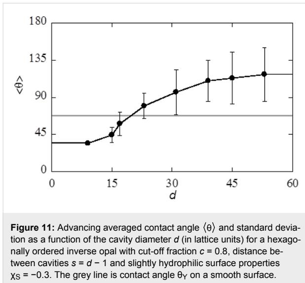
**Figure 11:** Advancing averaged contact angle  $\langle \theta \rangle$  and standard deviation as a function of the cavity diameter  $d$  (in lattice units) for a hexagonally ordered inverse opal with cut-off fraction  $c = 0.8$ , distance between cavities  $s = d - 1$  and slightly hydrophilic surface properties  $\chi_S = -0.3$ . The grey line is contact angle  $\theta_Y$  on a smooth surface.
