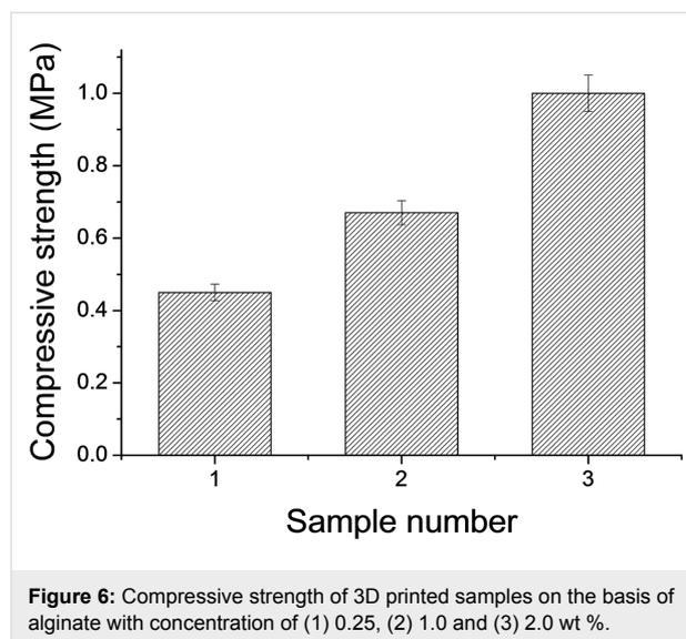
**Figure 6:** Compressive strength of 3D printed samples on the basis of alginate with concentration of (1) 0.25, (2) 1.0 and (3) 2.0 wt %.
