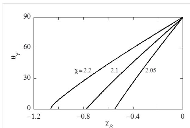
**Figure 4:** Contact angle of liquid on flat solid,  $\theta_Y$  as function of the interaction parameter of the liquid with the solid,  $\chi_S$ , for three different values of the interaction parameter of the liquid with the vapour,  $\chi$ .
