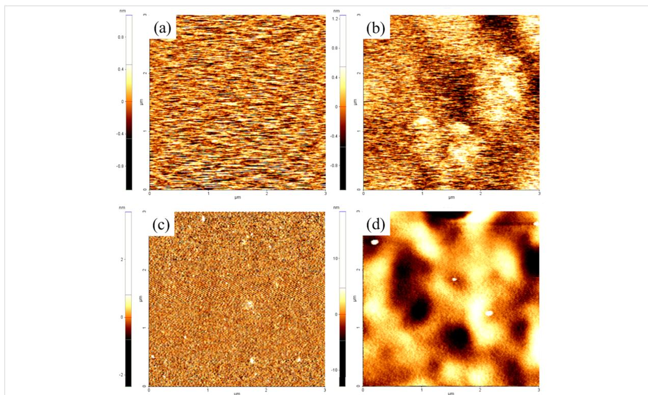
**Figure 1:** Typical AFM images of Si substrates before (a) and after (b) ODS-monolayer formation, (c) FAS17-monolayer formation, and (d) C<sub>10</sub>-hybrid film formation (scan areas are 3 × 3 μm<sup>2</sup>).
