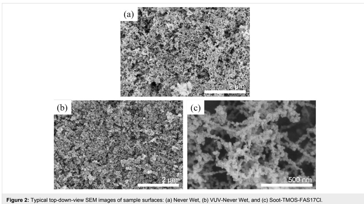
**Figure 2:** Typical top-down-view SEM images of sample surfaces: (a) Never Wet, (b) VUV-Never Wet, and (c) Soot-TMOS-FAS17Cl.
