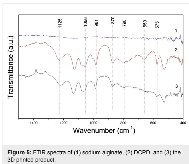
**Figure 5:** FTIR spectra of (1) sodium alginate, (2) DCPD, and (3) the 3D printed product.
