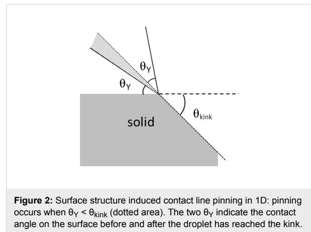
**Figure 2:** Surface structure induced contact line pinning in 1D: pinning occurs when  $\theta_Y < \theta_{kink}$  (dotted area). The two  $\theta_Y$  indicate the contact angle on the surface before and after the droplet has reached the kink.
