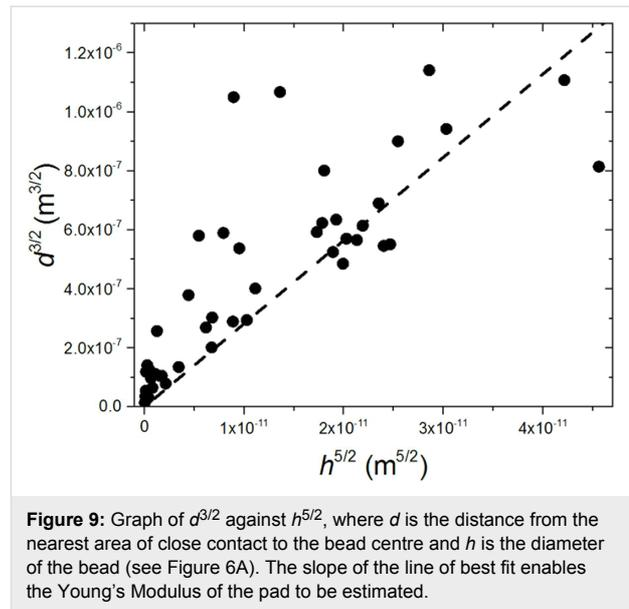
**Figure 9:** Graph of  $d^{3/2}$  against  $h^{5/2}$ , where  $d$  is the distance from the nearest area of close contact to the bead centre and  $h$  is the diameter of the bead (see Figure 6A). The slope of the line of best fit enables the Young's Modulus of the pad to be estimated.
