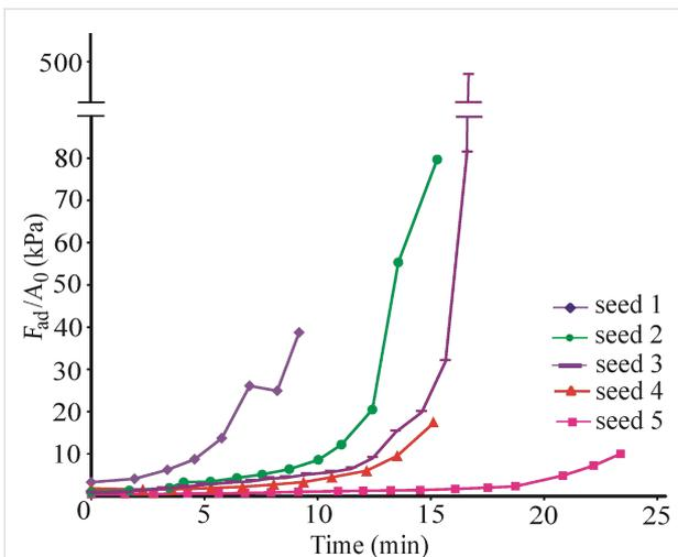
**Figure 4:** The ratio of pull-off force ( $F_{ad}$ ) to contact area ( $A_0$ ) (adhesion stress) for five individual seeds as a function of time. The smallest adhesion stress was observed for the seed demonstrated the highest contact area and pull-off force.
