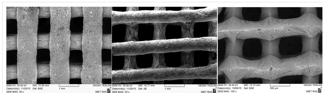
**Figure 1:** SEM micrographs of 3D printed samples.
