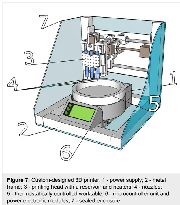
**Figure 7:** Custom-designed 3D printer. 1 - power supply; 2 - metal frame; 3 - printing head with a reservoir and heaters; 4 - nozzles; 5 - thermostatically controlled worktable; 6 - microcontroller unit and power electronic modules; 7 - sealed enclosure.
