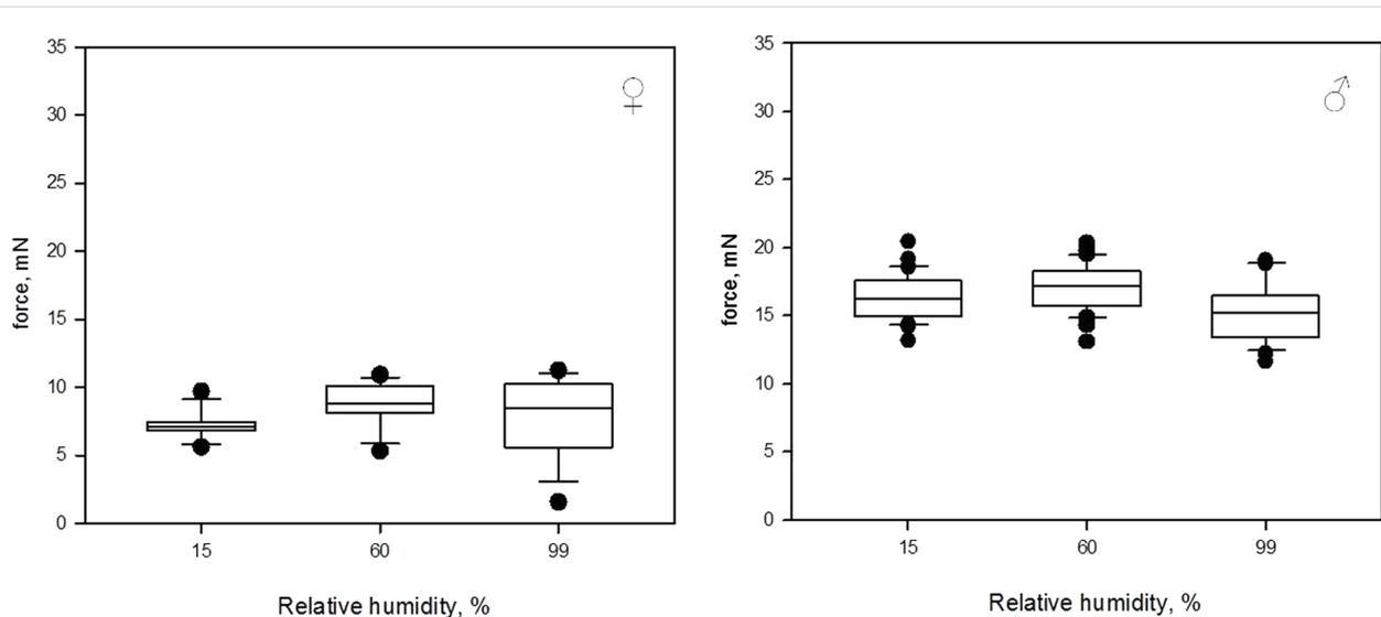
**Figure 4:** Box-and-whiskers diagrams based on the results of the second experiment with all three levels of RH tested at the same day. The ends of the boxes define the 25th and 75th percentiles, with a line at the median and error bars defining the 10th and 90th percentiles, black dots represent the outliers.
