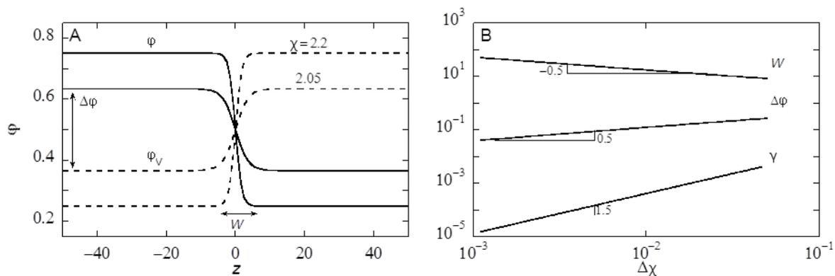
**Figure 3:** A) Examples of volume fraction profiles across a liquid/vapour interface found numerically by exact minimisation of Equation 6, with the interaction parameter  $\chi = 2.05$  and  $\chi = 2.2$  as indicated. B) Width of the interface ( $W$ ), density difference between the two phases ( $\Delta\varphi$ ) and dimensionless surface tension ( $\gamma$ ) as function of  $\Delta\chi = \chi - 2$  in double logarithmic coordinates.
