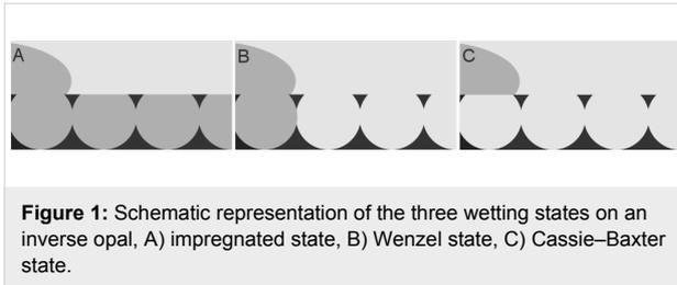
**Figure 1:** Schematic representation of the three wetting states on an inverse opal, A) impregnated state, B) Wenzel state, C) Cassie–Baxter state.
