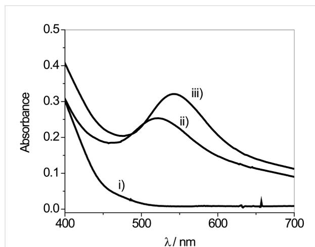
**Figure 2:** UV–vis spectra in glycerol: i) the HClAu<sub>4</sub> precursor; ii) the AuNPs synthesized with 8 min of irradiation time; iii) the AuNPs synthesized with 13 min of irradiation time ( $\lambda_{\text{irradiation}} = 300 \text{ nm}$ ).
