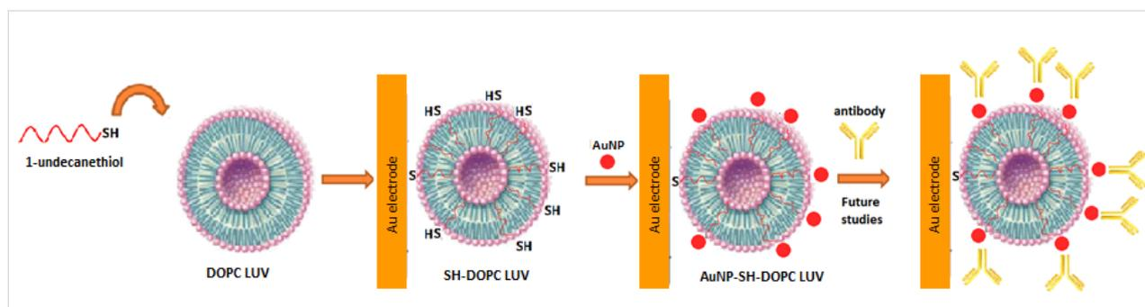
**Figure 1:** Platform to design a possible immunosensor.
