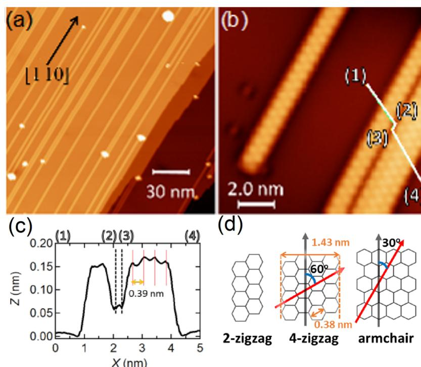
**Figure 1:** STM images of SiNRs on Ag(110) with (a)  $V_S = -500$  mV,  $I_t = 10$  pA and (b)  $V_S = -100$  mV,  $I_t = 30$  pA. (c) Cross-sectional height profile along the (1)–(4) line shown in (b). (d) Schematic structural models of SiNR structures. The black arrows dictate the longitudinal direction and the red arrows represent the row of the honeycomb units across the ribbons.
