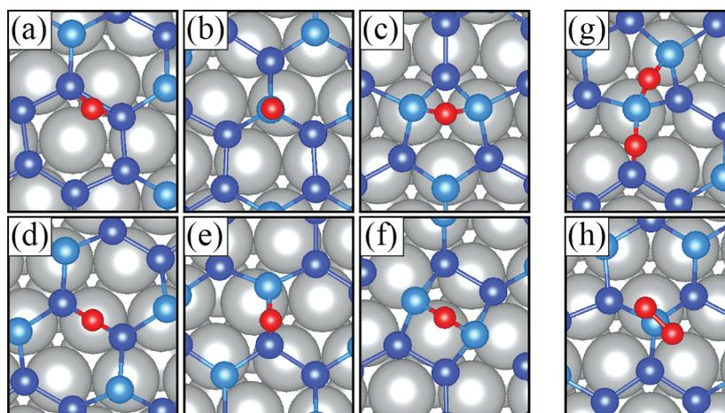
**Figure 4:** Final configurations of silicene-coated Ag(111) after capturing an oxygen atom at the sites (a)  $H_1$ , (b)  $T_1$ , (c)  $H_2$ , (d)  $T_2$ , (e)  $T_3$  and (f)  $H_3$ . Final configurations (g) in-S and (h) top-S of silicene-coated Ag(111) after capturing an O<sub>2</sub> molecule.
