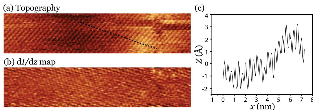
**Figure 3:** (a) STM image of a MoS<sub>2</sub> surface after the deposition of 0.2 monolayers of Si. (b) Spatial map of  $dI/dz$ . In both images the atomic structure is resolved. (c) Line-scan taken along the dotted line depicted in panel (a). Sample bias is 1.2 V and tunnel current is 0.5 nA.
