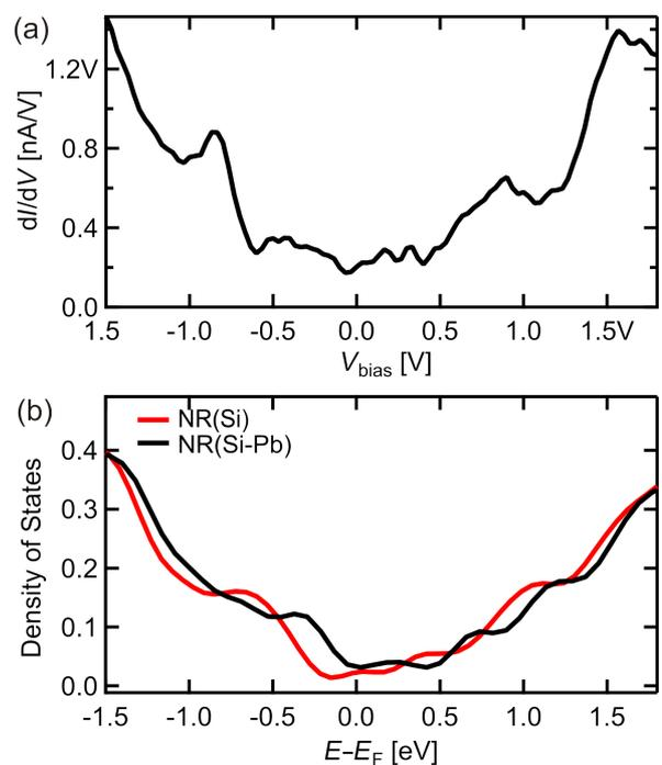
**Figure 5:** (a)  $dI/dV$  point spectroscopy data acquired on top of the Si NR. (b) Total density of states of Si NR system in the absence (red line) and in the presence of Pb atoms (black line). Note that the system is metallic.
