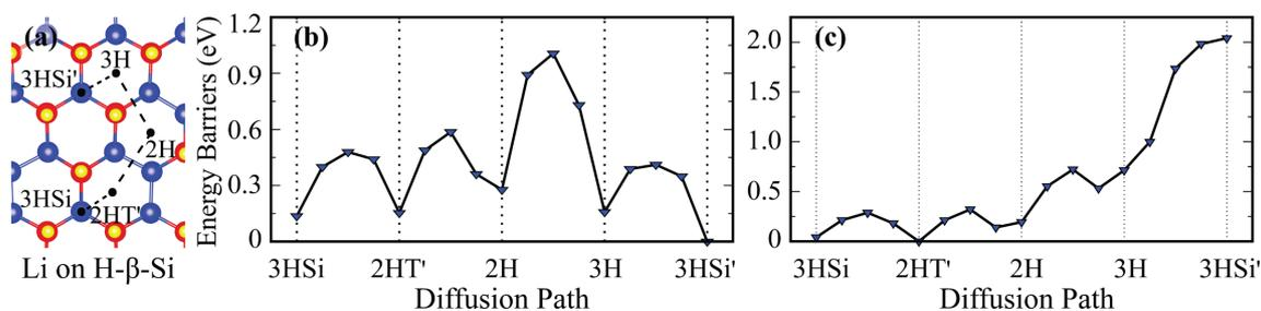
**Figure 3:** (a) Top view of possible adsorption sites for Li atom on H- $\beta$ -Si. Energy barrier graphs of (b) the first and (c) the second Li atom on H- $\beta$ -Si. A possible diffusion path of Li atom is illustrated by dashed black lines.
