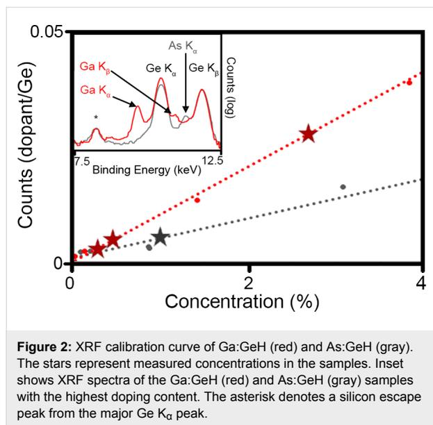
**Figure 2:** XRF calibration curve of Ga:GeH (red) and As:GeH (gray). The stars represent measured concentrations in the samples. Inset shows XRF spectra of the Ga:GeH (red) and As:GeH (gray) samples with the highest doping content. The asterisk denotes a silicon escape peak from the major Ge K $\alpha$  peak.
