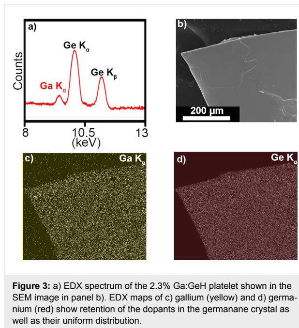
**Figure 3:** a) EDX spectrum of the 2.3% Ga:GeH platelet shown in the SEM image in panel b). EDX maps of c) gallium (yellow) and d) germanium (red) show retention of the dopants in the germanane crystal as well as their uniform distribution.
