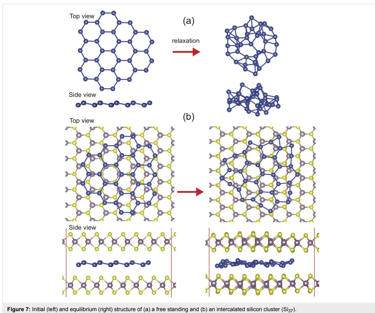
is known that layered materials such as MoS<sub>2</sub> have a tendency to host intercalants. In this work we provide additional evidence for silicon intercalation by using STS and XPS. Since silicon intercalates it is interesting to scrutinize if there are possibilities to grow a 2D layer in between two layers of MoS<sub>2</sub>. Our density functional theory calculations show that 2D silicon clusters intercalated between MoS<sub>2</sub> layers are stable.
