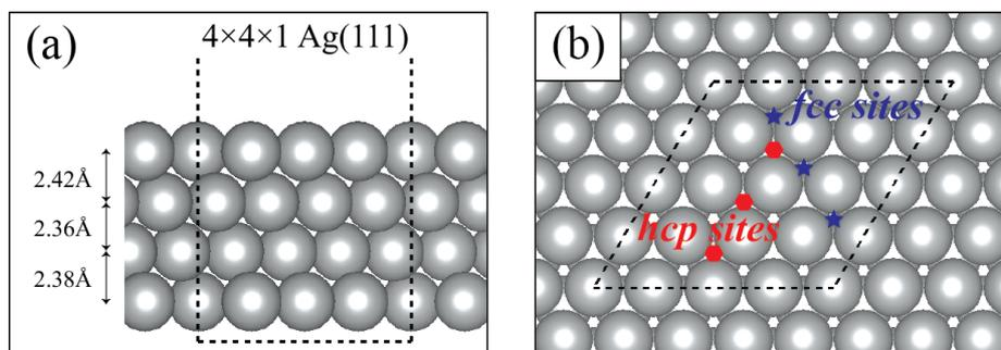
**Figure 1:** (a) Side view of the Ag(111) supercell structure and (b) top view of the Ag(111) supercell structure with possible oxygen captured sites. Definitions and oxygen binding energies of all sites are given in Table 1.
