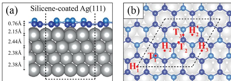
**Figure 3:** (a) Side view of the silicene-coated Ag(111) supercell structure and (b) top view of the silicene-coated Ag(111) supercell structure with possible oxygen-capture sites. Definitions and oxygen binding energies of all sites are given in Table 1.
