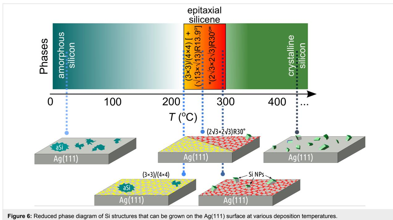
**Figure 6:** Reduced phase diagram of Si structures that can be grown on the Ag(111) surface at various deposition temperatures.
