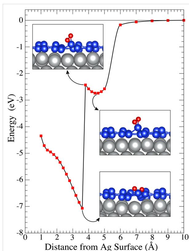
**Figure 6:** Indentation calculations for an O<sub>2</sub> molecule. Inset graphs show structures according to local-minimum states of O<sub>2</sub>, before and after reaching the global minimum state of the system.
