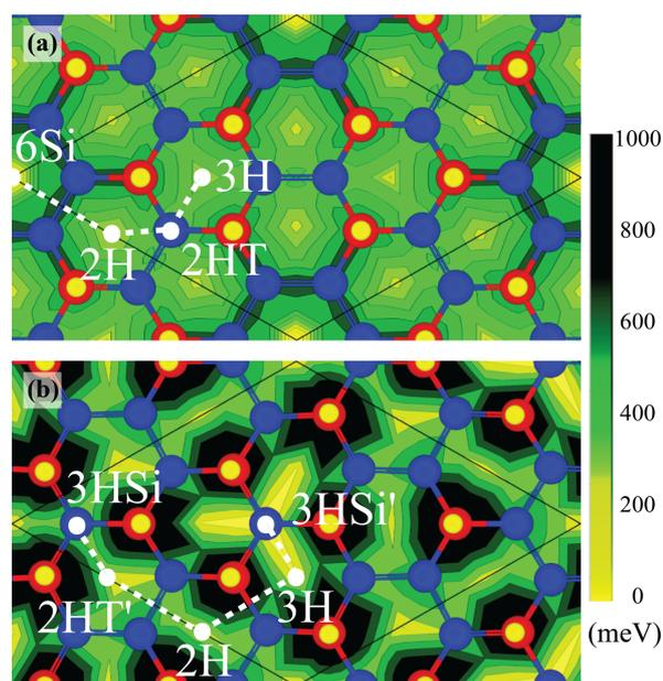
**Figure 4:** (Color online) Contour plots of the energy barriers (in meV) seen by Li atom adsorbed on (a) H- $\alpha$ -Si and (b) H- $\beta$ -Si. Possible diffusion paths of Li on hydrogenated  $\alpha$  and  $\beta$  silicene surfaces are illustrated by white dashed lines.
