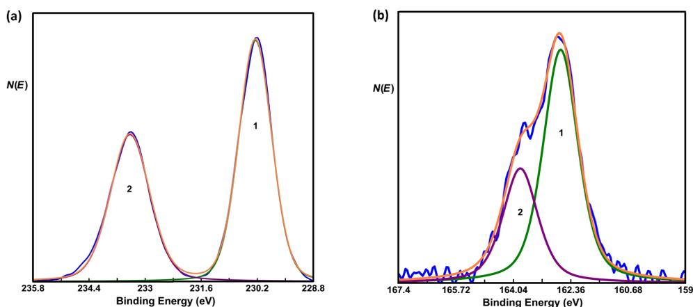
**Figure 4:** Core-level spectra of (a) Mo and (b) S before depositing Si. The spectra are fitted with two GL function peaks. In (a), 1 and 2 represent the Mo  $3d_{5/2}$  and  $3d_{3/2}$  peaks, respectively. In (b), 1 and 2 represent the S  $2p_{3/2}$  and  $2p_{1/2}$  peaks, respectively. In both figures, the resultant fitted spectra are represented by an orange line.
