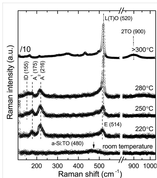
**Figure 2:** Raman spectra of the various structures obtained upon Si deposition at room temperature RT, 220, 250, 280, and 300 °C. In the spectral range between 550 and 830  $\text{cm}^{-1}$ , no features were observed. The spectra are stacked for clarity. The topmost Raman spectrum was divided by 10 to fit the rest of spectra in the plot.
