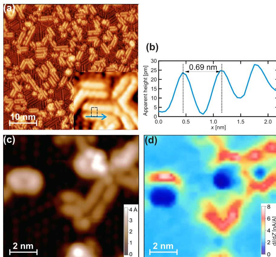
**Figure 1:** (a) STM topography ( $U = 2.0$  V,  $I = 0.5$  nA) of Si nanoribbons on a  $\text{Si}(111)\sqrt{3} \times \sqrt{3}$ -Pb surface. (b) Line profile along blue arrow marked in the inset of (a). The arrow points in the  $[1\ 10]$  direction. The unit cell of a nanoribbon is also marked in the inset of (a). (c, d) Results of a simultaneously measured topography and  $dI/dz$  map of the same area. Scanning parameters were  $U = 1$  V,  $I = 0.5$  nA.
