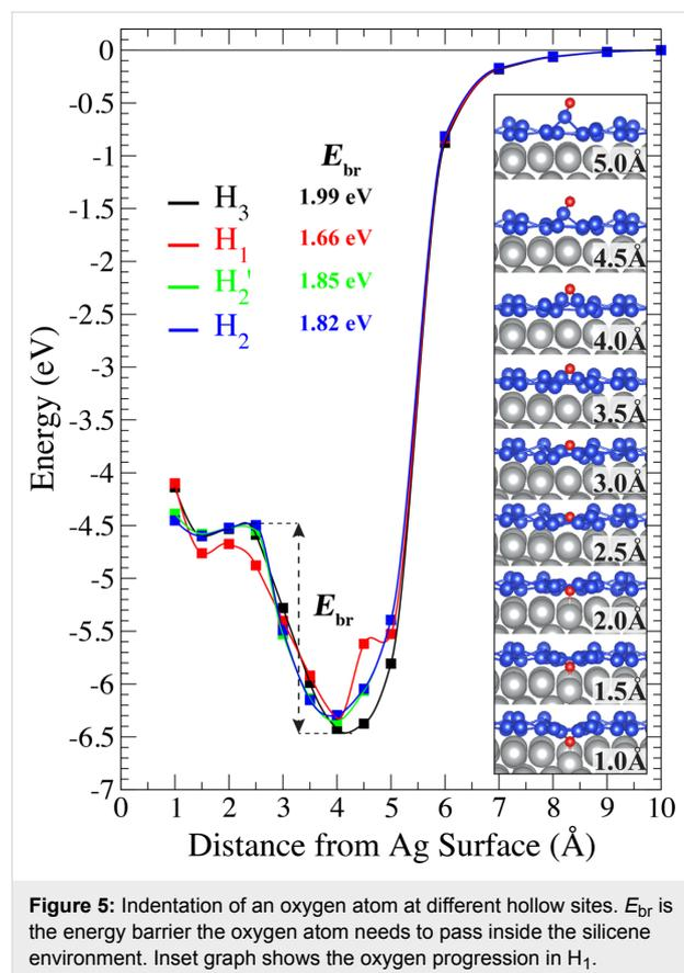
**Figure 5:** Indentation of an oxygen atom at different hollow sites.  $E_{br}$  is the energy barrier the oxygen atom needs to pass inside the silicene environment. Inset graph shows the oxygen progression in  $H_1$ .
