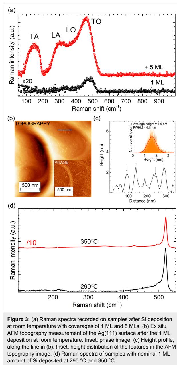
**Figure 3:** (a) Raman spectra recorded on samples after Si deposition at room temperature with coverages of 1 ML and 5 MLs. (b) Ex situ AFM topography measurement of the Ag(111) surface after the 1 ML deposition at room temperature. Inset: phase image. (c) Height profile, along the line in (b). Inset: height distribution of the features in the AFM topography image. (d) Raman spectra of samples with nominal 1 ML amount of Si deposited at 290  $^\circ\text{C}$  and 350  $^\circ\text{C}$ .
