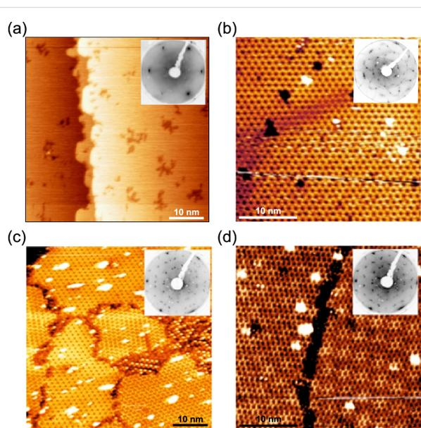
**Figure 1:** (a) STM topographic images ( $U_{\text{bias}} = -1.0$  V,  $I = 1.08$  nA) and corresponding low-energy electron diffraction (LEED) patterns (insets) of (a) 0.1 ML of Si deposited onto Ag(111) at room temperature, (b) 1 ML of Si deposited at 220 °C resulting in  $(3 \times 3)$  silicene formation, (c) 1 ML of Si deposited at 240 °C showing the formation of several phases, and (d) 1 ML of Si deposited at 280 °C with a clear “ $(2\sqrt{3} \times 2\sqrt{3})R30^\circ$ ” reconstruction.
