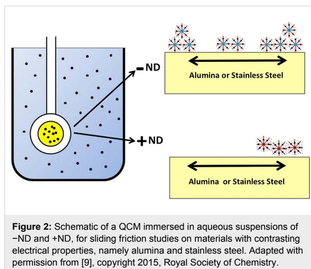
The QCM measurement experiments were complemented by AFM and SEM measurements of the surface topography before and after the ND exposure, as well as macroscale measurements of  $\mu_k$ . The materials were inspired by Liu et al.'s sugges-
