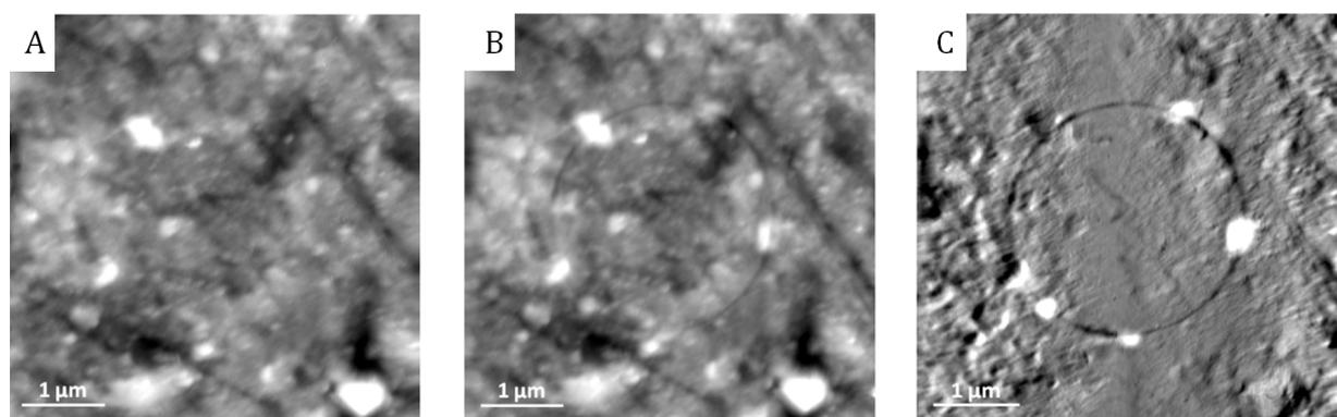
**Figure 4:** A and B (grey scale is 35 nm) are the AFM contact mode topographic images before and after the wear experiment; C (grey scale is 12 nm) is the height difference (B) – (A) obtained on a copper-based composite (image size:  $5 \times 5 \mu\text{m}$ ).
