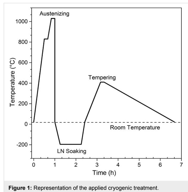
Figure 1: Representation of the applied cryogenic treatment.
