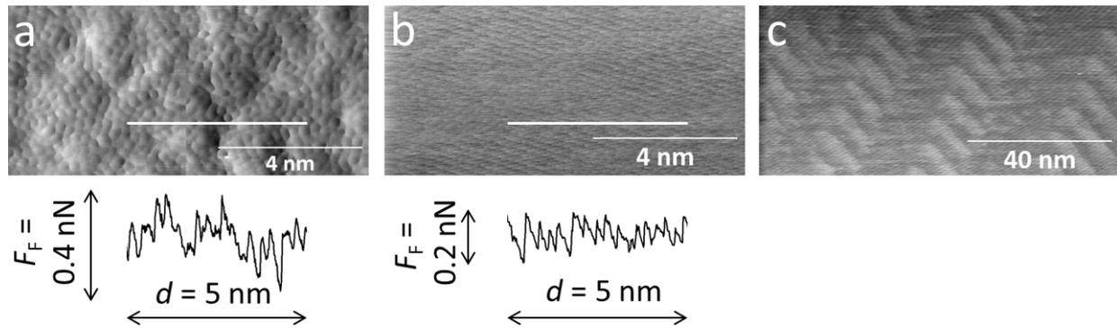
**Figure 1:** Friction force maps for a) an oxidized Si(100) surface scanned with an intact Ar-sputter cleaned SiO<sub>x</sub>/Si tip, b) Au(111), and c) the topography of the Au(111) herringbone reconstruction scanned with an intact SiO<sub>x</sub>/Si tip. One line was extracted from a) and b) to visualize the stick-slip pattern on Si(100) and on Au(111).
