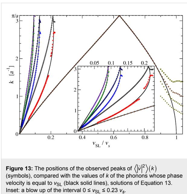
wave vectors of the excited phonons for a given  $v_{SL}$ . Above the speed of sound  $v_s$ , Equation 13 has no solution and indeed the spectrum displays no sharp peak, see Figure 9a. Correspondingly the “nonresonant” friction is very small, see the right side of Figure 6.
