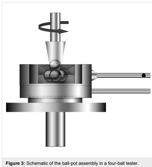
Figure 3: Schematic of the ball-pot assembly in a four-ball tester.
