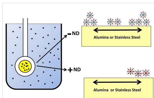
**Figure 2:** Schematic of a QCM immersed in aqueous suspensions of –ND and +ND, for sliding friction studies on materials with contrasting electrical properties, namely alumina and stainless steel. Adapted with permission from [9], copyright 2015, Royal Society of Chemistry.
