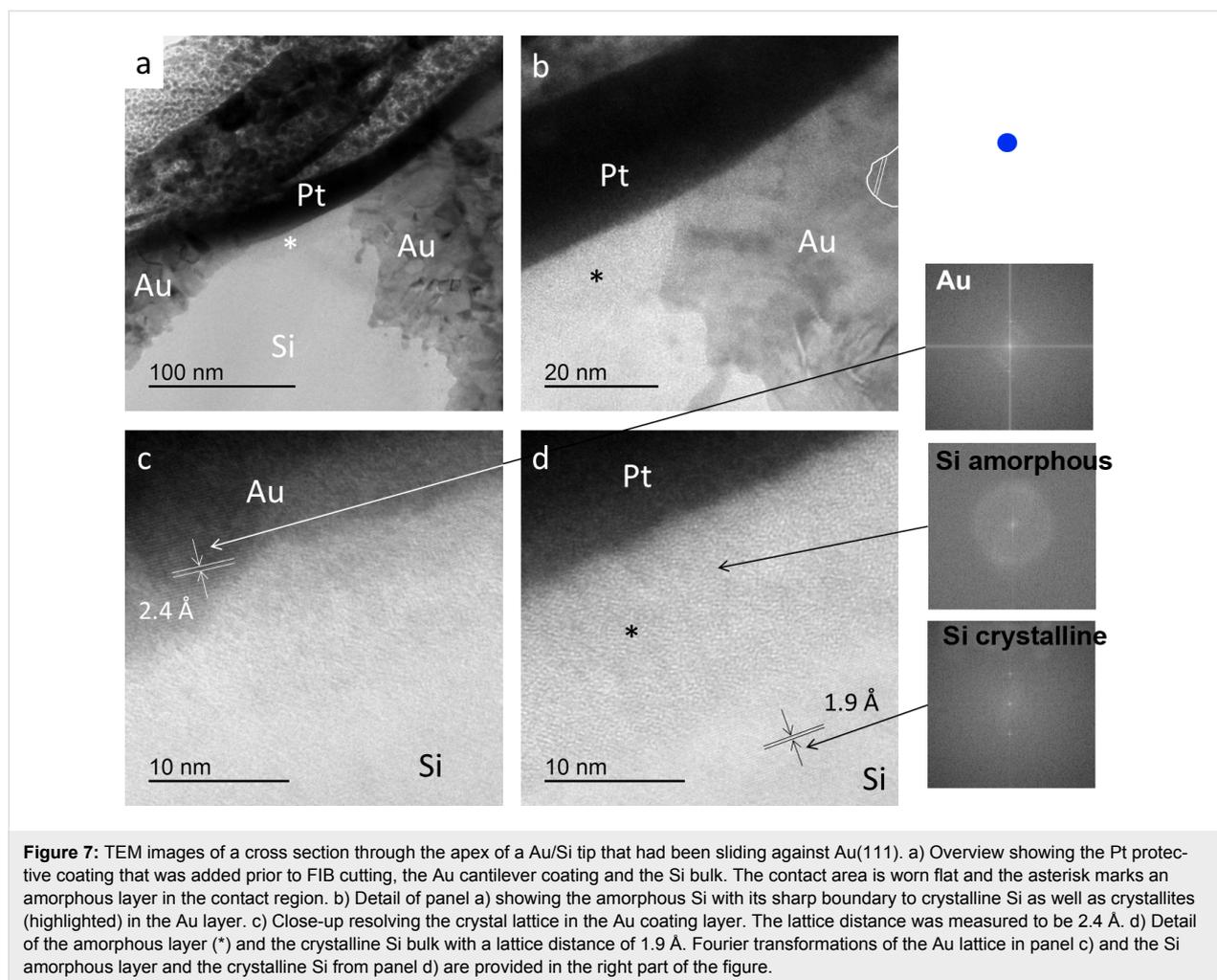
does not require oxidation to occur. Fourier transformation of the images (right side of Figure 7) revealed crystalline order for the tip material lattice and amorphous short-range structure for the layer that was transformed by the sliding contact.
