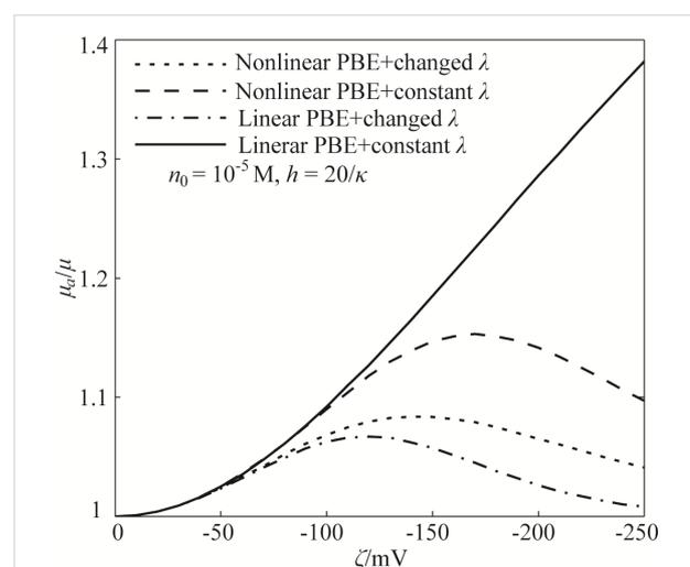
**Figure 3:** The effect of the zeta potential on the apparent viscosity of the lubricant based on different assumptions and theoretical models. The “Nonlinear PBE+changed  $\lambda$ ” case is the model established in the present work.
