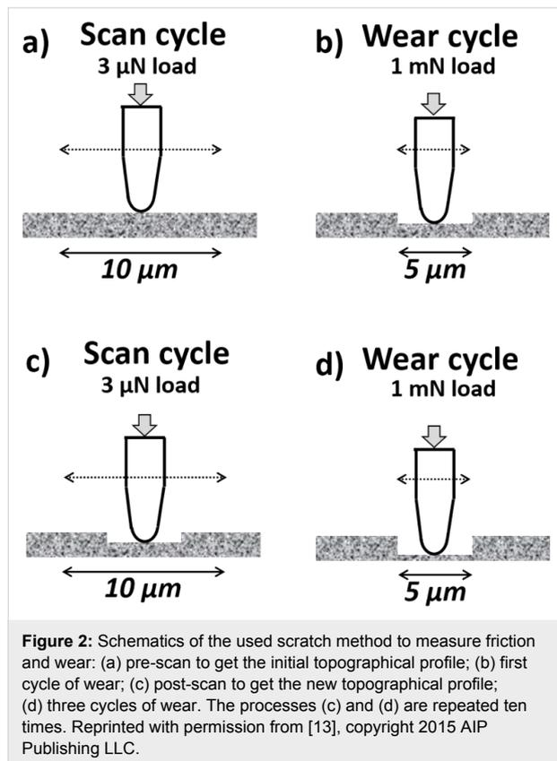
For the nanoscratch tests, a conical diamond tip with an apex radius of  $5 \mu\text{m}$  was employed. The applied normal load was set at  $1000 \mu\text{N}$  and each reported value corresponds to the average of at least three valid tests. The theoretical Hertzian contact pressure was estimated at  $10.7 \text{ GPa}$ .
