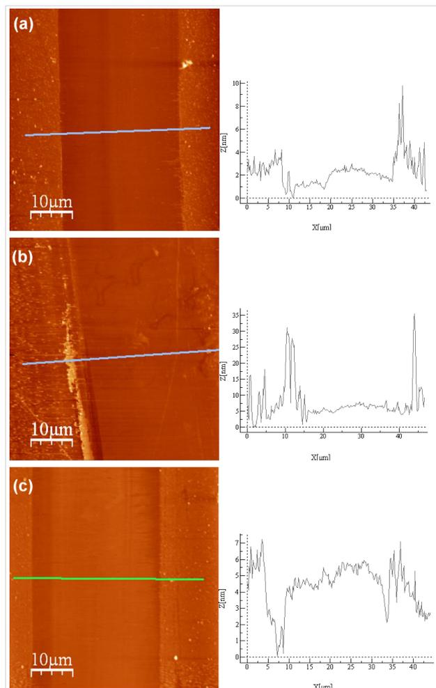
**Figure 6:** AFM images and height profiles of the sliding tracks in (a) dry PEG, (b) PEG + [EMIM][TfO] and (c) PEG + [EMIM][EtSO<sub>4</sub>].
