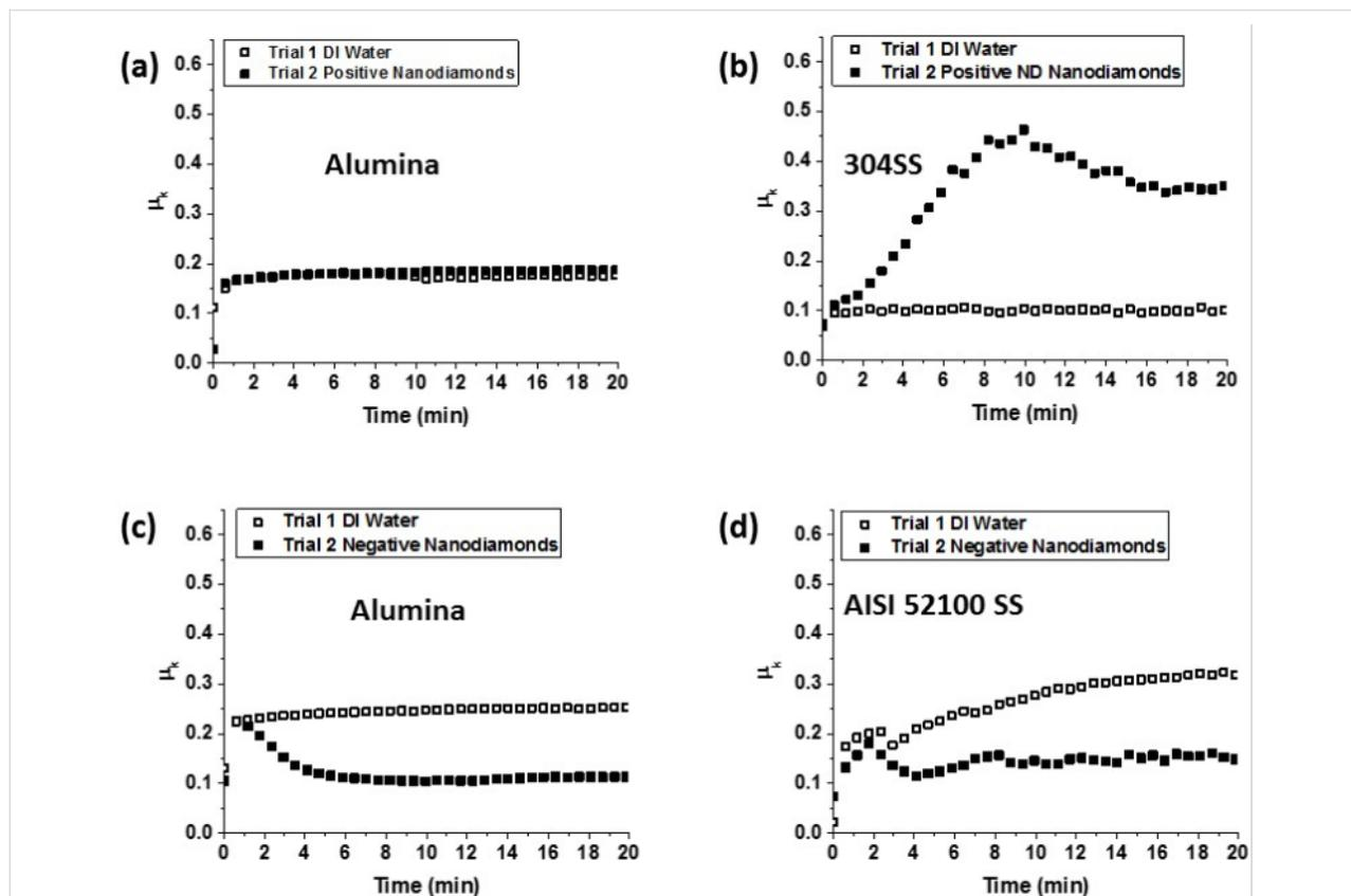
**Figure 3:** Representative friction coefficient versus time plots for alumina (left) and stainless steel (right) contacts lubricated with pure DI water (open squares), positively (a,b) and negatively (c,d) (filled squares) charged ND suspensions. Addition of –ND to water (c,d) consistently lowered the friction coefficient while addition of +ND to water consistently (a,b) failed to lower the friction coefficient.
