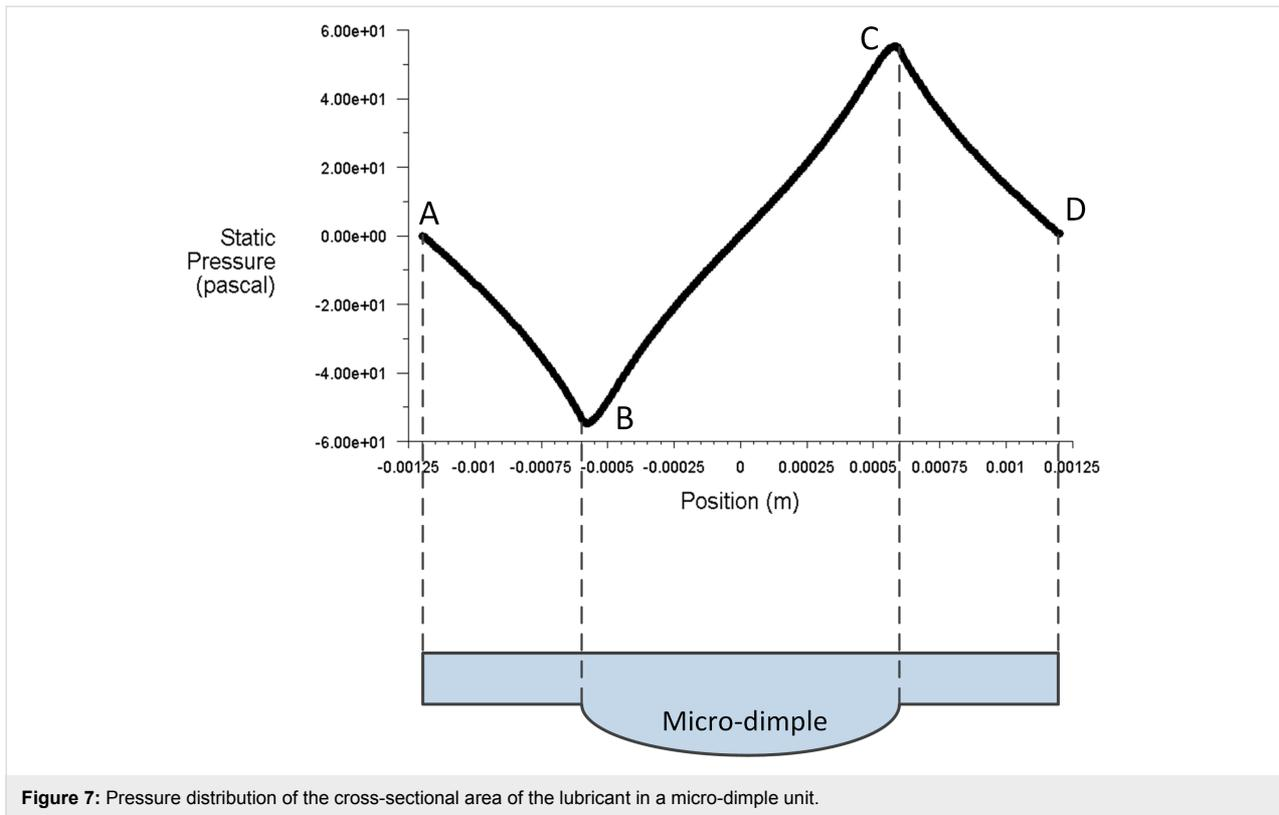
**Figure 7:** Pressure distribution of the cross-sectional area of the lubricant in a micro-dimple unit.
