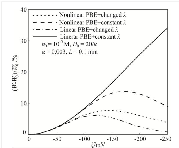
**Figure 5:** Comparison of the hydrodynamic load capacity of the lubricant including the effect of the zeta potential based on different assumptions and theoretical models. The “Nonlinear PBE+changed  $\lambda$ ” is the model established and used in the present work.
