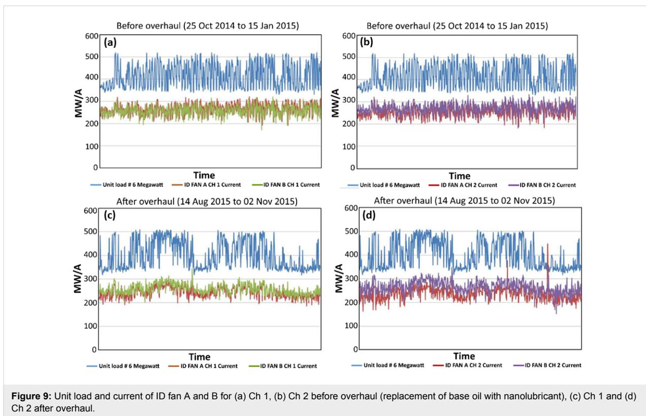
In summary, before the overhaul for Ch 1 there was no difference in current but after deployment of N-rGO nanolubricant the difference observed was 15 A. In case of Ch 2, before overhaul the difference was 20 Amp, which increased to 35 Amp after the implementation of nanolubricant. So, in conclusion the average difference due to the application of nanolubricant is 15 A for both channels.
