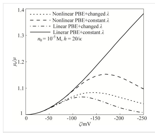
**Figure 3:** The effect of the zeta potential on the apparent viscosity of the lubricant based on different assumptions and theoretical models. The “Nonlinear PBE+changed  $\lambda$ ” case is the model established in the present work.
