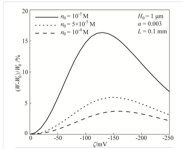
**Figure 6:** The effect of zeta potential on the hydrodynamic load capacity of the lubricant and the dependence of the hydrodynamic load capacity on the ion concentration based on the model of nonlinear PBE and varying electrical conductivity.
