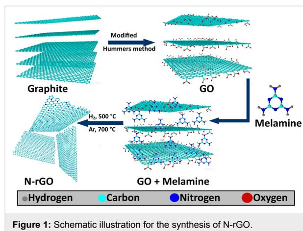
Figure 1: Schematic illustration for the synthesis of N-rGO.
