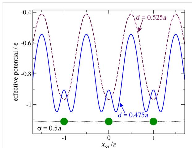
**Figure 2:** The potential-energy profile experienced by the slider as it moves along a hypothetical chain with atoms frozen at positions  $x_j = ja$  (big circles), for a LJ parameter  $\sigma = 0.5a$ . Dashed curve: as obtained with  $d = 0.525a > \sigma$ ; solid curve: with  $d = 0.475a < \sigma$ , the value adopted for the rest of this work.
