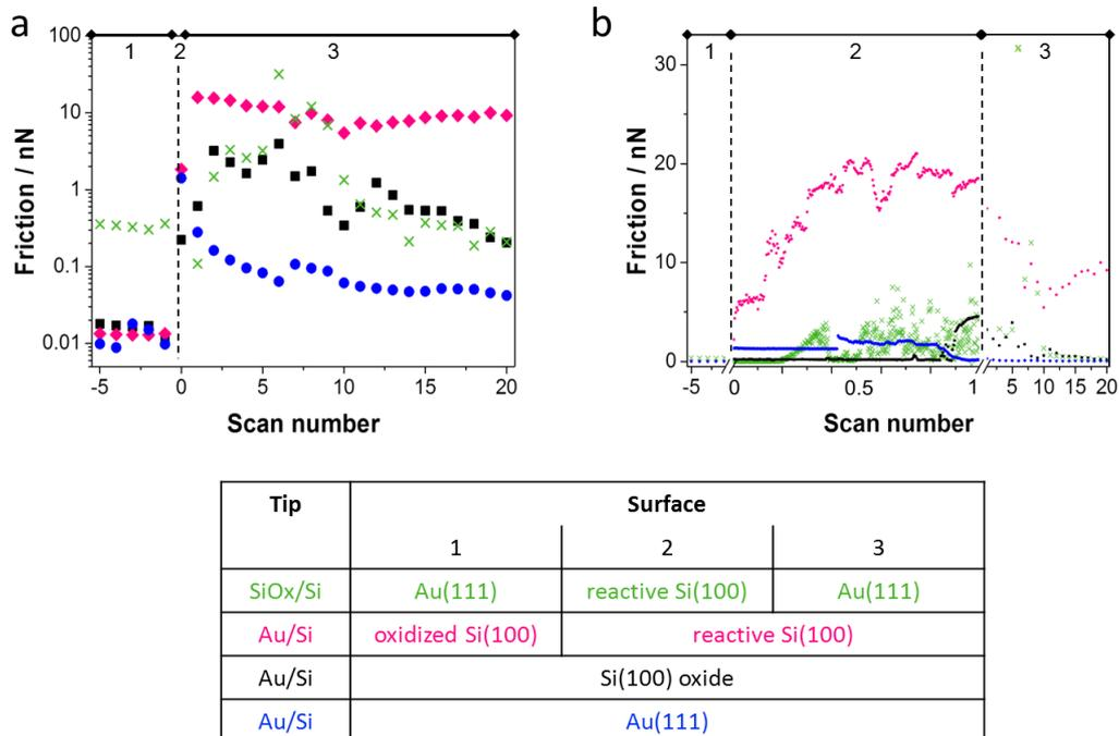
**Figure 3:** Development of friction for different tip–surface pairs upon activation of the interface. 1 – Control experiment with intact surface and tip; 2 – onset of activation; 3 – friction values for scanning sequences after activation. a) Emphasis on average friction values per scan before and after activation. b) Emphasis on the onset of the interfacial reaction showing the average friction values per scan line for the frame in which the activation occurred.
