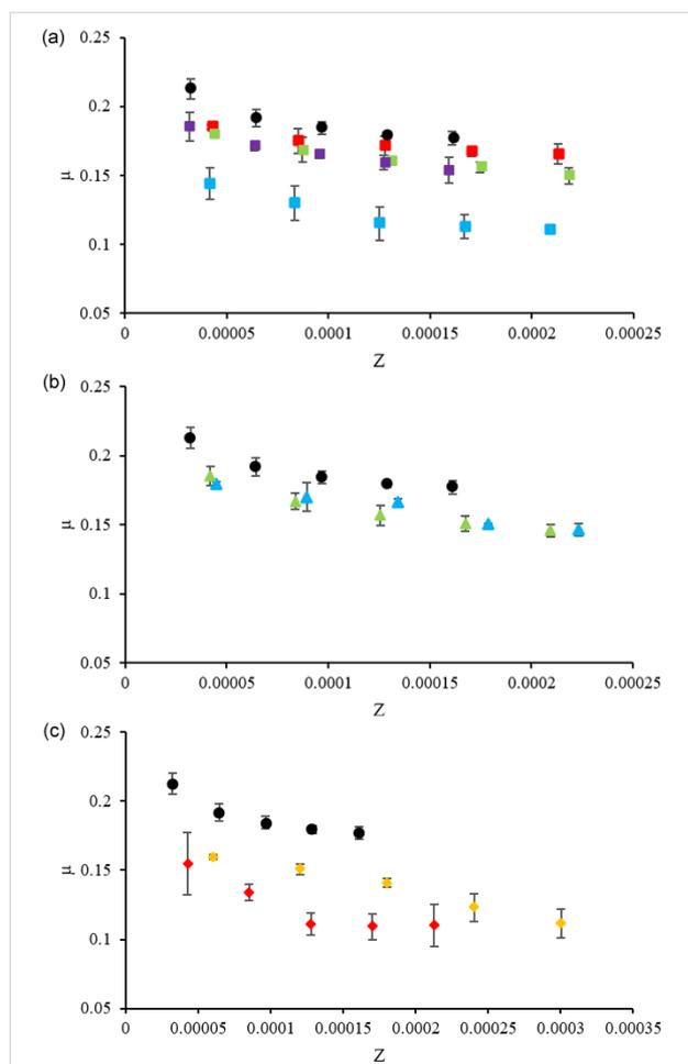
**Figure 5:** CoF vs Sommerfeld parameter,  $Z$ , for (a) TfO-based, (b) DCA-based and (c) EtSO<sub>4</sub>-based ILs mixed with PEG: PEG (black circles), PEG + [EMIM][TfO] (red squares), PEG + [BMIM][TfO] (blue squares), PEG + [C<sub>2</sub>OHMIM][TfO] (green squares), PEG + [AMIM][TfO] (purple squares), PEG + [BMIM][DCA] (blue triangles), PEG + [C<sub>2</sub>OHMIM][DCA] (green triangles), PEG + [EMIM][EtSO<sub>4</sub>] (red diamonds), PEG + [EMIM][EtSO<sub>4</sub>] (yellow diamonds).
