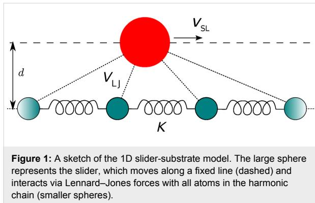
The slider is also a pointlike particle, with horizontal position  $x_{\text{SL}}$  and mass  $m_{\text{SL}}$ . We usually take  $m_{\text{SL}} > m$ , but this condition is by no means required. The slider follows a guide at a fixed distance  $d$  from the chain and interacts with each chain atom through a Lennard–Jones (LJ) term. Indicating with  $R_j = [d^2 + (x_{\text{SL}} - x_j)^2]^{1/2}$  the distance between the slider and the  $j$ -th particle, the total slider-chain interaction energy is
