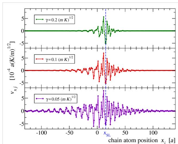
**Figure 5:** Three snapshots of the instantaneous velocities of a few chain atoms as a function of their position while interacting with the slider, whose instantaneous position  $x_{SL}$  is marked by a vertical dashed line. The three calculations are executed with the same  $v_{SL} = 0.1 v_s$ , but with three different values of  $\gamma$ , which produce visibly different damping of the same excited phonon waves away from the interaction point.
