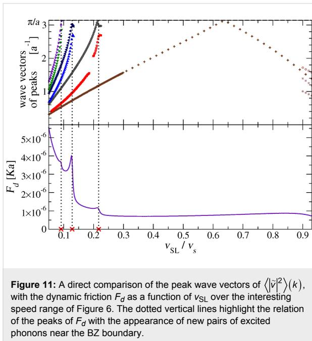
their phase velocities  $\omega/|k|$  match the slider speed  $v_{\text{SL}}$ . We start by searching all values of  $k$  such that the phonon phase velocity matches a given speed  $v_{\text{SL}}$ :
