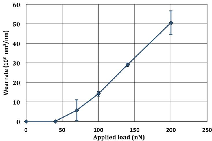
**Figure 6:** Wear rate as a function of the applied normal load with a given sliding velocity ( $880 \mu\text{m/s}$ ) and a 2 min duration wear. Experiments were carried with the  $\text{Si}_3\text{N}_4$  probe.
