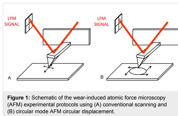
**Figure 1:** Schematic of the wear-induced atomic force microscopy (AFM) experimental protocols using (A) conventional scanning and (B) circular mode AFM circular displacement.
