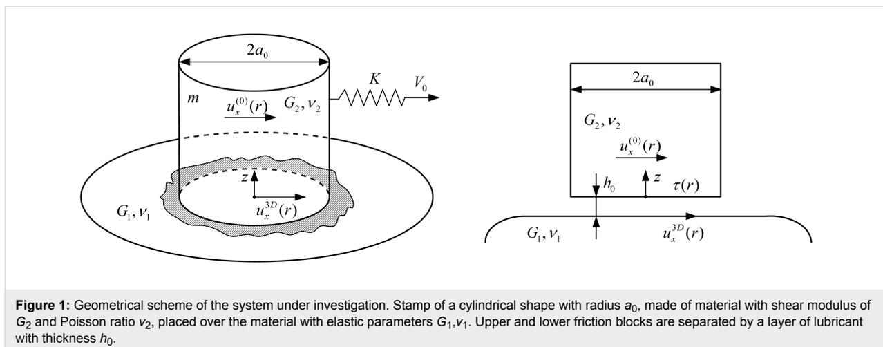
**Figure 1:** Geometrical scheme of the system under investigation. Stamp of a cylindrical shape with radius  $a_0$ , made of material with shear modulus of  $G_2$  and Poisson ratio  $\nu_2$ , placed over the material with elastic parameters  $G_1, \nu_1$ . Upper and lower friction blocks are separated by a layer of lubricant with thickness  $h_0$ .
