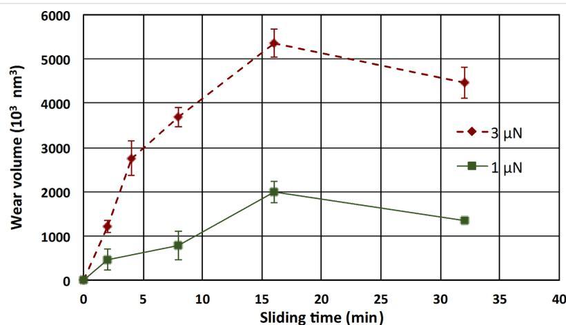
**Figure 5:** Wear volume as a function of the sliding time at a sliding velocity of 880  $\mu\text{m/s}$  and a normal load of 1  $\mu\text{N}$  (green squares) and 3  $\mu\text{N}$  (red diamonds). Experiments were carried with a diamond-like carbon (DLC) probe. Error bars are the standard deviation and the data result from an average between the maximum wear volume and the minimum wear volume issued from the calculation described in the Experimental section.
