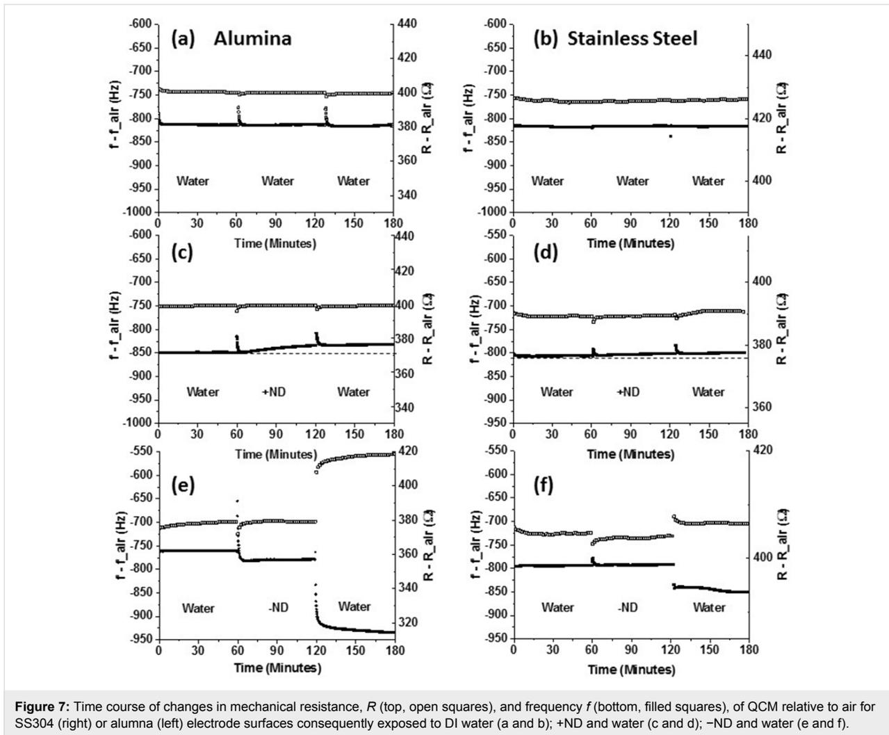
**Figure 7:** Time course of changes in mechanical resistance,  $R$  (top, open squares), and frequency  $f$  (bottom, filled squares), of QCM relative to air for SS304 (right) or alumina (left) electrode surfaces consequently exposed to DI water (a and b); +ND and water (c and d); -ND and water (e and f).
