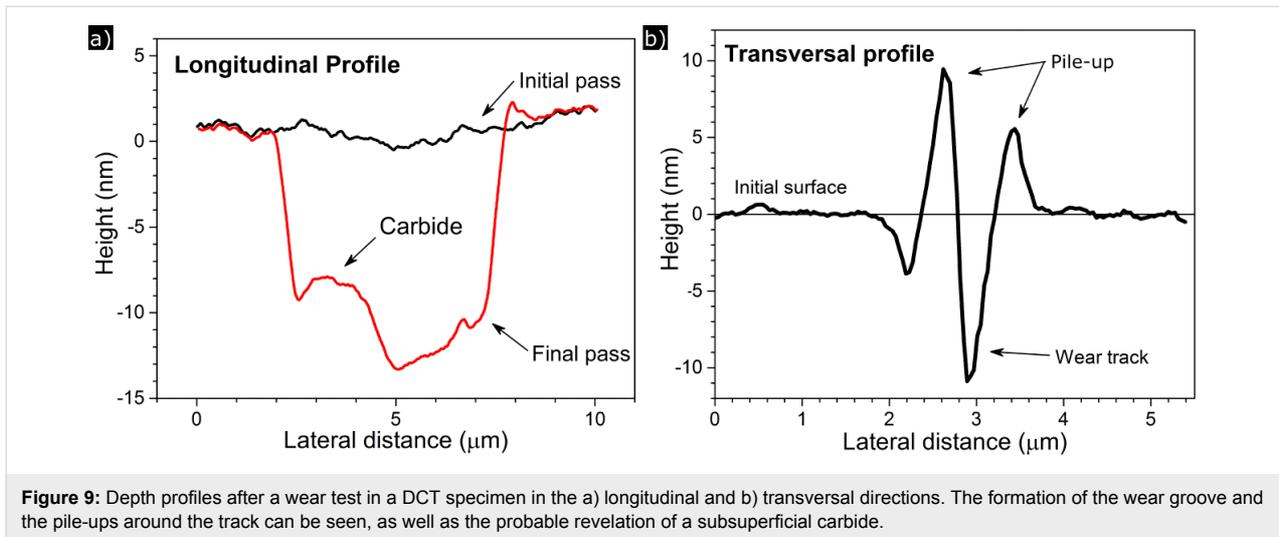
**Figure 9:** Depth profiles after a wear test in a DCT specimen in the a) longitudinal and b) transversal directions. The formation of the wear groove and the pile-ups around the track can be seen, as well as the probable revelation of a subsuperficial carbide.
