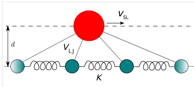
**Figure 1:** A sketch of the 1D slider-substrate model. The large sphere represents the slider, which moves along a fixed line (dashed) and interacts via Lennard–Jones forces with all atoms in the harmonic chain (smaller spheres).
