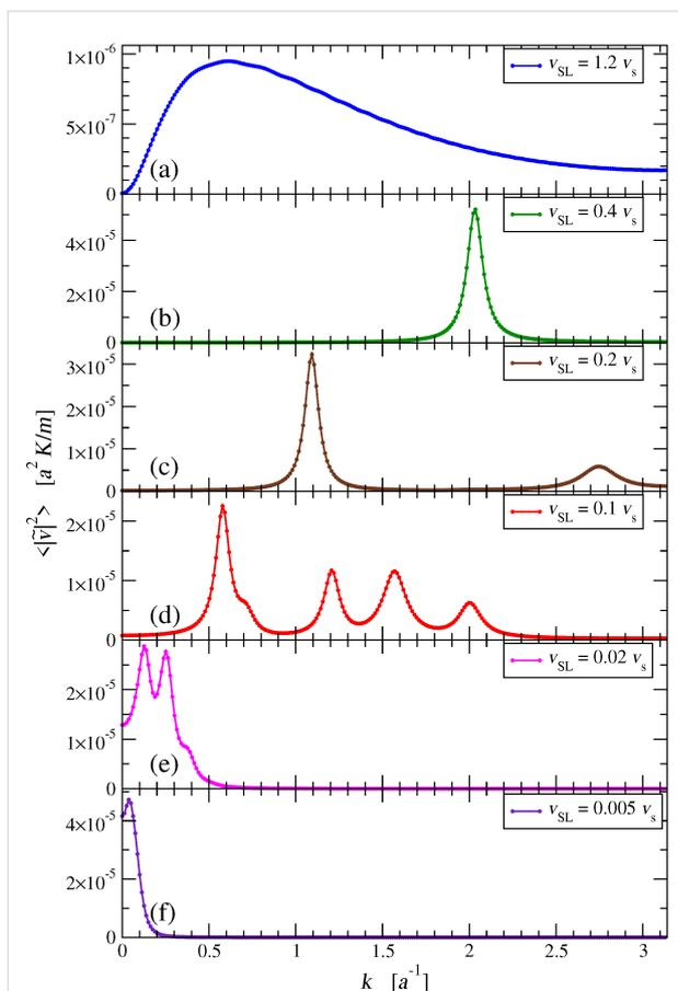
**Figure 9:** The time-averaged square modulus of the Fourier transform of the chain velocities, for a few characteristic values of  $v_{\text{SL}}$ : (a) supersonic speed; (b) single-peak subsonic region; (c) appearance of the second pair of peaks; (d) multi peak region near  $v_{\text{SL}} \approx 0.1 v_s$ ; (e) small-speed collapse of the dissipation peaks toward  $k = 0$ ; (f) full collapse to one peak at very small  $v_{\text{SL}} \ll v_s$ .
