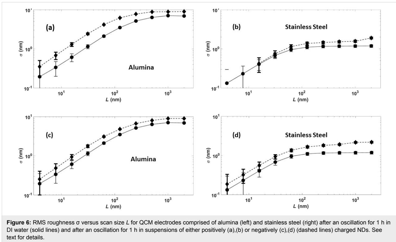
All samples exhibited increases in  $\sigma_s$  after an oscillation in ND suspensions (Table 2). Alumina surfaces, however, exhibited greater increases in  $\sigma_s$  than SS304. Only the SS304 sample exposed to +ND exhibited a change in  $D$ , increasing from 2.2 to 2.3, which corresponds to a more jagged surface texture [30]. It is interesting to note that this is the only surface studied that exhibited a striking increase in friction upon an exposure to the NDs.
