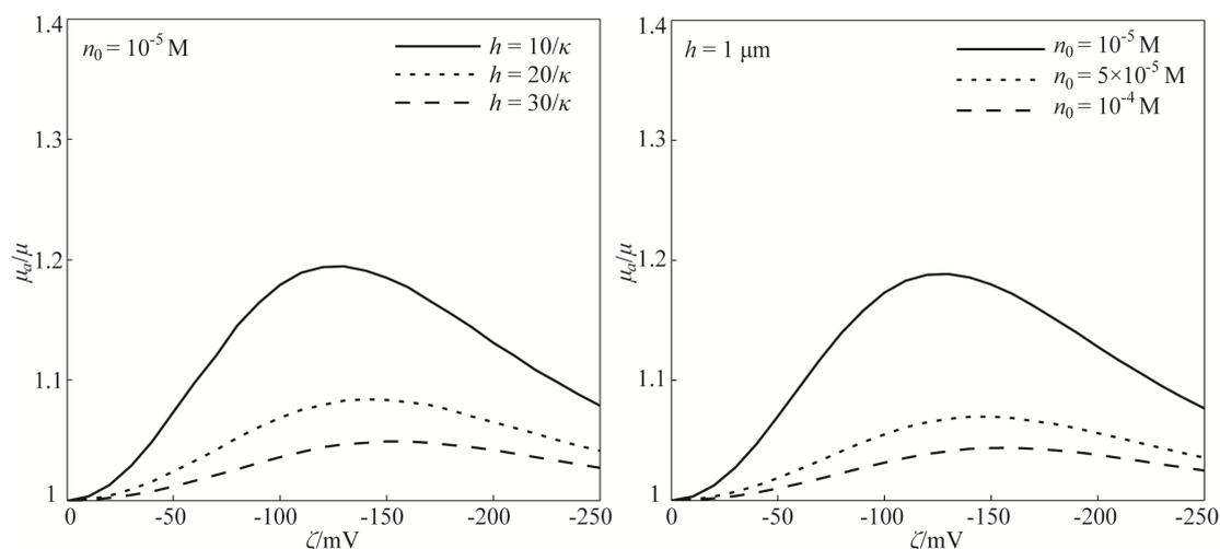
**Figure 4:** The effect of the zeta potential on the apparent viscosity of the lubricant and the dependence of the EDL-induced apparent viscosity on the lubricant film thickness and ion concentration of the lubricant based on the model of nonlinear PBE and modified electrical conductivity.
