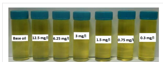
Figure 2: N-rGO dispersion nanolubricant at different concentration.
