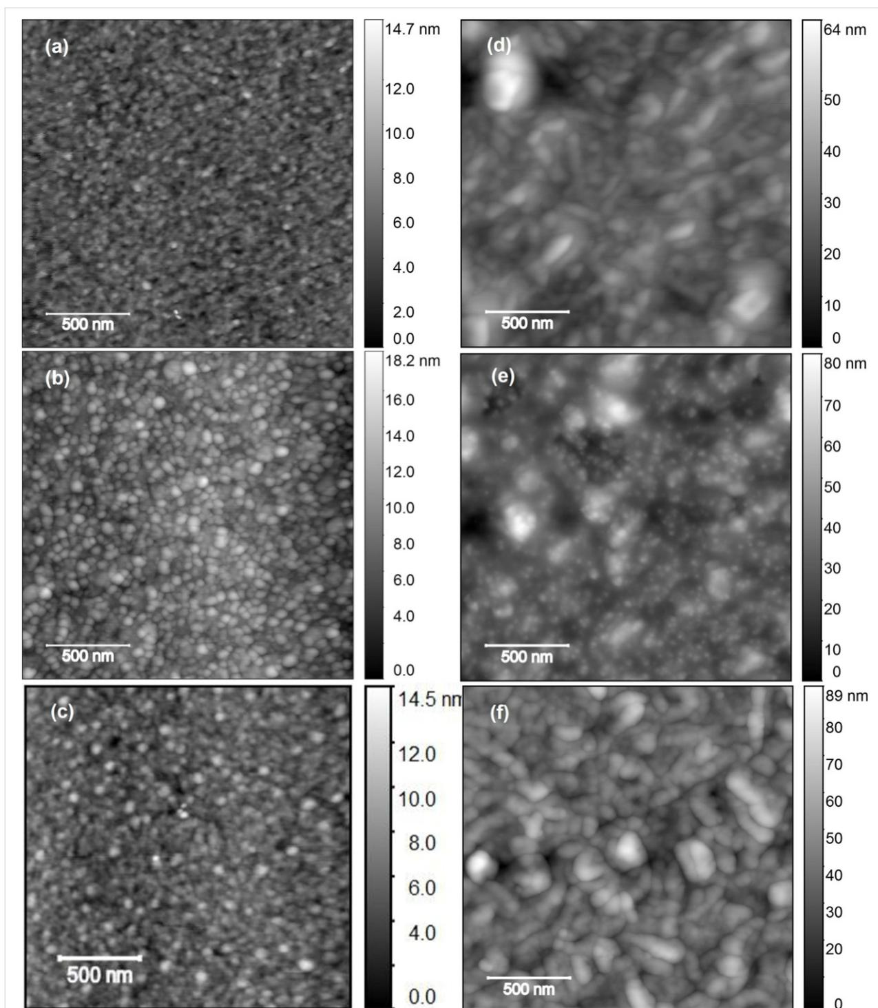
**Figure 4:** Representative AFM images of stainless steel 304 (left) and alumina (right) QCM electrodes after 1 h of oscillation in DI water (upper), -ND (middle) and +ND (lower) suspensions and then rinsing in DI water.
