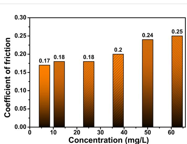
Figure 5: Coefficient of friction at high N-rGO concentrations.
