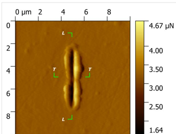
**Figure 8:** Scanning probe microscopy (SPM) image after 30 cycles of nanoscratch testing in a DCT specimen. The depth profiles below in Figure 9 were taken in the longitudinal (L–L) and transversal (T–T) directions.
