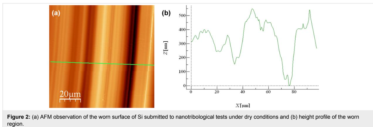
**Figure 2:** (a) AFM observation of the worn surface of Si submitted to nanotribological tests under dry conditions and (b) height profile of the worn region.
