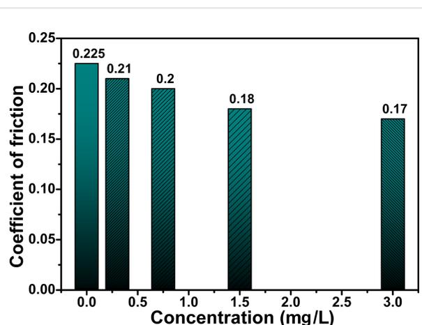
Figure 4: Coefficient of friction at low N-rGO concentrations.
