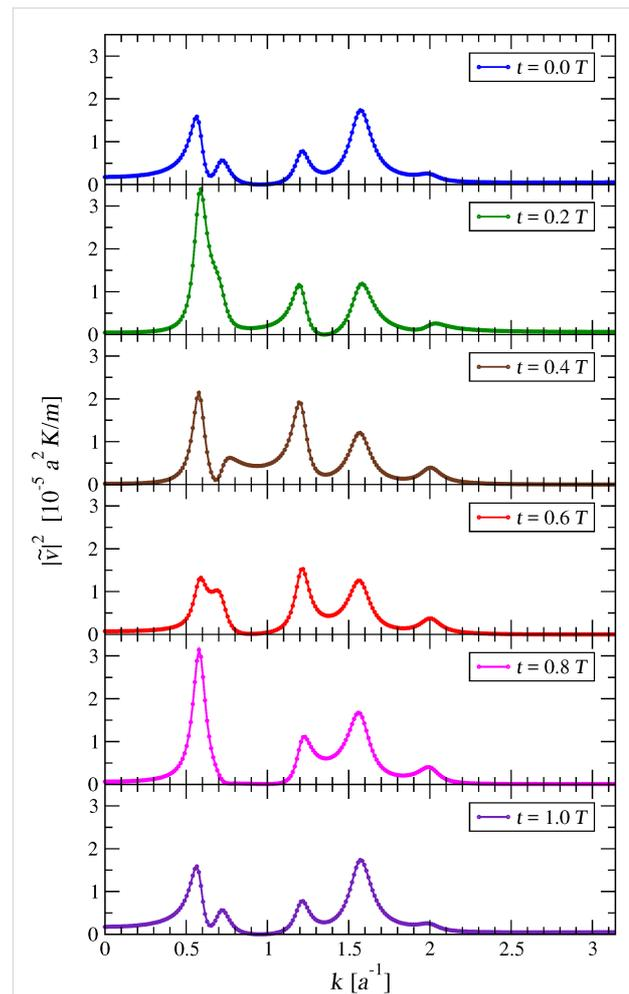
**Figure 8:** The square modulus of the Fourier transforms of the velocities  $v_j(t)$ , at six subsequent times. Here the slider velocity is  $v_{\text{SL}} = 0.1 v_s$ . Comparing the plots of  $|\tilde{v}(k, 0)|^2$  and  $|\tilde{v}(k, T)|^2$ , one sees that  $|\tilde{v}|^2$  repeats itself identically after one entire period  $T = a/v_{\text{SL}} = 10 (m/K)^{1/2}$ .
