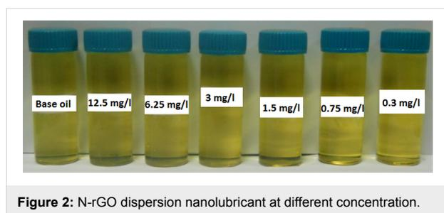
Figure 2: N-rGO dispersion nanolubricant at different concentration.
