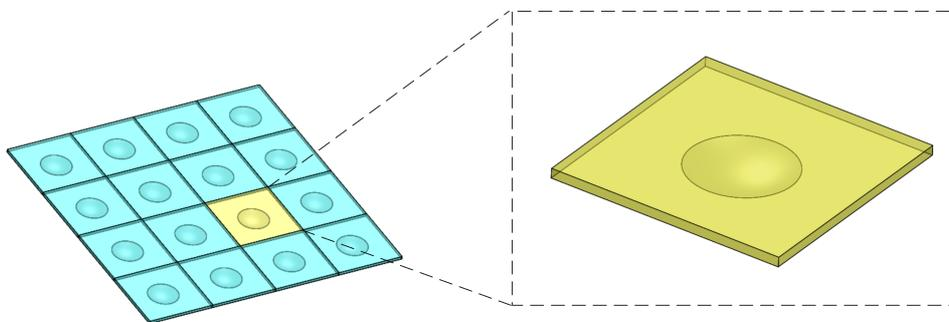
**Figure 1:** Three-dimensional geometric model of fluid in a micro-dimple array and a single micro-dimple unit.
