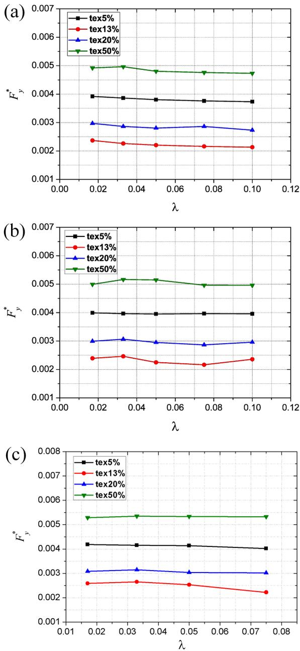
**Figure 12:** Effect of texture density and aspect ratio on the dimensionless average film shear force for (a)  $Re = 5$ , (b)  $Re = 50$  and (c)  $Re = 250$ .
