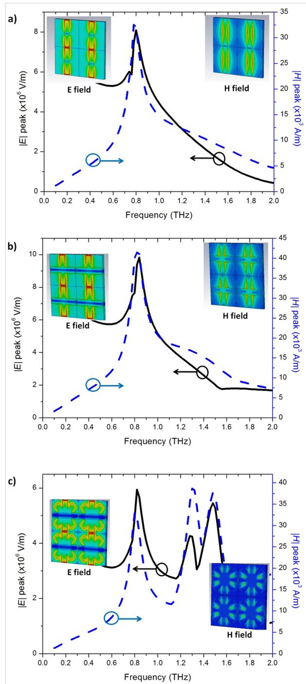
**Figure 6:** The peak value of electric field and magnetic field of: a) Cut-wire sandwich structure, b) cross-shaped sandwich structure, and c) star-shaped sandwich structure. The insets of (a–c) in each panel show electric and magnetic field distributions of the cut-wire sandwich structure at 0.78 THz, cross-shaped sandwich structure at 0.82 THz, and star-shaped sandwich structure at 0.81 THz, respectively.
