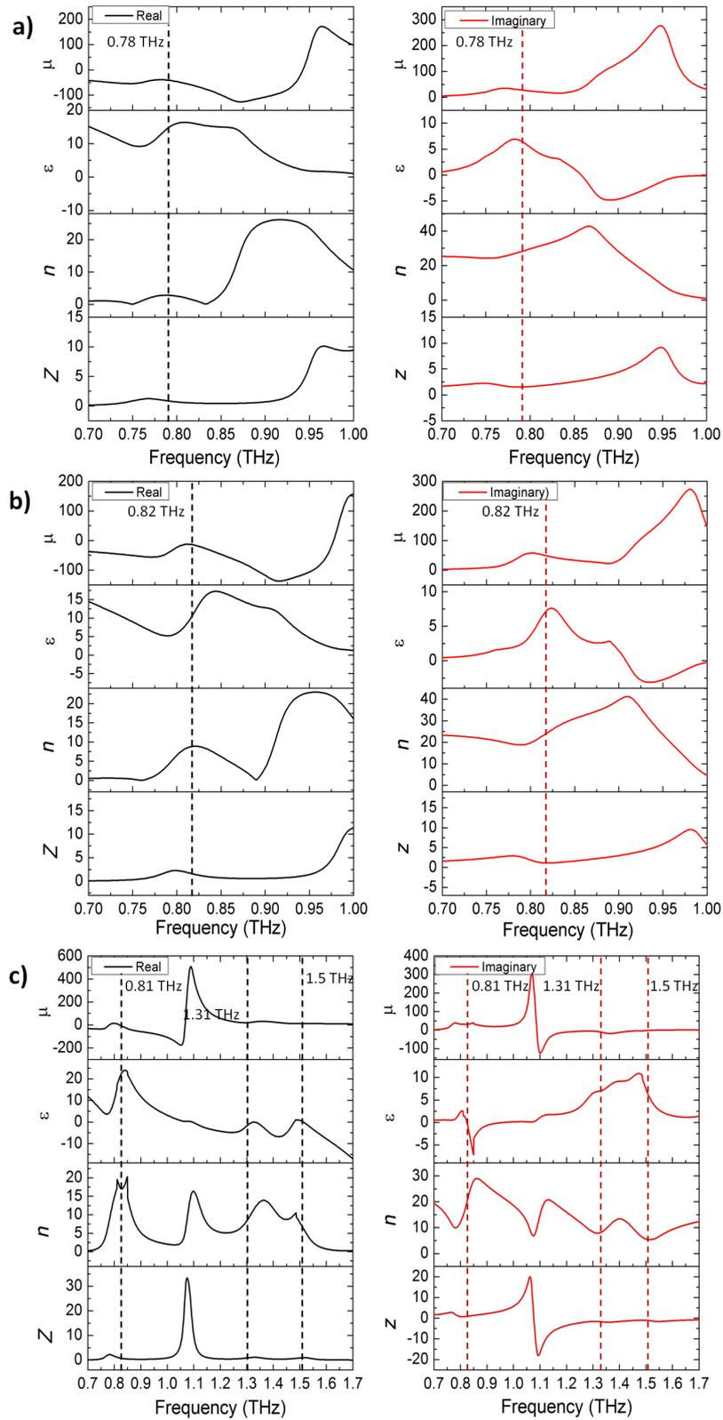
**Figure 5:** Permeability ( $\mu$ ), permittivity ( $\epsilon$ ), refractive index ( $n$ ), and impedance ( $Z$ ) properties of: a) Cut-wire sandwich structure, b) cross-shaped sandwich structure, and c) star-shaped sandwich structure. The black and red curves represent the real and imaginary part of each value, respectively.
