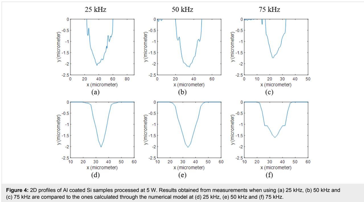
**Figure 4:** 2D profiles of Al coated Si samples processed at 5 W. Results obtained from measurements when using (a) 25 kHz, (b) 50 kHz and (c) 75 kHz are compared to the ones calculated through the numerical model at (d) 25 kHz, (e) 50 kHz and (f) 75 kHz.
