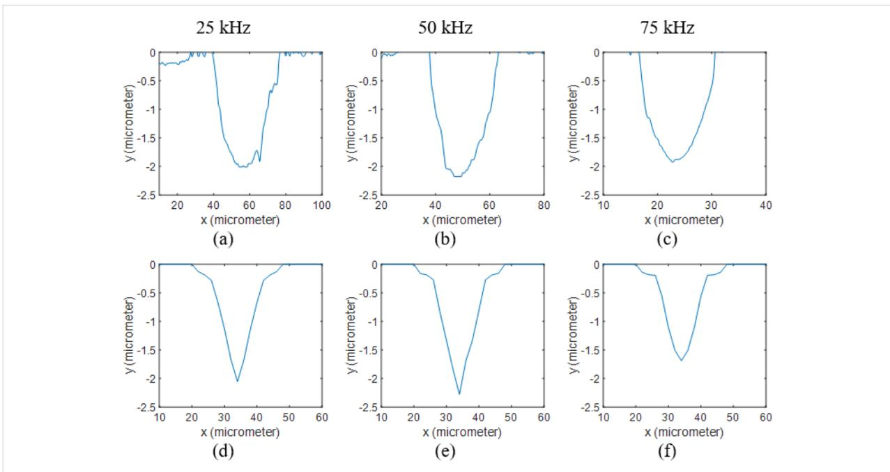
**Figure 6:** 2D profiles of Au coated Si samples processed at 5 W. Results obtained from measurements when using (a) 25 kHz, (b) 50 kHz and (c) 75 kHz are compared to the ones calculated through the numerical model at (d) 25 kHz, (e) 50 kHz and (f) 75 kHz.
