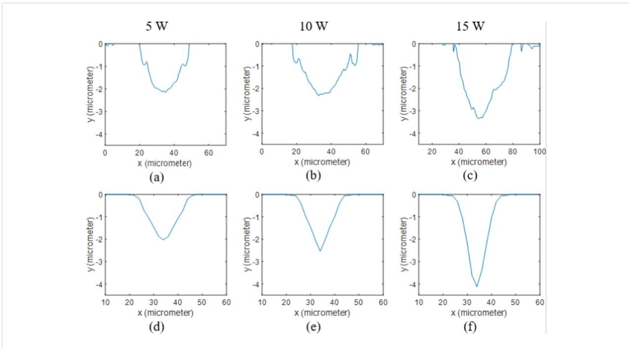
**Figure 5:** 2D profiles of Al coated Si samples processed at 50 kHz. Results obtained from measurements when using (a) 5 W, (b) 10 W and (c) 15 W are compared to the ones calculated through the numerical model at (d) 5 W, (e) 10 W and (f) 15 W.
