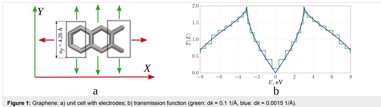
**Figure 1:** Graphene: a) unit cell with electrodes; b) transmission function (green:  $dk = 0.1 \text{ 1/\AA}$ , blue:  $dk = 0.0015 \text{ 1/\AA}$ ).
