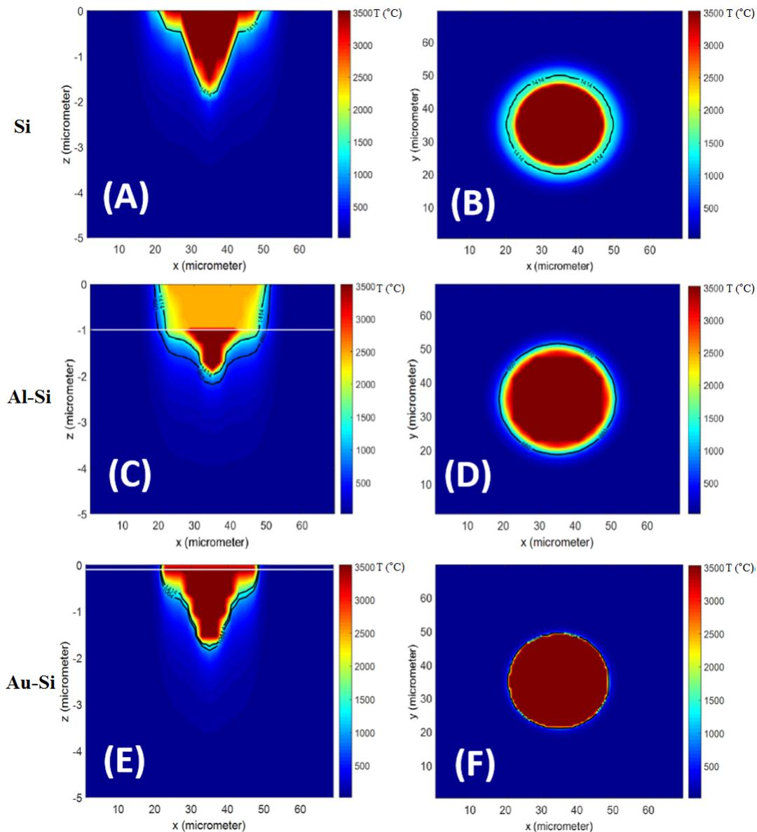
**Figure 3:** Temperature contours obtained from the numerical model at the end of the pulse at 50 kHz and 5 W for (a) cross-section of uncoated Si, (b) surface of uncoated Si, (c) cross-section of Al coated Si (d) surface of Al coated Si, (e) cross-section of Au coated Si, (f) surface of Au coated Si. The melting points of the materials are depicted by black lines and the interface between the layers is shown by white lines.
