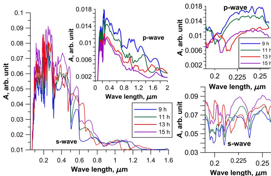
**Figure 6:** The absorption coefficient of 2D CNT-graphene hybrid nanocomposite with the same tube (18,0) and different intertube distances. The insets on the right side show the absorption coefficient for the wavelength range of 190–260 nm.
