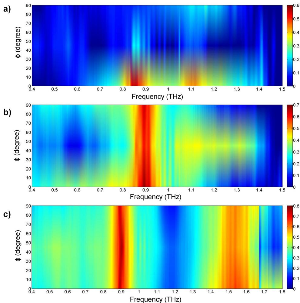
**Figure 9:** Measured absorbance results for polarization angles from  $0^\circ$  to  $90^\circ$  for: a) Cut-wire sandwich structure, b) cross-shaped sandwich structure, and c) star-shaped sandwich structure.
