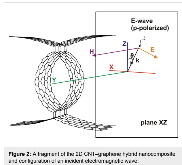
**Figure 2:** A fragment of the 2D CNT–graphene hybrid nanocomposite and configuration of an incident electromagnetic wave.
