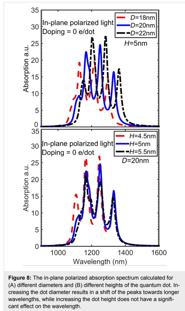
**Figure 8:** The in-plane polarized absorption spectrum calculated for (A) different diameters and (B) different heights of the quantum dot. Increasing the dot diameter results in a shift of the peaks towards longer wavelengths, while increasing the dot height does not have a significant effect on the wavelength.
