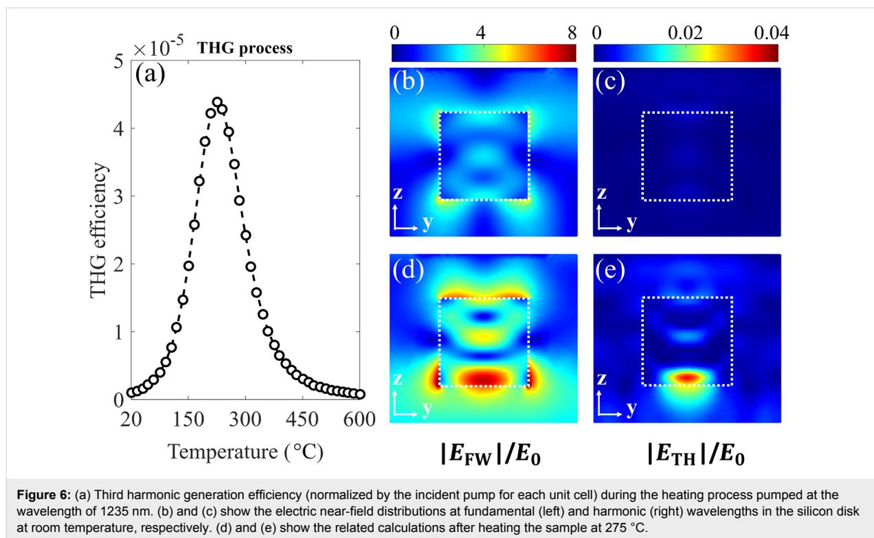
**Figure 6:** (a) Third harmonic generation efficiency (normalized by the incident pump for each unit cell) during the heating process pumped at the wavelength of 1235 nm. (b) and (c) show the electric near-field distributions at fundamental (left) and harmonic (right) wavelengths in the silicon disk at room temperature, respectively. (d) and (e) show the related calculations after heating the sample at 275  $^{\circ}\text{C}$ .
