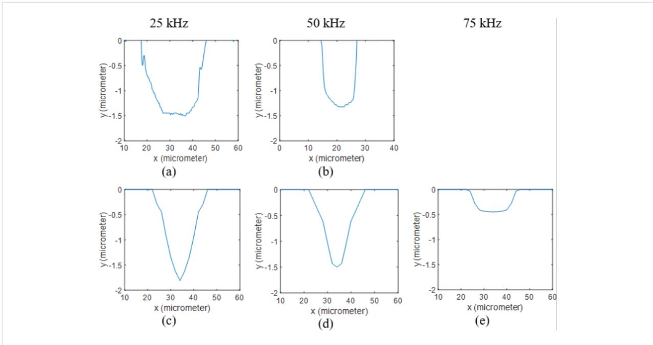
**Figure 1:** 2D profiles of uncoated Si samples processed at 5 W. Results obtained from measurements when using (a) 25 kHz and (b) 50 kHz are compared to the ones calculated through the numerical model at (c) 25 kHz, (d) 50 kHz and (e) 75 kHz.
