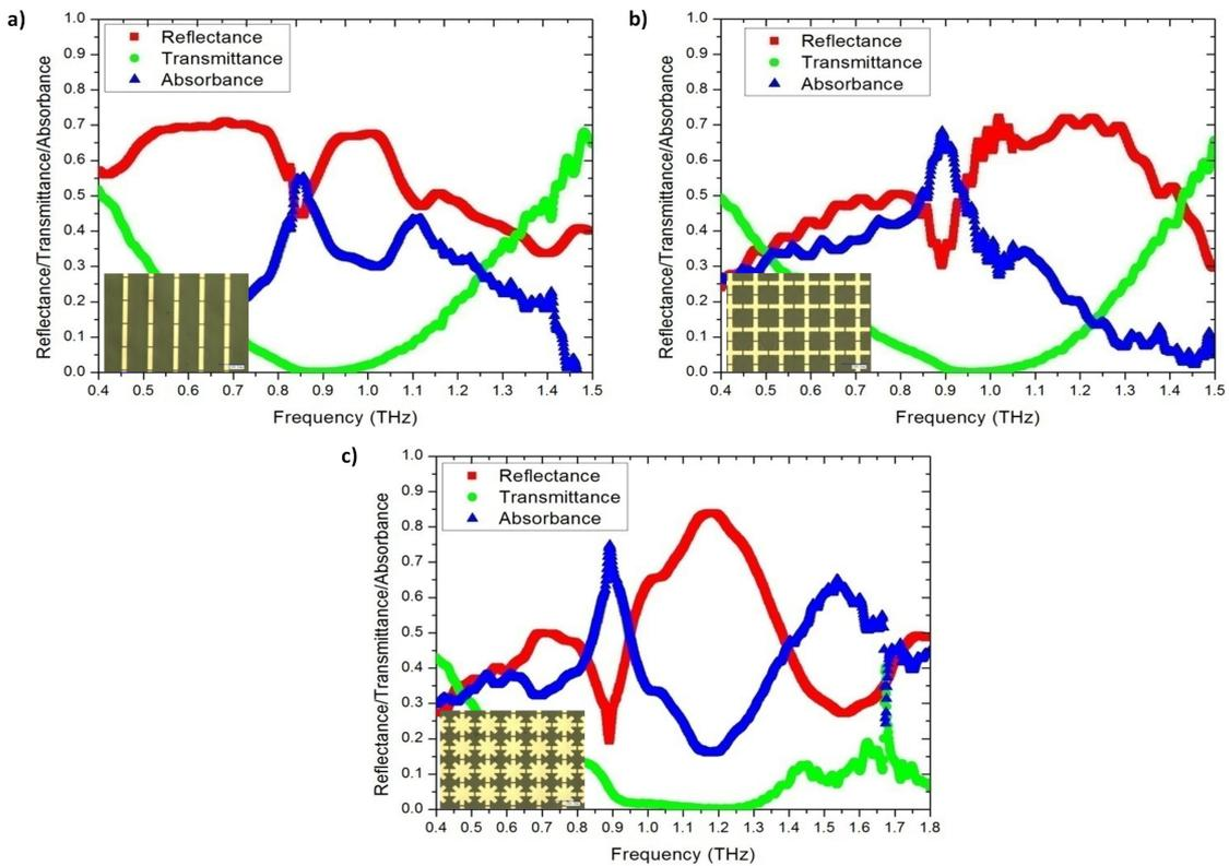
**Figure 8:** The measured results of reflectance, transmittance and absorbance under normal incidence: a) Cut-wire sandwich structure, b) cross-shaped sandwich structure, and c) star-shaped sandwich structure.
