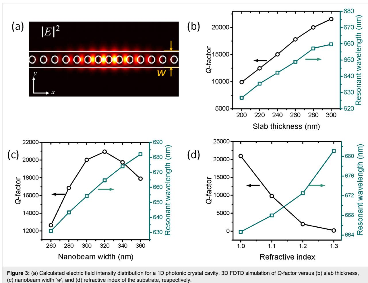
**Figure 3:** (a) Calculated electric field intensity distribution for a 1D photonic crystal cavity. 3D FDTD simulation of  $Q$ -factor versus (b) slab thickness, (c) nanobeam width ‘ $w$ ’, and (d) refractive index of the substrate, respectively.
