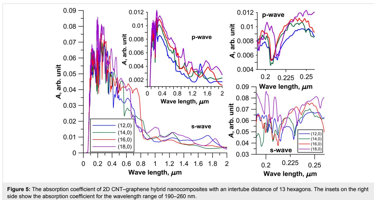
**Figure 5:** The absorption coefficient of 2D CNT–graphene hybrid nanocomposites with an intertube distance of 13 hexagons. The insets on the right side show the absorption coefficient for the wavelength range of 190–260 nm.
