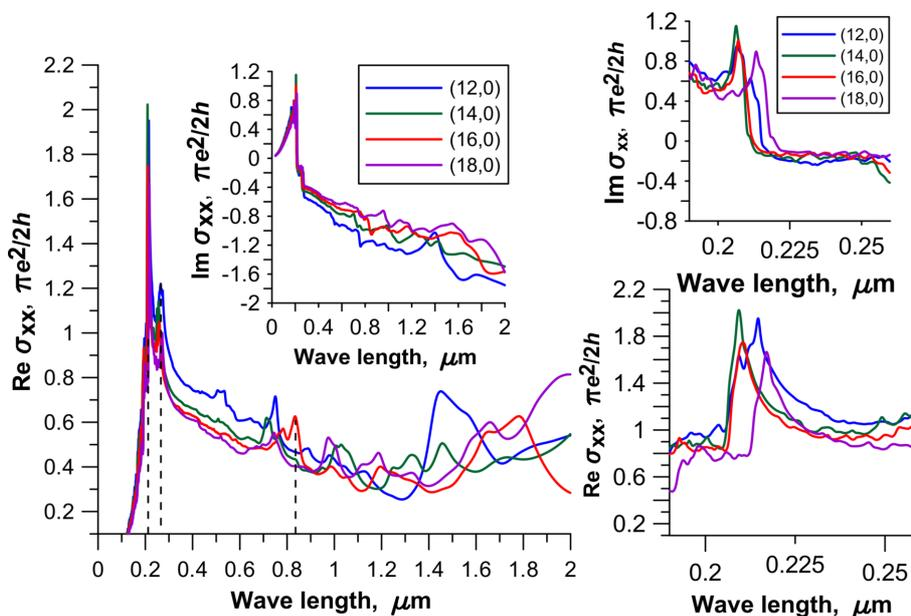
**Figure 3:** The optical conductivity of 2D CNT–graphene hybrid nanocomposites with an intertube distance of 13 hexagons in the direction perpendicular to the nanotube axis. The insets on the right side show the graphs of optical conductivity for the wavelength range of 190–260 nm.
