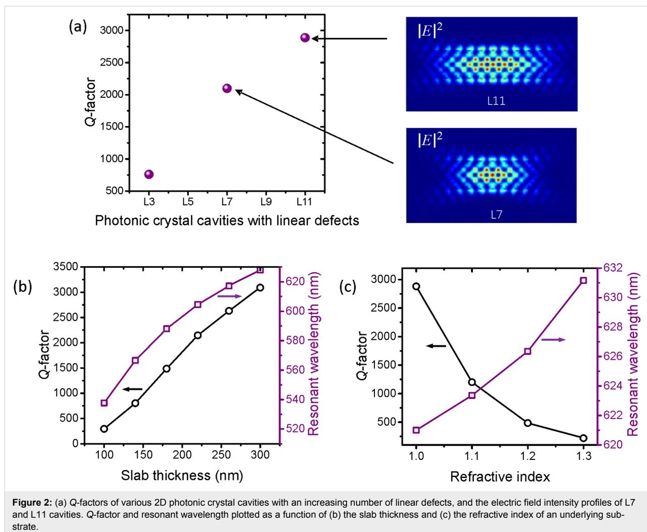
**Figure 2:** (a)  $Q$ -factors of various 2D photonic crystal cavities with an increasing number of linear defects, and the electric field intensity profiles of L7 and L11 cavities.  $Q$ -factor and resonant wavelength plotted as a function of (b) the slab thickness and (c) the refractive index of an underlying substrate.
