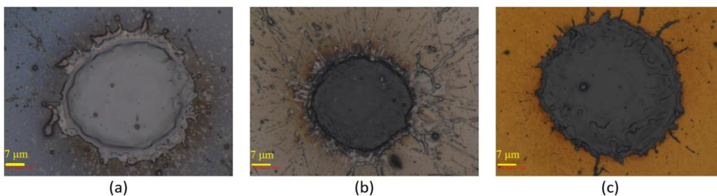
**Figure 8:** (a) Isolated pulse on the surface of silicon, (b) Isolated pulse on the surface of silicon coated by aluminum thin film, (c) Isolated pulse on the surface of silicon coated by gold thin film.
