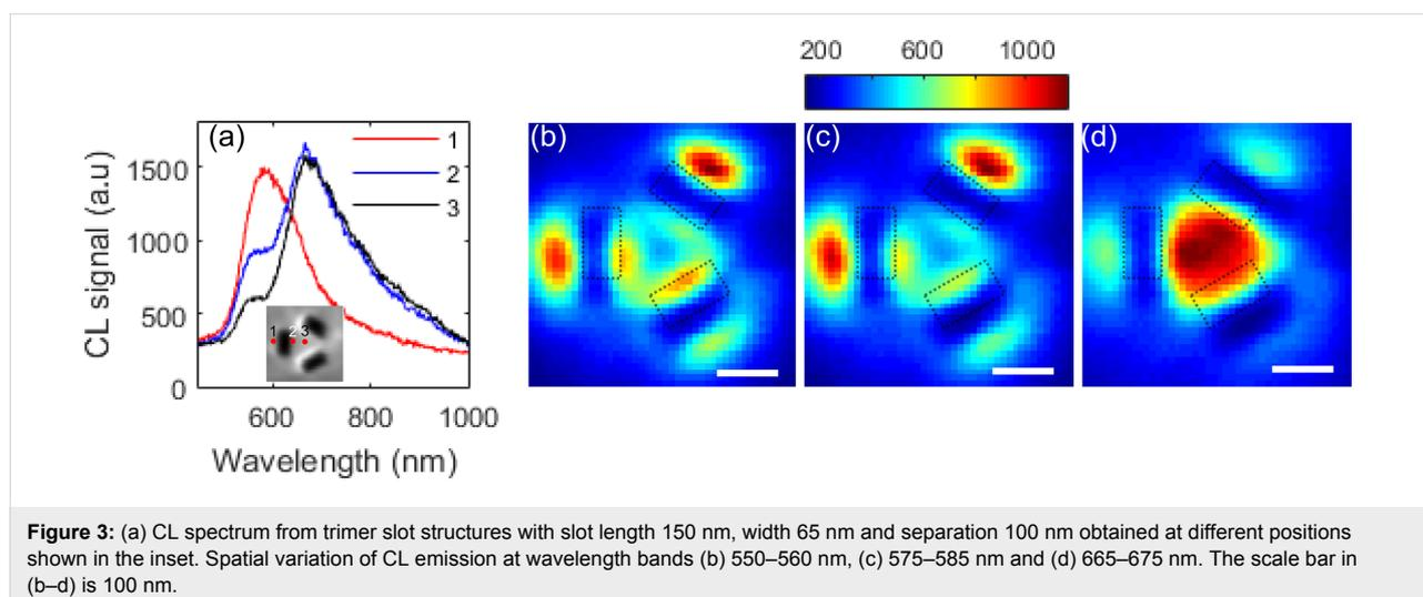
depends on the excitation point and that the emission into different wavelength bands depends on the spatial location. At shorter wavelengths, we see that excitation just outside the slots produces the strongest CL emission, but when electrons are incident in the central region, the peak in emission is red-shifted.
