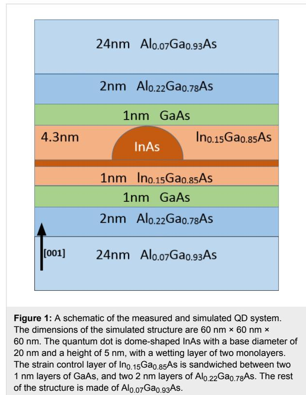
The band structure calculations do not need all of atoms to be included in the simulation, since bound states decay exponentially outside the quantum dot. The band structure calculations are performed using a  $40\text{ nm} \times 40\text{ nm} \times 20\text{ nm}$  box surrounding the quantum dot. This box contains only 1.5 million atoms. Well-defined and well-calibrated tight-binding models are
