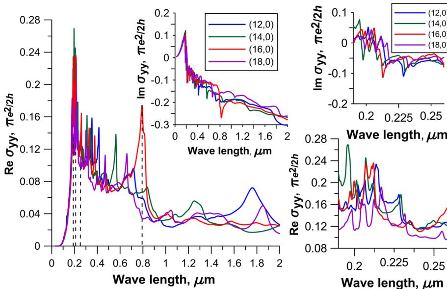
**Figure 4:** The optical conductivity of 2D CNT–graphene hybrid nanocomposites with an intertube distance of 13 hexagons along the nanotube axis. The insets on the right side show the graphs of optical conductivity for the wavelength range of 190–260 nm.
