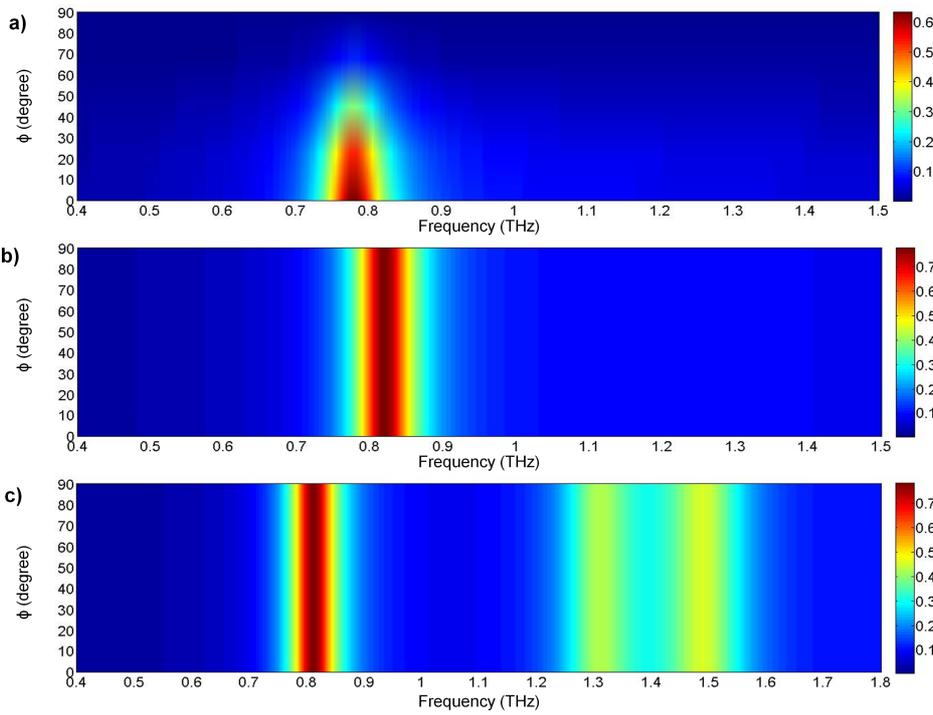
**Figure 7:** The simulation result of the absorbance difference for polarization angles from 0° to 90° of: a) Cut-wire sandwich structure, b) cross-shaped sandwich structure, and c) star-shaped sandwich structure.
