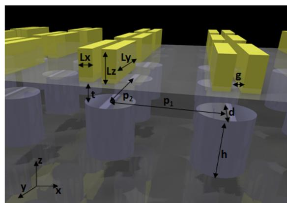
**Figure 1:** Diagram of the metasurface. The geometrical parameters are  $L_x = 100$  nm,  $L_y = 600$  nm,  $L_z = 200$  nm,  $t = 200$  nm,  $d = 400$  nm,  $h = 400$  nm,  $g = 60$  nm,  $p_1 = 850$  nm,  $p_2 = 850$  nm.
