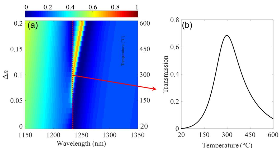
**Figure 4:** (a) The transmission spectrum during the heating process. (b) The transmission at 1235 nm during the heating process.
