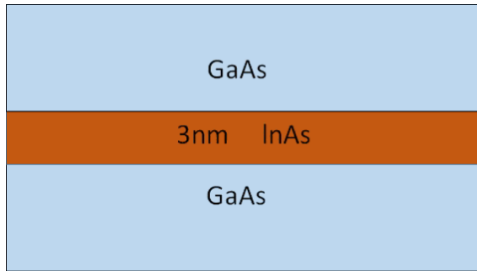
Figure 4: An InAs/GaAs quantum well of thickness 3 nm used for the optimization of the anharmonic strain model.
