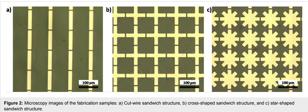
**Figure 2:** Microscopy images of the fabrication samples: a) Cut-wire sandwich structure, b) cross-shaped sandwich structure, and c) star-shaped sandwich structure.
