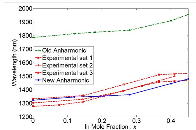
**Figure 10:** Experimental and simulation results of the optical transition of the QD system reported in [9]. Increasing the In mole fraction increases the transition wavelength. The optimization of the anharmonic strain model has greatly improved the simulation results.
