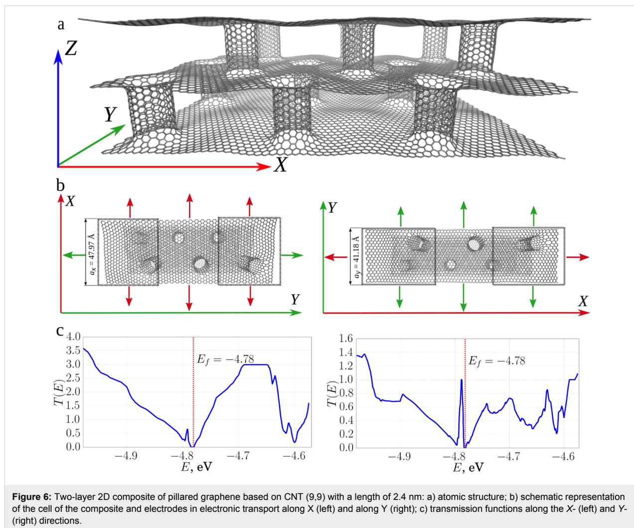
**Figure 6:** Two-layer 2D composite of pillared graphene based on CNT (9,9) with a length of 2.4 nm: a) atomic structure; b) schematic representation of the cell of the composite and electrodes in electronic transport along X (left) and along Y (right); c) transmission functions along the X- (left) and Y- (right) directions.
