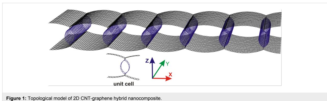
**Figure 1:** Topological model of 2D CNT-graphene hybrid nanocomposite.
