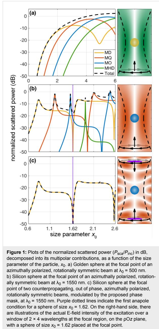
$\alpha_0 = 400$  nm. We have already avoided any interference by the electric modes and this sphere could be a promising candidate to host a magnetic anapole state, if it were not, as we can see, for the overlapping magnetic quadrupole and octupole that interfere and spoil the anapole condition of the magnetic dipole.
