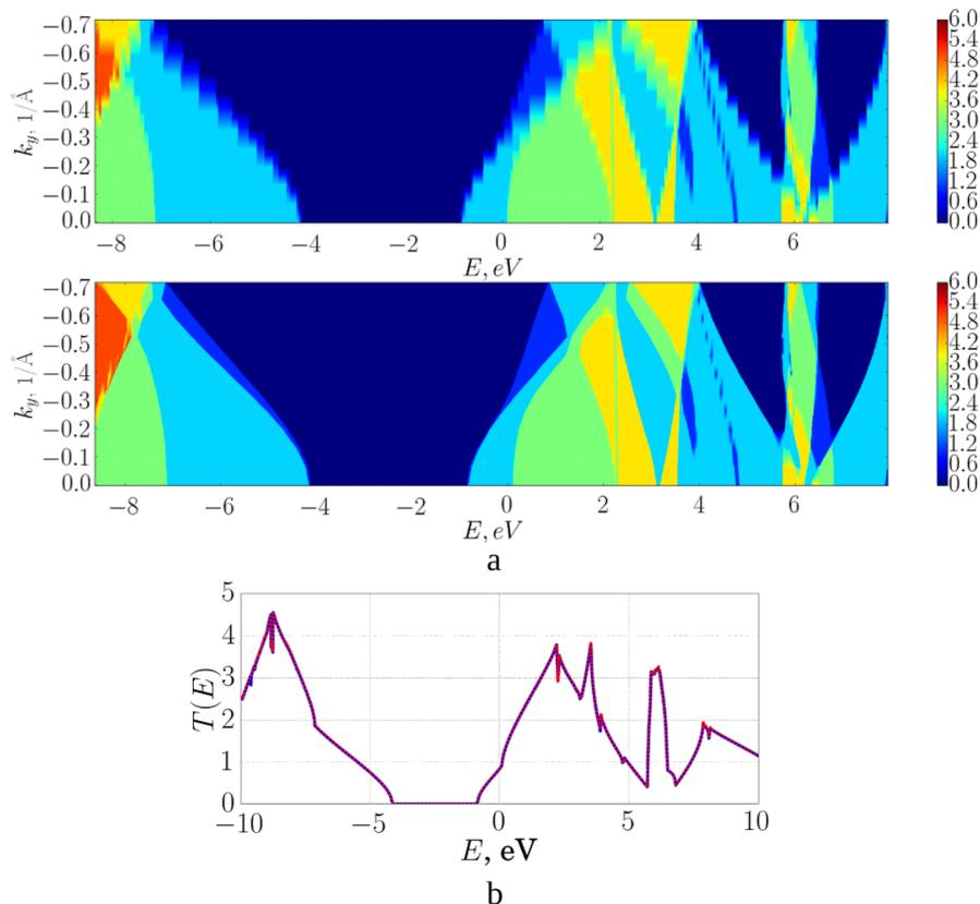
**Figure 4:** Graphane transmission function: a) a map of  $T(E)$  for the initial partitioning over  $k_y$  (top) and (bottom) after applying the interpolating function  $T(E, k_y)$ ; b) averaged  $T(E)$  over all  $k_y$  (blue: interpolated, red: converged).
