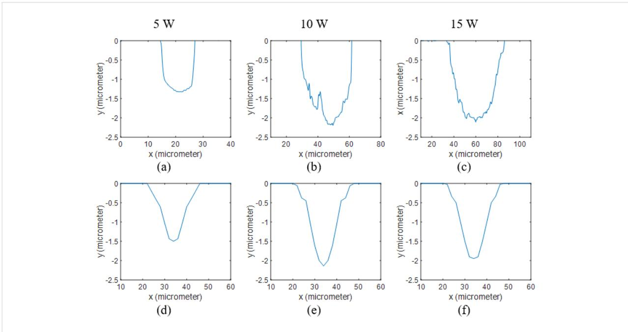
**Figure 2:** 2D profiles of uncoated Si samples processed at 50 kHz. Results obtained from measurements when using (a) 5 W, (b) 10 W and (c) 15 W are compared to the ones calculated through the numerical model at (d) 5 W, (e) 10 W and (f) 15 W.
