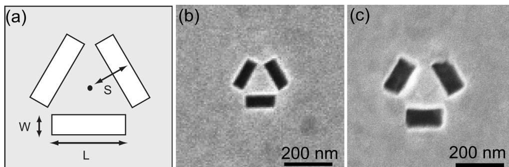
**Figure 1:** Scanning electron micrographs aperture structures with dimensions defined in (a). Fabricated slot trimer structures with (b)  $L = 95$  nm,  $W = 34$  nm and  $S = 60$  nm, and (c)  $L = 150$  nm,  $W = 40$  and  $S = 100$  nm.
