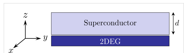
Figure 1: A 2DEG is proximity-coupled to an s -wave superconductor with finite thickness d . Both systems are taken to be infinite in the xy -plane.
