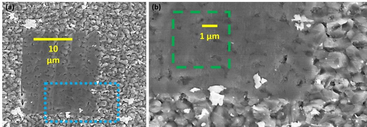
**Figure 3:** (a) SEM micrograph of a locally planarized polycrystalline CdTe solar cell. The dotted rectangular overlay indicates the location of a higher-magnification SEM image (b) in which the dashed square outline identifies the area studied for Figure 2 and Figure 4.
