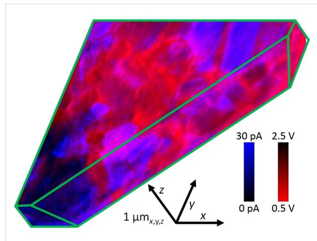
**Figure 4:** Three-dimensional CT-AFM of the short-circuit current ( $I_{SC}^*$ , dark to blue contrast) merged with the directly measured open-circuit voltage ( $V_{OC}^*$ , red to dark) volumetrically rendered to partially reveal an  $xy$  plane,  $xz$  and  $yz$  cross sections, and an oblique  $xyz$  cut to uniquely expose the nanoscale properties through the specimen thickness. The identified axes also serve as scale bars.
