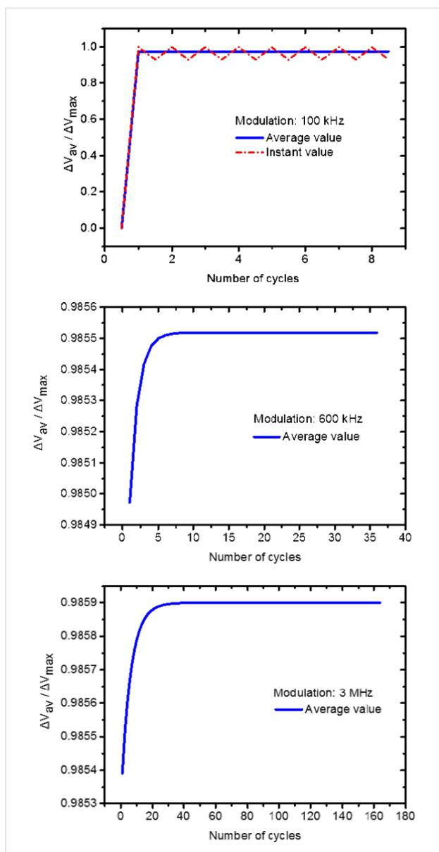
**Figure 6:** Simulated  $SPV_{AV}$  as a function of the number of excitation cycles for different excitation modulation frequencies. From top to bottom: 100 kHz, 600 kHz and 3 MHz. The simulation at 100 kHz includes the SPV instant value oscillation as depicted by the red dashed line. The graphs depicting the results from simulations at 600 kHz and 3 MHz were zoomed-in so that the convergence process can be noticed.
