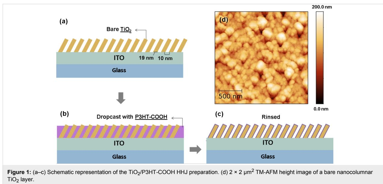
**Figure 1:** (a–c) Schematic representation of the TiO<sub>2</sub>/P3HT-COOH HHJ preparation. (d) 2 × 2 μm<sup>2</sup> TM-AFM height image of a bare nanocolumnar TiO<sub>2</sub> layer.
