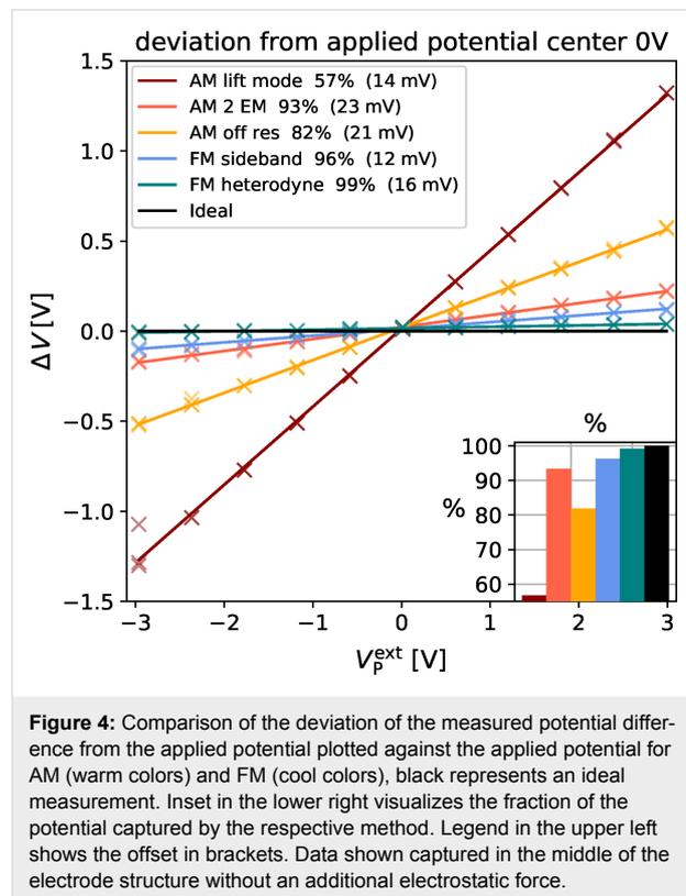
**Figure 4:** Comparison of the deviation of the measured potential difference from the applied potential plotted against the applied potential for AM (warm colors) and FM (cool colors), black represents an ideal measurement. Inset in the lower right visualizes the fraction of the potential captured by the respective method. Legend in the upper left shows the offset in brackets. Data shown captured in the middle of the electrode structure without an additional electrostatic force.
