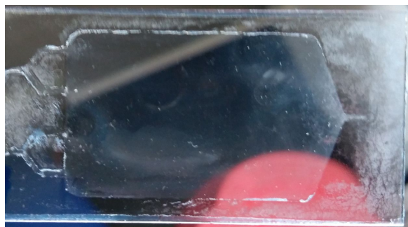
Figure 2: Chamber cover after deposition. The shape of the chamber is outlined by the PTFE paste used for sealing. A white film can be seen on the glass slide.
