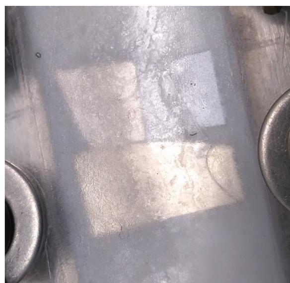
**Figure 3:** Samples in chamber during deposition, immediately before being taken out of the chamber. The glass slide was held in place by an acrylic block, immediately upon removal of the block the chamber unsealed and the films started reacting with air.
