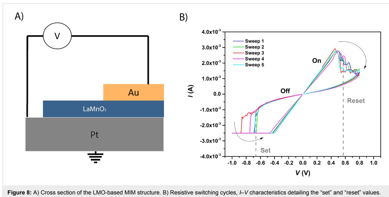
**Figure 8:** A) Cross section of the LMO-based MIM structure. B) Resistive switching cycles,  $I$ - $V$  characteristics detailing the “set” and “reset” values.
