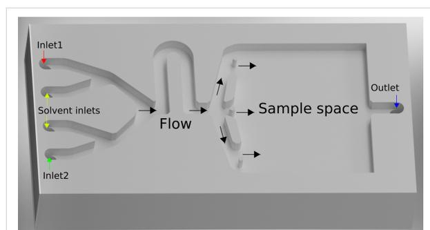
**Figure 1:** Illustration of the experimental deposition chamber. Top view, without cover. The chamber is closed from the top and then sequentially flooded with solutions.
