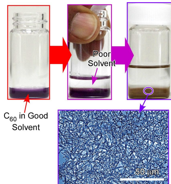
Figure 15: Liquid-liquid interfacial precipitation to fabricate fullerene assemblies (crystals) with various morphologies (in this case, assembly of one-dimensional nanowhiskers). Fullerene molecules, such as C_{60} and C_{70} , are dissolved in a liquid phase (good solvent) that contacts an immiscible liquid phase in which the molecules are poorly soluble (poor solvent).
