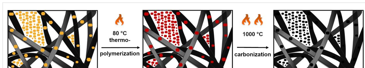
**Figure 1:** Schematic illustration of the synthesis route using the soft-templating approach to obtain porous carbon–carbon composite electrodes. The colours represent the changes of the appearance of the materials during the synthesis.
