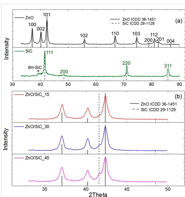
**Figure 3:** X-ray diffraction patterns of (a) ZnO nanofibers and nanocrystalline SiC and (b) ZnO/SiC nanocomposites. The vertical solid and dotted lines correspond to ICDD 36-1451 (ZnO, wurtzite) and ICDD 29-1129 (SiC-3C polytype) references, respectively.
