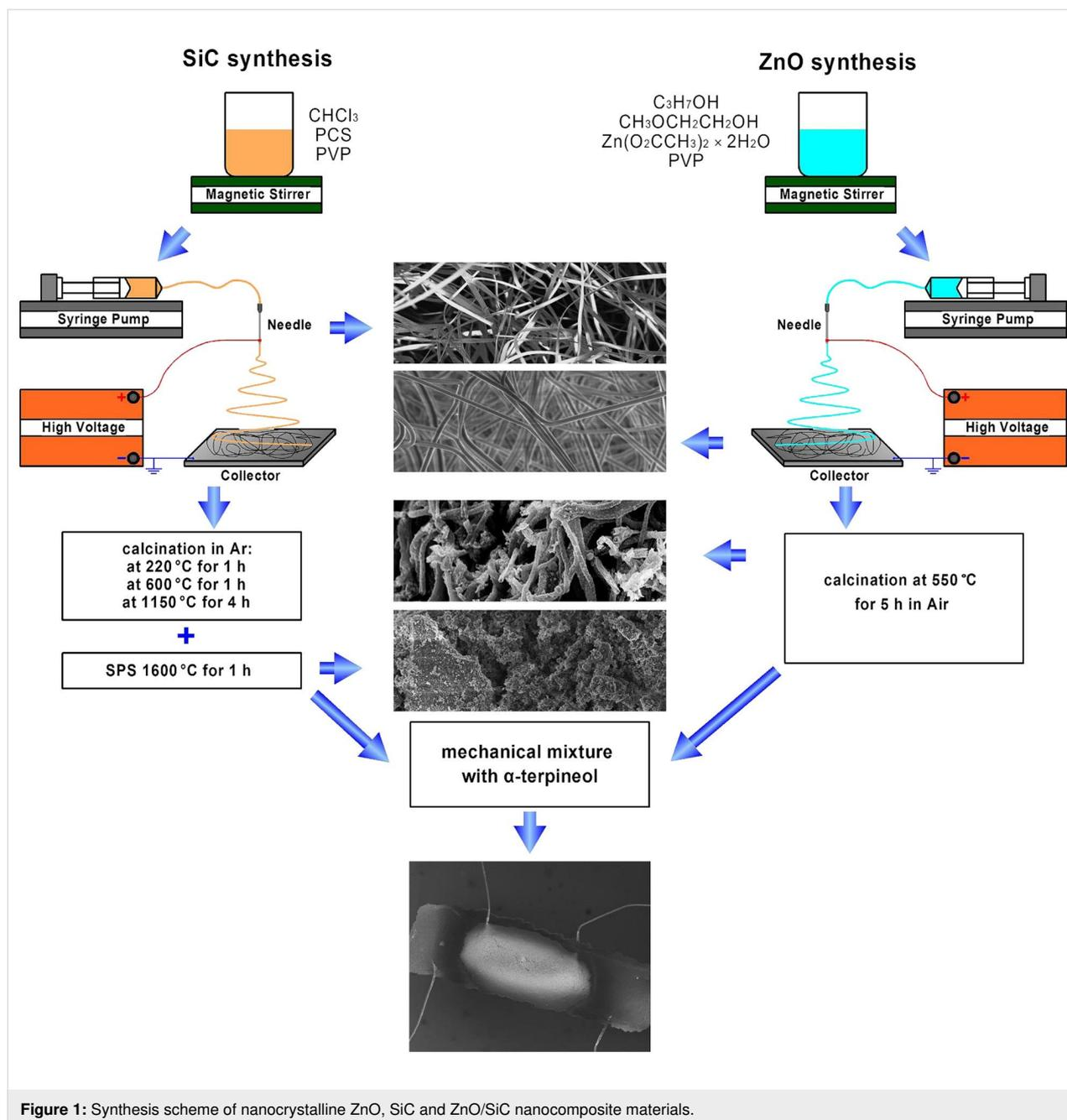
**Figure 1:** Synthesis scheme of nanocrystalline ZnO, SiC and ZnO/SiC nanocomposite materials.
