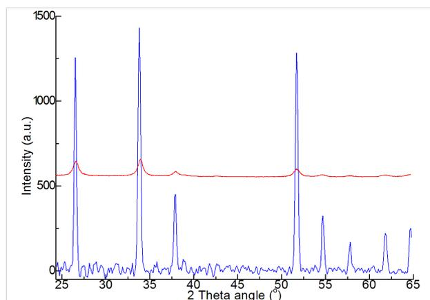
**Figure 4:** Experimental diffractograms of SnO<sub>2</sub> nanowire (blue) and SnO<sub>2</sub> nanopowder (red).
