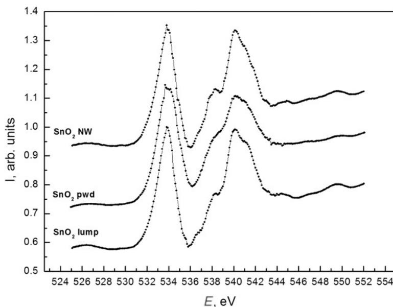
**Figure 8:** XANES O K spectra of SnO<sub>2</sub> wire-like crystals (top) [37,38], SnO<sub>2</sub> powder (middle) and sintered SnO<sub>2</sub> lump reference sample (bottom).
