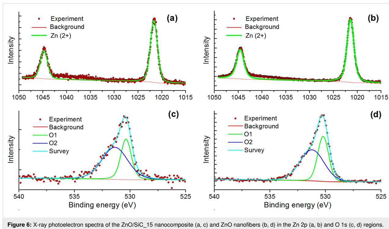
**Figure 6:** X-ray photoelectron spectra of the ZnO/SiC<sub>15</sub> nanocomposite (a, c) and ZnO nanofibers (b, d) in the Zn 2p (a, b) and O 1s (c, d) regions.
