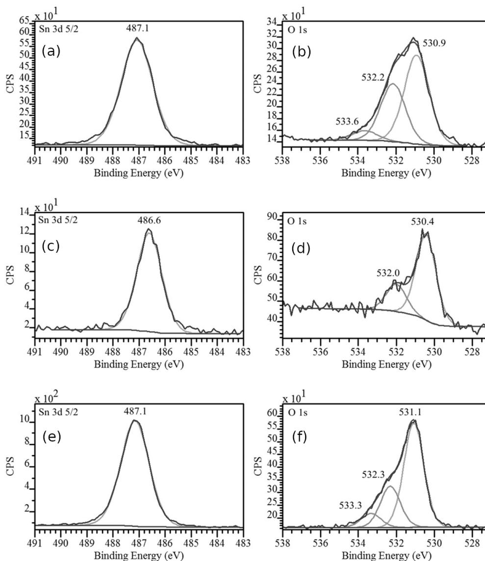
**Figure 6:** XPS spectra of (a) SnO<sub>2</sub> powder, Sn 3d<sub>5/2</sub>; (b) SnO<sub>2</sub> powder, O 1s; (c) SnO<sub>2</sub> nanowires, Sn 3d<sub>5/2</sub>; (d) SnO<sub>2</sub> nanowires, O 1s; (e) SnO<sub>2</sub> sintered lump, Sn 3d<sub>5/2</sub>; (f) SnO<sub>2</sub> sintered lump, O 1s.
