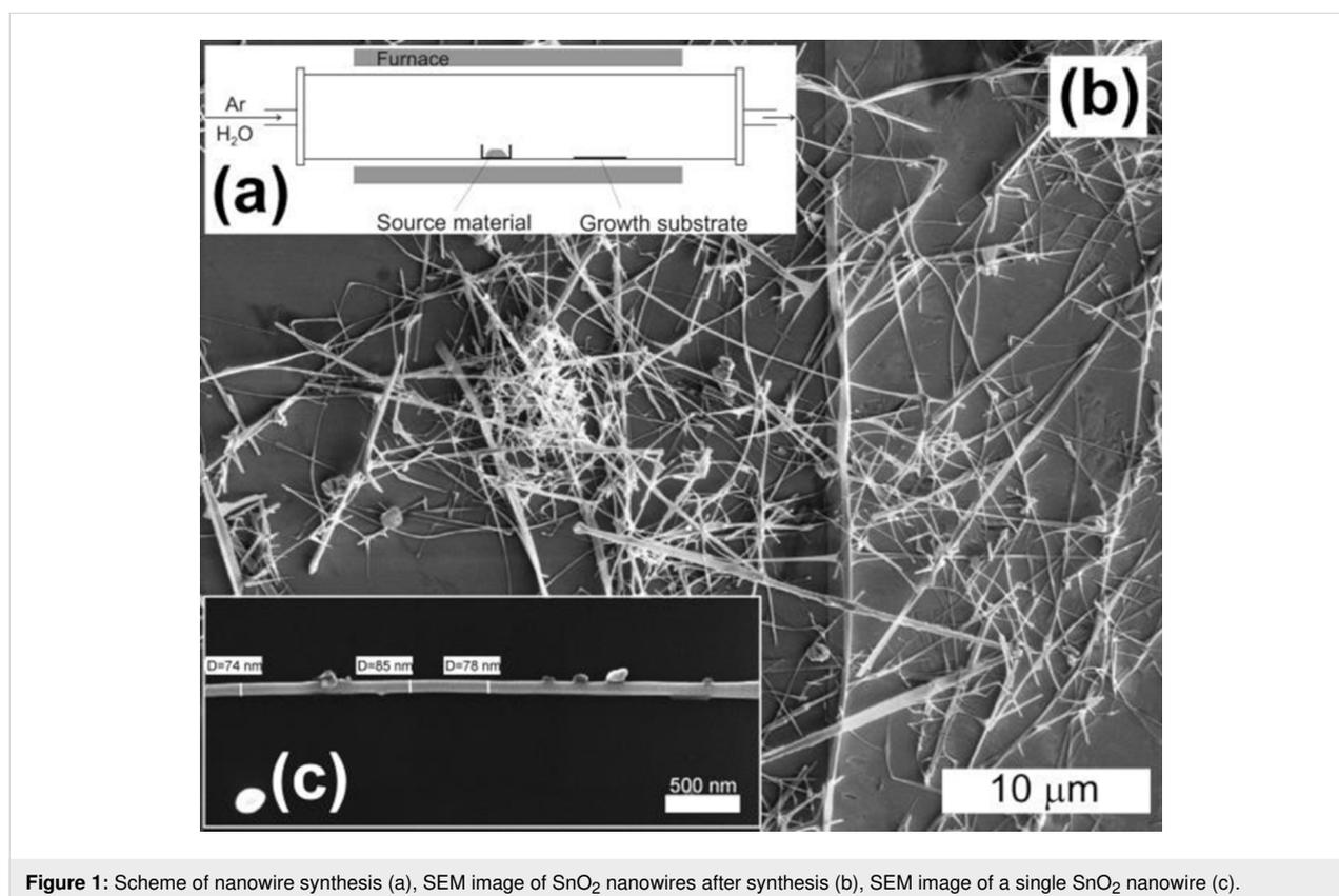
**Figure 1:** Scheme of nanowire synthesis (a), SEM image of  $\text{SnO}_2$  nanowires after synthesis (b), SEM image of a single  $\text{SnO}_2$  nanowire (c).
