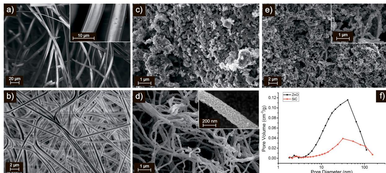
**Figure 2:** SEM micrographs of polymer nanofibers containing polycarbosilane (a) and zinc acetate (b). SEM micrographs of annealed SiC (c) and ZnO (d). (e) SEM micrograph of ZnO/SiC<sub>45</sub> nanocomposite. (f) Pore size distribution of annealed ZnO and SiC.
