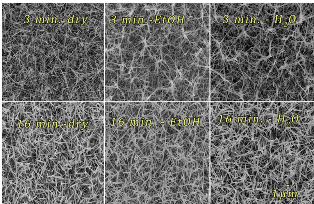
**Figure 4:** SEM images of dry samples in comparison with the one after immersion in EtOH and water for two different sputtering times of 3 and 16 min.
