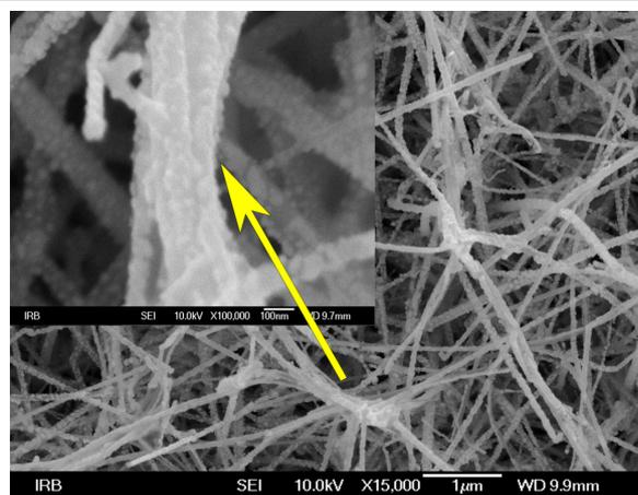
**Figure 5:** SEM images of SiNWs obtained through VLS deposition at 500 °C, then sputtered Ag for 3 min and finally immersed in H<sub>2</sub>O.
