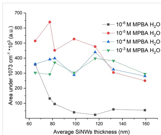
**Figure 6:** Average SERS values of 4-MPBA for different SiNW thicknesses after  $\text{H}_2\text{O}$  immersion.
