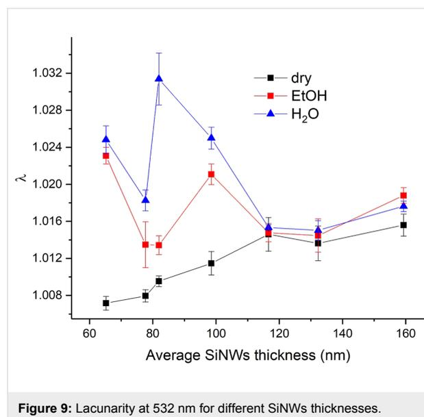
**Figure 9:** Lacunarity at 532 nm for different SiNWs thicknesses.
