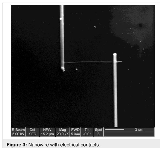
**Figure 3:** Nanowire with electrical contacts.
