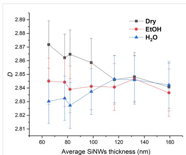
**Figure 8:** Fractal dimension ( $D$ ) of Ag-plated SiNWs after immersion in EtOH and H<sub>2</sub>O.
