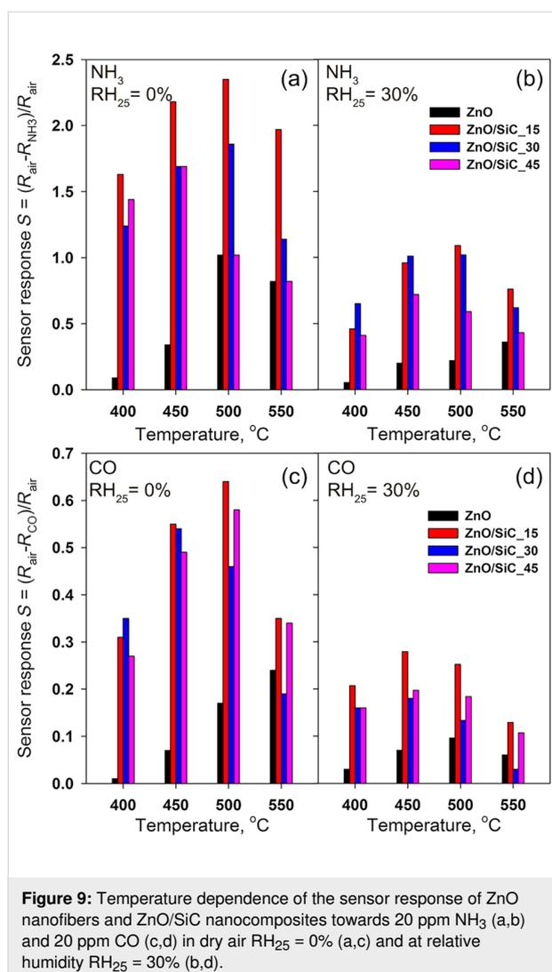
**Figure 9:** Temperature dependence of the sensor response of ZnO nanofibers and ZnO/SiC nanocomposites towards 20 ppm NH<sub>3</sub> (a,b) and 20 ppm CO (c,d) in dry air RH<sub>25</sub> = 0% (a,c) and at relative humidity RH<sub>25</sub> = 30% (b,d).
