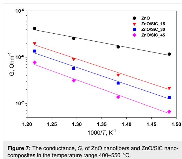
**Figure 7:** The conductance,  $G$ , of ZnO nanofibers and ZnO/SiC nanocomposites in the temperature range 400–550 °C.
