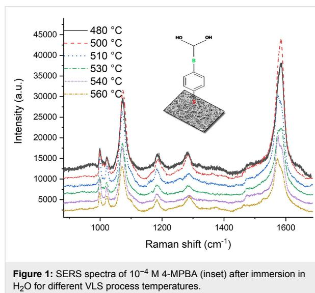
**Figure 1:** SERS spectra of 10<sup>-4</sup> M 4-MPBA (inset) after immersion in H<sub>2</sub>O for different VLS process temperatures.
