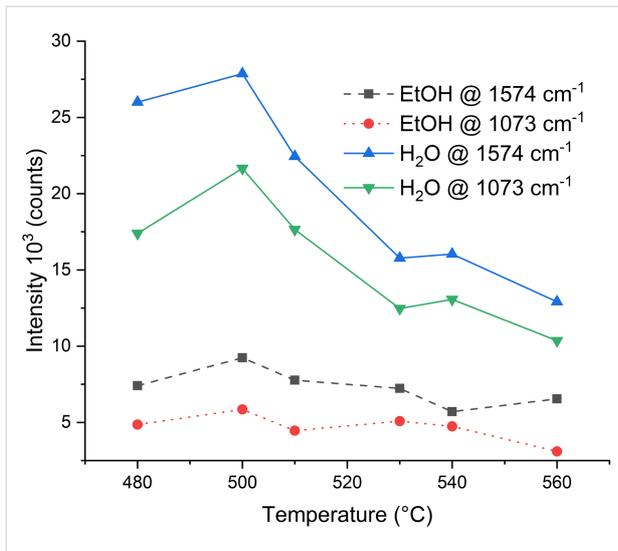
**Figure 2:** SERS intensities of the 1073 and 1574 cm<sup>-1</sup> bands before (denoted EtOH) and after H<sub>2</sub>O washing for different VLS process temperatures.
