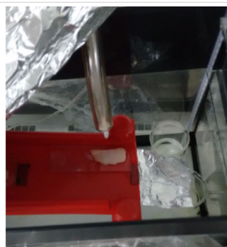
Figure 14: Schematic presentation of the setup utilized for ex vivo liquid falling mucoadhesion tests.
