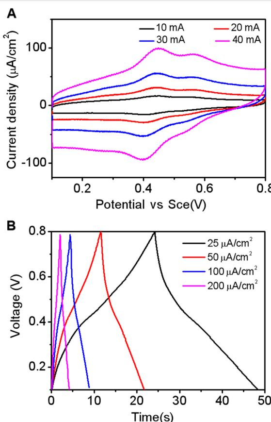
**Figure 4:** Characterization of hydrogels as supercapacitors. (A) Cyclic voltammograms at different scan rates. (B) Galvanostatic charge–discharge curves of C-WY hydrogels at different current densities.
