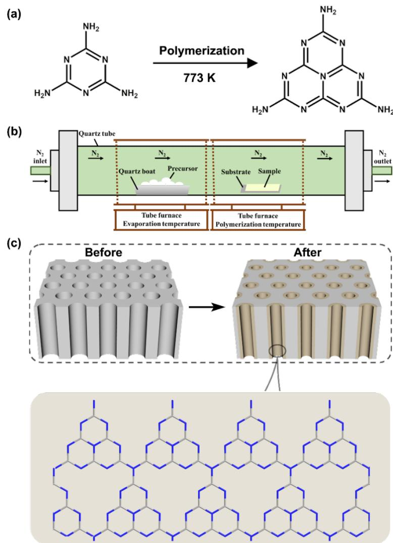
**Figure 1:** Fabrication process of carbon nitride nanotubes. (a) Synthetic route of polymeric carbon nitride nanotubes. (b) Schematic illustration of the fabrication process by vapor deposition–polymerization. (c) Schematic diagram of AAO substrate, carbon nitride nanotubes and molecular structure of the carbon nitride nanotubes.
