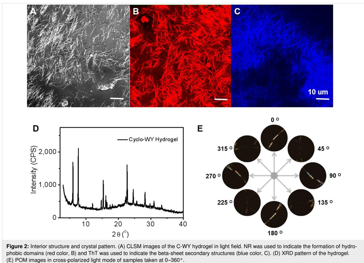
**Figure 2:** Interior structure and crystal pattern. (A) CLSM images of the C-WY hydrogel in light field. NR was used to indicate the formation of hydrophobic domains (red color, B) and ThT was used to indicate the beta-sheet secondary structures (blue color, C). (D) XRD pattern of the hydrogel. (E) POM images in cross-polarized light mode of samples taken at 0–360°.
