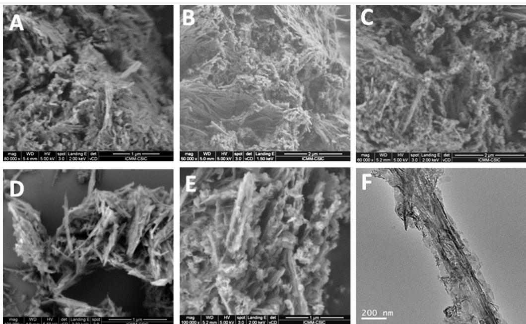
**Figure 6:** FE-SEM images of (A) MCPA-LDH/Sep2:1\_150C, (B) MCPA-LDH/Sep1:1\_150C, (C) MCPA-LDH/Sep0.5:1\_60C, (D) LDH/Sep0.5:1\_150C, and (E) MCPA-LDH/Sep0.5:1\_150C hybrid nanoarchitectures prepared by coprecipitation from different LDH/sepiolite ratios; (F) TEM image of the MCPA-LDH/Sep0.5:1\_60C hybrid nanoarchitecture.
