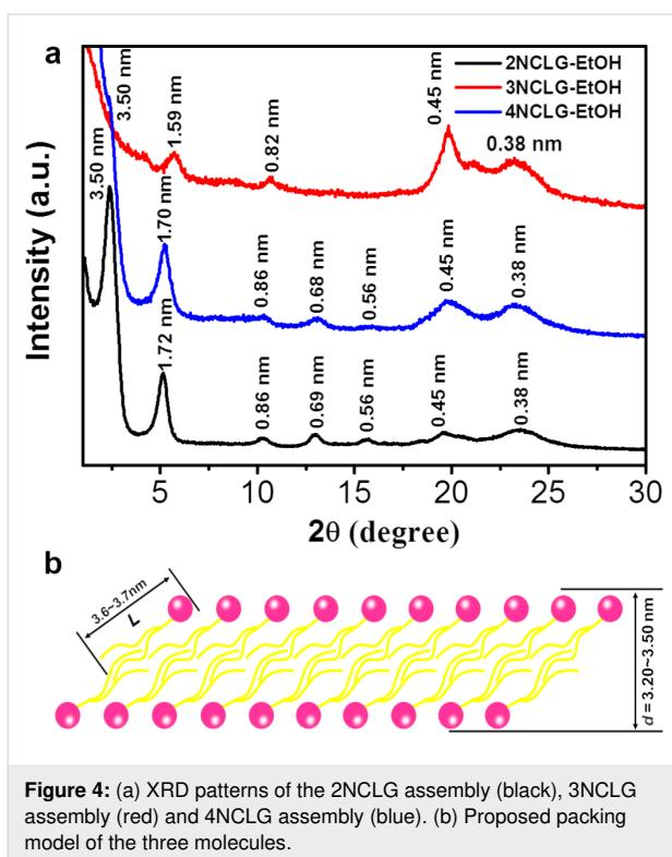
**Figure 4:** (a) XRD patterns of the 2NCLG assembly (black), 3NCLG assembly (red) and 4NCLG assembly (blue). (b) Proposed packing model of the three molecules.
