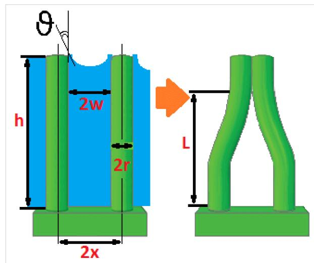
**Figure 1:** Schematic illustration of elastocapillary self-assembly of NWs induced by the surface tension between the residual fluid film and the NWs.
