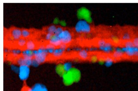
**Figure 4:**  $\text{ZnO}-\text{Fe}_3\text{O}_4$ @sepiolite nanoarchitecture prepared in two steps: First, the fiber clay is modified by assembly of magnetite NPs. After that, the  $\text{ZnO}$  NPs are added yielding a magnetic photocatalyst. The STEM images on the right shows the silicate component (red), the magnetite NPs (green) and the  $\text{ZnO}$  NPs (blue) analyzed with an EDAX detector and a Gatan Tridiem energy filter; reprinted with permission from [133], copyright 2017 Elsevier.
