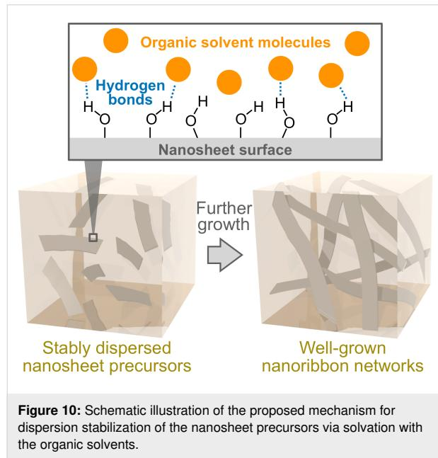
**Figure 10:** Schematic illustration of the proposed mechanism for dispersion stabilization of the nanosheet precursors via solvation with the organic solvents.
