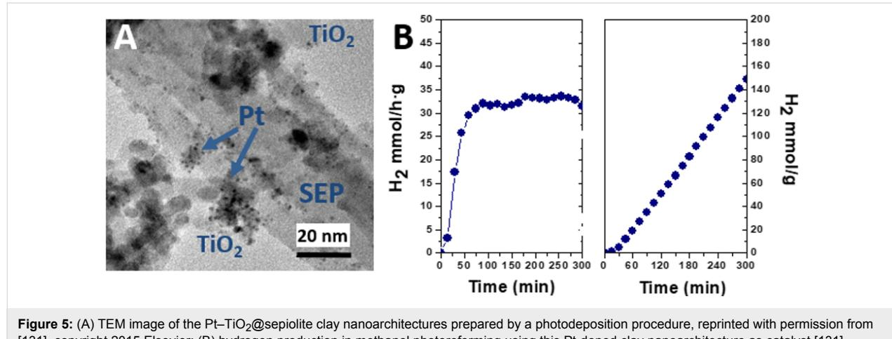
**Figure 5:** (A) TEM image of the  $\text{Pt-TiO}_2$ @sepiolite clay nanoarchitectures prepared by a photodeposition procedure, reprinted with permission from [131], copyright 2015 Elsevier; (B) hydrogen production in methanol photoreforming using this  $\text{Pt}$ -doped clay nanoarchitecture as catalyst [131].
