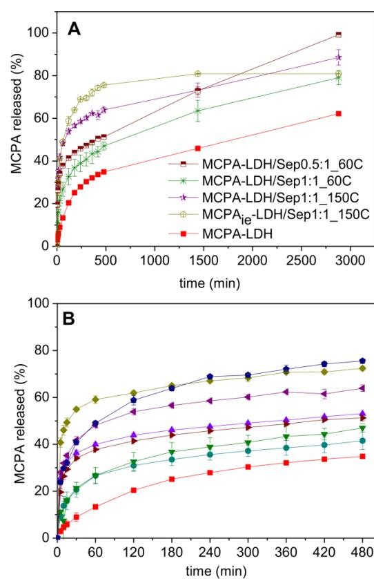
**Figure 7:** (A) In vitro release of MCPA from the hybrid formulations in deionized water (pH approx. 5.5), and (B) zoom of the same graph showing the release behavior in the first 500 min of the study.
