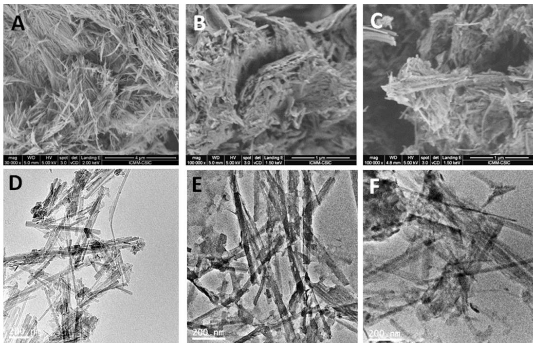
**Figure 3:** FE-SEM images of (A) sepiolite, (B) LDH/Sep1:1\_150C and (C) MCPA<sub>ie</sub>-LDH/Sep1:1\_150C nanoarchitectures; TEM images of (D) LDH/Sep0.5:1\_150C, and the LDH/Sep1:1\_150C nanoarchitecture (E) before and (F) after the ion exchange treatment with MCPA.
