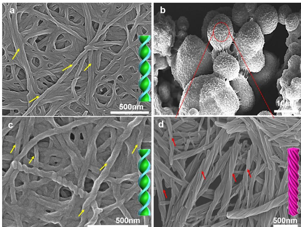
**Figure 2:** SEM images of NCLG assemblies in EtOH: (a) 2NCLG, (b,d) 3NCLG, and (c) 4NCLG self-assembled structures. The concentration is 12 mg/mL.
