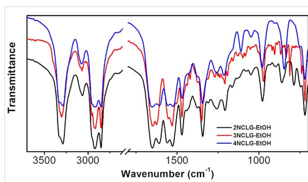
**Figure 5:** FTIR spectra of the 2NCLG assembly (black), 3NCLG assembly (red) and 4NCLG assembly (blue) obtained in EtOH.
