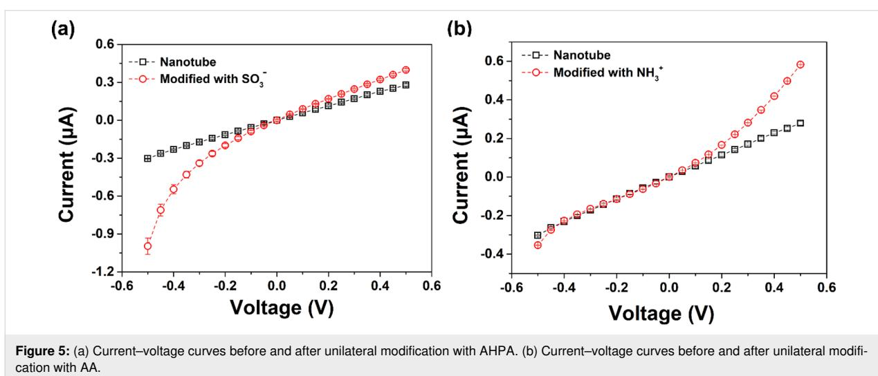
**Figure 5:** (a) Current–voltage curves before and after unilateral modification with AHPA. (b) Current–voltage curves before and after unilateral modification with AA.
