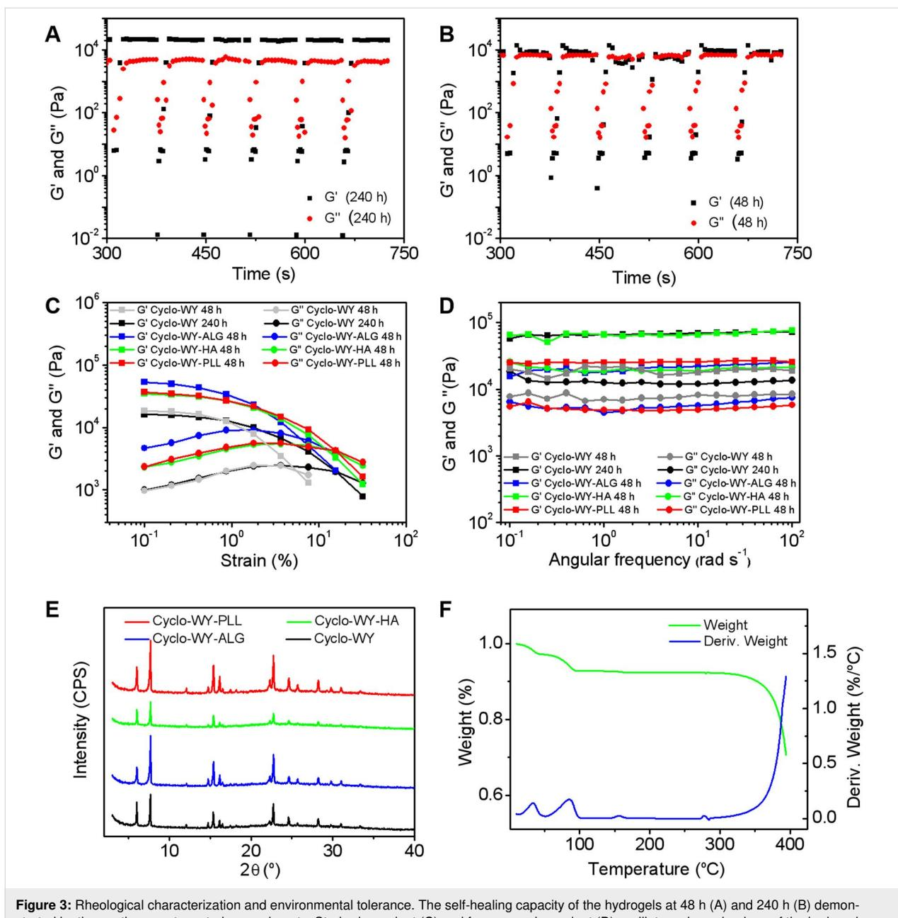
**Figure 3:** Rheological characterization and environmental tolerance. The self-healing capacity of the hydrogels at 48 h (A) and 240 h (B) demonstrated by the continuous step-strain experiments. Strain-dependent (C) and frequency-dependent (D) oscillatory shear rheology of the hydrogels under various conditions. (E) XRD patterns of hydrogels with various polymers. (F) TG curves of the C-WY hydrogel.
