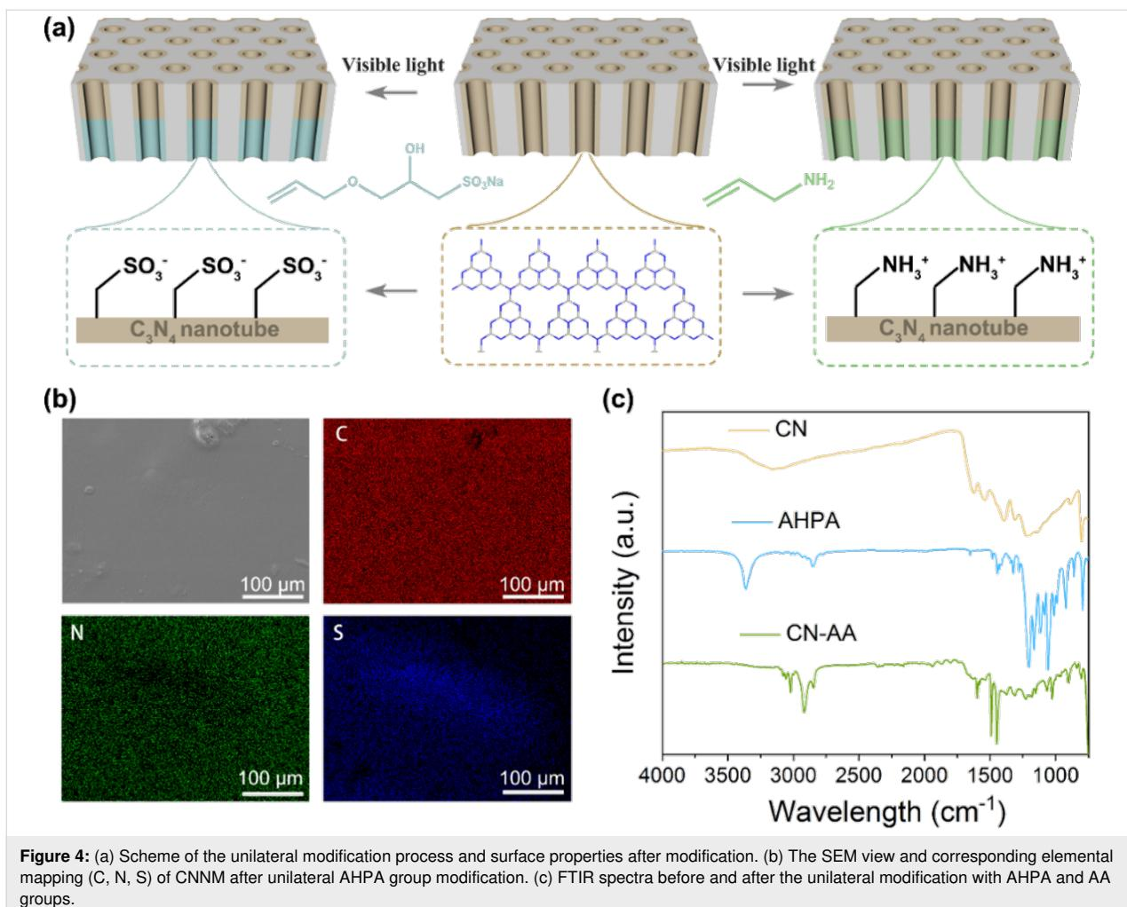
**Figure 4:** (a) Scheme of the unilateral modification process and surface properties after modification. (b) The SEM view and corresponding elemental mapping (C, N, S) of CNNM after unilateral AHPA group modification. (c) FTIR spectra before and after the unilateral modification with AHPA and AA groups.
