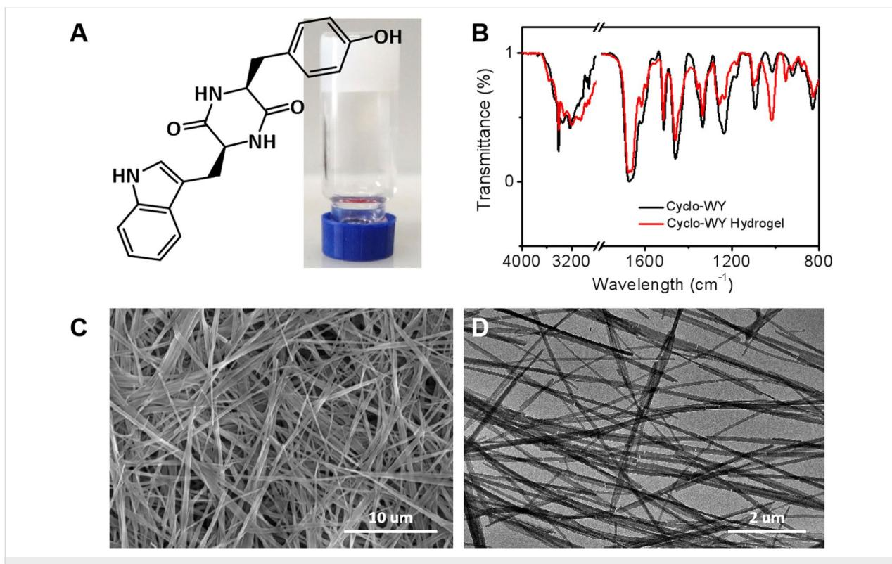
**Figure 1:** CDP-based supramolecular hydrogels. (A) The structure of C-WY and a photo of the C-WY hydrogel. (B) FTIR spectra of C-WY powder and the C-WY hydrogel. (C) SEM and (D) TEM images of the C-WY hydrogel.
