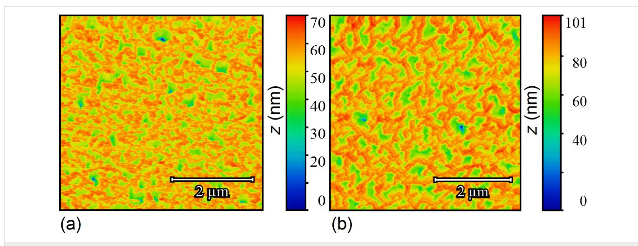
**Figure 2:** Representative AFM images of sample SiNW1 (a) and sample SiNW2 (b). The probed areas have a size of  $5 \times 5 \mu\text{m}^2$ . The AFM measurements have been performed by using a NT-MDT Solver Pro 4H microscope, using tapping mode in ambient atmosphere and at room temperature.
