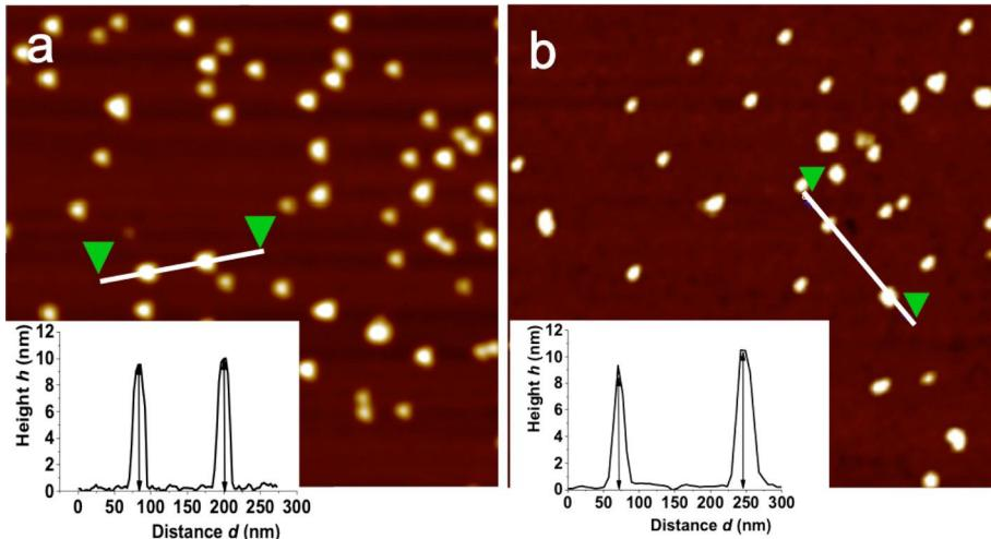
**Figure 9:** AFM topography images ( $1 \times 1 \mu\text{m}$ ) and height profiles of a) IONP@C<sub>2</sub>F<sub>5</sub>OEG<sub>8</sub>Den and b) IONP@C<sub>2</sub>H<sub>5</sub>OEG<sub>8</sub>Den. Dispersions of IONPs in ethanol ( $0.002 \text{ mg mL}^{-1}$ ) were spin-coated on silicon wafers.
