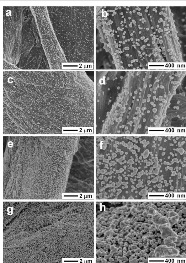
**Figure 1:** FE-SEM micrographs of the paper-based SERS substrates Ag-NP/cellulose-NF-A (a,b), B (c,d), C (e,f), and D (g,h), which were fabricated with reaction times of 2, 4, 6, and 8 min, respectively.
