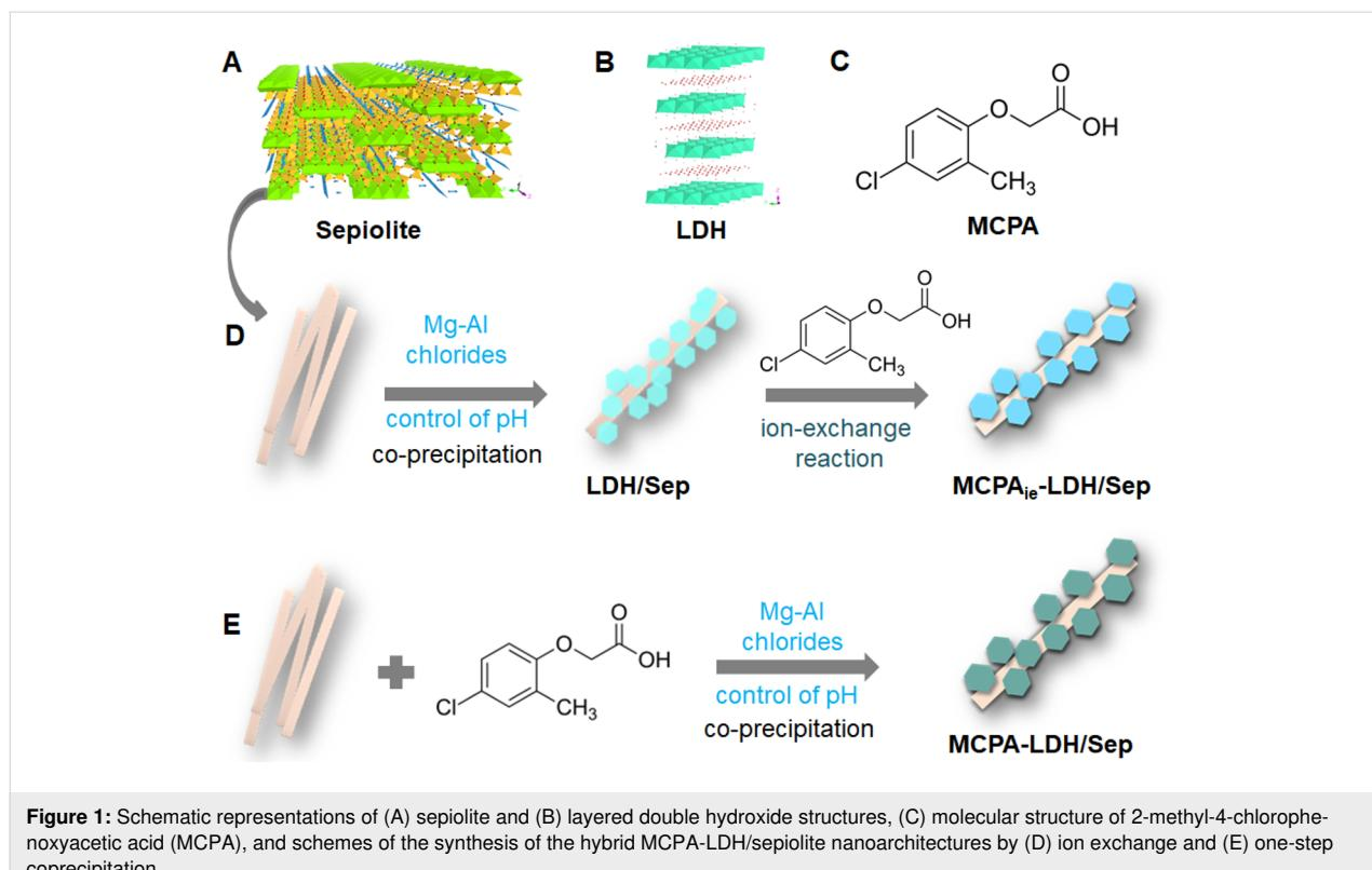
**Figure 1:** Schematic representations of (A) sepiolite and (B) layered double hydroxide structures, (C) molecular structure of 2-methyl-4-chlorophenoxyacetic acid (MCPA), and schemes of the synthesis of the hybrid MCPA-LDH/sepiolite nanoarchitectures by (D) ion exchange and (E) one-step coprecipitation.
