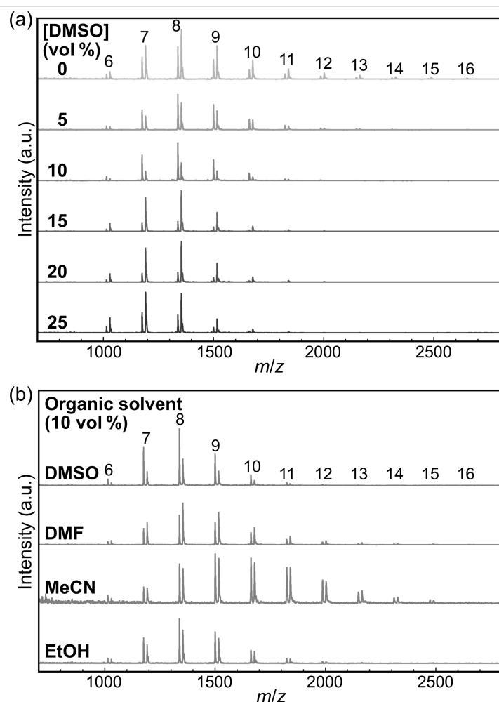
**Figure 6:** MALDI-TOF mass spectra of the products with (a) DMSO at various concentrations and (b) various organic solvents at 10 vol %. The numbers above the peaks denote the DP values of the cellulose oligomers. The spectra show two series of peaks corresponding to cellulose oligomers with sodium and potassium ion adducts.
