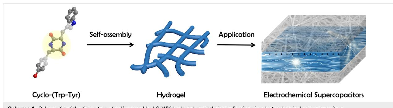
**Scheme 1:** Schematic of the formation of self-assembled C-WY hydrogels and their applications in electrochemical supercapacitors.
