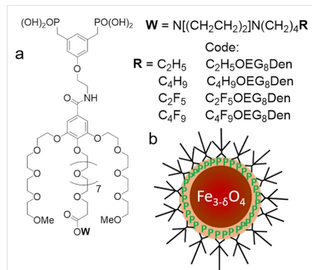
**Figure 1:** a) Molecular structure of the dendrons investigated ( $C_nX_{2n+1}OEG_8Den$ ,  $X = F$  or  $H$ ;  $n = 2$  and 4); b) Schematic representation of a dendronized IONP showing the anchoring of the bisphosphonate function on the iron oxide.
