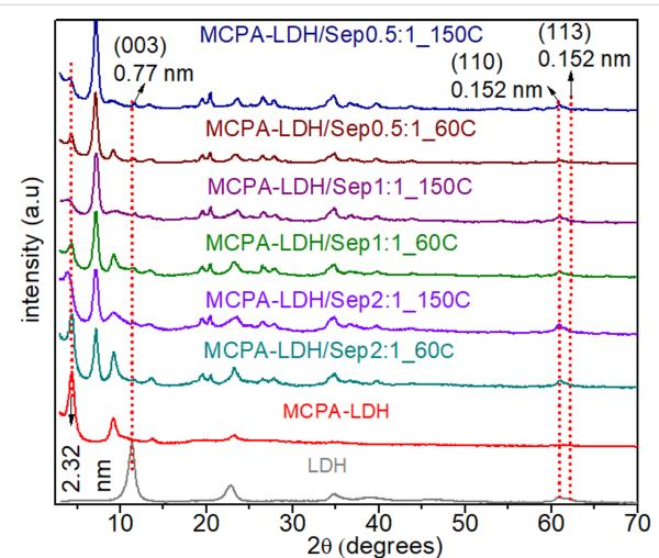
**Figure 4:** XRD patterns of hybrid nanoarchitectures prepared by coprecipitation of MgAl-LDH in the presence of sepiolite and MCPA at different theoretical LDH/sepiolite ratios (x:1).
