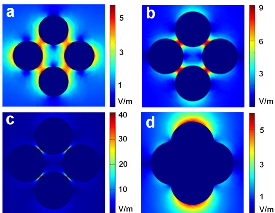
**Figure 5:** Electric field intensity distributions (indicated by the color bar) of the silver nanoparticles (diameter 70 nm) with different inter-particle spacings of 15 nm (a), 5 nm (b), 1 nm (c), and aggregated particles (d) at an excitation wavelength of 514 nm.
