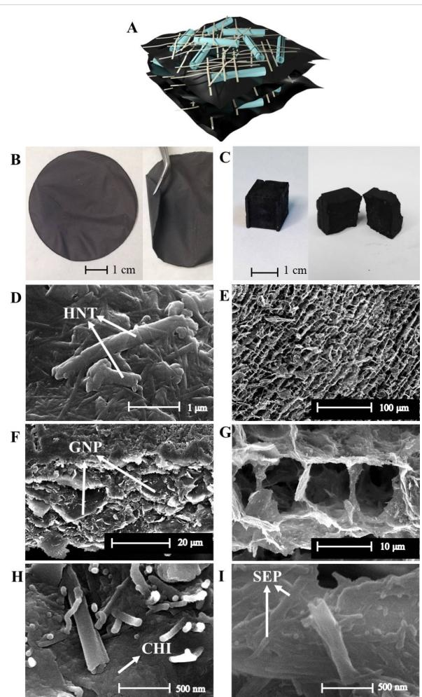
**Figure 3:** Schematic representation of particle assembly in the multicomponent bionanocomposites: A) cross section of processed materials: HNTs and SEP are represented as tubes and fibres, while chitosan, GNPs and MWCNTs are depicted in the black matrix. Photographs of B) Film-1 and C) Foam-1. SEM micrographs of the film: D) upper surface, F) and H) cross section; SEM micrographs of the foam: E) and G) pore architecture, I) cell walls.
