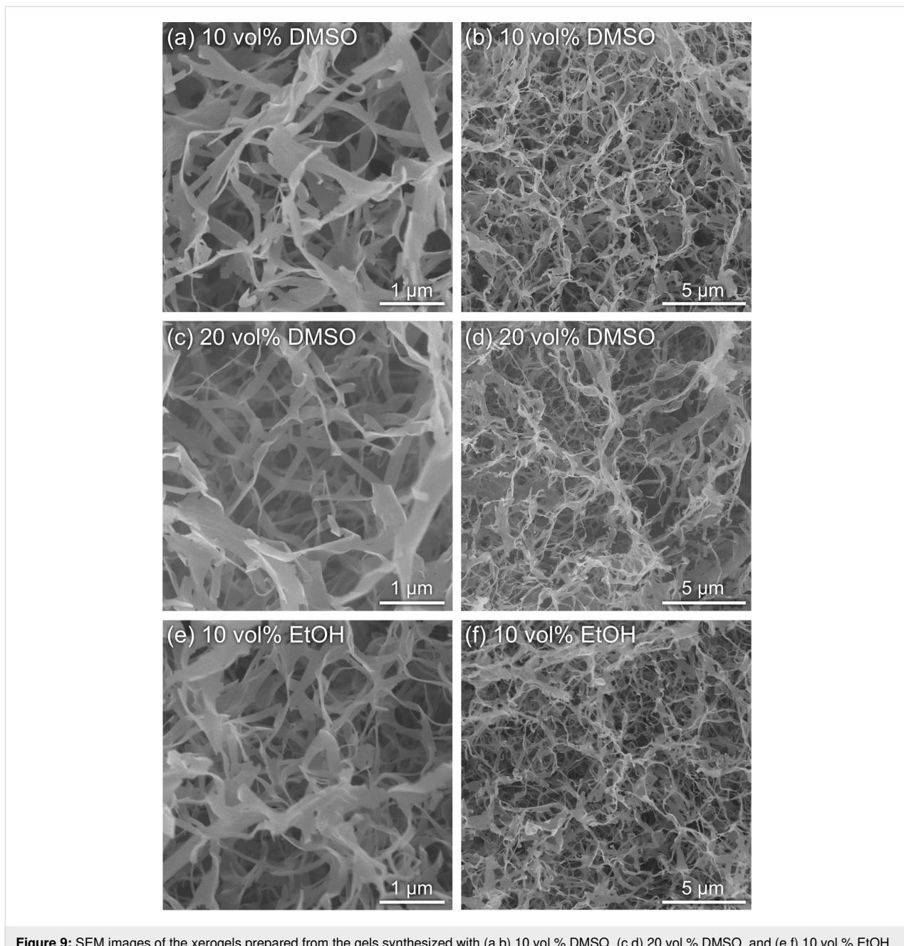
**Figure 9:** SEM images of the xerogels prepared from the gels synthesized with (a,b) 10 vol % DMSO, (c,d) 20 vol % DMSO, and (e,f) 10 vol % EtOH.
