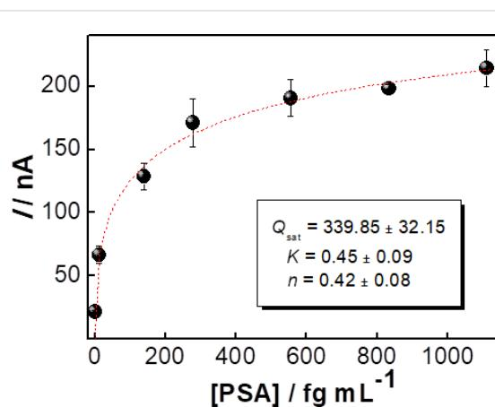
**Figure 2:** Peak current as a function of the PSA concentration fitted with a Langmuir–Freundlich equation (dashed line).
