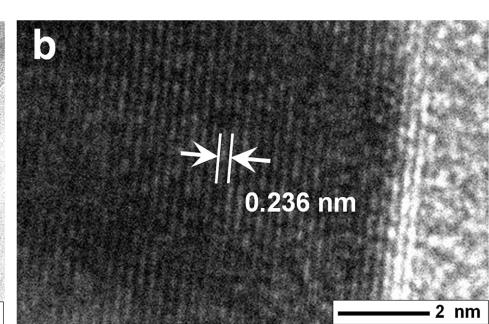
**Figure 2:** TEM image of Ag-NP/cellulose-NF-C (a), and HR-TEM image of an individual silver nanoparticle showing the lattice of metallic silver (b).
