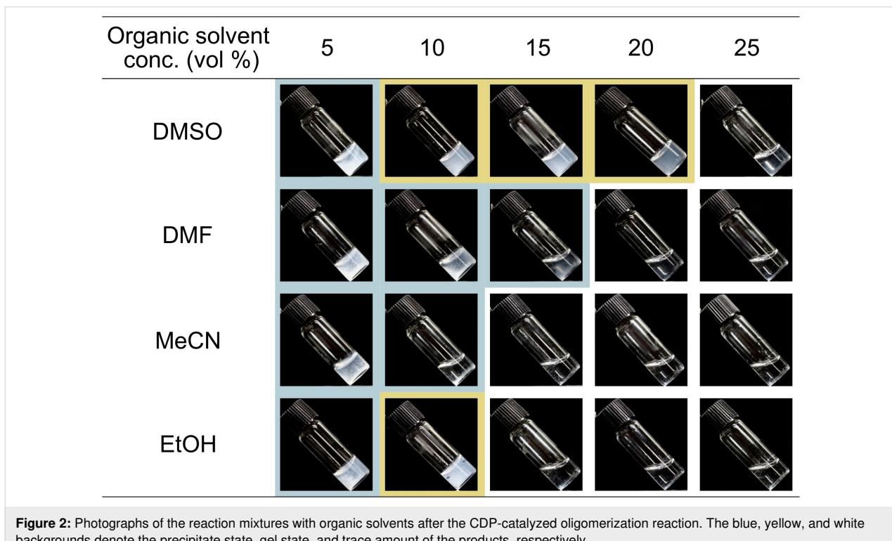
**Figure 2:** Photographs of the reaction mixtures with organic solvents after the CDP-catalyzed oligomerization reaction. The blue, yellow, and white backgrounds denote the precipitate state, gel state, and trace amount of the products, respectively.
