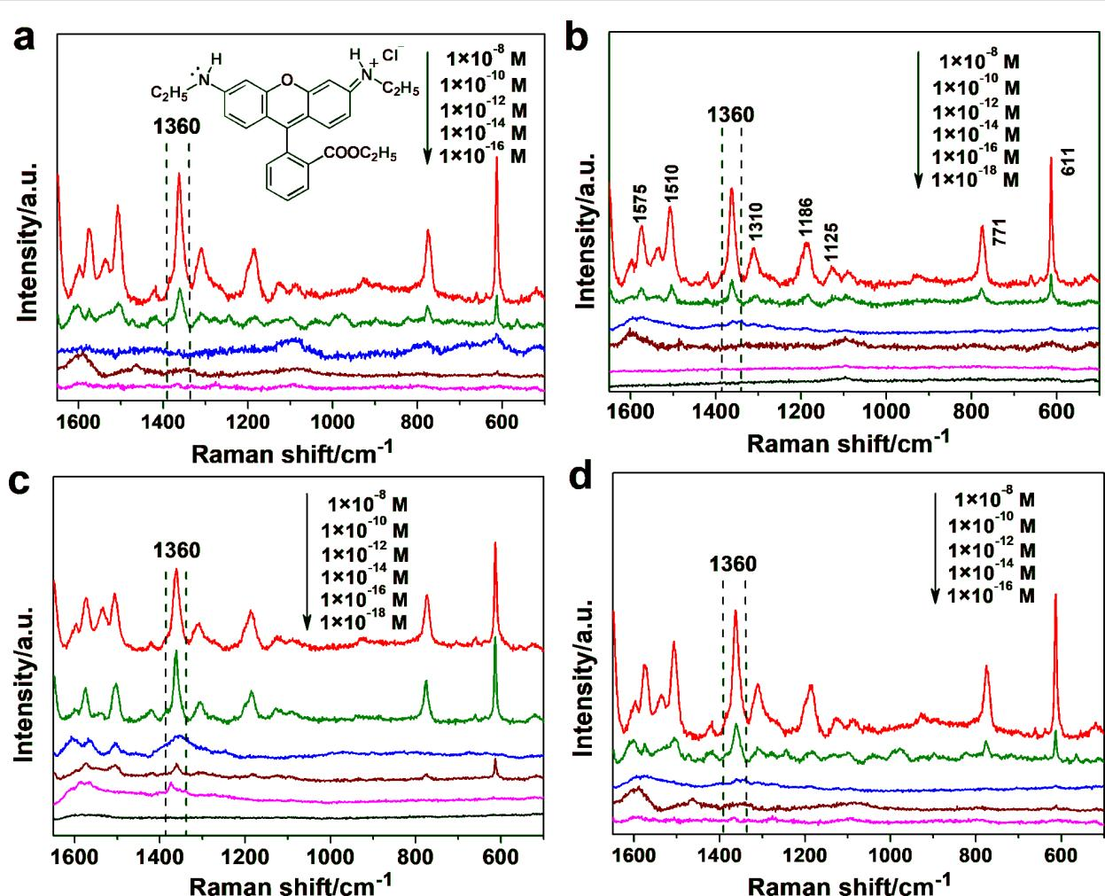
**Figure 4:** SERS spectra of Rhodamine 6G (R6G) at different concentrations obtained by employing Ag-NP/cellulose-NF-A (a), -B (b), -C (c), and -D (d) composite sheets as the substrates. The characteristic band at  $1360\text{ cm}^{-1}$  was used as the reference, and the SERS measurements were acquired from four randomly selected locations on each of the samples. The inset of (a) is the molecular structure of R6G.
