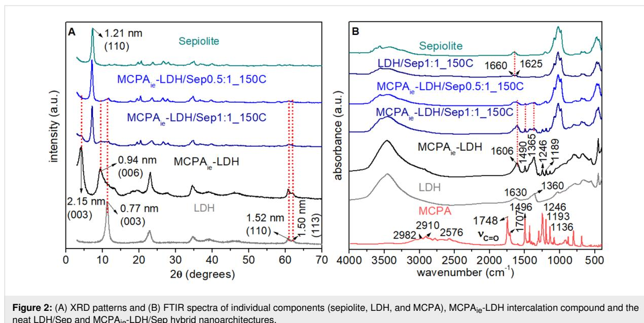
**Figure 2:** (A) XRD patterns and (B) FTIR spectra of individual components (sepiolite, LDH, and MCPA), MCPA<sub>ie</sub>-LDH intercalation compound and the neat LDH/Sep and MCPA<sub>ie</sub>-LDH/Sep hybrid nanoarchitectures.
