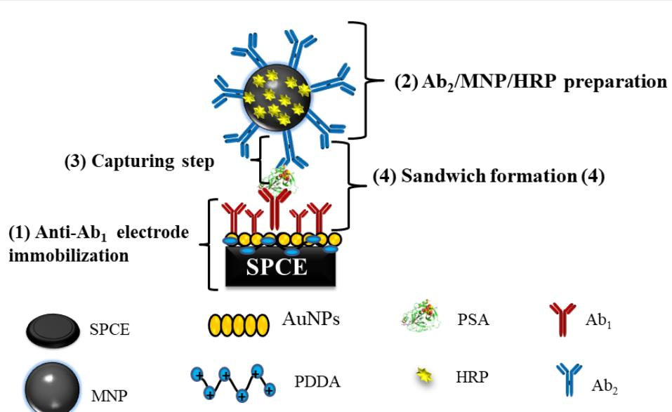
**Figure 6:** Schematic illustration of the fabrication of sandwich-type electrochemical immunosensors (INu-SPCEs).
