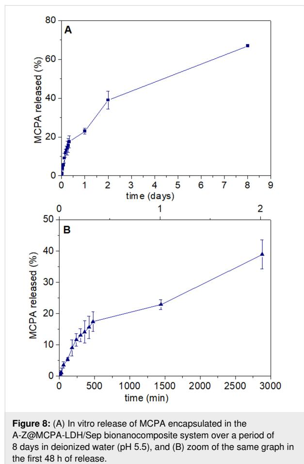
**Figure 8:** (A) In vitro release of MCPA encapsulated in the A-Z@MCPA-LDH/Sep bionanocomposite system over a period of 8 days in deionized water (pH 5.5), and (B) zoom of the same graph in the first 48 h of release.
