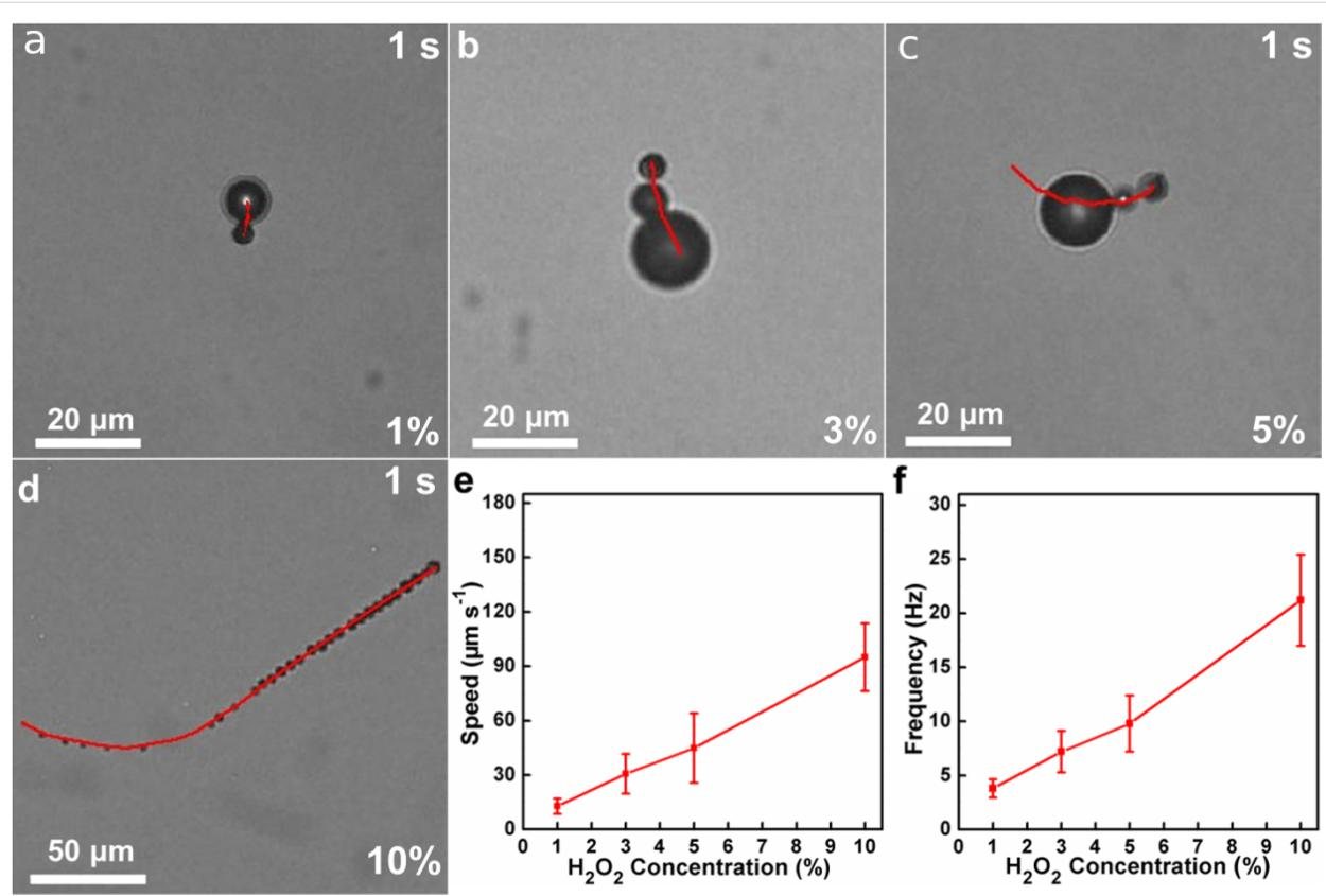
**Figure 2:** Images of the Janus UCNPs capsule motors for different H<sub>2</sub>O<sub>2</sub> concentrations: (a) 1%, (b) 3%, (c) 5% and (d) 10% after a period of 1 s. (e) Effect of the H<sub>2</sub>O<sub>2</sub> concentration on the average speed of the Janus UCNPs capsule motors. (f) Relationship of the oxygen bubble expulsion frequency of Janus UCNPs capsule motors with different H<sub>2</sub>O<sub>2</sub> concentration.
