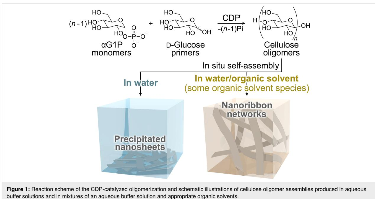
**Figure 1:** Reaction scheme of the CDP-catalyzed oligomerization and schematic illustrations of cellulose oligomer assemblies produced in aqueous buffer solutions and in mixtures of an aqueous buffer solution and appropriate organic solvents.
