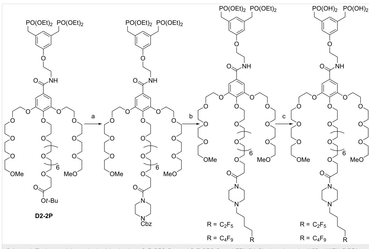
**Scheme 1:** Final steps of the synthesis of the dendrons  $C_2F_5OEG_6Den$  and  $C_4F_9OEG_6Den$ . a) TFA/CH<sub>2</sub>Cl<sub>2</sub>, then piperazine-NCBz, HATU, DIPEA/DMF; 99% (2 steps); b) H<sub>2</sub>, Pd/C/ MeOH, then perfluoroalkyl iodide, K<sub>2</sub>CO<sub>3</sub>/CH<sub>3</sub>CN; 80% for  $C_2F_5$  and 55% for  $C_4F_9$ ; c) TMSBr/CH<sub>2</sub>Cl<sub>2</sub>; 79% for  $C_2F_5$  and 80% for  $C_4F_9$ .
