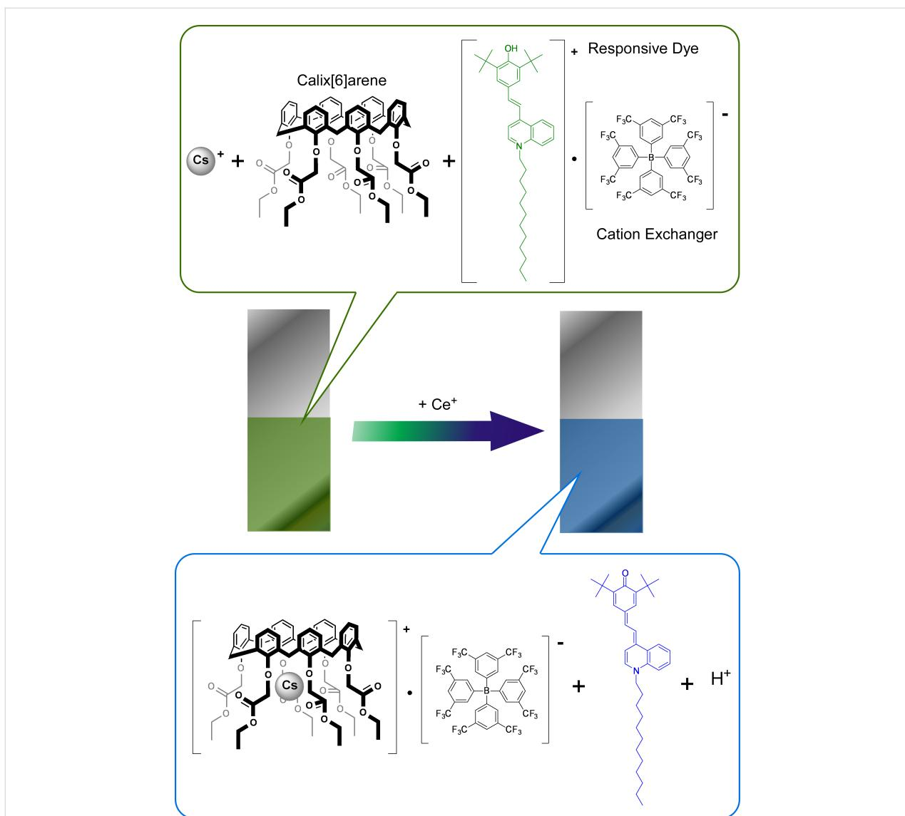
**Figure 4:** An optode sensor to visually detect cesium ions in domestic water and seawater, comprised of a calix[6]arene derivative, responsive dye KD-M1337, and cation exchanger.
