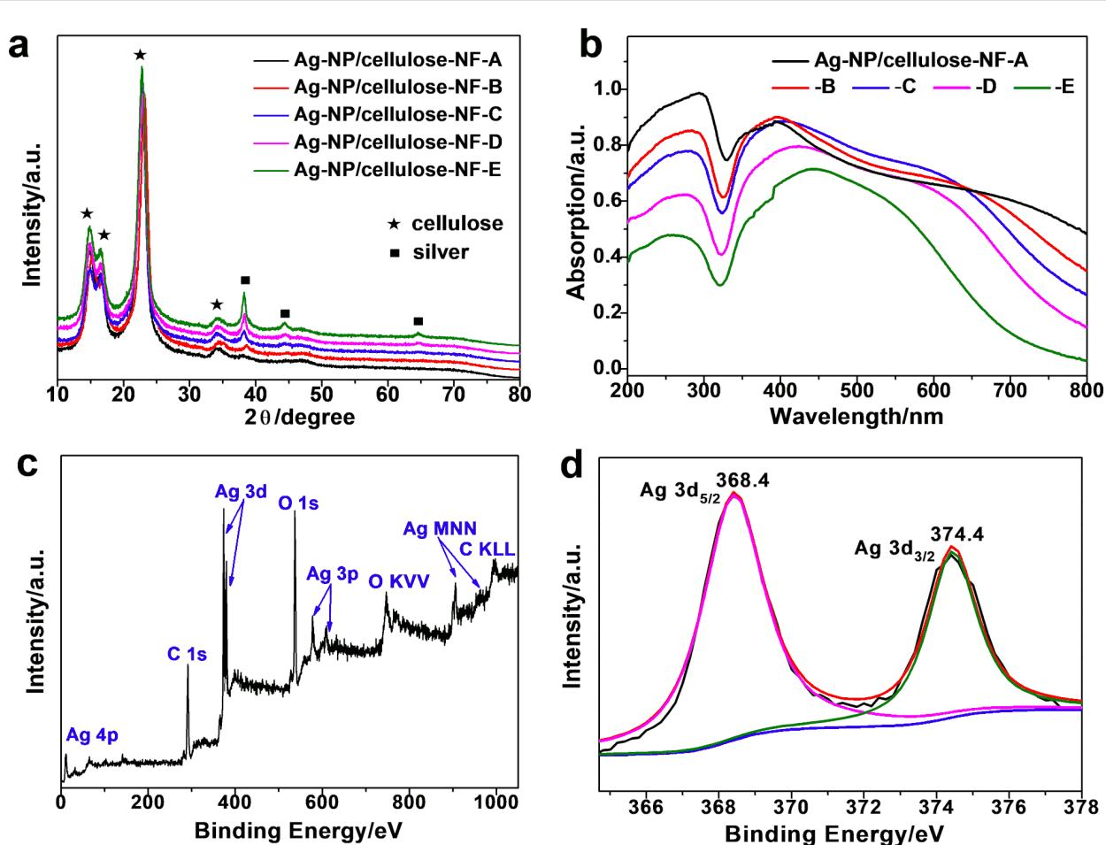
**Figure 3:** X-ray diffraction patterns (a) and diffuse reflectance UV-vis spectra (b) of Ag-NP/cellulose-NF-A, B, C, D, and E. X-ray photoelectron spectroscopy (XPS) survey spectrum (c) and high-resolution XPS spectrum of the Ag 3d region (d) of sample Ag-NP/cellulose-NF-C.
