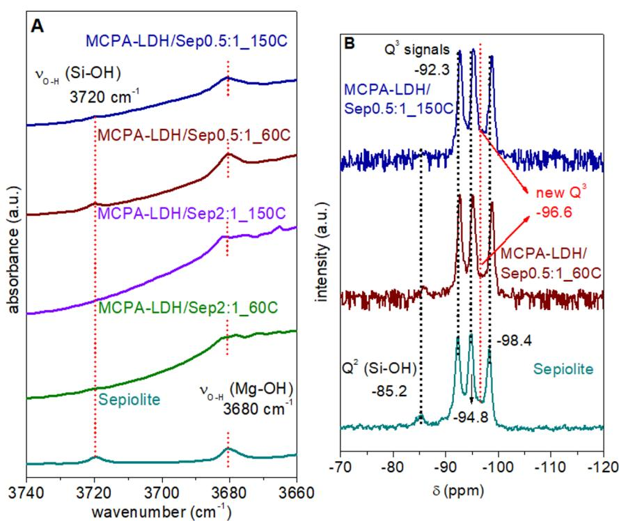
**Figure 5:** (A) FTIR (3800 to 3600  $\text{cm}^{-1}$  region) and (B)  $^{29}\text{Si}$  MAS NMR spectra of neat sepiolite and hybrid nanoarchitectures prepared by coprecipitation of the MgAl-LDH in the presence of sepiolite and MCPA at different theoretical LDH/sepiolite ratios (x:1).
