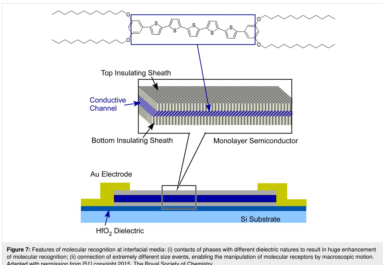
**Figure 7:** Features of molecular recognition at interfacial media: (i) contacts of phases with different dielectric natures to result in huge enhancement of molecular recognition; (ii) connection of extremely different size events, enabling the manipulation of molecular receptors by macroscopic motion. Adapted with permission from [51] copyright 2015, The Royal Society of Chemistry.
