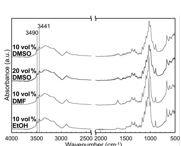
**Figure 8:** ATR-FTIR absorption spectra of the products with organic solvents. The numbers above the peaks denote the wavenumber.
