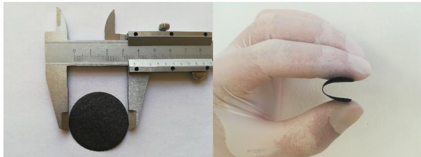
**Figure 1:** Image of the  $\text{MoS}_2$ -based composite paper showing its size and flexibility.
