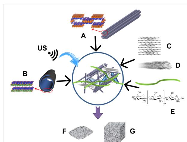
**Figure 1:** Schematic representation of the different components integrated in the bionanocomposite materials, i.e., (A) sepiolite fibrous clay, (B) halloysite nanotubes, (C) graphene nanoplatelets, (D) multiwalled carbon nanotubes, and (E) chitosan biopolymer, prepared in aqueous media under ultrasound irradiation (US). The resulting nanoarchitected materials can be formed into films (F) or foams (G).
