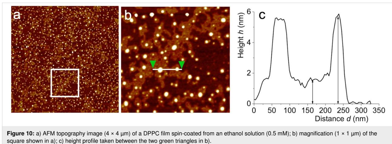
**Figure 10:** a) AFM topography image ( $4 \times 4 \mu\text{m}$ ) of a DPPC film spin-coated from an ethanol solution (0.5 mM); b) magnification ( $1 \times 1 \mu\text{m}$ ) of the square shown in a); c) height profile taken between the two green triangles in b).
