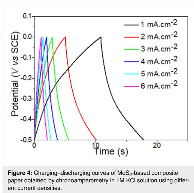
**Figure 4:** Charging–discharging curves of MoS<sub>2</sub>-based composite paper obtained by chronoamperometry in 1M KCl solution using different current densities.
