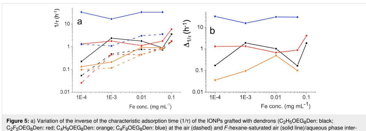
**Figure 5:** a) Variation of the inverse of the characteristic adsorption time ( $1/\tau$ ) of the IONPs grafted with dendrons ( $C_2H_5OEG_8Den$ : black;  $C_2F_5OEG_8Den$ : red;  $C_4H_9OEG_8Den$ : orange;  $C_4F_9OEG_8Den$ : blue) at the air (dashed) and *F*-hexane-saturated air (solid line)/aqueous phase interface. b) Variation of the differences of  $1/\tau$  measured under air and *F*-hexane-saturated air ( $\Delta 1/\tau$ ) as a function of the Fe concentration (same color code).
