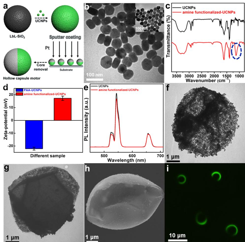
**Figure 1:** (a) Schematic representation of the fabrication process of Janus UCNP-modified polyelectrolyte capsule motors. (b) TEM images, (c) FTIR spectra, (d) zeta potential and (e) fluorescence emission spectrum of UCNPs with different surface functional groups. TEM images of UCNP-modified capsule (f) and Janus UCNP capsule motor (g). (h) SEM image of the Janus UCNP capsule motor. (i) Fluorescence microscope image of the Janus UCNP capsule motors.
