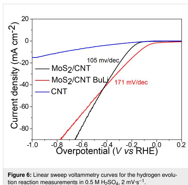
**Figure 6:** Linear sweep voltammetry curves for the hydrogen evolution reaction measurements in 0.5 M  $\text{H}_2\text{SO}_4$ ,  $2 \text{ mV}\cdot\text{s}^{-1}$ .
