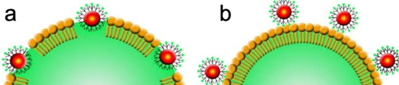
**Figure 8:** Schematic representation of dendronized IONPs a) incorporated within the MB DPPC shell and b) located at the surface of this shell.
