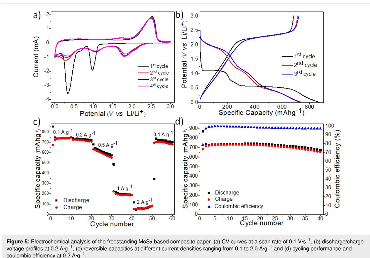
**Figure 5:** Electrochemical analysis of the freestanding MoS<sub>2</sub>-based composite paper. (a) CV curves at a scan rate of  $0.1 \text{ V}\cdot\text{s}^{-1}$ , (b) discharge/charge voltage profiles at  $0.2 \text{ A}\cdot\text{g}^{-1}$ , (c) reversible capacities at different current densities ranging from  $0.1$  to  $2.0 \text{ A}\cdot\text{g}^{-1}$  and (d) cycling performance and coulombic efficiency at  $0.2 \text{ A}\cdot\text{g}^{-1}$ .
