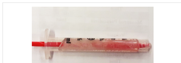
Figure 4: Facile syringe-tube assembly used in fabricating the hydrogel channels.
