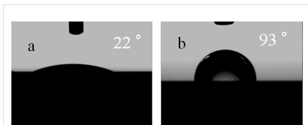
**Figure 9:** Static-contact-angle images of water droplets on a silicon wafer cast with (a) original imogolite and (b) DDPO<sub>4</sub>-imogolite. Reprinted with permission from W. Ma et al., *Chem. Lett.* 2011, 40, 159–161 [33]. © 2011, The Chemical Society of Japan.
