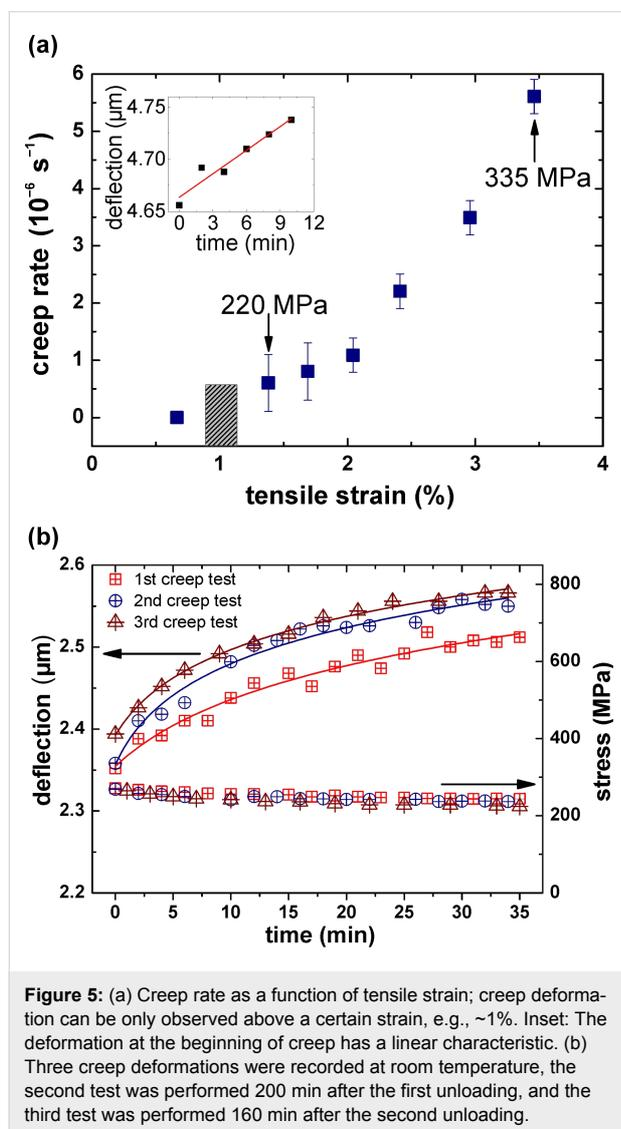
**Figure 5:** (a) Creep rate as a function of tensile strain; creep deformation can be only observed above a certain strain, e.g., ~1%. Inset: The deformation at the beginning of creep has a linear characteristic. (b) Three creep deformations were recorded at room temperature, the second test was performed 200 min after the first unloading, and the third test was performed 160 min after the second unloading.
