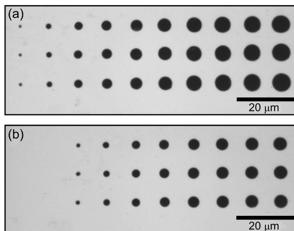
**Figure 4:** Optical micrograph of a laser-fabricated dot pattern. HDT-SAMs on a Au/glass substrate exposing a 30 nm thick Au layer are processed with single laser pulses with distinct  $\tau$  between 50  $\mu\text{s}$  (left) and 10 ms (right) and (a)  $P = 24.3$  mW, (b)  $P = 20.3$  mW. After laser processing, the pattern is transferred to the Au layer by wet-chemical etching.
