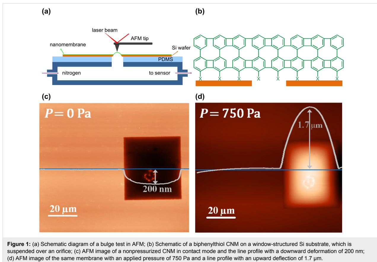
**Figure 1:** (a) Schematic diagram of a bulge test in AFM; (b) Schematic of a biphenylthiol CNM on a window-structured Si substrate, which is suspended over an orifice; (c) AFM image of a nonpressurized CNM in contact mode and the line profile with a downward deformation of 200 nm; (d) AFM image of the same membrane with an applied pressure of 750 Pa and a line profile with an upward deflection of 1.7 μm.
