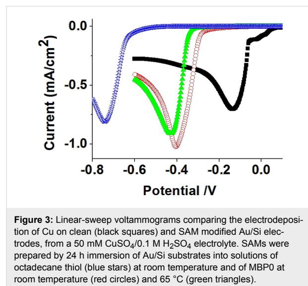
**Figure 3:** Linear-sweep voltammograms comparing the electrodeposition of Cu on clean (black squares) and SAM modified Au/Si electrodes, from a  $50$  mM  $\text{CuSO}_4/0.1$  M  $\text{H}_2\text{SO}_4$  electrolyte. SAMs were prepared by  $24$  h immersion of Au/Si substrates into solutions of octadecane thiol (blue stars) at room temperature and of MBP0 at room temperature (red circles) and  $65^\circ\text{C}$  (green triangles).
