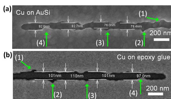
**Figure 7:** SEM images of a SAM templated copper deposit on the original MBPO coated Au/Si substrate (a) and after transfer to epoxy glue (b). The passivating line of the cross-linked SAM was written by using an e-beam dose of  $750 \text{ mC/cm}^2$ . Deposition parameters are  $-0.7 \text{ V}$  for  $1 \text{ s}$ ,  $-0.25 \text{ V}$  for  $20 \text{ s}$ . The numbered green arrows mark the corresponding features in (a) and (b).
