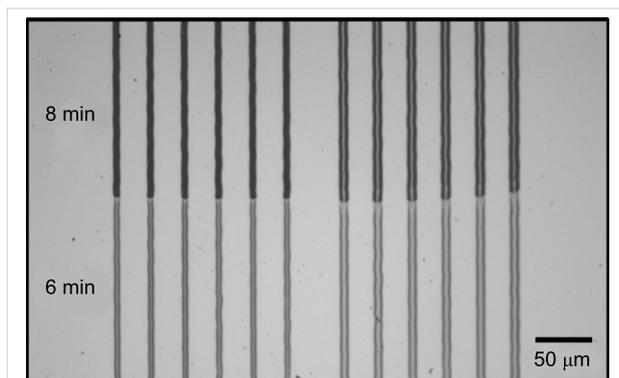
**Figure 8:** Optical micrograph of a laser-patterned HDT SAM on a Au/glass substrate exposing a 10 nm thick Au layer after wet-chemical etching. The micrograph displays surface areas that have been dipped into the etchant for 6 min (bottom) or 8 min (top).
