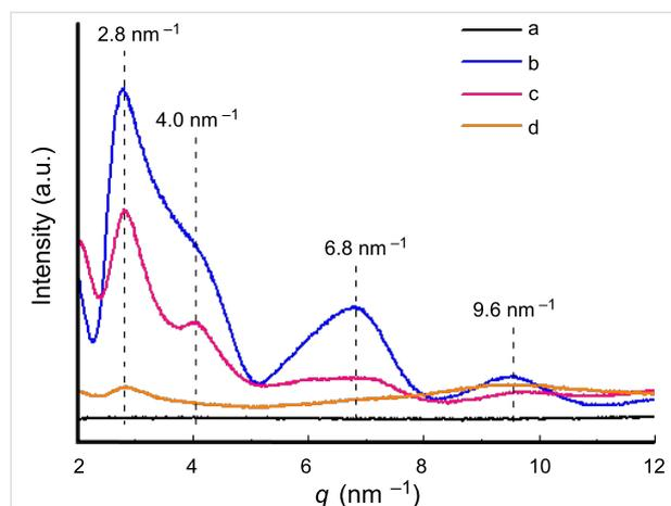
**Figure 14:** WAXD profiles of (a) quartz-glass capillary background, (b) bare imogolite, (c) BMPOPO<sub>4</sub>-imogolite, and (d) PMMA-g-imogolite with  $M_n = 32700$  and  $M_w/M_n = 1.33$ . Reprinted with permission from W. Ma et al., *Chem. Commun.* **2011**, 47, 5813–5815 [40]. © 2011, The Royal Society of Chemistry.
