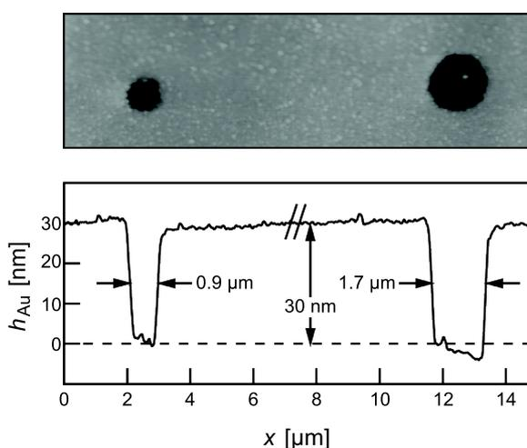
**Figure 5:** AFM data from patterning experiments with HDT-SAMs on Au/glass substrates exposing a 30 nm thick Au layer. The structures were fabricated by using single laser pulses at  $P = 24.3$  mW and with distinct  $\tau$  of 50  $\mu\text{s}$  (left) and 100  $\mu\text{s}$  (right). Pattern transfer to the Au layer was carried out by wet-chemical etching. Diameters refer to values at half-depth.
