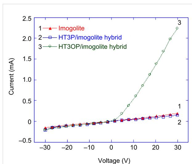
**Figure 19:**  $I$ - $V$  curves of imogolite, HT3P/imogolite, and HT3OP/imogolite hybrid. Reprinted with permission from W. O. Yah et al., *Bull. Chem. Soc. Jpn.* 2011, 84, 893–902 [60]. © 2011, The Chemical Society of Japan.
