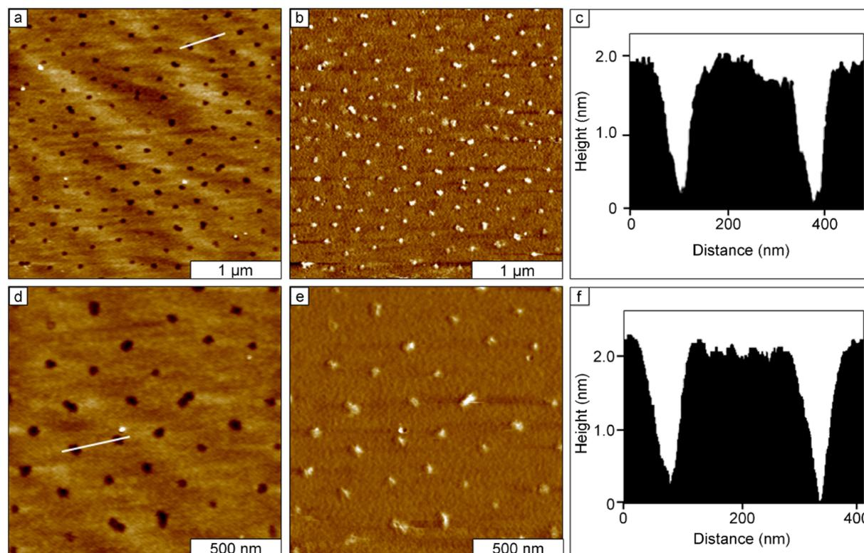
**Figure 6:** Nanostructured film of OTS produced by immersion of annealed silica masks in OTS solutions. Contact-mode AFM images are shown for OTS nanostructures formed on Si(111) with 250 nm silica mesospheres: (a)  $2.75 \times 2.75 \mu\text{m}^2$  topograph; (b) corresponding lateral-force view; (c) height profile of the line in (a); (d)  $1.5 \times 1.5 \mu\text{m}^2$  zoom-in view of (a); (e) lateral-force frame simultaneously acquired with (d); (f) cursor plot for the line in (d).
