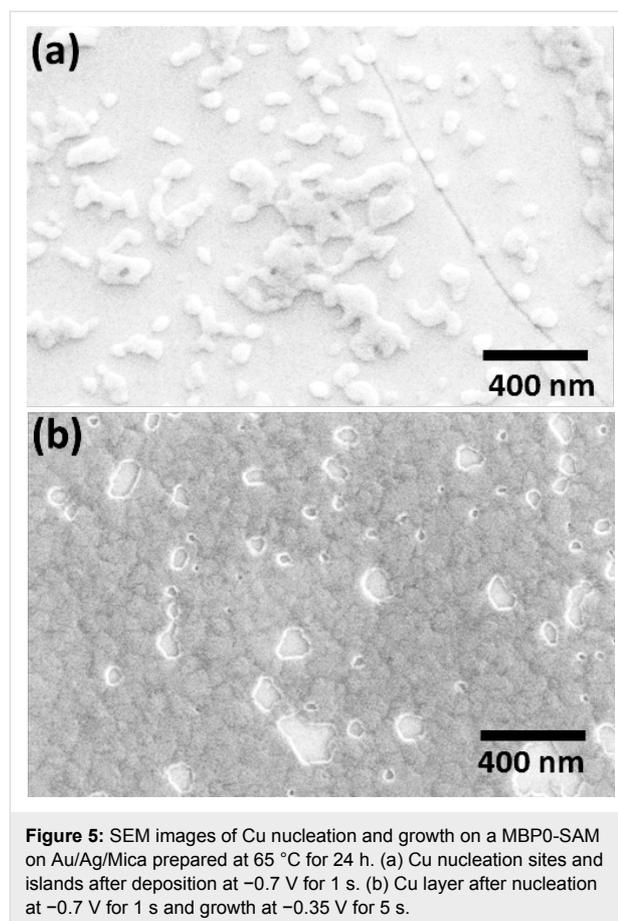
**Figure 5:** SEM images of Cu nucleation and growth on a MBP0-SAM on Au/Ag/Mica prepared at  $65$  °C for 24 h. (a) Cu nucleation sites and islands after deposition at  $-0.7$  V for 1 s. (b) Cu layer after nucleation at  $-0.7$  V for 1 s and growth at  $-0.35$  V for 5 s.
