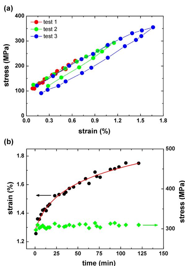
**Figure 4:** (a) Stress–strain relationship of three loading–unloading measurements on a NBPT CNM with different maximum strains at ~0.65%, ~1.2% and ~1.7%; (b) Strain exhibits a nonlinear increase at a stress of  $304 \pm 15$  MPa, indicating a tensile-creep behavior.
