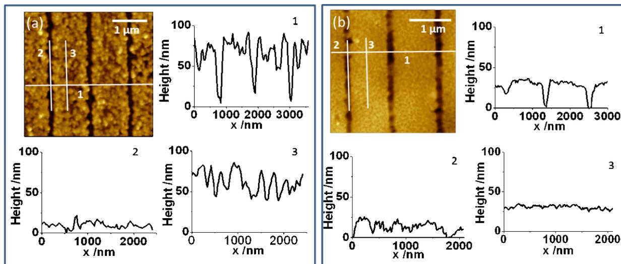
**Figure 8:** AFM topography images of Cu electrodeposited onto an e-beam-patterned MBP0-SAM on Au/Si (a) before and (b) after lift-off. The height profiles shown are taken along the numbered cross-sections. Lines of cross-linked MBP0 were written by using a dose of 1000 mC/cm<sup>2</sup>. The parameters for Cu deposition were  $-0.7$  V for 1 s,  $-0.35$  V for 10 s.
