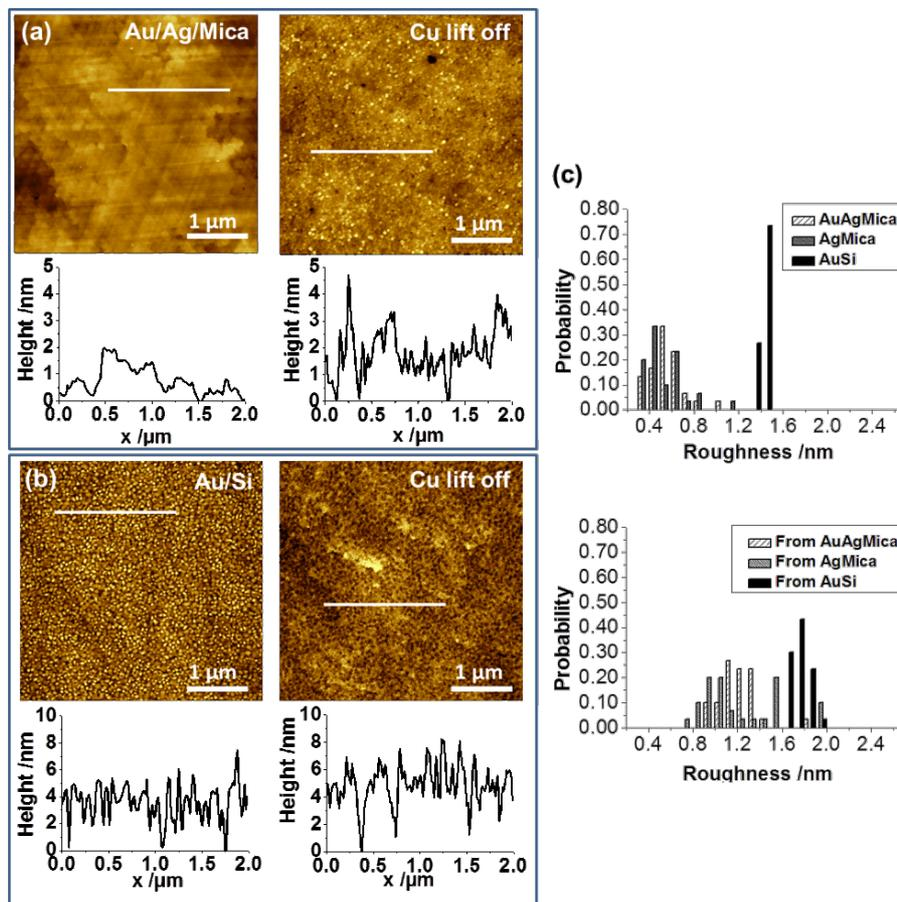
**Figure 10:** (a,b) AFM topography images and height profiles along the lines indicated, comparing the roughness of different substrates with the corresponding surface of the Cu film after lift-off; (a) Au/Ag/mica (b) Au/Si. Conditions for Cu deposition:  $-0.8$  V for 2 s and  $-0.35$  V. (c) Roughness histograms of substrates (top) and Cu surfaces after lift-off (bottom) from 30 measurements of areas  $1 \times 1 \mu\text{m}^2$  in size for each surface.
