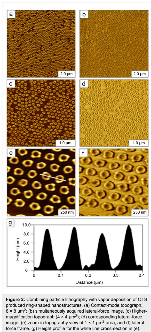
**Figure 2:** Combining particle lithography with vapor deposition of OTS produced ring-shaped nanostructures. (a) Contact-mode topograph,  $8 \times 8 \mu\text{m}^2$ ; (b) simultaneously acquired lateral-force image. (c) Higher-magnification topograph ( $4 \times 4 \mu\text{m}^2$ ); (d) corresponding lateral-force image. (e) zoom-in topography view of  $1 \times 1 \mu\text{m}^2$  area; and (f) lateral-force frame. (g) Height profile for the white line cross-section in (e).
