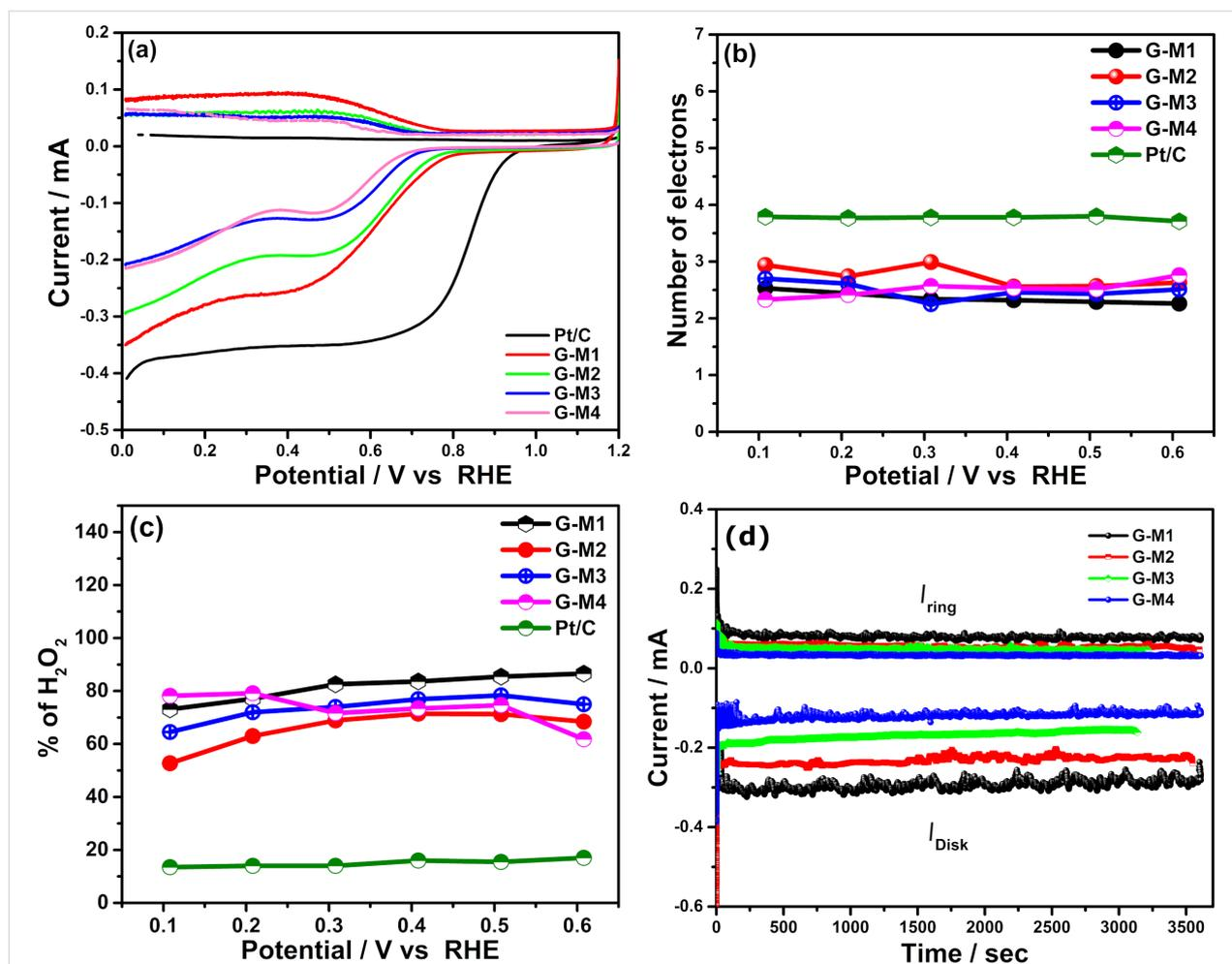
**Figure 4:** (a) LSV scans of O<sub>2</sub> reduction and H<sub>2</sub>O<sub>2</sub> (HO<sub>2</sub><sup>-</sup>) oxidation on different EEG-modified RRDE samples. (b) The number of electrons transferred during ORR per O<sub>2</sub> molecule and (c) the percentage (%) of formed H<sub>2</sub>O<sub>2</sub> (calculated from Figure 4a) is shown. (d) Chronoamperograms of O<sub>2</sub> reduction and H<sub>2</sub>O<sub>2</sub> oxidation processes at 0.358 V and 1.5 V vs RHE on different electrodes.
