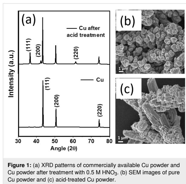
**Figure 1:** (a) XRD patterns of commercially available Cu powder and Cu powder after treatment with 0.5 M HNO<sub>3</sub>. (b) SEM images of pure Cu powder and (c) acid-treated Cu powder.
