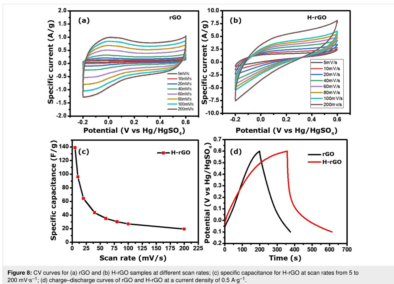
**Figure 8:** CV curves for (a) rGO and (b) H-rGO samples at different scan rates; (c) specific capacitance for H-rGO at scan rates from 5 to  $200\text{ mV}\cdot\text{s}^{-1}$ ; (d) charge–discharge curves of rGO and H-rGO at a current density of  $0.5\text{ A}\cdot\text{g}^{-1}$ .
