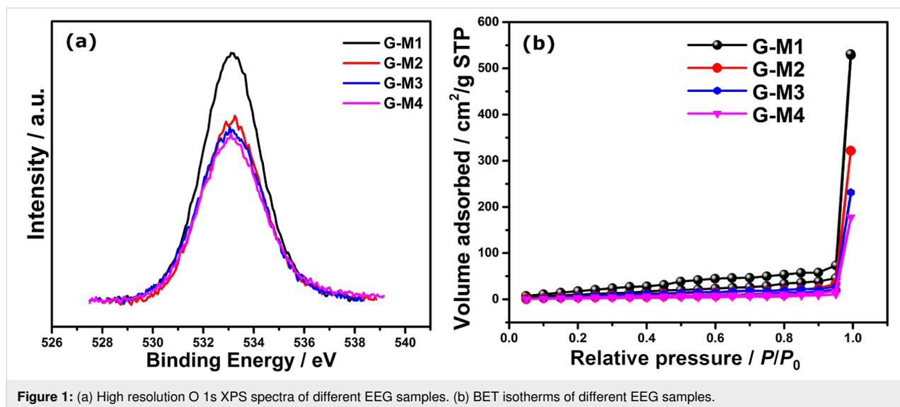
Figure 1: (a) High resolution O 1s XPS spectra of different EEG samples. (b) BET isotherms of different EEG samples.
