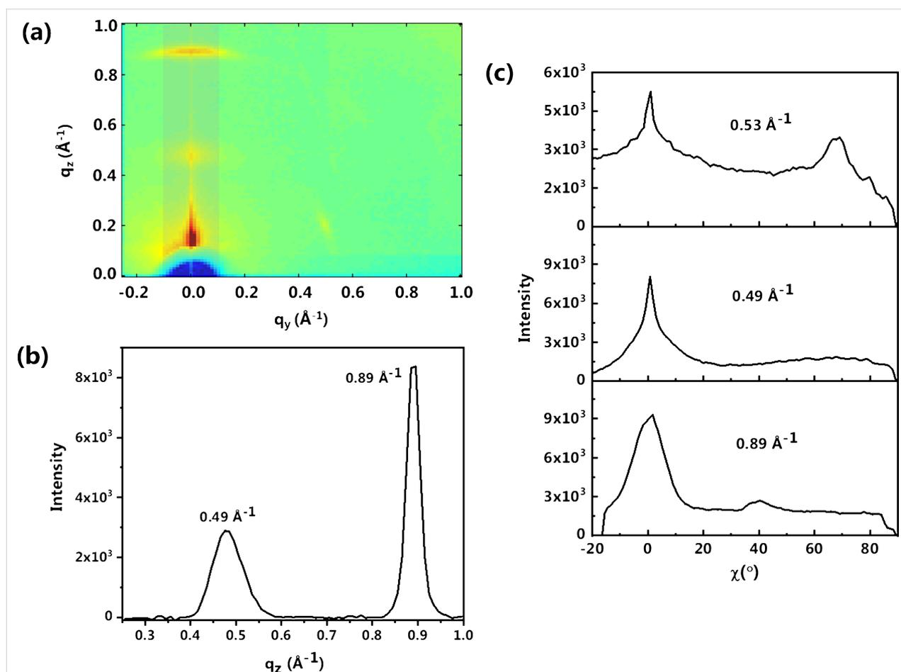
**Figure 3:** (a) 2D-GIXRD pattern of a 10 nm PbPc film on SLG/ $\text{SiO}_2/\text{Si}$ . (b) Profile section along the  $q_z$  direction. (c) Intensity as a function of the azimuthal angle for different Bragg peaks.
