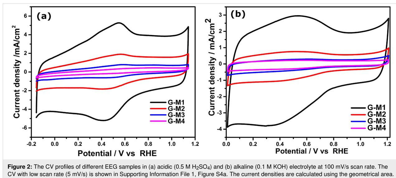
**Figure 2:** The CV profiles of different EEG samples in (a) acidic (0.5 M H<sub>2</sub>SO<sub>4</sub>) and (b) alkaline (0.1 M KOH) electrolyte at 100 mV/s scan rate. The CV with low scan rate (5 mV/s) is shown in Supporting Information File 1, Figure S4a. The current densities are calculated using the geometrical area.
