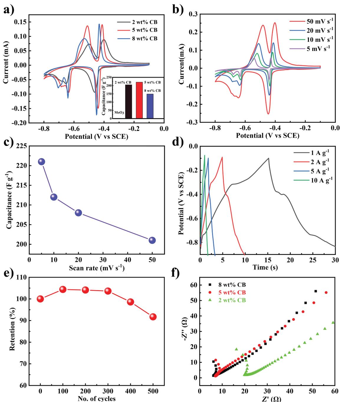
**Figure 3:** (a) CV measurement of MoO<sub>3</sub>/carbon black composites showing pseudo capacitive behavior, inset shows the change in capacitance with increasing mass fraction of carbon black; (b) performance of a composite electrode with 5 wt % CB as a function of the changing scan rate; (c) capacitance as a function of the scan rate, (d) galvanostatic charge–discharge profile of the 5 wt % CB composite; (e) capacitance retention of the 5 wt % CB composite; (f) EIS of the composites.
