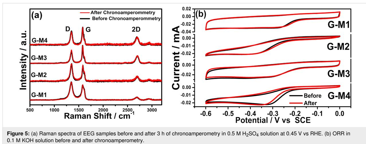
Figure 5: (a) Raman spectra of EEG samples before and after 3 h of chronoamperometry in  $0.5 \text{ M H}_2\text{SO}_4$  solution at  $0.45 \text{ V}$  vs RHE. (b) ORR in  $0.1 \text{ M KOH}$  solution before and after chronoamperometry.
