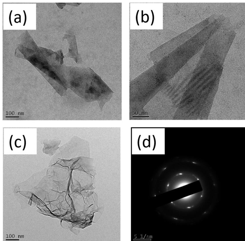
**Figure 5:** (a, b) TEM images of few-layered graphene partially rolled into nanoscrolls synthesized by irradiating graphite with microwaves in the presence of Zn metal for 30 s. (c) TEM image of graphite oxide after exfoliation through microwave irradiation in the presence of Zn metal for 30 s and (d) the corresponding selected area electron diffraction pattern.
