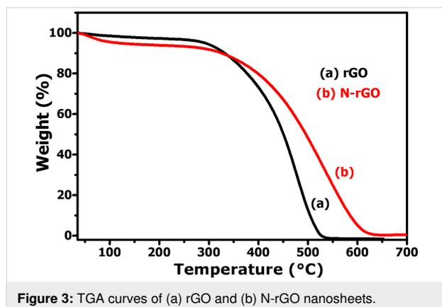
The second weight loss (93.4%) for rGO occurring between  $350$  and  $540\text{ }^{\circ}\text{C}$  can be ascribed to the decomposition of the carbon network. For N-rGO nanosheets, a significant weight loss
