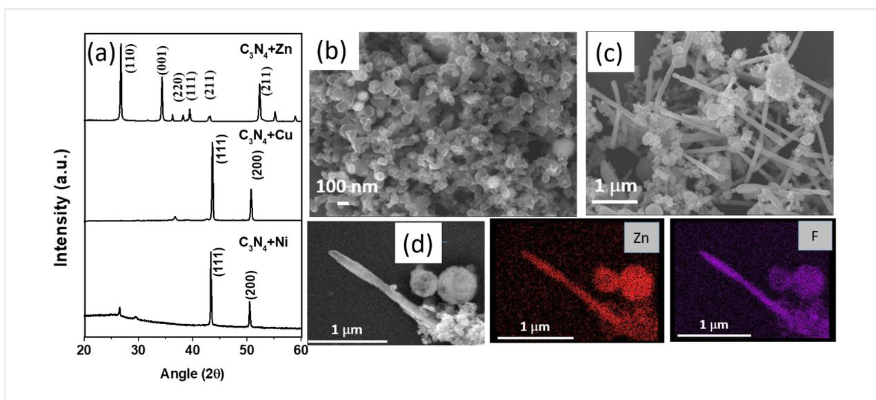
**Figure 3:** (a) XRD patterns of carbon-coated Cu and Ni nanoparticles and  $\text{ZnF}_2$  nanorods. (b) SEM images of carbon-coated Cu nanoparticles. (c) SEM images of  $\text{ZnF}_2$  nanorods. (d) SEM image and EDS elemental mapping of a single  $\text{ZnF}_2$  nanorod.
