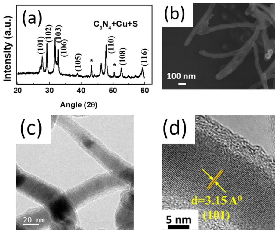
**Figure 4:** (a) XRD patterns of  $\text{CuS}$  nanorods synthesized in the presence of sulfur by microwave irradiation of copper in the presence of  $g\text{-C}_3\text{N}_4$  in a Teflon beaker for 2 min. (b) SEM, (c) TEM and (d) HRTEM images of  $\text{CuS}$  nanorods. The asterisk (\*) in panel (a) indicates the reflections from Cu.
