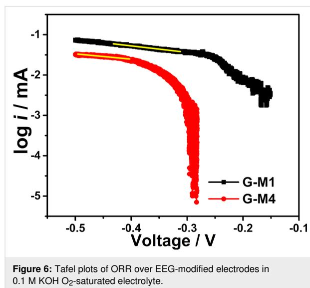
Figure 6: Tafel plots of ORR over EEG-modified electrodes in  $0.1 \text{ M KOH}$   $\text{O}_2$ -saturated electrolyte.
