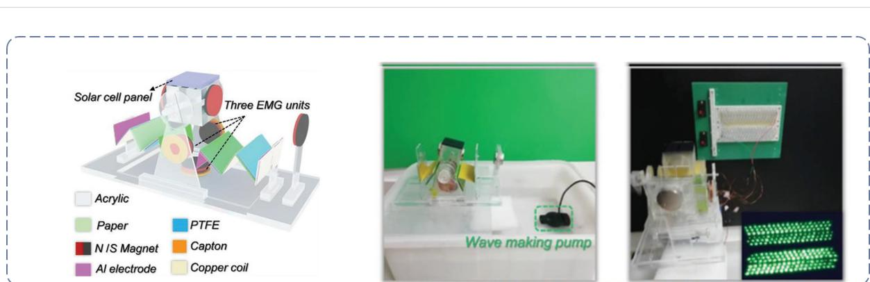
**Figure 12:** Harvesting water wave energy with a hybrid generator [163] Copyright © 2019 WILEY-VCH Verlag GmbH & Co. KGaA, Weinheim. Adapted with permission from Hongmei Yang et al., “A Nonencapsulative Pendulum-Like Paper-Based Hybrid Nanogenerator for Energy Harvesting”, Advanced Energy Materials, John Wiley and Sons.
