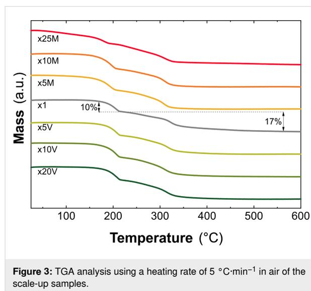
**Figure 3:** TGA analysis using a heating rate of 5 °C·min<sup>-1</sup> in air of the scale-up samples.
