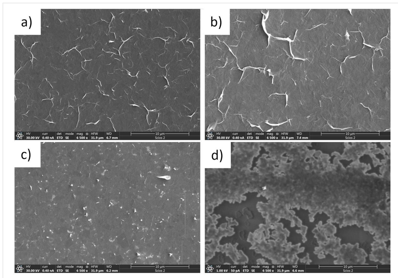
**Figure 4:** Scanning electron micrographs of films produced from the (a) initial graphene dispersion and from films produced after centrifugation at (b) 3 krpm (824g), (c) 4 krpm (1465g), and (d) 5 krpm (2289g).
