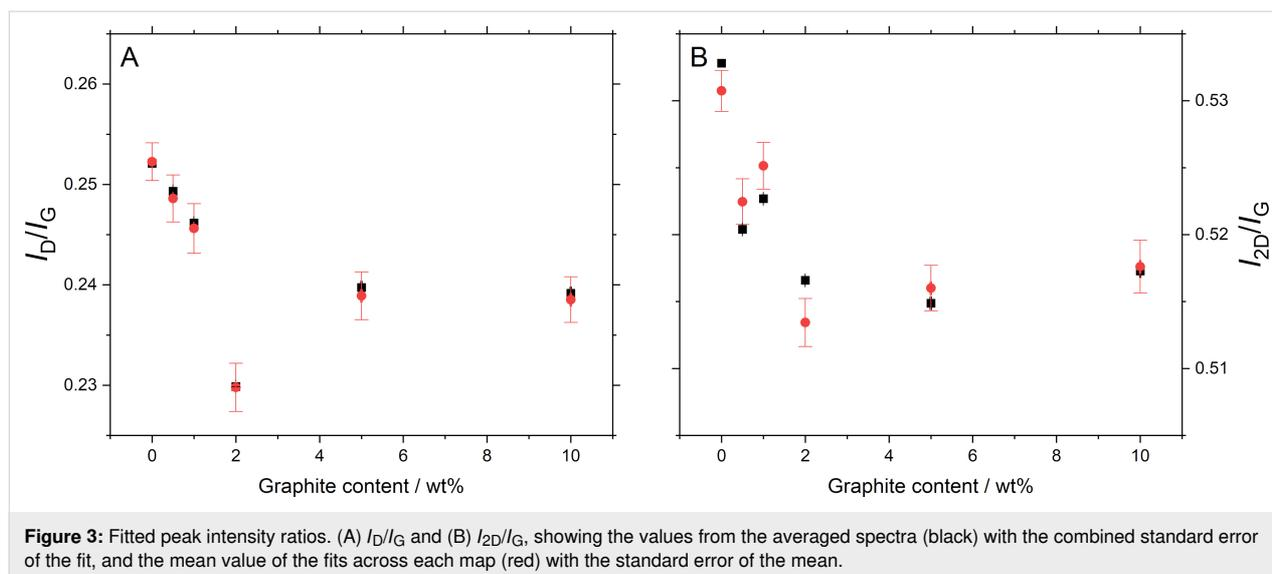
**Figure 3:** Fitted peak intensity ratios. (A)  $I_D/I_G$  and (B)  $I_{2D}/I_G$ , showing the values from the averaged spectra (black) with the combined standard error of the fit, and the mean value of the fits across each map (red) with the standard error of the mean.
