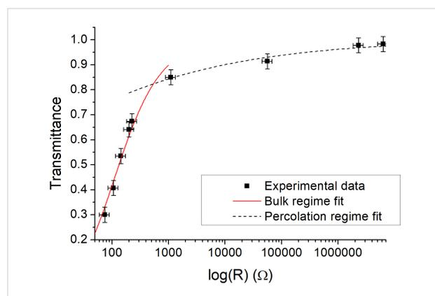
**Figure 6:** Dependence of the optical transparency on the electrical resistance of graphene films on a semi-logarithmic scale. The data can be divided into two regimes, the bulk regime (solid red line fit to Equation 1) and the percolation regime (dashed black line fit to Equation 2).
