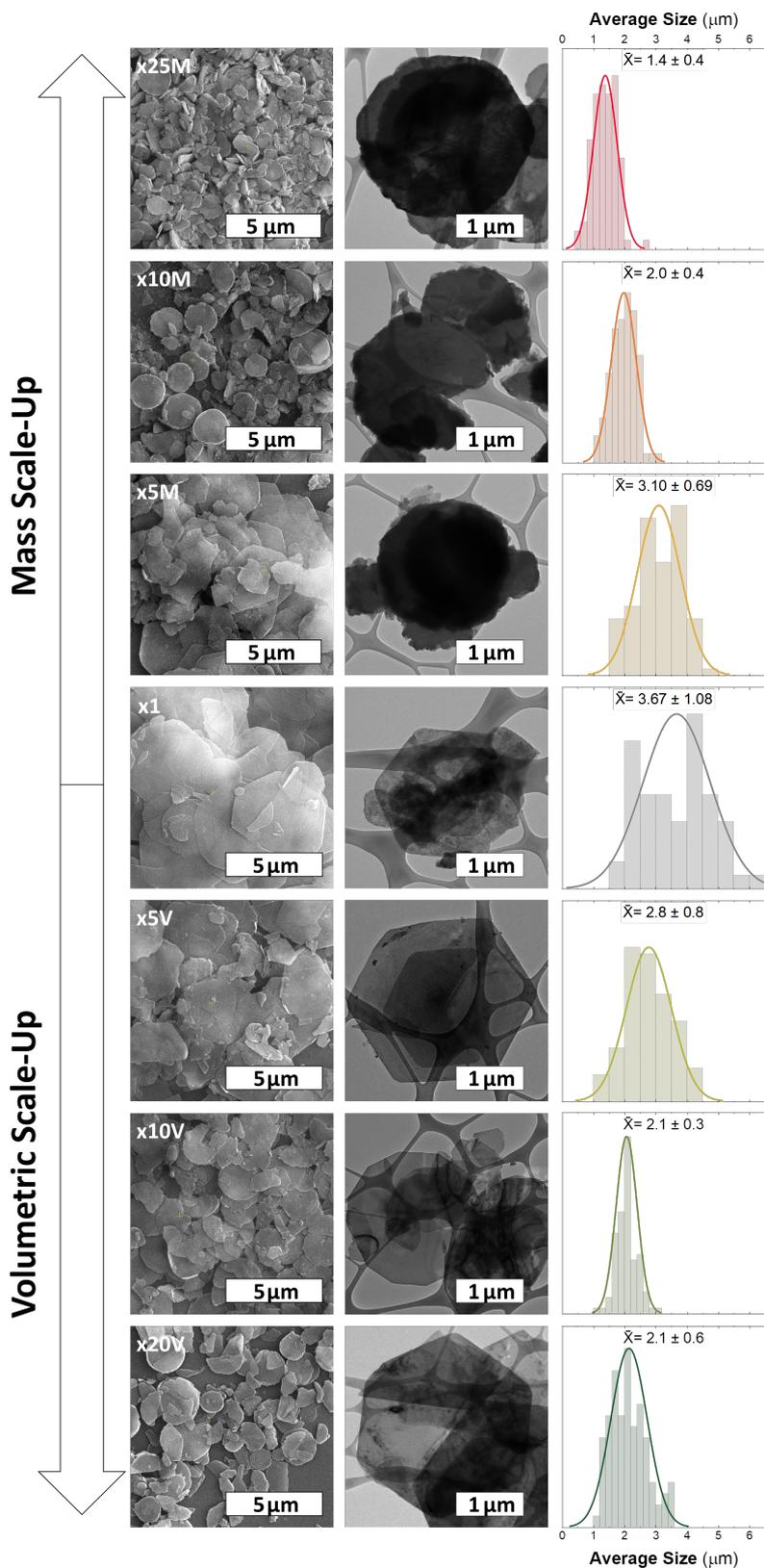
**Figure 4:** Microscopic characterization of CoAl-based LDH samples through (left) SEM and (center) TEM, and (right) the respective average size histograms.
