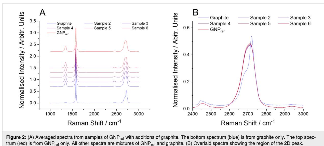
**Figure 2:** (A) Averaged spectra from samples of  $\text{GNP}_{\text{ref}}$  with additions of graphite. The bottom spectrum (blue) is from graphite only. The top spectrum (red) is from  $\text{GNP}_{\text{ref}}$  only. All other spectra are mixtures of  $\text{GNP}_{\text{ref}}$  and graphite. (B) Overlaid spectra showing the region of the 2D peak.
