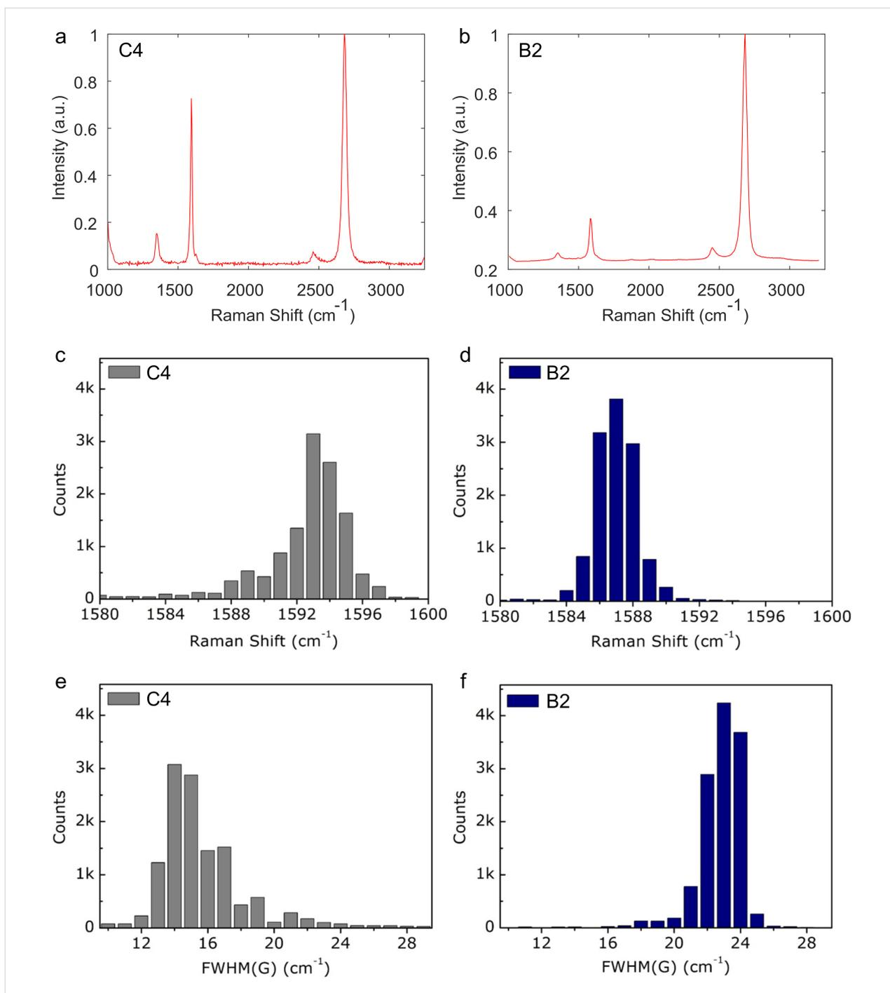
**Figure 3:** Statistical analysis of the Raman spectra of transistors prepared with transfers using PMMA mixtures with different molecular weights. (a, b) Representative Raman spectra of graphene transistor channels prepared using B2 and C4 mixtures, respectively. (c, d) Distributions of the G band peak position for B2 and C4, respectively. (e, f) Distributions of the FWHM of the G band.
