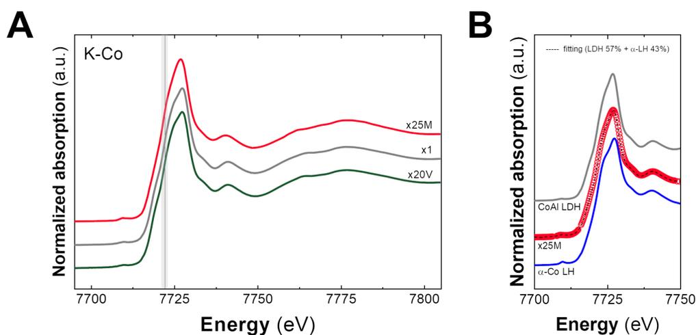
**Figure 2:** (A) Normalized XANES spectra at the Co K edge for the obtained samples. The grey line depicts the position of the absorption edge characteristic to  $\text{Co}^{\text{II}}$ . (B) Linear fit combination by employing  $\text{CoAl-LDH}$  and  $\alpha$ - $\text{Co}$  LH as references, suggesting fractions of 57% of LDH and 43% of the impurity.
