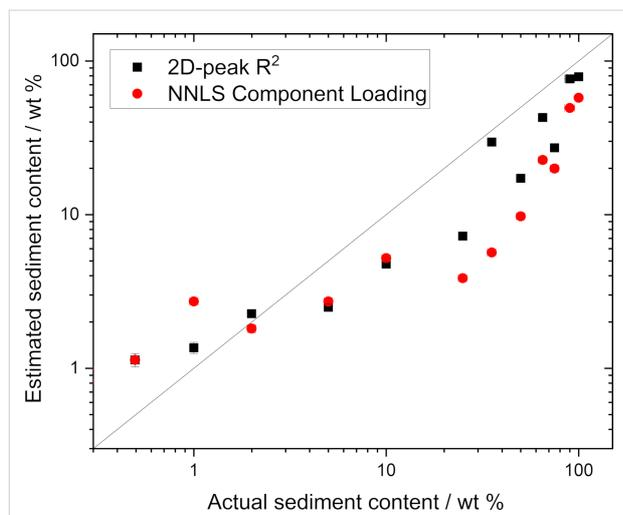
**Figure 8:** Estimated sediment content calculated from the fraction of measured spectra that are “sediment-like” based on either adjusted  $R^2$  value from fitting the 2D peak or from NNLS fitting. The line shows the expected linear trend, rather than a fit to the data.
