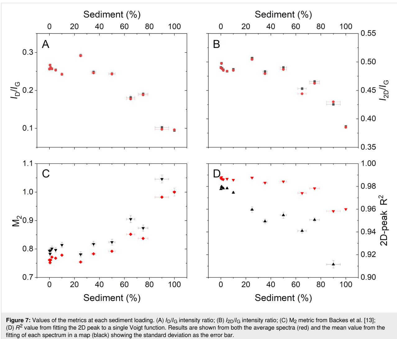
shows the widest range of use when many individual Raman spectra are fitted and then averaged, as shown in Figure 7D. However, even in this case there is little change in the calculated value from samples with up to 10 wt % sediment added.
