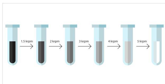
**Figure 1:** The process of cascade centrifugation.
