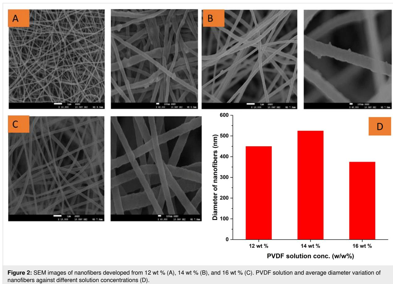
**Figure 2:** SEM images of nanofibers developed from 12 wt % (A), 14 wt % (B), and 16 wt % (C). PVDF solution and average diameter variation of nanofibers against different solution concentrations (D).
