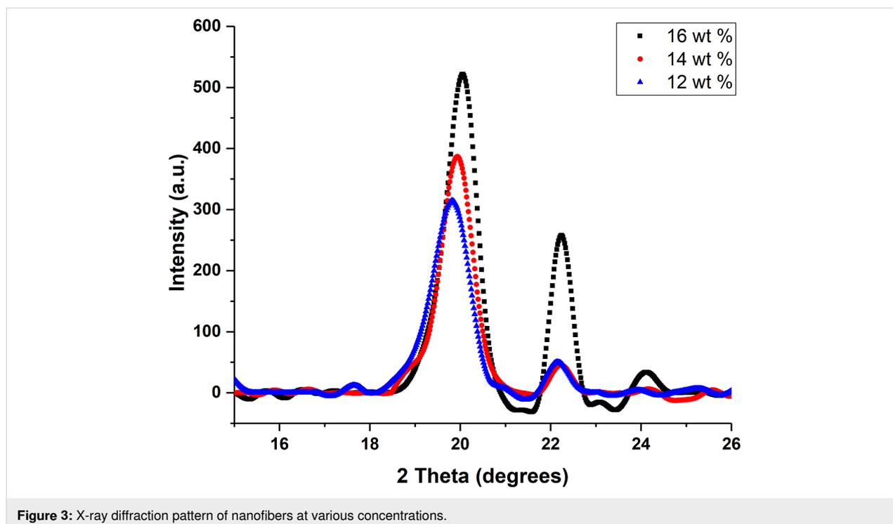
**Figure 3:** X-ray diffraction pattern of nanofibers at various concentrations.
