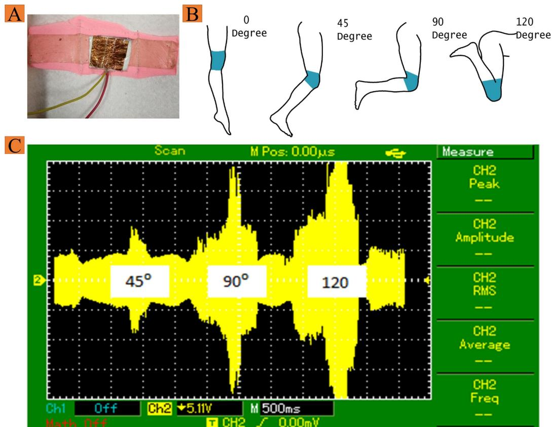
**Figure 5:** Integration of nanofibrous mesh into a knitted fabric for human body angle measurement (A), schematics showing the dressed knee at different bending angles (B), and digital oscilloscope graph at the corresponding angles (C).
