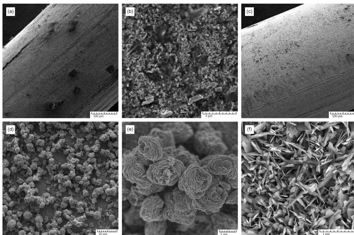
**Figure 1:** SEM images of copper oxide samples. (a, b) General view and morphology of a CuO film obtained by thermal oxidation on a copper wire; (c, d) general view of a copper wire with CuO layer obtained by chemical hydrothermal oxidation; (e) 3D flower-like nanostructured formations on the surface of the main CuO layer (f).
