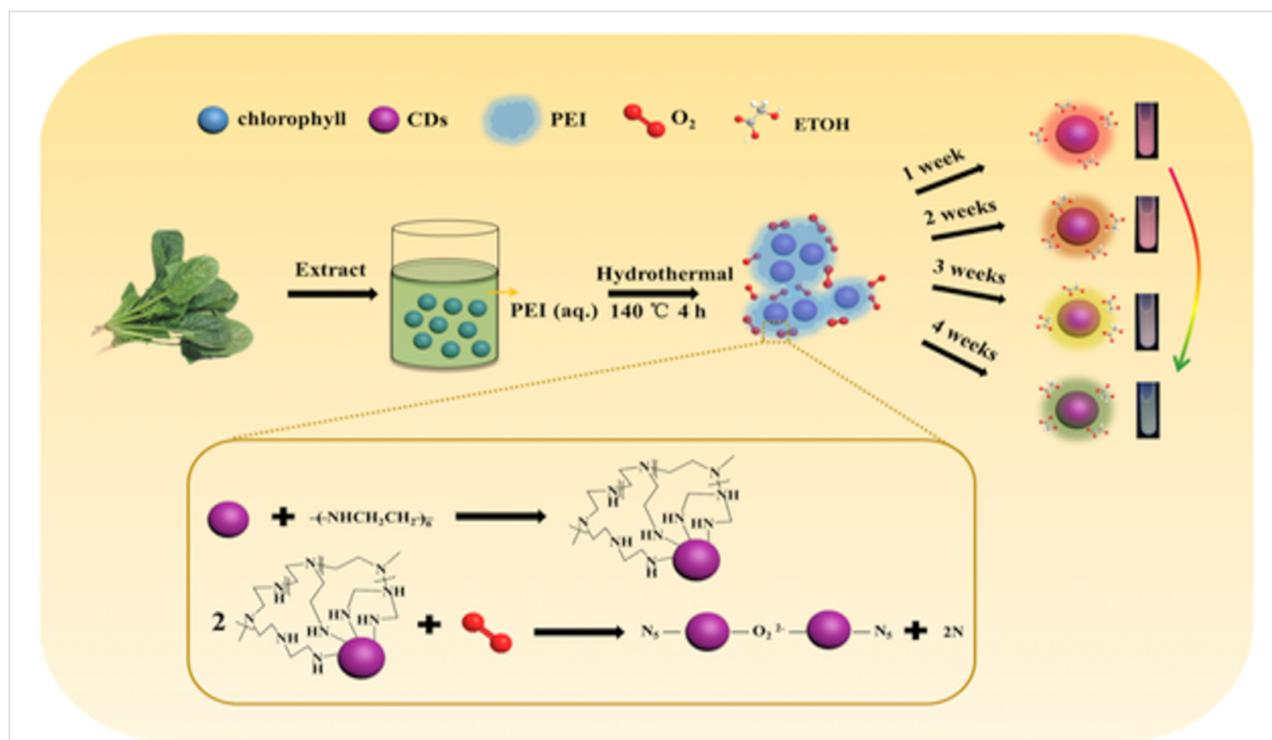
**Figure 5:** Schematic representation of the whole process. Figure 5 was reprinted from [102], Journal of Luminescence, vol. 227, by X. Xu; L. Cai; G. Hu; L. Mo; Y. Zheng; C. Hu; B. Lei; X. Zhang; Y. Liu; J. Zhuang, "Red-emissive carbon dots from spinach: Characterization and application in visual detection of time", article no. 117534, Copyright Elsevier (2020), with permission from Elsevier. This content is not subject to CC BY 4.0.
