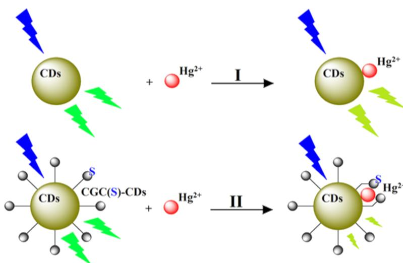
**Figure 10:** Detection mechanism of  $\text{Hg}^{2+}$  by using the CGCS-CDs as fluorescence probe. Figure 10 was reprinted from [142], *Microchemical Journal*, vol. 145, by G. Liu; H. Jia; N. Li; X. Li; Z. Yu; J. Wang; Y. Song, "High-fluorescent carbon dots (CDs) originated from China grass carp scales (CGCS) for effective detection of  $\text{Hg(II)}$  ions", pages 718-728, Copyright Elsevier (2019), with permission from Elsevier. This content is not subject to CC BY 4.0.
