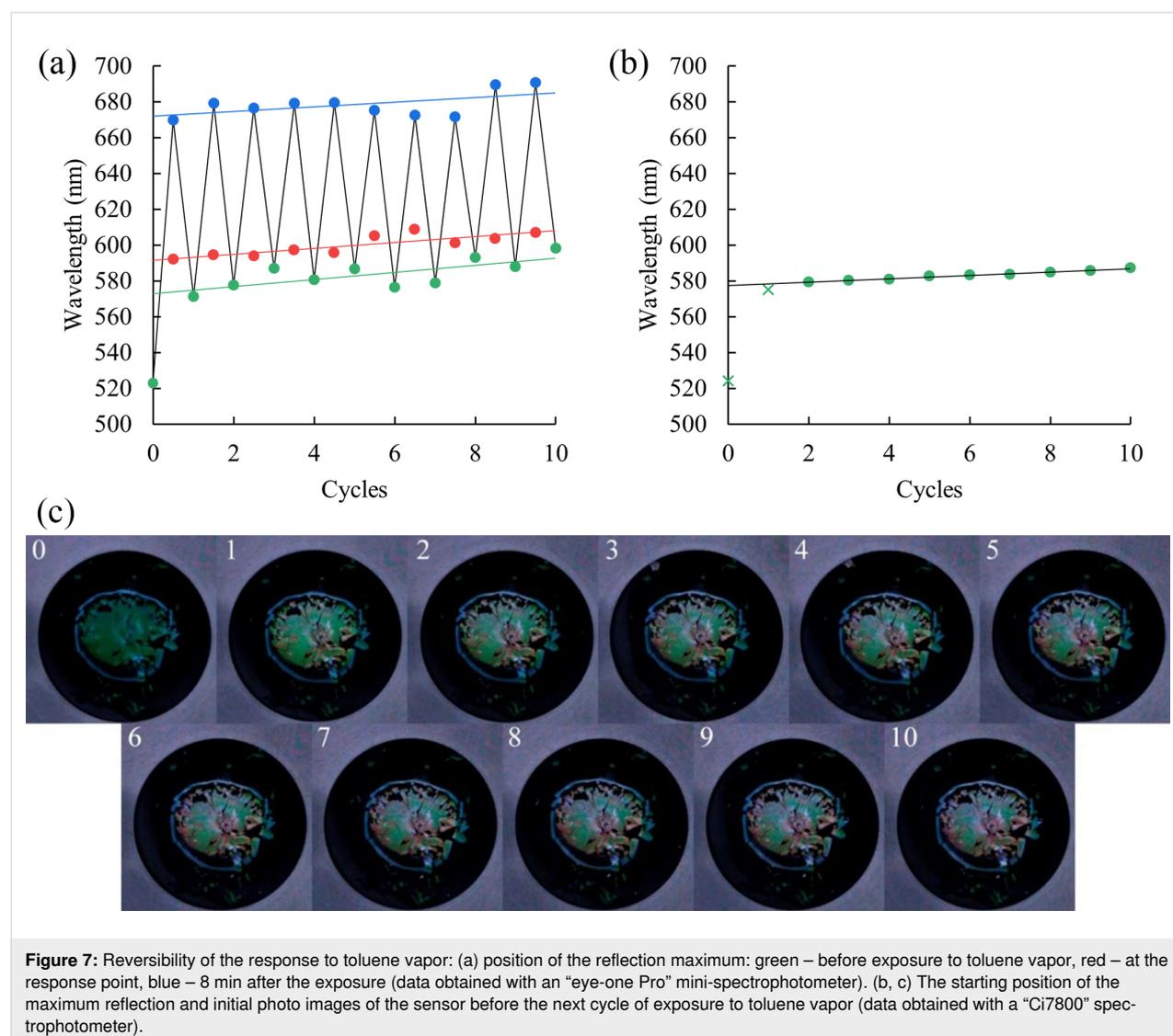
**Figure 7:** Reversibility of the response to toluene vapor: (a) position of the reflection maximum: green – before exposure to toluene vapor, red – at the response point, blue – 8 min after the exposure (data obtained with an “eye-one Pro” mini-spectrophotometer). (b, c) The starting position of the maximum reflection and initial photo images of the sensor before the next cycle of exposure to toluene vapor (data obtained with a “Ci7800” spectrophotometer).
