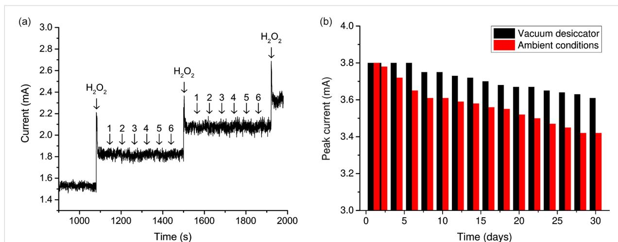
**Figure 7:** (a) Amperometric response of the nanostructured CuO electrode in 0.1 M NaOH with stepwise addition of H<sub>2</sub>O<sub>2</sub> at concentrations from 100 to 300 μM and the most common interfering substances: (1) ascorbic acid, (2) uric acid, (3) dopamine, (4) NaCl, (5) glucose, and (6) acetaminophen. (b) Stability study and the dependence of the change in the electrochemical signal on the storage time of the samples.
