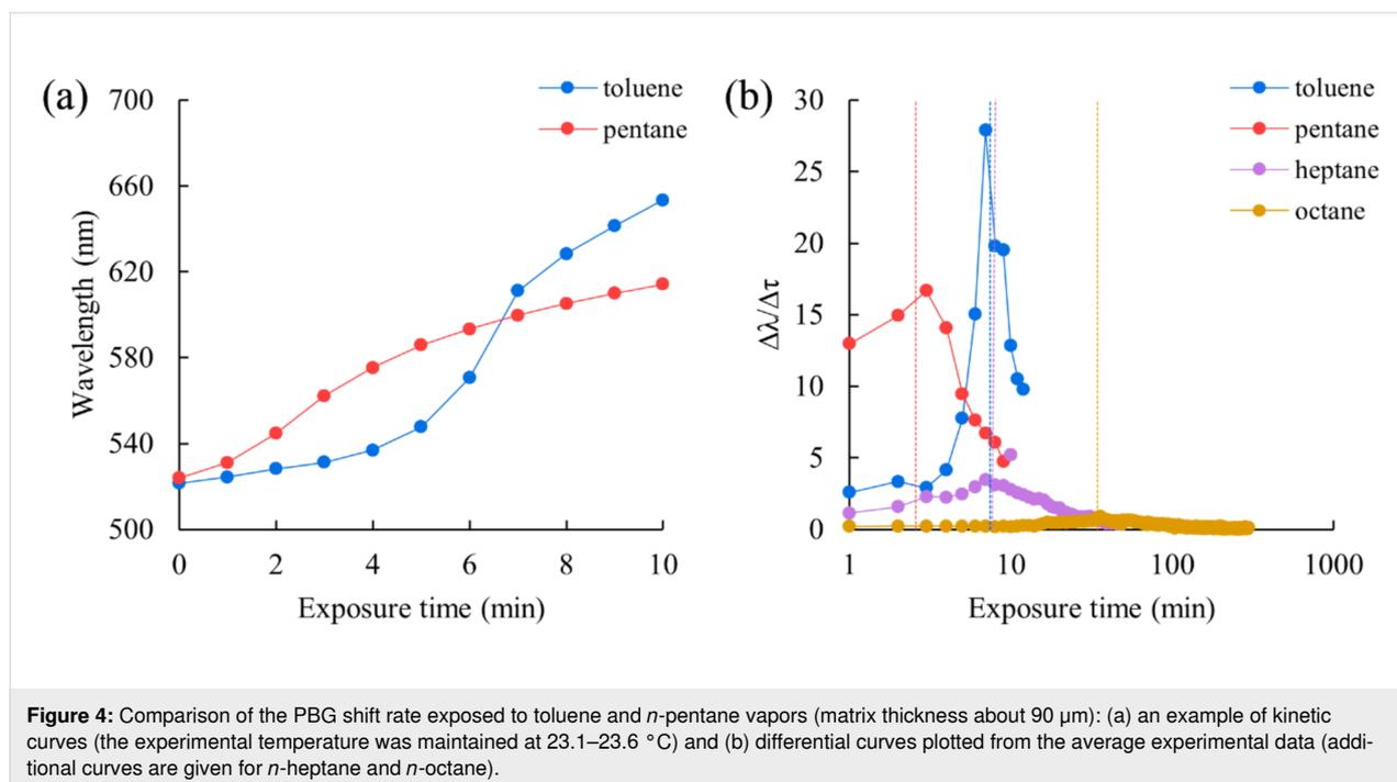
**Figure 4:** Comparison of the PBG shift rate exposed to toluene and  $n$ -pentane vapors (matrix thickness about 90  $\mu\text{m}$ ): (a) an example of kinetic curves (the experimental temperature was maintained at 23.1–23.6  $^{\circ}\text{C}$ ) and (b) differential curves plotted from the average experimental data (additional curves are given for  $n$ -heptane and  $n$ -octane).
