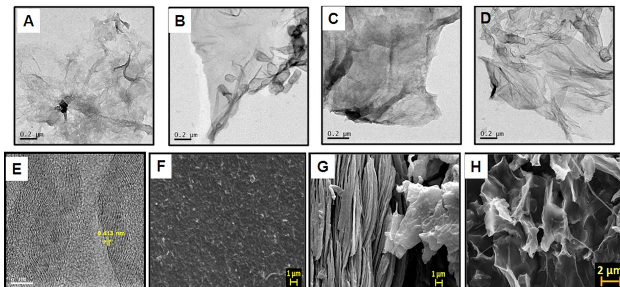
**Figure 3:** (A) TEM images of as-synthesized GO, ERGO synthesized in different electrolytes: (B) PBS pH 4.5, (C) pH 7, and (D) pH 9.6. (E) HRTEM image of ERGO in PBS pH 4.5. (F) SEM micrographs of as-synthesized GO, (G) ERGO in PBS pH 4.5 and (H) FESEM of ERGO in PBS pH 4.5 at different magnifications.
