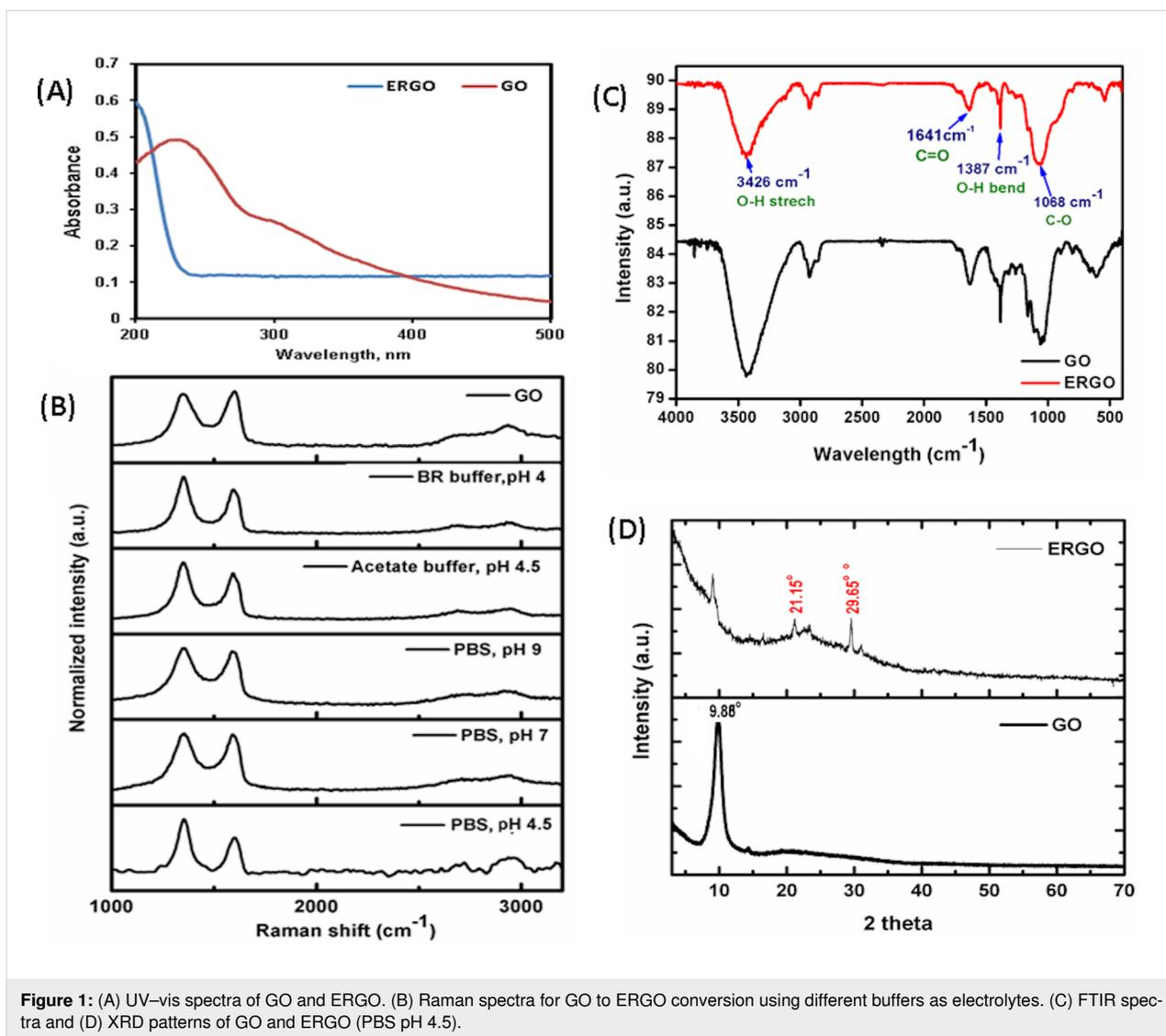
**Figure 1:** (A) UV-vis spectra of GO and ERGO. (B) Raman spectra for GO to ERGO conversion using different buffers as electrolytes. (C) FTIR spectra and (D) XRD patterns of GO and ERGO (PBS pH 4.5).
