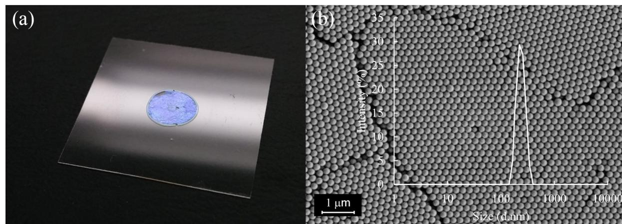
**Figure 2:** (a) Photo of the sensor and (b) electron microscopy image of a CCA of polystyrene particles without a PDMS layer on a glass substrate (effective particle size = 201 nm). The data obtained with dynamic light scattering slightly overestimates the diameter in comparison with the data obtained from microphotographs. This may be related to the specificity of the dynamic light scattering (DLS) method (hydrodynamic diameter measurement).
