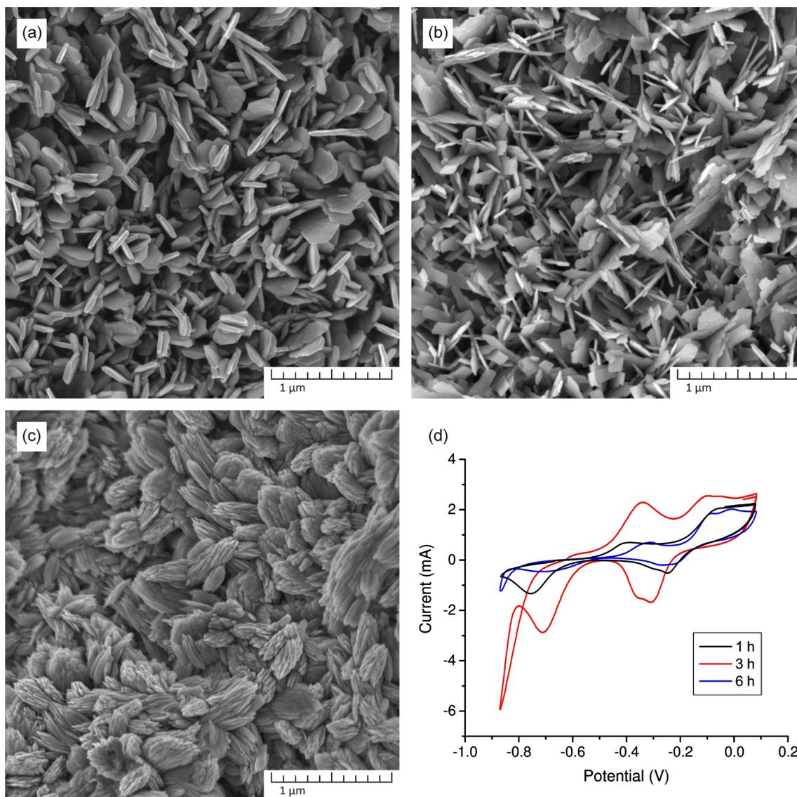
**Figure 4:** SEM images of CuO nanostructures obtained via hydrothermal oxidation method after (a) 1 h, (b) 3 h, and (c) 6 h. (d) CV curves of the CuO samples after 1, 3, and 6 h of synthesis time. Measurements were carried out in 0.1 M NaOH solution containing 1 mM  $\text{H}_2\text{O}_2$ .
