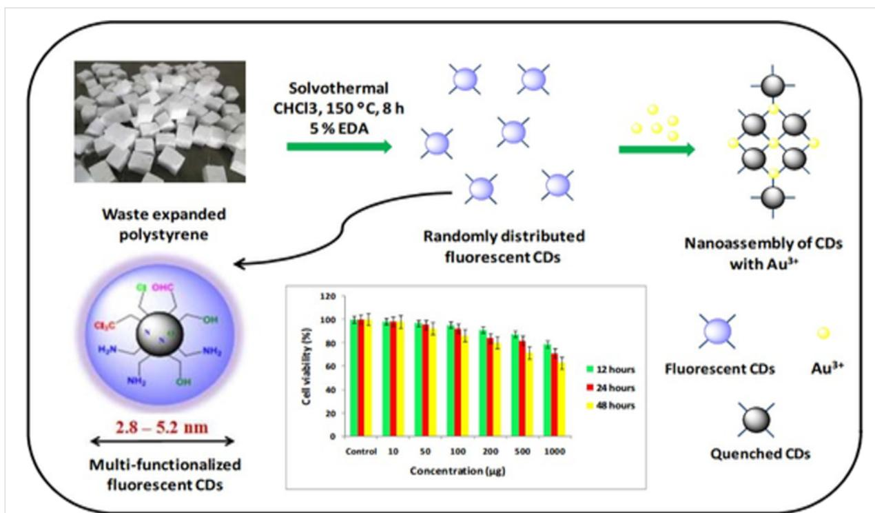
**Figure 17:** Highly luminescent, multi-functionalized, cell-viable CDs were prepared from waste expanded polystyrene and demonstrated as an efficient probe for Au<sup>3+</sup> sensing. Reprinted with permission from [154], Copyright 2020 American Chemical Society. This content is not subject to CC BY 4.0.
