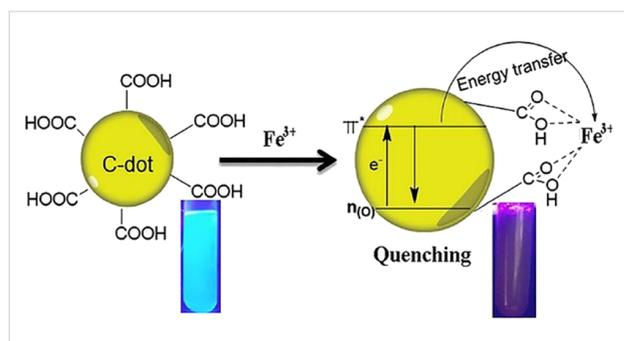
**Figure 9:** The proposed quenching mechanism of CDs prepared from betel leaves. Figure 9 was reprinted from [140], *Materials Today: Proceedings*, vol. 34, by D. Raja; D. Sundaramurthy, “Facile synthesis of fluorescent carbon quantum dots from Betel leaves (*Piper betle*) for  $\text{Fe}^{3+}$  sensing”, pages 488-492, Copyright Elsevier (2021), with permission from Elsevier. This content is not subject to CC BY 4.0.
