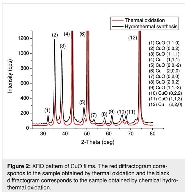
**Figure 2:** XRD pattern of CuO films. The red diffractogram corresponds to the sample obtained by thermal oxidation and the black diffractogram corresponds to the sample obtained by chemical hydrothermal oxidation.
