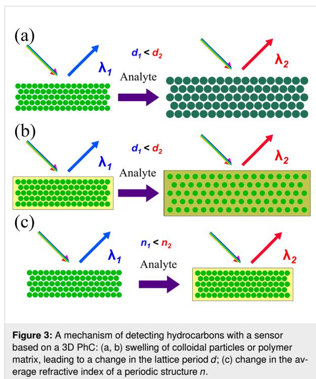
**Figure 3:** A mechanism of detecting hydrocarbons with a sensor based on a 3D PhC: (a, b) swelling of colloidal particles or polymer matrix, leading to a change in the lattice period  $d$ ; (c) change in the average refractive index of a periodic structure  $n$ .
