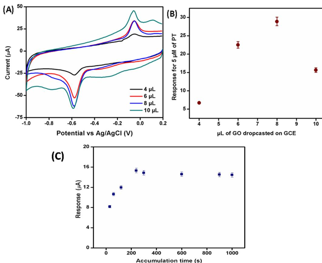
**Figure 6:** (A) Cyclic voltammograms of  $10 \mu\text{M}$  PT in PBS, pH 7, with different amounts of GO deposited on bare GCE for the preparation of modified ERGO/GCE. (B) Peak current of cyclic voltammetry using  $10 \mu\text{M}$  PT with different amounts of GO deposited on bare GCE for preparation of modified ERGO/GCE. (C) Peak response of  $10 \mu\text{M}$  PT with variation of the accumulation time before voltammetric measurements.
