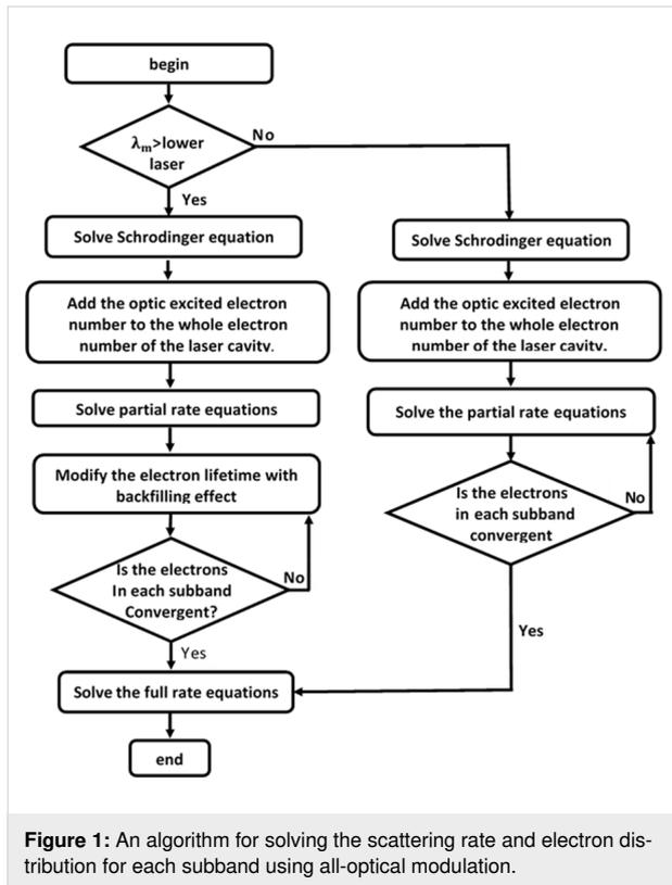
The number of photoexcited electrons, which is closely related to the number and area density of photons, forms the basis of the subsequent numerical calculation. When the modulated QCL is illuminated on the facet of its active region at an angle of 30°, almost all the laser energy is absorbed [19], so we disregard this loss, and the initial photoexcited electrons are generated from the valence band.
