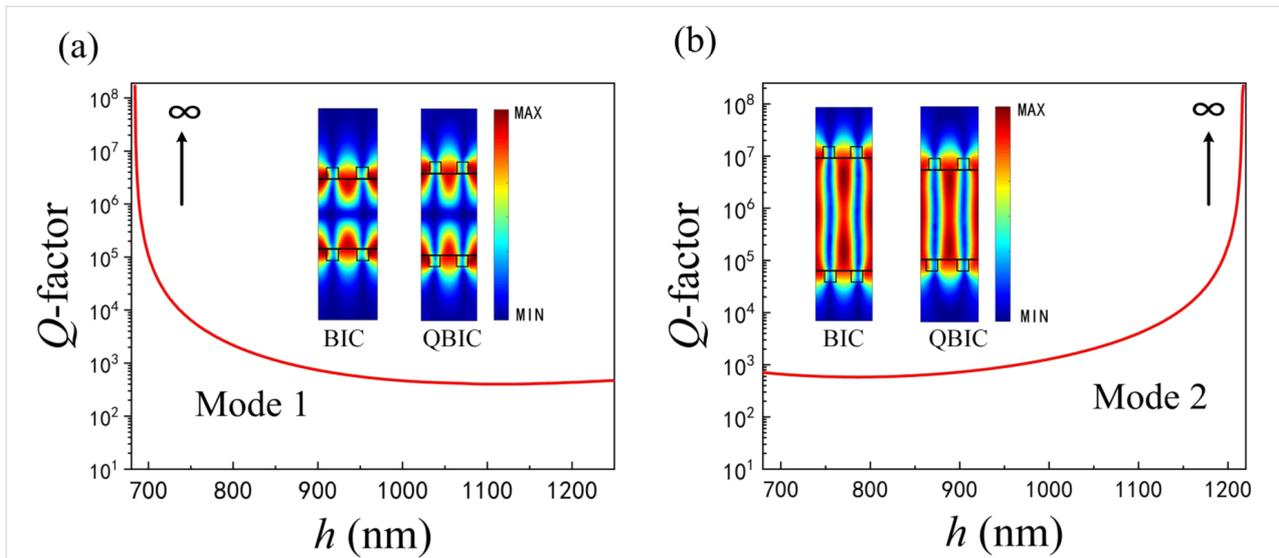
**Figure 7:** The  $Q$ -factor as a function of cavity length  $h$  of a) mode 1 and b) mode 2. The insets show the field distributions of the corresponding BIC and QBIC for the two modes.
