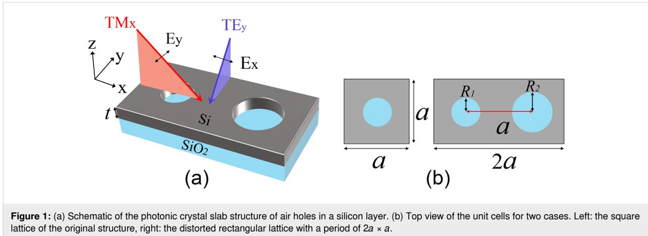
**Figure 1:** (a) Schematic of the photonic crystal slab structure of air holes in a silicon layer. (b) Top view of the unit cells for two cases. Left: the square lattice of the original structure, right: the distorted rectangular lattice with a period of  $2a \times a$ .
