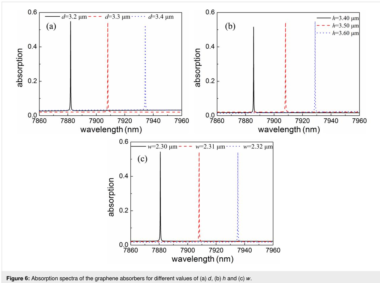
ultrasharp absorption can be maintained with a large tolerance regarding the geometric parameters, which is beneficial for real-life fabrication.
