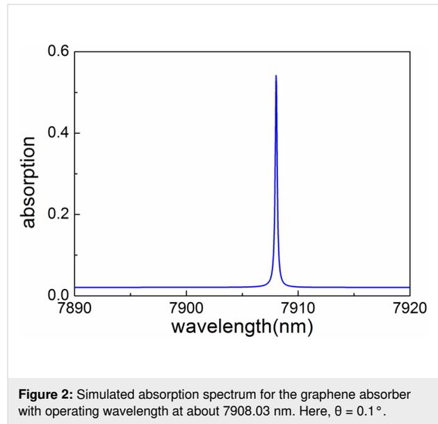
**Figure 2:** Simulated absorption spectrum for the graphene absorber with operating wavelength at about 7908.03 nm. Here,  $\theta = 0.1^\circ$ .
