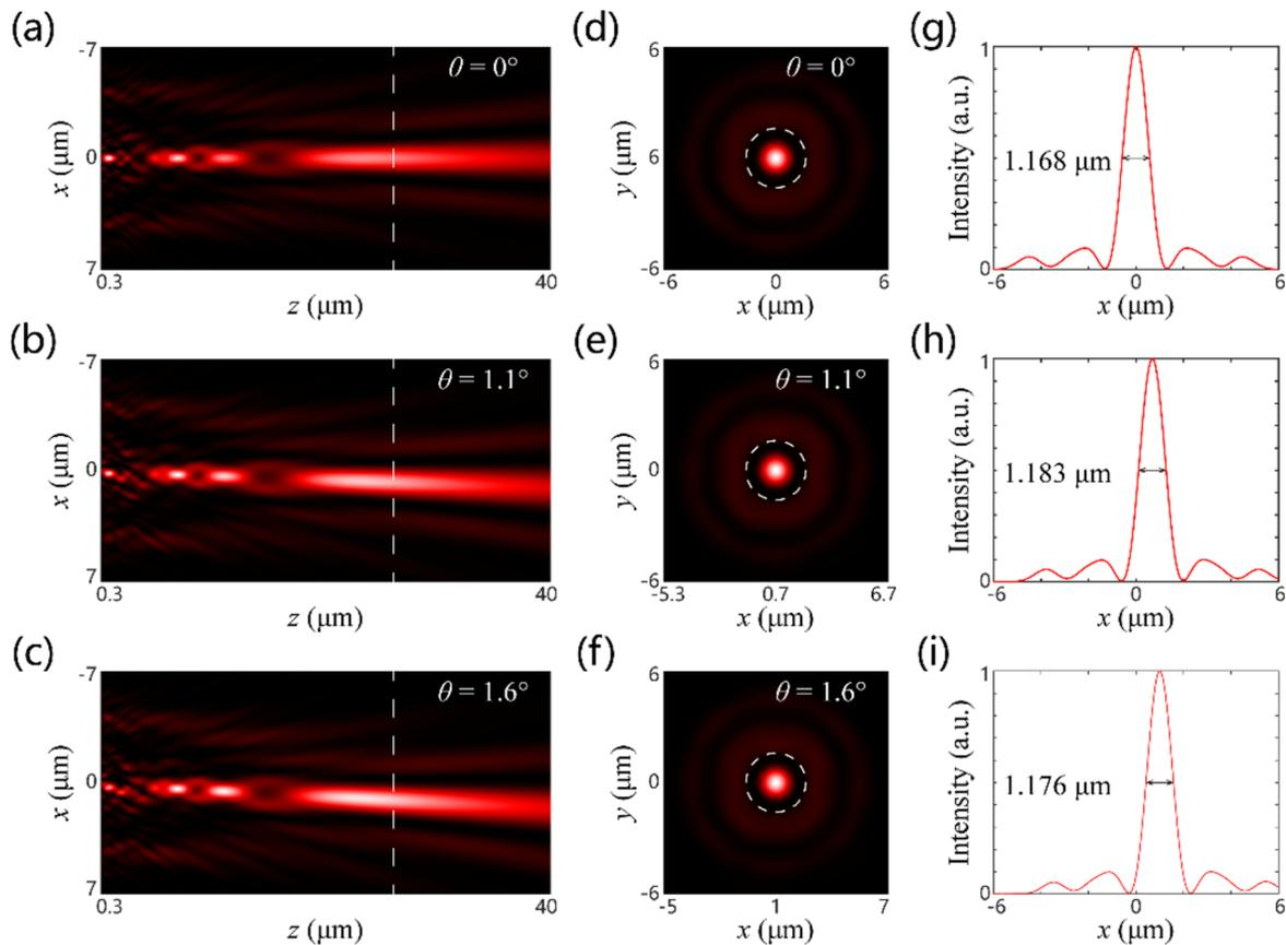
**Figure 5:** Simulated intensity distributions for different incident angles with LCP incidence corresponding to the SSL with long focal length. (a–c) Intensity distributions along the propagating direction. The dashed white lines represent the focal plane of the SSL. (d–f) Intensity distributions in the focal plane. The dashed white circles represent the diffraction-limited focal spot (Airy disk). (g–i) Intensity distributions of the sub-diffraction spot along the  $x$ -direction.
