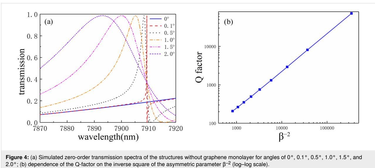
**Figure 4:** (a) Simulated zero-order transmission spectra of the structures without graphene monolayer for angles of  $0^\circ$ ,  $0.1^\circ$ ,  $0.5^\circ$ ,  $1.0^\circ$ ,  $1.5^\circ$ , and  $2.0^\circ$ ; (b) dependence of the Q-factor on the inverse square of the asymmetric parameter  $\beta^{-2}$  (log–log scale).
