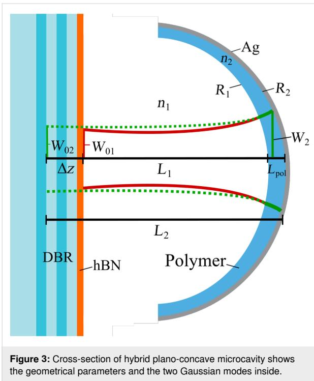
**Figure 3:** Cross-section of hybrid plano-concave microcavity shows the geometrical parameters and the two Gaussian modes inside.
