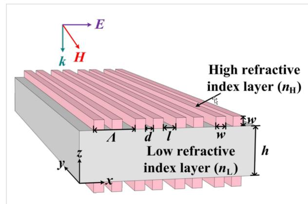
**Figure 1:** Schematic of the double-layer symmetric gratings structure.
