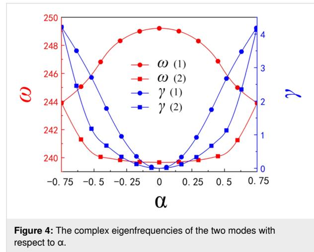
Figure 4: The complex eigenfrequencies of the two modes with respect to  $\alpha$ .
