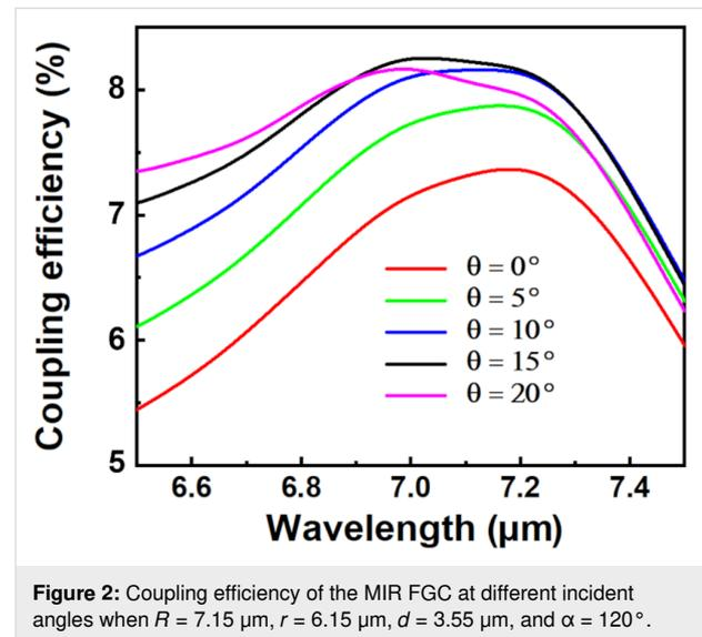
**Figure 2:** Coupling efficiency of the MIR FGC at different incident angles when  $R = 7.15 \mu\text{m}$ ,  $r = 6.15 \mu\text{m}$ ,  $d = 3.55 \mu\text{m}$ , and  $\alpha = 120^\circ$ .
