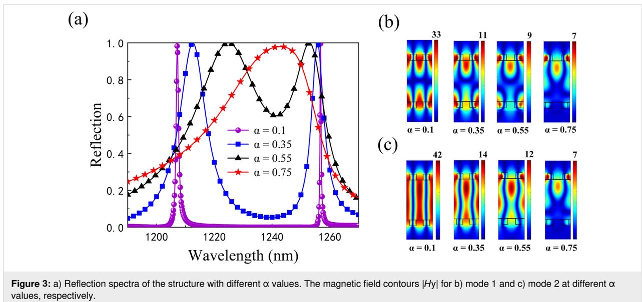
**Figure 3:** a) Reflection spectra of the structure with different  $\alpha$  values. The magnetic field contours  $|H_y|$  for b) mode 1 and c) mode 2 at different  $\alpha$  values, respectively.
