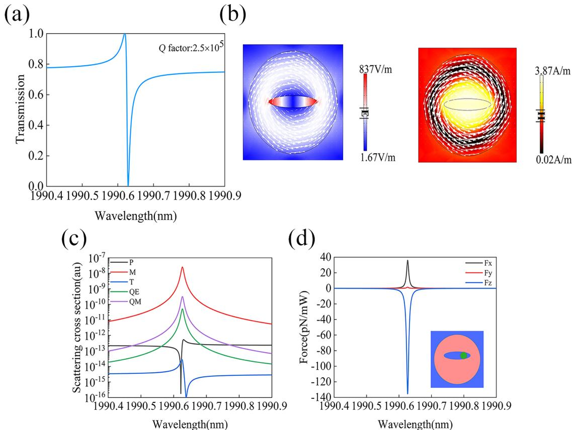
**Figure 4:** (a) Calculated transmission spectrum through the metasurface supporting the quasi-BIC resonance. (b) Electric and magnetic field distributions at the quasi-BIC resonance, where the white arrows represents the displacement current vectors. (c) Contributions from different multipoles to the overall scattering as a function of wavelength. (d) Calculated optical force spectrum on the PS sphere; the inset shows one unit cell of the geometry and the position of the PS.
