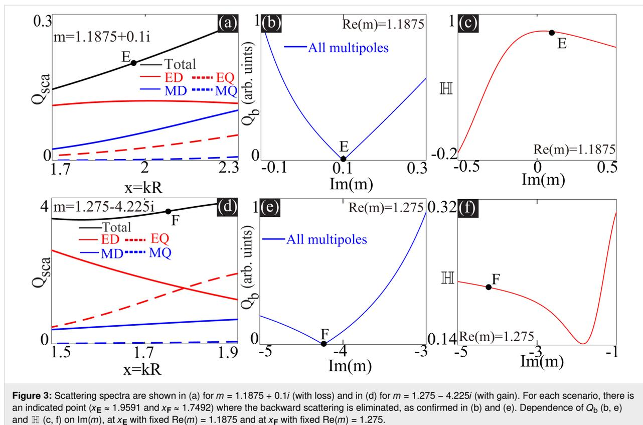
is far from unity at the indicated Kerker scattering points ( $\mathbb{H}_E = 0.857$ ,  $\mathbb{H}_F = 0.2115$ ). In other words, rotation symmetry and helicity conservation lead to zero backward scattering, while rotation symmetry and zero backward scattering does not necessarily imply helicity conservation.
