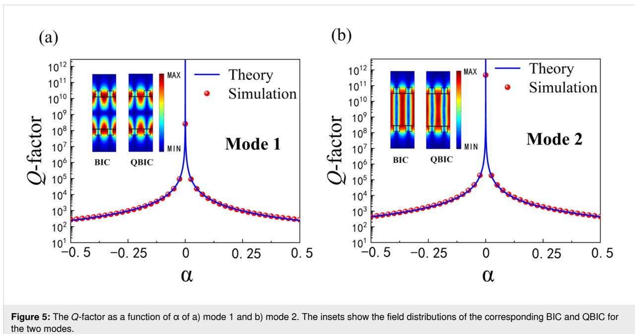
Figure 5: The  $Q$ -factor as a function of  $\alpha$  of a) mode 1 and b) mode 2. The insets show the field distributions of the corresponding BIC and QBIC for the two modes.
