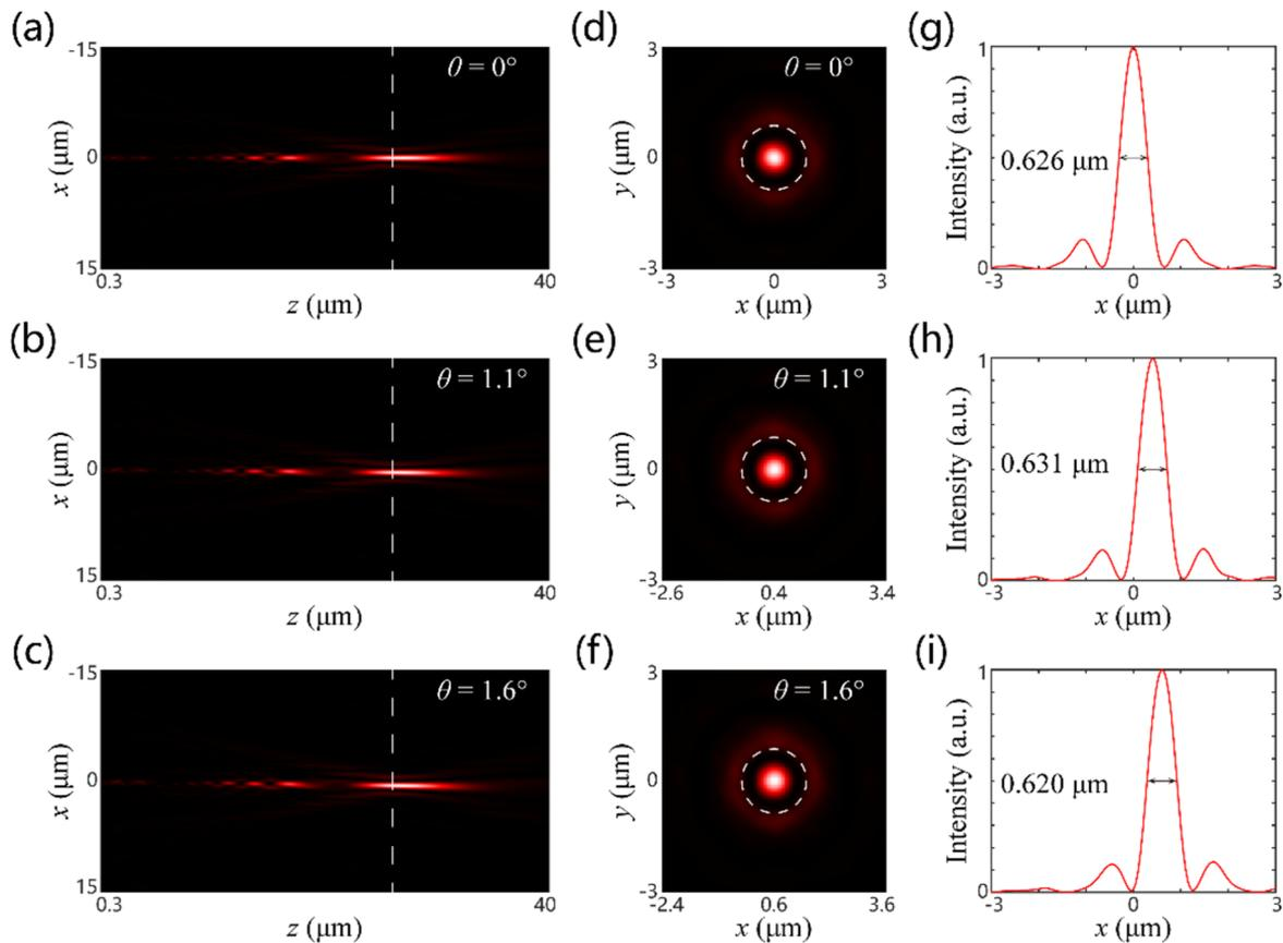
**Figure 4:** Simulated intensity distributions for different incident angles with RCP incidence corresponding to the SSL with short focal length. (a–c) Intensity distributions along the propagating direction. The dashed white lines represent the focal plane of the SSL. (d–f) Intensity distributions in the focal plane. The dashed white circles represent the diffraction-limited focal spot (Airy disk). (g–i) Intensity distributions of the sub-diffraction spot along the  $x$ -direction.
