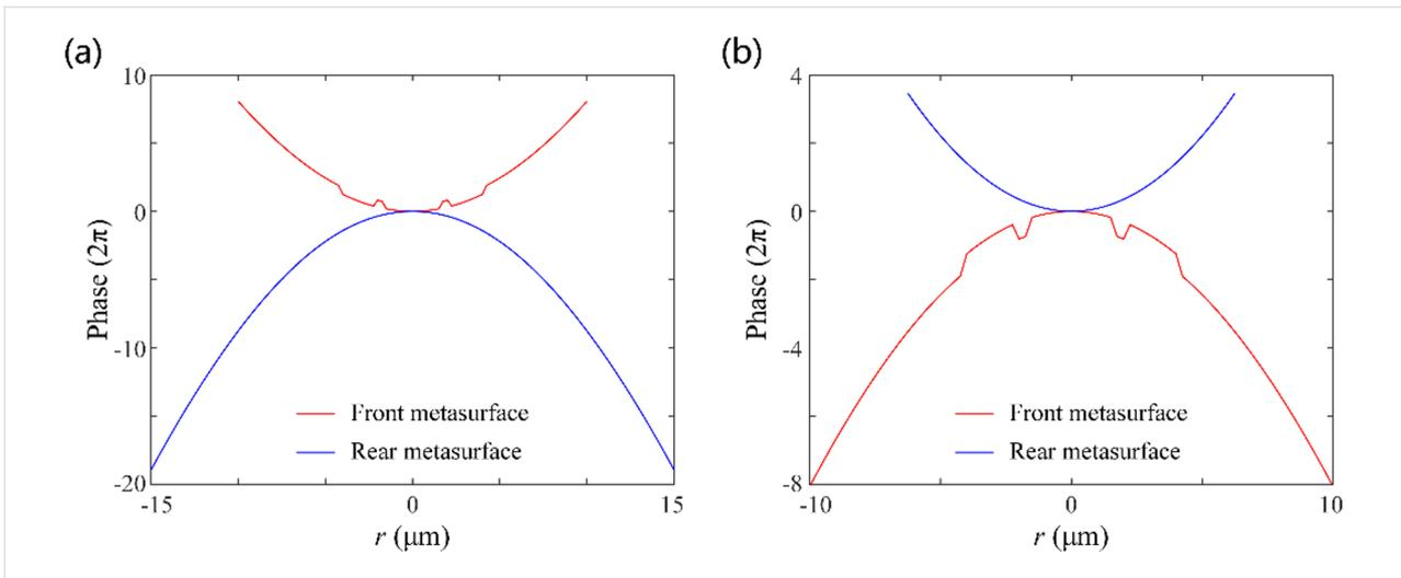
**Figure 2:** Phase profiles of the front and rear metasurfaces for (a) short and (b) long focal lengths.
