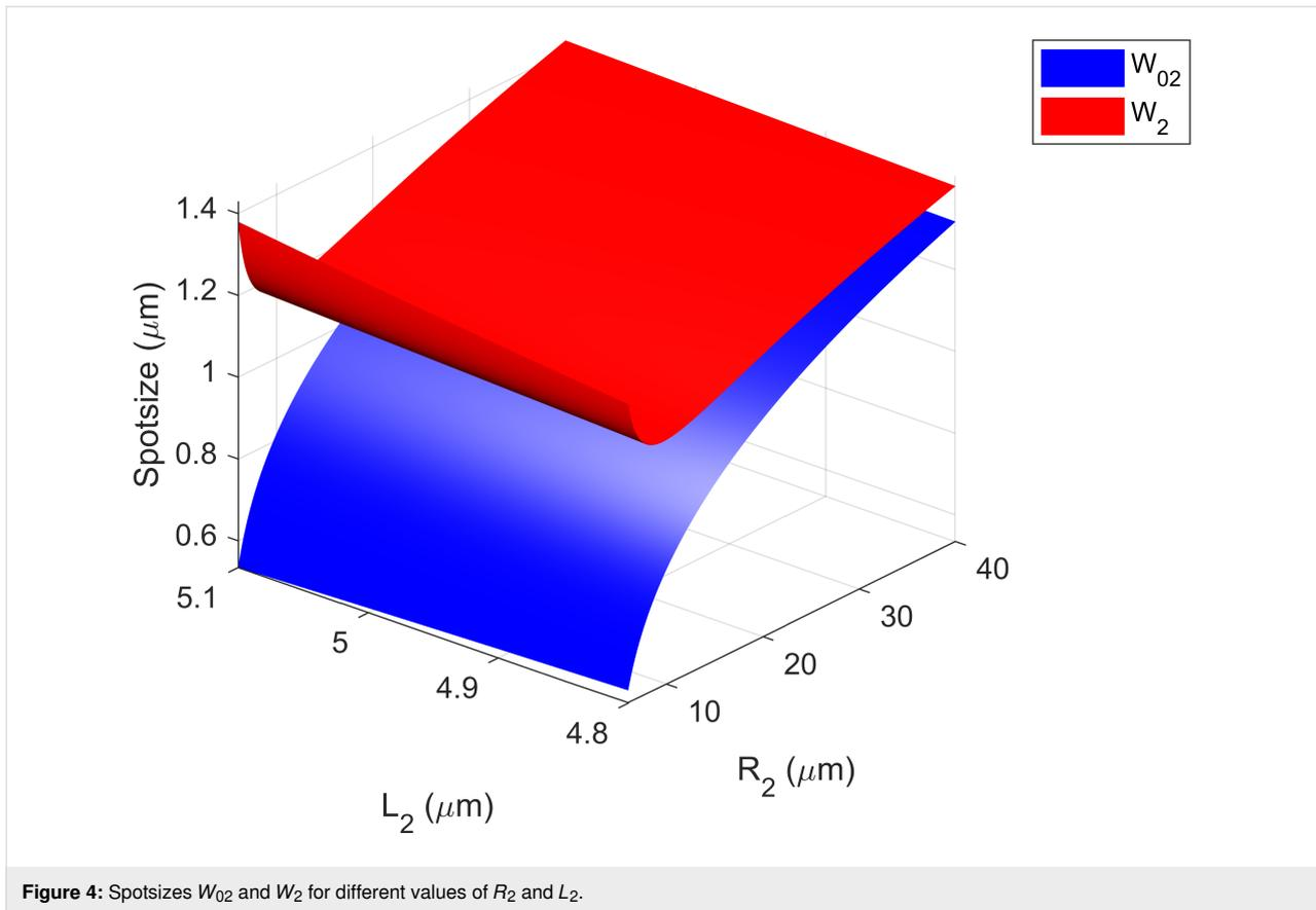
**Figure 4:** Spot sizes  $W_{02}$  and  $W_2$  for different values of  $R_2$  and  $L_2$ .
