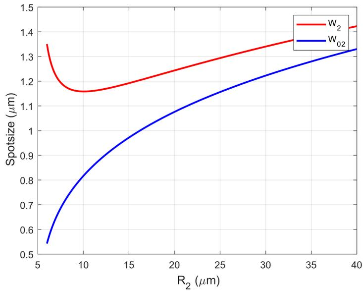
**Figure 5:** Transverse cut of Figure 4 through length  $L_2 = 5.03 \mu\text{m}$  to show dependence of  $R_2$  with spotsizes. As the values of  $R_2$  diminishes, while maintaining a constant  $L_2$ , the functions for  $W_{02}$  (blue) and  $W_2$  (red) start to diverge, arriving at the limit of the paraxial approximation (stability regime).
