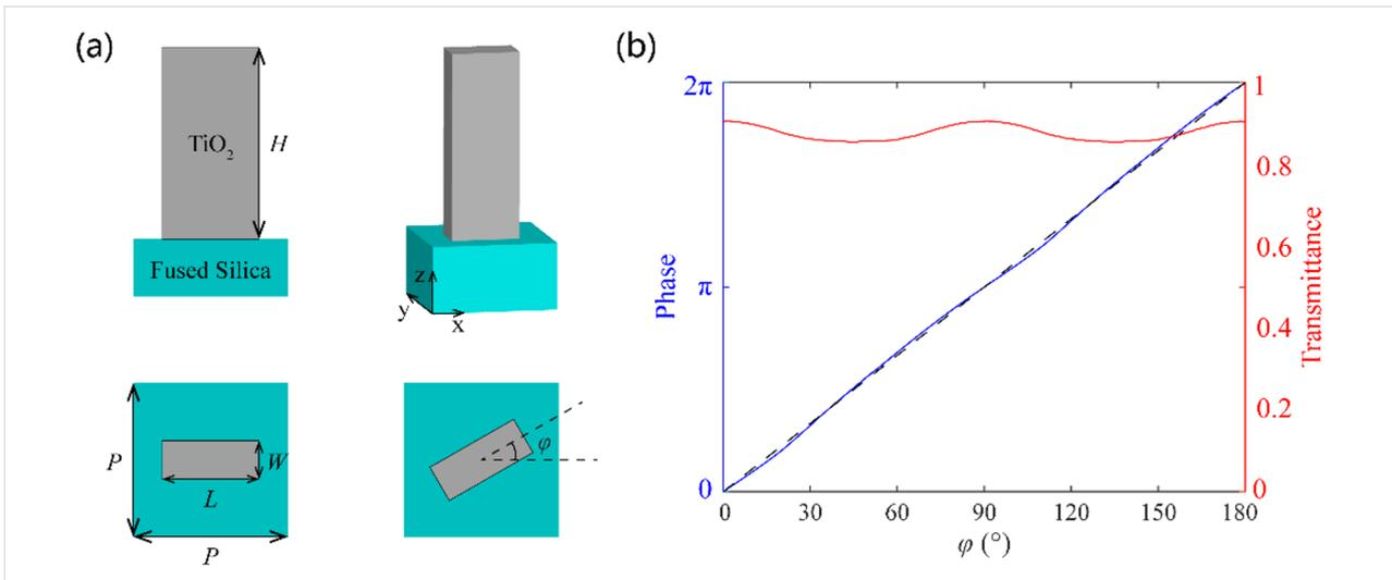
**Figure 3:** (a) Schematic of a TiO<sub>2</sub> rectangular nanopillar. (b) Simulated transmittance and phase modulations of the unit cells with different orientations. The black dashed line represents the theoretical modulated phase.
