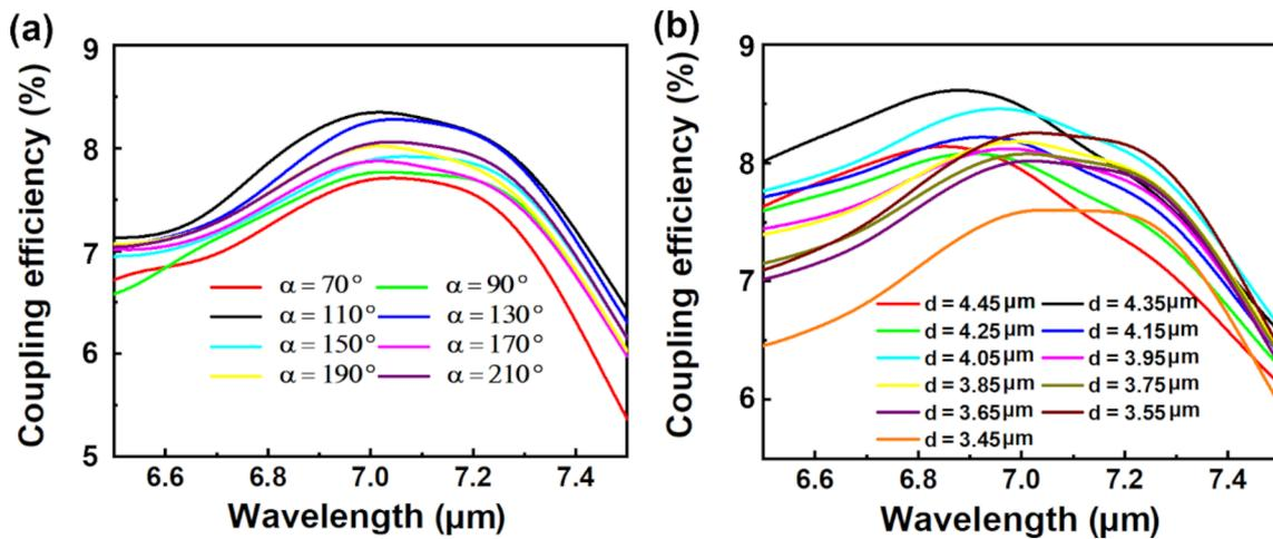
**Figure 4:** Coupling efficiency of the proposed MIR FGC at different (a) opening angle ( $d = 3.55 \mu\text{m}$ ) and (b) location ( $\alpha = 120^\circ$ ) with  $\theta = 15^\circ$ ,  $R = 7.15 \mu\text{m}$ , and  $r = 6.15 \mu\text{m}$ .
