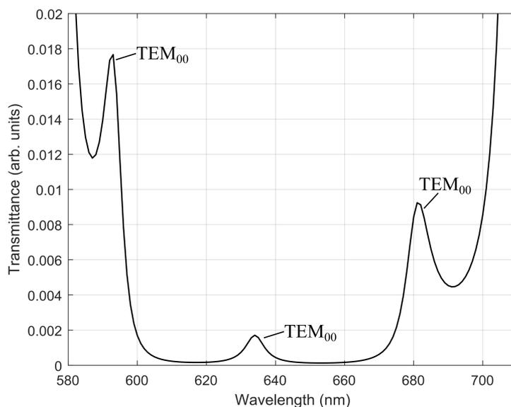
**Figure 7:** Transmittance of plano-concave cavity shows the fundamental TEM modes at 595 nm, 636 nm and 684 nm.
