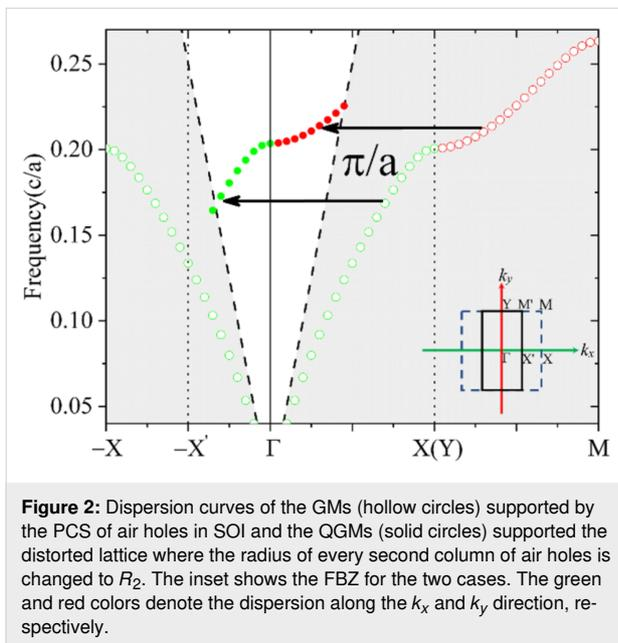
**Figure 2:** Dispersion curves of the GMs (hollow circles) supported by the PCS of air holes in SOI and the QGMs (solid circles) supported the distorted lattice where the radius of every second column of air holes is changed to  $R_2$ . The inset shows the FBZ for the two cases. The green and red colors denote the dispersion along the  $k_x$  and  $k_y$  direction, respectively.
