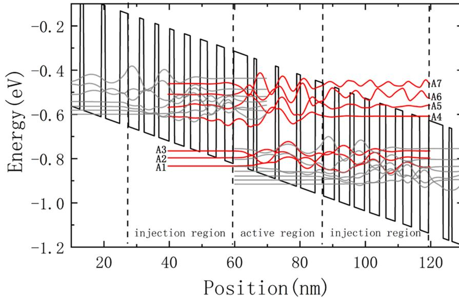
**Figure 2:** Calculated conduction subbands and moduli squared of relevant wave functions with a 53 kV/cm DC bias.
