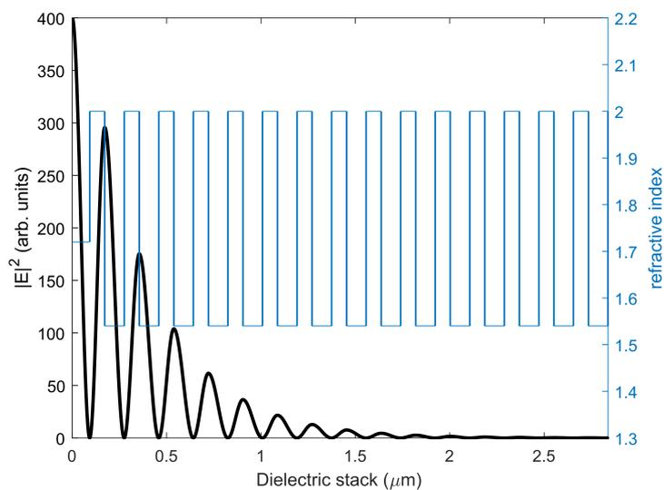
**Figure 6:** Electric field distribution of a hBN + DBR system on a  $L(HL)^{15}$  configuration. Maximum electric field intensity is found at the surface of the hBN layer. Vertical lines (blue) represent the boundaries between each dielectric layer.
