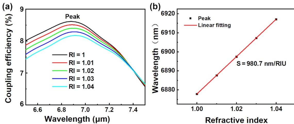
Figure 6: Sensing performance of the proposed MIR FGC.
