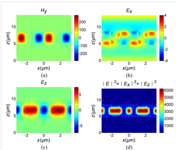
**Figure 3:** Electromagnetic field distributions: (a)  $\text{real}(H_y)$ , (b)  $\text{real}(E_x)$ , (c)  $\text{real}(E_z)$ , and (d)  $|E|^2 = |E_x|^2 + |E_z|^2$ . The regions enclosed by the white dash line are the dielectric grating. A graphene monolayer, which cannot be displayed due to its ultrathin thickness, is attached to the dielectric grating. The origin of the  $z$ -axis is located at a surface  $5 \mu\text{m}$  below the dielectric grating.
