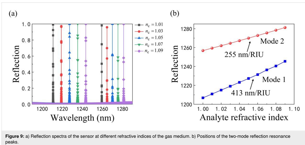
**Figure 9:** a) Reflection spectra of the sensor at different refractive indices of the gas medium. b) Positions of the two-mode reflection resonance peaks.
