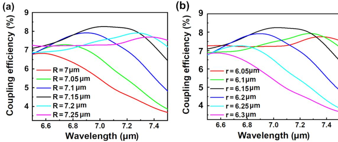
**Figure 3:** Coupling efficiency of the proposed MIR FGC at different (a) outer radii ( $r = 6.15 \mu\text{m}$ ) and (b) inner radii ( $R = 7.15 \mu\text{m}$ ) with  $\theta = 15^\circ$ ,  $d = 3.55 \mu\text{m}$ , and  $\alpha = 120^\circ$ .
