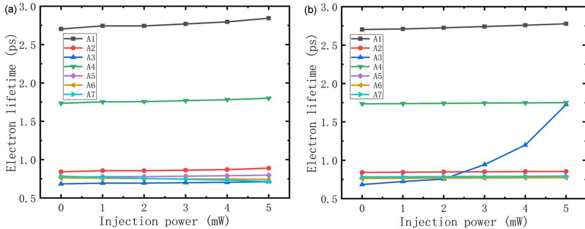
**Figure 4:** Electron lifetime of each subband using optical injection at wavelengths of 1550 nm (a) and 820 nm (b).
