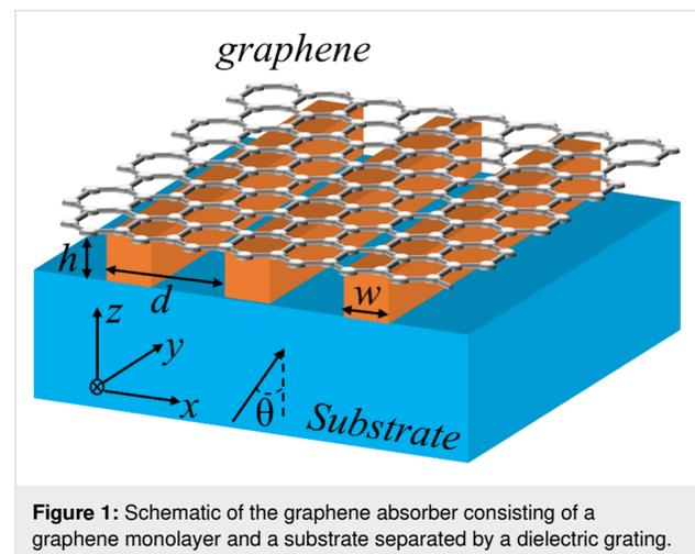
**Figure 1:** Schematic of the graphene absorber consisting of a graphene monolayer and a substrate separated by a dielectric grating.
